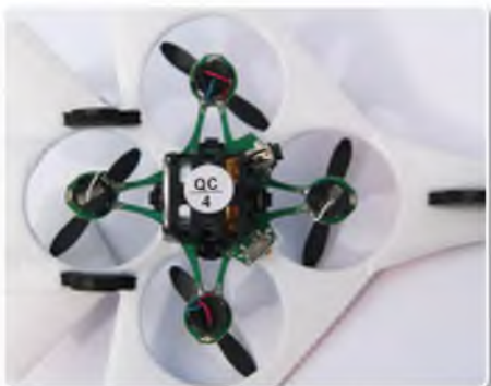
The actual quad element has an integral 1S 120 LiPo charged via a USB lead
