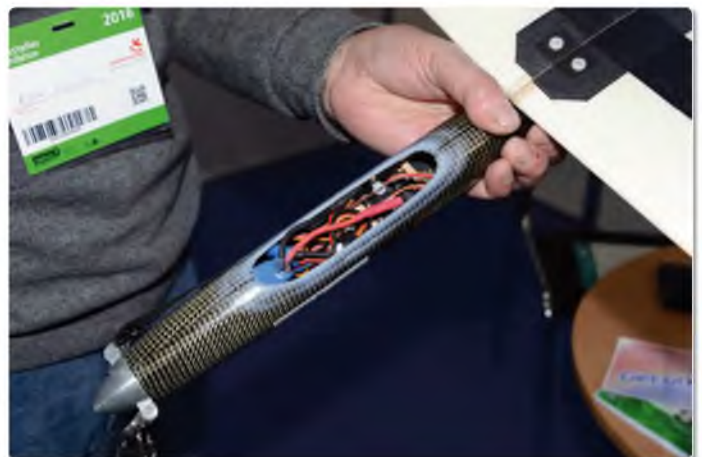
Adding the radio and LiPo brings the ready to fly weight to around 780 g
