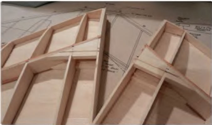
Top 1/4" balsa gussets fitted and sanded to rib profile with vertical slots cut to suit 1/16" ply wing joiner
