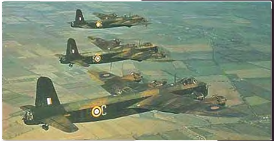
Stirlings in formation. It is surprising how often photos show the tailwheels left down for serviceability reasons; they've even removed the doors as well!
