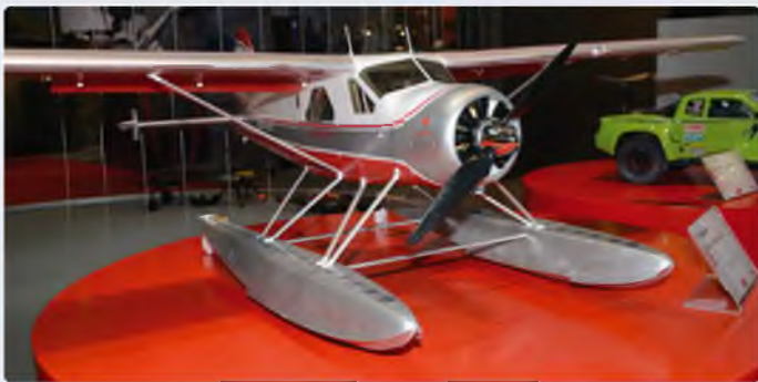
Pride of place at the front of the Hobbico stand went to this neat moulded 'AeroCell' foam replica of a DHC-2 Beaver. With a wingspan of just over 1.5 metres the 3S LiPo powered Beaver comes in an authentic 'Lady Esther' red and silver trim, and is supplied with 'tundra' wheels and a matching float set
