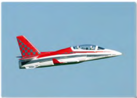
By not flying flat out for the entire flight it is possible to get five minutes from the 3S 850 mAh LiPo
