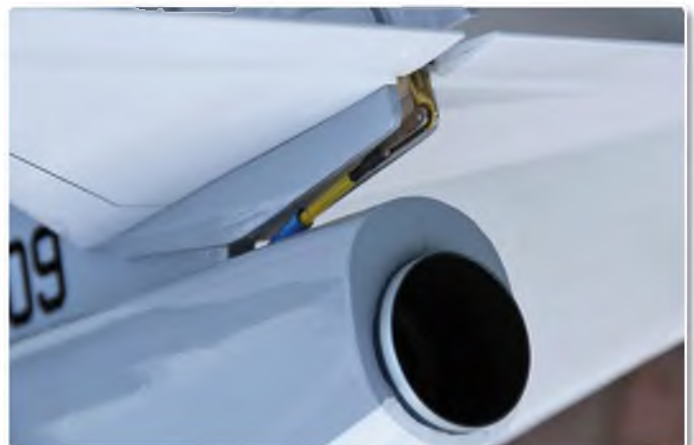
Elevator horn connection with the shroud removed for clarity
