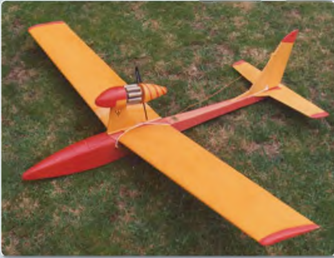
I built this Chris Foss Middle Phase II slope soarer to get some flying practice. I then modified it for electric power. Not a great success, being underpowered and overweight with the NiCad batteries of the time. With all that weight high up lateral stability was marginal, needing a blip of right rudder to start it turning, followed by a blip of left rudder to straighten it up. The model was eventually passed on without the electric modification
