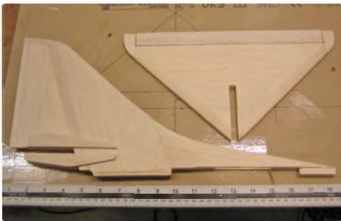
Fin and tailplane sanded to section. Cover prior to fitting. Fin doublers should be covered before fitting to fin also, aiding the covering process
