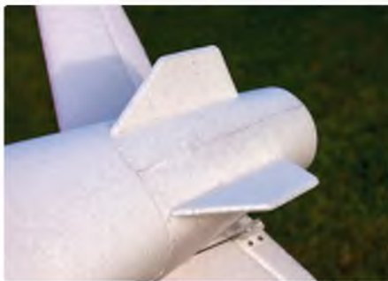
Left: The ventral fins locate into slots. Right: After the first flight Brian rotated them, raising the leading edges by about 15 degrees but at Century, Mark's model flies well at the original setting. They are cosmetic anyway, so it may be a good idea to leave them off for the first flight to set up the model. You can then tack them in place to judge the effect on flight characteristics for yourself
