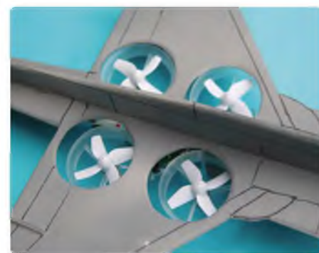
Sadly even with 4-blade impellers there was not enough power to fly with the Harrier body in place
