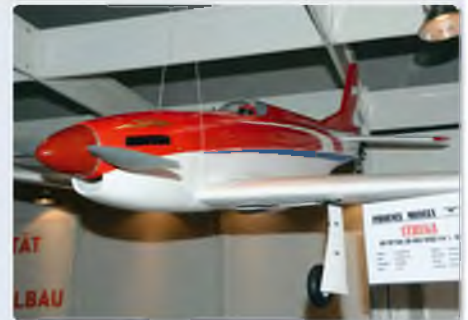
Staying with the racing theme, Phoenix also displayed this Strega. At 1:6.5 scale, the modified Mustang has a wingspan of 1750 mm and suits 20-30 cc engines or equivalent electric power
