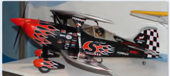
E-flite's P2 Prometheus looks stunning even when sitting still. Designed by Mike McConville the 1219 mm span model is based on the full size aerobatic biplane and uses Carbon-Z to give a high power to weight ratio to the large foam airframe without losing rigidity. Available as PNP or BNF, Prometheus requires a 6S-4400 LiPo
