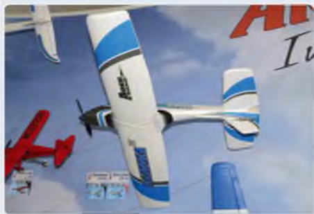
New style Gamma V2 is equipped with a brushed motor set for a 2S LiPo and sports a new style cowl and trim, as well as a toughened undercarriage. 'Nav' lights are built into the wingtips and under the fuselage
