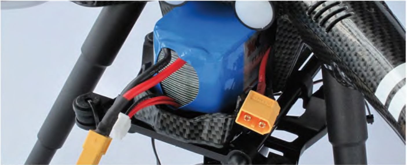
Battery access is through a flap at the front. There is plenty of room to tuck the wiring and balance lead inside
