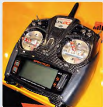
'BLING!', as our new columnist Chris Golds would say... Shiny new DX20 has all the bells and whistles you would expect from a state-of-the-art 20-channel Tx, including machined aluminium quad-bearing gimbals, a carbon fibre front case and a large 4000 mAh battery
