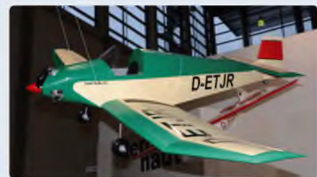
One of our favourite new models was the aero-naut Jodel D.9, a 1:3 scale model for 20 cc plus engines or 8S electric power. 2.4 m wingspan for four function R/C
