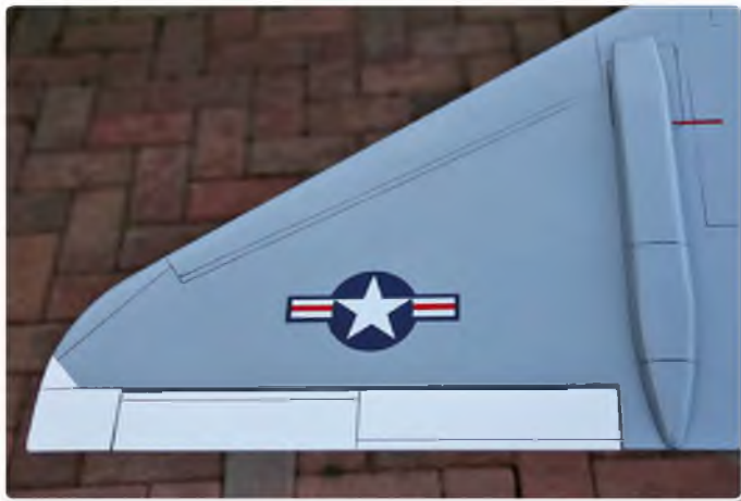
Underside of wing panel shows the extent and fit of the aileron and the wheel bay pontoon. This acts as a skid - ideal for those smooth landings!
