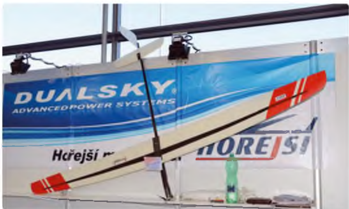
Geronimo electric glider for the F5J-100 competition class from Horejší Model. Wingspan is 2540 mm and the sleek glider weighs just over 500 g without R/C or LiPo www.horejsi.cz/
