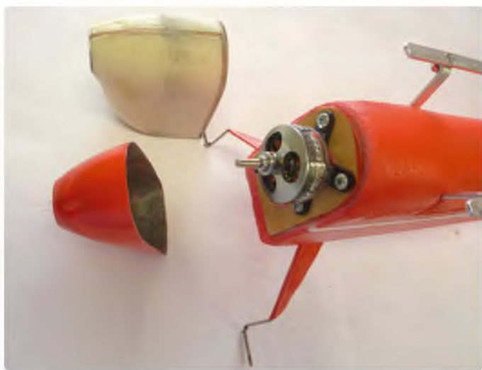
Fuselage front end showing moulded cowling and plug
