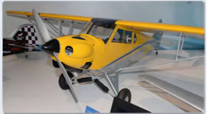
Hangar 9 Carbon Cub 15 cc is finished in UltraCote and features plug-in wings and a shock-absorbing undercarriage for flying off less than perfect strips. Or fly off water using optional floats. Evolution 15 cc is the perfect engine for this 2.28 m span scale beauty
