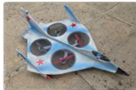
The 3 mm square mesh covering the props was a nice idea but didn't work
