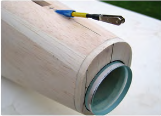
Rear fuselage fitted with end cap F9 and sanded to section. Note the amount of rounding necessary – triangular stock is evident and acts as good guide when shaping. Moisturiser cream bottle top for tailpipe, diameter as per plan
