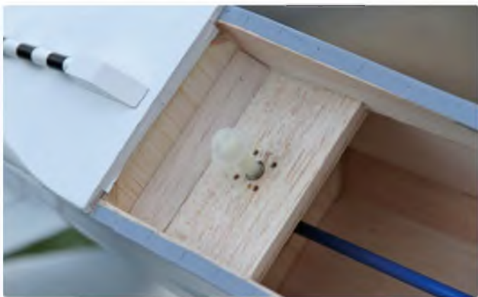
F6 detail showing 1/8" ply and 1/8" balsa laminate. The captive nut is mounted from the rear side for the 6 mm nylon wing retaining bolt
