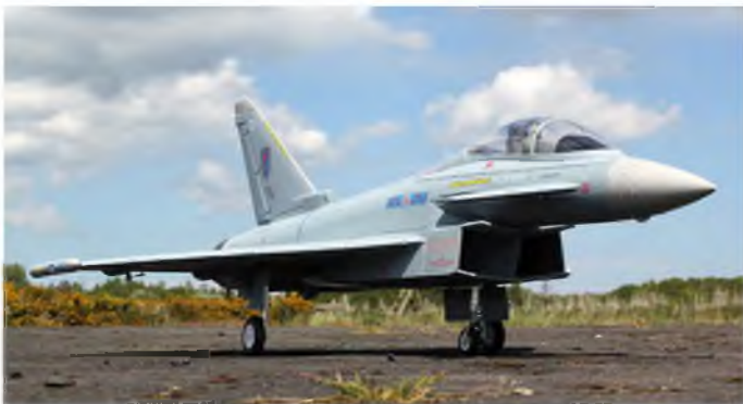
Low shot of the Eurofighter. Twin air intakes allow plenty of air into the 12-blade fan unit
