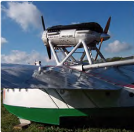
Close up of the nacelle and engines. The original plane had three bladed, metal propellers and black painting on the bottom hulls. A lot of literature confirms it was a green colour, but the Air Force Instruction Manual describes a special black painting based on bitumen, so Erick decided to make the correction
