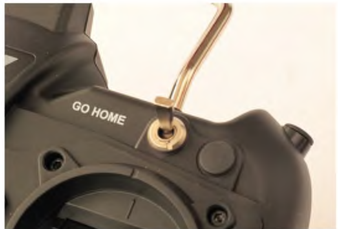
Provided you have a good GPS signal the Go Home switch can be used to bring the drone back to the take-off point for an automatic landing
