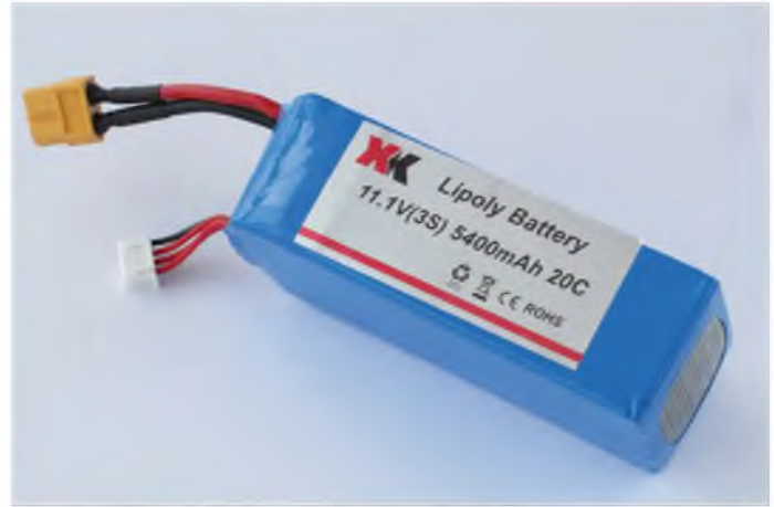
The 3S 5400 mAh has conventional modelling type power and balance connectors. It proved very economical in use, giving ample flight times
