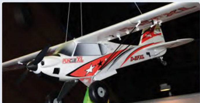
FUNCUB XL is a chunky 1.7 metre span rendition of the famous lightplane. Additional fun elements include flaps and options such as an aerotow release, a payload dropping bay, and navigation and landing lights
