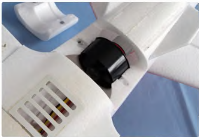
The fan unit can be accessed via an under-fuselage hatch, held with more magnets
