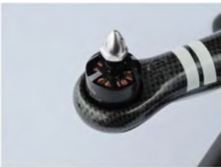
The propellers are secured using domed prop nuts
