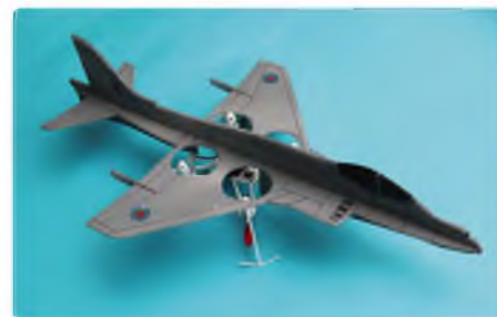
The body from the Inductrix fitted, but the holes were well out of line
