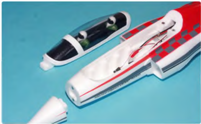
The nose is held on with magnets and is designed to pop off in a bad landing. Likewise the neat canopy hatch is retained using magnets too
