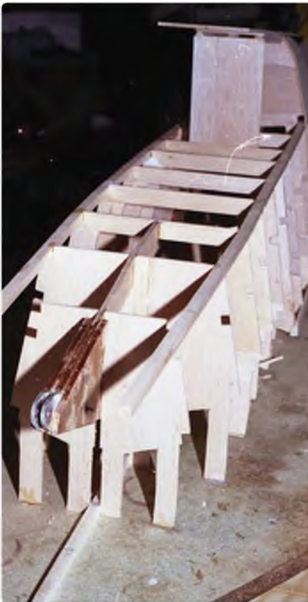
Rear part of a float, showing the metal eye used to connect it to the boom
