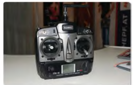
This Jeti DS-6 transmitter was developed as an inexpensive R/C transmitter with the features of a Jeti Duplex EX radio at a more affordable price, so beginners can start with a Jeti system and avoid a costly transition from another brand. It offers six channels and 10 model memories, plus telemetry, which can be read via an attachable Jetibox. Paired receivers and sensors can be programmed via the Jetibox http://www.hepf.at/jeti-duplex-ex-computersender-ds-6/
