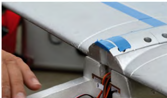
See the gap between the two patches of tape over the wing centre section? That's the calculated centre of gravity. The manufacturer's point was over 34 mm further back, way too much for safety!
