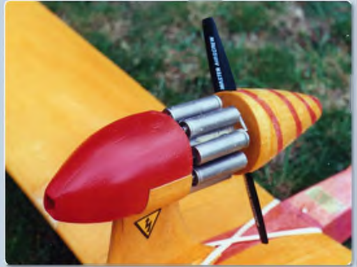
I built this Chris Foss Middle Phase II slope soarer to get some flying practice. I then modified it for electric power. Not a great success, being underpowered and overweight with the NiCad batteries of the time. With all that weight high up lateral stability was marginal, needing a blip of right rudder to start it turning, followed by a blip of left rudder to straighten it up. The model was eventually passed on without the electric modification
