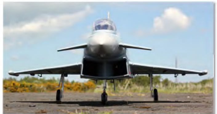
Head on the Eurofighter looks aggressive. You can see the metal sprung oleos clearly. Rubber tyres are used
