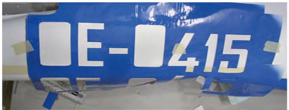
Using the cut out to line up the decals
