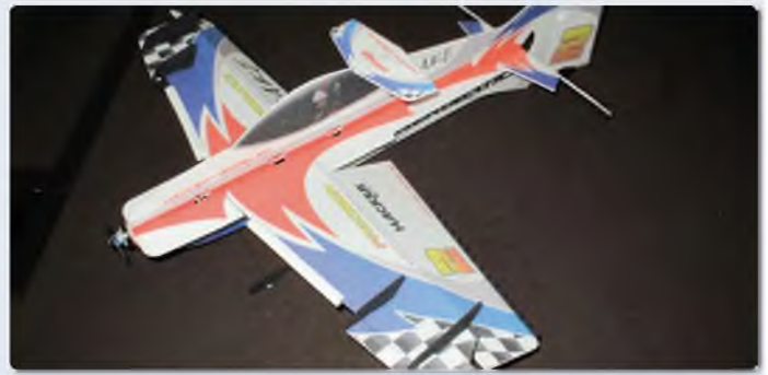
Shake is a 'shock style' indoor ARF for precision F3P aerobatics. Spanning 840 mm it is CNC cut from 4 mm EPP and is claimed to be almost unbreakable – a perfect practice plane! Available in three colour schemes
