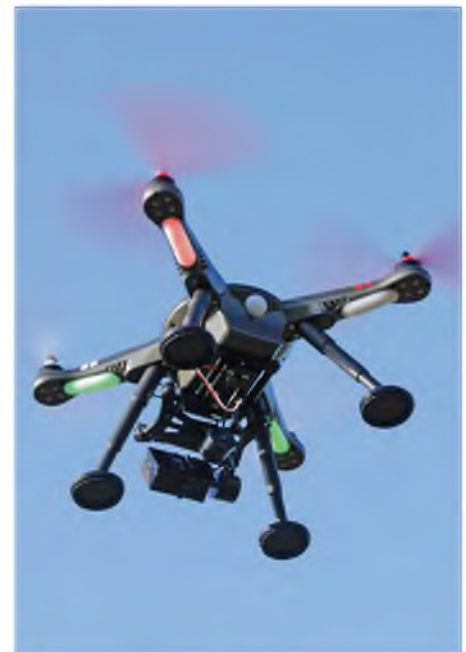
Under-boom lights, front headlights, coloured props and a flashing rear indicator all help with orientation of this all-black quadcopter
