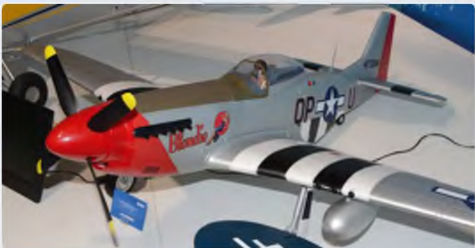
'Blondie' from E-flite is their latest 1.2 m span BNF P-51D Mustang and comes fitted with AS3X stabilisation. Features include retracts, flaps and removable drop tanks. Requires a 3S-2200 LiPo
