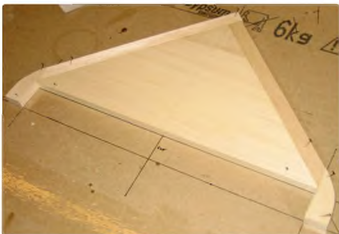
Tailplane LE from medium 3/8"x 1/2" strip. Note the grain direction on other parts. The production plan was altered slightly to include wider elevator chord so production assembly will vary slightly at the tip
