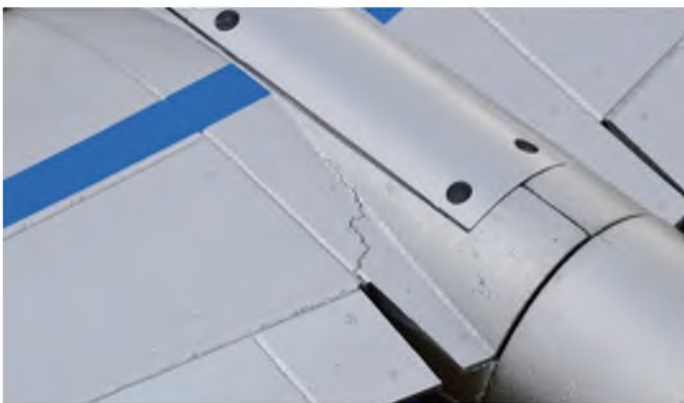
Oops! The result of our Kev's ruffy-tufty landing in the weeds. Non-critical, a dab of cyano fixed it in seconds
