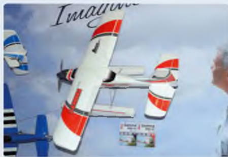
Gamma Pro V2 has similar styling enhancements but uses a brushless 3S set up and features ailerons for more advanced aerobatics. Seen here with the optional float set that can also be fitted to the V2. Both models are 775 mm wingspan
