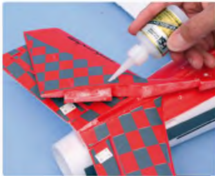
Tail parts are also cyanoed in place
