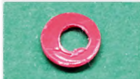
Flexible plastic retainers are easy to make. Shown here is one for Micki's Cub, used to keep the strut machine screws from being lost
