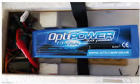
Large battery bay allows for a 5000 mAh 6S (22.2 V) battery to be fitted with ease
