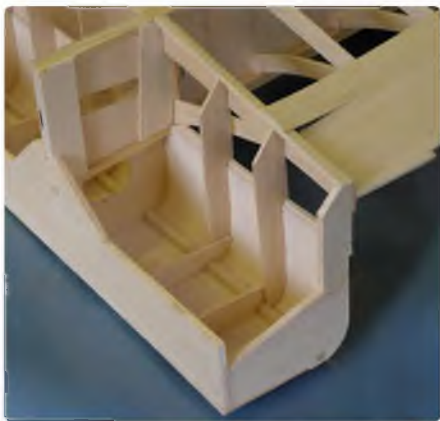
Half of the fuselage underside being built onto the wing root
