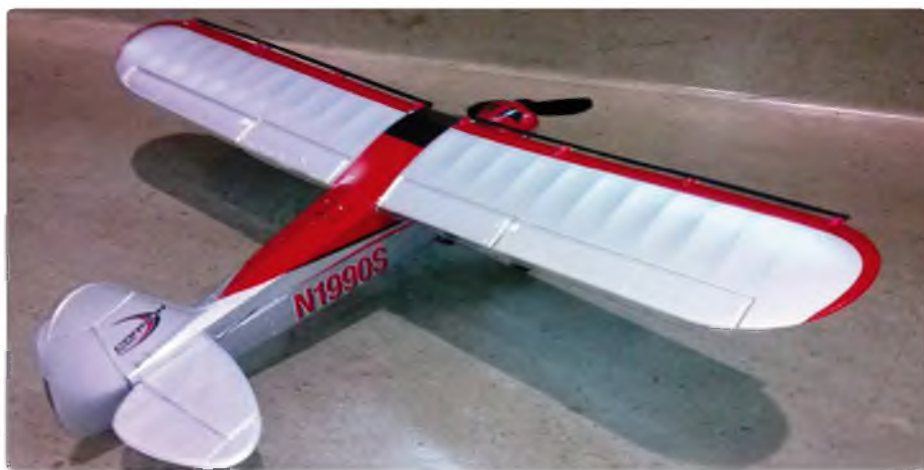
From Arnaldo Correia, a flapped and slatted Cub
