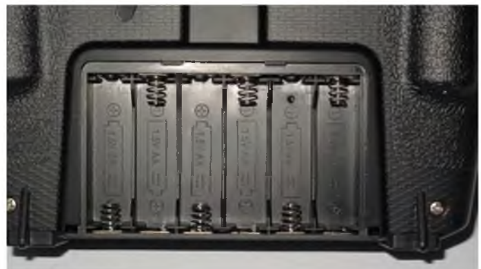
The Tx battery bay takes six AA size cells
