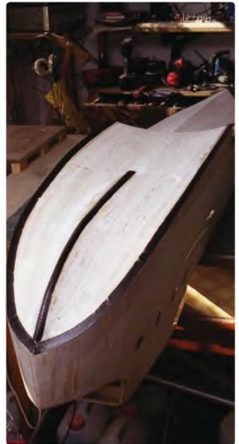
Float edges were strengthened with carbon strips
