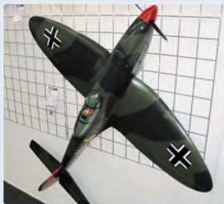
With those wings it has got to be a Heinkel! The He112B competed to be the Luftwaffe's new fighter in the 1930s but lost out to the Bf 109. Provision is made for electric retracts (not included) in the 1550 mm span wing, but sprung oleo legs are supplied. Suits a 15 cc petrol engine, a .91 four-stroke or a 1200 – 2200W 650 KV brushless motor and 6S 4000 – 5000 mAh LiPo
