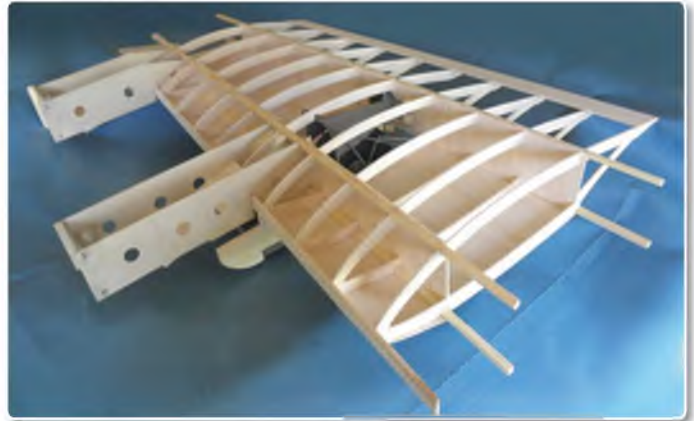
Top surface formers added, then top spars and webbing. Front spar next then engine bearers
