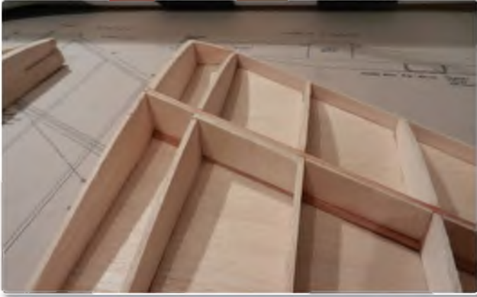
1/16" shear webbing is added between the top and bottom spars; additional 1/8" webbing is added to the rear of the initial 1/16" webbing between ribs 2 and 3 to aid wing joiner assembly
