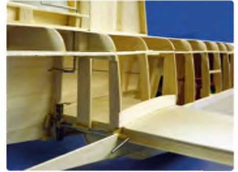
The fin and tailplane operating systems in place
