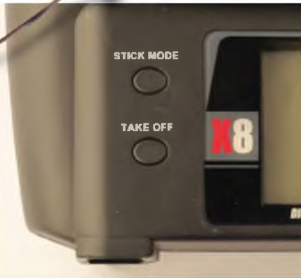
Buttons on the other side of the screen change the stick mode and initiate 'one-key' take-offs and landings
