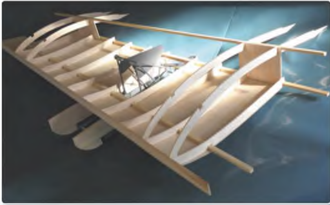
How the wing starts. Lay down sheet, add lower spars and give sheet shape by adding underside formers
