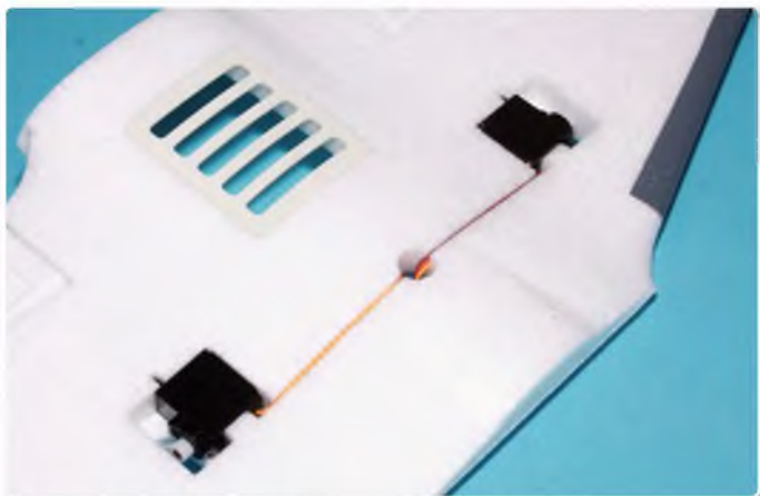
Close up on the factory fitted wing servos
