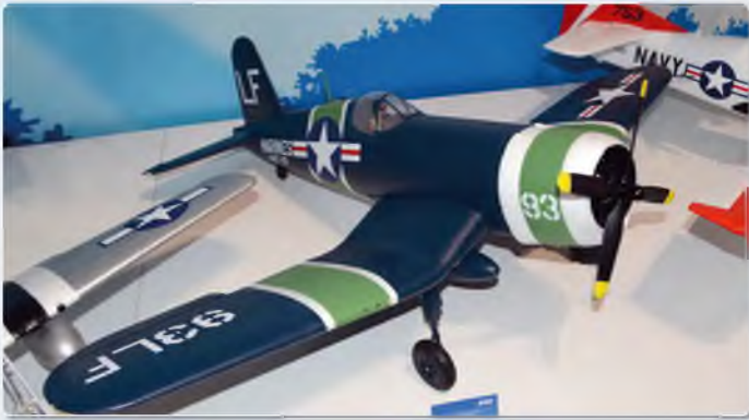
At the rear of Horizon Hobby's maze like stand we found a selection of new aircraft. Here is the E-flite F-4U-4 fitted with flaps and 90 degree rotating electric retracts. 1.2 m span BNF model has a 850 KV motor and suits 3S-2200 packs www.horizonhobby.co.uk/
