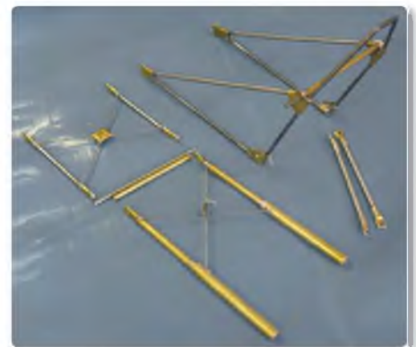
Some of the parts for the first main wheel leg
