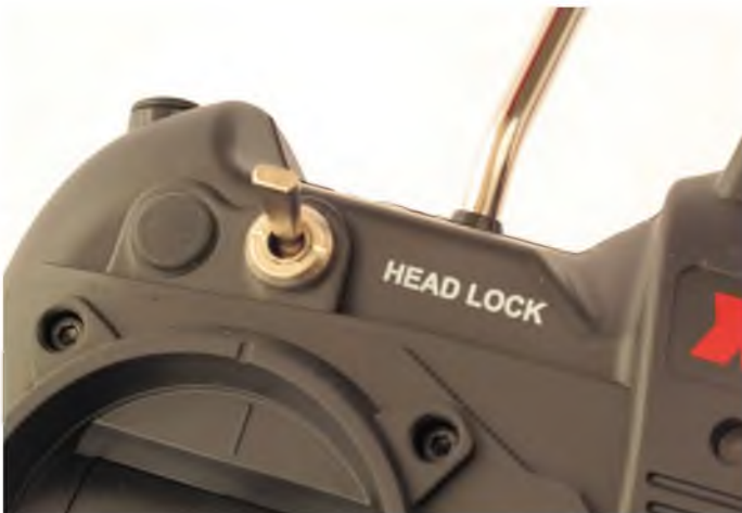
Use the Head Lock switch to keep the camera pointing in the same direction to provide a panning shot whilst you sweep the drone sideways
