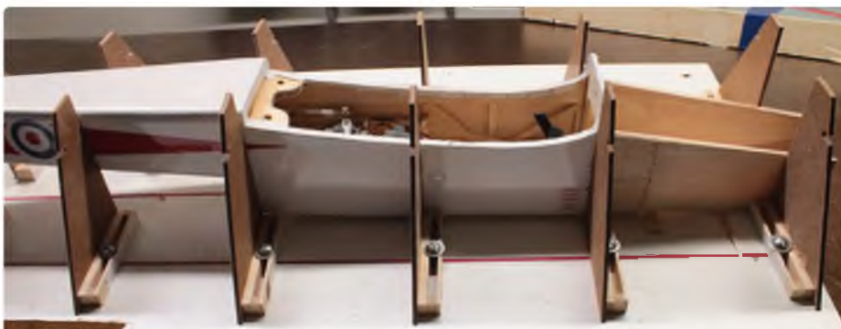
My Shrike needed a nose job (please, don't ask why!), so into the jig she went. Viewing angle only makes the front jig station look backwards (as proven by the location of the slot in the station backbone)
