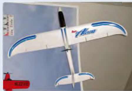
Alara is Firelands' new take on the 'pusher glider with swept up wingtips' style of sport/beginner model. As with all new Ares models it comes ready to 'Pair To Fly' with Hitec Red radios
