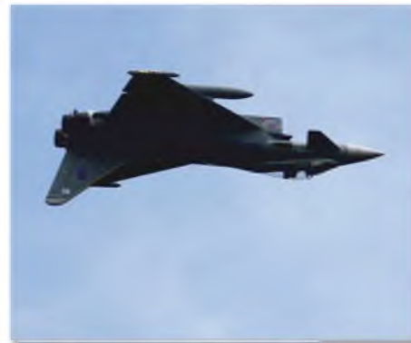
Inverted flight requires the slightest bit of 'down' to fly nice and level
