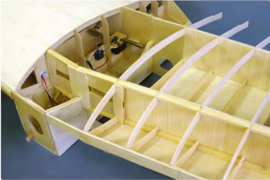
Building the port wing onto the starboard wing
