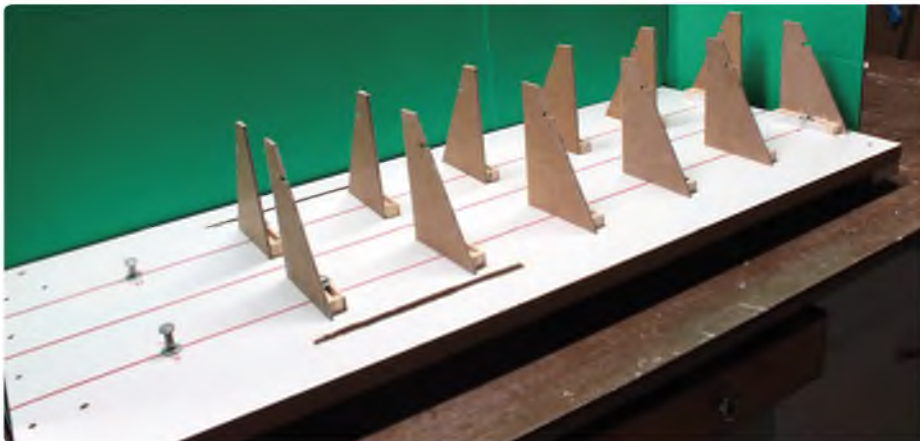
Note the red trim tape guidelines to either side of the centre line. All are protected with a coat of polyurethane varnish. Bolts in station seven holes are hex-head because I ran out of slotted head screws during home repairs and haven't been to the DIY store to replace them
