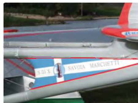
The end of one boom. Note the control cables and the 'Savoia-Marchetti' marking
