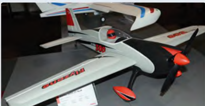
We like the unusual colour scheme on this Flyzone Extra 300 SX but it could be a bit tricky to see on a dull winter's day! The 1055 mm span aerobat comes with factory fitted servos, brushless motor and ESC. Suits 3S-1800 LiPo packs
