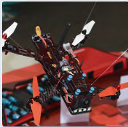
Frenzied flying displays by this 3D Alpha 300Q quadcopter drew appreciative audiences throughout the duration of the Fair. Highly agile machine spans 30 x 30 cm and weighs 460 g
