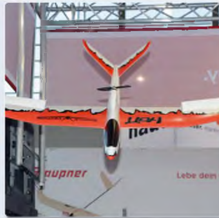
V-Venture is a good-looking V-tail pylon pusher glider. Wingspan is 1350 mm
