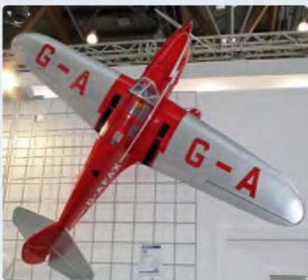
The B.A. Eagle dates from 1934 and became the Eagle II in 1935. This is the basis for the Black Horse version in its red and silver livery. The 1790 mm wing is equipped with flaps and this attractive monoplane can either be powered by a .61 glow engine or a 1200 – 2200W 650 KV brushless motor and a 6S 4000 – 5000 mAh LiPo
