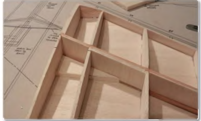
Lower 1/4" balsa gusset fitted to wing panel
