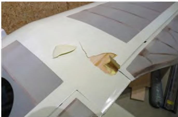
Damage to the Minimoa's starboard wing
