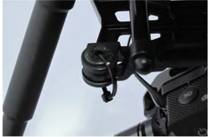
The dual axis gimbal is soft mounted and restrained with tie-wraps for added security
