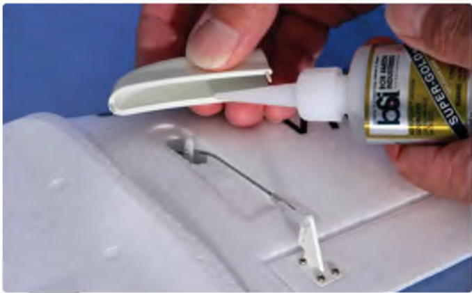
The aileron pushrods are above the wing so they cannot catch in the grass. Neat covers are cyanoed over them to fair everything in
