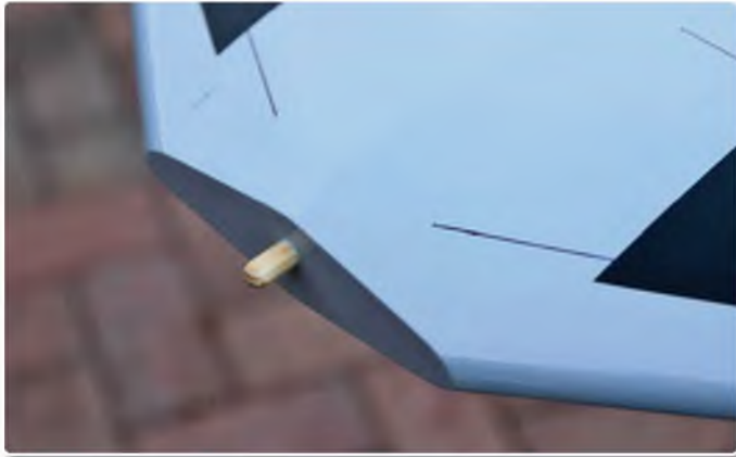
LE wing dowel and ply lined front face. The shape requires the chamfering of the fuselage wing root doublers to accommodate the wing fully
