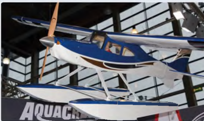
Avistar is a 30 cc class high wing trainer/sports model that can be flown from land or off water using the optional float set. Choose between a 30-35 cc engine for power, or fit an 8-10 cell LiPo brushless motor set. The 2.3 m span wing has flaps and ailerons
