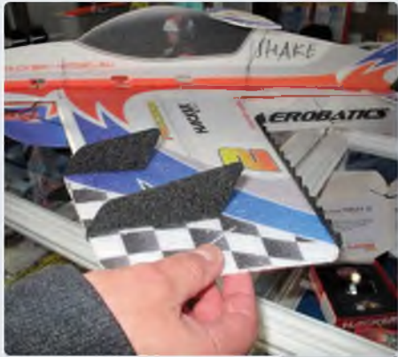
View of the wing fences and trailing edge dive brakes fitted to the Shake
