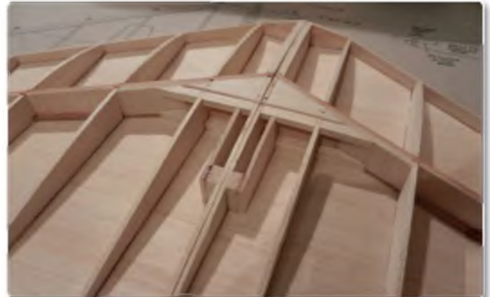
Wing joiner dry fitted. Wing is built with 14 mm dihedral at Rib 8 at each panel tip. The servo box is built up prior to the removal of the central Rib 1 section
