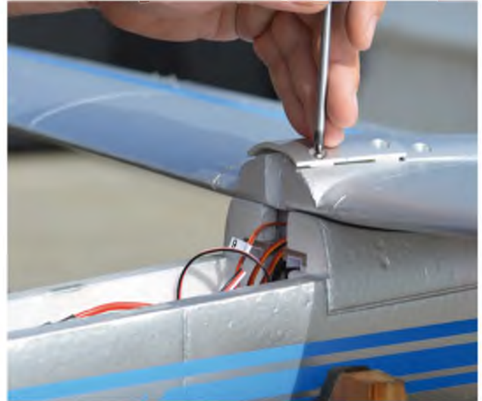
Wing mounting system is a peg at the trailing edge and this four-screwed shaped plastic clamp plate at the front. A change from 'normal', but it works
