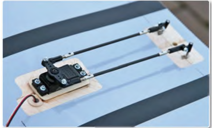
Wing servo arrangement. Standard size servos were used throughout, although two mini servos could easily be fitted to enable flaperons
