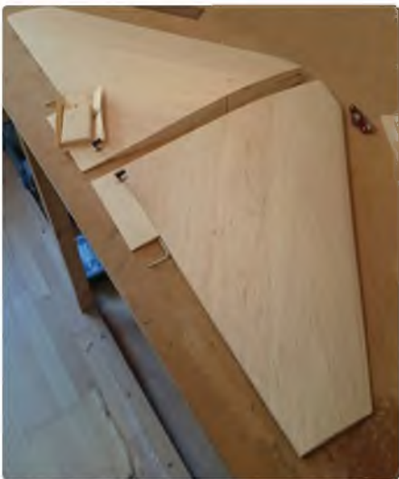
TWO degrees of washout is built into each panel at the tip by chocking the TE whilst the top skins are added. Note the fixed section of TE secures the aileron torque rods. Keep the torque rods less than 20 mm high to clear the wing bolt captive nut in former F6
