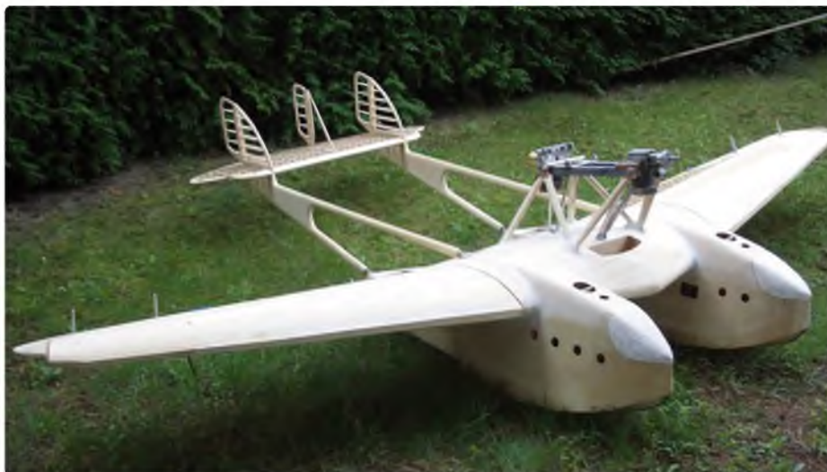
First assembly of the model. At 3.5 m span it is a large model to be made from balsa using traditional construction
