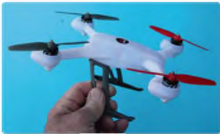
The Blade 200 QX makes an ideal basis for a quad jet with plenty of surplus lifting capacity
