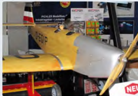
Available with a matching sound system, this Klemm L25 spans 2200 mm and suits 3500 – 4500 mAh 3S LiPo packs www.pichler.de/extronwp/
