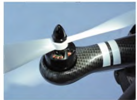
Clockwise rotating motors are marked using black prop nuts. Note how the prop and boom arrows are reversed in this picture
