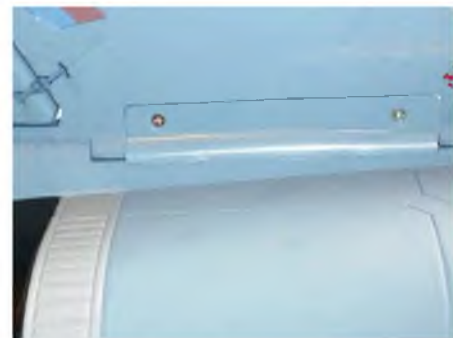
The tail section is also screwed into position. Note the hinges used in the rudder control surface
