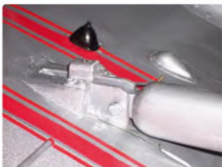
The boom connection with the wing
