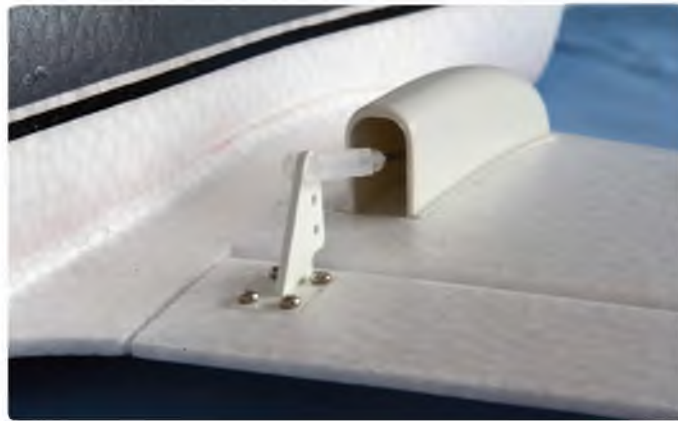
The aileron pushrods are above the wing so they cannot catch in the grass. Neat covers are cyanoed over them to fair everything in
