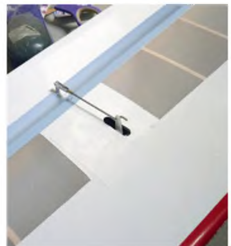
A patch of vinyl with a slot cut into it makes an excellent servo hatch cover
