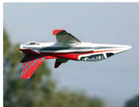
A fair amount of down elevator was needed to maintain inverted flight
