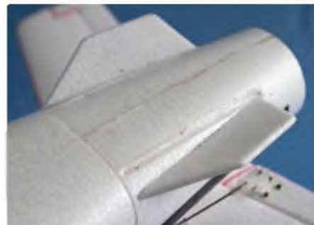
Left: The ventral fins locate into slots. Right: After the first flight Brian rotated them, raising the leading edges by about 15 degrees but at Century, Mark's model flies well at the original setting. They are cosmetic anyway, so it may be a good idea to leave them off for the first flight to set up the model. You can then tack them in place to judge the effect on flight characteristics for yourself
