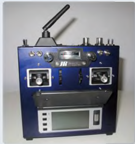
Behind the retro styling the Colt and Mercury systems benefit from JR's thoroughly modern 2.4 GHz DMSS protocol, with an LCD screen and menu scroll bar hidden beneath the flip up panel beneath the stick units
