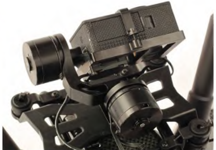
The two brushless gimbal motors provide a smooth and level camera platform
