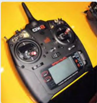
Spektrum's popular DX8 transmitter returns in G2 (second generation) format and now comes with a whopping 250 model memory and multicopter programming, as well as the more traditional aero, heli and glider set-ups. Also has voice alerts and wireless trainer functions
