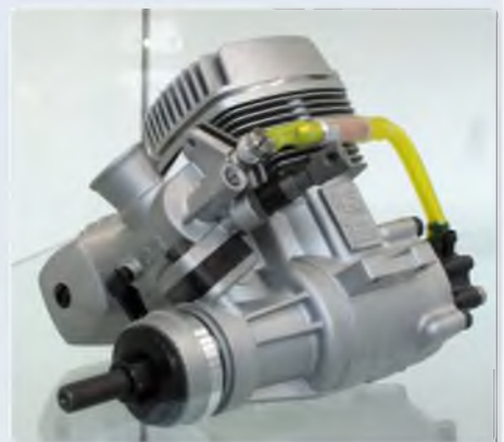
This OS GGT-10 uses the latest model engine technology. It is a petrol engine that uses a special G5 glowplug and runs on a 33:1 ratio petrol/oil mix via a pumped fuelling system and a specially designed carburetor. The GGT-10 is designed to be used in place of a .40-.55 engine and fits in the same mounting space as an OS 46AX and 55AX
