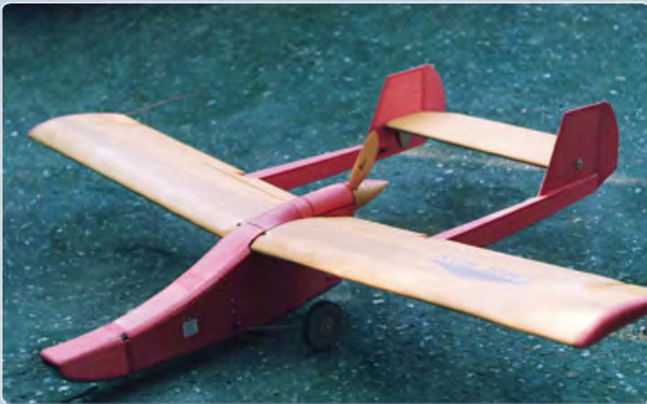
The pusher was repaired and rebuilt with twin booms. The canard was replaced by an all-moving-tailplane, with twin fins and rudders. I dispensed with the speed controller as I needed all the power I could get. Instead I used a servo operating a micro switch with a diode/resistor/capacitor suppressor across the contacts to stop them being destroyed by the arc when they opened. I am about to intrepidly launch it on its first flight. It was flown by a friend of mine who was much more practiced at flying than I was. The model flew very well until a glitch in the second - hand radio equipment I was using put all the servos hard over one way
