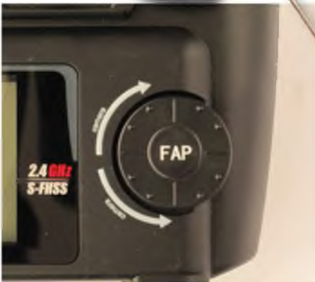
The FAP dial can be used to tilt the camera up or down. And when pressed it initiates the Fly Around Point function
