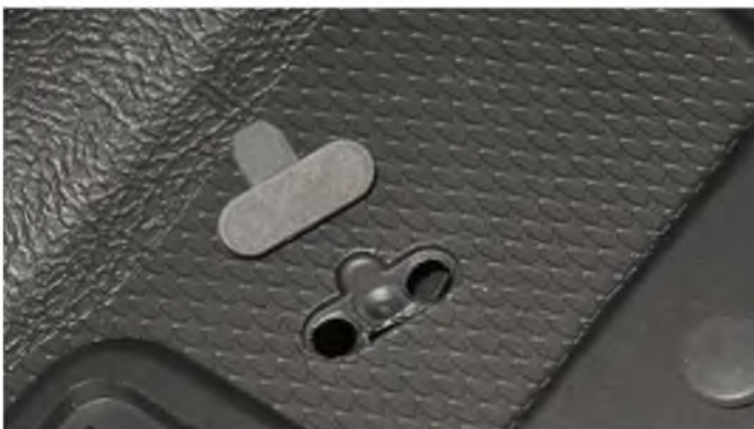
Rubber covers presumably allow access to stick tension screws (there's no mention in the instructions), although we were happy fly the X-380C as supplied
