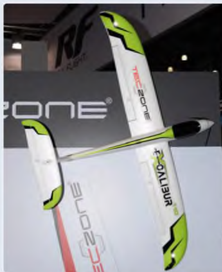
Left: This neat Teczone E-Xcalibur 110 has a span of just over one metre and suits 1200 mAh 3S LiPo packs. Servos are installed but it requires a four-channel R/C system
