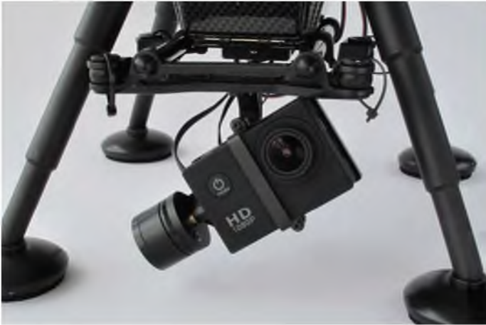
The camera sits at an angle when at rest but soon straightens up when power is applied to the drone
