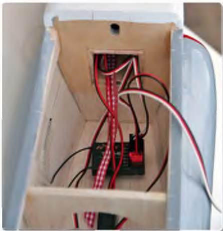
Front of wing bay looking onto F3, faced with 1/16" ply and showing the battery tube (a ribbon is tied to the battery for ease of removal/adjustment) and the hole for the wing dowel
