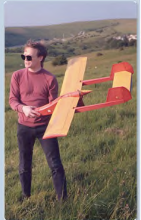
The pusher was repaired and rebuilt with twin booms. The canard was replaced by an all-moving-tailplane, with twin fins and rudders. I dispensed with the speed controller as I needed all the power I could get. Instead I used a servo operating a micro switch with a diode/resistor/capacitor suppressor across the contacts to stop them being destroyed by the arc when they opened. I am about to intrepidly launch it on its first flight. It was flown by a friend of mine who was much more practiced at flying than I was. The model flew very well until a glitch in the second - hand radio equipment I was using put all the servos hard over one way
