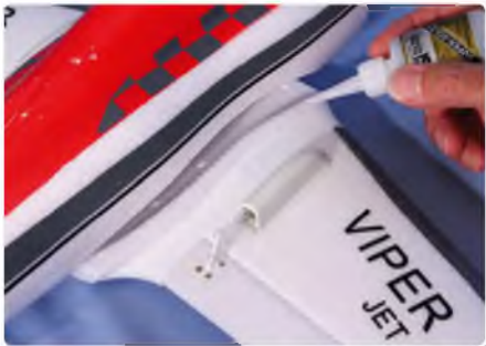
Watch out for any stray leads! The wing is glued to the fuselage. A few drops around the wing seat will do so don't go mad!
