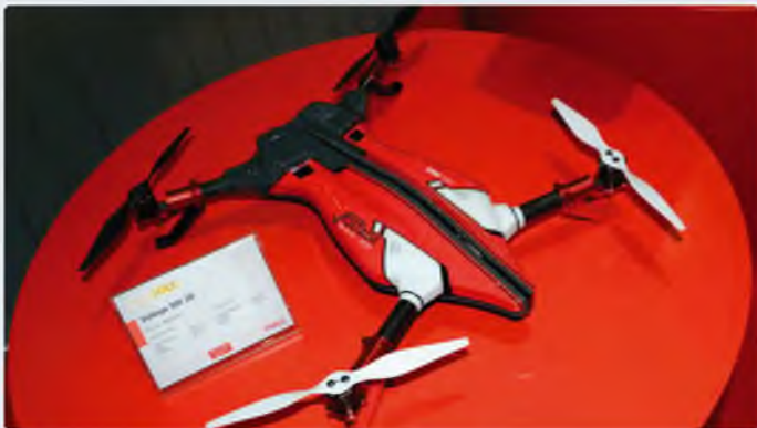
Voltage 500 3D is a fully assembled aerobatic quadcopter that lets you perform all the same type of stunts that are possible with a 3D helicopter, including loops, flips, tic-tocs, funnels and globes. For less experienced (or rusty!) pilots there is also a familiar quadcopter stability mode, with automatic pitch limiting so that you can get accustomed to the agile flight characteristics of this 3D quadcopter easily and safely. Requires a 3S/4S 2200 mAh LiPo or higher
