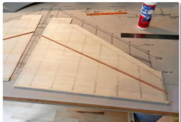
Initial wing assembly with bottom skins marked up with positions of lower spars, LE, TE and ribs. Bottom spar and TE shown fitted. All ribs from 1/8" balsa to aid skin adhesion
