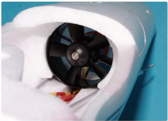
View of the 5-blade ducted fan
