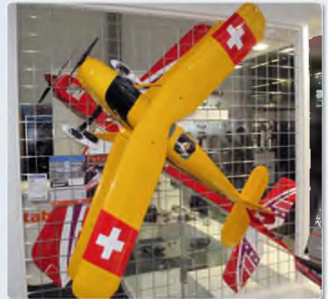
You'll easily keep track of this brightly coloured Bucker Bu 131 Jungmann during aeros. This 1.8 m span scale biplane from Black Horse suits 1.20 cu in glow or 20 – 30 cc petrol engines. Alternatively fly it with a 1800 – 2300W 450 KV brushless outrunner and a 6S 4000 – 5000 mAh LiPo
