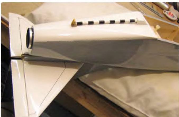
Rear fuselage covered. Arrestor hook is made from 1/4" dowel length fitted between two ply hard-points, drilled and pinned into the fuselage under-skin; this has proven robust as the model does not touch down on this
