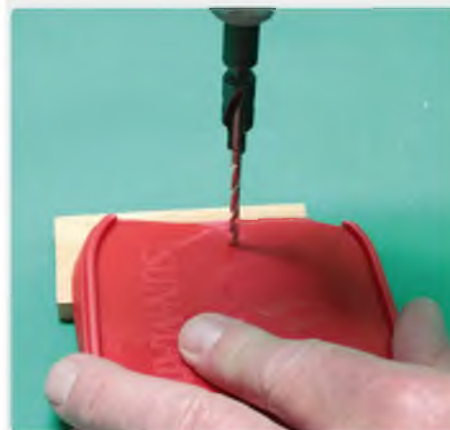
Step 1: Using a soft plastic lid (yes, I like raisins in my breakfast oatmeal!) and drill a series of holes slightly smaller in diameter than your machine screws' thickness
