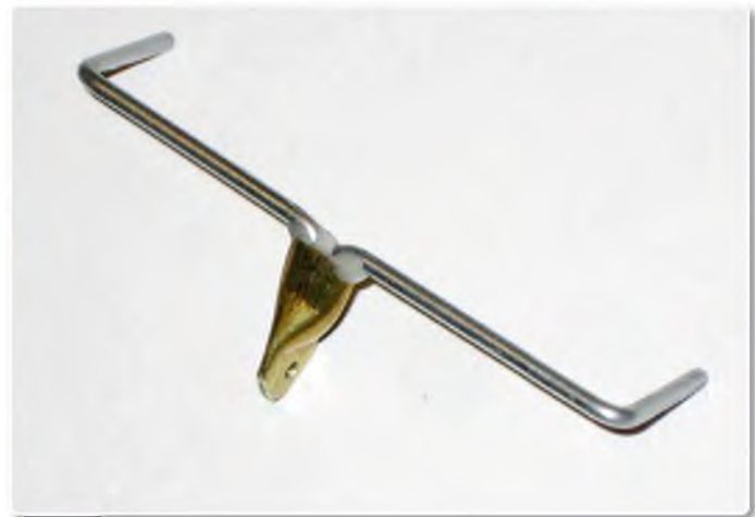
Elevator actuator from lengths of M2 rod and 5 mm brass tube, fixed with solder or slow setting epoxy. Brass tube crimped and drilled to suit M2 clevis. Height of actuator is critical to suit the snake output so make sure it clears the fuselage
