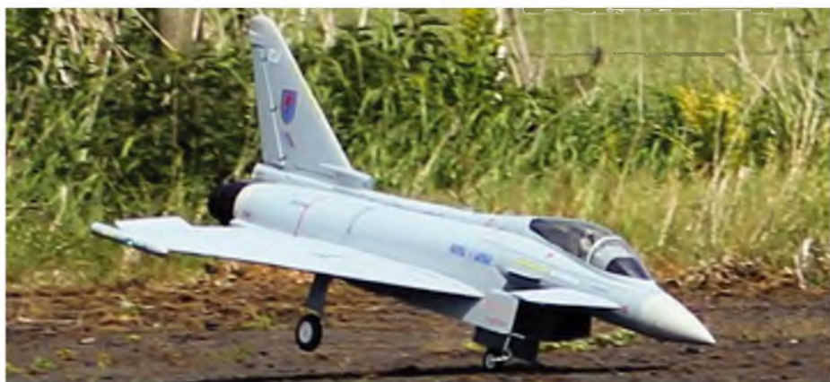
OUCH! A heavy nose bounce on tarmac but no damage whatsoever thanks to the shock absorbing nose wheel
