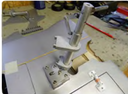
Make sure the legs are fitted the correct way around. The trailing links need to be facing the rear!
