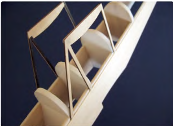
4 mm Depron formers in the parallel section of the fuselage
