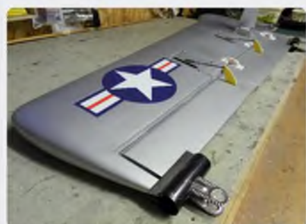
Bulldog clips were used to keep the surfaces at neutral while the pushrods were being made up to the correct lengths
