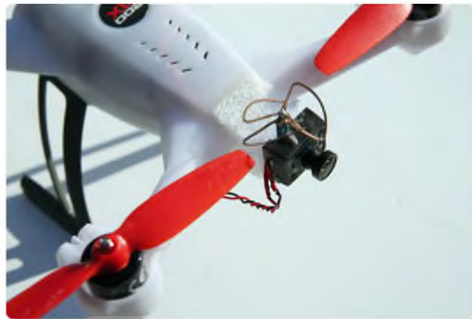
Horizon Hobby micro camera fitted to my Blade QX 200 quad
