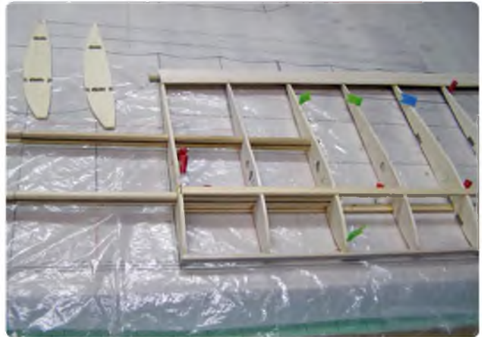
Wing joiners are glued in at this time
