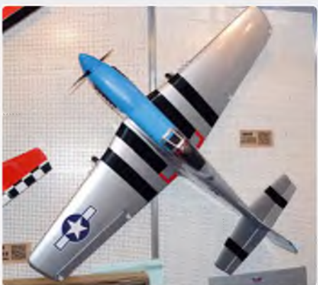
This P-51 Mustang is just over 1.7 metres in span and suits .60-.90 two-stroke engines, 20 cc petrol motors or 6S-4500 electric motor sets
