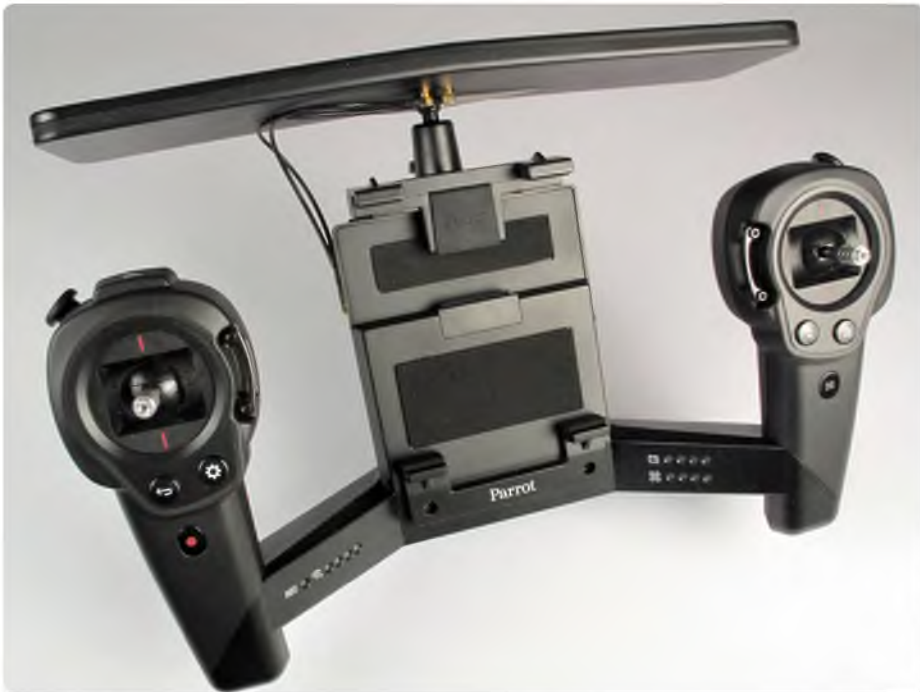
Futuristic Black Skycontroller is dominated by the widely spaced sticks and handgrips, and the huge dual band MIMO antenna
