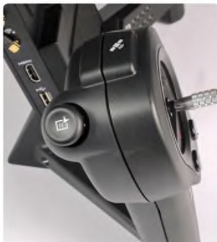
This left shoulder mounted button provides app navigation when using FPV goggles
