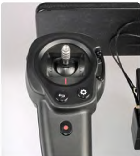
Left hand stick unit. The two buttons below the stick allow for screen changes when wearing FPV glasses. The button with the red dot is the video recording switch
