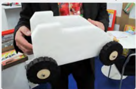
This quick to assemble foam dolly is a simple and effective way of getting Hacker's EPP semi-scale gliders off the ground when aerotowing
