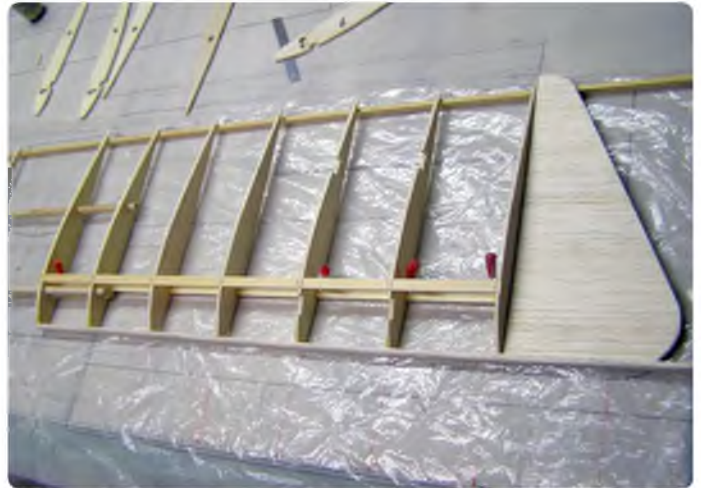
The bottom wing is partially built
