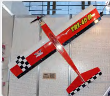
Other SF Models included Tri-40 II, a low wing sport model with classic styling. 1.6 m span for .40 two-stroke, .60 four-stroke or 10 cc petrol engines. Can also be flown with a 840 KV brushless motor on a 4S-2600 LiPo
