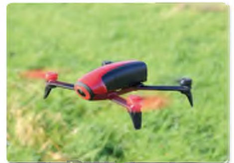
Bebop 2 contains a new Ublox Neo 8M GPS chip. The number of maximum visible satellites has also been increased to 19, compared to 12 for the original drone. Increased GPS reliability is an advantage for the automated flight modes such as Return to Home and Flight Plan, as well as high altitude stability
