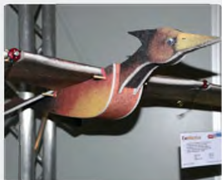
Looking for something a bit different? Exceloctylus is a twin EP flying dinosaur with a 1.6 m wingspan. It is operated by ailerons and an inverted V-tail
