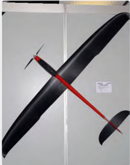
If you like carbon, you'll love this hot electric glider! Streamtec Carbon Design spans 2210 mm and features RDS (Rotary Drive System) linkages
