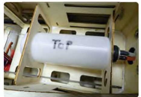
The fuel tank supplied looks a little lost in the voluminous front fuselage
