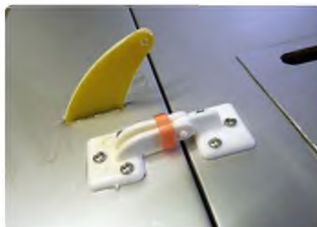
Neville fitted his own retaining rings, cut from fuel tubing. The control horns, pre-cut from epoxy board, are simply glued into slots in each control surface – works well!
