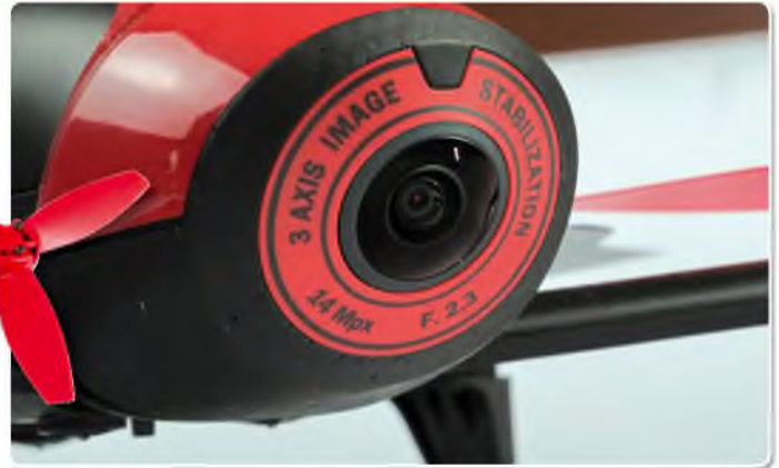
Bebop 2 has a new 180° fisheye lens that is more tilted towards the ground than the original so it captures more of the ground and less sky. The lens also catches more light for better video quality in low light conditions
