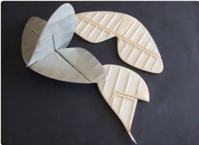
Finished tailplane and fin, and 'just finished' parts ready for covering with silver Solite
