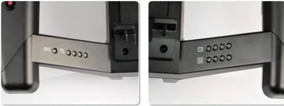
On the arm that connects the centre of the unit to the right handgrip are battery level indicators for both the Bebop and the Skycontroller. The left arm has a series of lights that show the strength of the WiFi signal and when the camera is recording video
