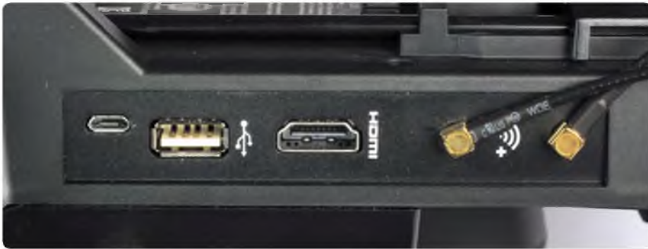
Data connections on the side of the Skycontroller. The HDMI port can be used to connect optional FPV goggles
