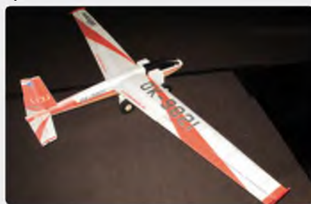
This quick to assemble foam dolly is a simple and effective way of getting Hacker's EPP semi-scale gliders off the ground when aerotowing
