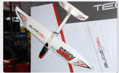
TecZone AirPusher 140 is Hobbico's latest take on the 'pylon mounted pusher' electric glider format. 1.4 metre wingspan, as the name suggests
