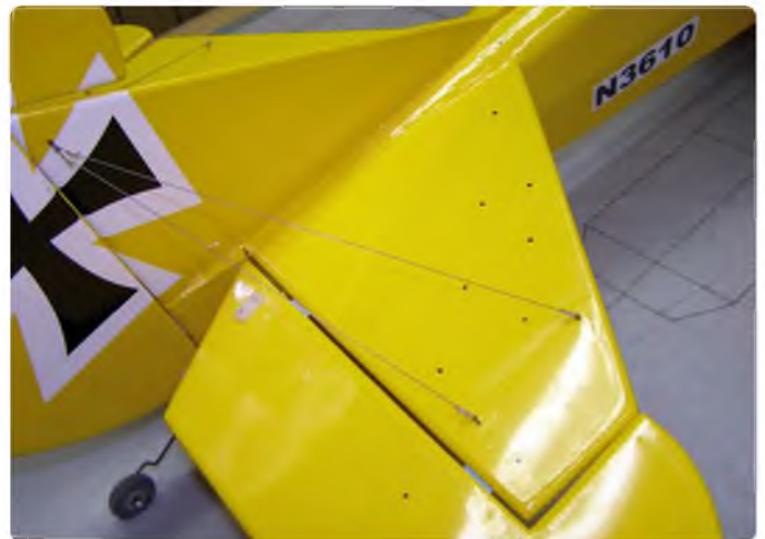
Twin stabiliser flying wires for additional strength
