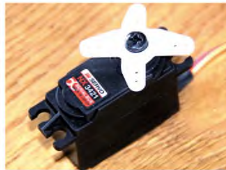
Digital servos have good holding power and should be used throughout an installation in turbine-powered models (Dave Gladwin photo)
