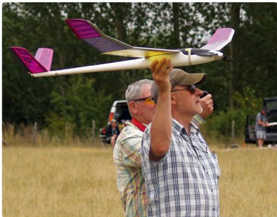
Closer view of the Highlight as Jon prepares to launch. This is a relatively old design and has a fuselage of 'reasonable' proportions. It currently houses an 1800 3S battery, which might yet go on a diet for 2016? As with several older R/E designs this one also lacks airbrakes of any kind, which can make descending from lift and landing with accuracy... taxing!
