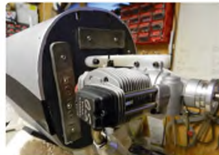
Close to a pound of lead was required to get the balance point correct, probably due to the lightweight OS engine used. A petrol engine would probably need a lot less weight
