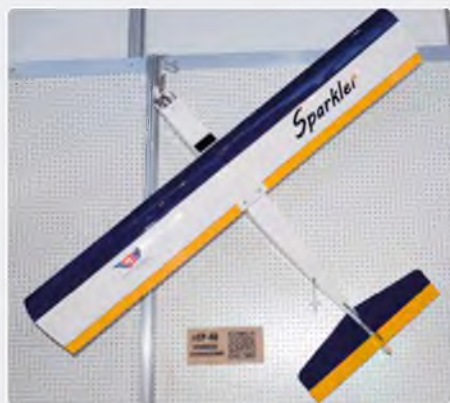
Get back to basics with the Sparkler, a 1.2 m high-wing sports model for electric power using a 3S 2200 mAh LiPo
