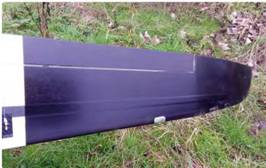
I spray painted the underside of my Sapphire tips with about eight coats of Pound Shop black car paint. I kept the wing in a warm workshop, gave it a very quick dust over, then gentle blow-dried. I was very surprised how good a finish I got and all for 4 g per wing of added weight
