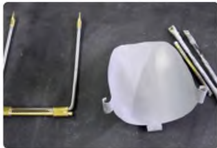
New strut on the left, with old parts for comparison, and mudguard to be reused
