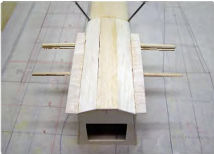
All the sheeting is done on the bottom of the front section of the fuselage The rear section is added
