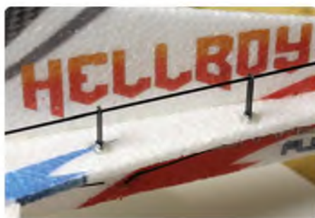
One millimetre diameter CF pushrods need supporting but this provides a very 'slop-free' action
