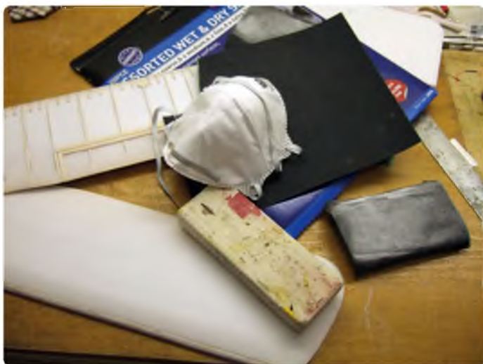
Top Depron surface now sanded to aerofoil section. A dust mask is essential!
