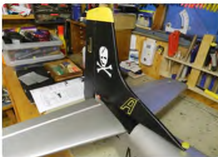
The tailplane and fin are glued in place - after checking and double checking!
