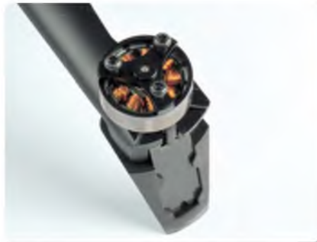
The props mount directly to the brushless motors and lock onto the three screw-heads. The motors have a higher winding density and extra reinforcements, giving better shock resistance
