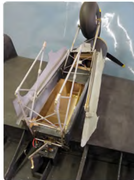
The gear part disassembled for new strengthened links. The new main gantry and tie beams are already in place
