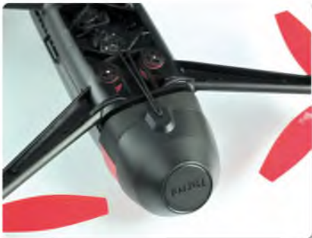
The fisheye lens is protected by a slip on cover
