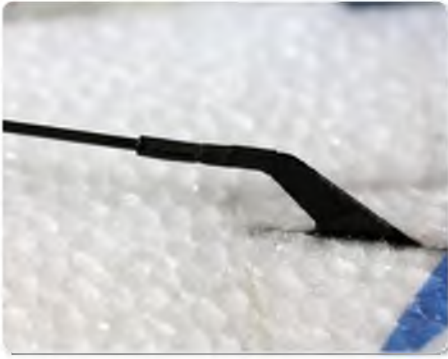
Heat shrink linkages are not my favourite system but do avoid 'slop' in the system
