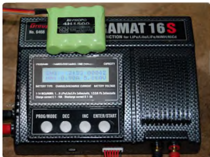
4-cell 4.8 V NiMH on charge at 0.9 A
