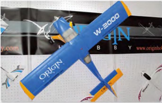
Wilga 2000 from Origin Hobby spans 1330 mm for a 1200 KV motor via a 30 A brushless ESC
