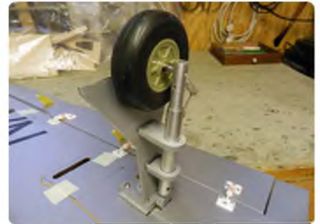
That's better! The final effect with the dummy wheel doors fitted to the main legs
