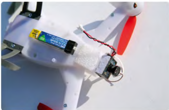
A 1S LiPo powers the FPV camera
