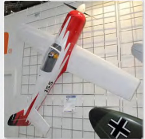
Radial Rocket from Black Horse is just over 1.4 metre wingspan and suits .46-.55 IC engines or 1000 – 1800 W, 800 KV brushless electric set ups. Inspired by the full size homebuilt, the Rocket features a spatted fixed undercarriage for durability and ease of operation
