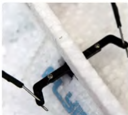
Extended servo arms require quite a powerful micro servo
