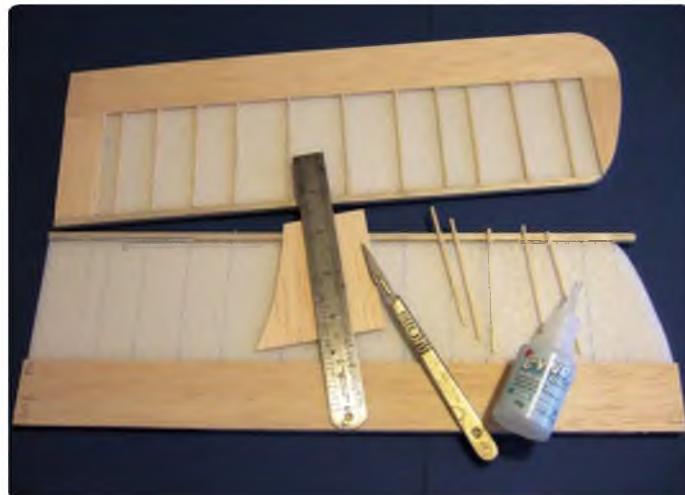
Rib positions marked and added using cyano friendly glue
