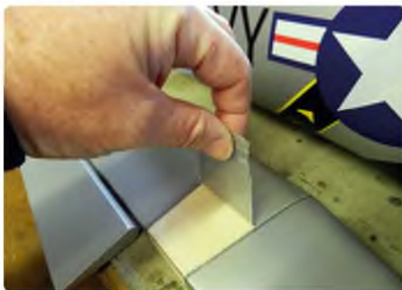
The unwanted covering can then be peeled away prior to applying glue to fix the tailplane in place
