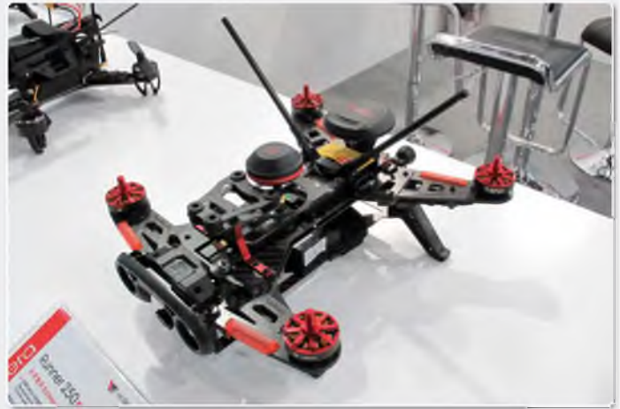
Runner 250 is fitted with 'intelligent direction warning lamps' – basically flashing indicators that show which way the drone is turning, just like your car! FPV pilots need all the help they can get during high speed races
