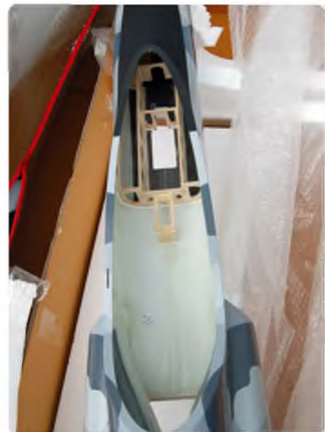
This is how Mark's kit came before the woodwork was sealed and painted. The wood trays are supplied loose, so are easily treated to the same finish
