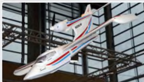
Seawind is a 1438 mm wingspan model based on the US amphibious aircraft. Powered by a 3S brushless motor set it can be flown from land and water thanks to its retracting undercarriage. Also features nav lights and flaps
