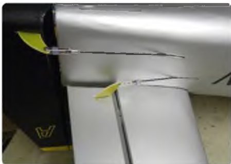
Epoxy horns and close fitting metal clevises result in slop free tail pushrods
