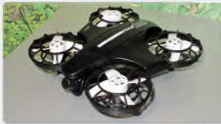
Blade Inductrix 200 FPV Drone is a compact, 155 mm square, easy to fly aircraft that is compatible with Fat Shark Teleporter V4 headsets. Supplied with a custom 800 mAh 3S LiPo
