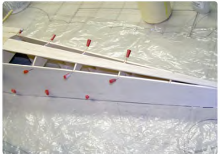
All the sheeting is done on the bottom of the front section of the fuselage The rear section is added
