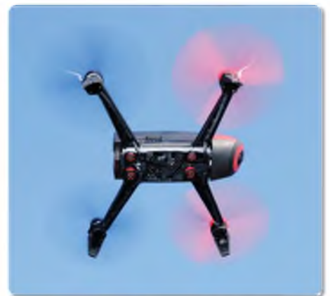
Underside view giving a good view of the large, red anti-vibration grommets
