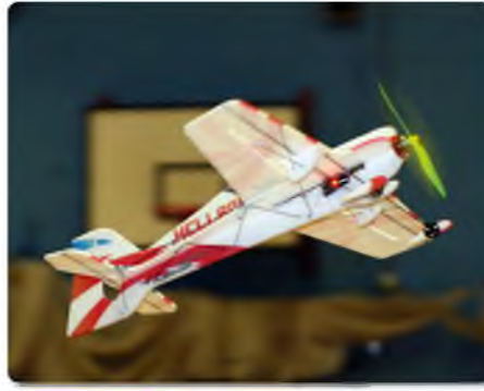
An underside view shows the CF bracing and, at this point, an undercarriage!
