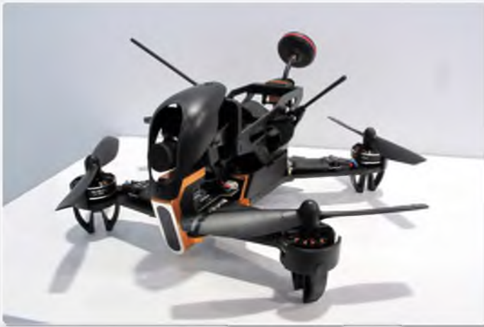
Walkera's stand was dominated by drones. F210 is their new FPV racer that features a 'bow' design chassis cut from carbon fibre and fitted with a new F3 flight controller
