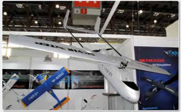
Origin were displaying several commercial drones including this 1.8 metre span twin boom pusher, the FPV 'Skyhunter'
