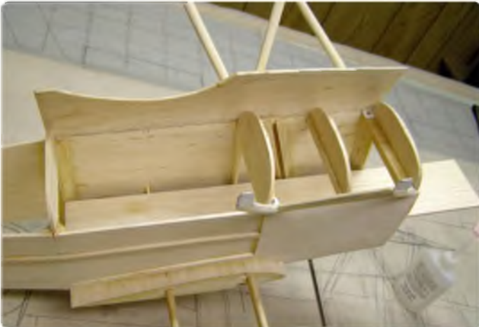
Top of the front fuselage section is sheeted. Notice the battery floor in place
