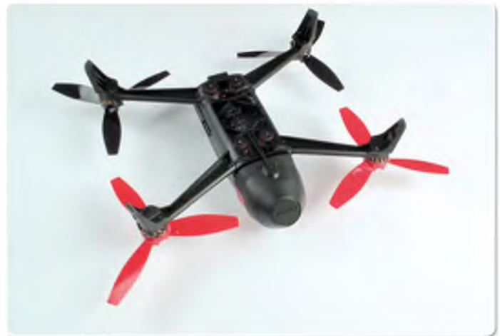
Pairs of large grommets front and rear provide effective isolation of the camera from motor vibrations
