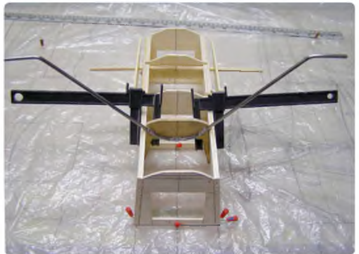
The front half of the fuselage is built upside down
