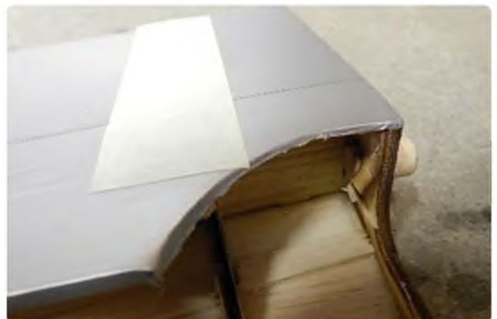
A small amount of 'break out' is visible where the front wing incidence peg has been inserted
