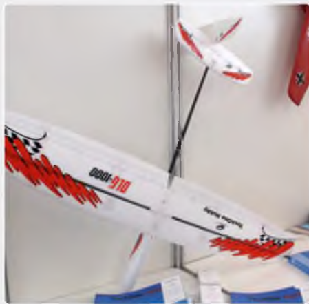
DLG-1000 has a wingtip mounted peg for discus style hand launching
