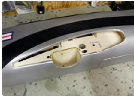
The wing panels are a tight fit in the cuffs on either side of the fuselage
