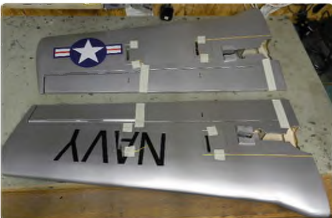
Neatly finished wing panels come with the servo hatches, flaps and ailerons taped in place
