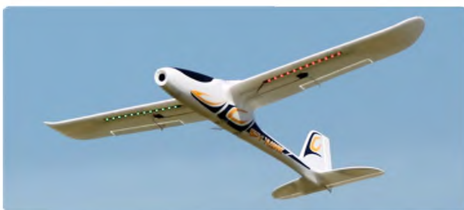
The underwing LEDs show up clearly even on a sunny day
