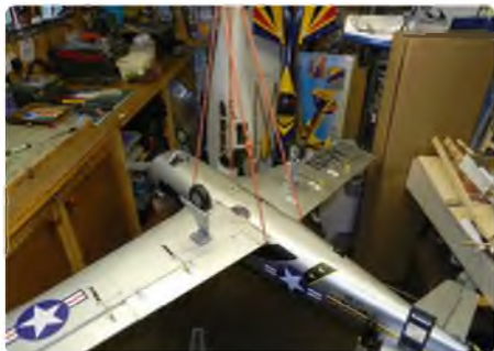
Neville used a rope sling to accurately set up the recommended Centre of Gravity
