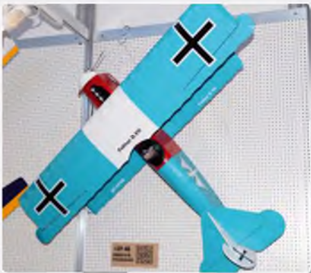
This attractive colour scheme decorated a Fokker D.VII on the Super Flying Models stand. Of 1200 mm span the laser cut ARTF is powered with an 850 KV brushless motor and 4S-220 LiPo
