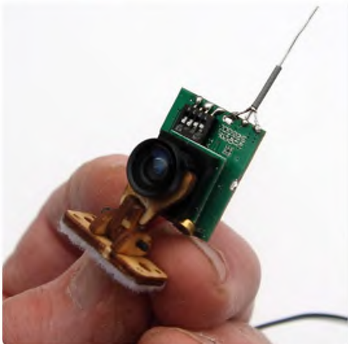
The 3.6 g micro FPV camera and Tx from Banggood. First tests are very promising
