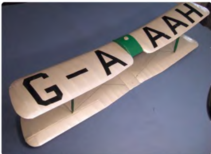
When the wings are fully assembled it is possible to remove the entire wing assembly in one piece over the tail without de-rigging
