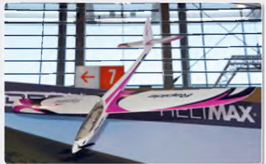
Flyzone's 1475 mm Sensei FS (Flight Stabilisation) trainer features WISE stabilisation. This offers three piloting modes, starting with Beginner, which limits bank and pitch to 30 degrees. WISE also offers a 'bailout' function to resume level flight, as well as automatic take-off and landing. Best of all it works with most commonly available R/C systems. Sensei FS also features a 'Drop Door' payload system – ideal for toffee bombing!
