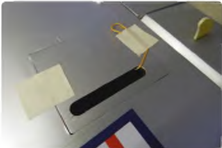
Wing servo hatches are taped up with pull strings with which to pull through the servo leads
