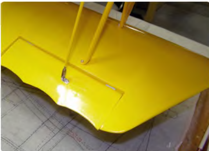
Attachment of the connecting rod between the top and bottom ailerons
