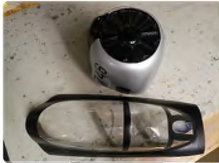
The cleanly moulded canopy and factory painted fibreglass cowl are notable features of this fairly big model
