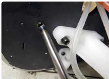
The piano wire 'drill' is perfect for making lined up holes in the front fuselage formers so that the throttle pushrod can pass through
