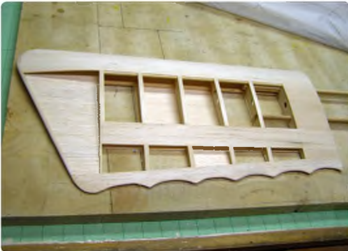
The wing panel is sheeted before the aileron is separated
