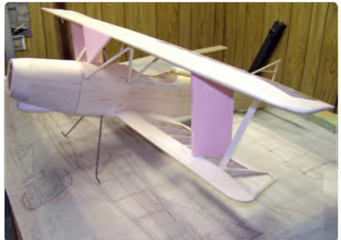
Foam templates are used to align the wing geometry
