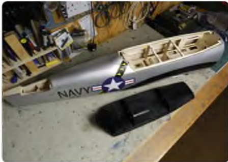
There's plenty of space inside the cavernous fuselage for either an electric or IC installation
