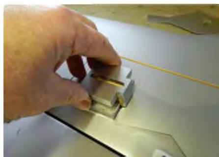
Additional torque blocks are fitted on top of the retract mounts to enable fitting of the fixed undercarriage legs supplied in the kit
