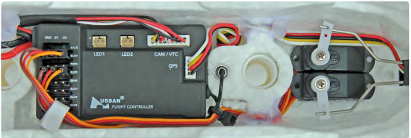
The servo and special Rx area
