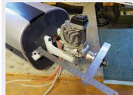
Lightly clamping a short steel rule between the prop washer and prop driver forms a straight edge against which the correct depth for the engine can be accurately set
