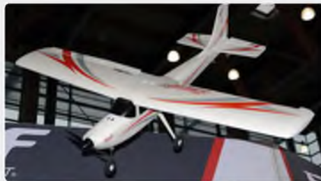
Right: Flyzone Rapide is categorised as a 1522 mm wingspan 'warmliner'. Fitted with a brushless motor set, the AeroCell moulded foam glider promises a high level of aerobatic agility
