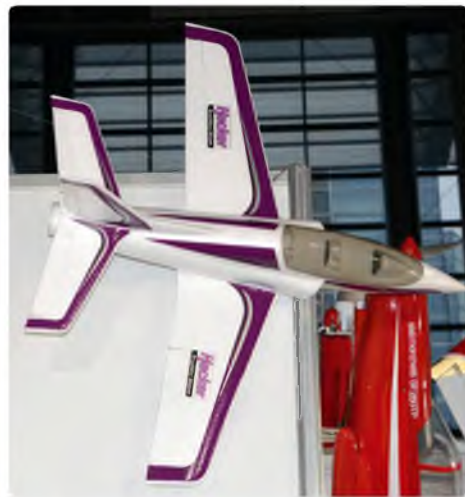
An ideal aeroplane for the Hacker Stream-Fan 70/3500 EDF, this sleek foam Viper Jet is just 1040 mm in span. Suits a 4S 3800 mAh LiPo on the 3500 EDF, although up to 6S can be fitted if using the Stream-Fan 70/2700 www.hacker-motor-shop.com/
