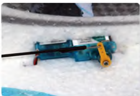
End to end servo mounting makes for a firm installation
