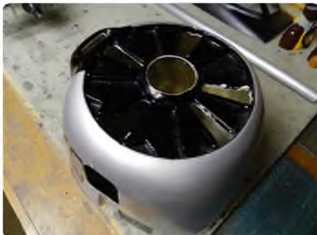
Cutting out some of the gaps between the dummy radial cylinders allows cooling air to enter the engine bay
