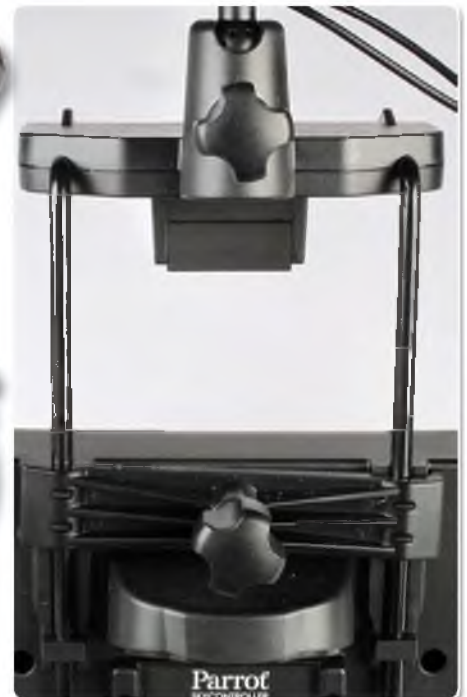
Left & above: Back panel showing the battery mount and the sliders for the adjustable tablet mount. The antenna orientation can be changed and locked in place using the top locking screw
