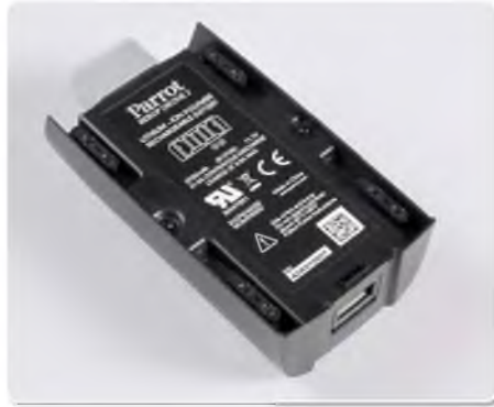
The combo includes two of these 2700 mAh LiPo packs. A soft cover over the contacts helps stop short circuits whilst in storage and transit
