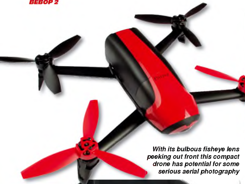
Bebop 2 has a new 180° fisheye lens that is more tilted towards the ground than the original so it captures more of the ground and less sky. The lens also catches more light for better video quality in low light conditions
