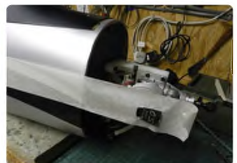
Long lengths of broad masking tape can be used to locate the position of any engine parts that need to poke out of the cowling
