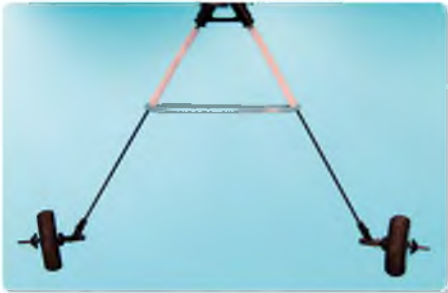
The longer U/C legs showing the tube extensions
