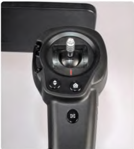
Right hand stick with the Take Off/Landing button below left and the Return Home button on the right. The Emergency Landing button in the centre of the grip has now been replaced with a handy button that re-centres the camera
