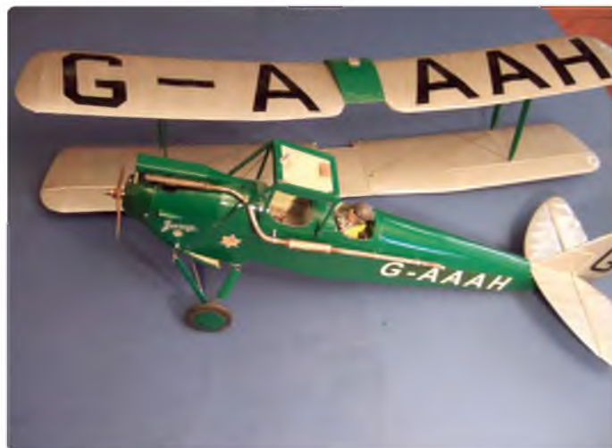
When the wings are fully assembled it is possible to remove the entire wing assembly in one piece over the tail without de-rigging
