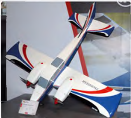
Great Planes Twinstar EP is a 1205 mm wingspan twin motor sports model of ARTF built up construction, covered in Monokote. Requires a 3S 2200 mAh LiPo and four function R/C
