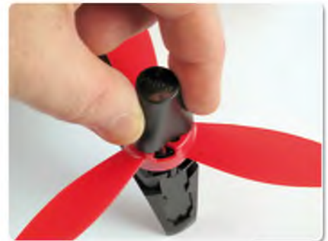
Spare props are supplied, along with a small hand tool to twist them off. Bebop 2 has 6" propellers versus the 5.5" props on the Bebop 1, which Parrot claim gives it over 10% more thrust
