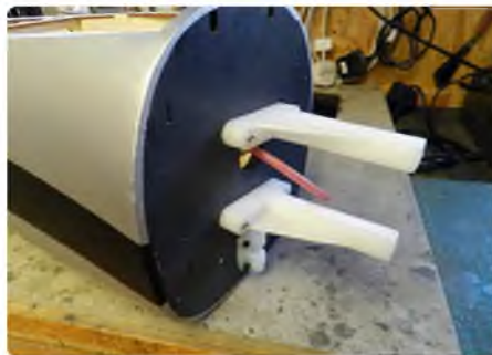
The IC engine bearers fitted the pre-installed blind nuts accurately
