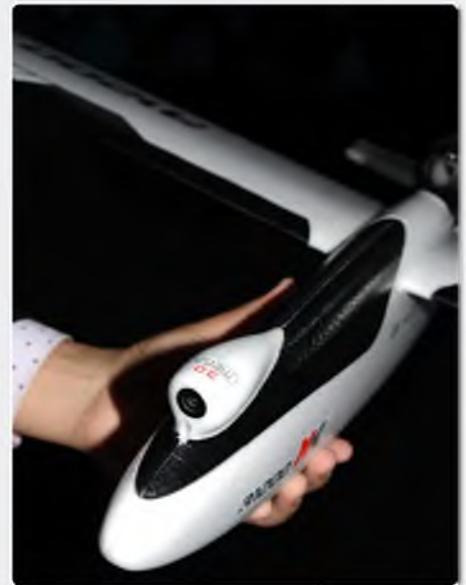
A closer look at the 1080p HD camera fitted in the canopy of the A1200
