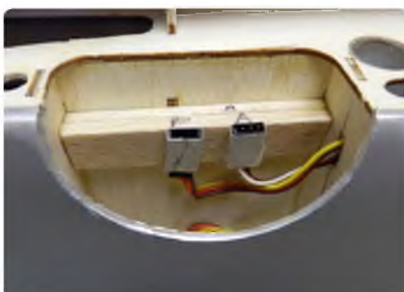
Some scrap balsa was used inside the wheel bays to make up fixed connecting points for the aileron and flap extension leads
