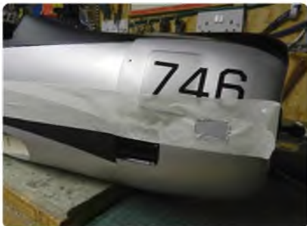
The marked hole can be easily transferred to the cowl for cutting out
