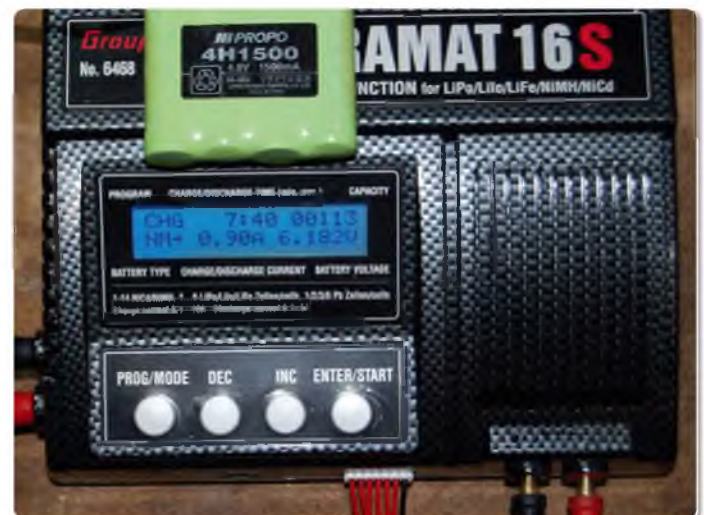
After 2 mins 5.86 V and after 7 mins 6.18 V... So not 4.8 V!
