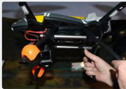
HeliMax Form 500 has folding motor arms for compact storage and features a novel twin rail mounting system so you can fit bespoke payloads. An action camera mount is included to get you started. Supplied with a 5000 mAh LiPo
