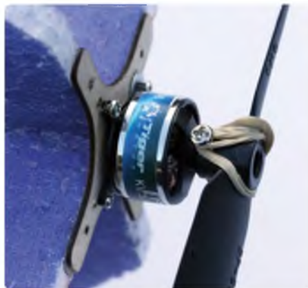
The Yak also uses a 2S Tiger brushless that is at its best with a 6" prop
