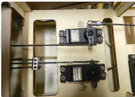
Dual elevator pushrods are connected to the servo using a triple connector block
