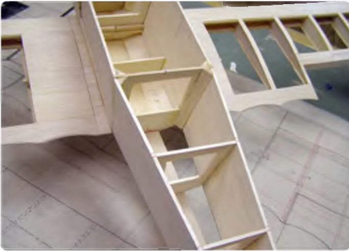
Vertical triangular stock pieces stiffen the joints between the front and rear sections
