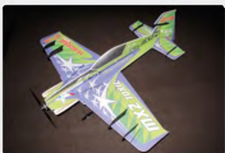
The Toxic series of 'shock style' models includes an MX2 and Edge 540. Constructed from 5 mm pre-cut and coloured EPP, they span around 830 mm and suit MFORCE 2815CA-20 motors and a 2S 350 mAh LiPo
