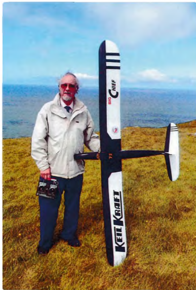
Alan Charlesworth with his reworking of Keil Kraft's 'Chief' vintage A2 glider. Stretched to 82" and engineered for the rigours of Welsh slope sites, the 'Big Chief' nonetheless incorporates an actual KK kit
