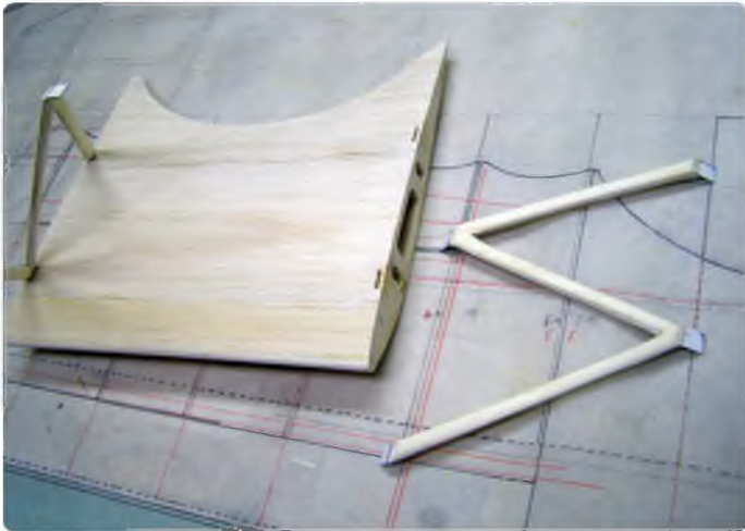
The centre-section is sheeted. Notice the slots cut out in the sheeting for the cabanes' aluminium tabs to go into
