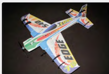
The Toxic series of 'shock style' models includes an MX2 and Edge 540. Constructed from 5 mm pre-cut and coloured EPP, they span around 830 mm and suit MFORCE 2815CA-20 motors and a 2S 350 mAh LiPo
