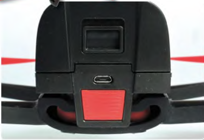
The battery clips on to the rear of the chassis. The power switch doubles up as a large, bright red flashing taillight that indicates that the drone is communicating with the Skycontroller or smart device
