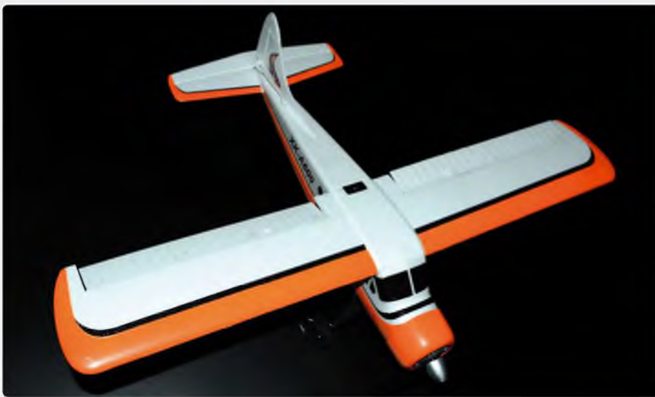
Above: DHC-2 A600 is a miniature Beaver with 580 mm span wings and powered by a 300 mAh LiPo
