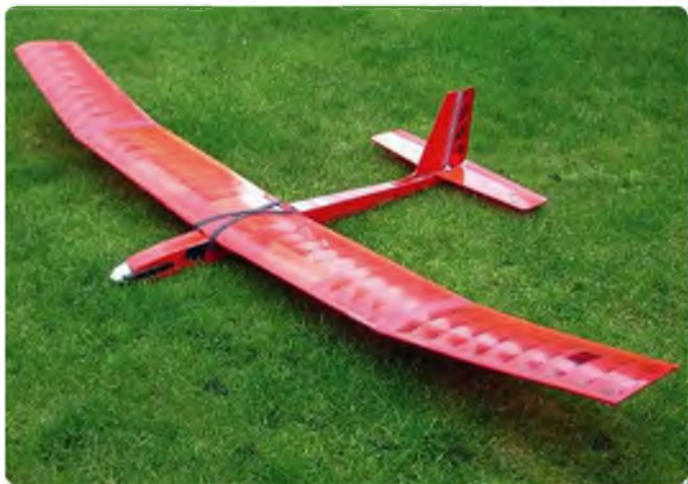
Better view of the Gentle Lady showing its simple lines and construction. The wing section is as flat bottomed as it could possibly be. Only the leading edge strip is rounded and both the spars are on the bottom surface. A 2.5 m version is in the offing – more anon...
