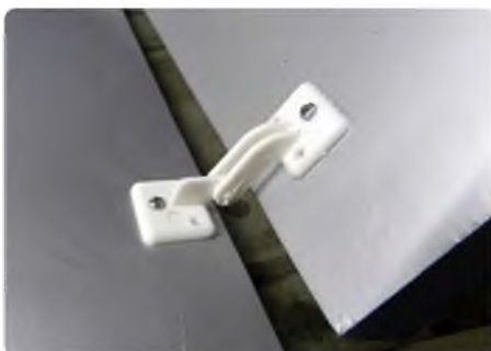
Upside down view of a flap hinge. This design gives plenty of movement
