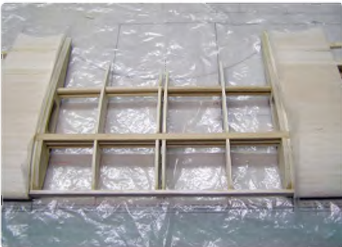
The centre-section of the top wing is built while joiners are keeping everything aligned
