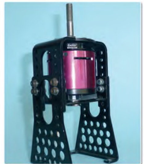
Adjustable metal motor mounts are ideal for mounting large brushless motors
