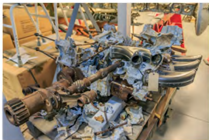
A good example of how different metals deteriorate in the sea over time. What looks like the remains of a Napier Sabre engine? The 2014 picture shows how it was originally. In the 2015 one several parts have been cleaned. The stainless steel exhaust stubs look like new, whereas the alloy block has deteriorated very badly
