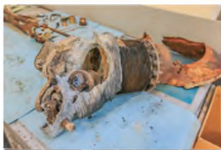
One of the cylinders from the Do17's Bramo 323P 9-cylinder radial engine (2014)
