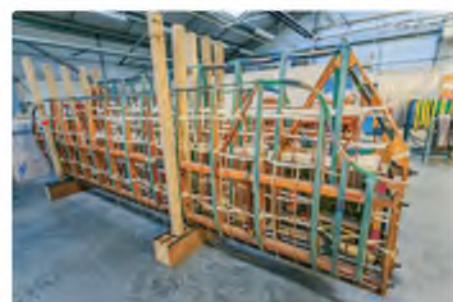
The wings have been stripped of their fabric and these too look in fairly good condition (2015)
