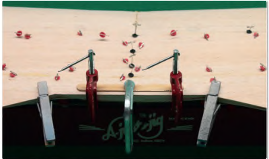
Mix and match your clamps to suit the job. The Waco's wing TE is too thick at the root for clothes pegs so I used 'C' clamps (plus dent-reducing dessert sticks) in the very centre. Spring clothes pegs worked fine on the thinner parts of the TE
