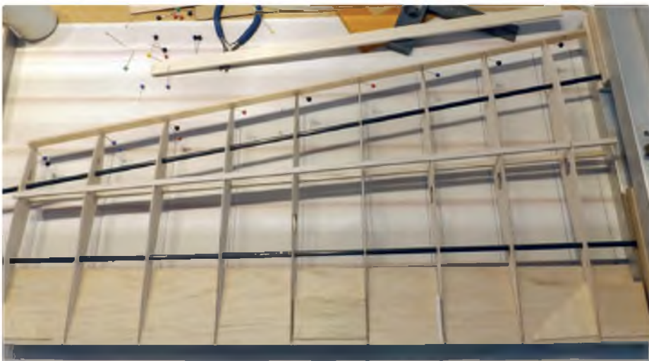
Stage 2 - Add the spars and Leading Edge, followed by the TE sheeting
