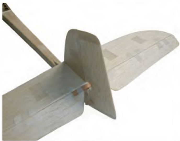
Tail end. The anti-warp balsa inserts are cross-grain
