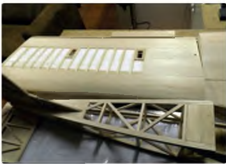
The Stick's sturdy structure is built up with balsa sticks, making it light and economical to build
