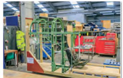
The original front/cockpit section was quite badly damaged. This is the new front end being rebuilt (2014/15)
