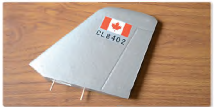
Two cocktail sticks were used to add support when gluing the central fin in place
