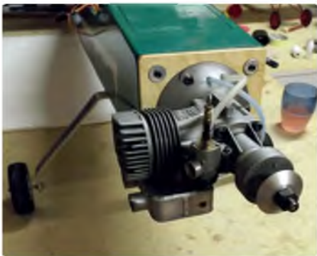
Engine mounting with a 25 cc Super Tigre motor that I was given
