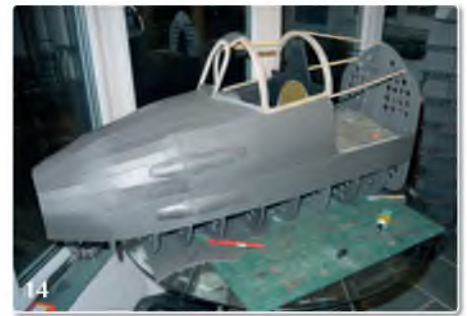
The Meteor's forward fuselage in Depron-build
