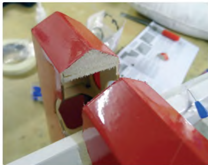
The rudder post needs to be cut away with a razor saw prior to fitting the tailplane
