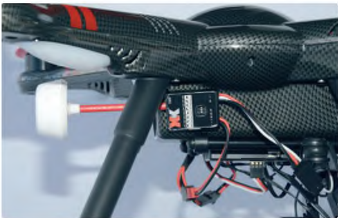
There's no dedicated position to mount the Launch Module on the X-380 so we taped it on horizontally, with the mushroom aerial pointing out the back
