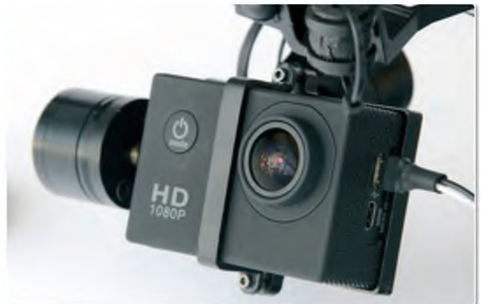
The AV lead plugs into the USB socket on the side of the camera. Be careful not to switch the camera off when plugging the lead in!
