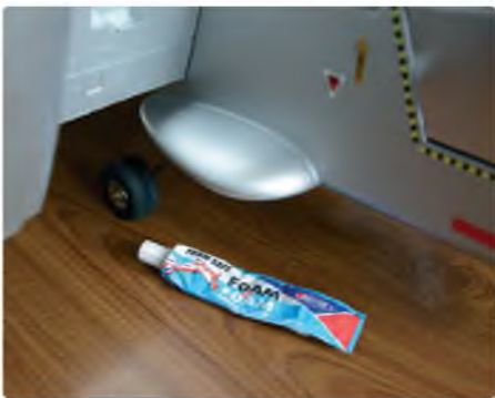
Foam 2 Foam glue was used instead of epoxy to glue on additional foam parts, like the undercarriage fairings
