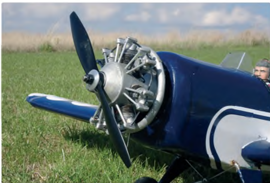
The dummy Rotec radial engine. See January issue for details of how to make one
