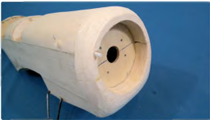
The front of the fuselage is made up from two laminations of 1/2" sheet and shaped to a smooth rounded contour
