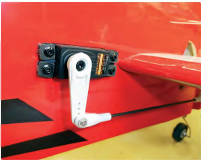
Close up on the elevator linkage using the longest throw available on the servo arm
