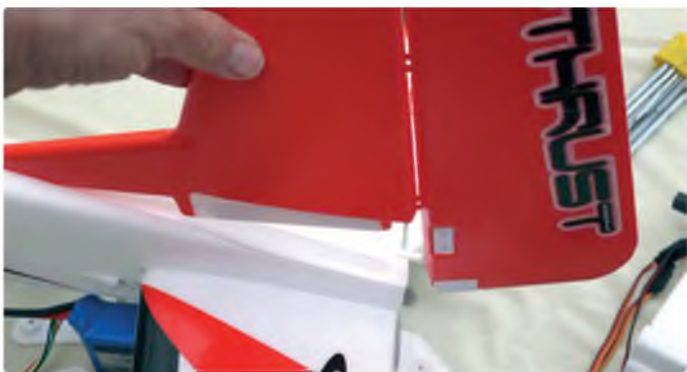
The horizontal stabiliser slots into the fuselage before the fin is slotted in and held in place with two Allen bolts installed from the underside of the fuselage. This clamps both tail surfaces in place so no gluing is required
