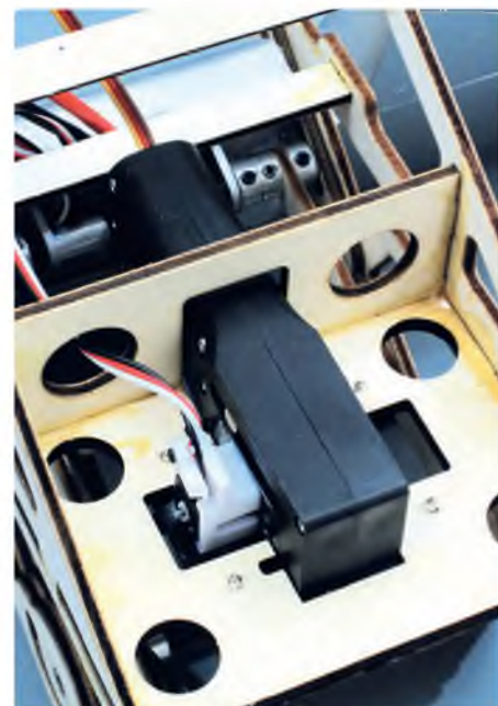
Wing tilt is performed by this actuator, which looks similar to an electronic retract
