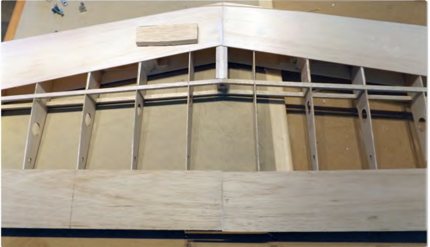
Stage 5 – The wing panels can be joined after removing them from the jig
