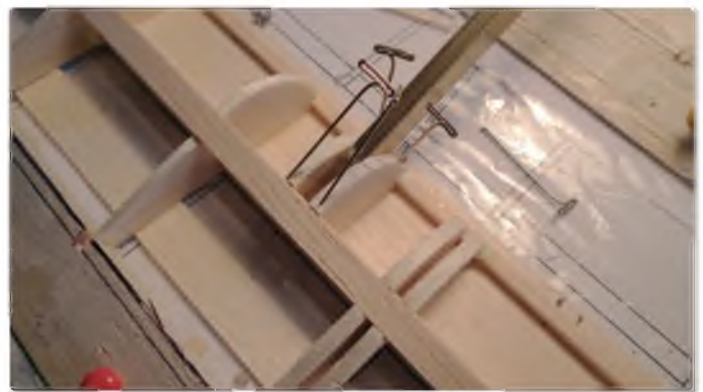
Fitting the ribs at the hinge points. Note use of rectangular brass tube for accurate spacing
