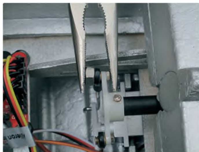
The ball links were very stiff so I used a nut as a protective sleeve and a pair of pliers to add the necessary pressure
