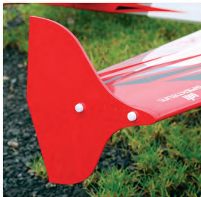
The SFG's make knife-edge a tad flatter, with less rudder input, but their effect is minor
