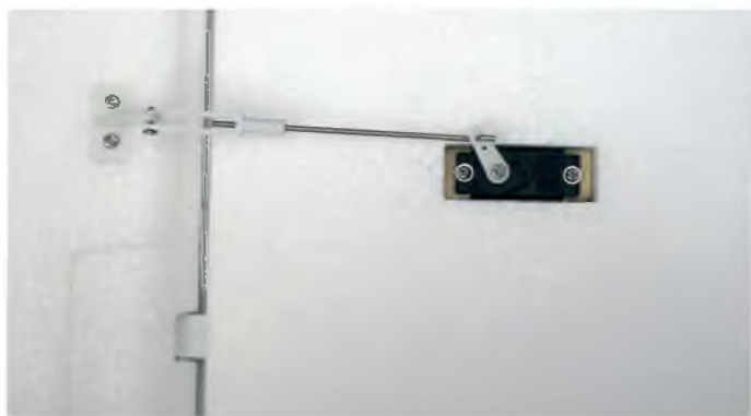
As supplied the flap servos are centred and the flaps have up and down movement. So the flap control arms were rotated on the servo splines to give more down deflection
