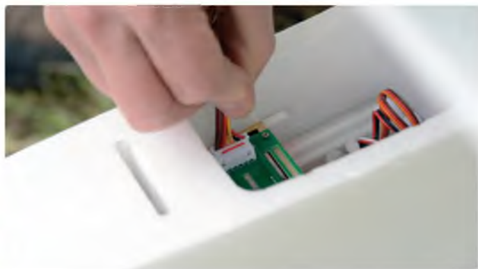
At the flying field the wing servos and LED lights are quickly connected to the PCB board. There's no chance of getting the servo connections wrong – very neat!
