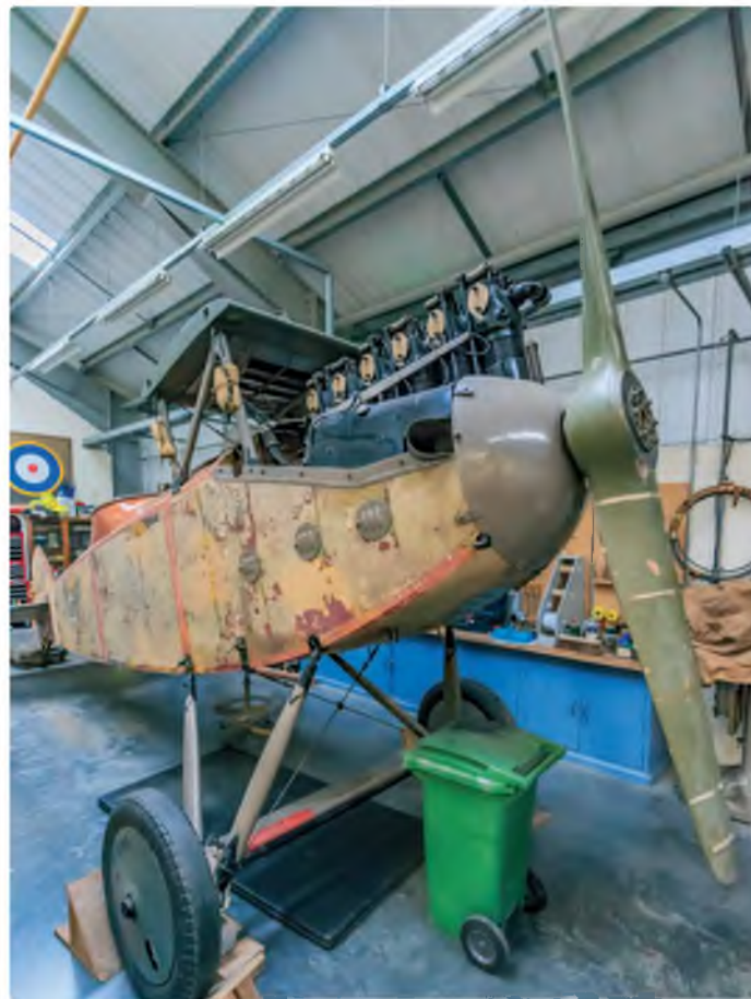
The old coverings have now been stripped off and work on the wood can begin. The LVC does look in fairly good condition for its age (2015)
