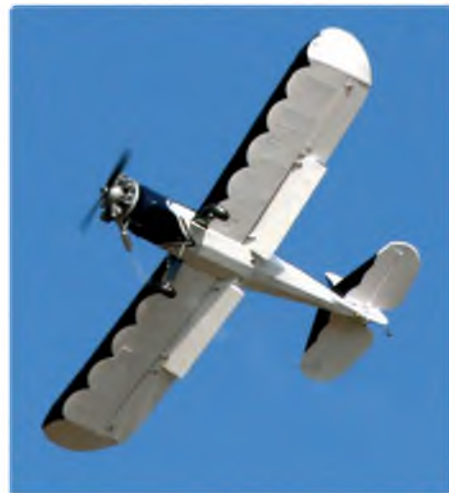
The large flaps slow the model without height loss but the LoCamp remains steady
