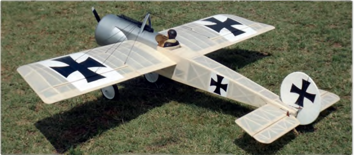
All the detail now added, with elastic rigging for appearance only
