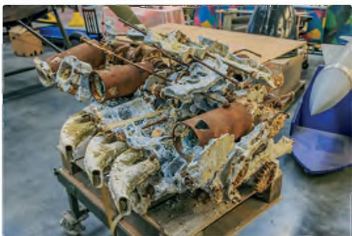
A good example of how different metals deteriorate in the sea over time. What looks like the remains of a Napier Sabre engine? The 2014 picture shows how it was originally. In the 2015 one several parts have been cleaned. The stainless steel exhaust stubs look like new, whereas the alloy block has deteriorated very badly
