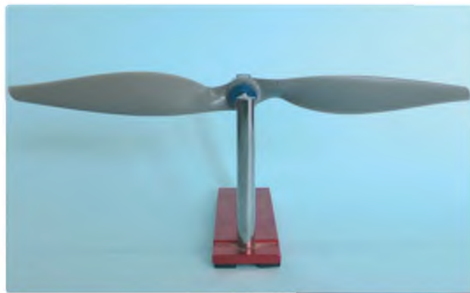
Balancing propellers is vitally important. Unbalanced props cause excessive wear on motor bearings
