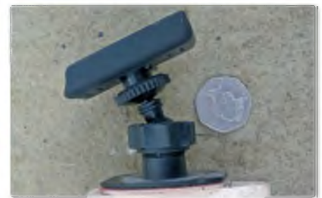
Coin of the realm showing the miniature Mobius and one of its ball mounts
