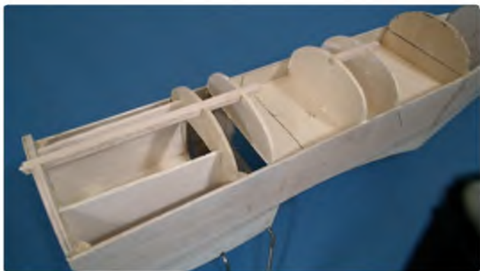
Spines fitted ready for top sheeting
