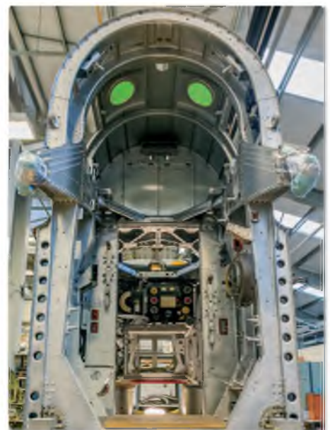
Looking inside the fuselage. The wireless operator's station can be seen complete with Tx 1154 and Rx 1155 at the back (2014)
