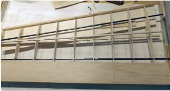
Stage 3 – Add the top Trailing Edge sheeting
