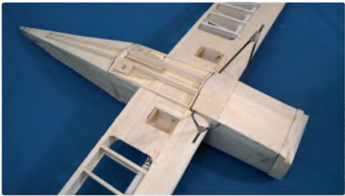
View of underside showing fairing and stringers
