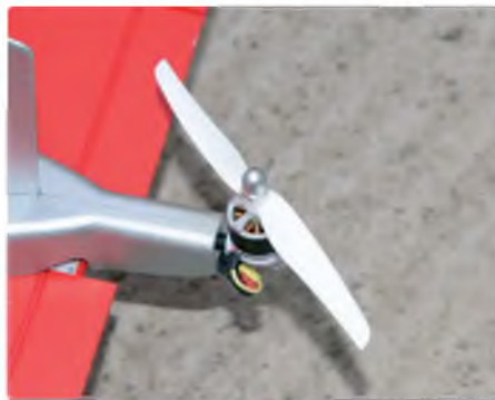
The rear motor tilts on a shaft to yaw the model and changes in thrust control pitch in the hover
