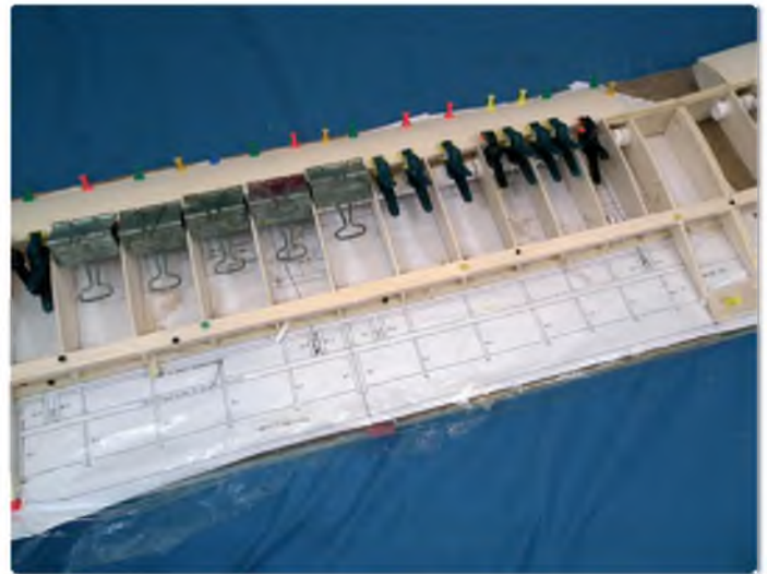
The wings being joined. Both leading edges can be covered with sheet before joining, using clamps and map pins to hold the sheet down
