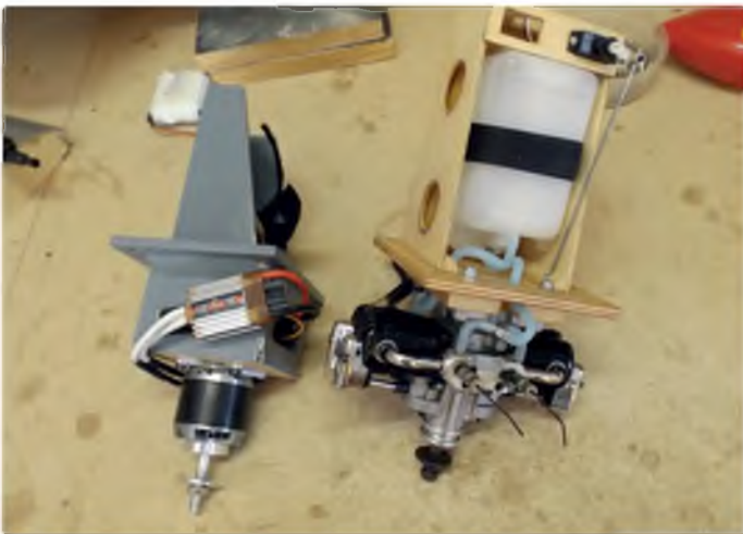
Glow and electric 'power modules' with all the required bits for each form of propulsion
