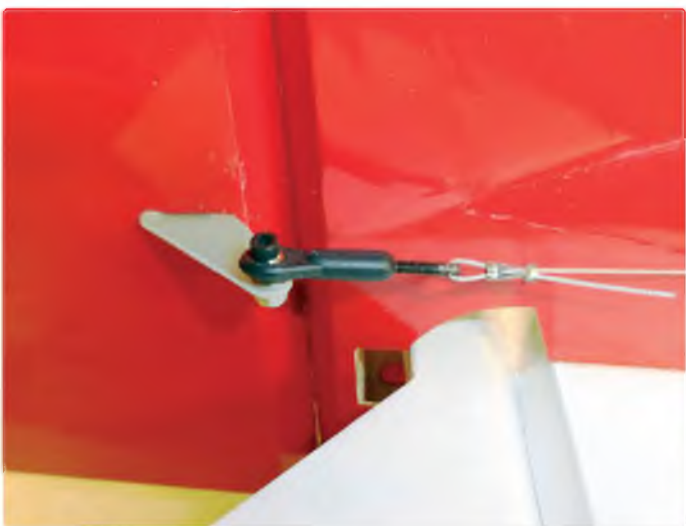
Rudder operation is via a closed loop system
