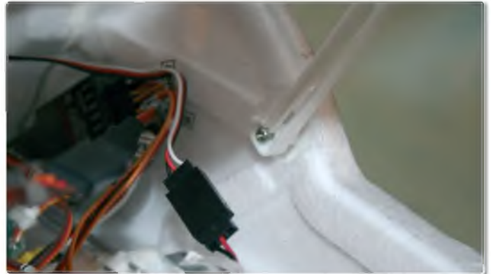
Swing stays lock the canopy open when accessing the radio and battery bay
