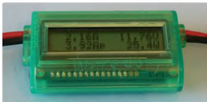
A Watt Meter is a 'must have' tool for setting up electric power systems. It removes all the guesswork
