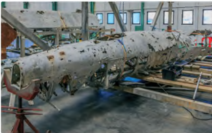
The aluminium airframe is in a very fragile state and it needs lots of support (2014)
