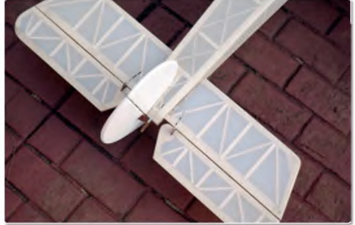
Elevator and rudder are operated using pull/pull cables
