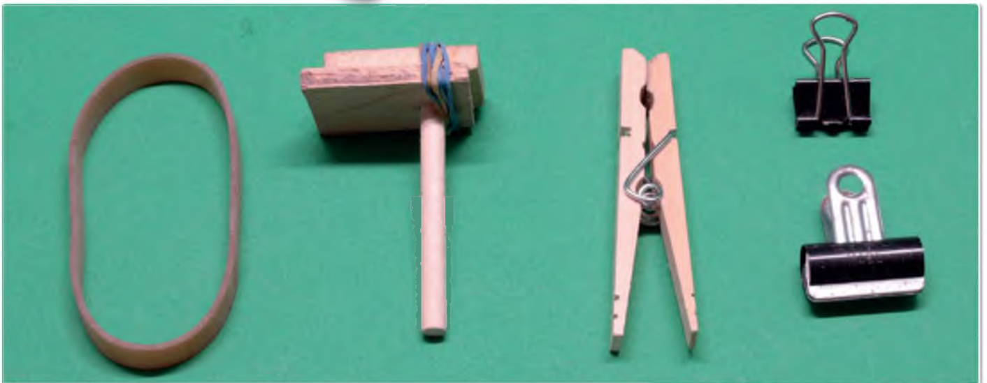
Elastic clamps (from left): Elastic band (surprise!), homemade thumb clamp, spring clothes peg and two binder clamps
