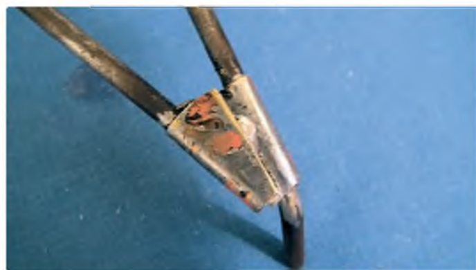
The bottom of the U/C legs are joined by wrapping with brass sheet and filling them with solder
