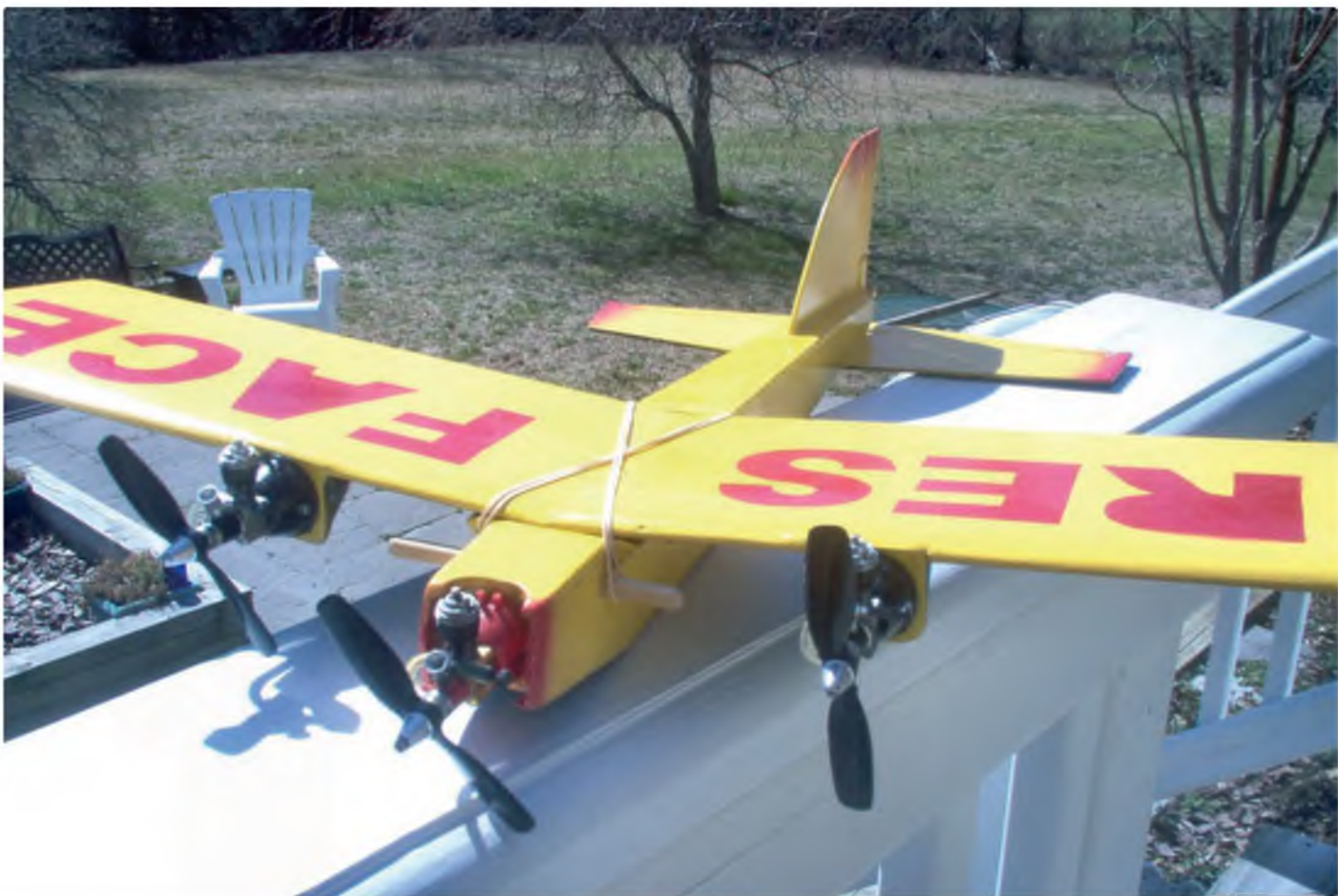
Eric Clutton's 'Sharkface' has made numerous appearances here over the years. Probably the most well known micro R/C model, it has a virtual fan club throughout the world. Raymond Lefrancois's incredible trimotor version flies well with three Cox TD .010s!
