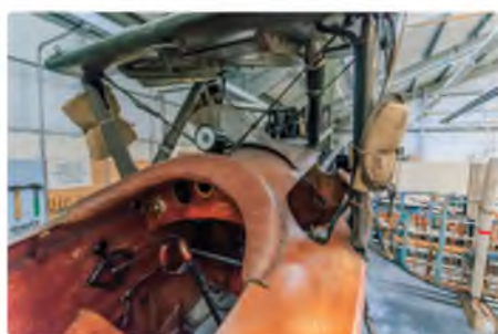
The old coverings have now been stripped off and work on the wood can begin. The LVC does look in fairly good condition for its age (2015)
