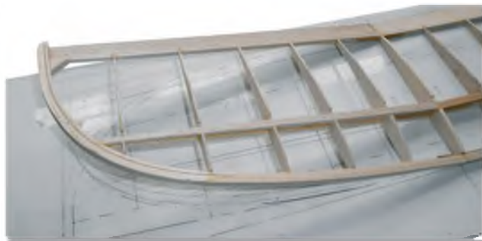
Wing build showing tip laminations (see text)
