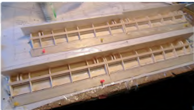
Glue balsa sheet to the leading edge and allow to dry before being bent over with the aid of water and a heat gun
