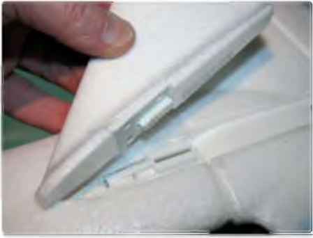
The upper fin is keyed in place with a slotted moulding
