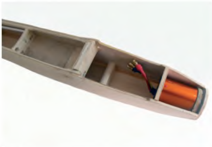
Basic fuselage with in-runner motor fitted for final shaping
