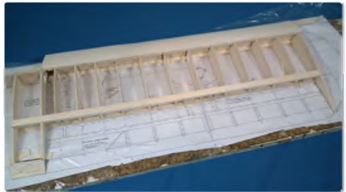
Top sheet applied to leading edge
