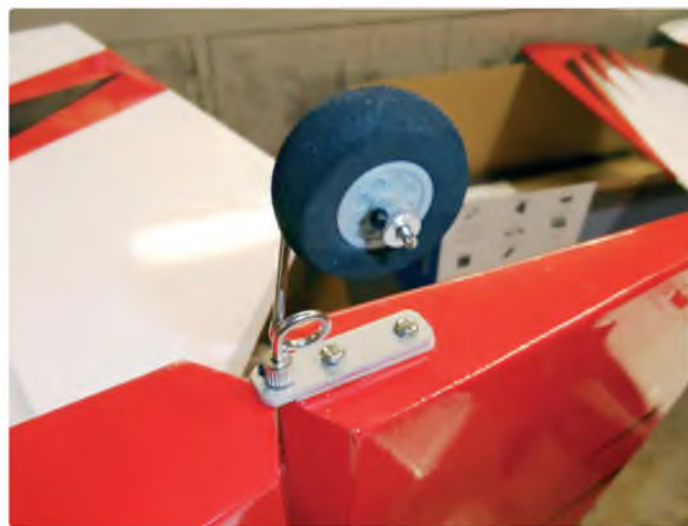
Detail view of the tail-wheel assembly
