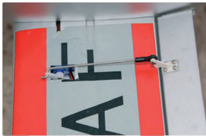
Aileron servos are pre-connected and were found to be well centred and giving the correct throws
