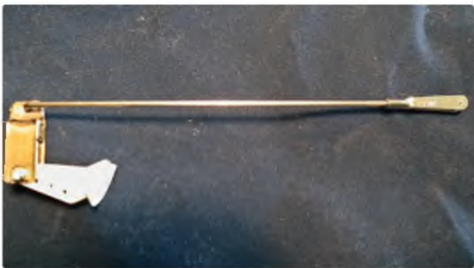
Complete aileron unit. The pushrod will need a bit of bending for free working
