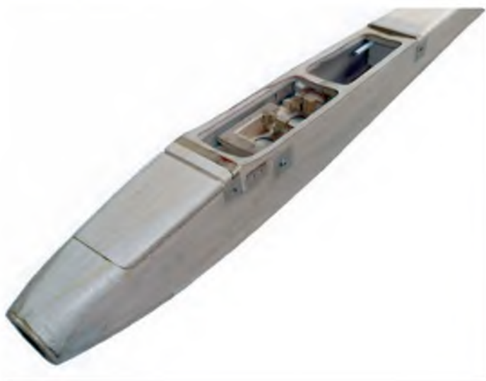
Nose after final sanding. Note the servo tray position
