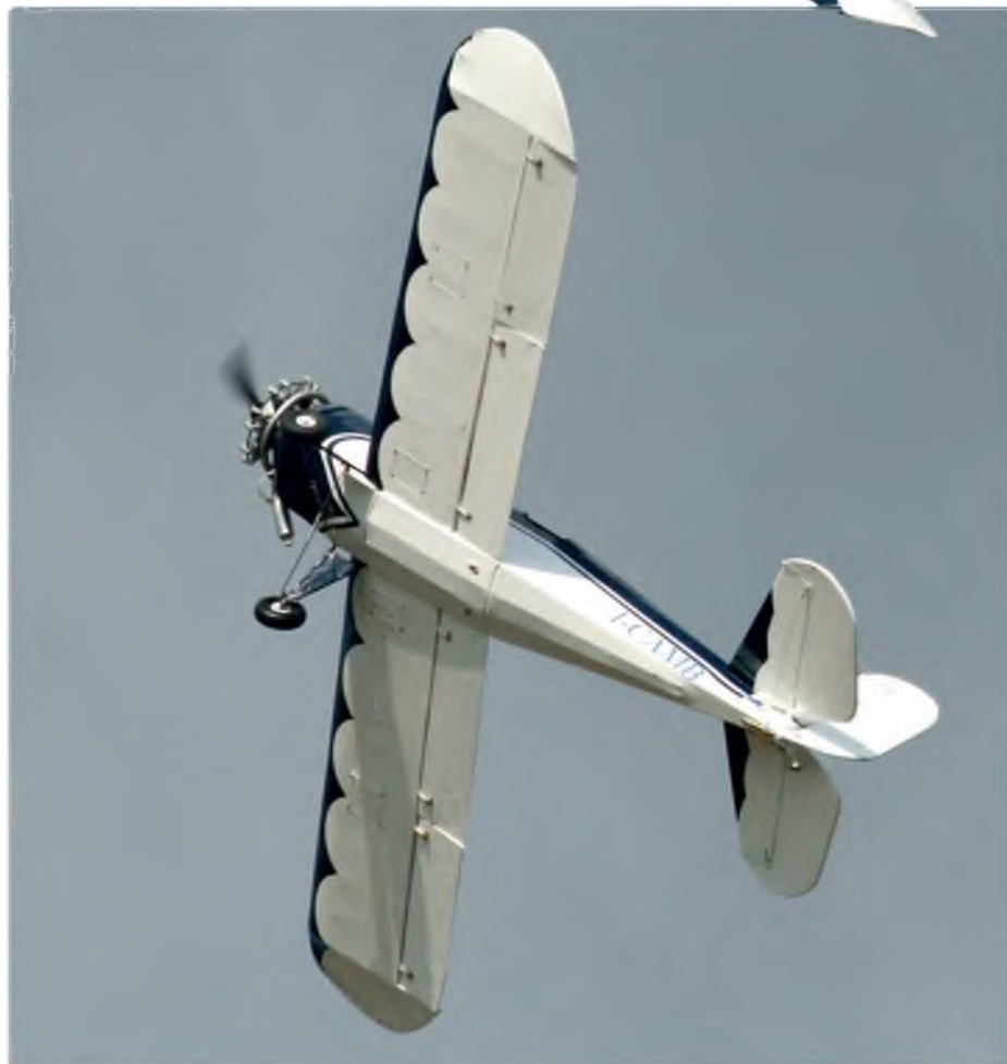
LoCamp's wing incorporates slotted flaps and Frise ailerons
