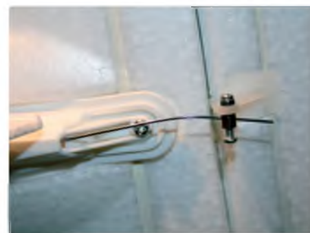
The tailplane is retained using a single screw at the rear of the tailplane mount. Elevator connection is via an EZ link – be sure the screw is nipped up tight!
