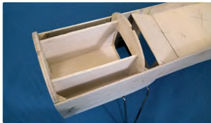
Detailed view of tank support box. Note triangular stock in corners
