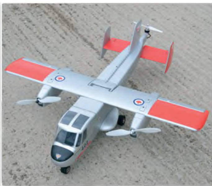
With the wing level the CL-84 converts to a conventional fixed wing aeroplane
