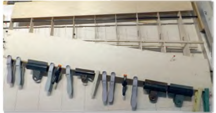
Stage 4 – LE sheeting clamped in place
