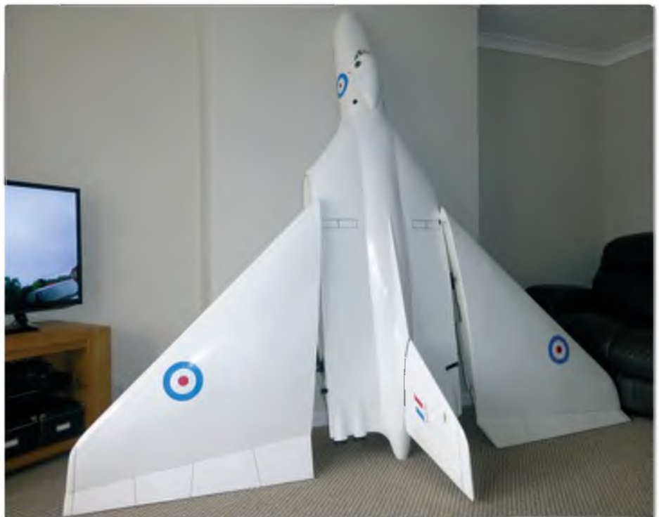
My large Vulcan bomber has a wingspan approaching eight feet and is powered by a single 120 mm fan running on 10S LiPo battery pack
