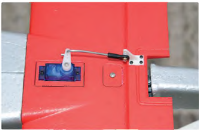
The elevator linkage was moved down a hole on the horn to increase the control throw
