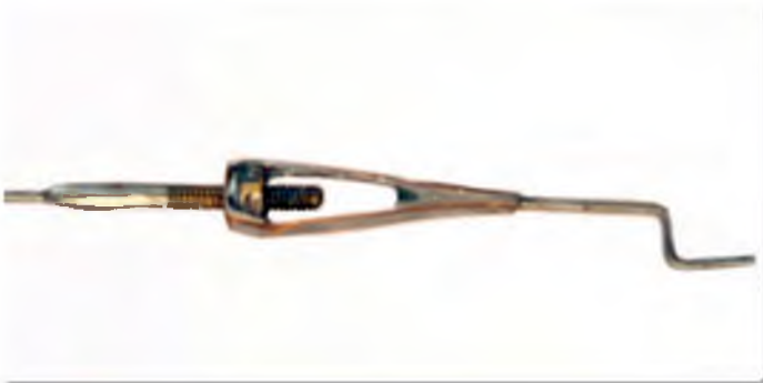
Homemade pushrod adjuster used at the servo end
