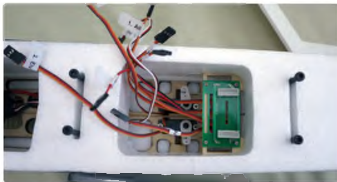
This neat PCB board provides the receiver hook up to the wing servos and LED lights. All leads are labelled to speed things up
