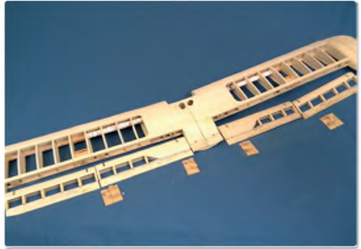
Complete wing ready for covering. The shrouds have not been glued into place yet
