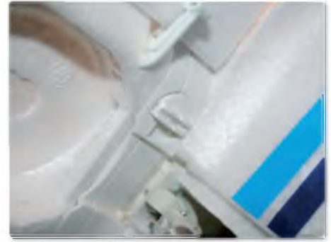
Turning two twist locks by 90 degrees clamps the wings panels firmly in place
