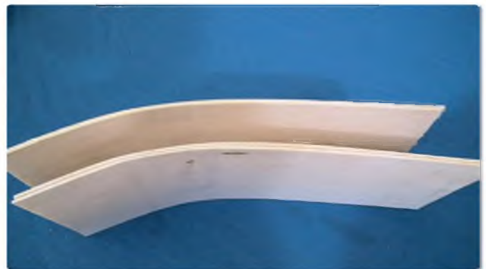
Roll supported balsa to form the sheet for the tips, ready to be cut to shape
