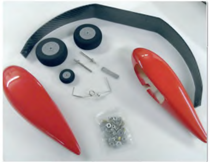
Carbon undercarriage and parts just prior to assembly
