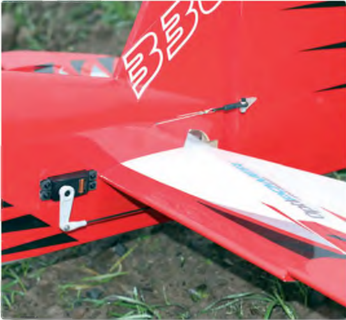
The finished elevator and rudder linkages ensure large and positive control movements. Perfect for 3D and Freestyle
