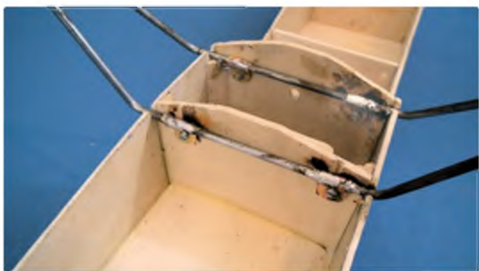
The undercarriage is bolted to the ply formers with brass 'P' clips that are soldered to the wire after bolting them in place
