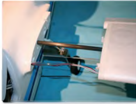
Wing panels are joined using a carbon rod. The aileron and light leads pass through a hole into the cabin. The wire flap pushrod goes through another hole and connects to the flap servo located on the rear bulkhead of the cabin
