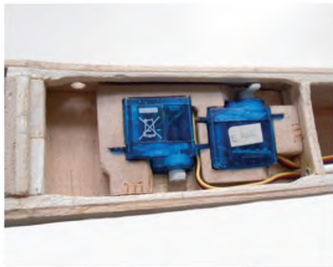
Servo tray mounted inside the fuselage
