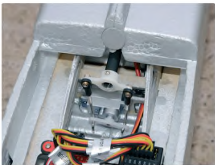
Two short pushrods need to be popped onto the ball links fitted to the rear motor control shaft
