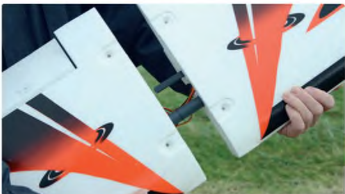
The two wing halves slot together onto a main tubular spar with alignment being assured by a smaller rectangular joiner. Clamps then hold the two halves together when the wing is bolted into place
