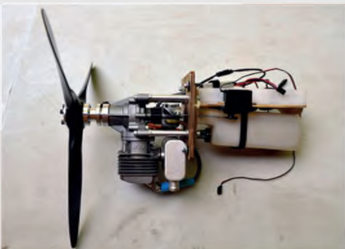
This engine, being tested prior to fitting in Jon Hancock's DC3, is a DLE 35 RA with a 590 cc fuel tank. The module contains everything to run the engine and is removed, complete, by the removal of four bolts. This allows for the assembly of the module outside of the aircraft. It also provides for the running of the engine, and its module, in the aircraft or on a simple test stand
