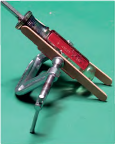
Reduce clamps denting your work by adding a pair of lolly sticks. (Yes, I know it's a screwdriver but it still shows my point!)
