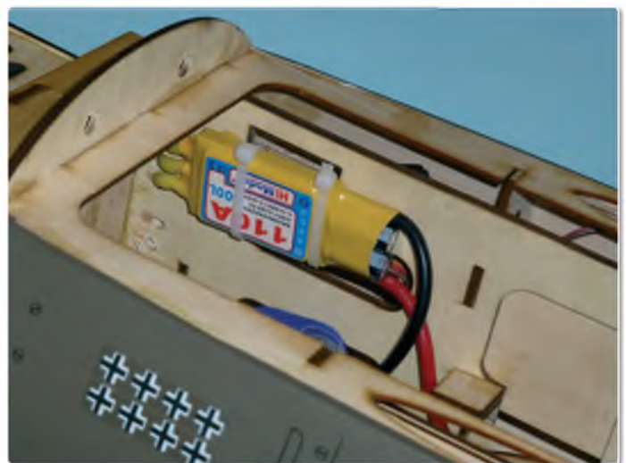
HiModel 'Cool' ESC as used in the author's Hangar 9 P-47. Rated at 110 A, it provides plenty of current 'redundancy'
