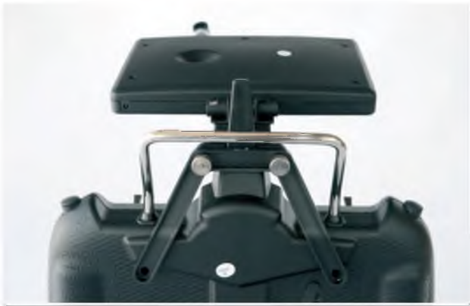
The inverted V-shaped bracket fits into a pair of holes in the back of the transmitter
