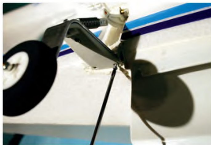
Screwing the main legs in place. The shock absorber is yet to be attached to the top mounting point
