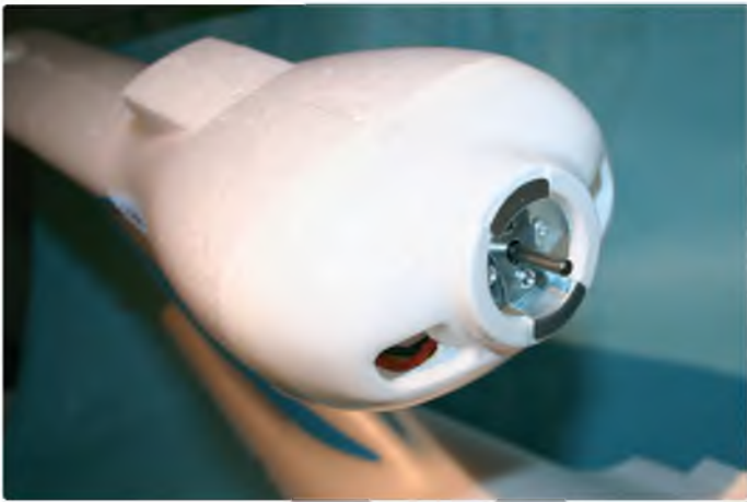
The brushless motor mount will be familiar to those of you who have built an ST Model before
