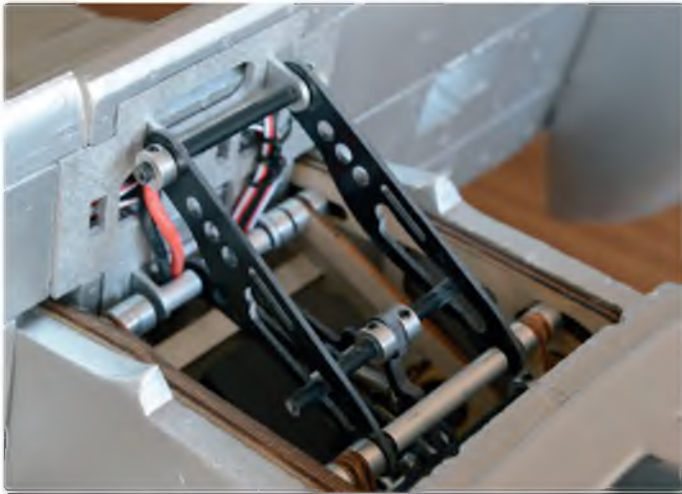
Tilt box in place after clearing out some blobs of glue from inside the fuselage
