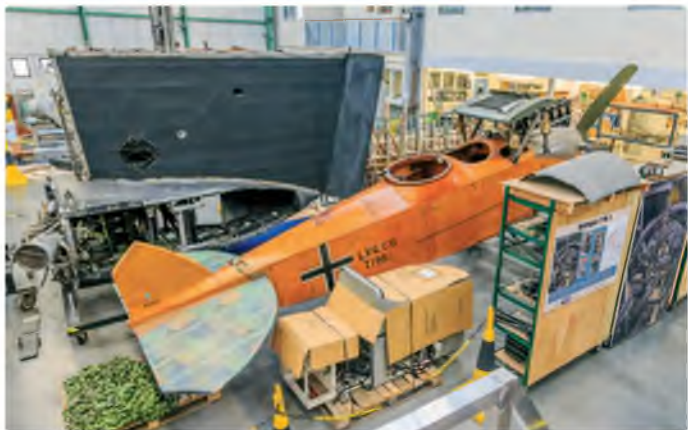
This picture was taken in 2014 before the restoration work began. One of the unique features of the LVC was its water-cooled engine. The radiator can be seen in the small bit of upper wing centre section
