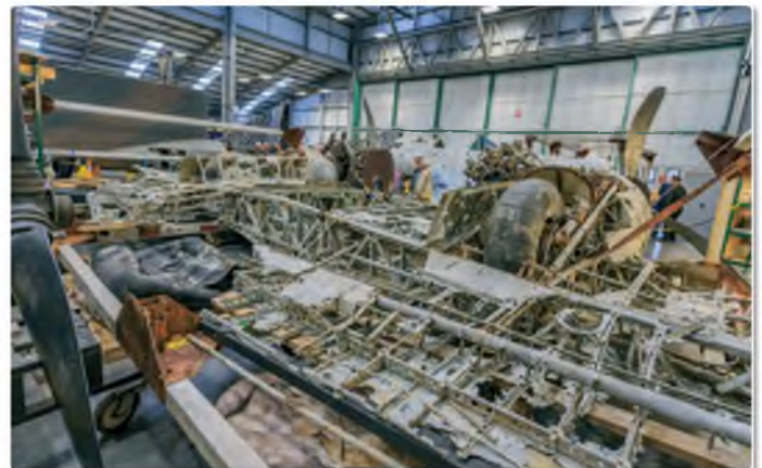
Much of the aluminium wing skin has corroded away (2015)
