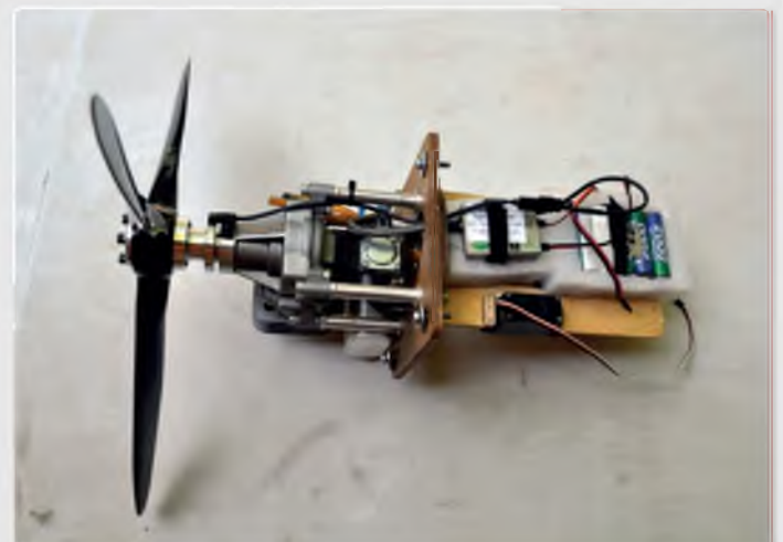
This engine, being tested prior to fitting in Jon Hancock's DC3, is a DLE 35 RA with a 590 cc fuel tank. The module contains everything to run the engine and is removed, complete, by the removal of four bolts. This allows for the assembly of the module outside of the aircraft. It also provides for the running of the engine, and its module, in the aircraft or on a simple test stand
