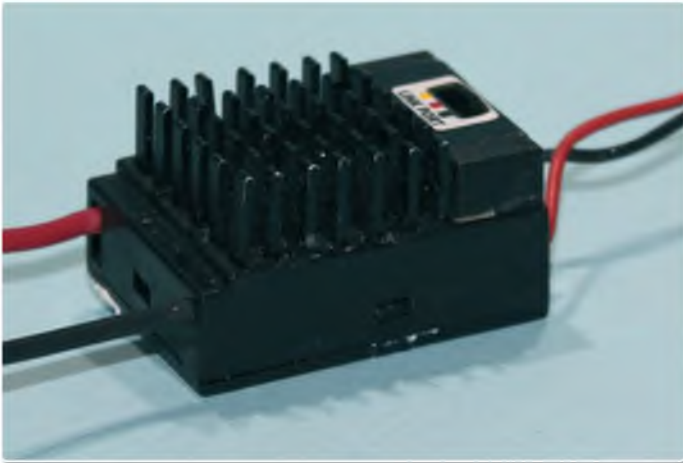
This 20 A SBEC unit from Castle Creations can be used to power receiver, servos and ancillaries, powered direct from the flight battery
