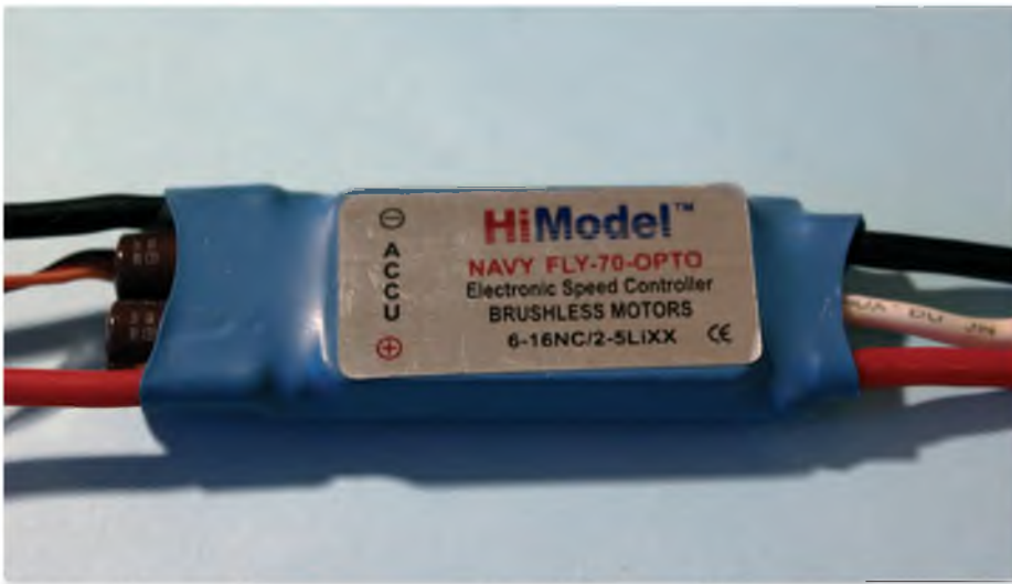
OPTO ESC's only provide power to the model's electric motor, requiring a separate power supply to run the receiver, servos and ancillaries
