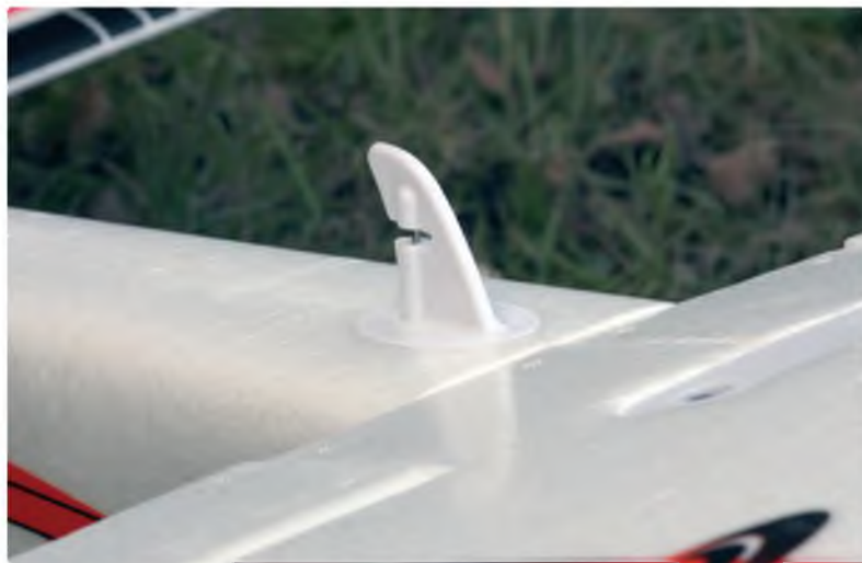
The glider tow release just behind the wing works well
