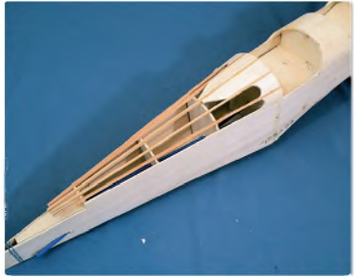
The stringers are fitted. Leave over length at the rear for final trimming
