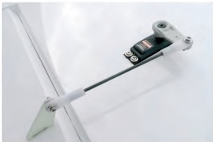
Aileron linkage complete – after opening up the holes in the servo arms to 5/64"
