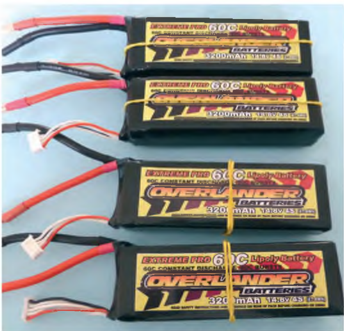
LiPo battery packs can be wired in 'series' to increase voltage and 'parallel' to increase capacity
