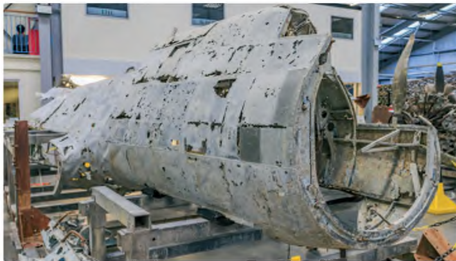
Looking at the front of the fuselage. The fuselage is inverted; this is how it was recovered from the seabed (2014 & 15)
