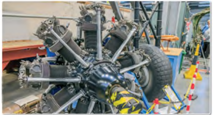
The Hampden's Bristol Pegasus XVIII 9-cylinder radial engine. Part of its undercarriage is in the background (2014)
