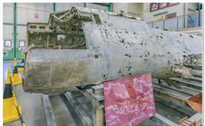
A closer look at the wafer thin aluminium skin on the fuselage. The drawing shows how the Dornier looked originally (2015)
