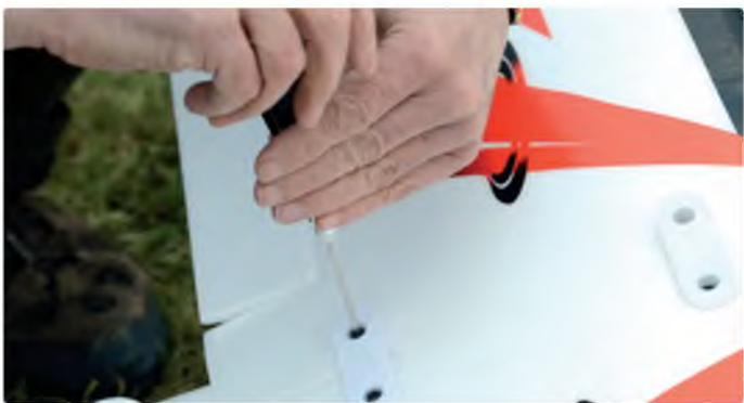
The wings are held in place with four Allen bolts that go through the two clamps that keep the two halves together
