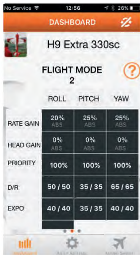
It's always interesting to get a glimpse of a top pilot's set up figures, shown here direct from the AR636 app. Note the generous Expo settings
