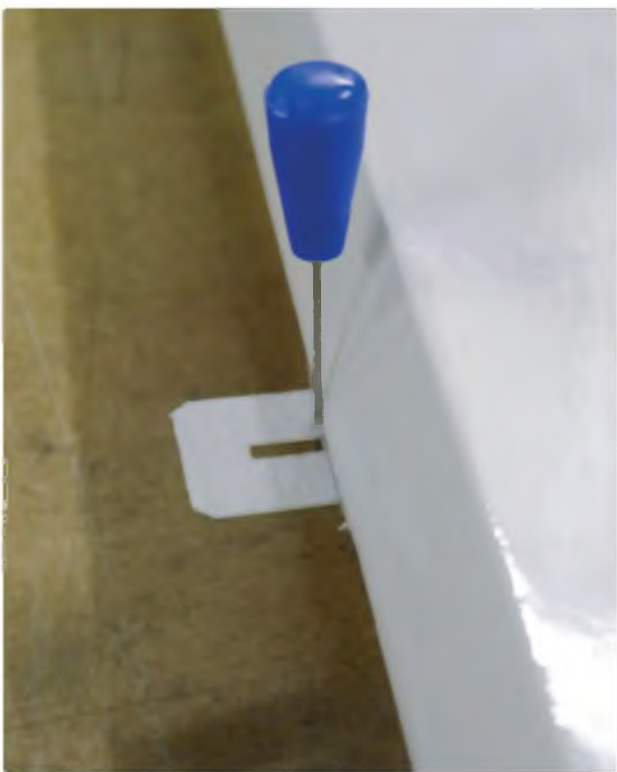
Using a pin as a depth marker stops the hinge from being inserted too far
