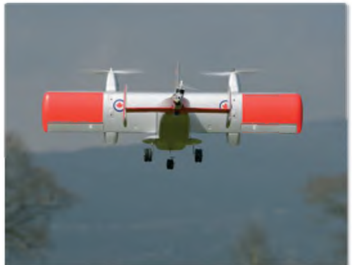
The rear motor tilts to yaw the model
