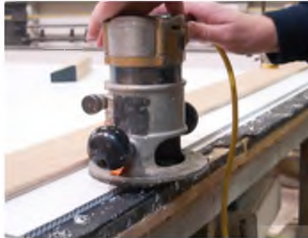
To give some mechanical strength at the ends the sides were rebated to accept them. The long edge where the top rests is also rebated, as is one side of the end panel. A router was used here; a knife would be possible but this was much quicker and more accurate
