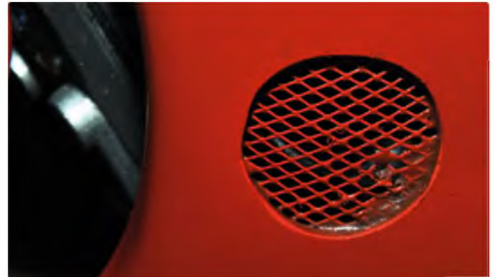
This model has a petrol engine. The mesh is to stop foreign objects from being drawn into the trumpet and it looks better than a 'black hole'
