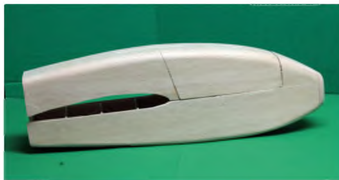
...then cut out the hatch and separate the three sections (for now)
