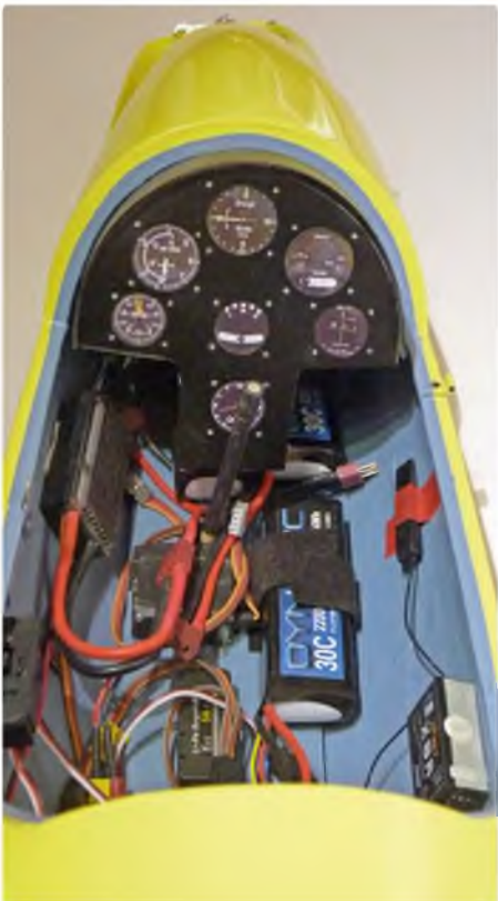
The pilot and instrument binnacle are easily removed to access the batteries. Note the animated control column
