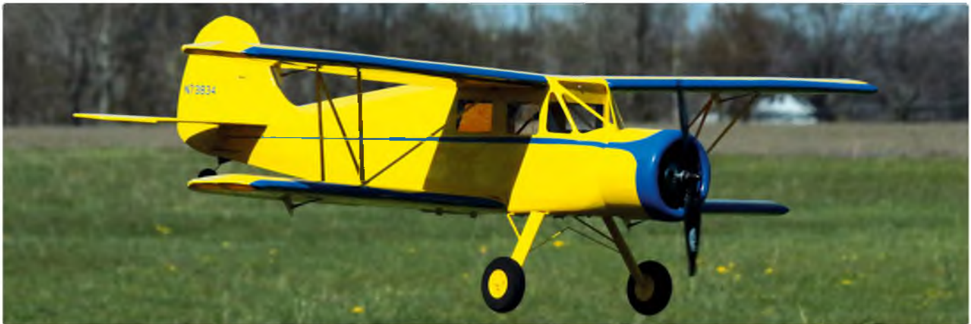
You can cover it with the same heatshrink film used on the rest of the model. Plus, a wooden cowling is easier to repair. Waco plan coming soon!
