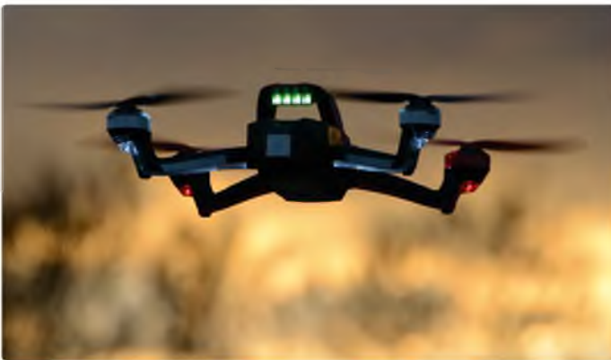
The rear LED's give you instant visual feedback
