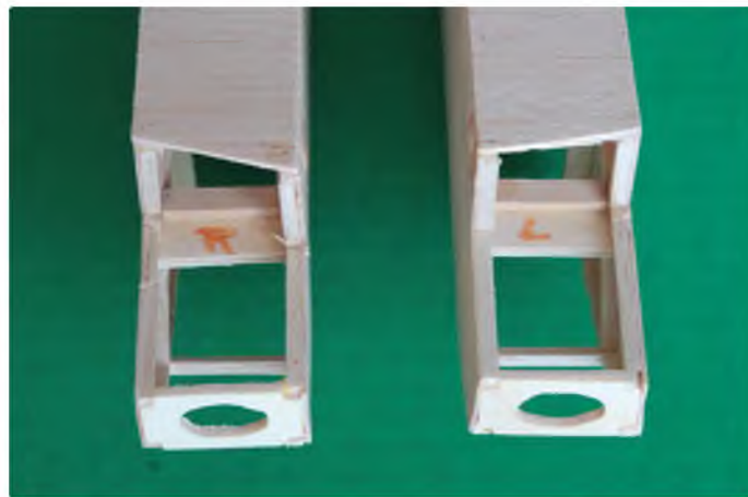
The most obvious differences in the two booms are the angles in the top sheeting and the lengths of the sides forward of the spars
