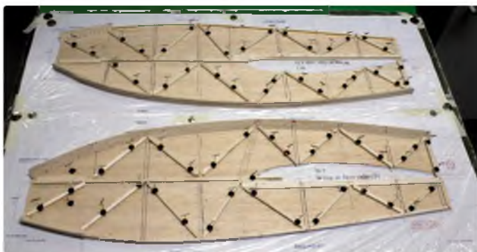
Frame up the fuselage pod the same way you did the booms...
