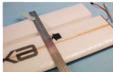
Lining up the aileron horns for a slop free assembly
