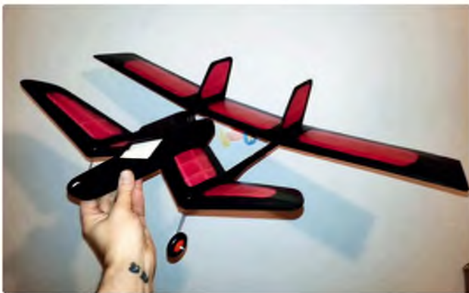
We saw Dan Mellor's 'Bonnacon' in its bare bones last time, seen here now with Dan's fine tissue covering and Tamiya acrylic paint finish. Great colour scheme as ever. By now its Irvine Mills .75 should be installed and it could be flying!
