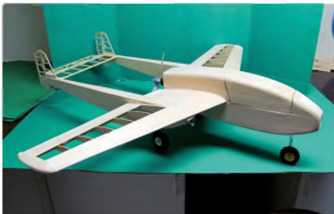
Once the pod is glued to the wing/boom/tail assembly it's time to cover and finish the gear installation
