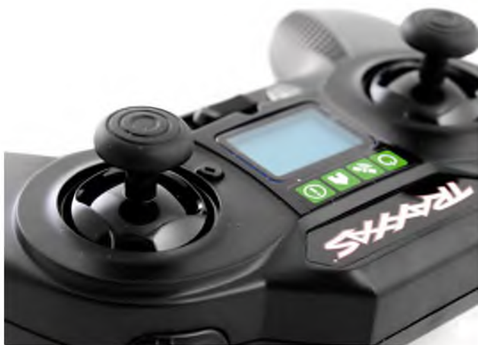
More 'traditional' style sticks can be swapped with these 'controller' ones
