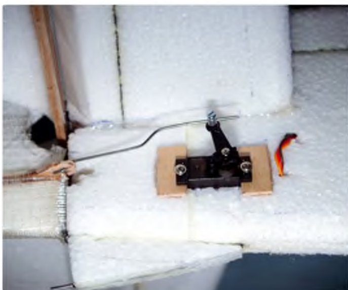
Rudder servo installation
