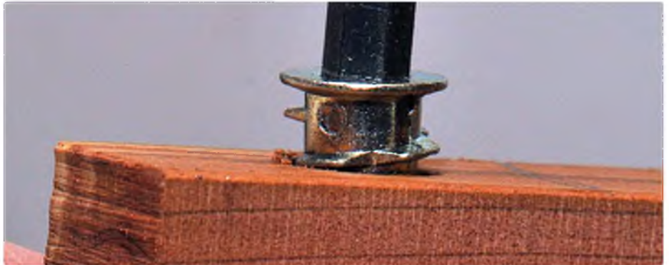
The insert is screwed in with an Allen key
