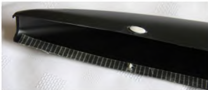
It's a good idea to reinforce the canopy with cross weave tape
