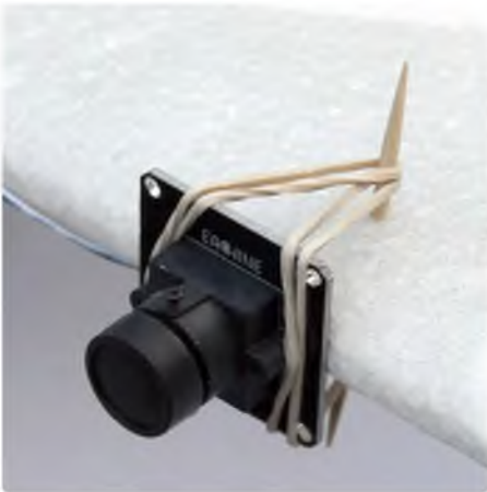
My first attempt with FPV used a camera fitted to my Flash profile foam model
