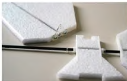
Don't omit the clear washers on the tailplane during assembly
