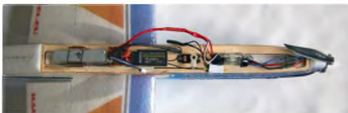
Completed equipment bay. There's plenty of room in there
