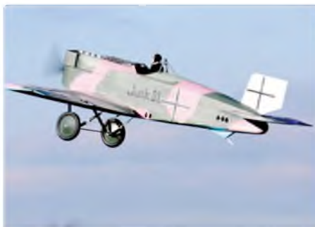
The Laser 300 V and 20" x 8" Xoar prop combination provides ample power
