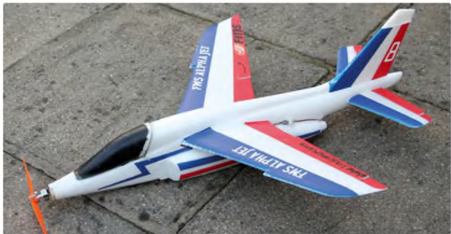
The larger FMS Alpha Jet conversion flew well with a tractor motor set up
