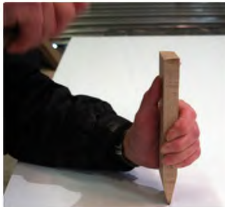
To encourage the sheet to bend along the selected flute it was found useful to create a dent in the inside surface. This blunt ended wooden chisel was created for the purpose and did a fine job
