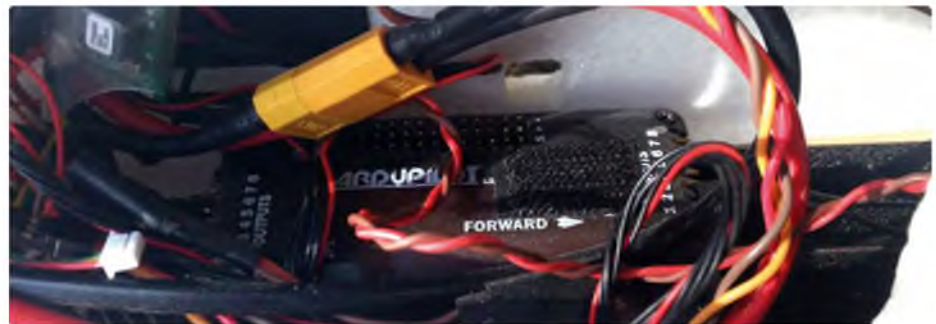
Ardupilot installed in the belly of a SkyWalker (photo courtesy of Neil Brooks)
