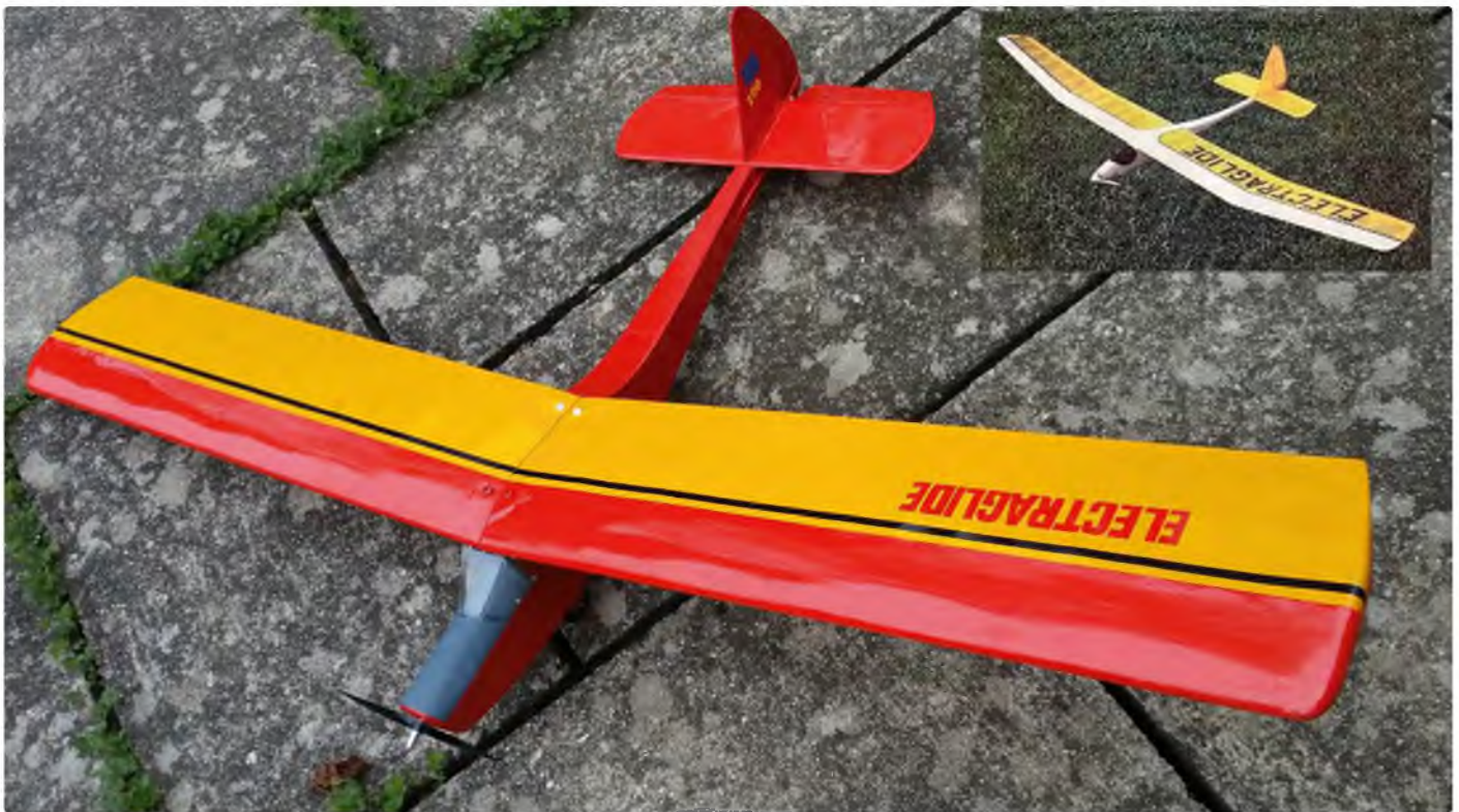
The Electraglide 62 shows off its 'stretched cabin model' lines. Simple direct drive can motor/NiCad pack power train did the job back in the day. Inset: from even later, the much larger and even more refined 'Electraglide 3'
