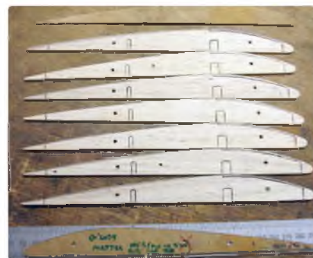
Goldberg Gentle Lady ribs. Flat bottomed from front to back, such ribs are often called Clark Y and are certainly easier to build. Look at the 1960s spar positioning – see text
