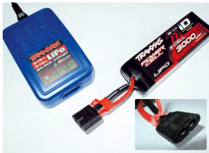
The battery and charger feature an integral balance lead so it's impossible to connect them together incorrectly
