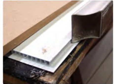
A Perma Grit tool was used to trim any surplus, or sharpness, from the cut edges
