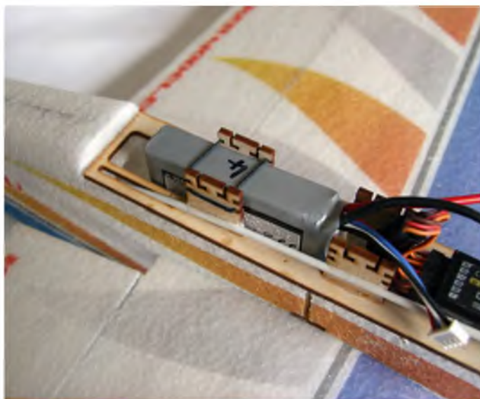
The LiPo is secured using an 'O' ring (not supplied). A great idea!
