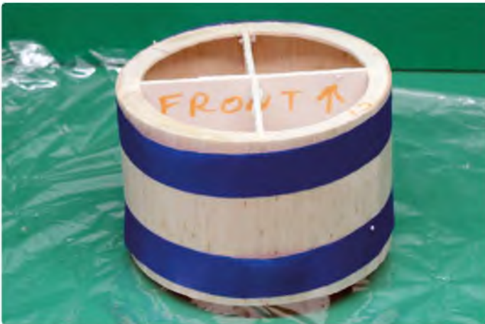
Wet the outside of the strip and wrap it around the rings, gluing as you go. Trim the end at the overlap, wrap with tape and let dry
