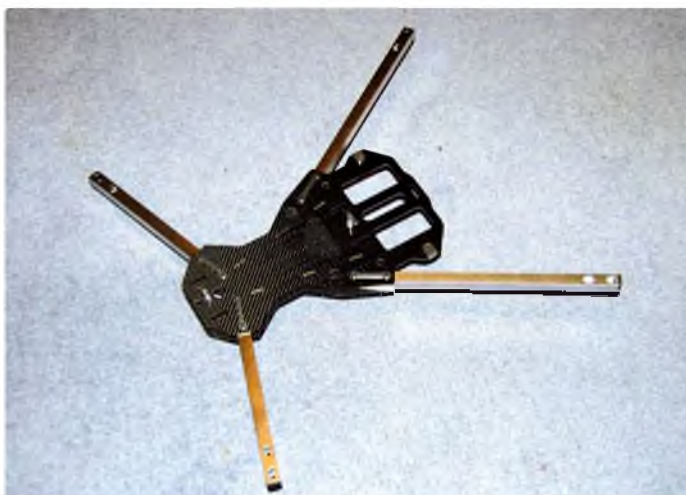
Basic frame and arms assembled ready for the motors
