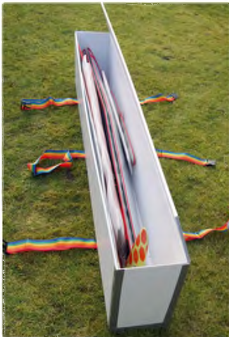
The finished box with a Maxa and a Pike Perfection inside, leaving plenty of room for more planes and equipment. The 3 x 50 mm wide luggage straps were £6 and provide useful handles, as well as keeping the top shut. For air transport the whole lid will be taped round as well
