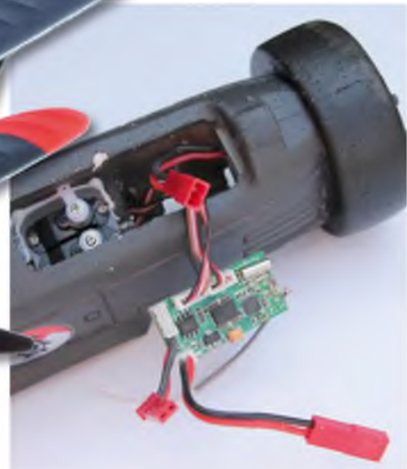
The original Rx/ESC module had to be removed
