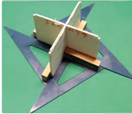
The two centre formers interlock. Use triangles when gluing to keep them square
