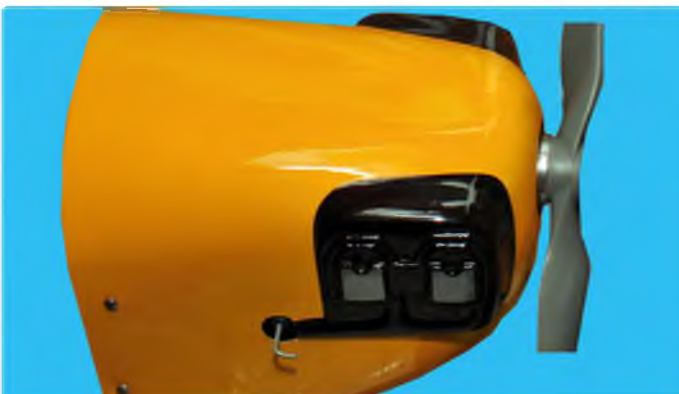
This is a replacement cowl fitted to a Seagull Cub. The screws are out of line as I had to use existing mounts on a damaged airframe
