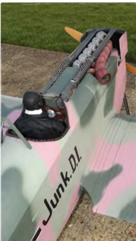
Thin self-adhesive vinyl strips are used to represent the corrugations of the Junkers' construction
