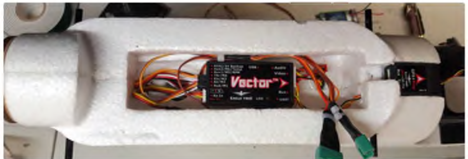
Vector installed in the ESC bay of a Skywalker (photo courtesy of Chris Blackburn)
