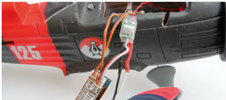
The Orange 4-ch micro Rx and brushed ESC. Note the neat gouge from a hot soldering iron!
