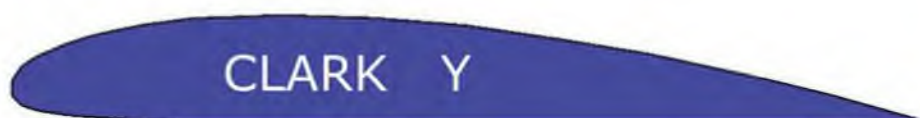
A 'proper' Clark 'Y' section. Note the upsweep to the underside near the leading edge
