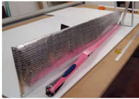
Phase 1 in the great Correx box build – checking that the fin on a Pike Perfection will fit into the chosen height (380 mm) before committing to the bending process
