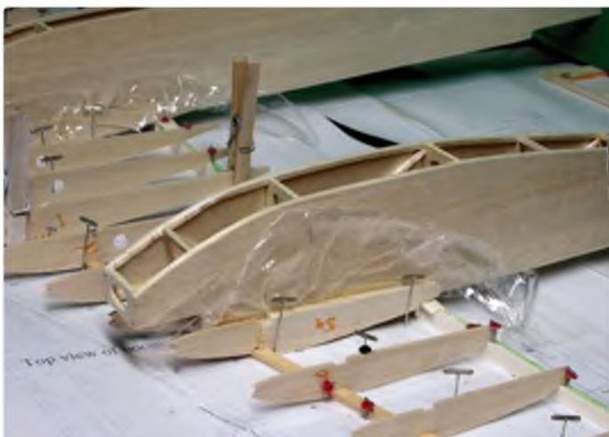
Use the booms as spacers for ribs W4 and W5/5a. Wrap in 'sandwich film' to keep from gluing them in place just yet
