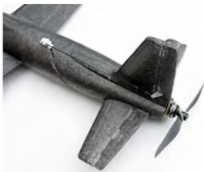
A 5 g pusher brushless motor and 1S 300 LiPo provided the power
