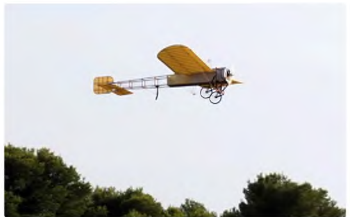
Bruchetelle's Bleriot XI, a gorgeous model with wing warping for roll function using a 30 kg servo
