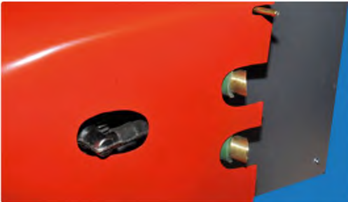
Cowl openings were cut with a Dremel sanding drum, using the template method as described for marking the retaining screws. Accurate and neat
