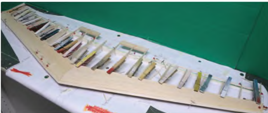
Sheet the underside leading edge before removing the wing from the building board. Moisten the wood to make it curl, then let it dry thoroughly before proceeding (slow-drying glues like aliphatic are superb for this task). All of the dihedral is in the wing bottom and the wing top is flat from tip to tip
