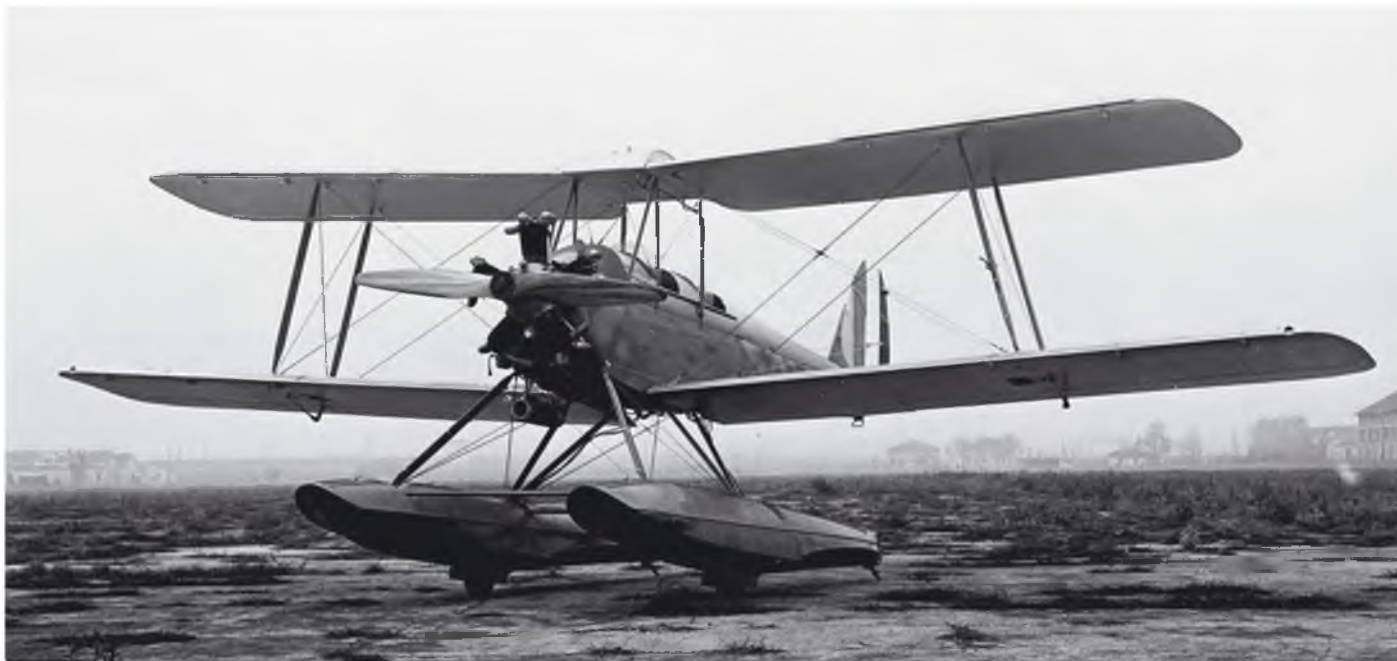
This Caproni Ca. 100 seaplane was equipped with a radial engine
