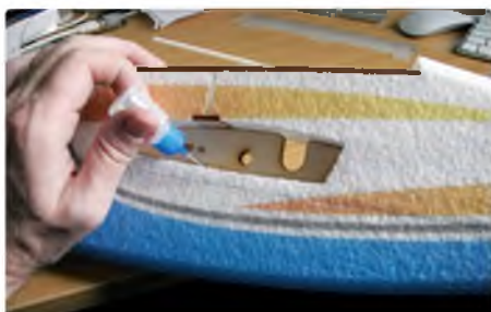
The ply central rib is easy to add
