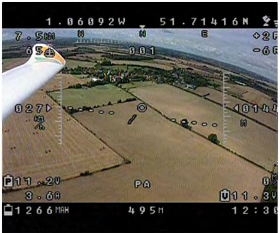
Using stabilisation to pan the camera over the wing using a Storm in a Bixler 2
