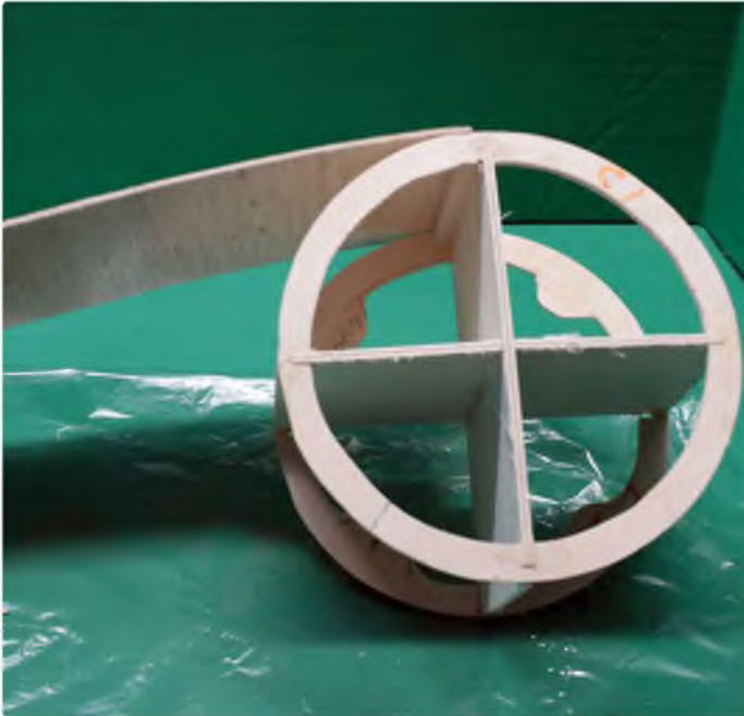
Glue the side strip to the middle of the anchor
