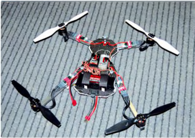
Props fitted for test flying. The residue you see on top of one black prop is from the prop number sticker that also denotes the top
