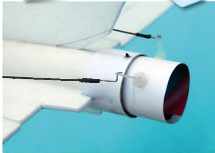
The two section tailpipe nozzle is linked to the elevon servos
