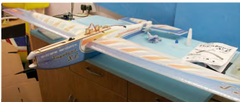
With the wings in place its time to check the alignment of the tailplane
