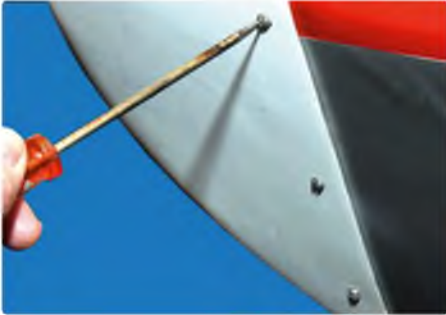
Cowl drilled and being checked for alignment. A small round file may be used to adjust minor inaccuracies
