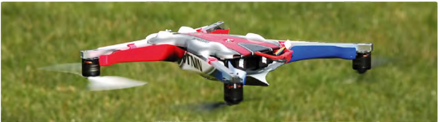
Switching into Stunt mode the motors now reverse below mid stick and you can roll or flip inverted!
