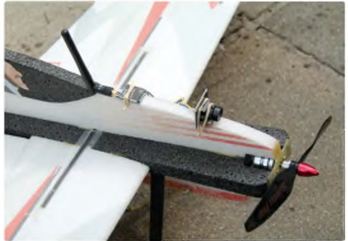
My first attempt with FPV used a camera fitted to my Flash profile foam model
