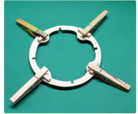
Glue scrap block to the back of the aft former to allow the sides to overlap the cowling base. Choose the block size to fit the overlap you need for your model.
