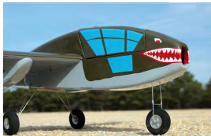
The large front hole was the engine air and cooling intake. For us it's how we cool the ESC
