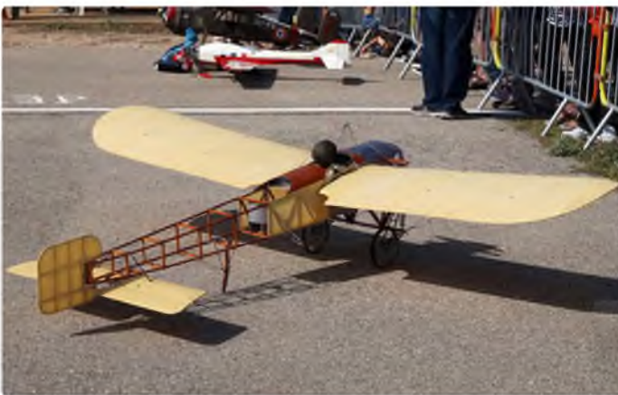
Bruchetelle's Bleriot XI, a gorgeous model with wing warping for roll function using a 30 kg servo
