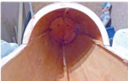
Dart fuselage interior, glassed and ready for fitting the motor
