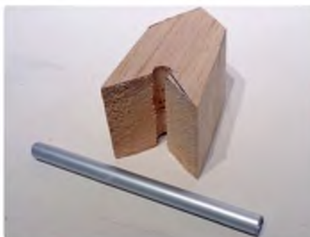
Parts for the Mk 3 Mobius stand. The short transverse tube is taped to the wing LE
