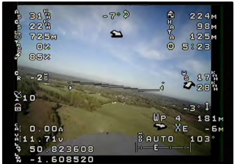
A particularly busy ArduPilot OSD configuration in autonomous mode in its way to waypoint 4 (photo courtesy of Neil Brooks)
