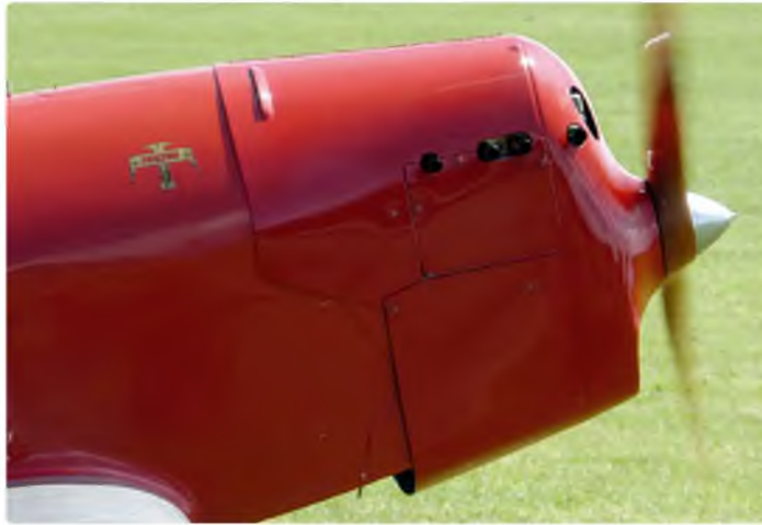
Left & below: Full size cowls can be quite complex. These two images are of a Chilton DW 1 cowl fixing and hinged top cover. It would be a challenge to make one in litho plate for scale modellers
