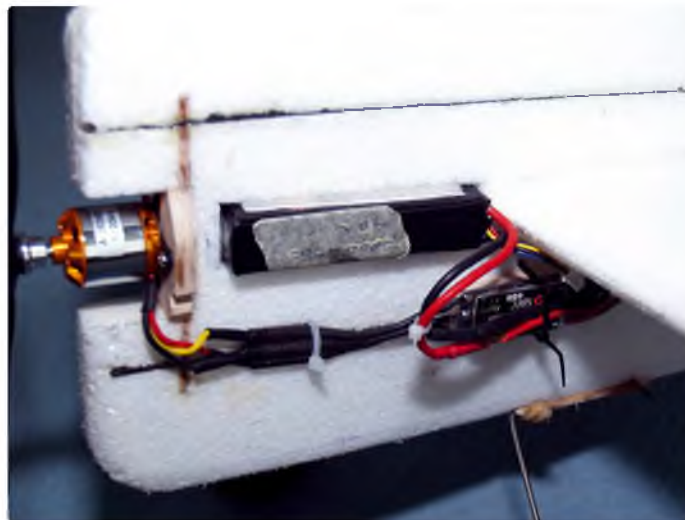
The battery fits neatly in the slotted fuselage recess
