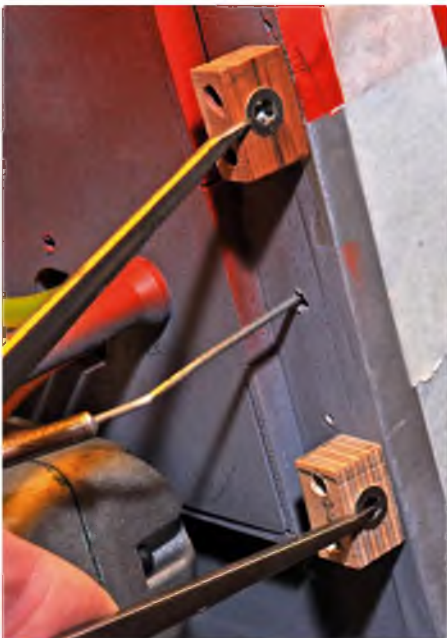
Measuring centres for the template
