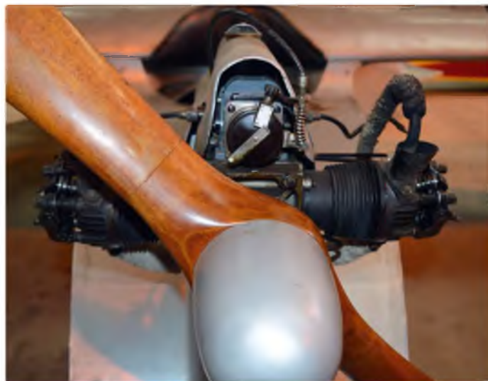
How tiny is that! The miniscule 3 HP A.B.C. engine that, 90+ years on, still gets the Wren aloft – but only just!
