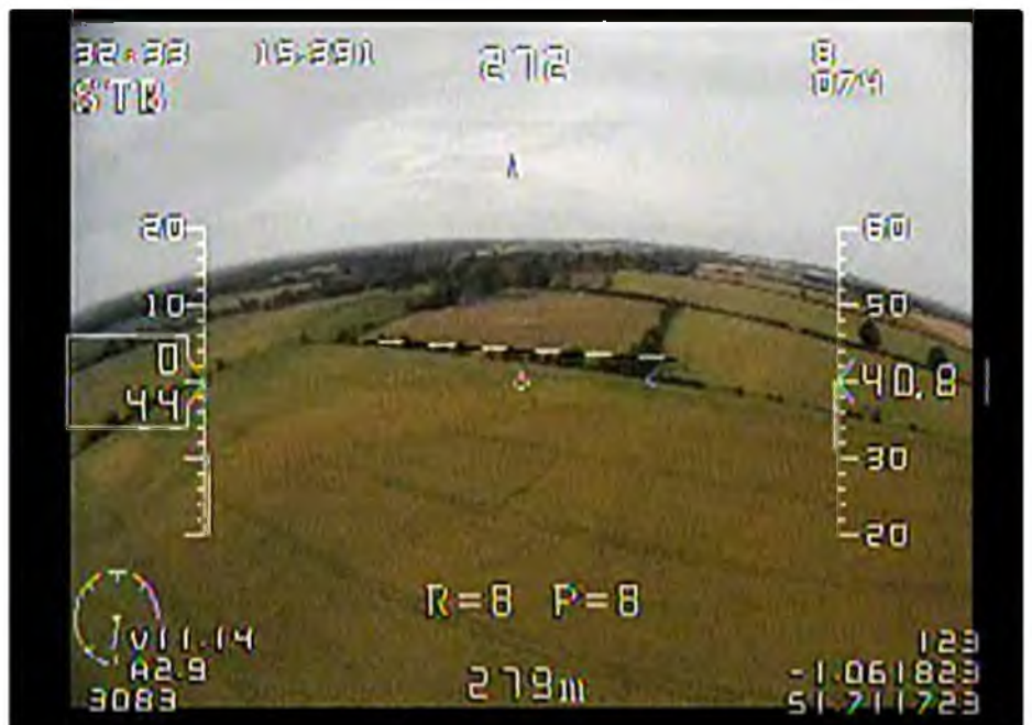
Using the MFD and adjusting the roll and pitch gains whilst in flight
