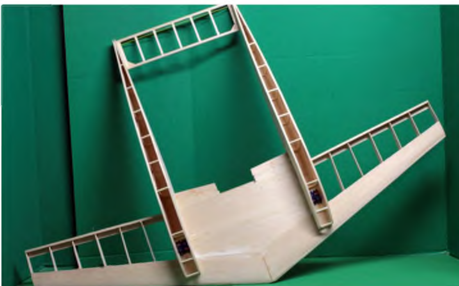
Outboard servos each drive the aileron on their side. Pull the servo leads to the centre section, then sheet over them. Later on we'll cut access holes and pull them out
