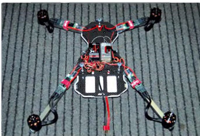
Installation complete, ready for binding and then motor direction testing
