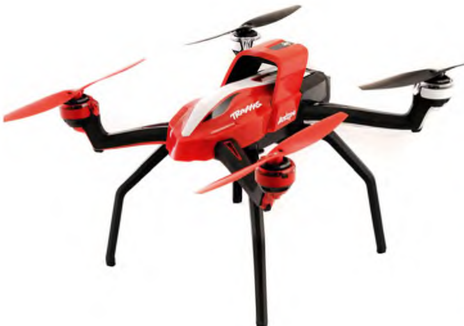
The legs on the Aton are quite long, meaning there's plenty of ground clearance when a camera is mounted
