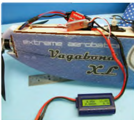
Before flight always check the power with a Watt Meter
