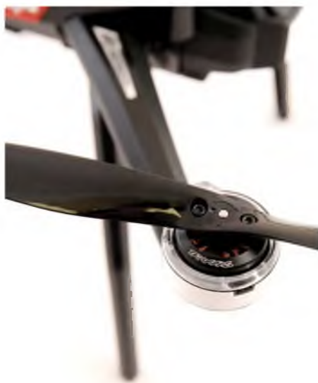
The legs on the Aton are quite long, meaning there's plenty of ground clearance when a camera is mounted
