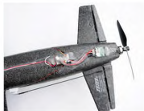
The motor, ESC and Rx can be seen in this photo
