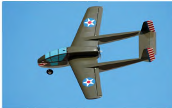
Belle will hold knife-edge attitude well but she won't maintain altitude. Please note: the US star on a wing always points forward. On a fuselage, one point always points upwards. It is as annoying to US modellers to see the stars backwards as it is for Brits to see the Union Jack upside down!
