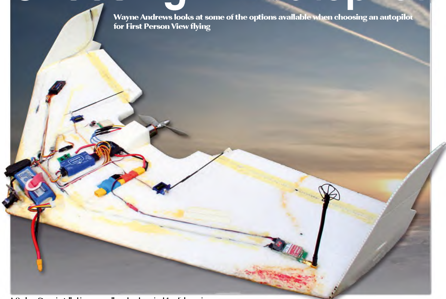
A Cyclops Storm installed in a very well used and repaired 1 m Falcon wing
