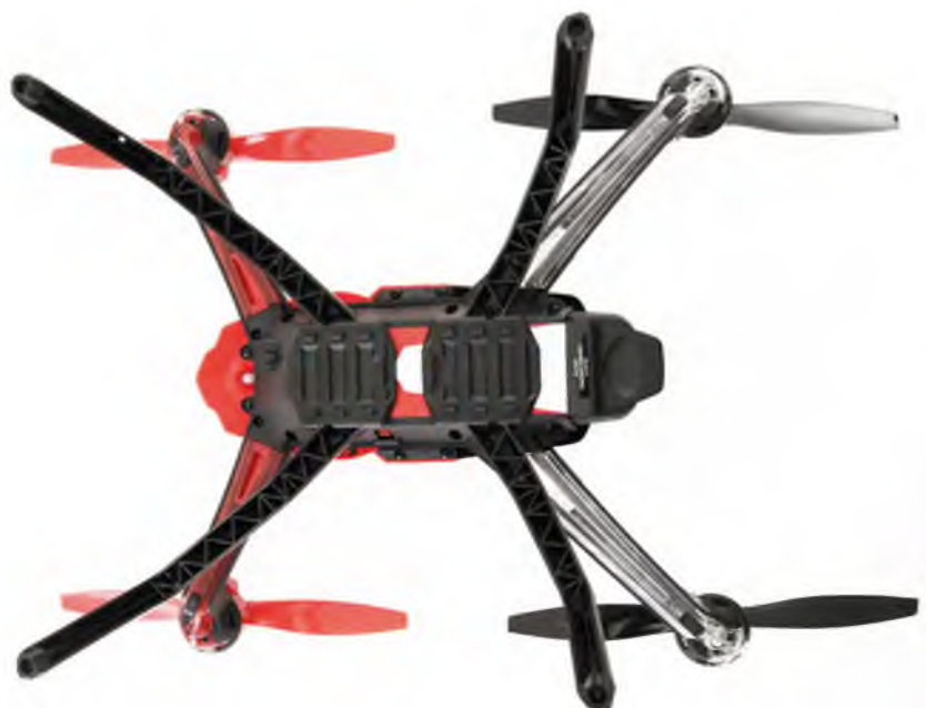
The camera mount clips into the plastic tabs on the underside of the model
