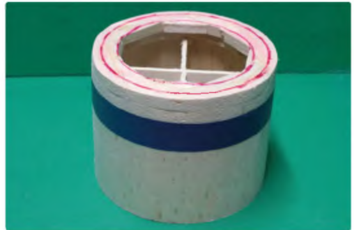
Masking tape protects the sides whilst we sand the front block. Rings mark the desired outer and inner edges of the 'peak' of the cowling
