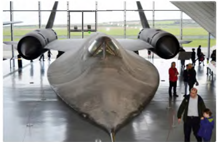
Another plane with the well-earned label of 'Icon' – the SR71 'spy' plane. Fantastically fast, it leaked fuel like a sieve until at service temperature!
