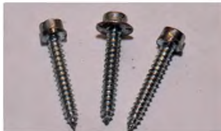
Ground down screw heads to fit the recesses. In the centre is the original screw
