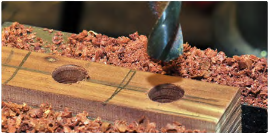
Drilling holes in hardwood for the flanged inserts
