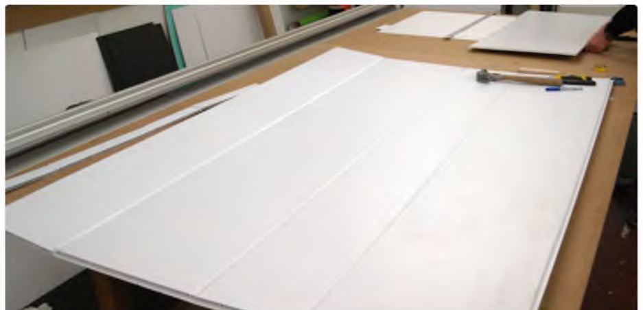
The sheet has been folded here and then left to return to the flat, which it has no hesitation about doing! Sensible people would do this bending somewhere warm, or wait for summer. Neither applied in our case, of course!
