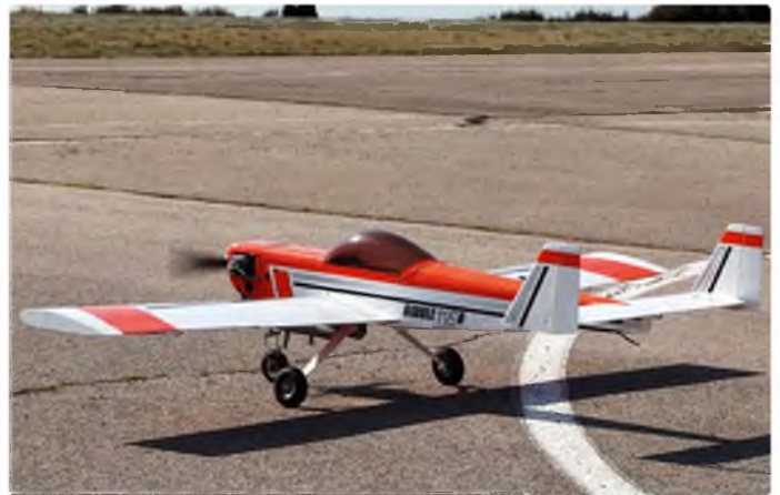
Bidule 11G flown by Bernard Claret, Chairman of LAG Helicopter Airbus. It is fitted with a DLE 116 petrol engine
