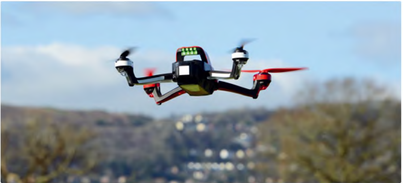
LED strips help to see the model in low light conditions
