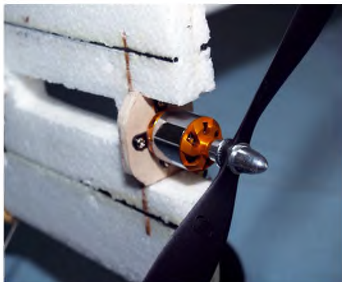
An inexpensive A2836/7 1120 KV (200 W) brushless motor was used to turn the 11" x 5.5" slow-fly prop
