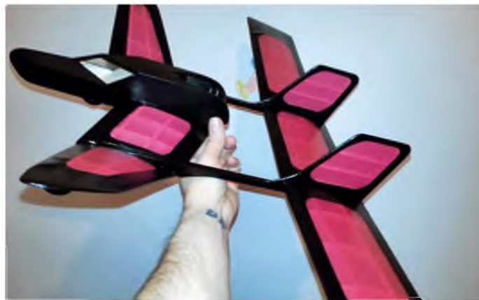
We saw Dan Mellor's 'Bonnacon' in its bare bones last time, seen here now with Dan's fine tissue covering and Tamiya acrylic paint finish. Great colour scheme as ever. By now its Irvine Mills .75 should be installed and it could be flying!
