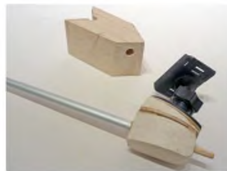
Parts for the Mk 3 Mobius stand. The short transverse tube is taped to the wing LE
