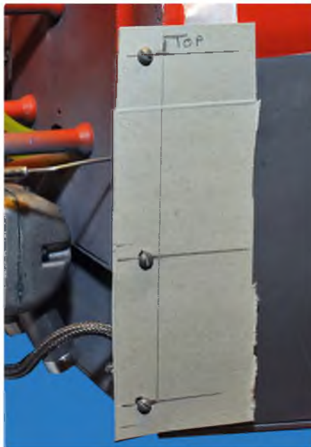
Template marked up and pierced. Test for accuracy before taping to the fuselage side
