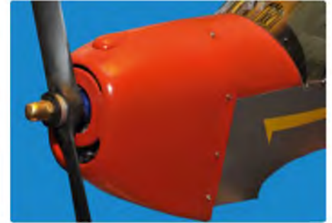
Finished cowl in place. It was painted only after all the holes had been made
