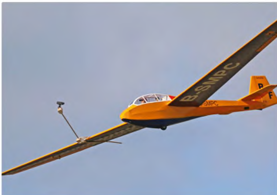
The 'high' camera mount being used on Smallpiece's 1:3.5 scale Bergfalke II 55
