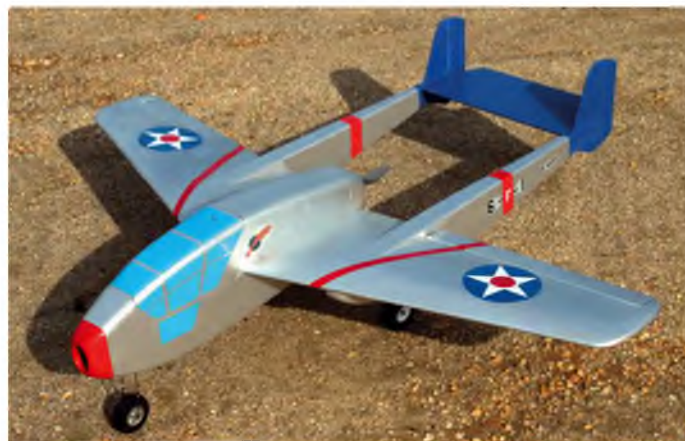
The XP-59's first set of 'clothes' was a covering of Doculam, painted with DIY store rattle-can paint. The colour scheme was based on photo of a desk model of the XP-59 in Fighting Six colours (USS Enterprise). That worked for the first flight but looked absolutely horrid
