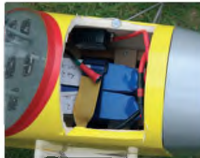
Plenty of room for twin 4S 5000 mAh batteries and a 150 amp telemetry sensor. A 10S pack could be used for more power
