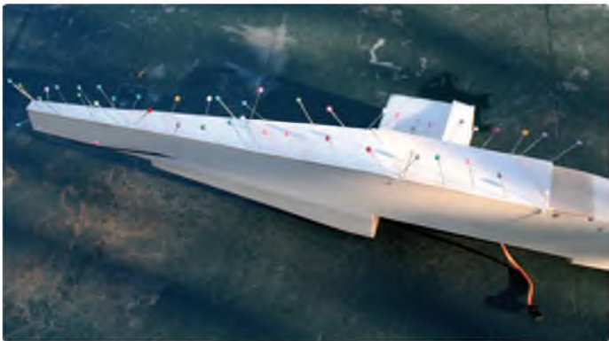
Sheet the fuselage bottom with 1/16" balsa, with grain diagonal. A 1/16" ply reinforcement is added for the undercarriage area
