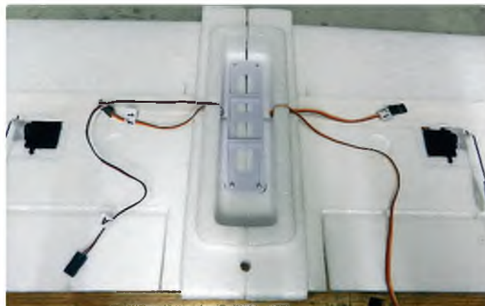
Plastic plates hold the wing panels together top and bottom
