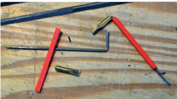
A pair of torque rod sets in the making
