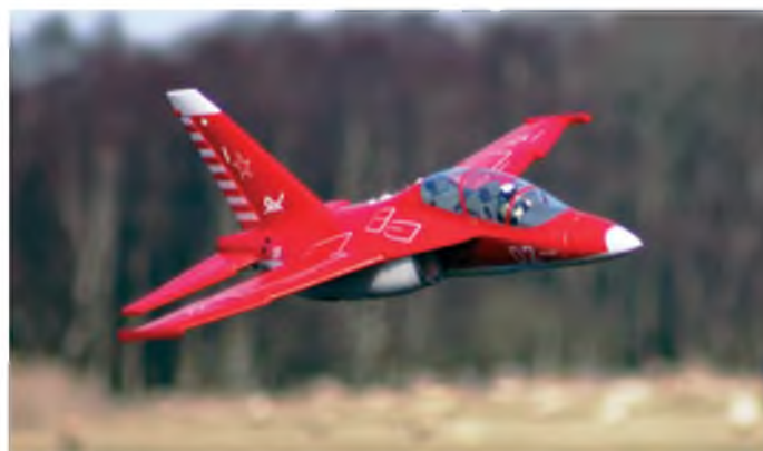
EDF foam jets offer high performance but the foam is an excellent heat insulator so good cooling is essential
