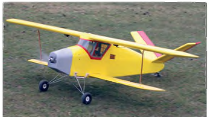
A steerable tailwheel makes taxiing easy
