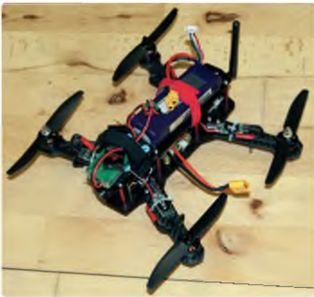
This racing quad has a top mounted flight pack and whip antenna
