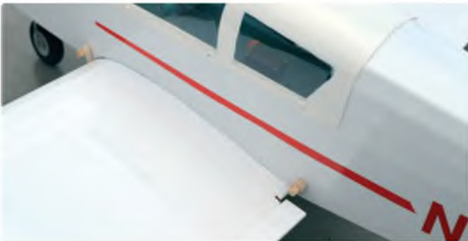
All done, with enough room for the securing rubber bands – a very practical solution
