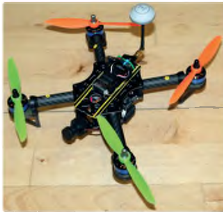
Note the domed clover leaf 5.8GHz TX antenna at the back of this model
