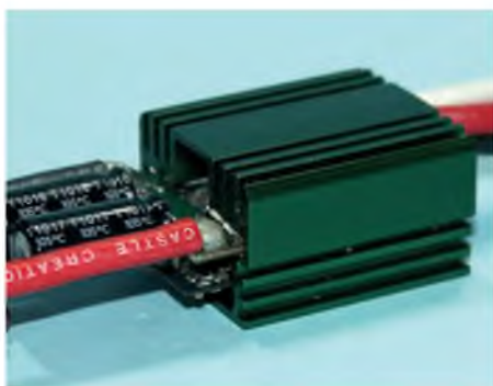
The heatsink on this Castle Creations' HV ESC fully encloses the circuitry, providing excellent cooling in the process
