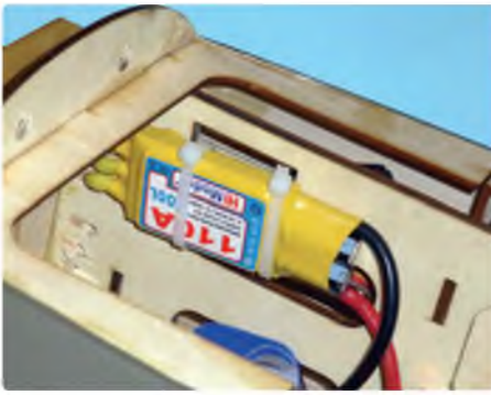
HiModel 'Cool' 110 A ESC provides plenty of 'redundancy' for current draw
