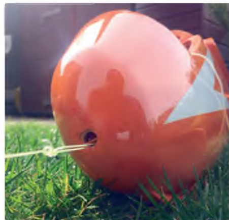
Multiplex tow release being embedded into the nose of my Mucha
