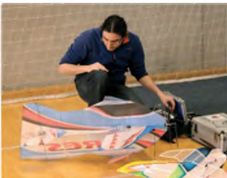
Above & below: Nicolas Pietu's model 'Ares'. A very high fuselage provided a big side area, which helps a lot in knife-edge flight. Many high coefficient manoeuvres in final sequences benefit from such construction
