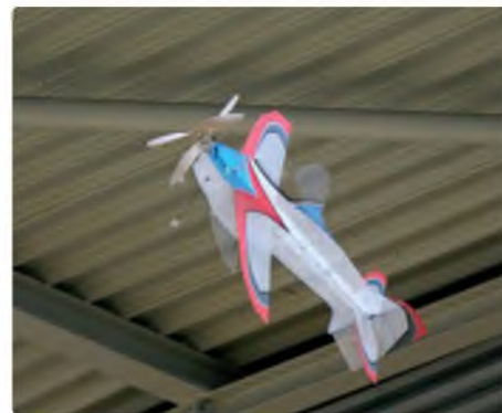
Janne Lappi's aeroplane 'Rane 2016'. With 84 cm wingspan and just 42 g RTF weight the model 'fitted' in the hall very well. The plane had no aerodynamic air brakes so all braking was provided by the 14 inch contra rotating propellers made from balsa wood
