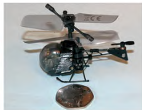
Even micro helicopters have ESCs! This one has two – one for the main rotor and one for the tail motor
