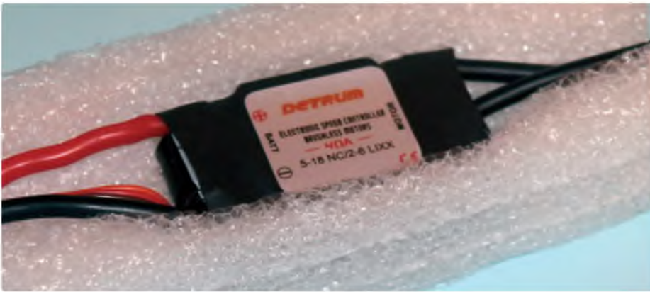
Cooling any ESC is very important. Never enclose an ESC in foam, for example
