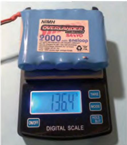
A 6-cell 'AA' 2000 NiMH battery weighs in at 136.4 g, whereas a 5 A BEC comes in at a mere 16 g – a saving of 120.4 g
