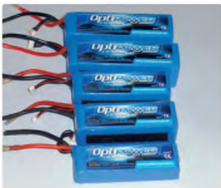
LiPo battery packs represent a considerable investment and using LVC (Low Voltage Cut-off) can stop LiPos being over discharged, greatly extending cycle life
