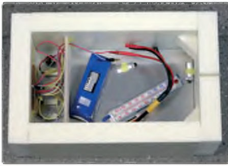
Warm LiPo batteries work better. The Finnish team use a compact heating box to keep their small 120 mAh 1S LiPo packs warm
