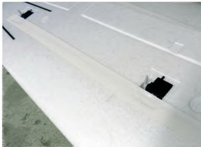
The servo leads were fixed in their grooves with dabs of hot glue and then covered with insulating tape
