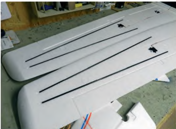
Twin carbon rods add strength but retain flexibility at the wing tips
