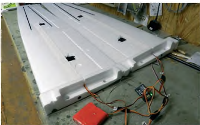
Using an old 4.8 V receiver pack to set up and test the aileron and flap linkages
