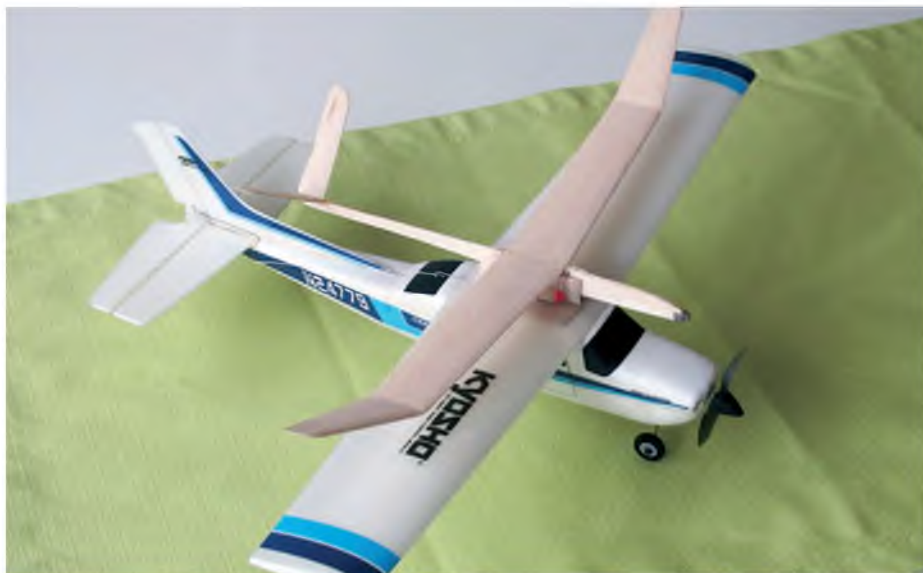
Horst Fenchel returns to micro glider piggybacking with his 38 cm span foamie Kyosho Cessna carrying a 33 cm all balsa F/F glider. Release is triggered by full rudder
