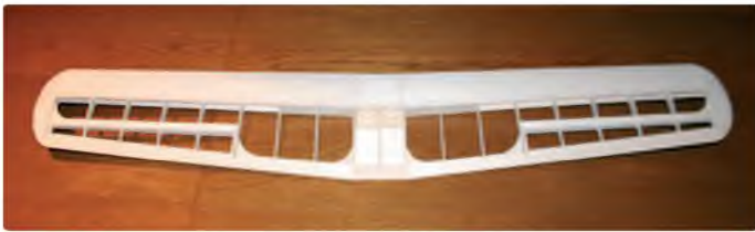
Both wings compared. The aileron wing is ready for parting off the ailerons
