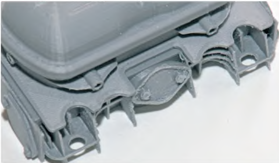
Rocker box mated with cylinder head and primed in grey paint
