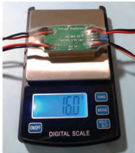
A 6-cell 'AA' 2000 NiMH battery weighs in at 136.4 g, whereas a 5 A BEC comes in at a mere 16 g – a saving of 120.4 g
