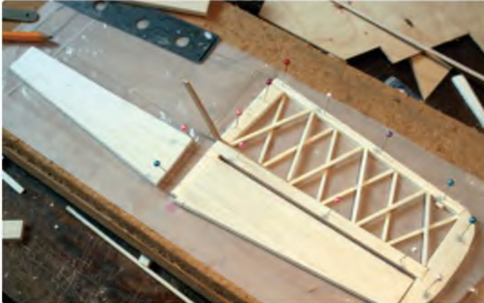
First half of tail under construction. Note the ply brace sticking up
