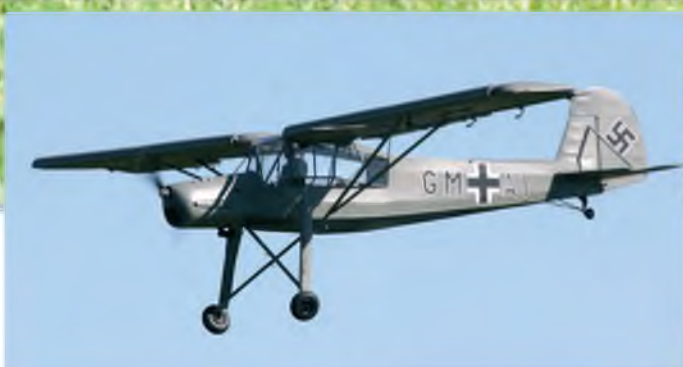
The Fiesler's undercarriage is fully sprung
