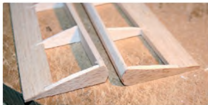
After cutting free from the wing the aileron ends are capped with 1/64" ply. Then check they fit correctly and move freely
