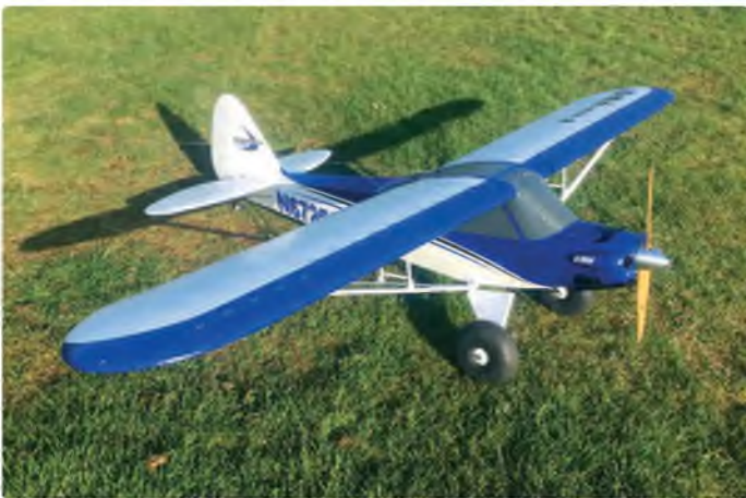
E-Flite's Carbon Cub is great for towing smaller models and comes with a ready installed tow release
