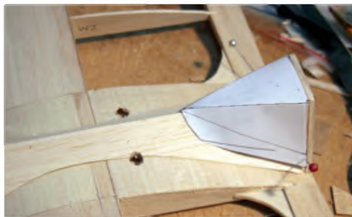
A paper pattern makes it easier to get the cockpit glazing just right
