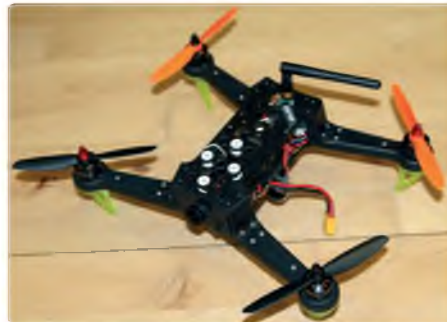
Different coloured props and spinners ensure that the props are fitted correctly
