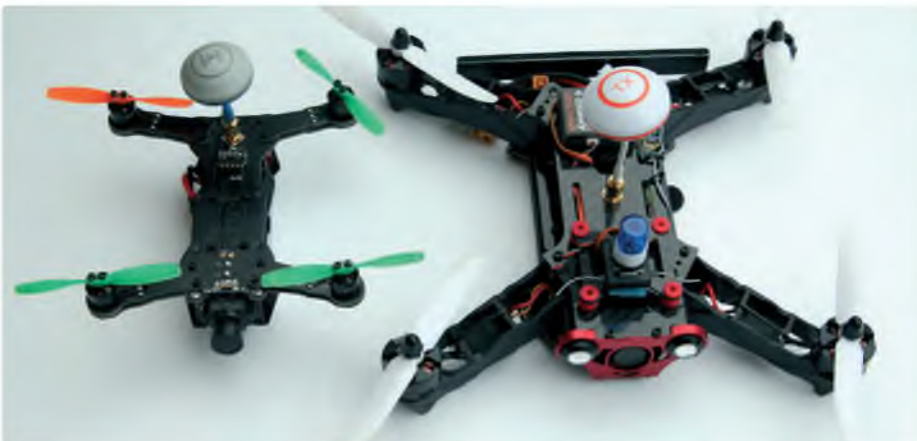
A size comparison between the 160 and 250 size racing quads
