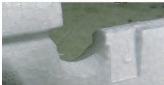
The cut-out for the elevator joiner needed to be chamfered to allow full movement of the rudder
