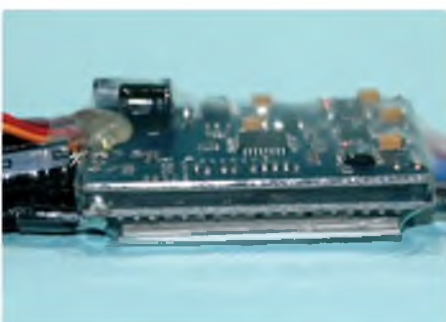
Designers often 'layer' circuit boards to save space. Great for design but not so good for cooling
