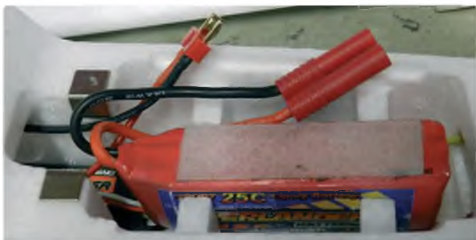
In common with most ARTF's the ESC is fitted with a Deans style connector. So Neville cut it off and fitted a matching connector to suit his LiPos. Making up a short adapter lead is another way around connector mismatch problems
