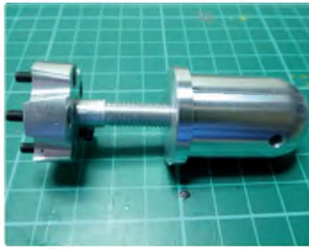
The supplied prop nut required re-tapping to fit the Dualsky prop adapter
