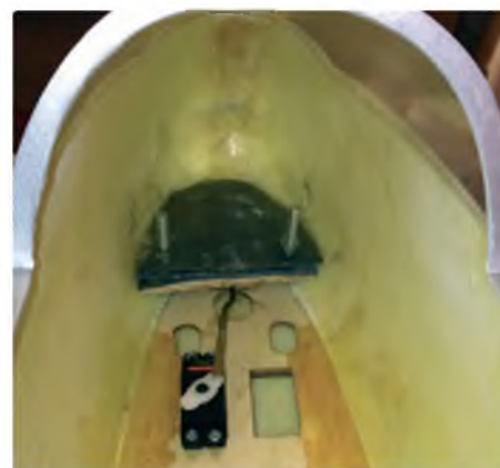
This E-Flite Blanik needed a strong link for the tow release. I replaced the stock item with better piano wire as the original bent under towing forces
