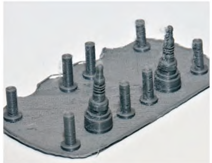
Base of upper cylinders with spark plugs and locating pillars for cylinders
