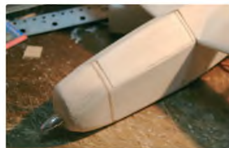
Finish sanded nose cowl and top hatch in place
