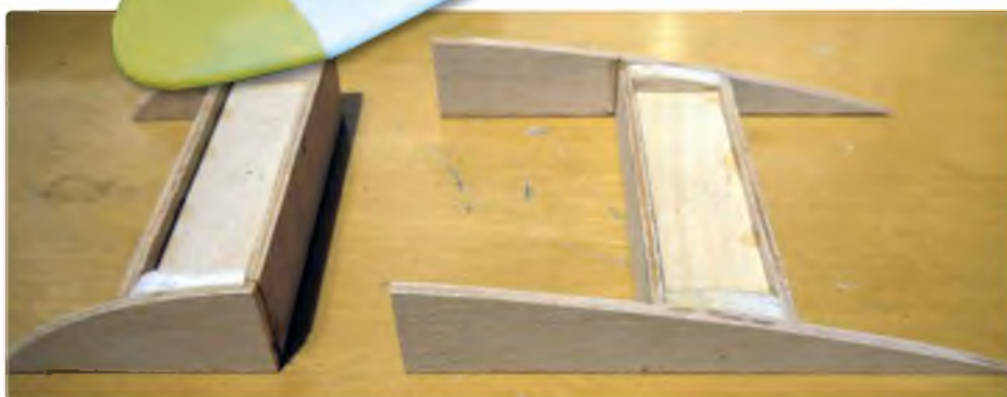
Wing centre section from 6 mm liteply doubles as the wing mount
