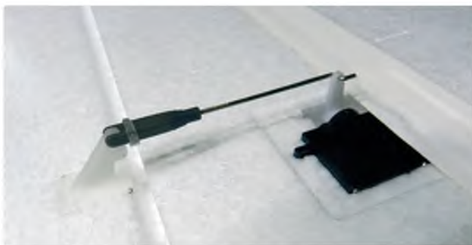
Wing linkages are short and direct
