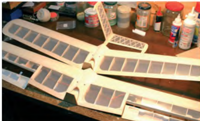
Flying surfaces covered in 38 micron document laminating film prior to tissue covering
