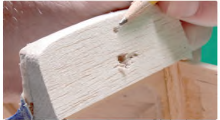
Remove the hatch. You should have a nicely marked dent in the wood, showing you where to drill. So, drill a 1/16" hole through the bulkhead. If the latch sticks drill out the hole in the bulkhead
