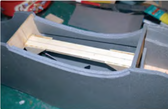
Lower wing to fuselage mount
