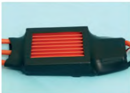
Some manufacturers cut the heatshrink tubing to expose the ESC's heatsink, which is ideal for improved cooling
