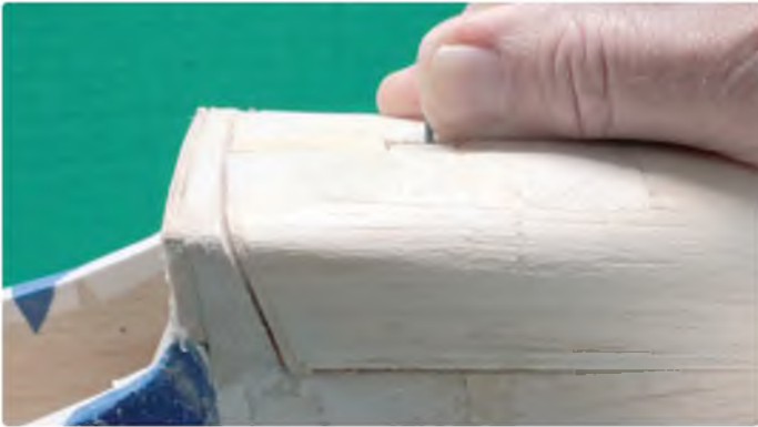
Retract the latch, put the hatch in place and PUSH the latch towards the locked position
