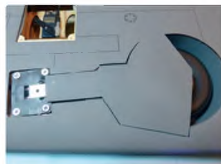
Electric retracts are available as an optional extra. Note the flap servo fitted behind the wheel well
