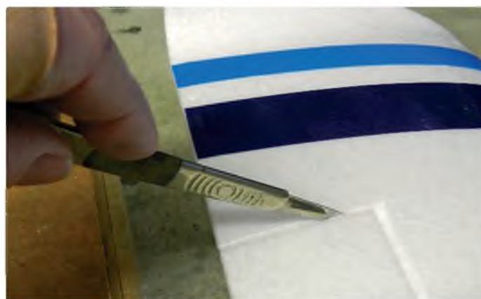
The flaps and ailerons need to be cut loose at each end using a sharp knife
