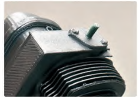
Plastic locating pin for exhaust stub. A wooden one would suffice
