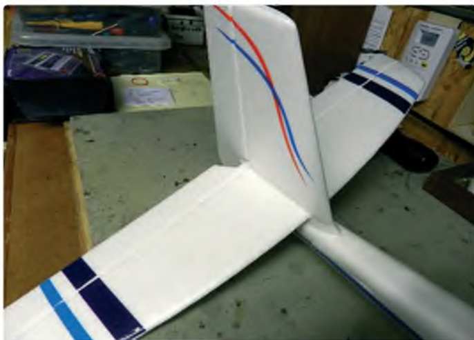
Fully assembled tail after gluing in place on the fuselage
