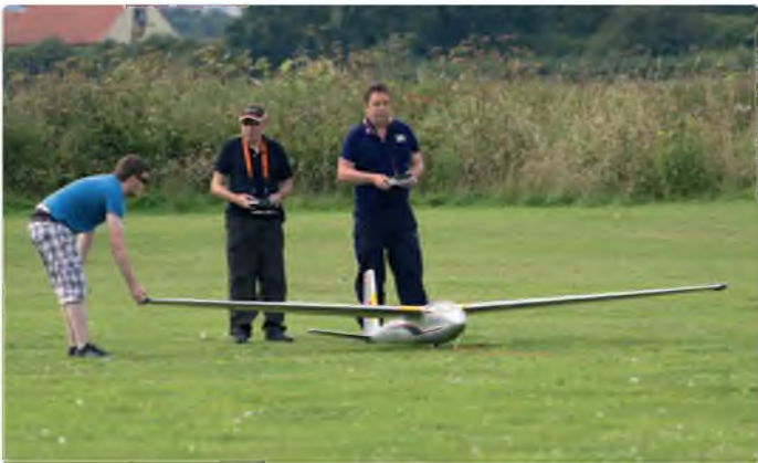
The helper should simply support the wing and release it immediately the glider starts rolling
