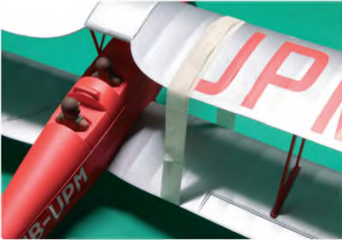
Masking tape's sticky glue would pull the paint off Micki's damaged micro foamie Tiger Moth. So I wrapped a loop, sticky side out, around the wings to hold them in place as the glue dried
