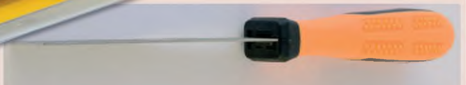
The file blades are thin and flexible
