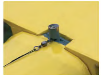
The tow hitch is a simple 'pin in tube' type, actuated by a servo in the fuselage. Note the swivel on the tow line
