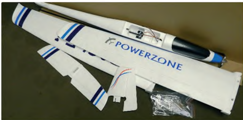
There are just a few airframe parts in the box, all neatly moulded from EPOFLEX foam
