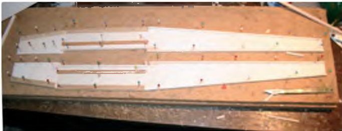
Preparing opposite fuselage sides with longerons and reinforcements
