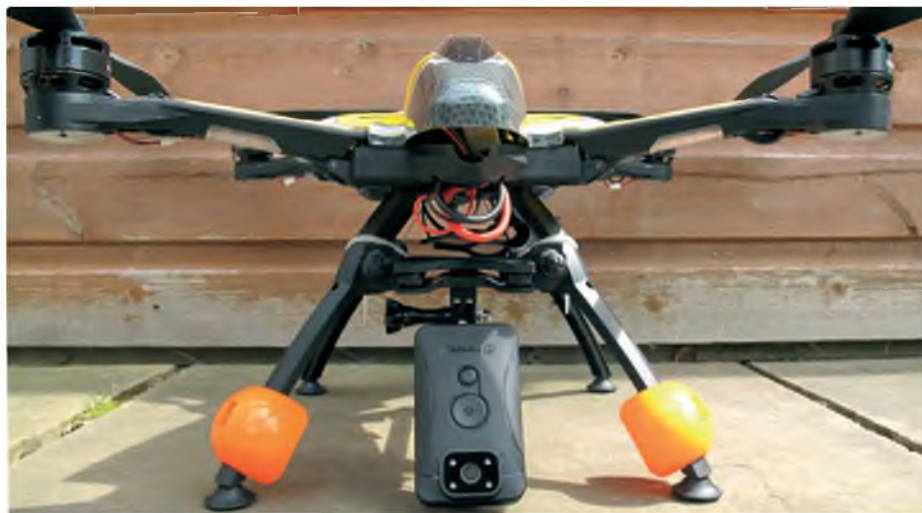
Even with the long legs of the Form500 drone the DrivePro Body 10's elongated case can touch the ground unless angled forwards or backwards
