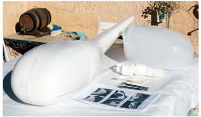
Kit contents. The precisely moulded fuselage and cockpit ooze quality. Note the horizontal and vertical lips on the front fuselage that help stiffen the structure
