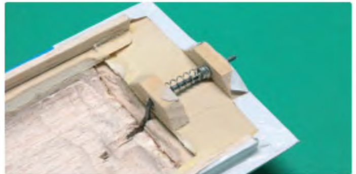
A variation on the latch mechanism is seen on the Shrike hatch. Here B1 and B2 are glued to the hatch framework, letting that substitute for plate A
