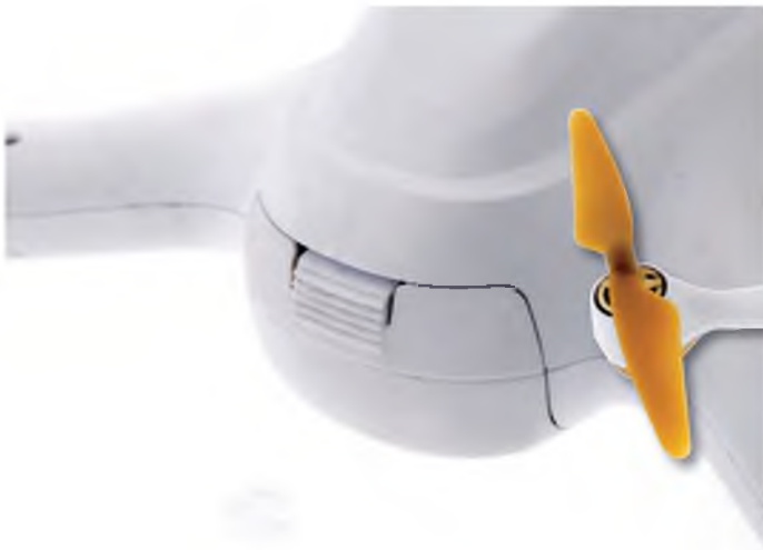
The battery compartment has a 'clip' style access panel
