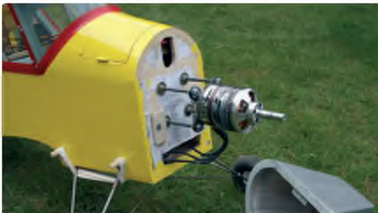
The motor is mounted on threaded studs fixed to the bulkhead with captive nuts, with a slot for ESC cooling and routing motor wires. The slot at the top is used for fuel tubes on the original model but provides cooling air to batteries in the electric conversion. The cowl is held in place with magnets and alignment pins
