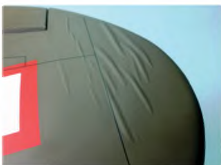
The matt covering was blistered in several places but a few minutes work with a covering iron soon cured the problem
