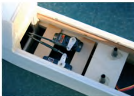
Two E-Max ES08A servos for V-tail ruddervators were installed at the rear of the wing opening and fitted with 1.5 mm carbon fibre pushrods
