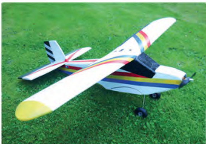
High wing monoplane, front and rear views. Note the inset ailerons and large tail end control surfaces. Also the wing blanking unit
