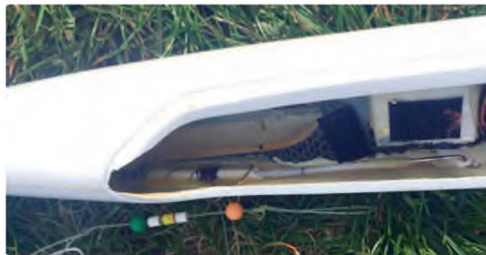
This Tangent Kult uses a simple slot and rod tow release. The outer sheath of the release is secured firmly to the fuselage
