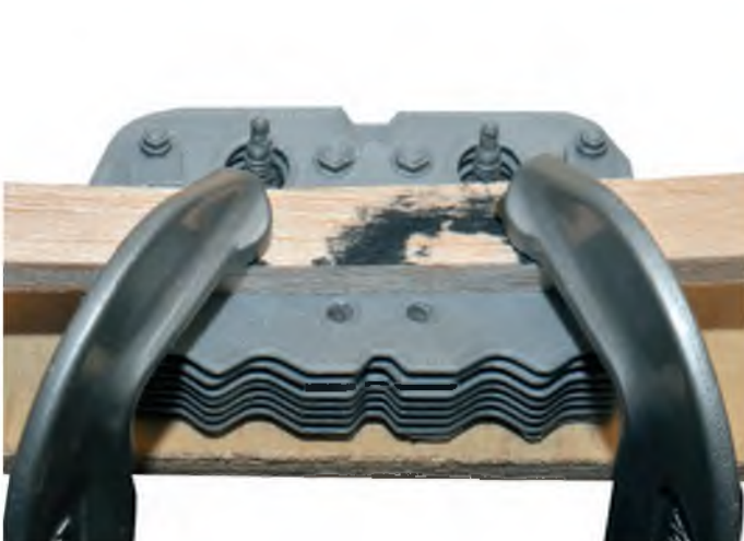
Using a balsa 'cushion', carefully clamp the cylinder shims in place
