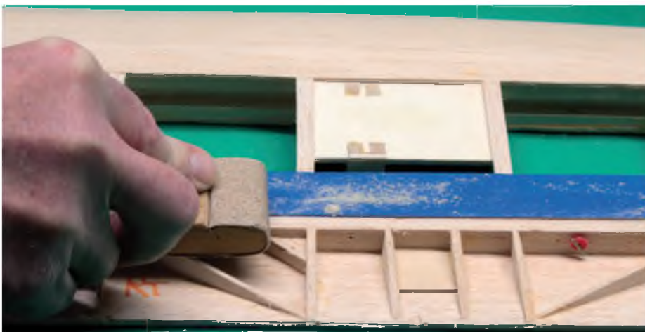
Masking tape protects soft parts when sanding. Coloured tape is good here as any sanding through the tape shows up quickly
