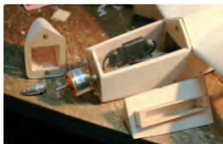
Nose cowl (note magnets) and top hatch removed. The ply box built into the hatch houses the 850 mAh 2S LiPo
