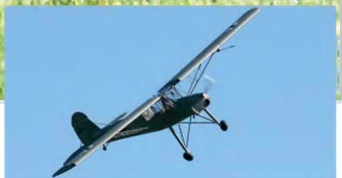
Built to quarter scale the Fi 156 has a wingspan of just over 140 inches and is powered by a 50 cc petrol engine
