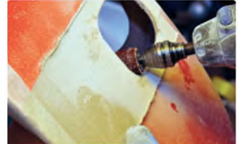
Using a template and Dremel tool to cut out the aperture in the cowl. Take care here!
