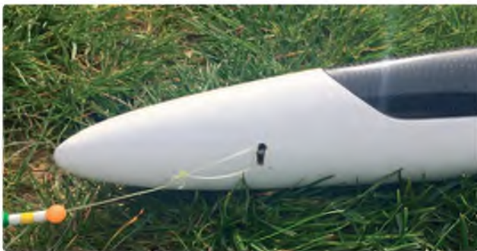
This Tangent Kult uses a simple slot and rod tow release. The outer sheath of the release is secured firmly to the fuselage
