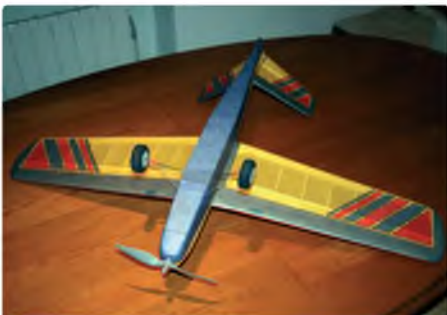
The doc lam film provides a good base for final decoration using lightweight tissue
