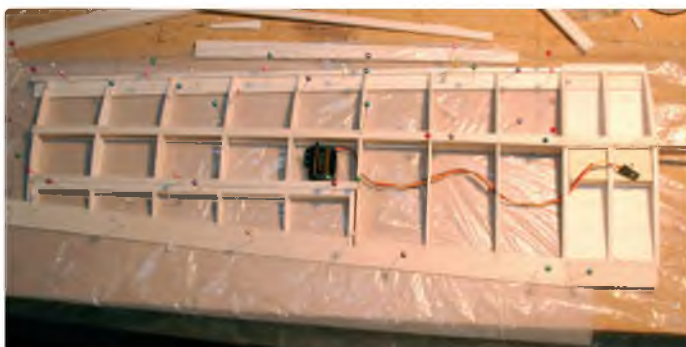
Left panel of aileron wing built onto centre section, with extra structure for the aileron and the servo installed
