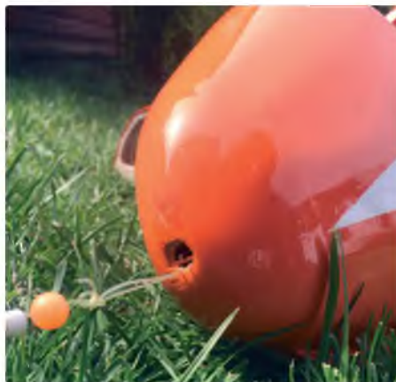
Multiplex tow release being embedded into the nose of my Mucha
