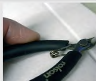
The excess tab is cut off using a pair of side cutters
