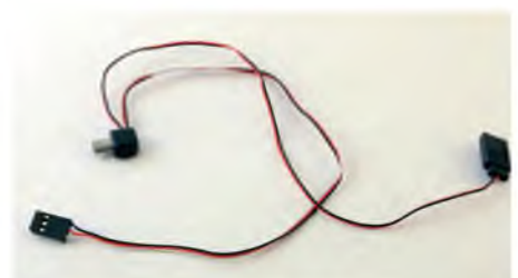
An optional FPV lead can be used to connect the camera to a video transmitter (VTX)
