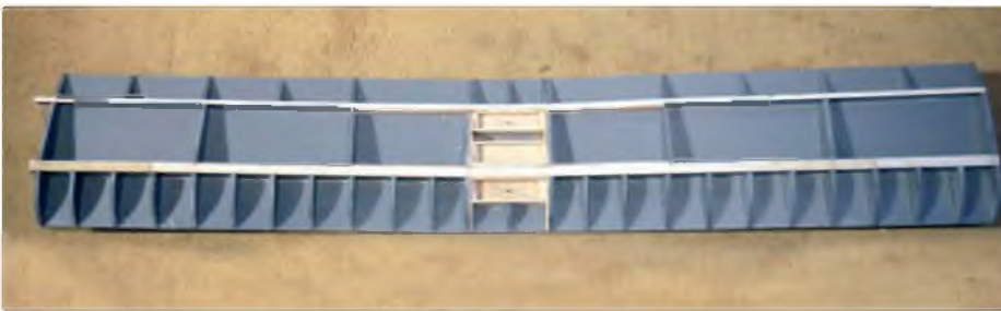
Non-aileron wing before covering the top surface
