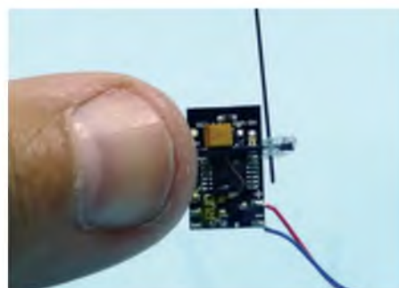
ESCs can be tiny. This tiny unit from Plantraco has a receiver, servo actuator and an ESC all in one unit – it's smaller than a thumbnail!
