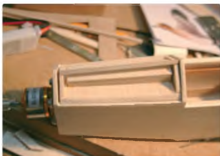
Building the top nose hatch on a 3/32" balsa base
