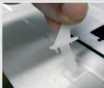
The long tab on the control horn is pushed through the cut
