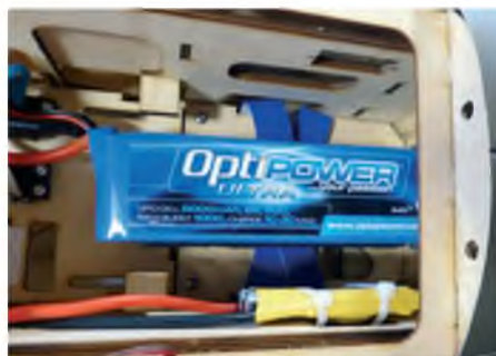
There's plenty of space for the Optipower 5000 6S LiPo in the large battery bay
