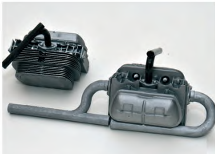
Check fit of the exhaust and inlet manifolds
