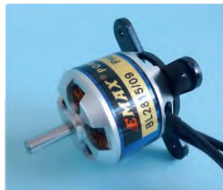
'Inrunner' brushless motors (left) require a different timing setting to their 'outrunner' counterparts (right) to obtain maximum performance and efficiency
