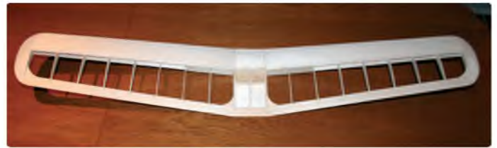
Both wings compared. The aileron wing is ready for parting off the ailerons
