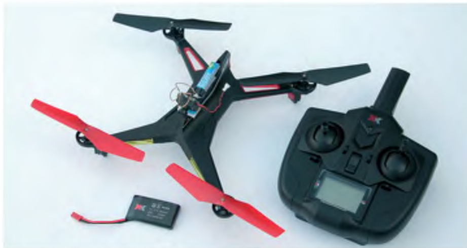
Blade 200 QX carries a VA 1100 micro camera with ease but is a little feisty for FPV indoor use with other models around
