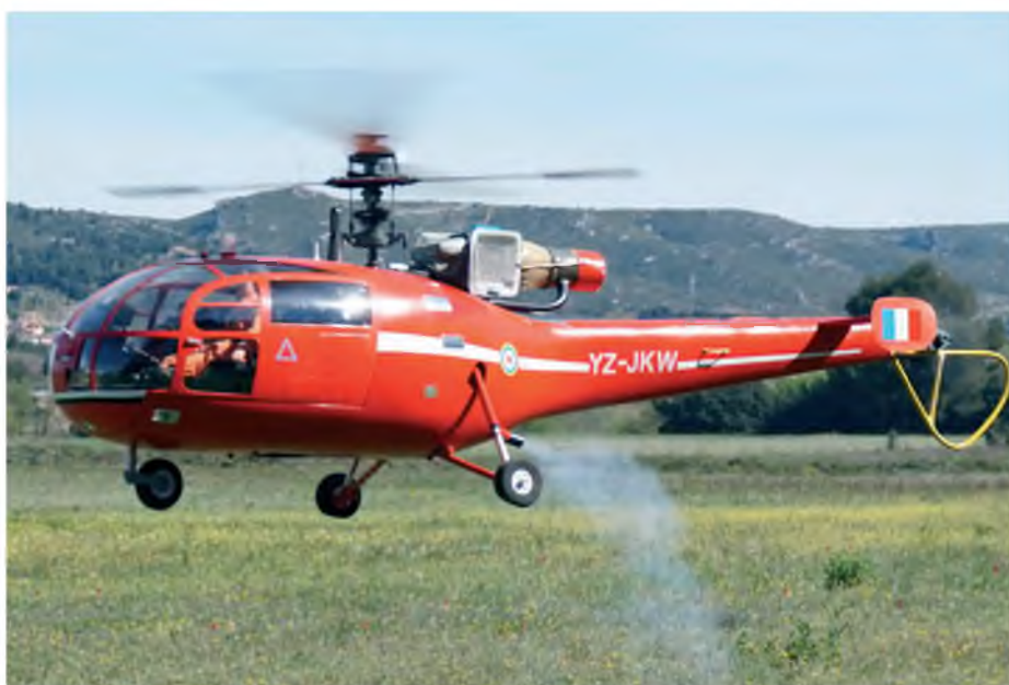
The flying qualities of the Alouette are almost identical to those of the donor T-Rex 600 but the additional 1 kg increases inertia but induces more drag
