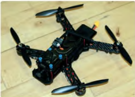
This photo shows a racing quad in more detail. The blue plastic parts are mounting points for a camera
