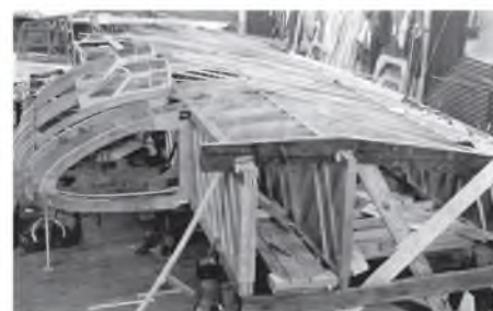
The S.55's cockpit was integrated into the large wing centre section
