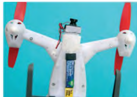
The 1S 150/200 LiPo for the camera is easily attached and is perfectly adequate
