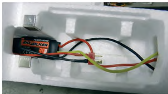
Battery bay ready for a 3S LiPo. The model comes with a 30 A ESC
