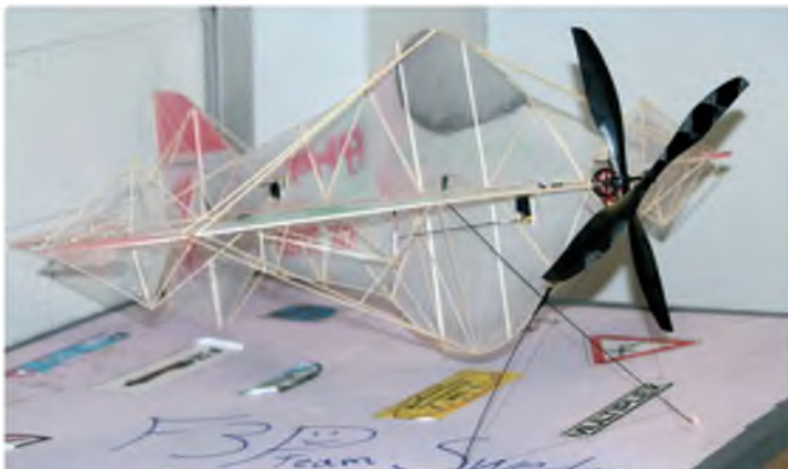
Interesting experiment by an F3P Swedish pilot, whose plane was built from balsa wood. The model is not as strong as one built from carbon but it is a good alternative. It is noticeably cheaper and the work with balsa is not so complicated
