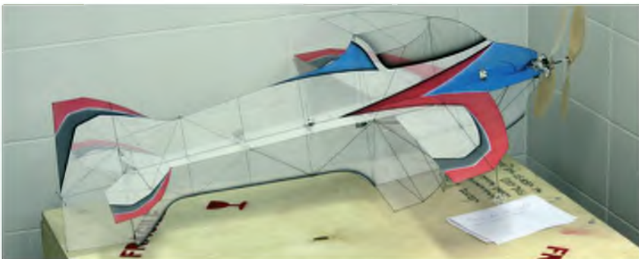
Janne Lappi's aeroplane 'Rane 2016'. With 84 cm wingspan and just 42 g RTF weight the model 'fitted' in the hall very well. The plane had no aerodynamic air brakes so all braking was provided by the 14 inch contra rotating propellers made from balsa wood
