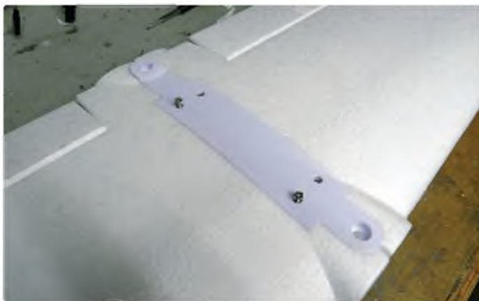
Plastic plates hold the wing panels together top and bottom
