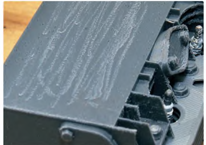
Top of the rocker box scored prior to gluing
