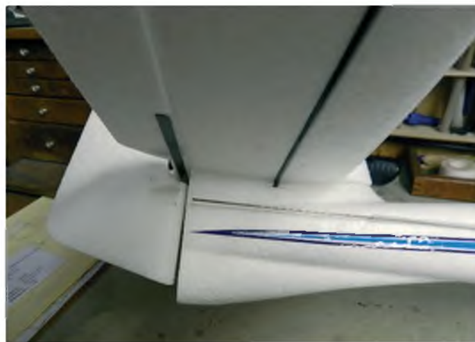
Tail linkages are made using 'wire in snake' style pushrods
