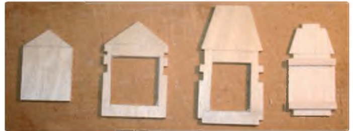
Main fuselage formers laminated from 1/32" ply + 1/16" balsa + 1/32" ply
