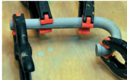
Clamping the exhaust halves while the glue sets
