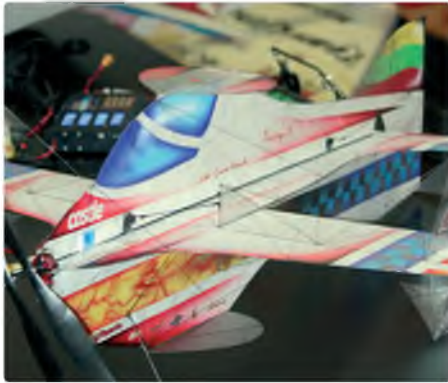
Donatas Pauzuolis' model 'Victory XL' is also built from carbon rods and tubes. This big plane was made especially for the huge hall in Poland where the second F3P World Championships was held in 2015. It uses an AL coaxial unit and new, light 12 inch props
