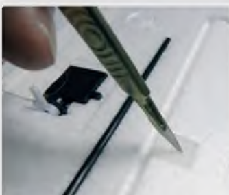
Cutting a small, central slot prior to fitting the control horns
