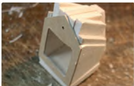
Rough assembled cowl ready for carving
