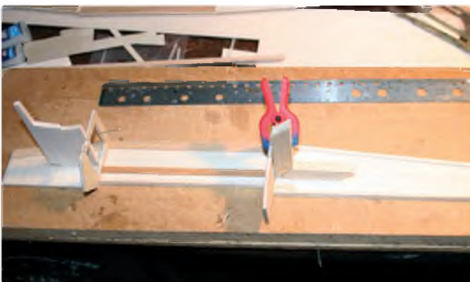
F2 and F3 assembled to first fuselage side
