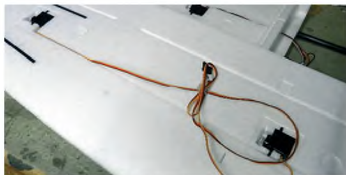
The long aileron and flap servo leads run in ready made channels underneath each wing
