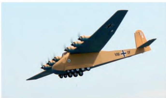
Multi motor electric models are much easier to power than their IC counterparts, such as my Messerschmitt Me 323 Gigant with six brushed motors all running from a single ESC
