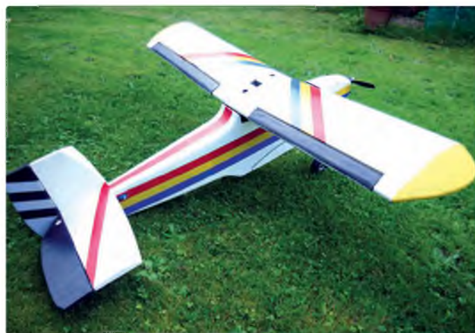
High wing monoplane, front and rear views. Note the inset ailerons and large tail end control surfaces. Also the wing blanking unit
