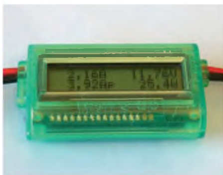
A Watt Meter provides exact information on current draw and motor power input, making it ideal for setting up electric models
