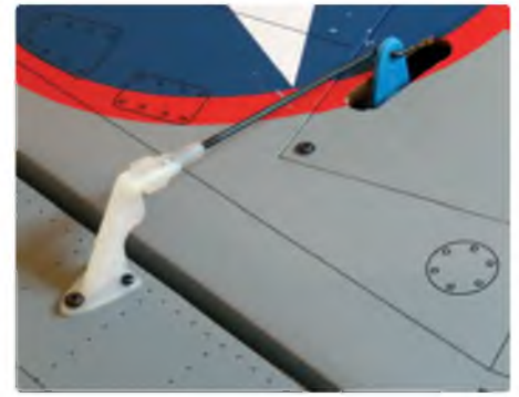
Solid linkages provide positive control with zero 'slop'
