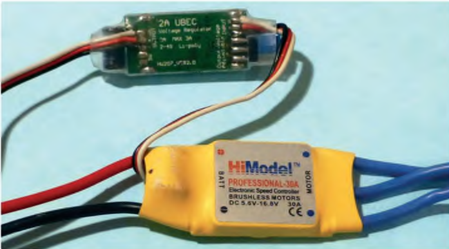
Some ESCs are supplied with a separate BEC as standard
