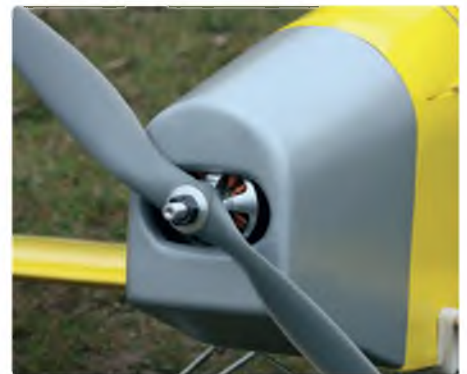
The cowl has large air inlet to cool the motor, ESC and batteries
