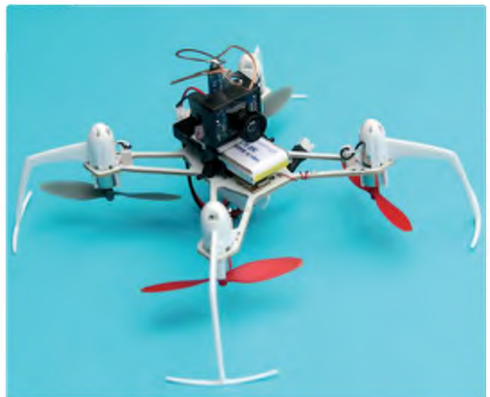
Nano QX 3D will also carry a camera but a patch lead is required for the different connector size
