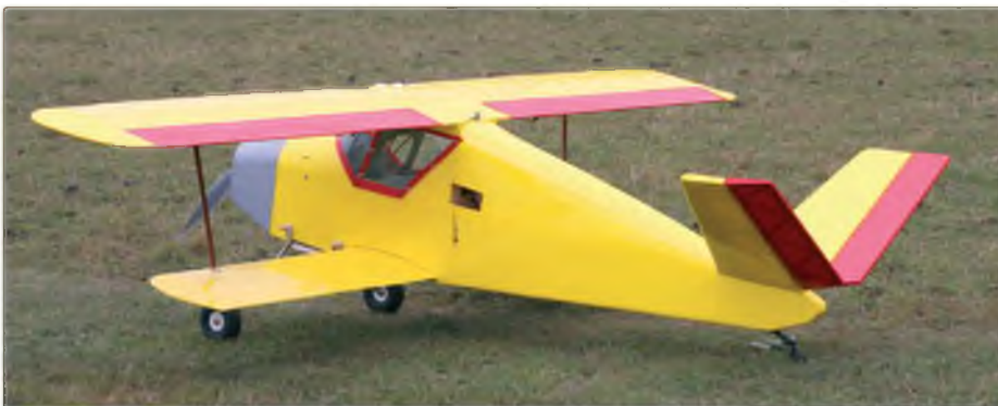
Rear three quarter view. Note the closed loop control to the steerable tailwheel, warm air outlets behind the cabin and the tow hitch at the rear of the top wing
