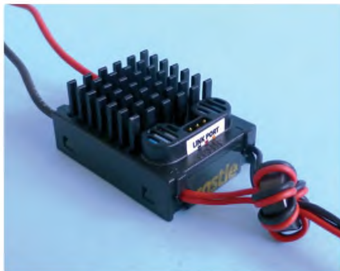
This stand-alone BEC from Castle Creations is rated at 20 amps, providing power for several full size servos as well as other ancillaries
