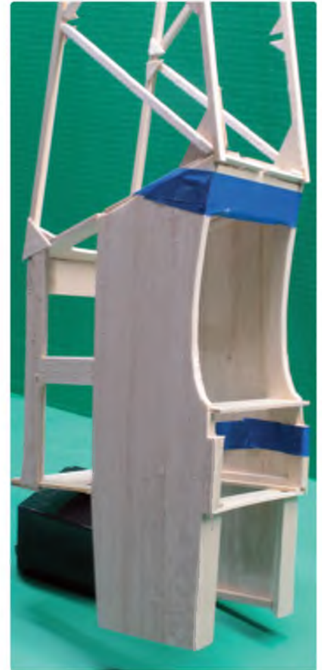
Masking tape makes a great, impromptu clamp. Remember that the tape sticks best to clean surfaces and to its own sticky side. Plan your tape/wood 'joints' so that stress is along the tape, not perpendicular to it
