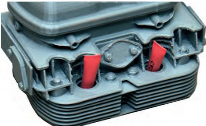
Spark plugs protected with heat shrink tubes (used cold) prior to painting
