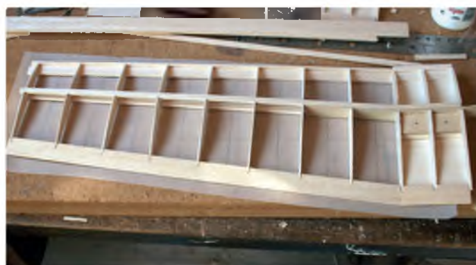
Left outer panel of plain wing being built onto centre section
