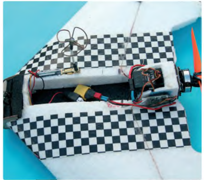
A modification moved the Rx back and gave a larger battery space
