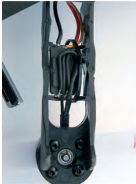
ESCs are very easy to access on racing quads and keep cool in the prop wash
