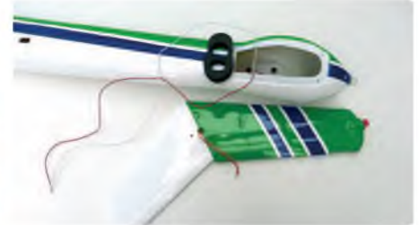
Feeding the anti-collision light wire through the fin is a bit fiddly; three screws hold the fin in place
