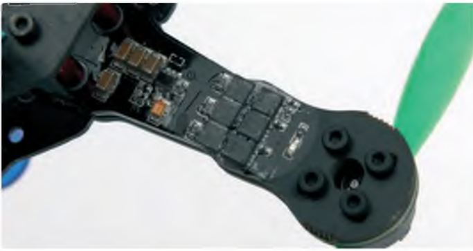
ESCs on this model are an integral part of the structure and could not be easily replaced
