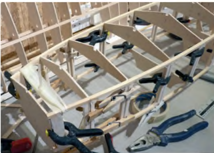
Cable tie or tape used to hold fuselage sides together at the front
