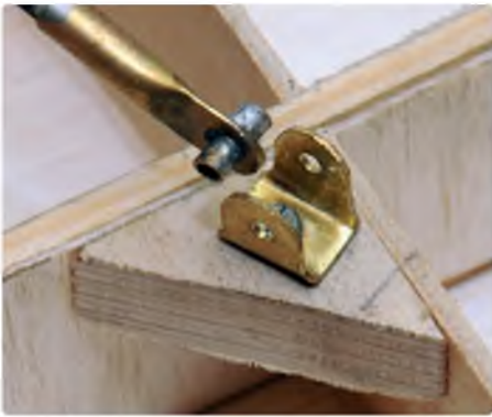
Original drag strut bracket and fixing. Note strong plywood insert
