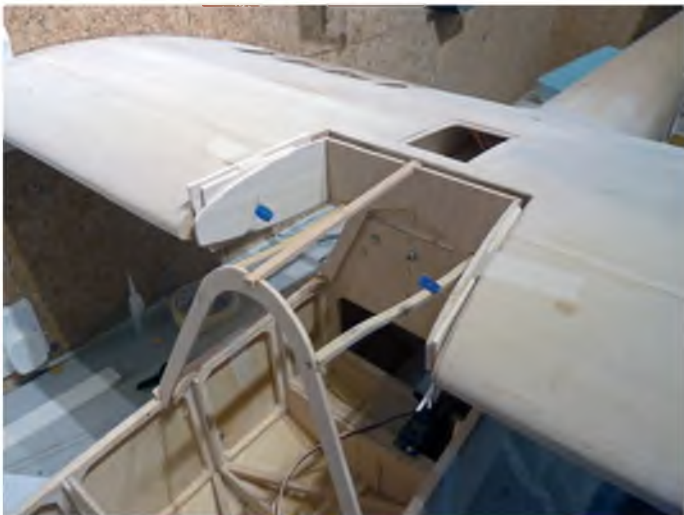
Setting up the rear canopy framework
