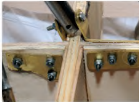
Brass brackets and backings test fitted with nuts and bolts. Allow space to allow for balsa sheet wing covering
