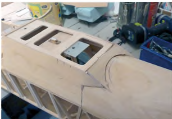
View of wing TE/fuselage fairing, to be finished off with filler
