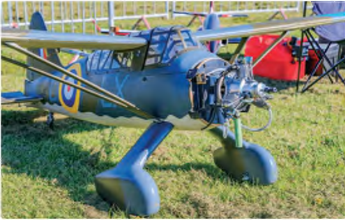
The Saito 60 cc 3 cylinder radial engine mounted to Barry Barker's Seagull Westland Lysander III
