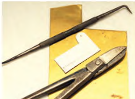
Brass sheet with scribe and tin snips used to cut it to shape
