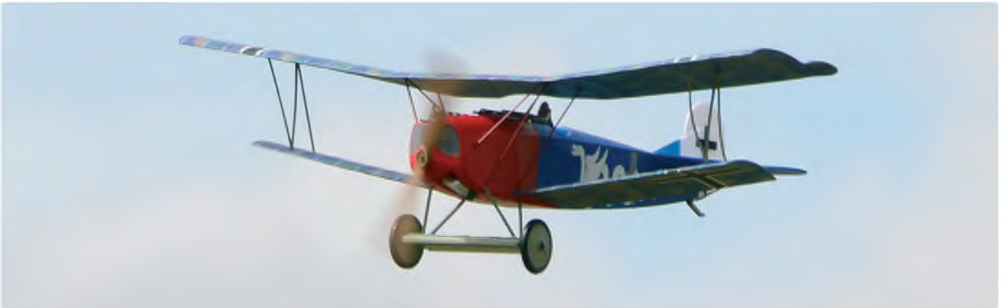
The interplane struts flex to soak up flying loads and to ensure high crash survivability. They work well, as we can testify!
