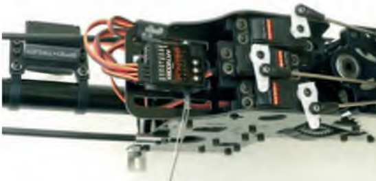
eCCPM servos fit behind the main shaft – it is best to use short servo arms
