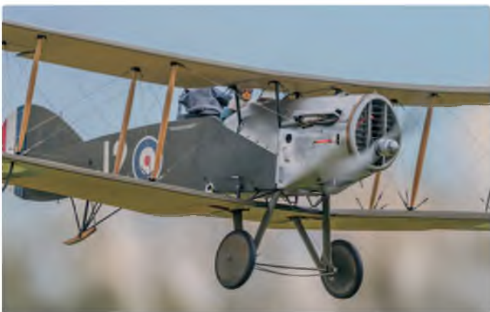
Another model owned and flown by Steve Carr, the Bristol F2 Fighter. The model comes from the Kavan stable and has a 2.39 m wingspan. Flies very well but needs a lot of rudder
