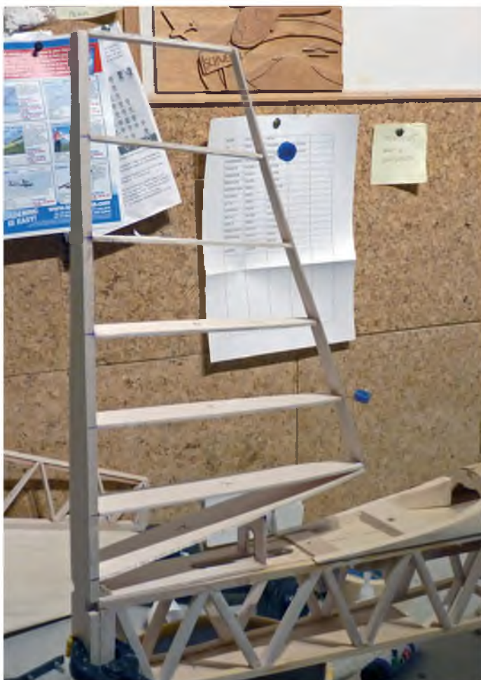
Setting up the basic fin structure
