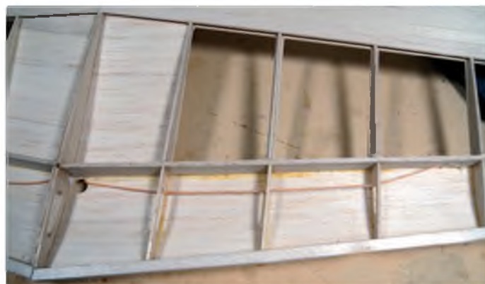
Guide in the thread for pulling through the servo leads
