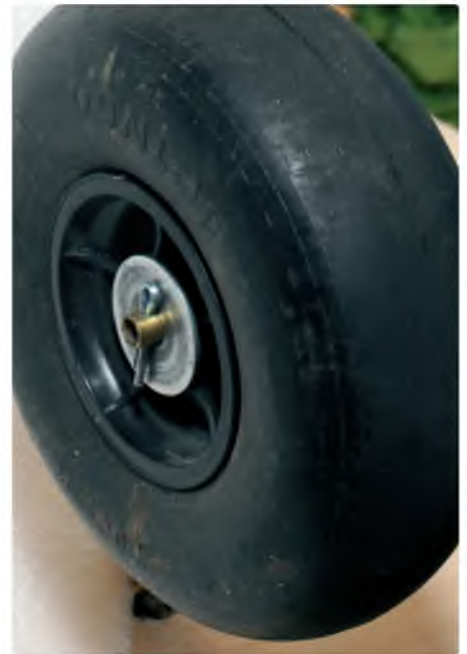
Wheel retained with a washer and split pin
