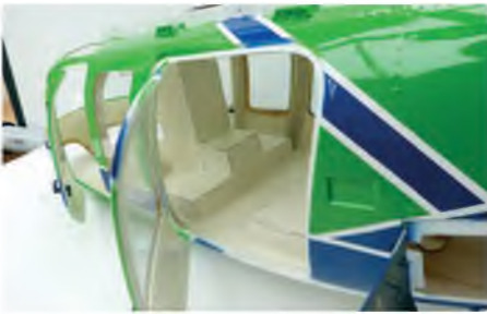
The doors are hinged with working handles and the clear glazing is properly fitted
