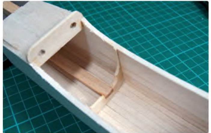
F3 is sanded out with a rotary drum sander to allow the tank to fit
