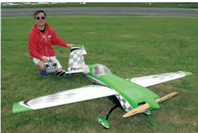
Chris Bransbury of the MacGregor Industries/JR Propo display team shows off his vivid green Extra 330 SC from the Pilot RC kit. Powered by a DualSky GA6000.8 Xmotor, energised by twin 6S 5000 mAh Optipower LiPo packs, this 88 inch wingspan beauty is controlled by a full JR XBus setup using JR NX8925 servos macgregor.co.uk/pilotrc.htm www.jrpropo.com/english/propo/XBus
