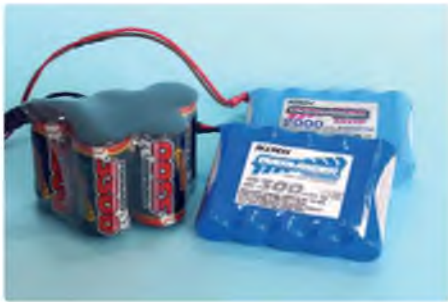
In some installations using larger Sub 'C' NiMH receiver packs can help obtain the correct Centre of Gravity
