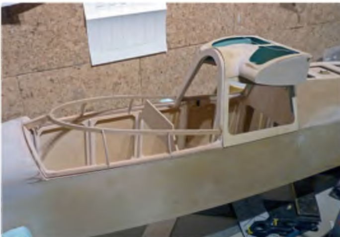
Setting up the front canopy framework
