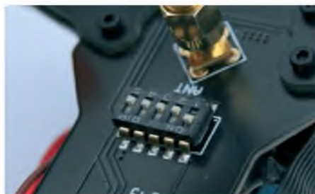
These DIP switches are used to set the 5.8 GHz video Tx channel
