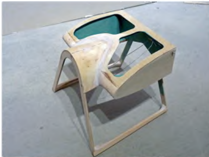
Rear canopy almost complete
