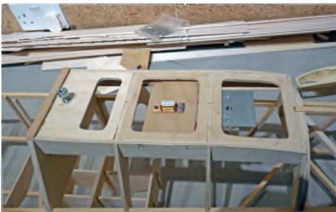
9-pin 'D' plug mounted on its own ply plate
