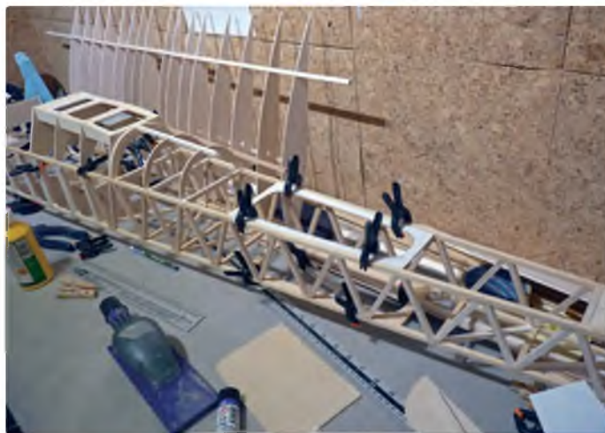
Temporary jiggling plates hold the rear of the fuselage straight
