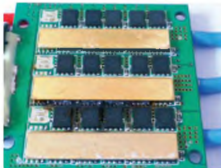
Right: The bottom row of MOSFET semiconductors have burnt out on this 100 A ESC. Correctly setting up the ESC can help avoid such failures
