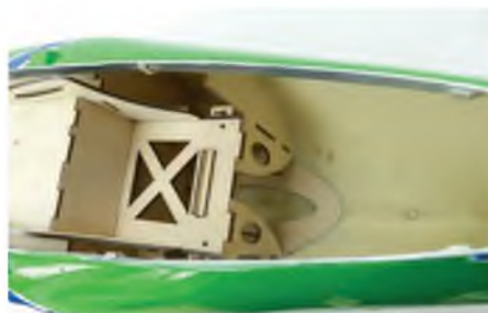
Here you can see the end of plywood plate that runs along the floor of the fuselage helping to spread the load
