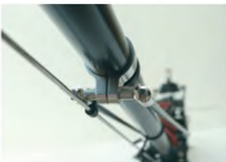
The boom stays need spacers to clear the boom
