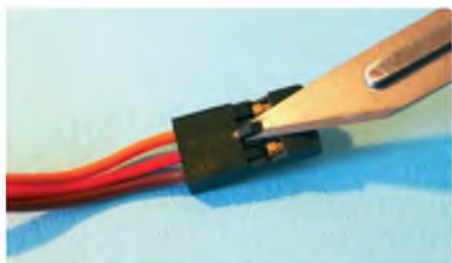
To disable an integrated BEC carefully remove the centre positive pin (usually red) from the receiver plug
