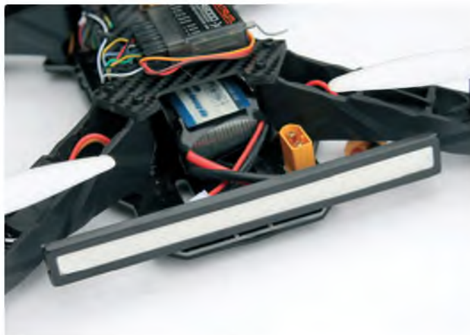
The rear red LED light strip is very effective and helps a lot with orientation when non FPV flying
