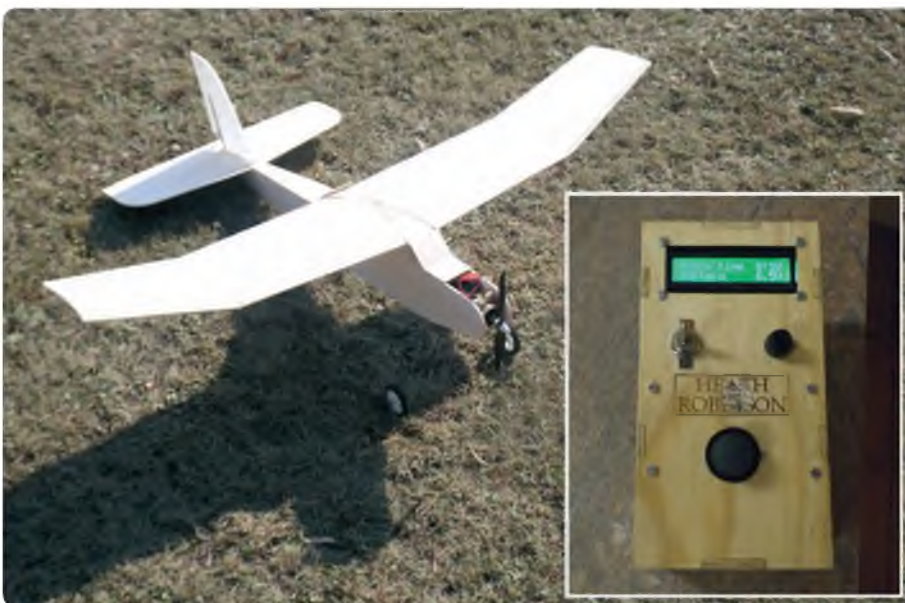
Chris Freeman's O/D Single Channel trainer was designed, built and flown in a weekend. Balsa and foam construction. A stable and reliable subject for learning the arcane art of Rudder Only. Inset: we think SC's readers will approve of Chris's transmitter!
