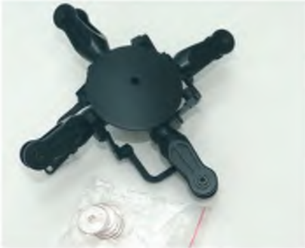
Fully assembled four blade rotor head. I checked all the screws, which were secure. All you need do is check the length of the control rods
