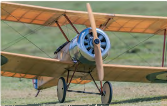
Paul Williams brings his Sopwith Pup into land. A third scale model built from the BalsaUSA kit, it has a geared Zenoh 38 cc petrol engine
