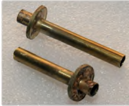
Wheel retainers are soldered onto axle
