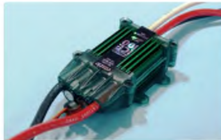
This 100 amp ESC from Castle Creations features a switching BEC, as opposed to a linear unit, so producing less heat
