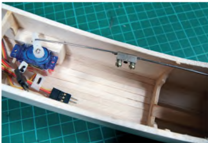
Simple 'adjustable' throttle linkage
