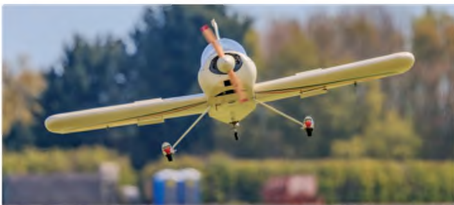
Above & right: CARF Corsair of Tony Hooper. The Corsair features a folding wing system, which Tony operates as the Corsair taxis out to the runway and the Moki five cylinder radial petrol engine sounds superb
