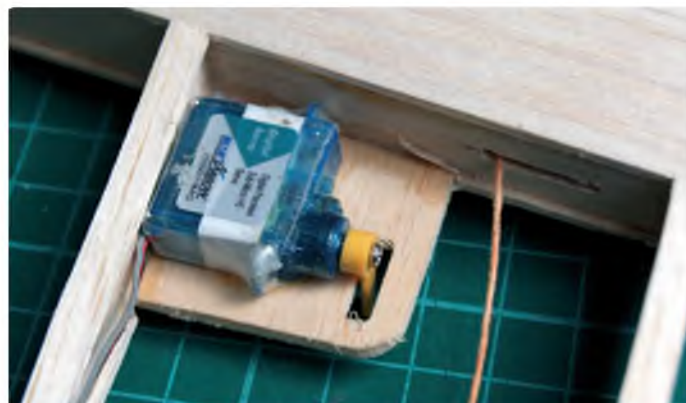
Aileron servo (D05010MG/5.7 g) viewed from top
