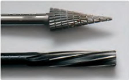
Milling tools used in pillar drill to cut correct size hole in lower oleo
