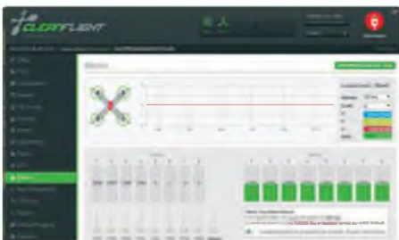
This is the page for testing the motors individually and together, plus setting motor revs, if required
