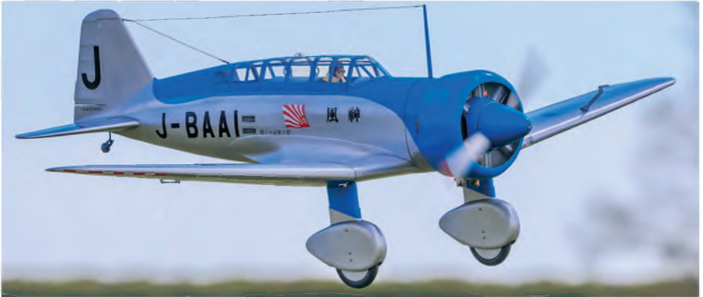
Built from a Dave Anderson plan by Brian Rawcliffe, this is a Mitsubishi Ki-15. The model has a 120" wingspan and weighs 36.5 lb
