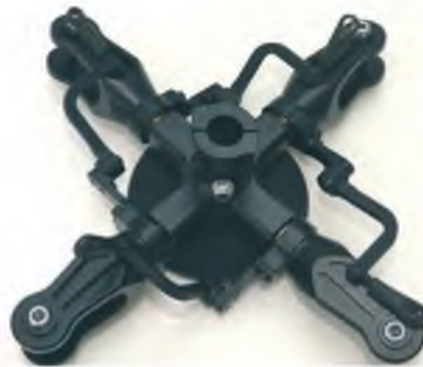
4 mm bolt and two pinch bolts secure the rotor head to the 12 mm main shaft
