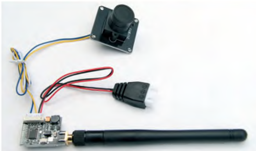
Budget price 5.8 GHz Tx sets like these are very inexpensive. This one from Eachine uses the balance lead from the flight pack for power
