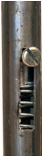
Oleo leg showing slot, spring and retaining bolt
