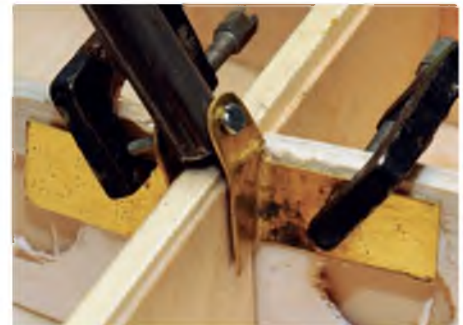
Main leg opposing brackets with oleo leg set at the correct angle. Check and check again!
