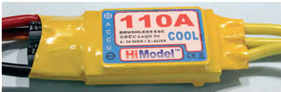
This 110 A ESC features an integrated BEC with a rating of 6 A. However, this will decrease as battery voltage increases
