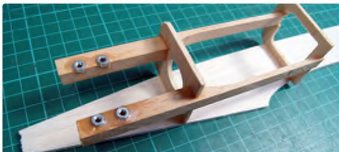
Front formers glued to the fuselage side
