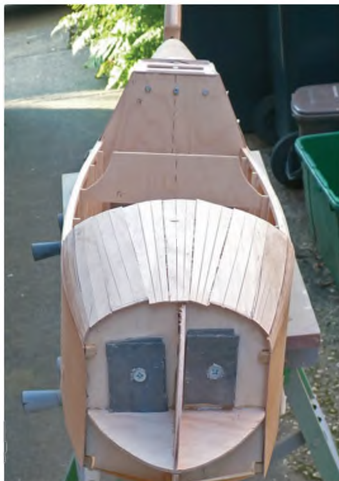
Extra lead ballast added to the F1 before applying the filler
