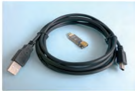
This USB programme link from Castle Creations allows the user to adjust ESC settings via a laptop or PC
