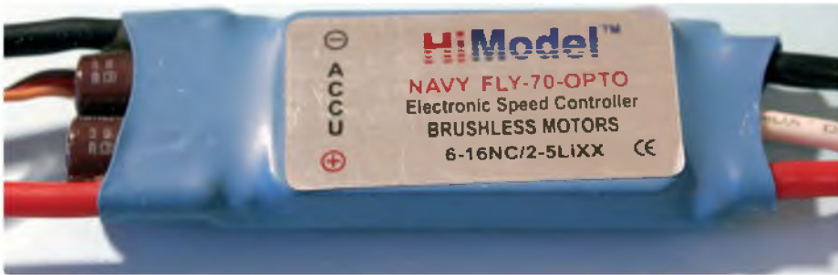
This 'OPTO' ESC has no integrated BEC so there is no need to remove the positive wire when fitting a UBEC
