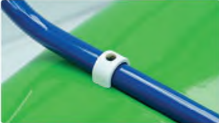
The undercarriage is supplied ready to fit and just needs four screws; dummy clamps are simply glued on top
