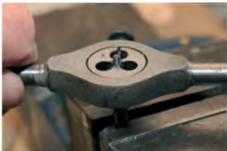
6BA threads being cut on the drag strut rear end
