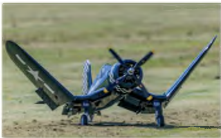
Above & right: CARF Corsair of Tony Hooper. The Corsair features a folding wing system, which Tony operates as the Corsair taxis out to the runway and the Moki five cylinder radial petrol engine sounds superb
