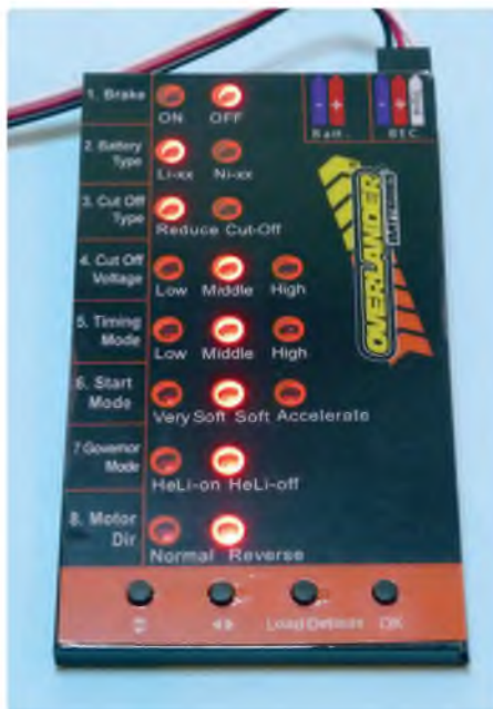
ESC Program cards make programming much easier. Each LED light indicates the relevant setting, changed by pressing the buttons. The motor 'beeps' to confirm setting, then disconnect – easy!
