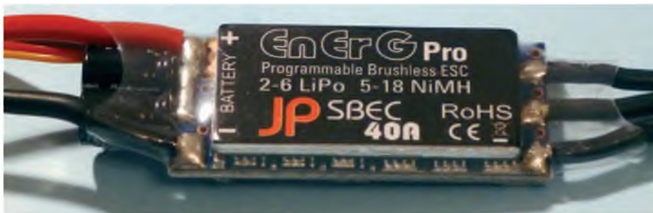
JP EnErG Pro ESCs feature Switching BECs and are fully programmable. This 40 A unit is low cost but can handle 2-6S LiPo packs
