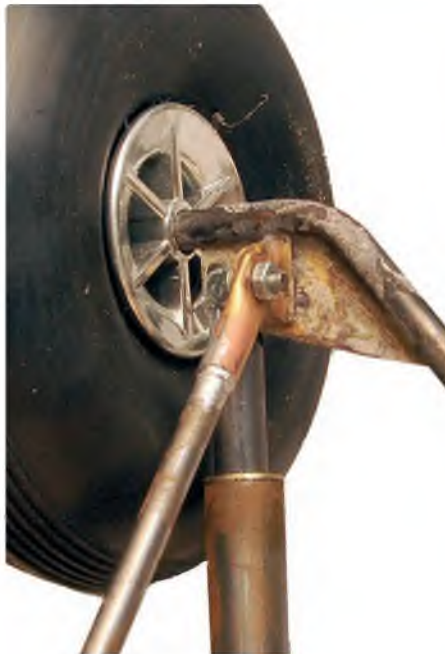
Brass shaped insert to accept lower oleo and drag strut ends
