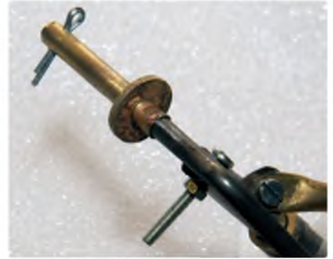
Wheel retainers fitted, complete with split pins
