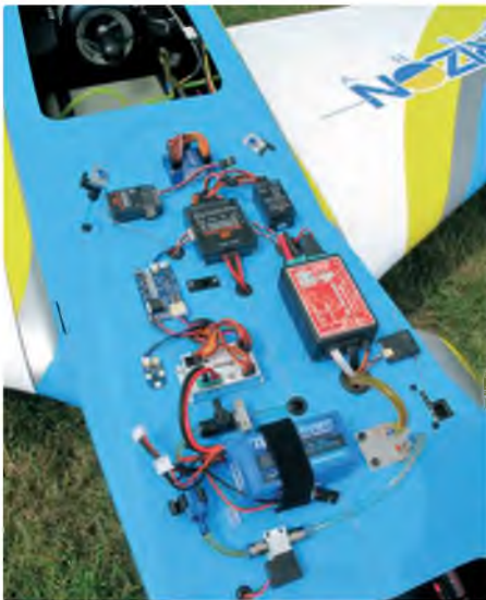
The avionics bay of one of Horizon Hobby's demo jets is a good illustration of the components needed to control a modern R/C jet. Neat job too!
