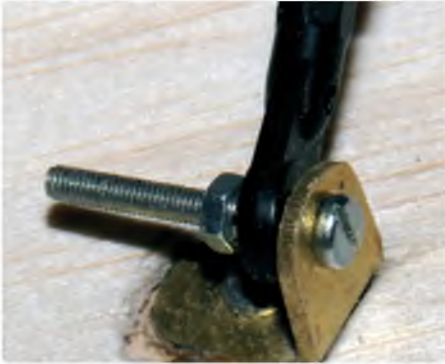
Drag strut fitted to modified bracket
