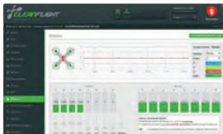
This screen shot shows the motors running, all at the same revs
