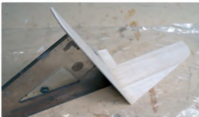
Assembled V-tail propped up against a 60 degree set square
