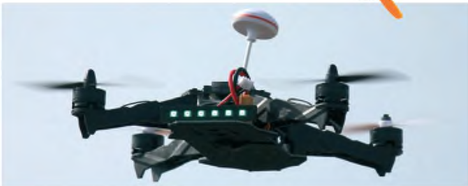
This 250 racer is the same as mine but is a more recent model. It now has a variable colour and function LED tail light bar
