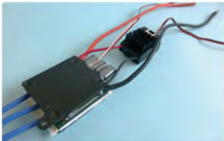
Castle Creations 20 amp BEC 'paralleled' to a 125 A 10S ESC ready for installation in the author's Vulcan bomber
