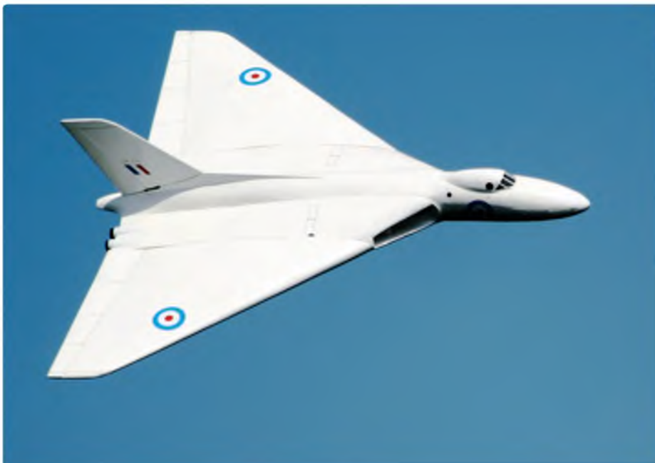
The author's large Vulcan bomber flying on a single 120 mm aeronaut carbon EDF unit, running on 10S (2 x 5S Optipower 50C 4700 mAh LiPo packs in series) with a Castle Creations 20 amp BEC
