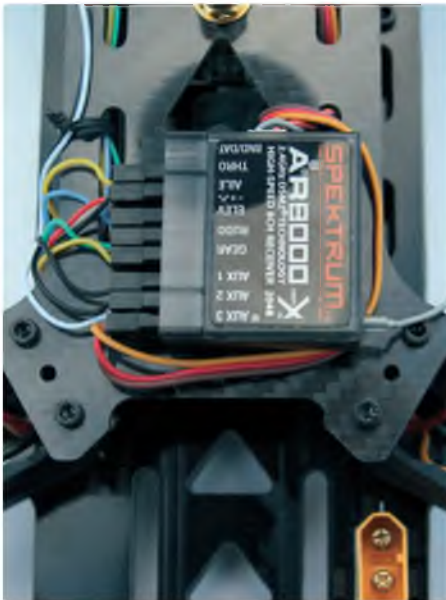
If you want a separate light switch function an eight channel Rx is required. A manual on/off switch is mounted on the board
