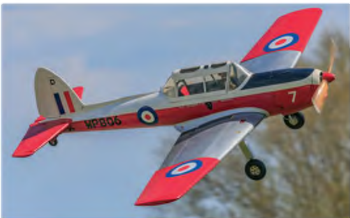
James Ladell's lovely DHC Chipmunk. 38% scale model uses a King 67 cc petrol engine, which has a 2.25:1 reduction gear fitted
