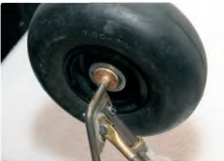
Rear of wheel showing washer and tube soldered in place
