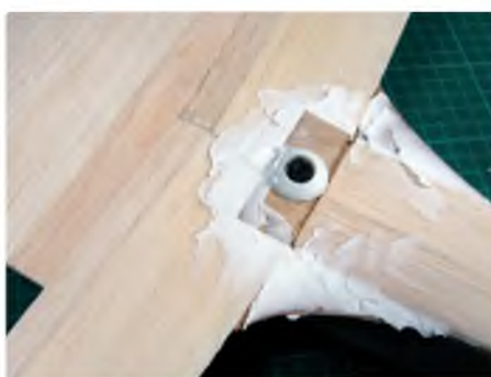
Tidy up the underside with filler
