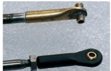
Drag strut ends, the bottom one is the second version with a ball joint clevis
