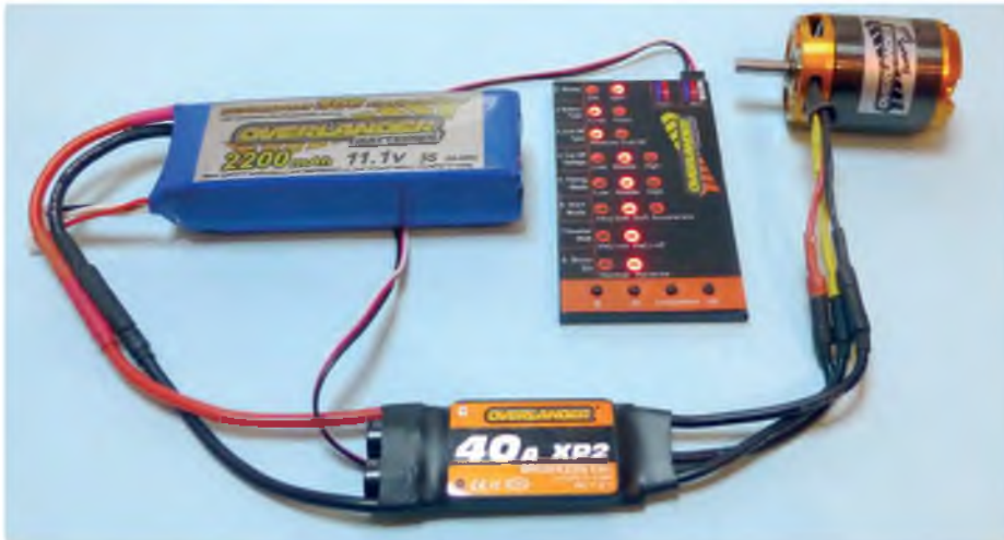
Wiring in a program card is an easy task, as can be seen from this simple set up
