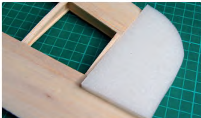
Depron tip block. Sand to shape. Balsa would be okay here too
