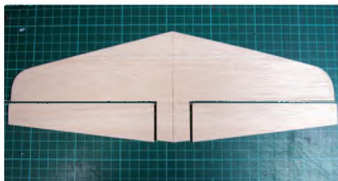
V-tail components cut from 1/8" balsa sheet
