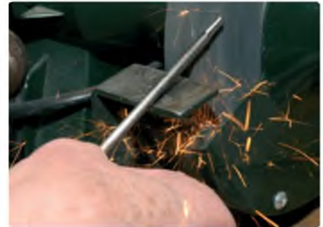
Grinding the drag strut down to tapping size carefully
