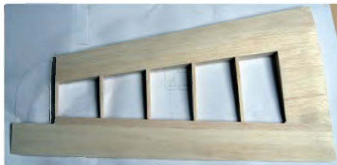
Top sheeting and cap strips done, and cleaned up
