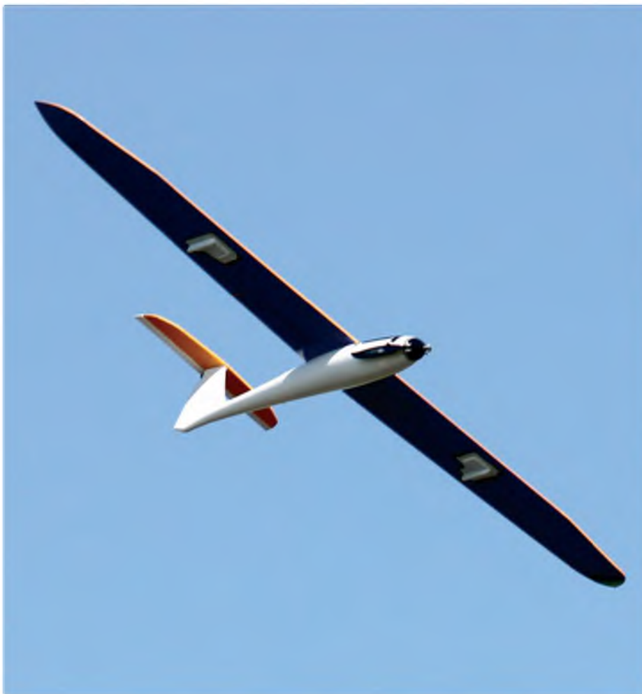
Being able to program the motor brake via the ESC allows folding props to reduce drag on glider installations
