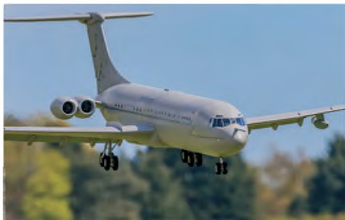
The 16 ft wingspan VC-10 is a popular model and looks very realistic in flight. It weighs 64 kg and has four Wren Supersport jet turbines. Dave Johnson is the usual pilot and says the model flies well
