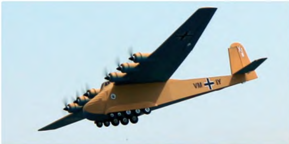
Above: Unlike brushless motors brushed motors, as fitted to the author's six 'engined' Me 323 Gigant from Graupner, can run from a single ESC!
