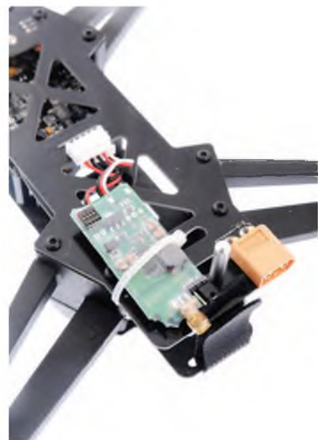
Rear view showing the video Tx board and the main XT style battery connector
