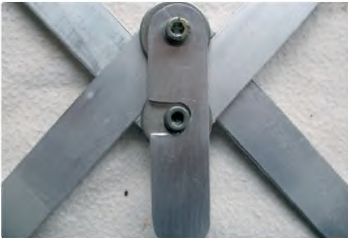
Collapsible cross bracing is locked by a simple turnbuckle
