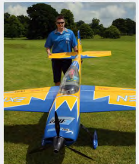
Matthew powers the big aerobat with a Plettenberg 37/6 motor and controls it with a Spektrum DX18 radio. Spektrum High Voltage servos all round. Matt is supported at shows and competitions by his father, Trevor
