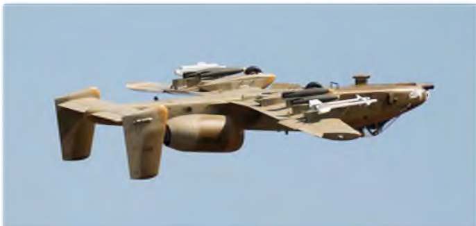
Scott Geller's Mibo A-10 Warthog. 1:5.5 scale, 118 in wingspan, 55 lb, JetCat P-160 turbines, Futaba MZ 18 radio
