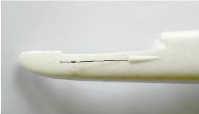
Tail pushrods use swing keepers to connect to the control horns
