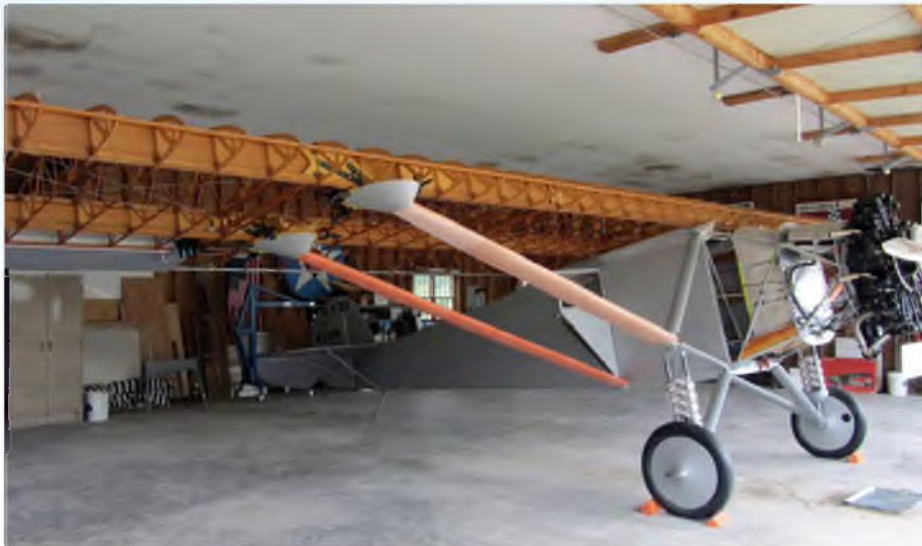
The Spirit replica two years ago, showing the finished fuselage and wing. The sheet metal cowlings and shock absorber fairings have yet to be done. The strut fairings are made from balsa wood!
