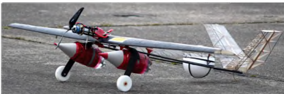
Two streamlined drinks bottles carry the payload on Stade's victorious Weight entry – nicknamed 'Madonna' by the Brits...
