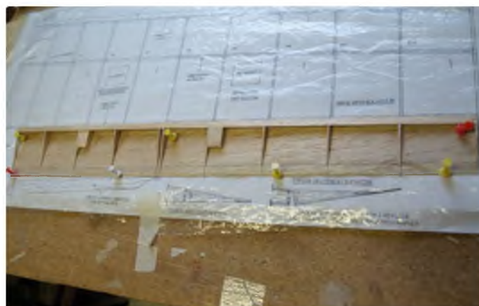
Elevator and aileron under construction. Top sheeting to be applied
