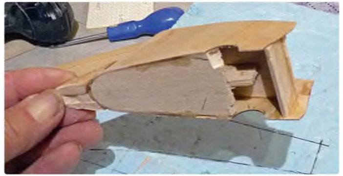
View of fin fairing structure
