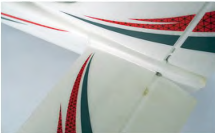
Jordan's first try at fitting the tail retaining bolt left it a bit loose. So be sure to use a correctly sized cross-head screwdriver and screw it fully home
