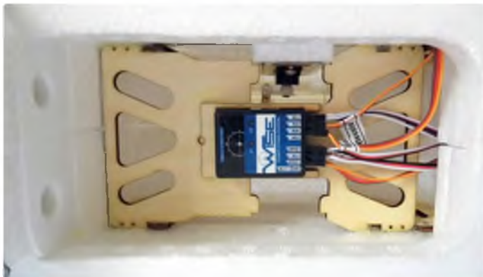
At the heart of the Sensei is the WISE 3-axis flight stabilisation system
