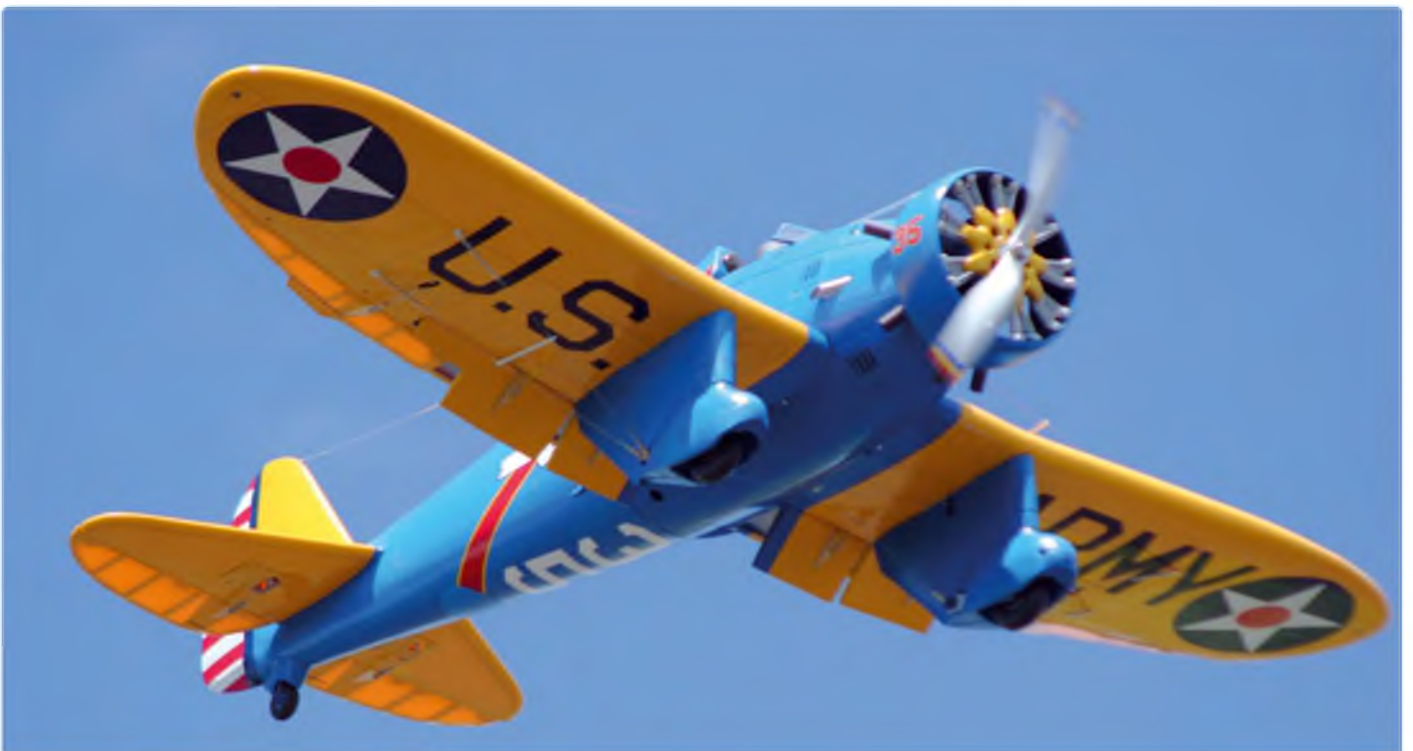
Overhead with full down 'split' flaps. Note the position of buzz number '35' under the rear fuselage
