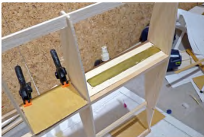
View of brass wing joiner box placement
