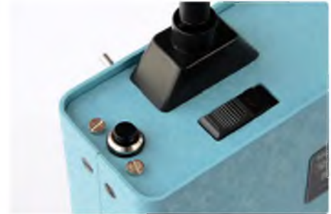
Top panel showing the offset antenna location, the power switch and Timer button. Note the slotted bolt heads
