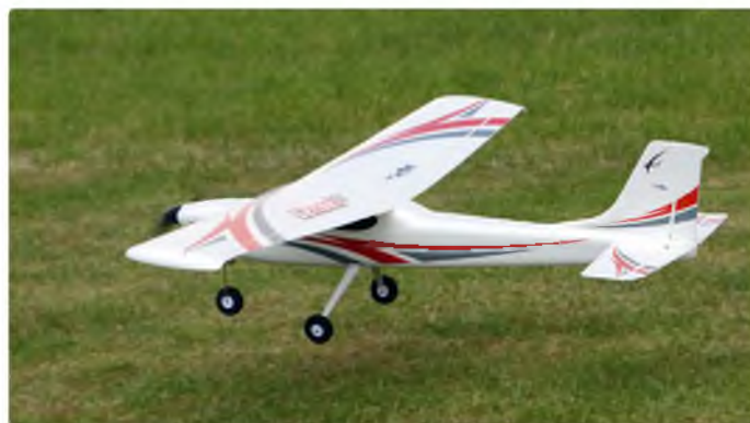
A small tad of up elevator settles her into the flare for a smooth touch down
