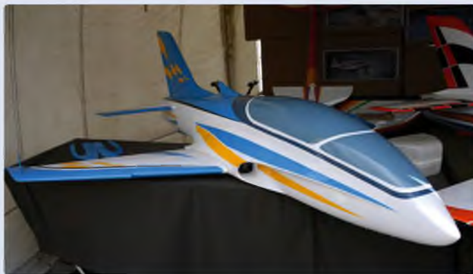
Aspire is a 93 inch span all-composite jet for 12-16 kg turbines. It comes highly prefabricated from the factory
