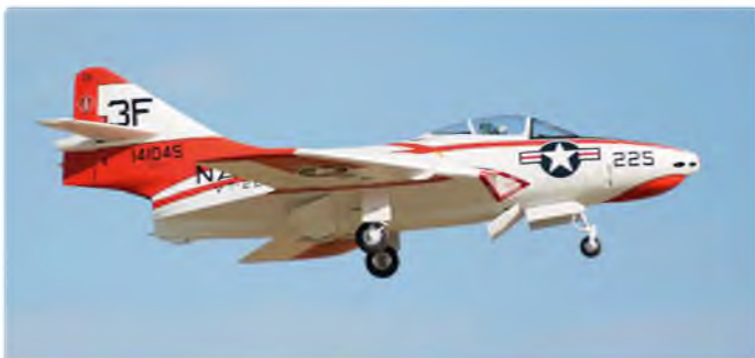
Mitch Buckley's Air World F-9F Cougar. JetCat P-180 turbine, JR12X radio
