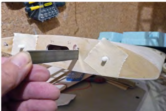
Masking out the MPX wing retaining system
