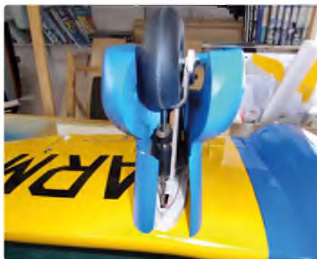
Port side spat and trouser ready for closure
