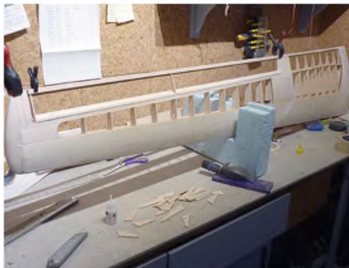
Initial stage of building the aileron
