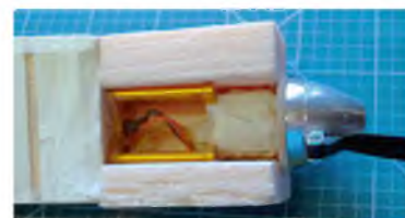
Alternative cowl. This is from blue or pink foam carved to shape and covered with glass cloth and epoxy resin
