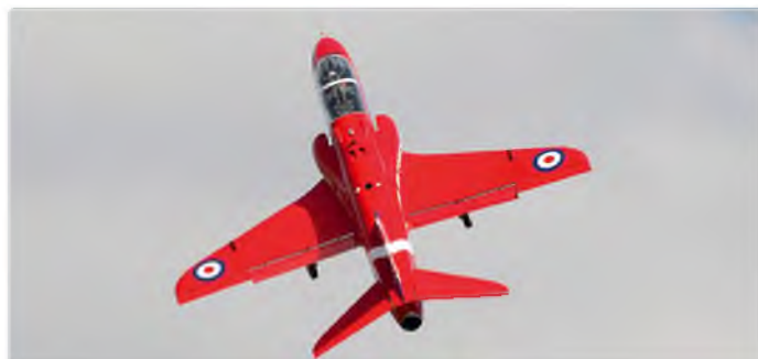
Jeff Stubbs' Comp ARF BAe Hawk, 1:375 scale, 98 in wingspan. Kingtech 210G turbine, Spektrum DX-18 radio, RAF Red Arrow colour scheme
