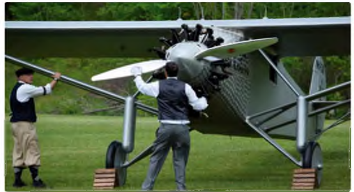
Switches off! The prop is rotated to starting position
