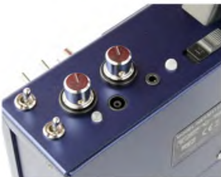
Top panel showing two more rotary knobs, another two switches, power and charging indicators and the charging and trainer jacks
