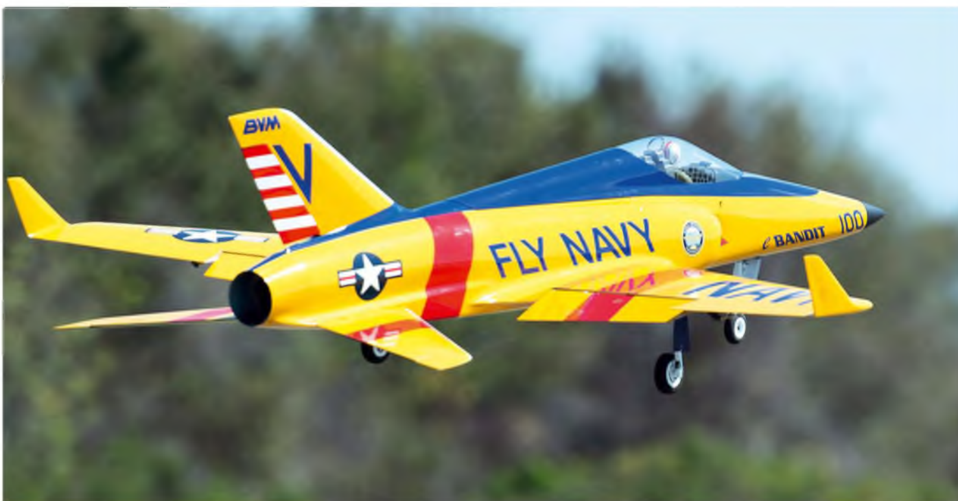
Rod Snyder's BVM E Bandit, 72 in wingspan, 18.5 lb. 3 x LiPo (4-cell 7700 mAh), BVM F12 Electric Power, Spektrum DX-18 radio. The winglets help decrease the landing speed and give you just a little more simulated lift
