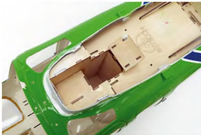
The enlarged 'broom cupboard' that carries one of the LiPo packs
