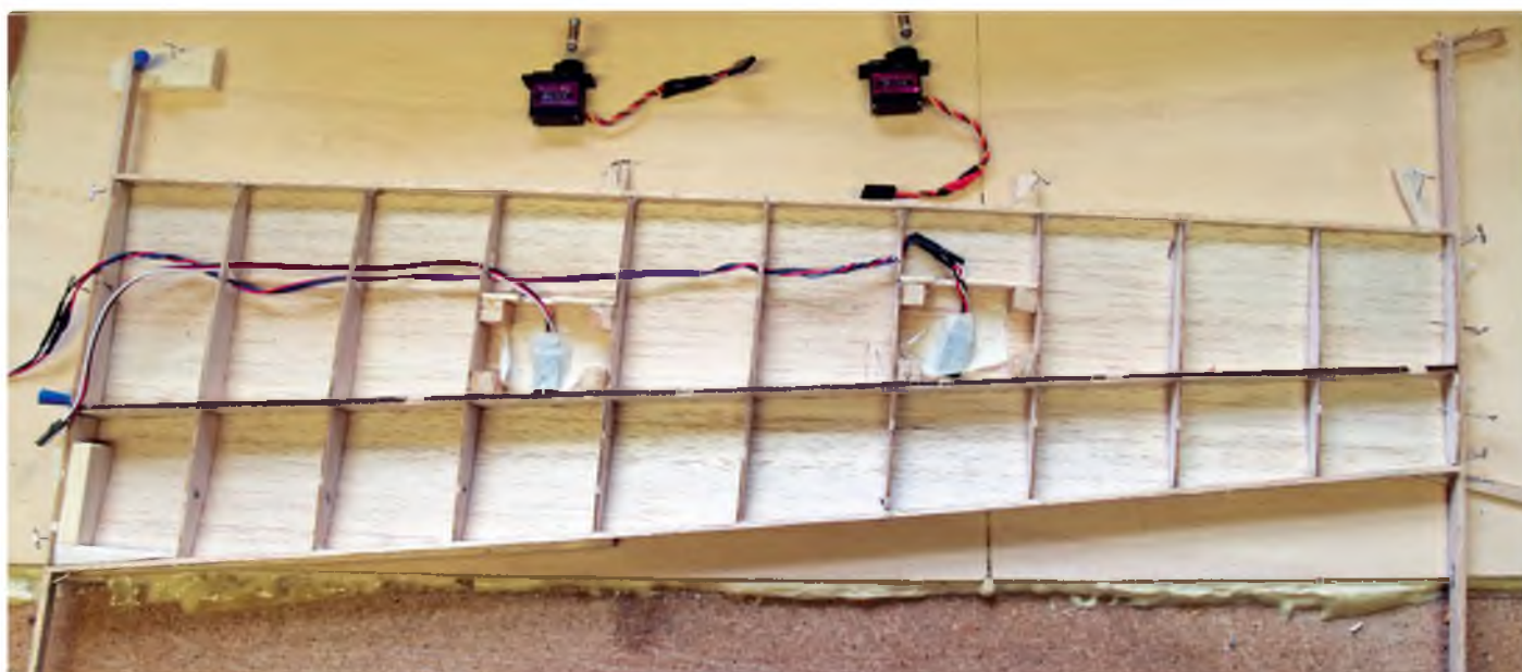
Overall wing construction seen from the underside with top sheeting in place. Note elevator and aileron servo mounting
