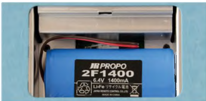
A 2S 1400 mAh Li-Fe battery comes plugged in to both sets as standard
