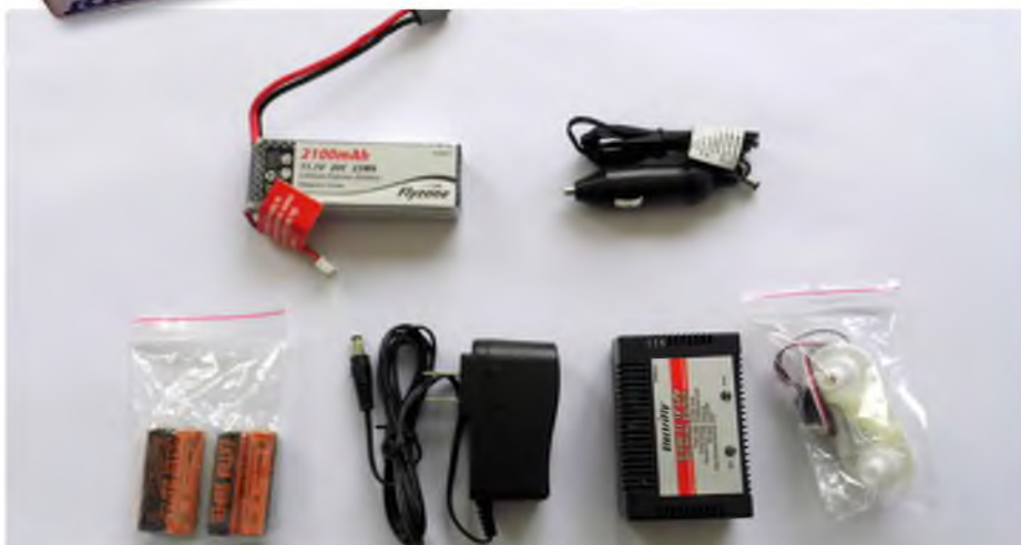
Additional parts in the RTF kit include a 2100 mAh LiPo and matching charger. Four AA cells are also provided to power the Tactic transmitter
