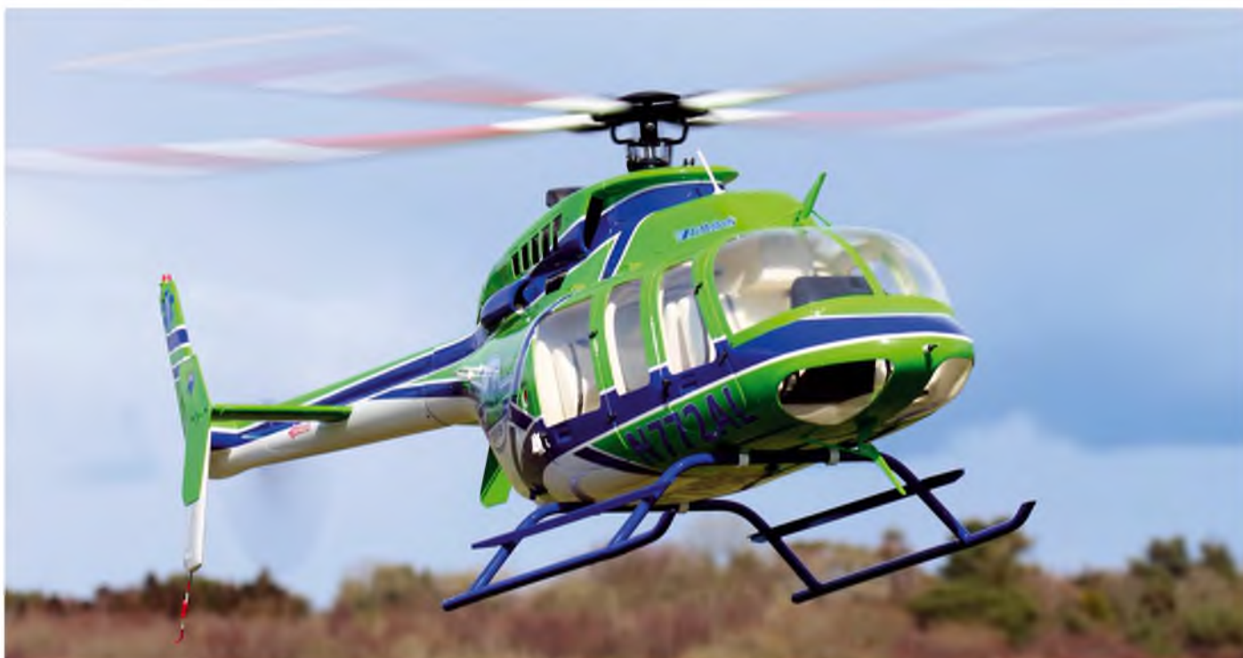
The forward raked mast means it hovers tail down
