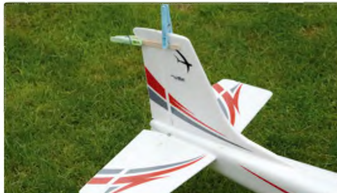
Handy tip! Clothes pegs and lolly stick splints were used to hold the control surfaces at neutral while the screw-lock connectors at the servo ends of the pushrods were fully tightened up
