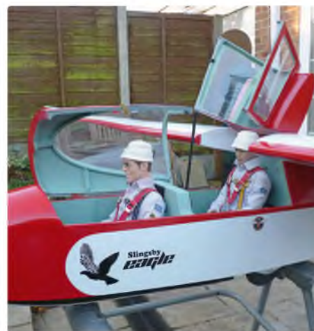
View of the open canopy arrangements
