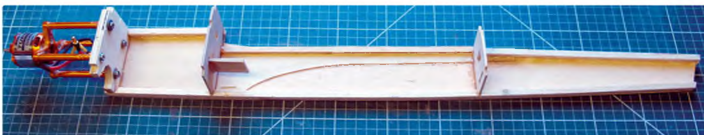
Port fuselage side to be fitted
