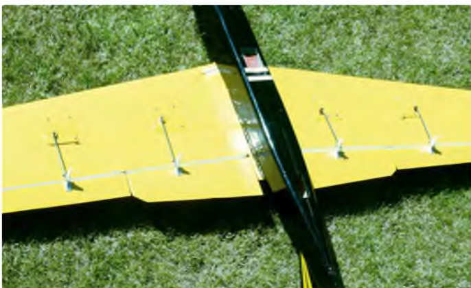
Servo positions on wing underside
