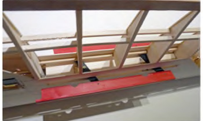
Pre-painted airbrake assembly in position
