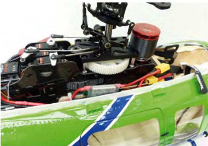
Safety Power Switch (SPS) on the right, with the power connectors close to the LiPo packs
