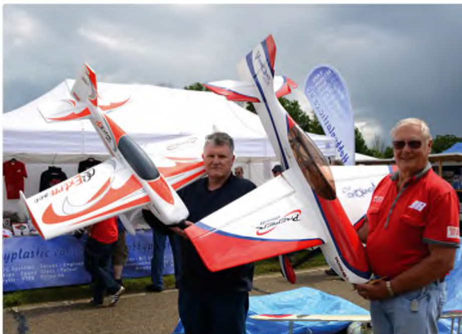
Hobbyplastic.co.uk were displaying a pair of new models by Premier Aircraft, both designed by top aerobatic ace Quique Somenzini. Dave Stickley (left) is holding the QQ Extra 300, a 47.8" span moulded foam model with an innovative ply sub-frame that connects the firewall to the wing spar. Paul Roberts (right) is holding the Ventique 60E, which is Quique's latest all-out 3D ship for 6S power
