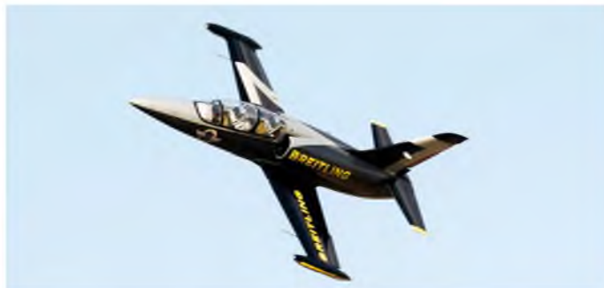
L-39 XXXL. 1:2.7 scale, 12 ft wingspan, 176 lb, JetCat P-400RX turbine. Built by Joseph Kager in Germany, the L-39 was not in the competition
