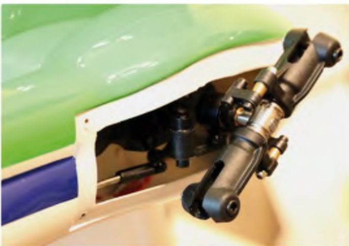
Tail gearbox in place
