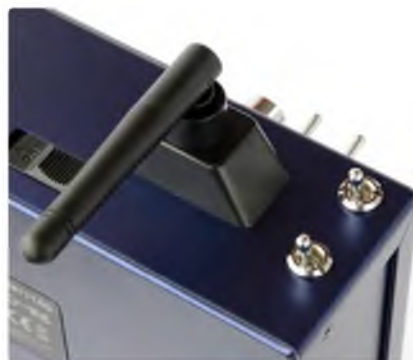
There are another two switches on the other side. The 2.4 GHz antenna should be pointed downwards in use, but maybe not at such an acute angle as shown here!
