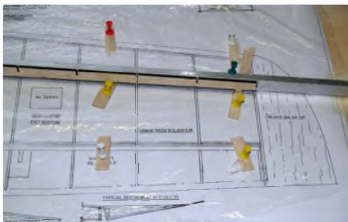
Initial set up to ensure straight spars. The mainspar is laid alongside aluminium angle and then glued to balsa sheet tabs
