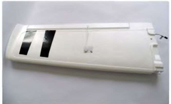
The wing panels are fully finished and fitted with shrouded servos
