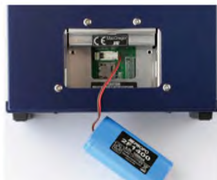
Gently removing the Li-Fe battery reveals the hinged Micro SD card slot (underneath the lead)
