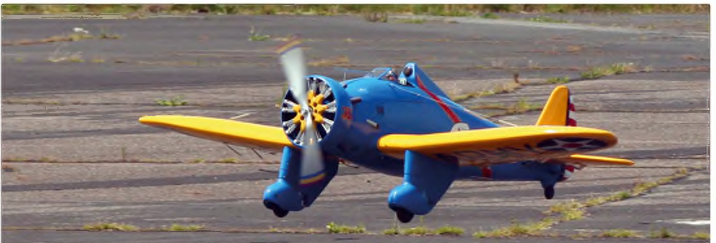
Keep the nose high and some power on when landing. And try to ensure a good three pointer to avoid it 'standing on its nose'
