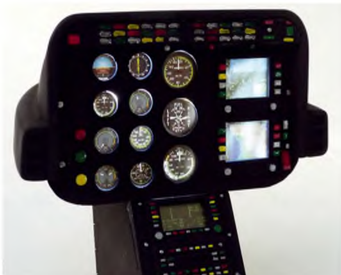
Console as it arrives, ready to glue in place. The dials are backlit with LEDs
