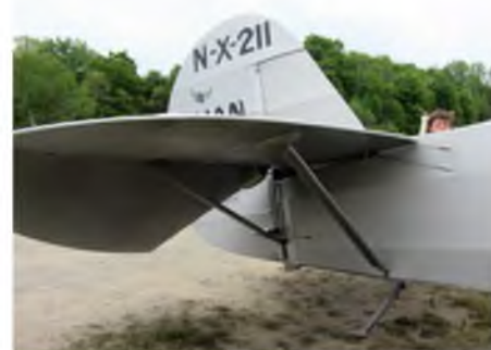
Above & below: Tail details, showing the corrected rudder shape
