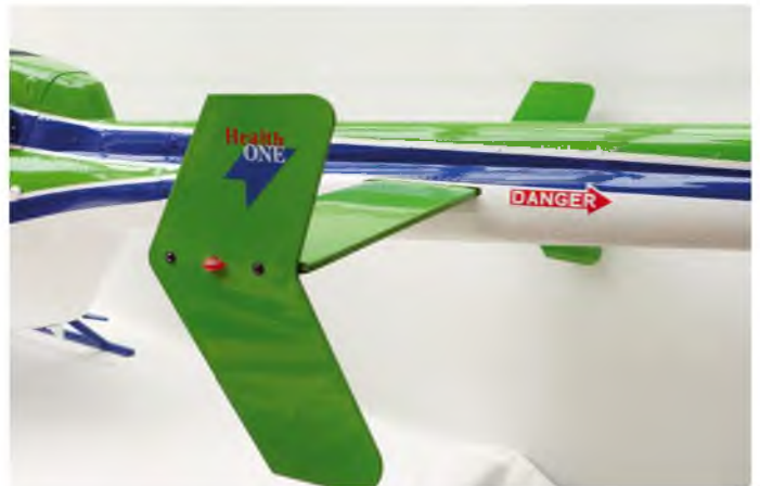
End fin with navigation light – red on left, green on right
