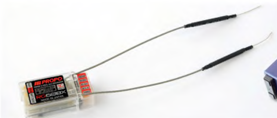
C.O.L.T. is supplied with an RG613BX XBus receiver. It says 'Made In Japan' on the label, which is a good indicator of production quality
