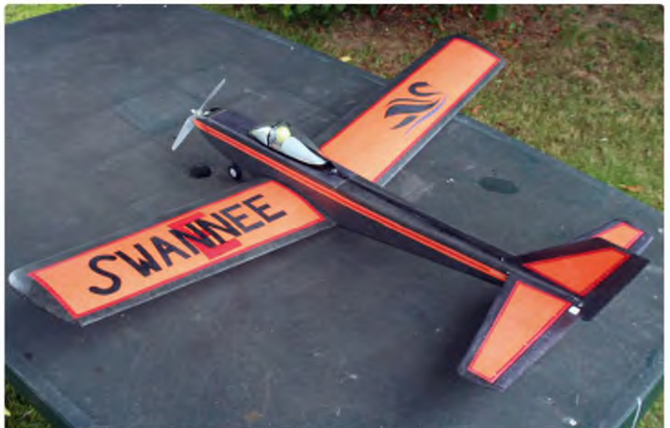
George is a long time Swanee fan; his current version is discreetly upgraded to electric power and rudder/elevator/throttle control. And according to the graphic on the wing, becomes the 'Swanee-E'!
