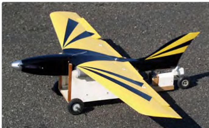
Pipedream mounted on launching trolley as an alternative to hand launching
