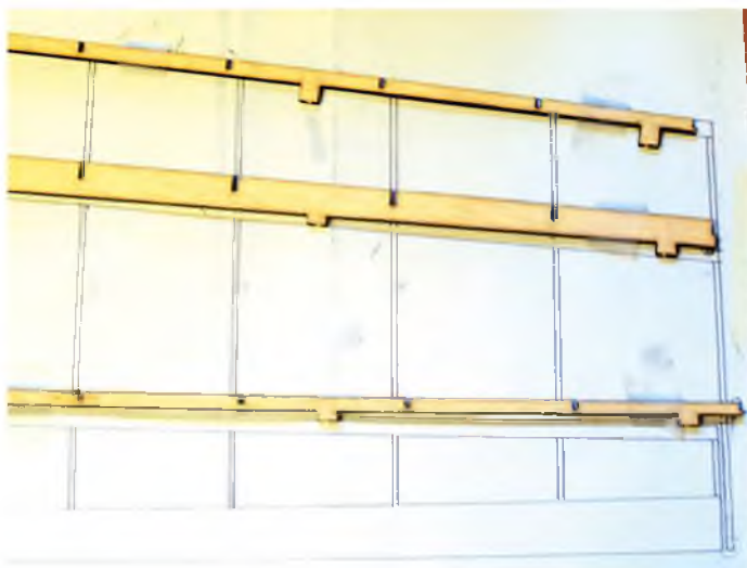
Start of the wing build. Laser cut false LE, mainspar and false TE set up
