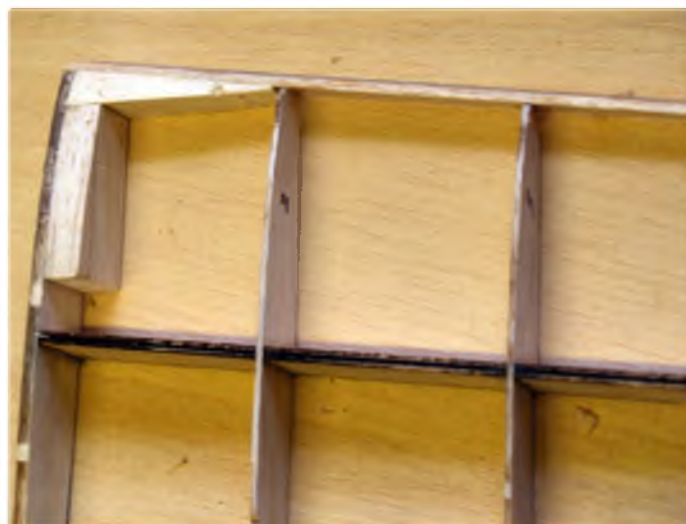
Wing construction at LE and centre section
