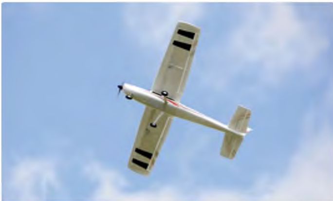
With the bomb doors safely tucked away the cleaned up Sensei shows her sensible proportions. Black stripes under the wings provide a simple but clear means of orientation
