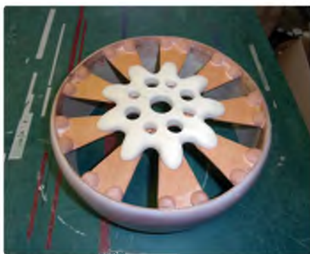
'Crankcase' shaped and rocker boxes fitted
