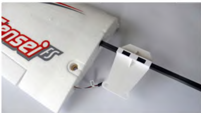
The square joiner and integral plate provide a secure fixing for the wing panels
