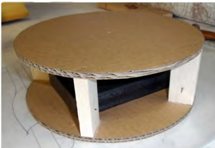
Cowling building frame
