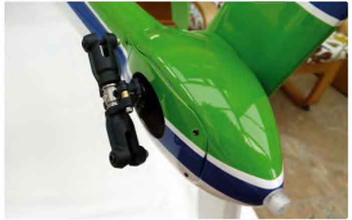
Tail rotor cover in place. It just slips over the rotor hub and you can also see the rear anti-collision light
