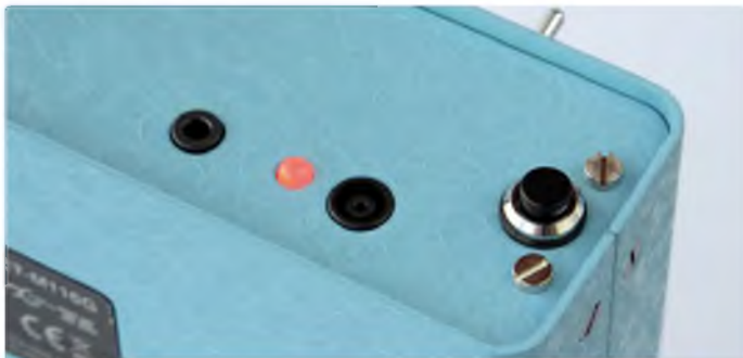
The other side of the top panel is home to the Trainer button, charging and trainer jacks, and the power lamp
