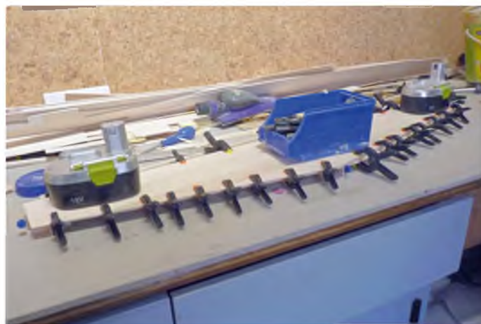
Tailplane final sheeting added
