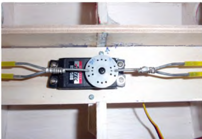
Flap servo with twin snake connectors
