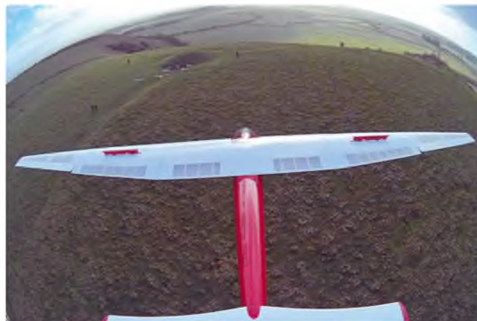
The mixing of brakes and ailerons is shown nicely in this on-board shot
