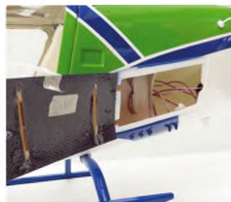
This is the luggage compartment where the lighting cables live. I used it for the LED control board
