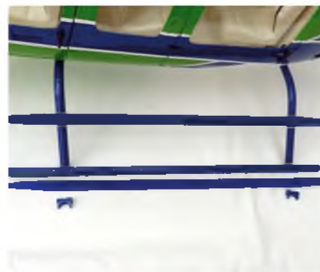
Skids with the step bar and showing the brackets that hold it in place
