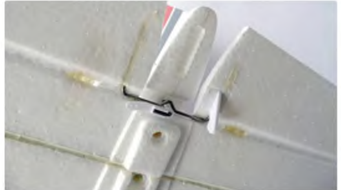
Tail pushrods use swing keepers to connect to the control horns
