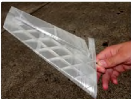
Stade Team Hydra's X-Wing tail surfaces are all 3D printed
