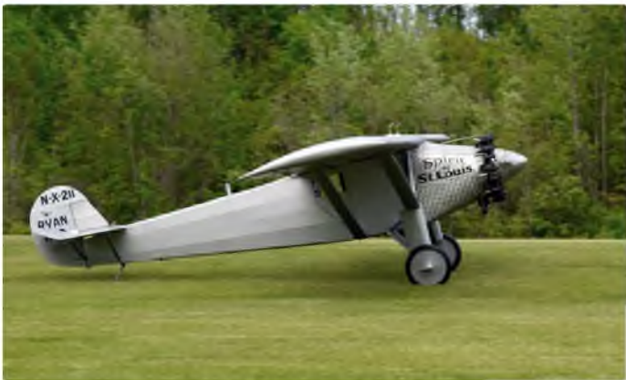
The Spirit taxiing after landing. Full up elevator is used to push down on that tail-skid to slow her down
