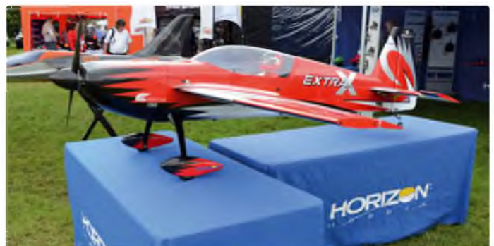
Horizon Hobby's display tents were back on the trade line for this show. Pride of place went to the Hangar 9 Extra 300X 120 cc ARF, a 35% scale version of the mid-wing aerobat. It features foam core balsa sheeted wings with dual carbon-fibre wing spars. The huge rudder is fitted with flat hinges so it can be removed for storage when the long hinge pin is pulled out
