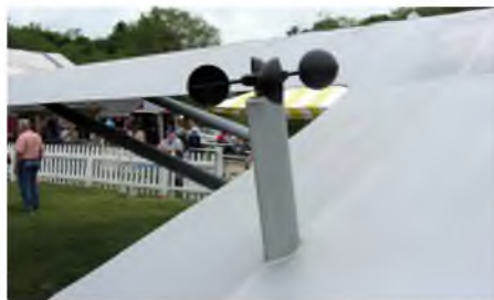
Anemometer mounted on top of the fuselage
