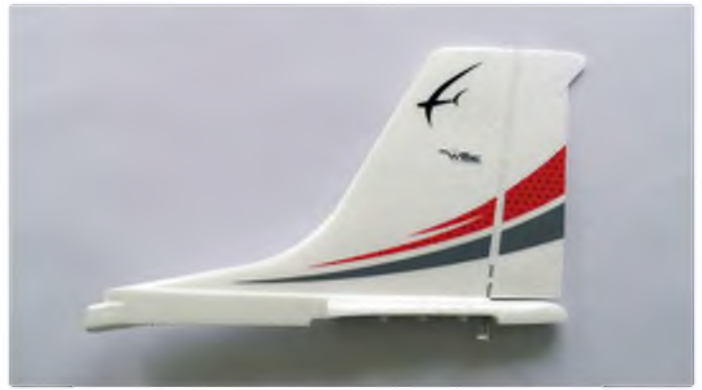
The tail parts are neatly moulded. They jig together and lock into place at the rear of the fuselage
