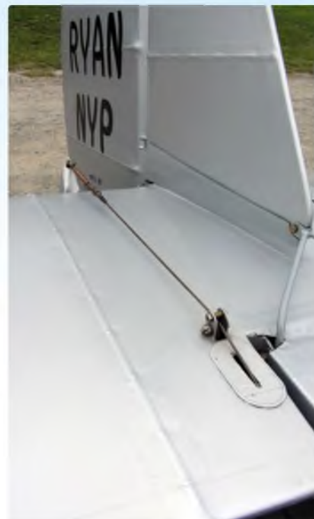
Above & below: Tail details, showing the corrected rudder shape
