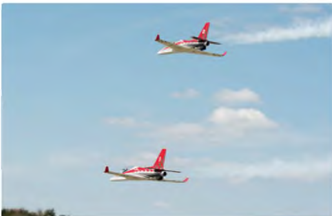
Red Flag Freestyle Champions, Team Viper, consisting of Californians Mike Adams and Ken McSpadden flying their 1/5 scale Skymaster Viper Jets. 102 in wingspan, 39 lb, JetCat P-180 RX turbines, Spektrum DX-18 radios
