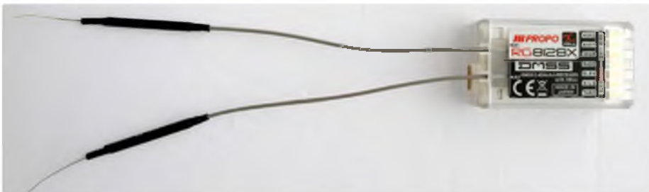
The RG812BX eight channel XBus receiver supplied makes a good starting point to use with the 14-channel transmitter
