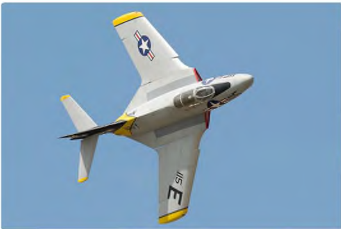
Gerardo Diaz's Skymaster F9F Cougar, 1/5th scale, 90 in wingspan, 34 lb. JetCat P-180RX1 turbine, Spektrum DX-18 radio
