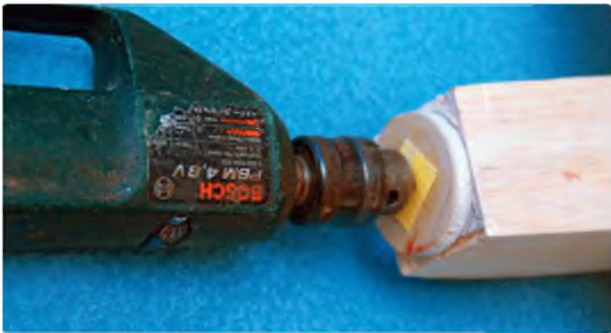
Sandpaper disc bolted to drill to obtain a true spinner outline
