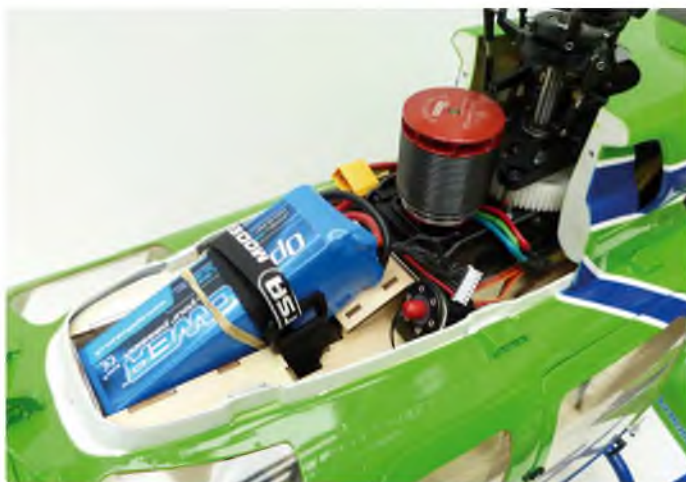
Packs in place and the SPS magnetic switch conveniently placed
