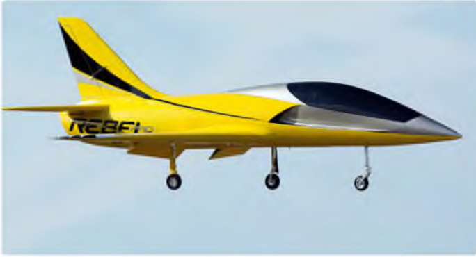
Columbian, Shneider Fajardo's Rebel Pro. 40 lb, Kingtech K-210 turbine, Spektrum DX-18 radio
