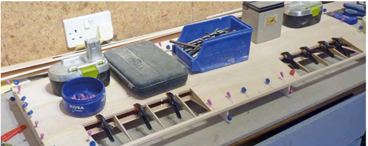
Centre section with top sheeting added and weighed down on jiggging supports
