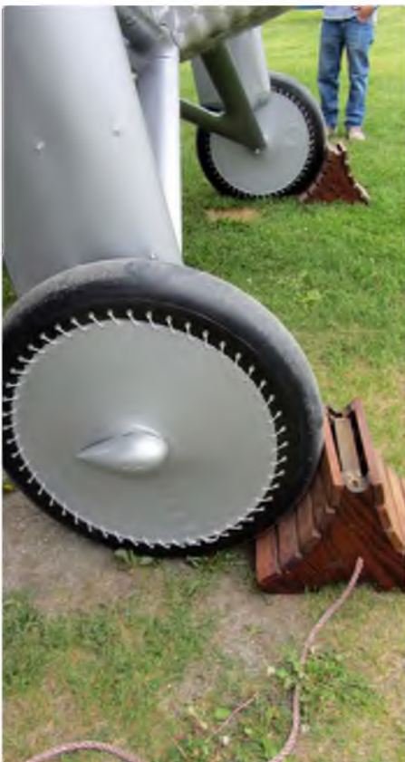
Above & below: Undercarriage details. The wheels have their covers and are nicely laced
