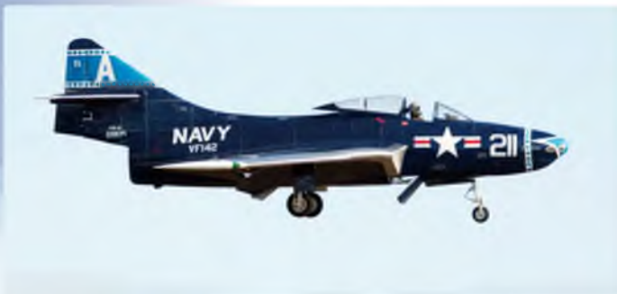
Red Flag Scale Jet Champion, Peter Goldsmith's Skymaster F-9F Cougar. 1/5 scale, Kingtech K-210 turbine, Spektrum DX-18 radio
