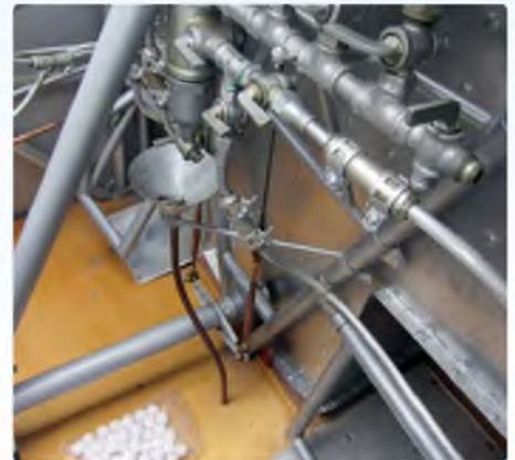
The Lunkenheimer valve or 'Gascolator'. This valve contained a trap to drain away any water in the gas before it reached the engine. The funnel and tube drain directly through the floor. This valve was supplied by the Smithsonian's National Air & Space Museum, along with a tachometer, and oil pressure and oil temperature gauges
