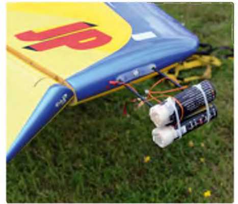
Close up on the wingtip mounted smoke canisters
