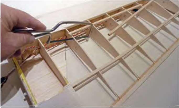
Retro-cutting the slots for the airbrake aperture
