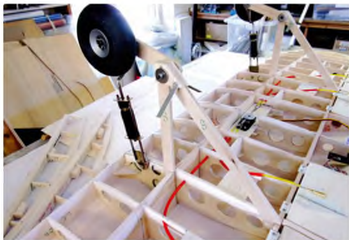
Undercarriage legs fitted
