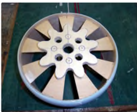
Foam cowling ring and balsa 'crankcase' fitted
