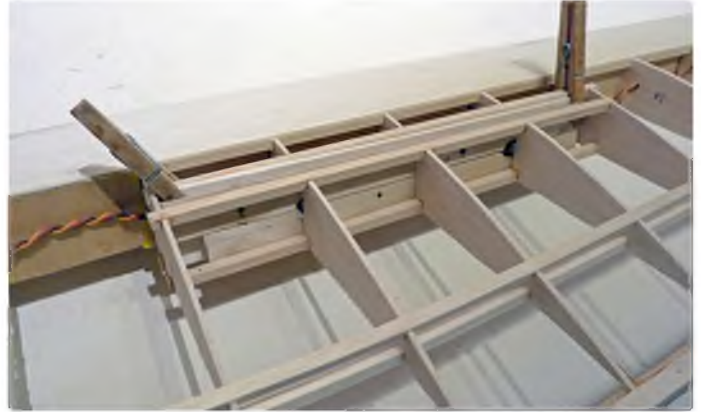
Test fit of the airbrake assembly
