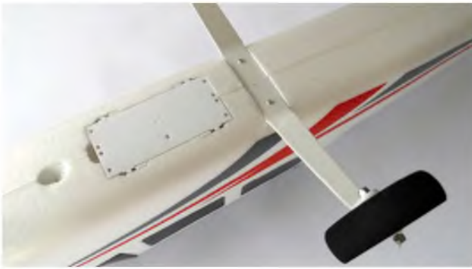
A recess in the fuselage just aft of the 'bomb drop' doors shows where the undercarriage is meant to fit. Two screws hold it securely in place
