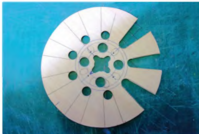
'Engine' back-plate being cut out
