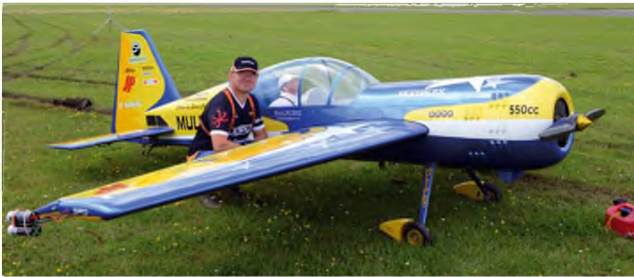
Steve Carr lends a sense of scale to his mighty 55% Yak 54, assembled from the Pilot RC kit. The 4.6 metre span model is operated using 22 Hitec servos and four Multiplex receivers, with telemetry. Power is by Steve's own design four-cylinder boxer two-stroke engine of 550 cc capacity
