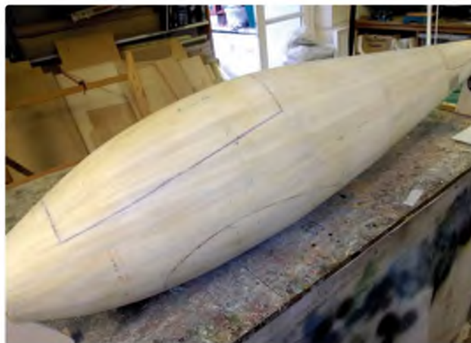
The whole fuselage shell weighs just 23 ounces
