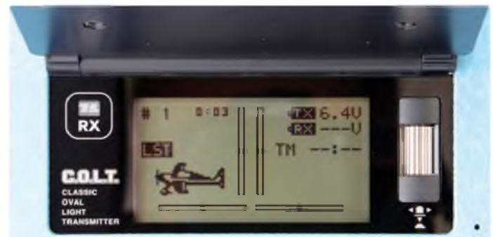
Main display screen. The icon changes depending on the aircraft type. It also shows receiver voltage via telemetry when the model is switched on
