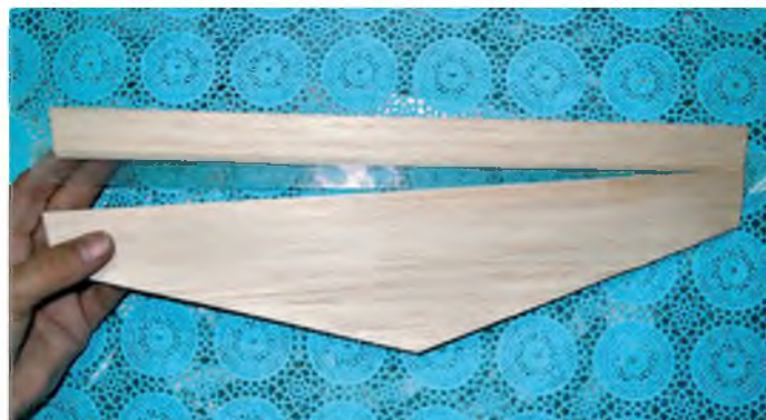
Cut out and fit the 5 mm (3/16") balsa stabiliser and elevator, then cover as preferred. Hinge with glass reinforced tape
