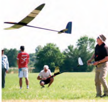
Pete Mitchell with his Ultima. This model is one of the first large electric Soarers to use pressed wings, where the skins are bonded to a foam core, a technique commonly used in F3K (hand launched glider) construction. Materials need considerable care in production, after which this 4 m glider can fly at 1100 g!
