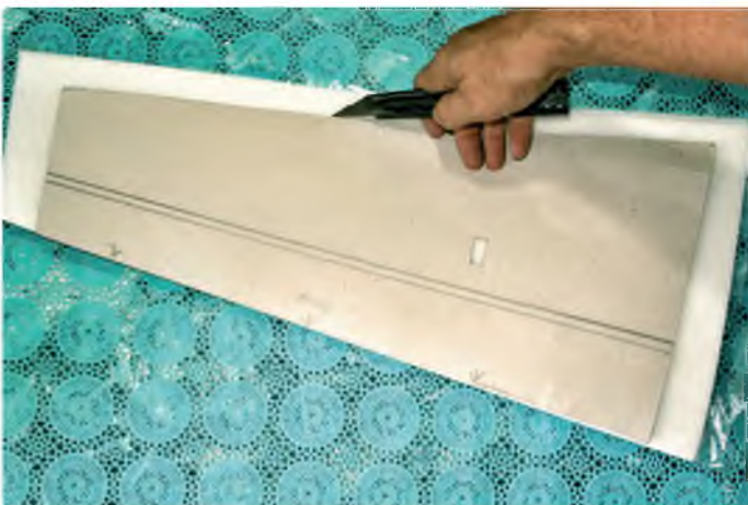
Trim along the trailing edge, root and tip with a sharp modelling knife
