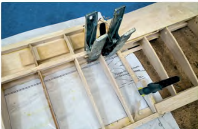
First stage of joining the wings. The second R-1 has just been fitted at this stage
