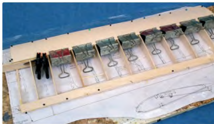
Gluing down the top leading edge sheet using lots of clamps and map pins
