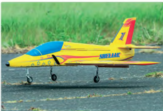
Terry Jessop's Red Wings Sheliak model. The Sheliak has a 2 metre wingspan and a JetCat P80 turbine
