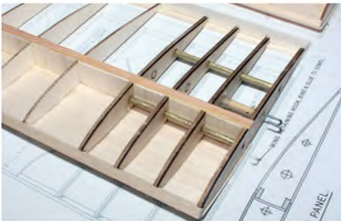
Vertical balsa webbing added to all panels
