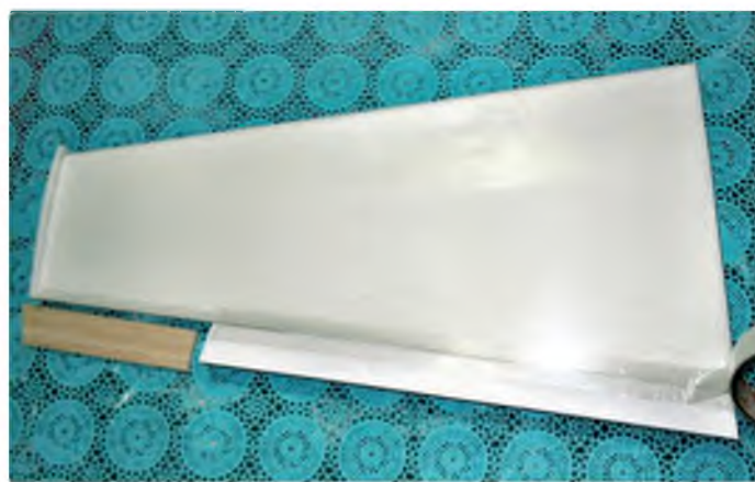
Add tips and ailerons, plus the balsa trailing edge insert, then gently sand smooth
