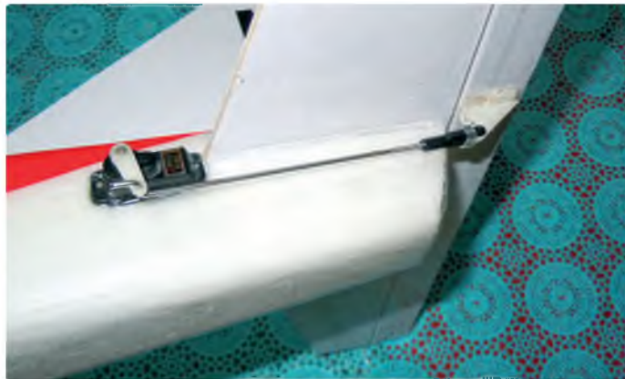
Final aileron and elevator servo installs, showing the pushrods and linkages
