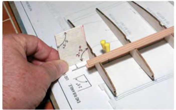
An angle template was made from scrap balsa to attain the correct dihedral for the roots and tips
