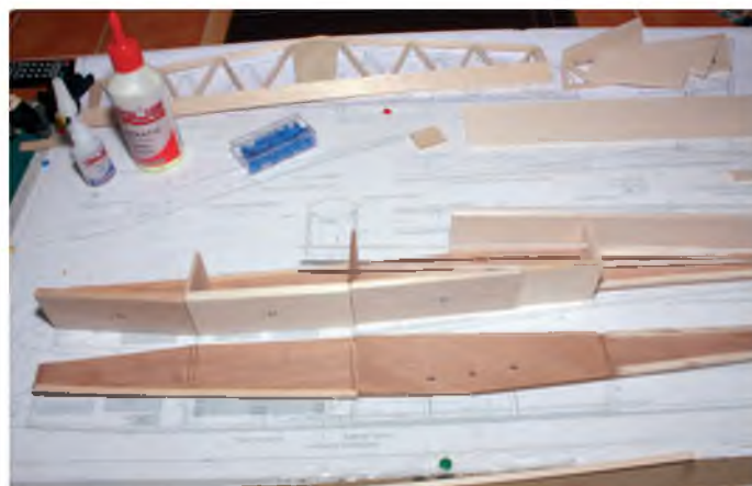
Sand to shape the bottom sheeting facing angles and fit the balsa longerons
