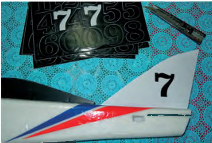
Attach the Correx profile canopy and the 5 mm (3/16") balsa fin with a hot glue gun. Add any decals required
