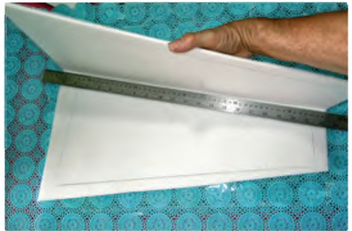
For the 'folded wing' method cut the wing panel oversize. Then mark and fold
