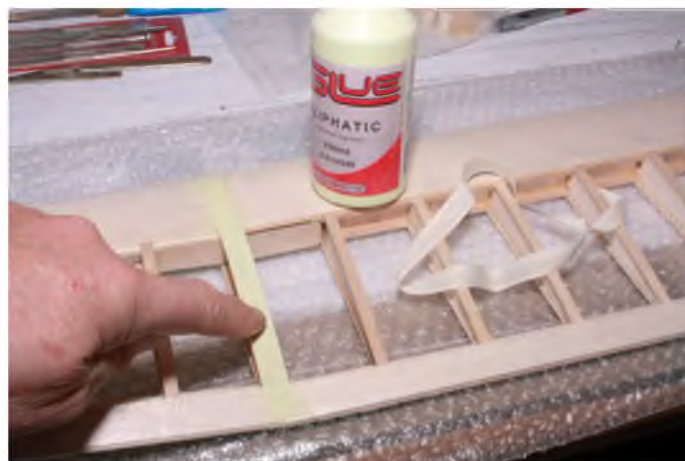
Applying the wing joiner ribbon with aliphatic glue
