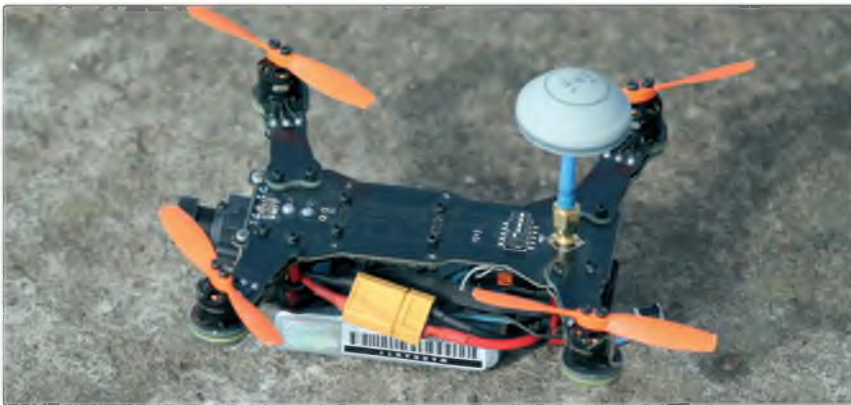
The 180 size racing quad is significantly smaller so flying one without FPV can give orientation problems
