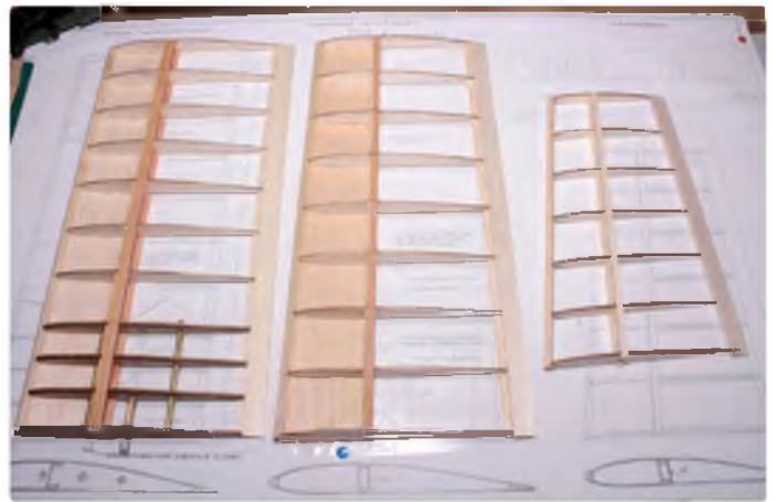
Bottom sheeting the root and centre wing panels
