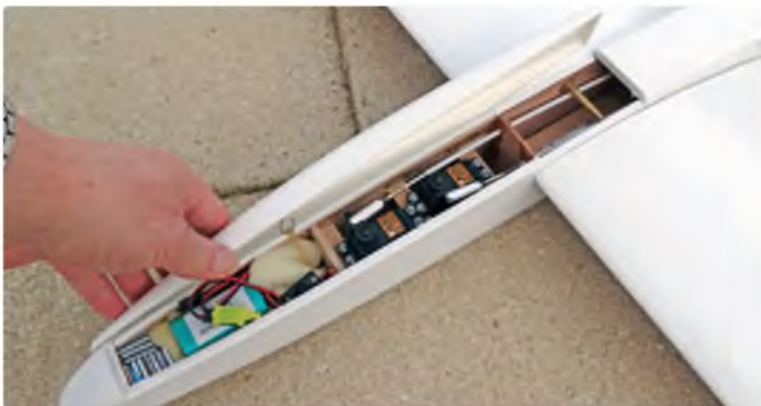
Radio bay installation
