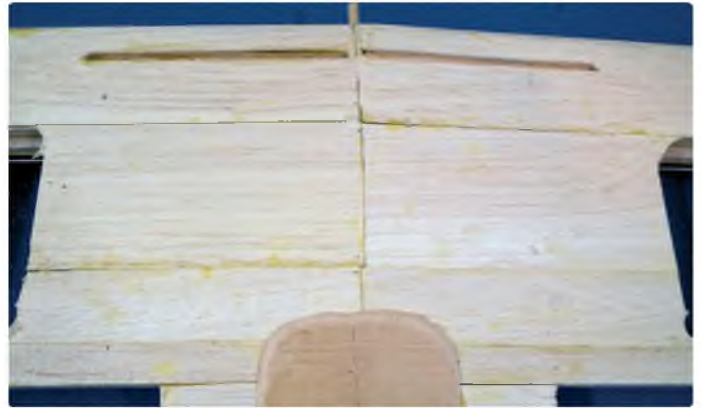
Underside of centre section showing the ply plate for the wing bolt head and U/C grooves
