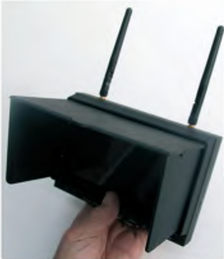
A sunshade is effective in most conditions
