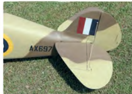
Fine scale modelling continues at the tail, which is made using the balsa core method of construction
