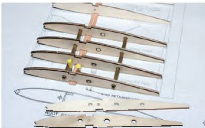
Plywood ribs are doubled with balsa root ribs to give added support for the brass joiner tubes. The centre hole is for the wing retaining hook dowel
