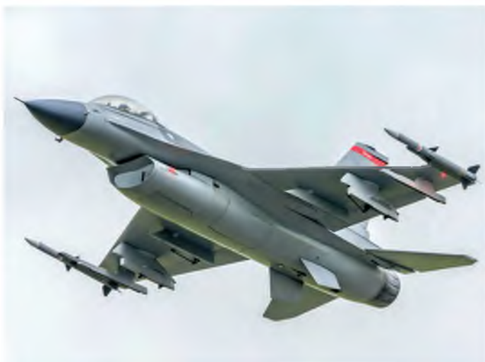
Mark Hinton's Jet Legend F-16. The model has a JetCat P180 turbine and also features a light system to simulate the afterburner
