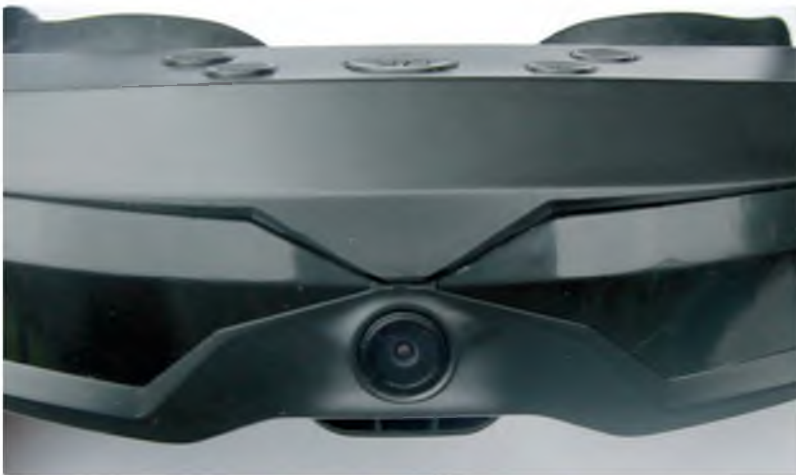
The forward facing camera on these Spexman goggles allows you to see where you are and what's happening around you, if required
