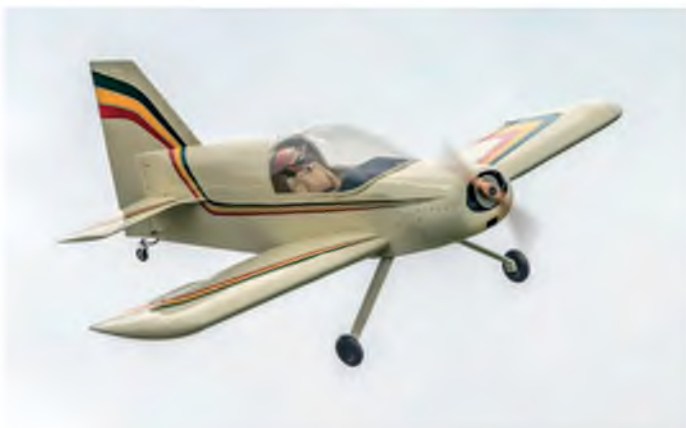
Paul Needham's Bede BD8. The 11' 6" wingspan Bede is powered by a DLE 222 petrol engine
