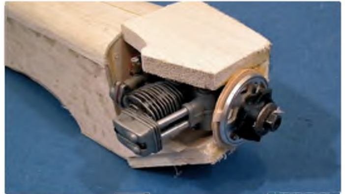
Half inch sheet cowl pieces glued in place
