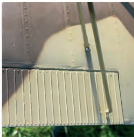
These pictures show the excellent rib stitching and corrugated control surfaces
