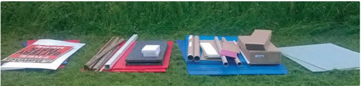
Scrapheap materials were a selection of Correx sheets, plastic and cardboard tubes, and a small assortment of balsa (not shown)
