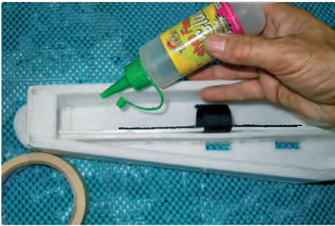
The radio tray is now glued in place
