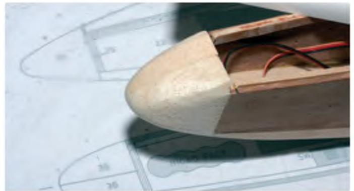
The nose block is shaped and sanded
