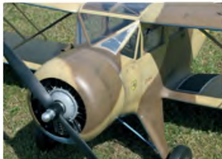
Like a lot of British scale modellers, Paul has chosen a Laser four-stroke engine to power this scale masterpiece. A Laser 120 four-stroke is well disguised behind the big dummy radial and cowling
