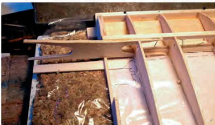
Dihedral brace being glued in place
