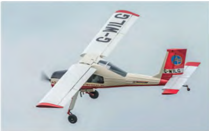
Mathew Harrowven's Wilga PZL-104 is a Frisch Modellbau kit. It has a DLE 170 cc petrol engine and a wingspan of 3.7 metres
