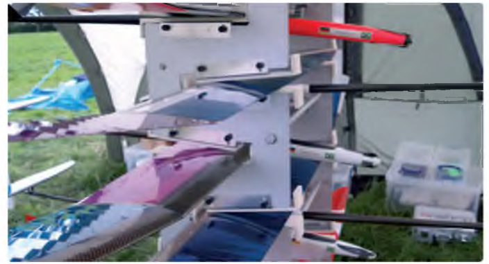
Each of the wing slots in the 'Freundl Tower' is adjustable to accommodate any particular aerofoil thickness. Any such system needs to be well fixed to the ground; the prospect of it blowing over does not warrant thinking about!
