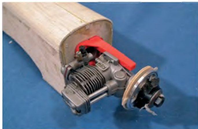
The spinner backplate is used to locate the nose ring accurately
