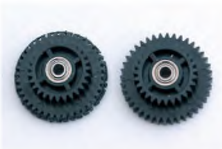
Compare these two gears – very mangled teeth on the damaged one
