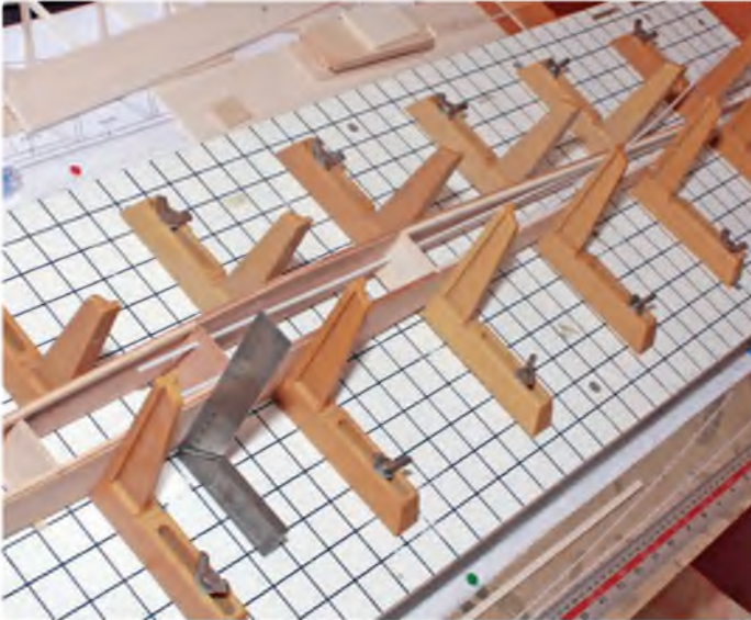
Using a jig is the best option for correct alignment of the fuselage
