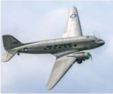
Built by John Lambert over 20 years ago, the 10 ft wingspan Dakota flew very well in the hands of son, Perry. Model has two Power 52 electric motors
