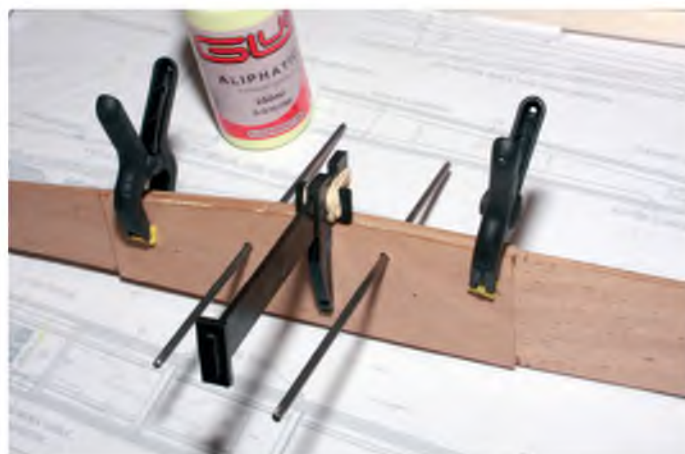
First stage of fuselage assembly is to align the wing joiners and glue doublers with back-to-back sides
