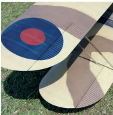
These pictures show the excellent rib stitching and corrugated control surfaces
