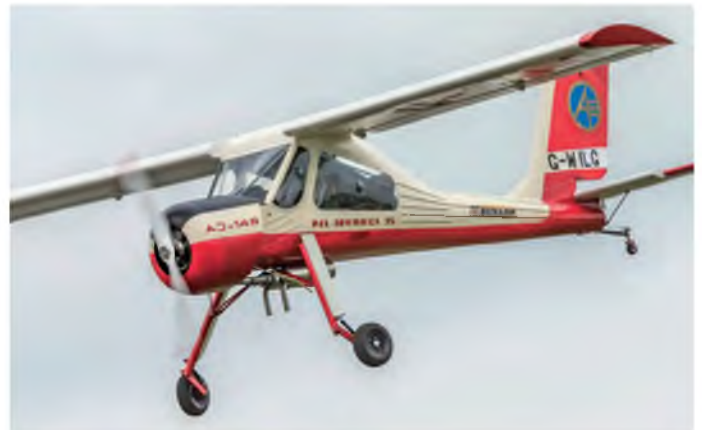
Mathew Harrowven's Wilga PZL-104 is a Frisch Modellbau kit. It has a DLE 170 cc petrol engine and a wingspan of 3.7 metres
