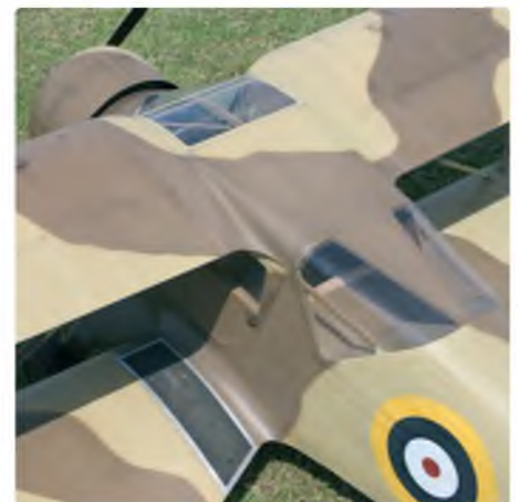
Centre section details include the sleek wing fairings, the wing walk-way and the nicely reproduced curved rear cockpit glazing
