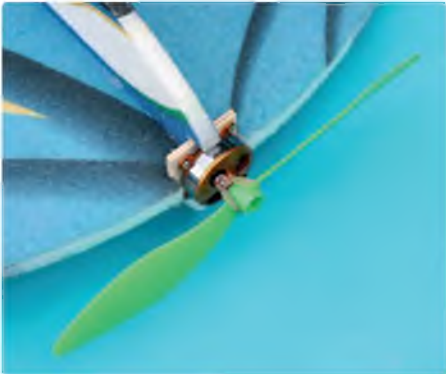
I used a 3 ply motor mount and more powerful brushless motor
