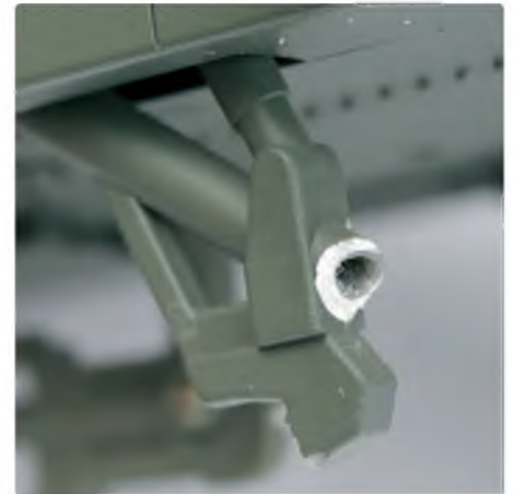
More pilot induced damage. The U/C leg needed a metal pin inserted but drilling a 1 mm hole in the leg strut has to be done with great care
