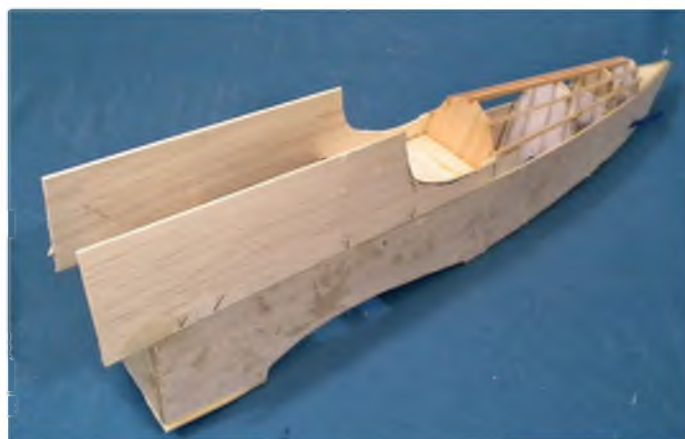
First stage of rolled sheet turtle deck
