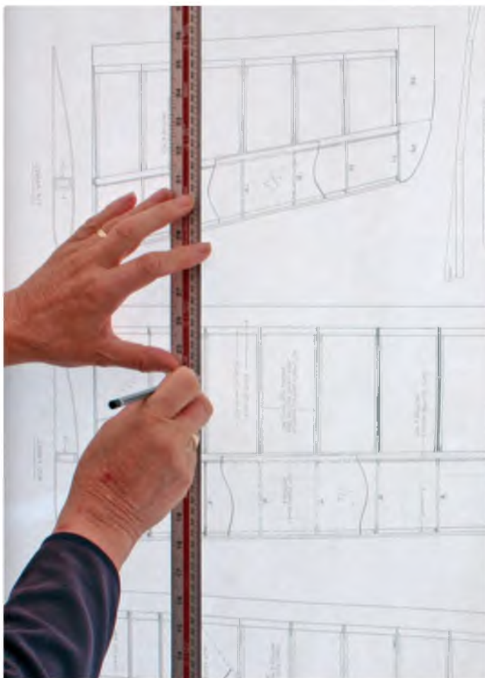
To construct the left wing, first the lines were traced through onto the back of the plan (using a glass door for lighting)
