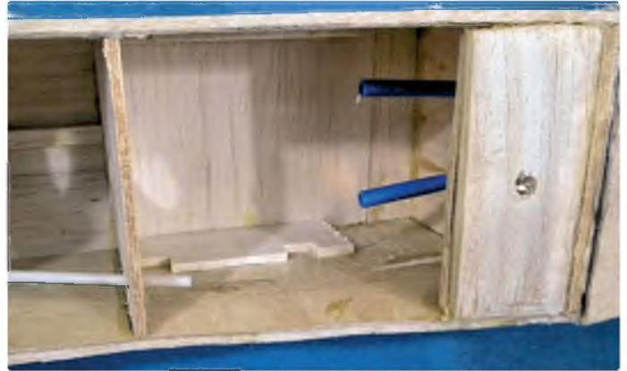
Servo bay showing treblers fitted to the sides
