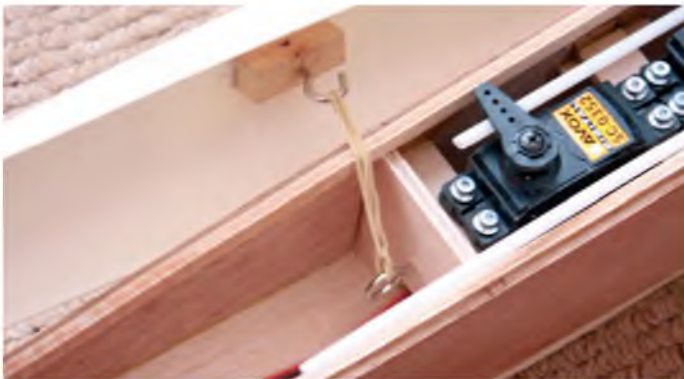
The method for retaining the canopy
