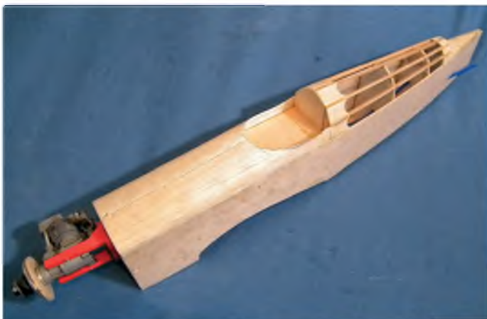
Turtle deck bent over and glued down. Stringers have also been added and the engine temporarily installed
