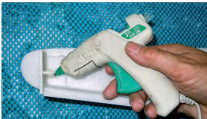
Attach the front former/motor mount with hot glue for added strength
