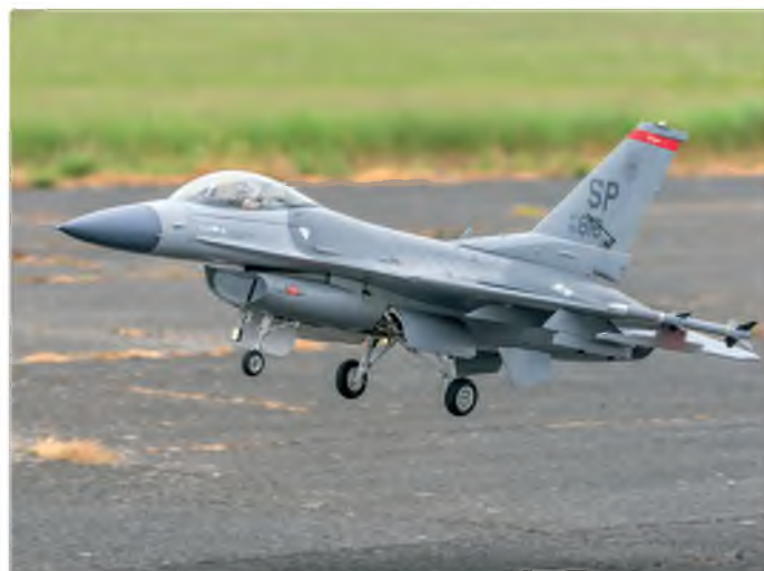
Mark Hinton's Jet Legend F-16. The model has a JetCat P180 turbine and also features a light system to simulate the afterburner
