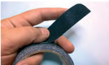
Grip tape (from a pound shop) is excellent for fitting to hand launch models and is ideal if you have limited strength in your fingers!
