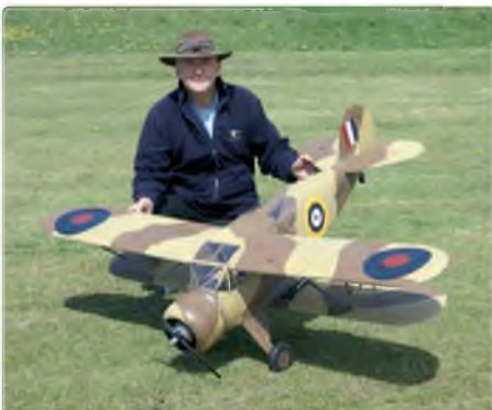
Built to 1:5.5 scale, the 72 inch wingspan YKC makes a nicely sized model aeroplane
