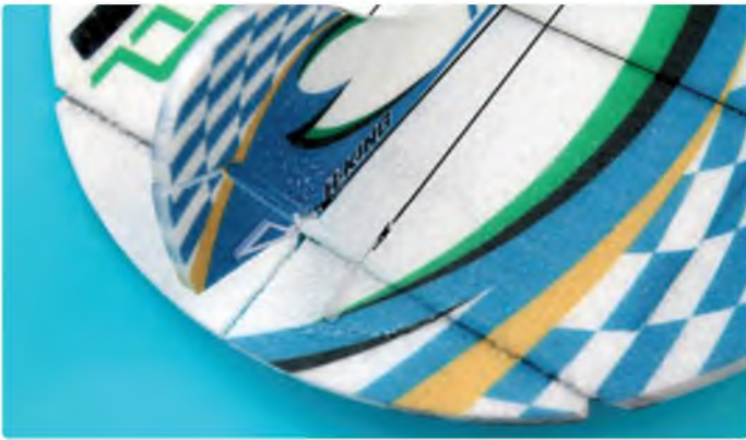
The elevator was cut in two to make the elevons. The additional rudder servo can be fitted close to the elevon servo
