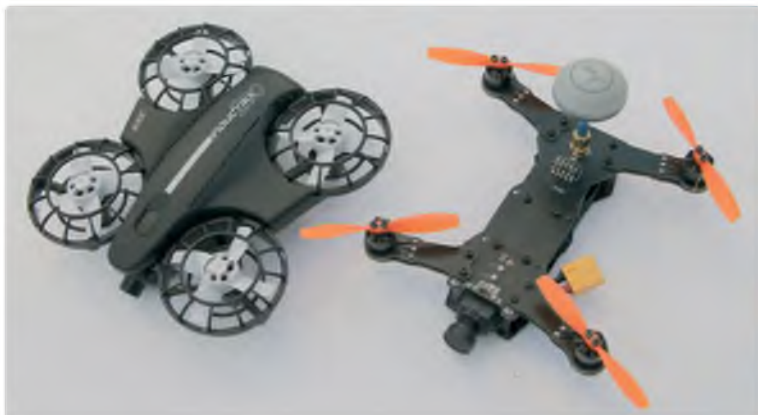
The Blade Inductrix 200 FPV quad is of a very similar size to a 180 racing quad
