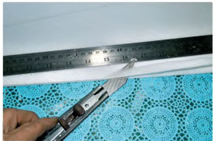
Carefully chamfer the trailing edges and sand to fit, ready to join
