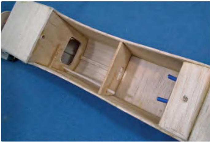
Inside the fuselage showing the wing bolt plate under the scrap balsa infill
