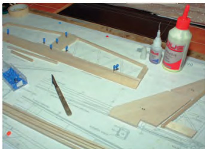
Laying up the tailplane from medium grade balsa and pre-cut fin parts
