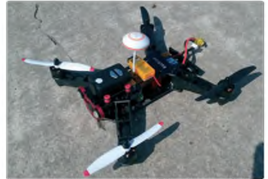
This top mounted Mobius camera can provide a high quality video record of your flight
