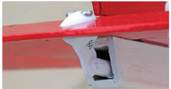
The elevator pushrod exits from inside the fuselage directly to the elevator horn
