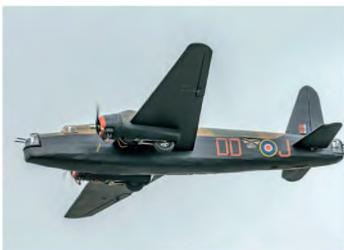
The Vickers Wellington built from a Tony Nijhuis kit by Tony Hooper. The 4 metre wingspan model is fitted with two Zenoah Zg 26 cc petrol engines
