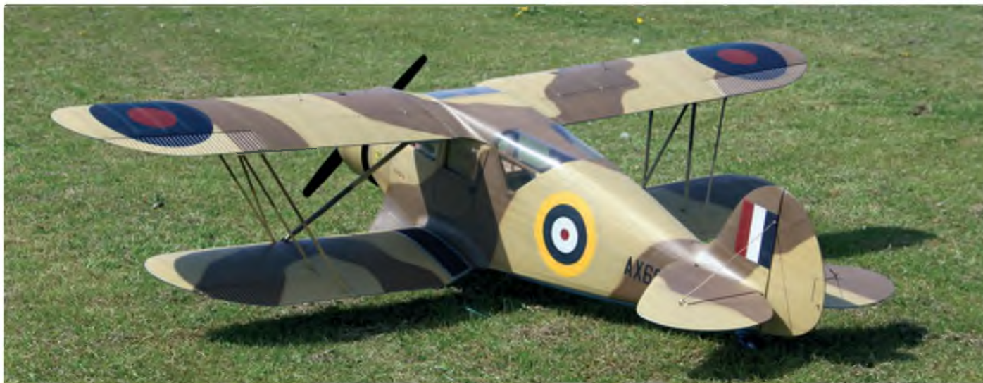
The Solartex covered camouflaged model is painted with Vallejo Model Color water based paints. Azure on the undersides, US Field Drab for the dark brown, with a three to one mix of Buff and Middlestone for the light brown
