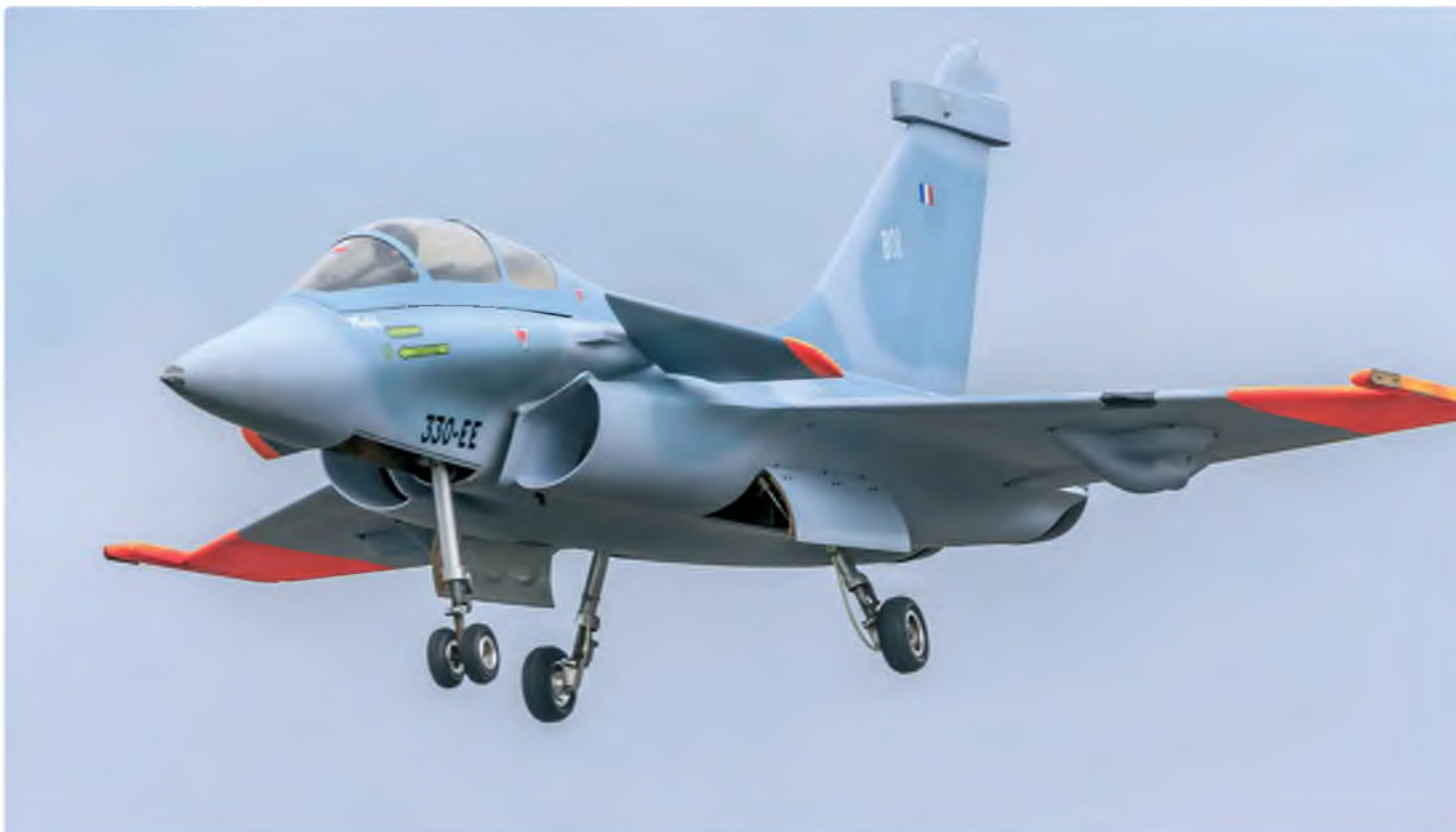
Diminutive Rafale of Dave Wilde. The model is a Fly Eagle kit and has a 45" wingspan and uses a Kingtech 80 jet turbine
