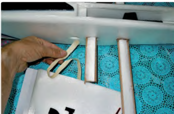
Fit the 1/4" thick hardwood spars with foam packers (top only). Apply hot glue to the spar and slide the wing panels on
