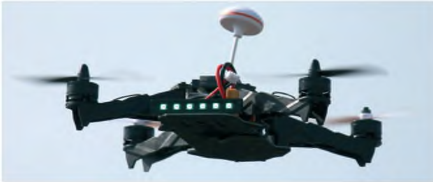
Even in quite bright sunlight a strip of rear lights show up well, especially the newer versions with alternating colours and animation
