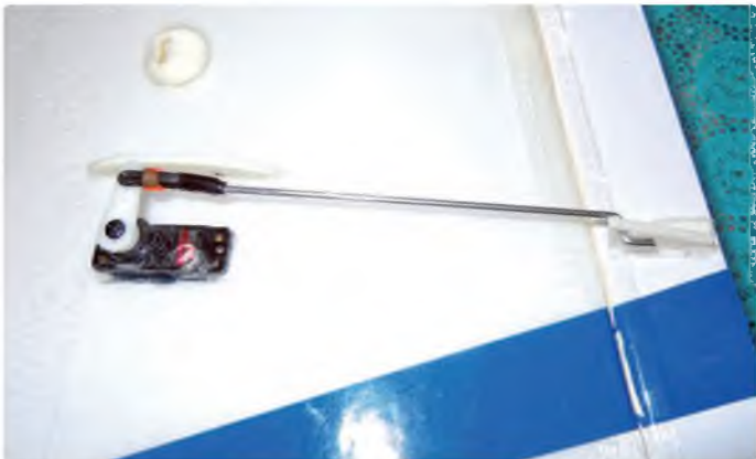
Final aileron and elevator servo installs, showing the pushrods and linkages
