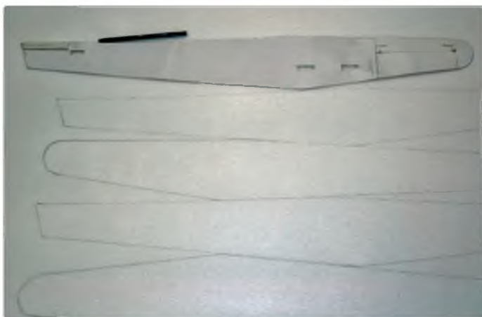
Make a template from the plan and draw up the four fuselage sides
