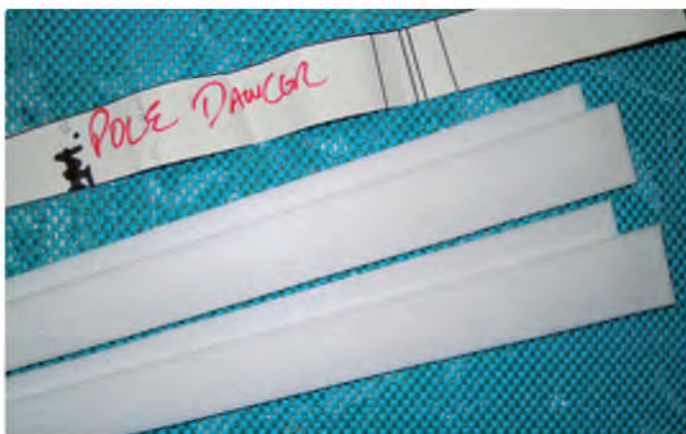
Cut four tapered parts for the fuselage, top and bottom. Then laminate to make two parts
