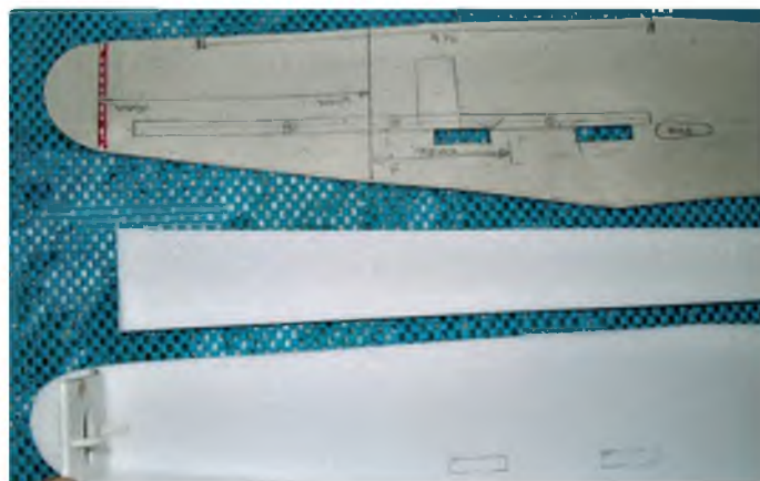
After sanding the edges smooth test fit dry, then glue the bottom to one fuselage side
