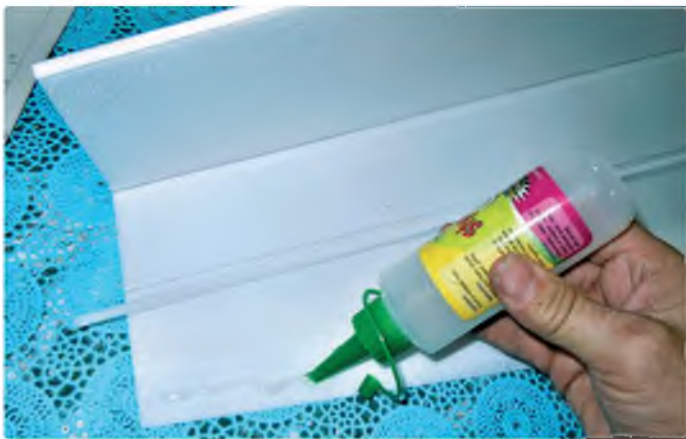
With the spar inset, glue the wing trailing edge, then tape up and allow to dry
