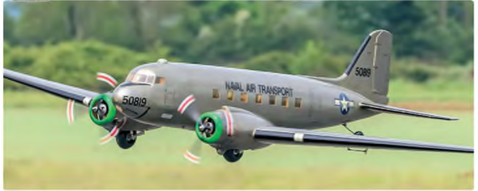
Built by John Lambert over 20 years ago, the 10 ft wingspan Dakota flew very well in the hands of son, Perry. Model has two Power 52 electric motors
