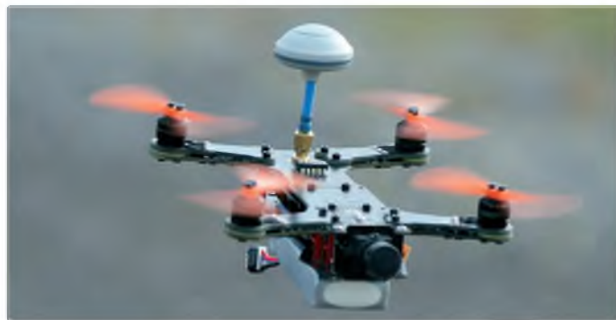
The camera is angled to match the nose down tilt of the quad in fast forward flight
