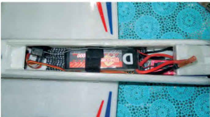
Position the battery to obtain the correct C of G
