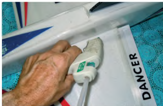
Apply hot glue to the root edges of the wings and stabiliser to hold them in place
