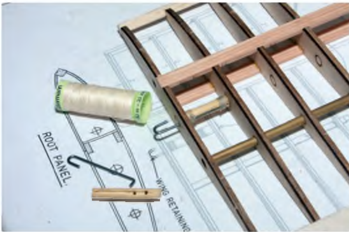
Assembling the wing retaining hook dowel
