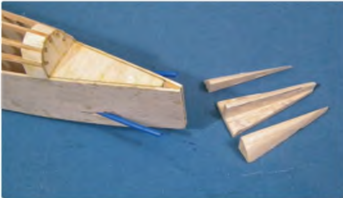
Making the fairing blocks that fit at the base of the fin
