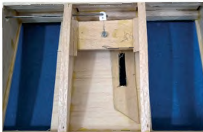
View of the bellcrank bay and lower sheet with pushrod slot
