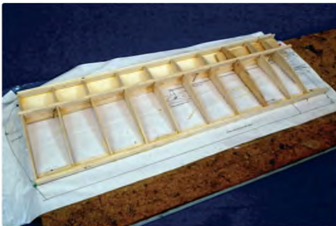
Leading edge added and lower L.E. sheet brought up and glued in place
