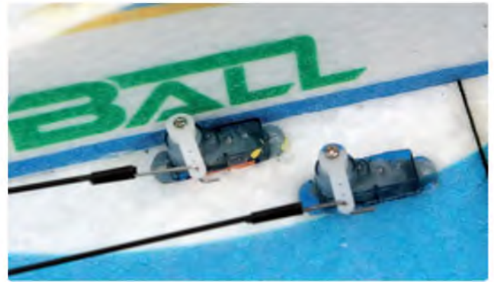
The elevator was cut in two to make the elevons. The additional rudder servo can be fitted close to the elevon servo
