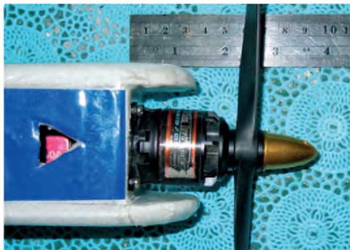
Motor side thrust is shown. Don't forget that all-important cooling air vent!
