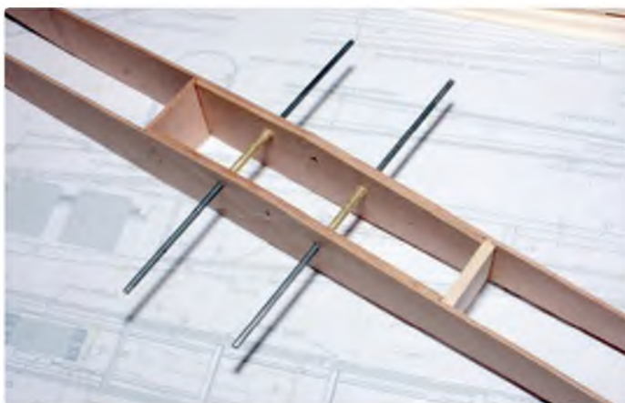
Test fit the joiner tubes and fit formers
