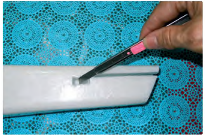
After adding the second fuselage side and sanding, cut out all the required holes, servo recesses and an access hatch
