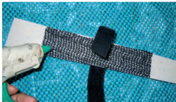
Attach a small piece of rubber non-slip mat and fix a Velcro strap to the radio tray floor for the LiPo battery restraint
