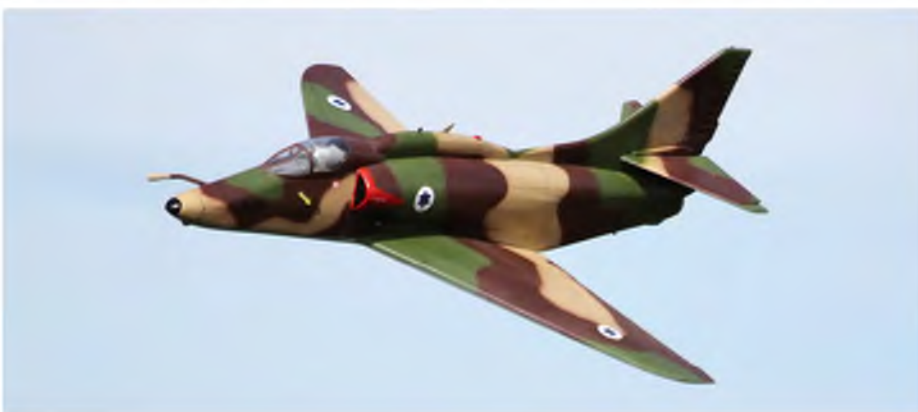
Peter Garsden's A-4 Skyhawk in flight. Built from the Traplet wood pack and with a span of just 36" the model performed very well and looked totally convincing in flight. Refuelling probe is a 3D printed part – contact the PSSA if you'd like one
