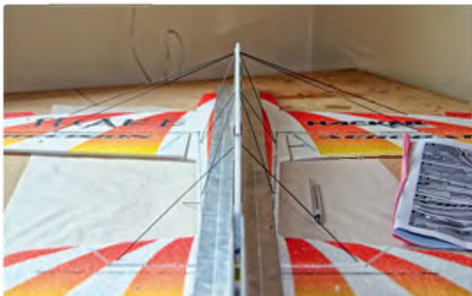
Aluminium angle on both sides of the fuselage keeps things straight whilst the carbon rod reinforcement is added
