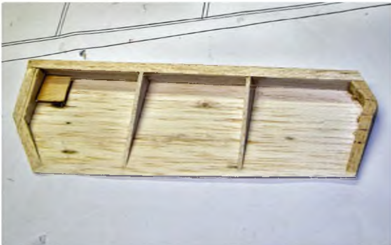
Rudder before final 3/32" balsa sheet is added
