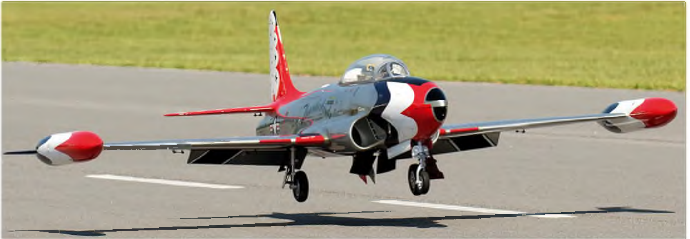
Franco DiMauro's T-33 from the Fei Bao kit. 1:4 scale, 100 in wingspan, Jet Rhino turbine, Spektrum DX-18 radio. Franco earned first place in Pro Jet Class
