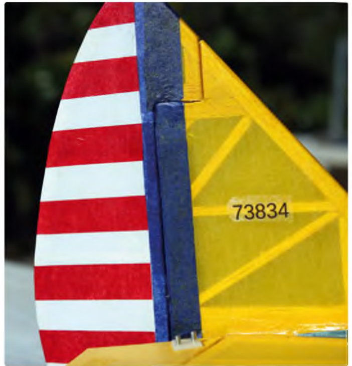
My American modelling license number, laser printed on white tissue and applied with water based dope substitute. The white tissue virtually disappears when 'doped'. Don't use real dope though as it will melt the toner!
