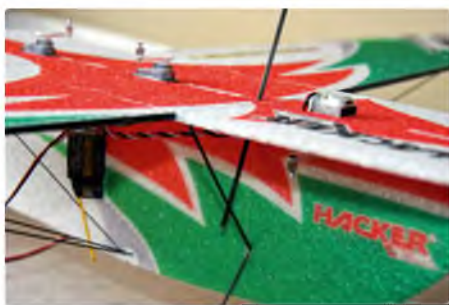
The servos are installed before the top fuselage is added. Vertical carbon strip is about to be glued in to align the two vertical fuselage halves
