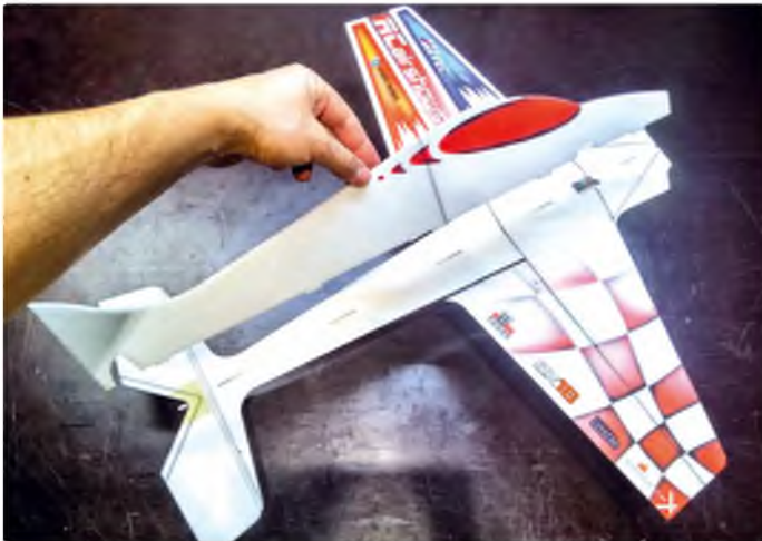
Place the vertical top fuselage onto the already assembled model
