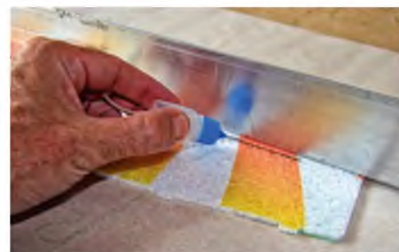
A dropper bottle was used to accurately control the amount of glue used
