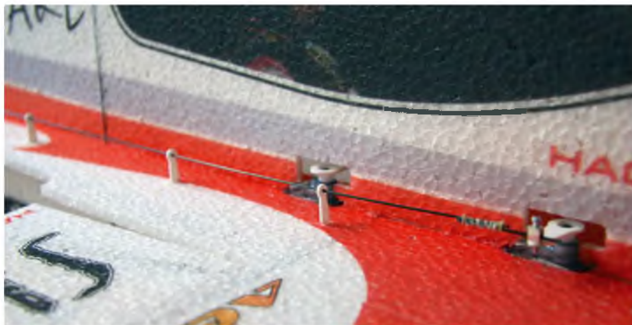
The pushrods are supported down the length of the fuselage
