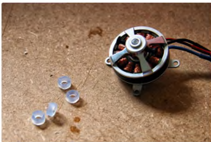
Grommets made out of fuel tubing were used to aid thrust line adjustment. The grommets can be seen clearly in the final assembly
