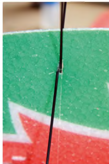
The undercarriage is reinforced with Kevlar thread
