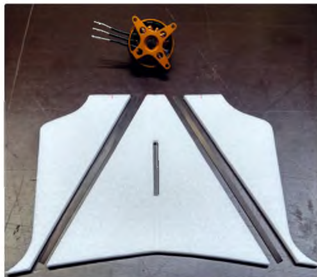
Motor mount reinforcement is made from 100 mm by 0.13 mm thick flat carbon strip
