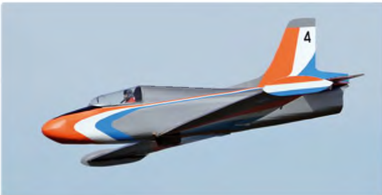
Not all models flown on the slope are balsa or foam creations! Harry Twist built this superb little Impala from Correx sheeting and it flies wonderfully well. It's certainly one of the cheapest routes to successful PSS flying if you fancied having a go!
