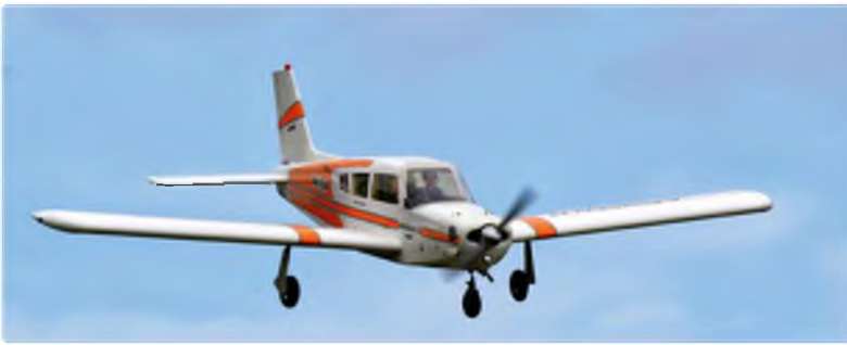
Left top & below: Bill's 15 lb Piper Arrow is powered by an RCV 91CD. The plane is over 10 years old
