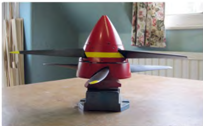
Painted and assembled spinner. The opposing pitch of the rear (driven) prop and the front (free-wheeling) prop can be clearly seen. The front spinner rotates with the driven prop
