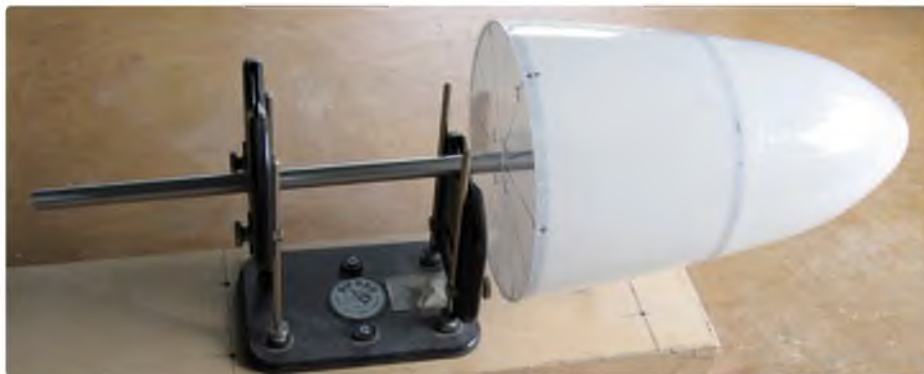
The epoxy glass Wyvern spinner on the balancer before being cut into three sections, for the CR prop. Balancing problems with the long spinner proved to be the Achilles heel of this design, although one successful flight was achieved before abandoning it
