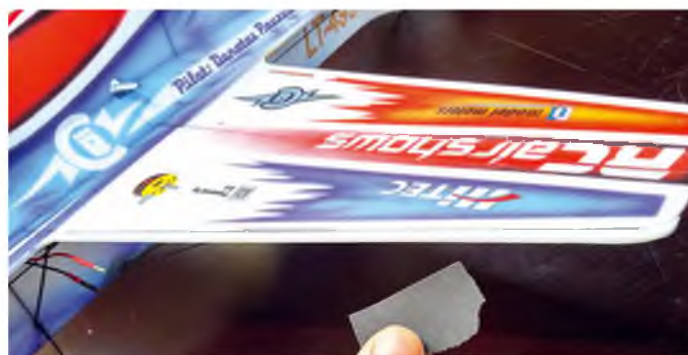
I believe that pylon racing models must have a rounded leading edge in order to create less drag in flight. So on the 3 mm leading edge I glue a piece of Depron and round it using sanding paper
