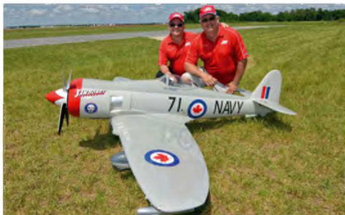
Team Sawbones, Greg Foushi and Bill Freeland with their Walt Carnes Hawker Sea Fury that earned them fifth place in the Unlimited Class. 1:5 scale, 93 in span, 45 lb, World Models kit. Moki 250 cc engine, Spektrum DX-18 QQ radio
