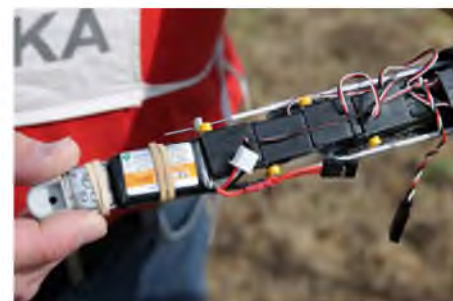
Front end close-up of Turi Hunziker's rocket glider. Four mini servos in a line, with the battery at the front. All pretty compact to improve boost prospects
