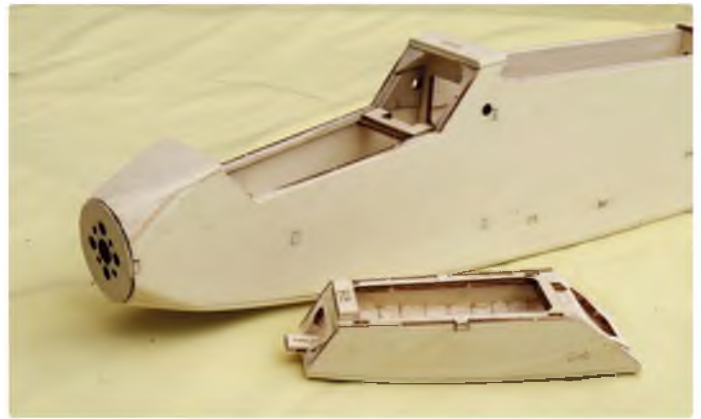
Once the upper ply sheeting on the nose has dried the canopy can be cut free. The rest of the canopy frame is fitted and the nose shaped to fit the spinner
