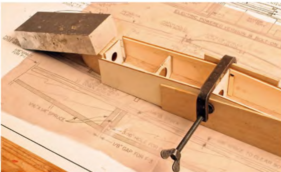
A slab sided fuselage is the easiest to build
