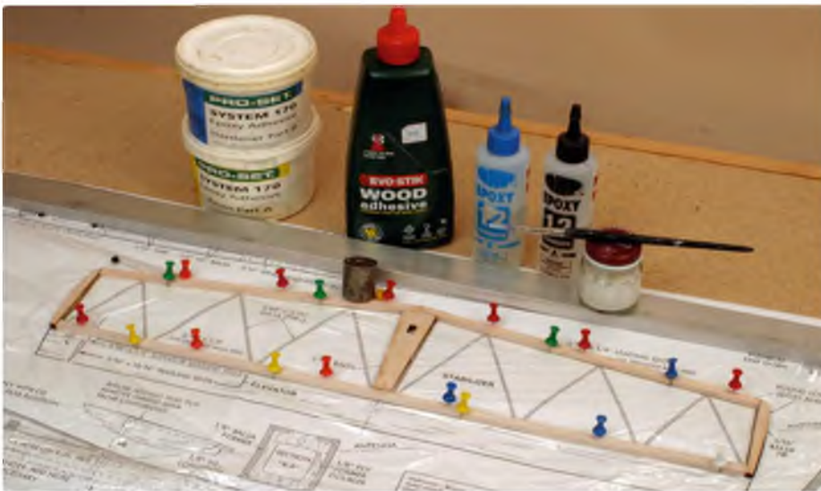
This tailplane is being built dead flat on top of the plan
