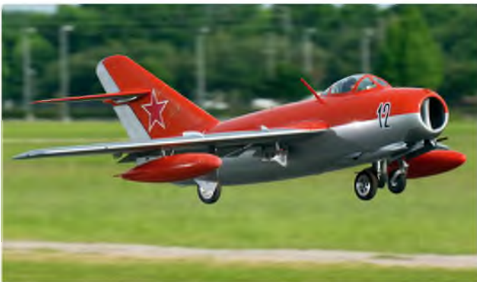
Mike Grady's MiG-15bis. BVM kit, 68 in wingspan, 22 lb, BVM electric ducted fan, Spektrum DX-18 radio. Pilot Dustin Buescher flew the MiG to first place in Team Class
