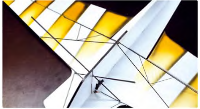
Landing gear, made from 1.5 mm carbon rod (length 180 mm), is attached to the airframe
