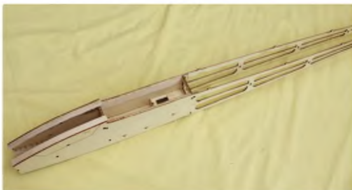
Clever design ensures that the fuselage sides are fully aligned, with no possibility of building a banana fuselage
