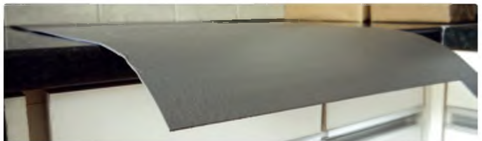
Curving Depron around a roll top kitchen work surface
