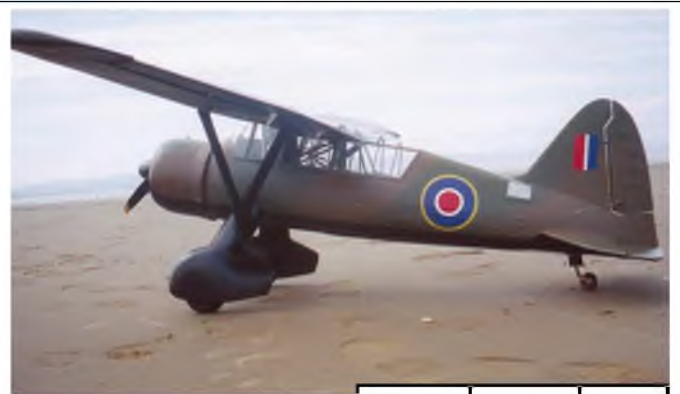
Westland Lysander (81") Power Source - .60 to .90 cu. in. 2-strokes; .90+ 4-strokes Wingspan - 81" / 2057 mm
