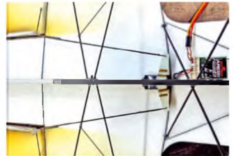
Control horns are made from 0.5 mm thick fibreglass sheet. The slightly bent aileron pushrods are attached to the servo arm, also made from fibreglass sheet
