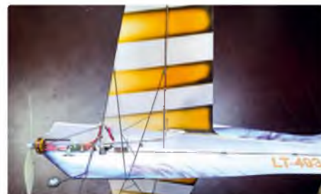
The elevator is controlled with pull-push system, with the servo mounted close to the nose. Make the pushrod from 1 mm by 520 mm carbon rod and support it at three points. For precise control a small ball link from a 250 size helicopter was used
