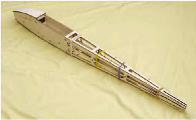
Assembled fuselage being held together with rubber bands while the glue dries. PVA glue was used for all joints
