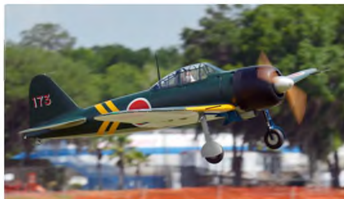
Beautifully detailed Zero fighter built from enlarged Meister Scale plans by Toshiaki Nakayama. 1:4 scale, 119 in wingspan, 50 lb, Moki 150 engine, Spektrum DX-18 radio. Pilot, Dino DiGiorgio earned first place in the Unlimited Class
