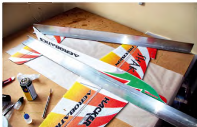
Adding the underside of the fuselage, using some aluminium angle (from B&Q) to make sure it is square
