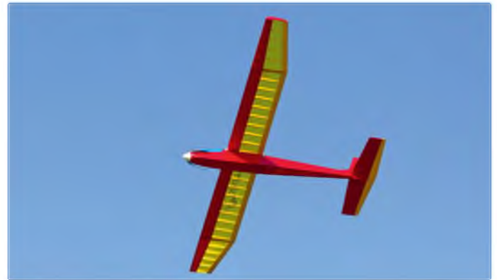
Overhead shot showing off the wing structure through the translucent covering
