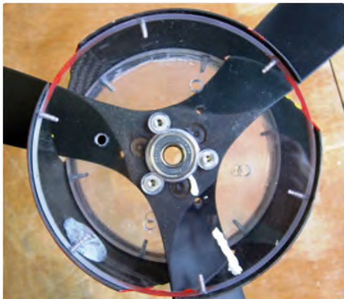
This is the free-wheeling prop, sandwiched between two 6 mm polycarbonate discs which have been drilled and tapped to accept M2.5 machine screws that secure the discs to the centre element of the CR spinner
