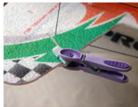
Keep the control surfaces straight whilst fitting the pushrods
