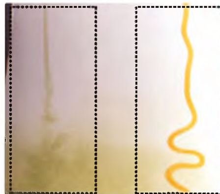
Mixability: Diluted v Non-diluted two-stroke oils
