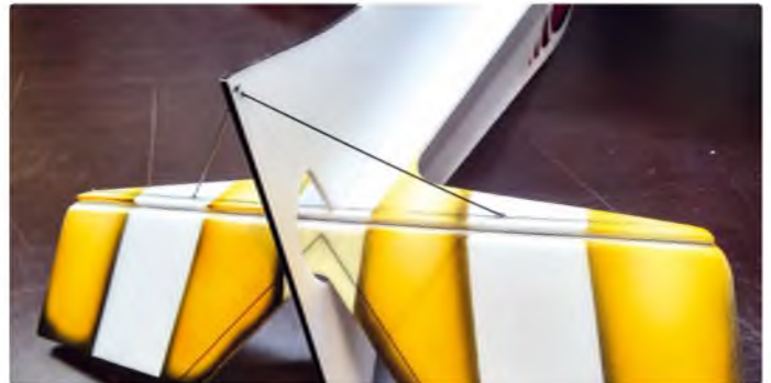
Some additional reinforcement is added to the tail section. The bottom of the fuselage is reinforced with 0.7 mm carbon rod. Flat 0.13 mm carbon strip is added to join and reinforce the rudder tail post
