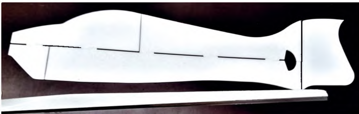
Arrow's fuselage is reinforced with 0.13 mm flat carbon
