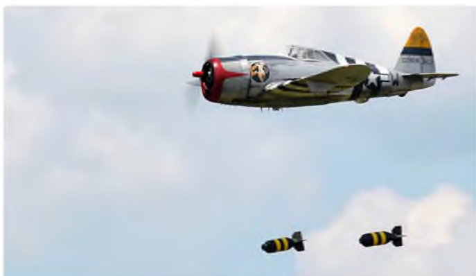
Air to air bomb run by Brian O'Meara's 1:3.3 scale P-47. 143 in wingspan, 116 lb, ZDZ 500 cc four-cylinder engine, Futaba 18MZ radio
