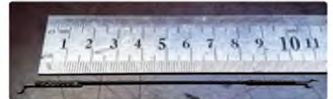
Aileron pushrods are assembled from 100 mm by 1 mm carbon rod. Pushrod ends are made using wire reinforced with CA glue and thread
