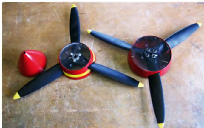
Showing the three elements of the CR prop. The left and right hand props are both 20 x 12 wooden units made by Fiala
