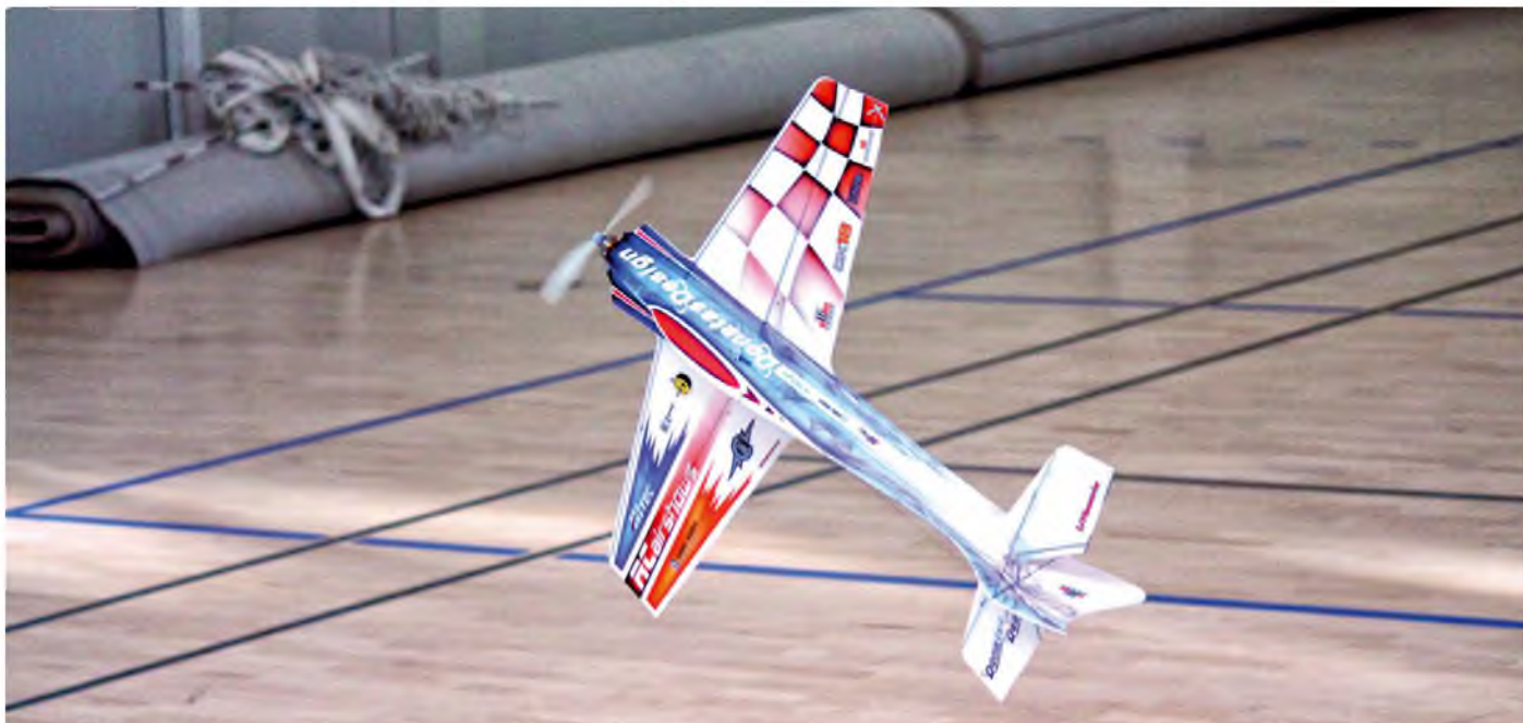
Only a small amount of rudder is required in knife - edge flight
