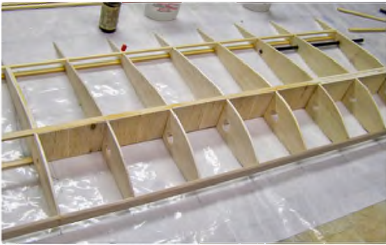
Fit 1/16" balsa webbing with grain vertical
