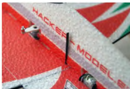
First glue to the lower surface then use the strips to make sure the top is vertical
