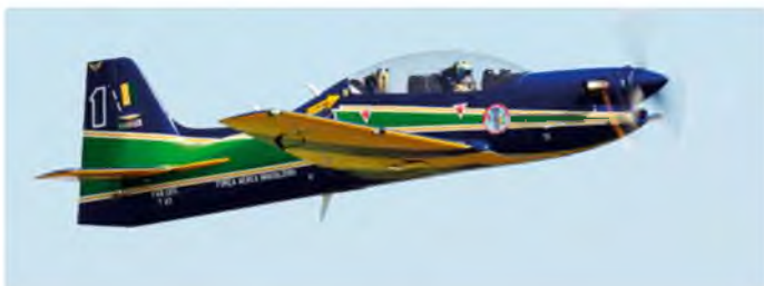
Gerson Louis Nissola's Tucano. 1:4 scale, CARF kit, 89 in wingspan, 40 lb, Jet Central TP, JR 12X radio. Team Brazil and their photographer Giovana Gastaldi are so much fun to chill with and we can't wait to see them again next year
