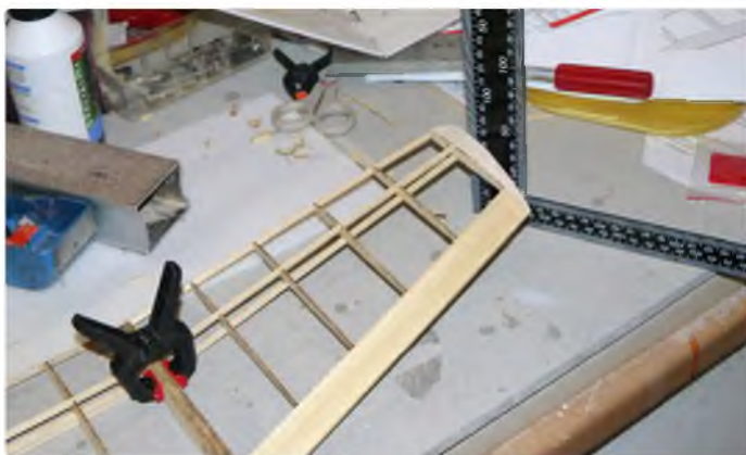
End section dihedral is provided by wing ribs cut from triangular section. A larger set square was used to check the dihedral so both port and starboard wings are the same
