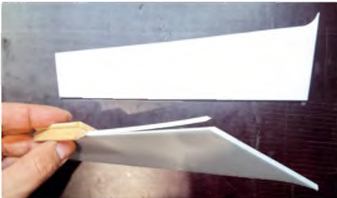
Home-made beveling tools were used to prepare the aileron hinge lines
