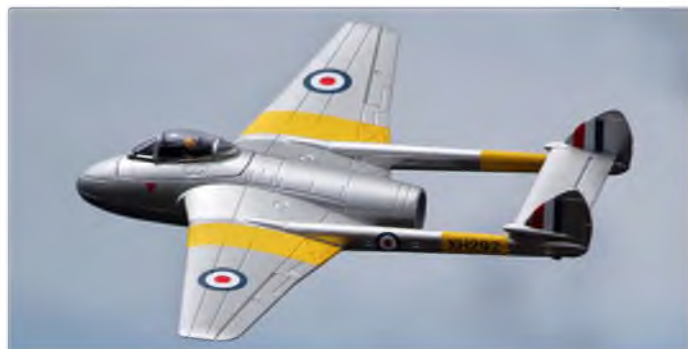
Small scale DH Vampire flown by Tim Mackey. An EDF ARTF kit converted to slope use, the ducted fan has been replaced by an amazing sound system with realistic jet noise and cannon fire. It kept us well amused on the slope!
