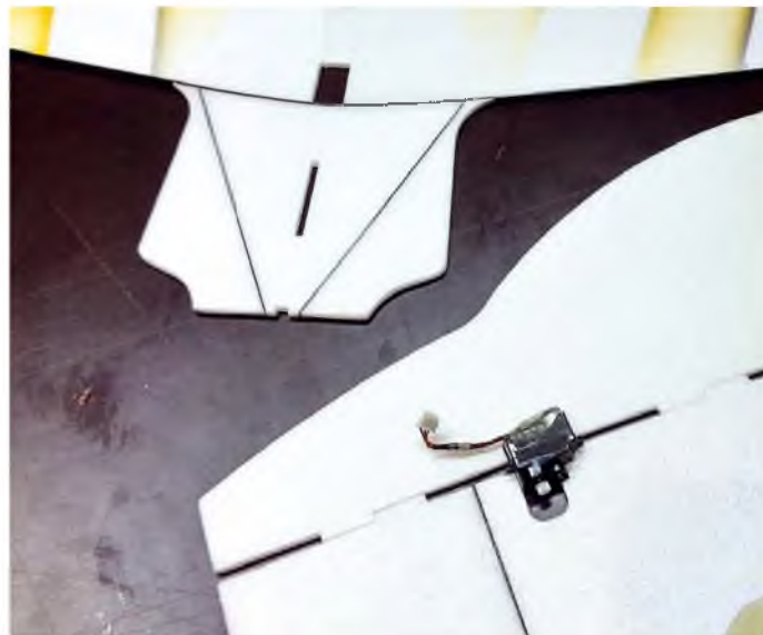
The aileron servo must be placed in the centre of the wing next to the leading edge. Cut the necessary holes in the vertical and horizontal aeroplane parts
