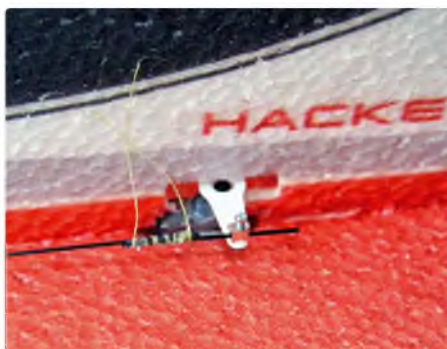
The elevator pushrod was a little short and needed a fix
