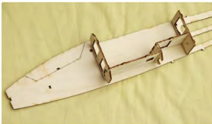
Main formers, servo and receiver tray mate up to fuselage sides, ensuring the sides are square
