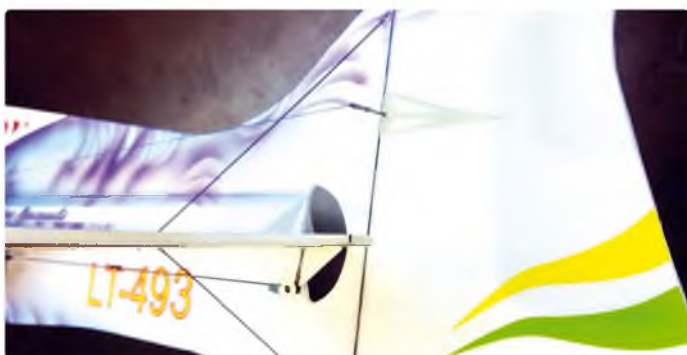
The vertical fuselage is supported using 0.7 mm carbon rod. The rudder pull-pull area is reinforced with a fibreglass triangle. The pull-pull cables are made from braided fishing line
