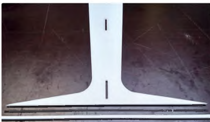
Elevator hinge line reinforcement is made from 250 mm by 0.13 mm flat carbon strip
