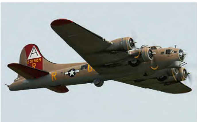
Fourth place in Unlimited Class went to builder Mike Grady and pilot David Payne with a B-17 bomber. Their Wingspan Models kit is 1:9 scale, 138 in wingspan and uses four Hacker A60 motors
