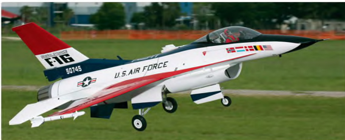
Dustin Buescher is on a roll this year and earned first place in the new X Class with his F-16. 129 inches long, Kingtech 210G turbine, Spektrum DX-18 radio
