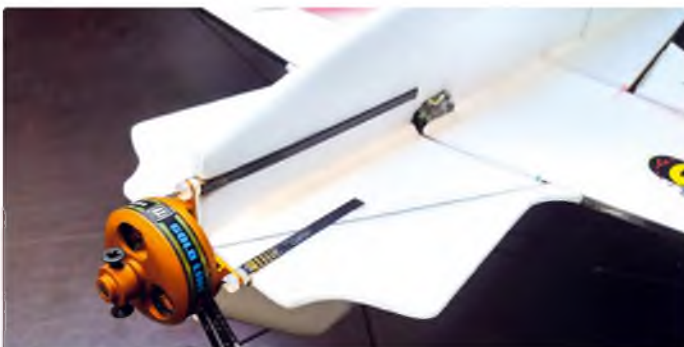
Adjustable motor mount placed on the fuselage, shown with an AXI 2203
