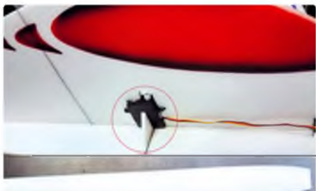
The rudder servo is mounted close to the Centre of Gravity. It is glued and reinforced with a triangular Depron support. Later it will be joined with a pull-pull connection
