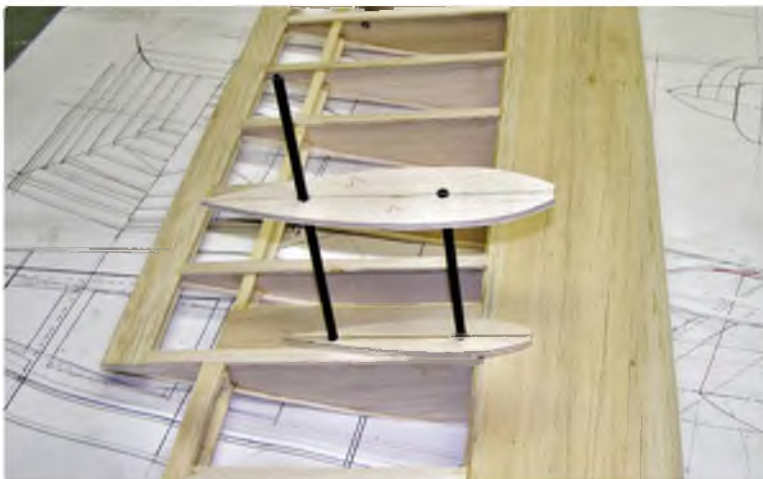
Align basic float to mark the fixing points
