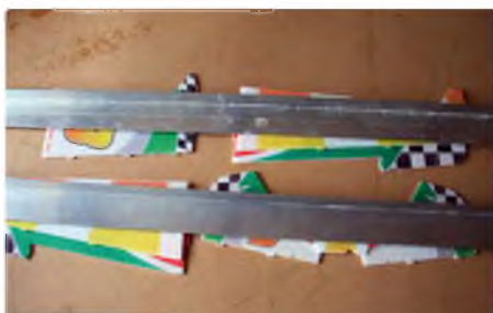
Make sure the control surfaces are flexible by folding them over and weighing them down for about an hour
