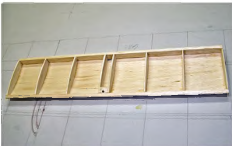
Stabiliser before the final 1/16" balsa sheet, block balsa tips and elevator are added
