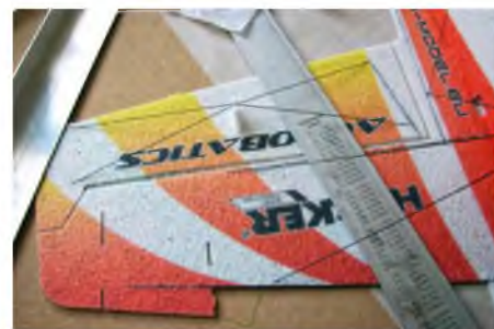
Wing reinforcement is typical of indoor planes
