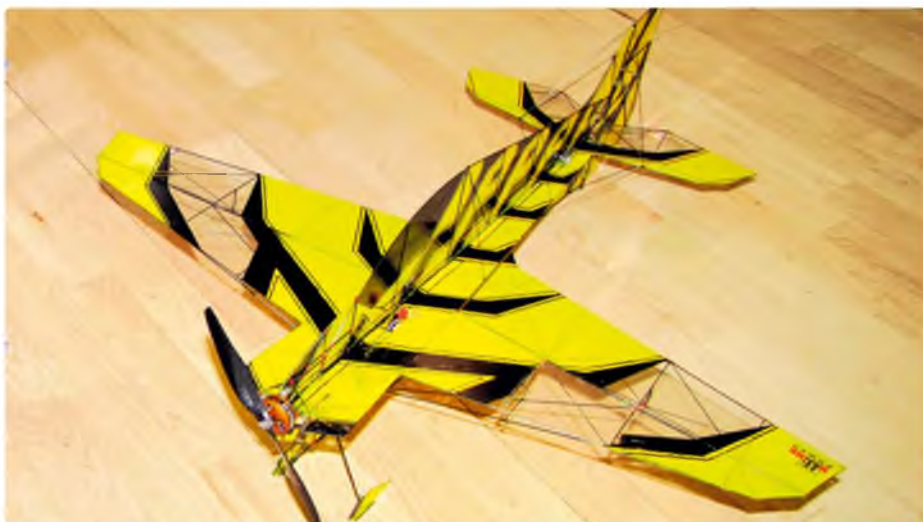
The same drawing was used by my friend to build a noticeably stronger and lighter version of the Arrow Pylon Racer from carbon rods and tubes
