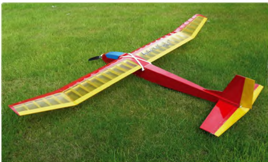
My model was covered with heat shrink film, using a two colour scheme with a translucent covering to show off the wing handy work. Decals are simple and easy to apply, being of the sticky back type
