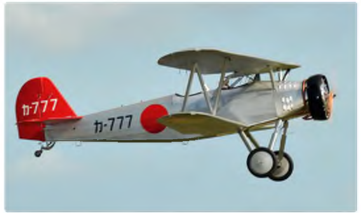
Barry Raborn's rare Japanese Willow, 1:5 scale. From the 3 Sea Bees kit, 80 in wingspan, Hacker motor, JR 12X radio. Barry earned fourth in the new X Class
