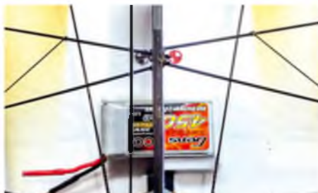
A battery box is built using Depron. Note its position close to the Centre of Gravity
