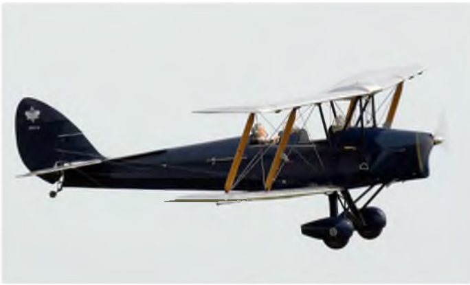
Jack Buckley's Tiger Moth DH 82A. 1:3 scale, Mick Reeves kit, 118 in wingspan, Desert Aircraft 150 cc engine, Futaba 14G radio. Jack earned fifth in the Expert Class
