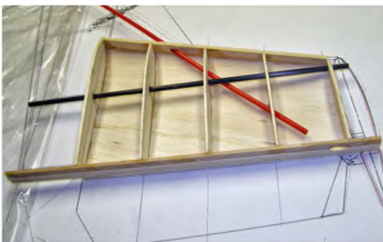
Basic fin assembly shows the carbon rod for stiffness and the elevator snake
