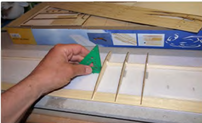
Wing panels are assembled over Depron foam templates, which align the ribs. A small set square was used to ensure the ribs were set at 90 degrees
