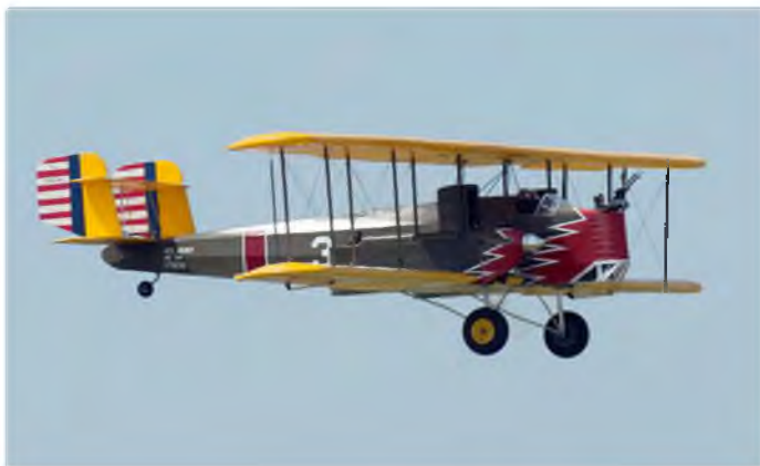
Curtis Switzer's Curtiss B-2 Condor from the Tom Czente plans. 168 in wingspan, 45 lb, twin Saito 180 engines, Jeti radio
