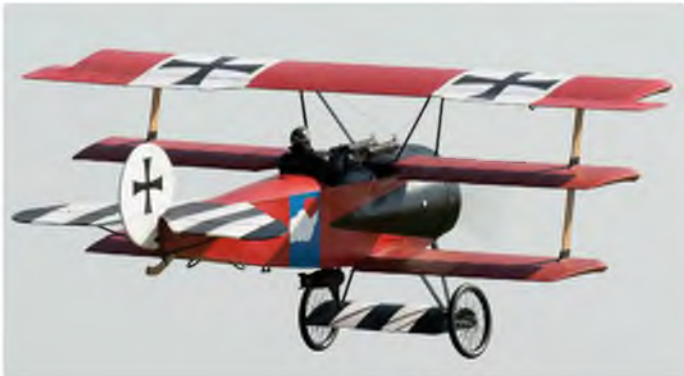
Gerry Yarrish's Fokker Triplane built from the Balsa USA kit. 1:3 scale, 94 in wingspan, 40 lb, GT80 engine, DX-18 radio. Gerry also flew in the Free Flight Scale Class with a smaller version of this aeroplane
