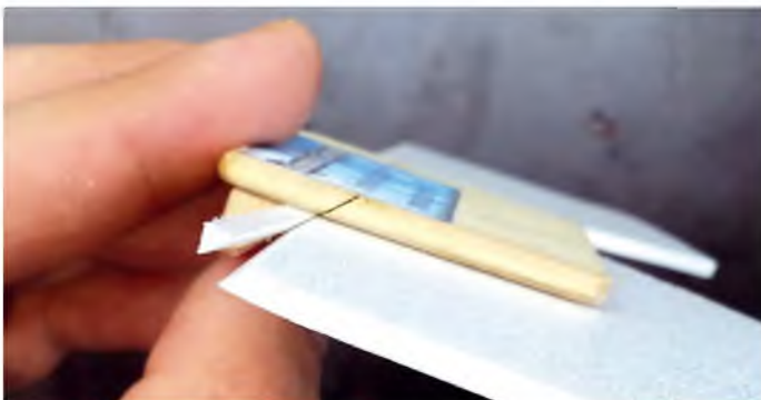
The elevator hinge line is prepared using a beveling tool
