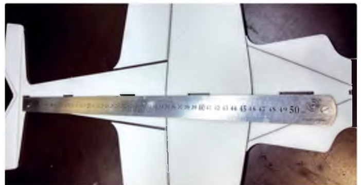
Put the ruler on the centre line as shown. Once the line is perfectly straight then glue the nose part to the wings and then the wings to the tail section
