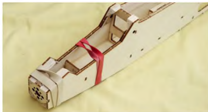
The kit comes with two optional motor mounts. Check which one suits your motor before gluing it in position
