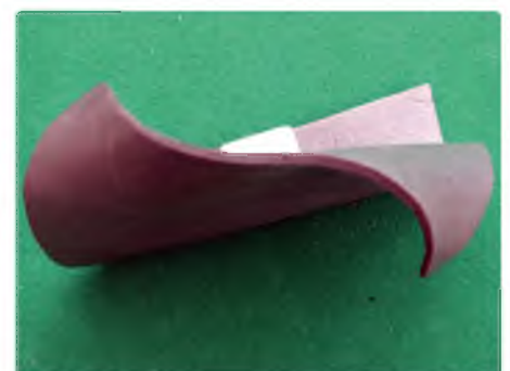
Depron can be massaged into quite intricate shapes
