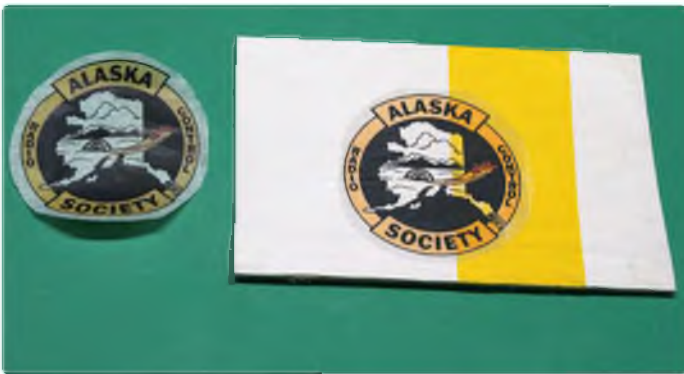
Two copies of old club emblems laser printed on white tissue, with one 'doped' onto yellow and white Litespan (using water-based 'dope') shows how transparent doped white tissue becomes
