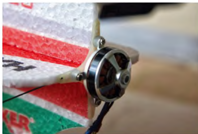
Grommets made out of fuel tubing were used to aid thrust line adjustment. The grommets can be seen clearly in the final assembly
