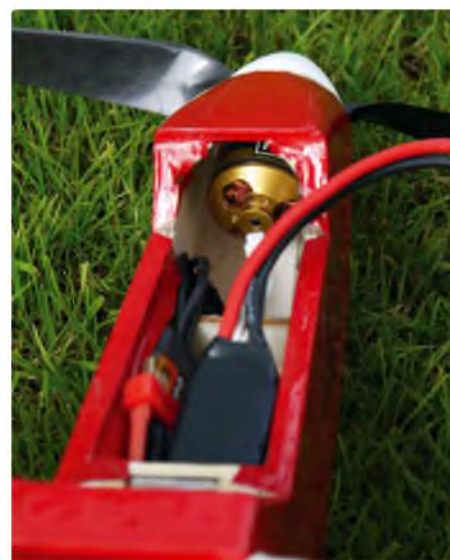
My chosen AXI 28 mm diameter motor is a tight fit. The motor wires are secured to the fuselage side to ensure that they don't rub on the motor can. The ESC and flight battery sit side-by-side
