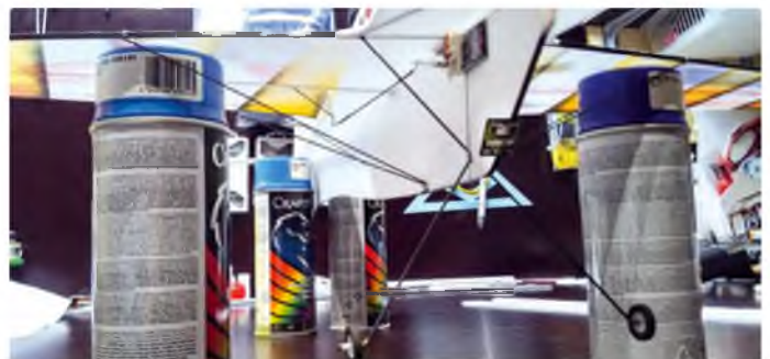
One more crucial step to ensure a rigid and straight flying aeroplane is to add fuselage reinforcement. For such a small size aeroplane the easiest way to achieve this is by adding a torsion box. In order to glue the torsion box on straight you need to be sure that the elevator and wing surfaces are level so place the aeroplane on four cans as shown. Make sure that the cans are exactly the same height. Now you can glue on the torsion box
