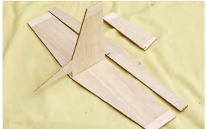
Tailplane surfaces are simple sheet affairs with anti-warp tips
