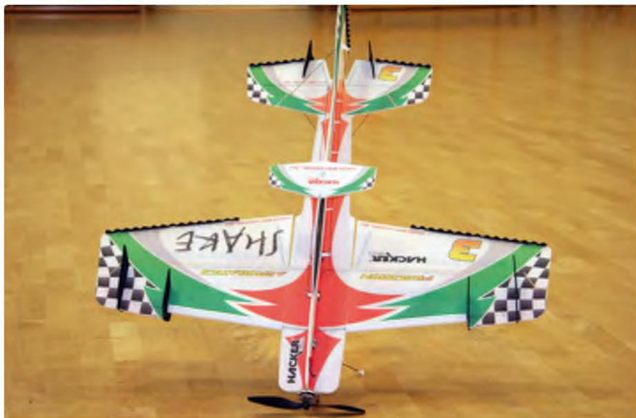
Plenty of airbrakes and side force generators make it a good aeroplane for indoor flying
