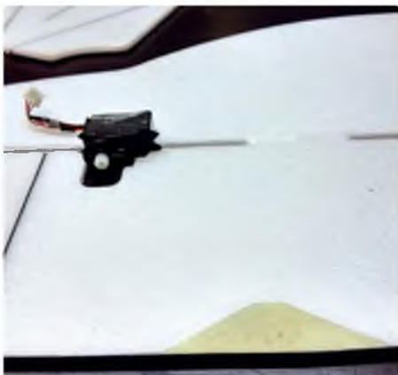
The area where the wing support will be joined with the fuselage must be reinforced using very thin plywood, fibreglass or carbon plate. 0.22 mm thickness fibreglass is shown here
