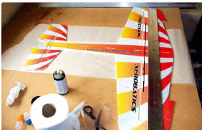
Make sure it is flat by weighing down the main components
