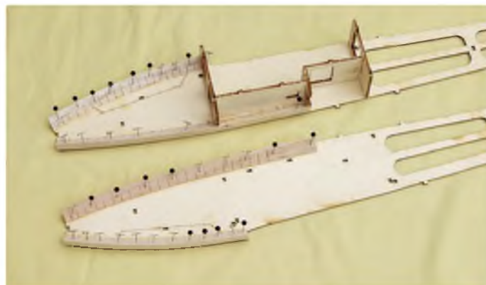
The only parts that require anything other than a light sanding are the triangular sections, which have to be notched to fit the curvature of the fuselage
