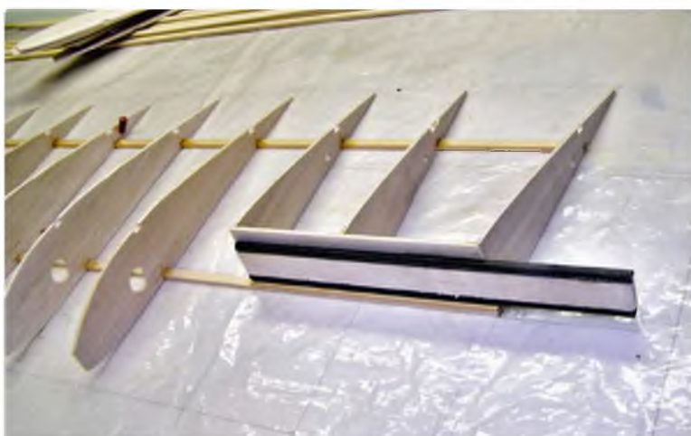
Sandwich the 1/4" plywood spar with 6 mm carbon fibre spar tubes
