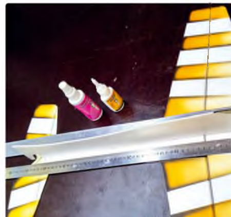
Glue on the vertical underside part of the fuselage
