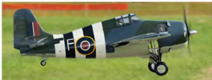
Builder Mike Barbee and pilot Frank Knoll's RAF Wildcat earned second place in the Team Class. The scratch built RAF plane uses a 3W 240 cc twin and a Futaba 18MZ radio
