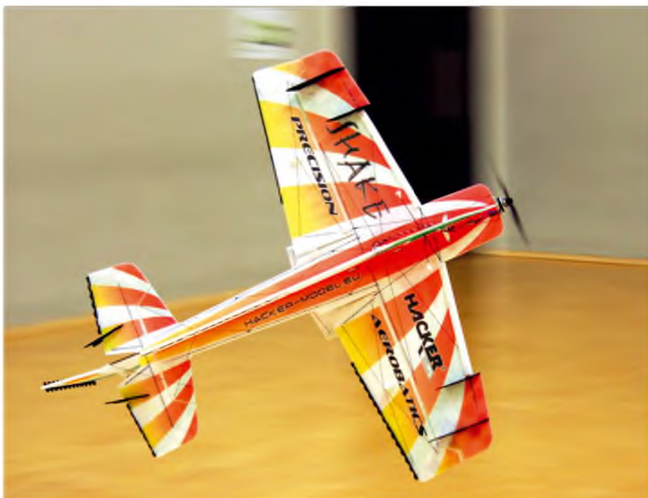
Knife-edge circle. See how little the rudder is deflected
