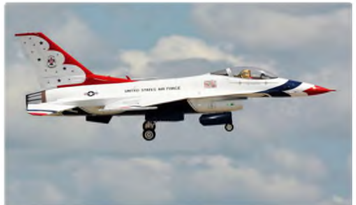
Boli Muentes has moved up to third place in the Pro Jet Class with his F-16 Thunderbird. BVM kit, 1:6 scale, 96 in long, JetCat 140 turbine, 28X radio
