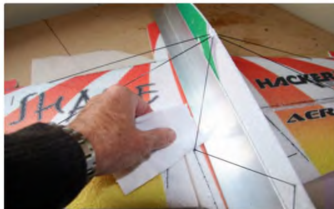
Every drop of excess glue counts so remove any surplus with toilet paper
