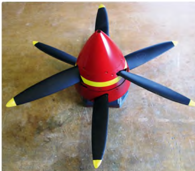
Another view of the assembled spinner. A special nut sits inside the tip of the spinner to fix it to the shaft extension. This was another critical part of the design (see text for details)
