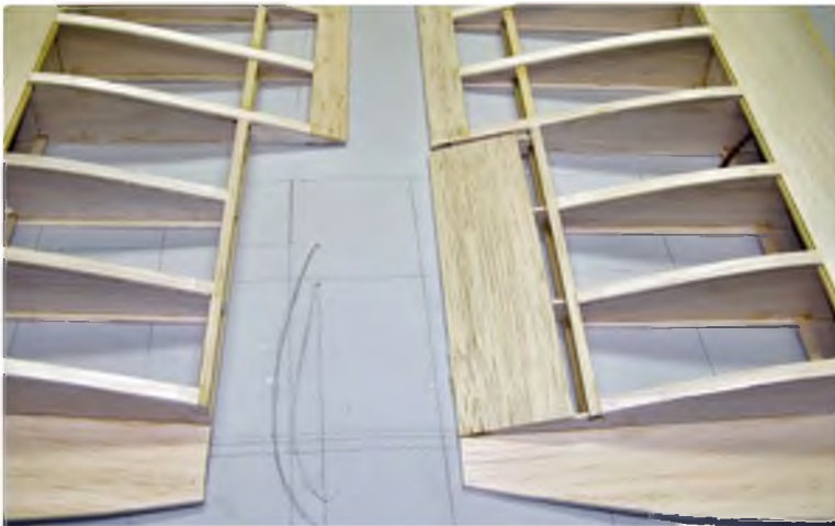
Ailerons can be conventionally hinged at the top or a Fowler type. Both methods are shown on the plan
