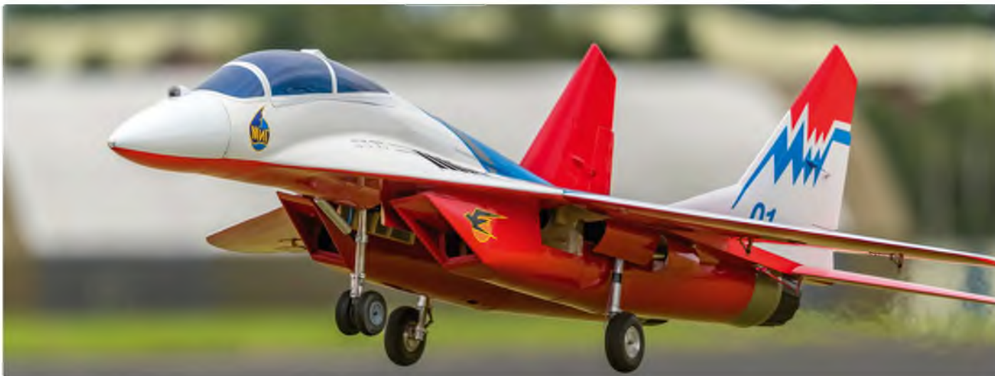
Above & below left: The massive 2.2 m wingspan MiG 29 owned and flown by Neil Hyde. The MiG has two AJJ 170 turbo jets to power this huge 29 kg model
