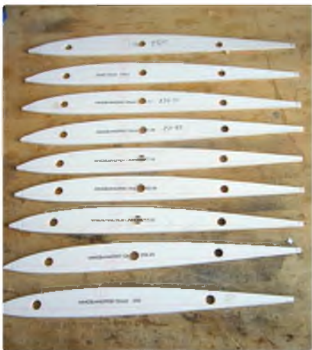
3/32" C grain ribs are cut from profiles on the plan
