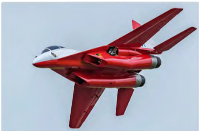
Above & below left: The massive 2.2 m wingspan MiG 29 owned and flown by Neil Hyde. The MiG has two AJJ 170 turbo jets to power this huge 29 kg model
