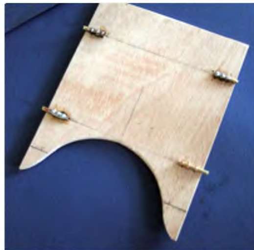
Upper wing central section base plate
