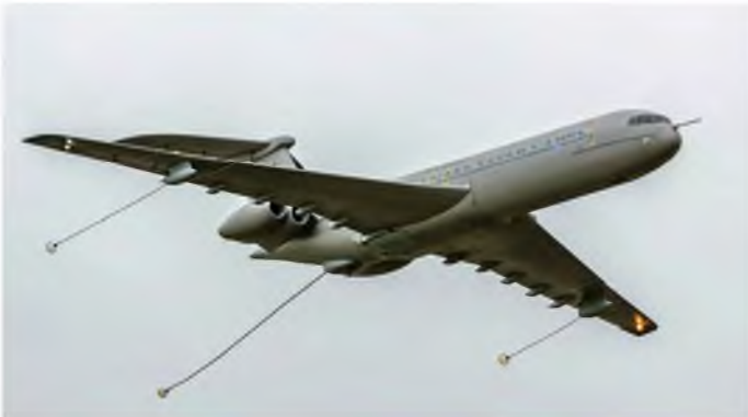
The elegant Vickers VC-10 being flown by Dave Johnson for the VC-10 team. The VC-10 weighs 64 kg and is powered by four Wren Supersport jet turbines
