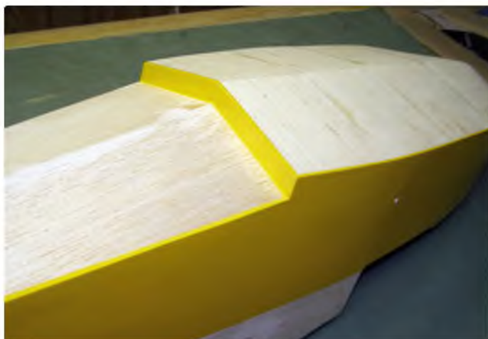
Bottom balsa sheeting and 'step'. Be sure to use a watertight covering!
