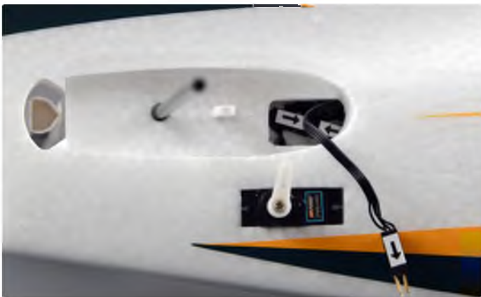
Tailplane recess showing the elevator servo and a tailplane light lead. One pair of connectors has already been tucked into the front of the recess
