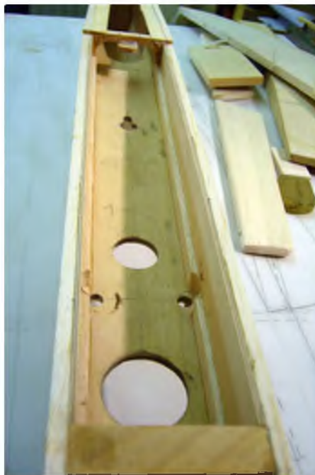
Ply for front hatch screw can be seen at the bottom of this shot
