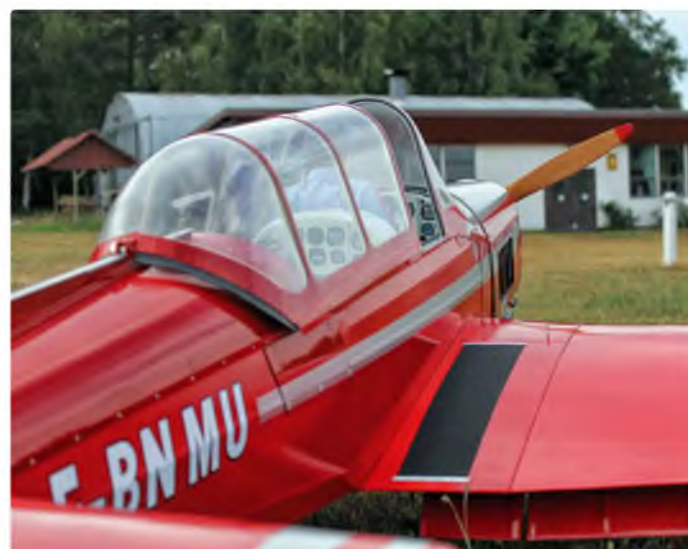
A rear quarter view of the Zlin showing the split flaps and a little taste of the cockpit detail
