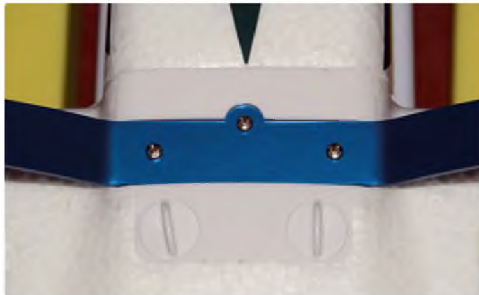
A semi-circular lug on the front of the undercarriage assembly ensures correct alignment
