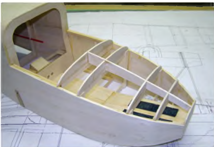
Front top deck taking shape
