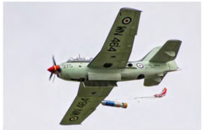
The weapons bay carries a Mk.30 homing torpedo that is dropped in flight from a low altitude. The small retardation 'chute slows the tin fish and ensures that it enters the water behind the Gannet, at the correct angle, and pointing in roughly the direction of the enemy
