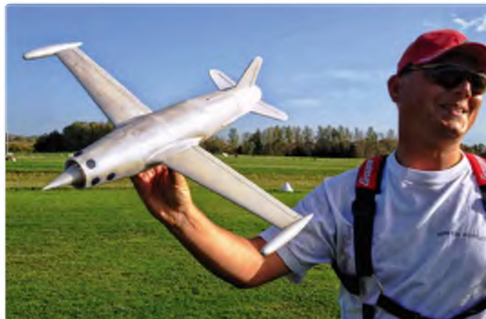
The little 'Leduc 010' is given scale by Daniel's mate. A thoroughly flyable model despite its odd 1950s looks. It is constructed from a mix of traditional balsa and the now almost universally used Depron
