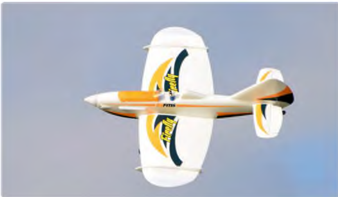
A flypast for the camera reveals the need for a little more rudder throw to crank the model over for knife-edge
