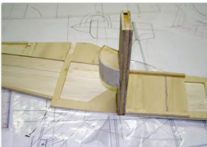
Fitting the landing gearbox to the left hand side panel
