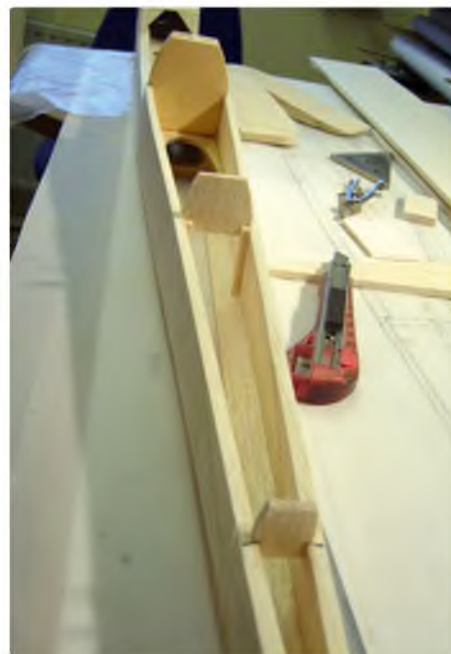
Sides brought together and rear sub formers in place
