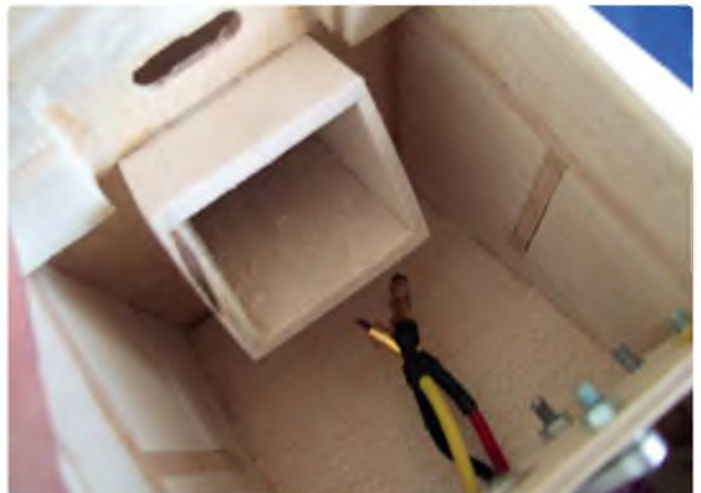
Battery box fitted
