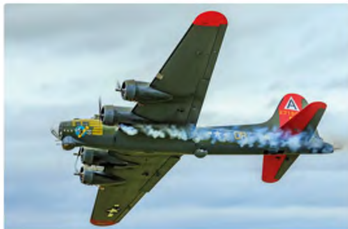
Andy Johnson puts Ken McCormick's 18 ft wingspan B-17 through its paces. Four Zenoah 38 cc petrol engines power the huge model
