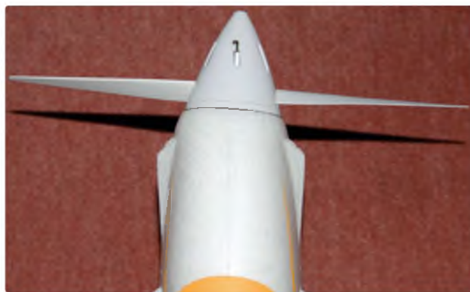
The spinner is grooved to allow cooling air to enter the model, assisted by vents on either side of the cowling. Note the decent amount of side-thrust
