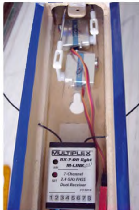
Rudder and elevator servos are shown side mounted and angled to follow the pushrods
