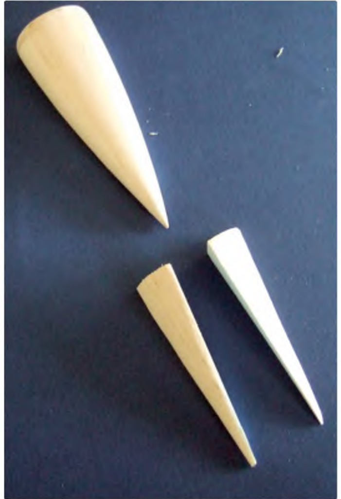
Head rest and tailplane fairings are from blue foam with thin balsa coverings
