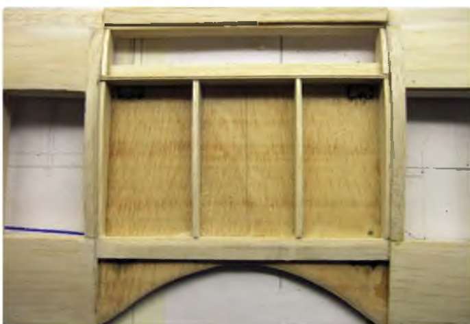
Upper wing centre section ready for top sheeting
