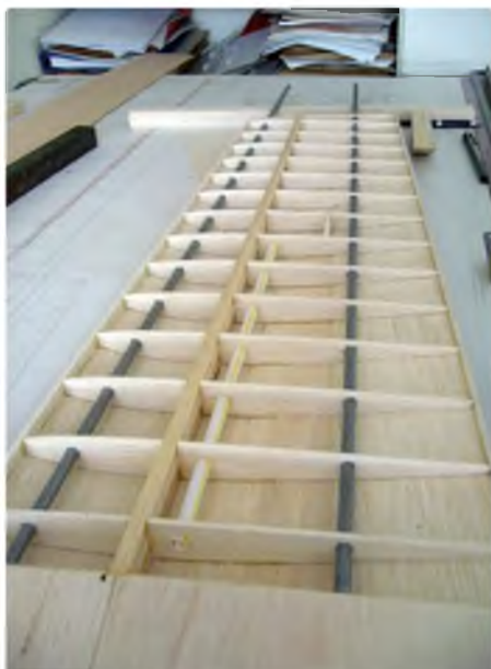
Bottom spar added, with webbing and straw tubes glued in for aileron wiring
