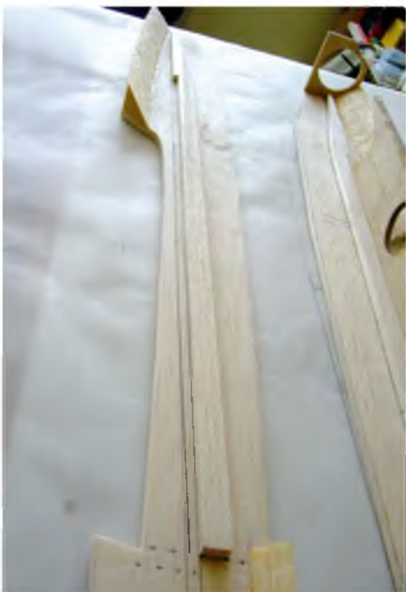
Front tri-stock on top, with crutch support and rear bottom tri-stock
