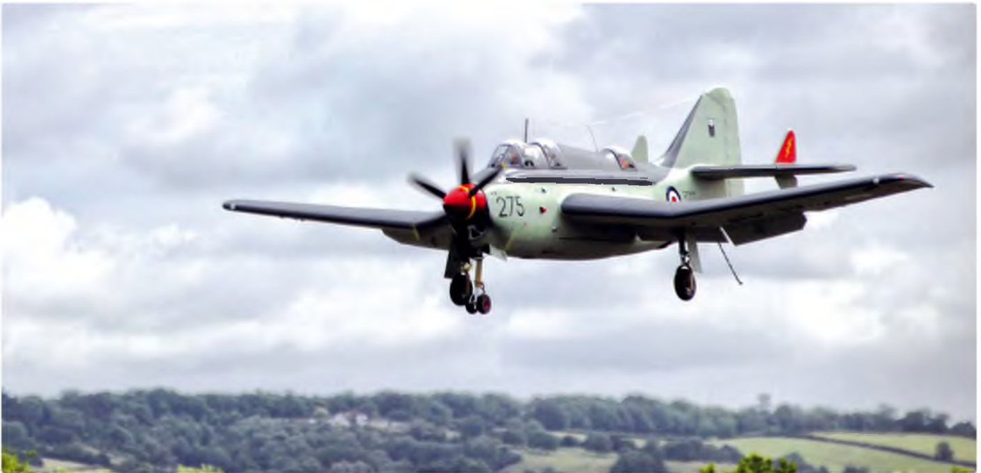
The CR prop looks good in the air, especially with a camera to 'freeze' the blades. Here the Gannet is on a landing approach, with the arrestor hook ready to grab the wires. Best to make sure the radome is retracted before you get to this point!
