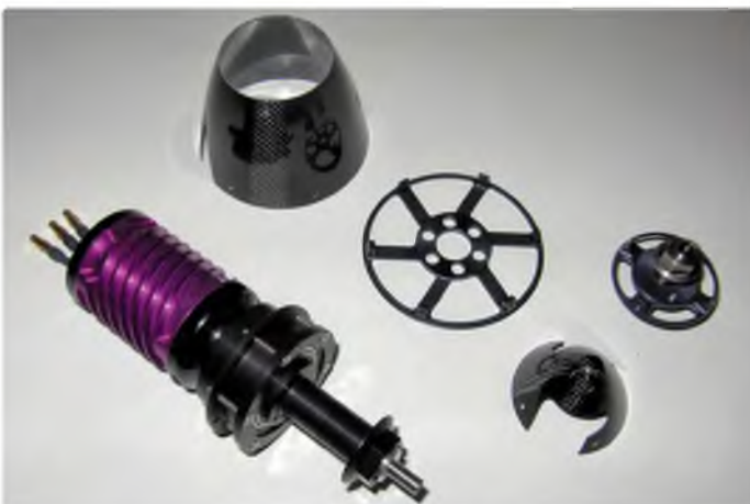
Hacker C54 motor fitted with the Ralph Schweizer Contra Drive
