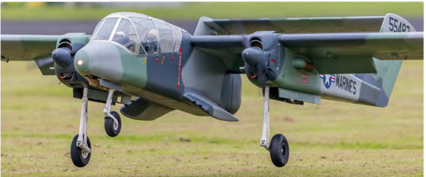
Steve Holland's large OV-10 Bronco. Built from a Tony Nijhuis plan, it has two Zenoah Zg 62 cc petrol engines for power
