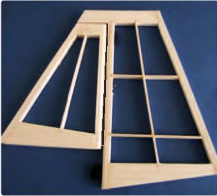
Tailplane and fin/rudder are framed using 1/4" balsa, with 1/4" x 1/16" ribs
