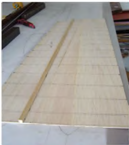
Upper spar is attached to the top sheeting
