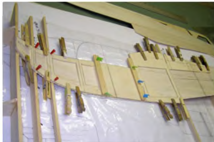
Use the bending jig shown on the plan to bend the fuselage to shape while the glue dries
