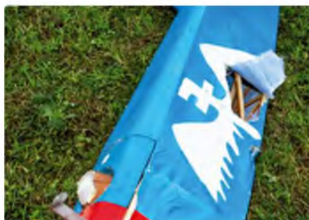
Combat Fokker has a ply fuselage to fend off the worst of any battle damage
