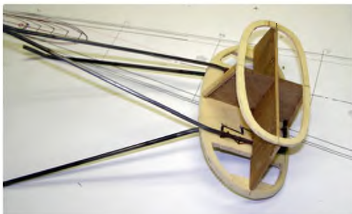
Front piano wire support legs now in place and the nacelle frame is attached
