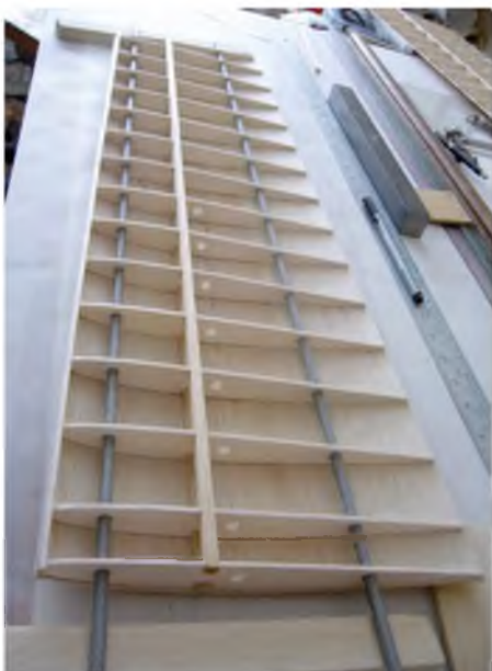
Ribs are glued to the sheet with cyano, rods slid in and the false LE added
