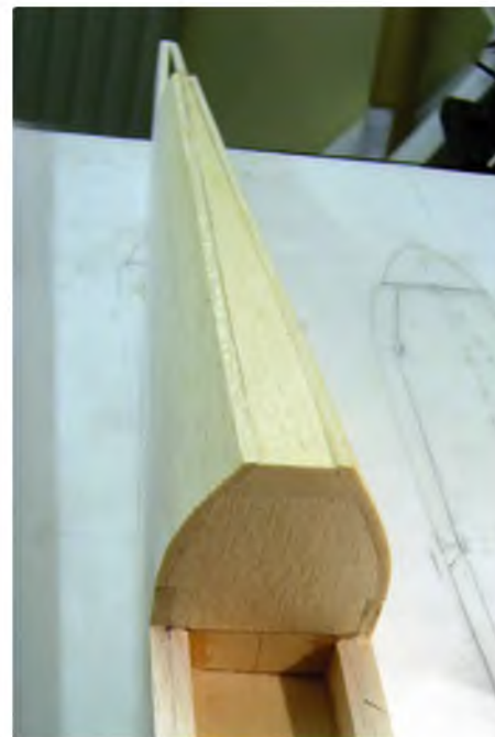
Rear top sheet is glued and shaped to match the sides of the formers before adding the balsa sides
