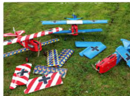
Wing panels are designed to be interchangeable, allowing for speedy repairs between bouts
