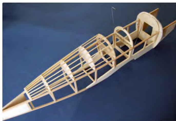
Rear formers and BBQ skewer stringers in place
