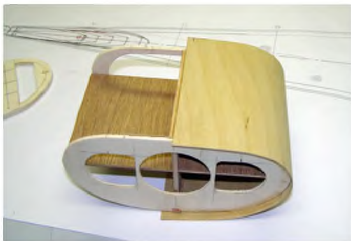
Basic cowl formed from formers N1-N2 with rolled 1/8" balsa sheet. Note the crosspiece is from temporary scrap to hold the shape
