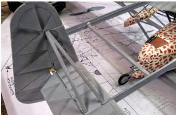
The super Sikorsky S39 shows off its strutter and paint job. It's a little over one metre wingspan. Daniel used a pen and airbrush to 'shadow' the tail feather internal construction
