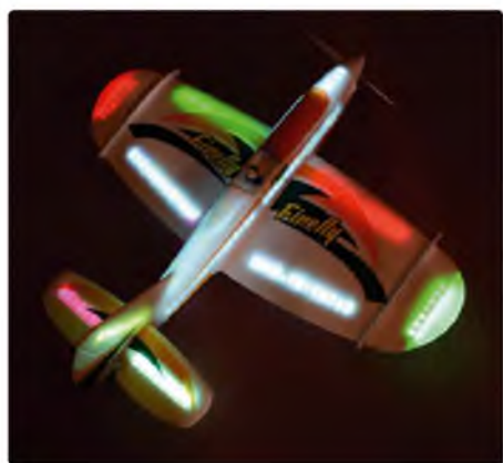
Testing the lights. There are 15 LED light strips in total
