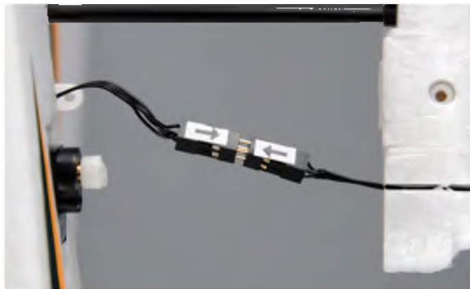
Matching up the arrows on the connectors ensures that the pins are fitted in the correct orientation
