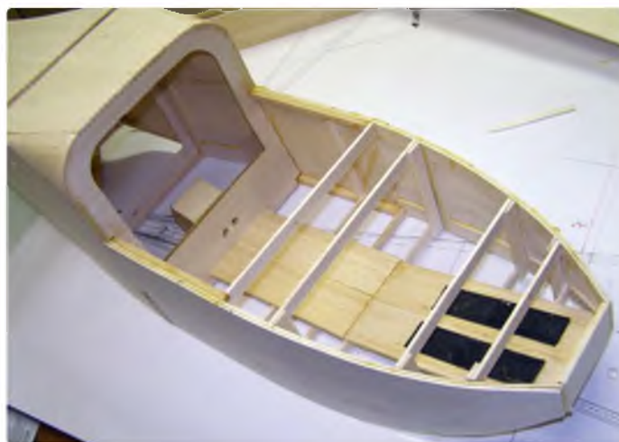
Landing gearbox in position behind former F9. Note the balsa battery tray and floor
