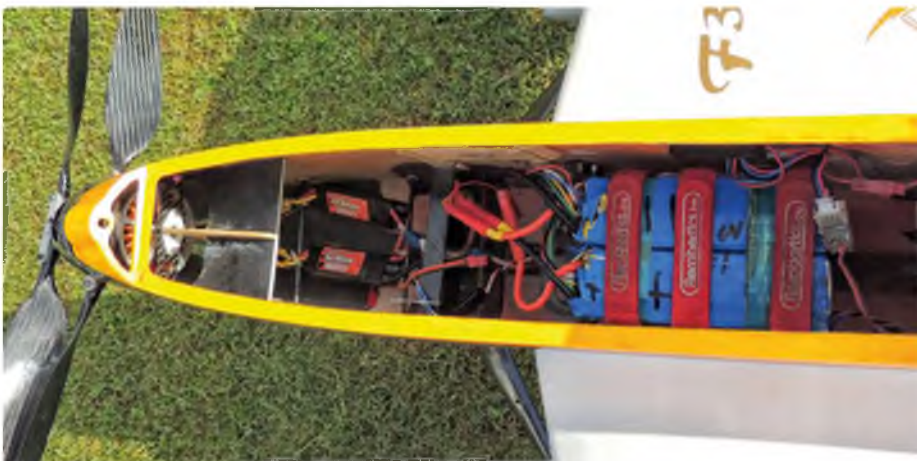
Interior shot of the Axis showing the motor installation
