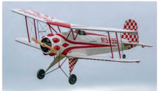
Jeff Pearson's large 118" wingspan Jungmeister. The power unit for the model is a 3W 140 cc flat twin petrol engine
