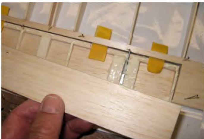
Solartex strips used for aileron hinges are secured with small balsa pegs
