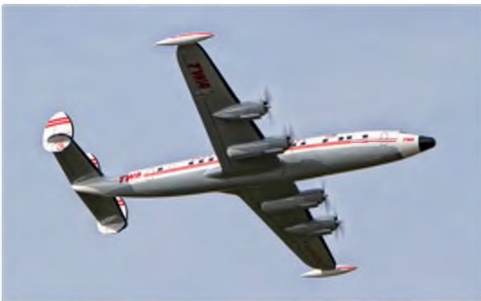
The 'Connie' whiffles past almost noiselessly on its four outrunner electric motors. Built from the Traplet plan, MW3663. A set containing the plan, four ABS cowls and laser cut wood pack is also available, SET3663
