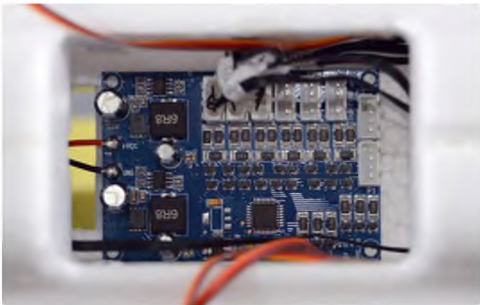
The lighting control board, with the XH light strip sockets starting to be populated
