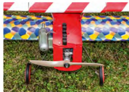
Combat pilots only use IC engines due to the fire risk from damaged LiPo packs. However, the RCMW plan will feature an electric conversion too for sport flying
