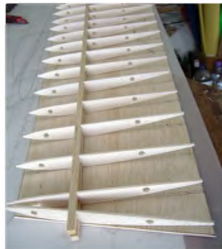
Ribs are attached to the spar and sheeting, then any excess sheeting is trimmed away
