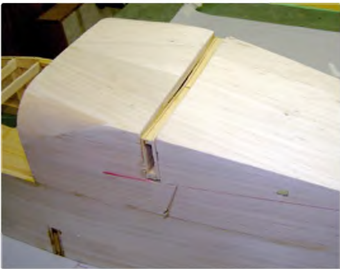
Spar box inset into top of fuselage
