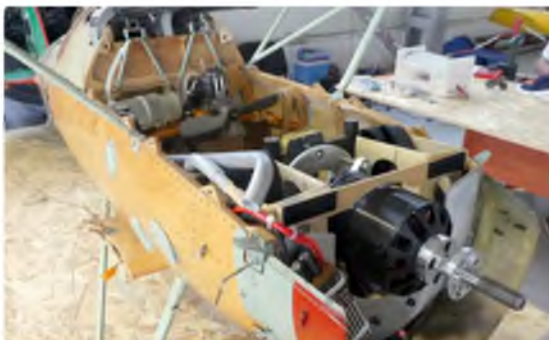
Yannic Bueb's electric Albatros. The OS four-stroke used to create engine sound can be seen on the rear bulkhead
