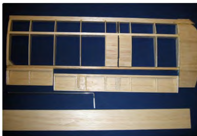
Building a lower wing
