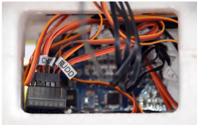
The hole in the wing bay is thick enough to mount a small receiver. The servo leads are marked with labels showing their respective functions
