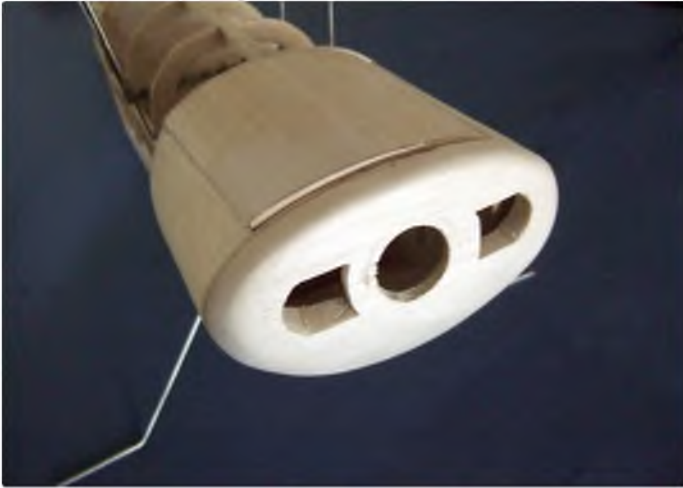
Nose block and cowl shaped from medium/soft balsa sheet. Laminate if necessary
