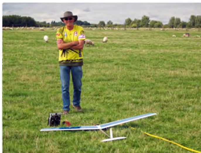
Brian Johnson flew this Highlight Speed, also known as a Nellie, in 2 m eSoaring! Originally with full span ailerons, now converted to flaps/aileron and about 7 degrees of dihedral. Getting the C of G in the right place is an ongoing process! Now known as Nellie the Elephant, although it goes up in lift well for such a beast!
