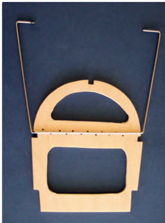
F5 with cabane struts ready for securing with thread and epoxy glue
