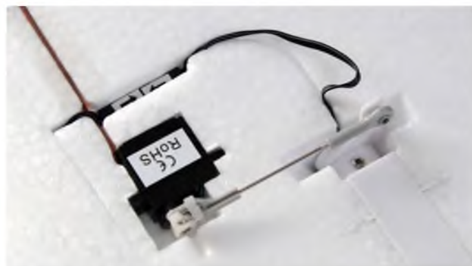
Wingtip servo and linkage connected to a steering arm. Any excess wiring can be tucked into the deep grooves pre-cut into the surface of the wing
