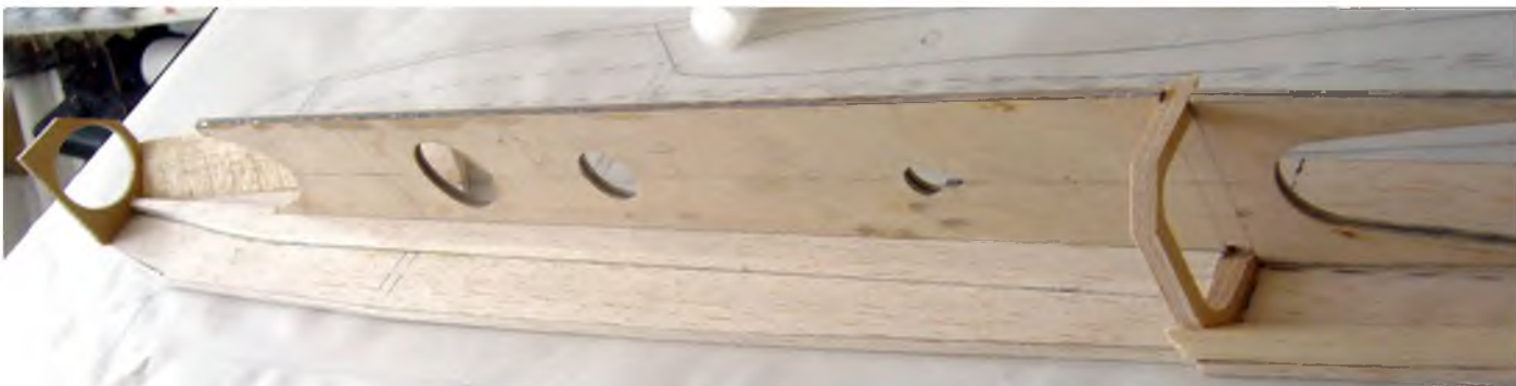
RH fuselage side with formers in place and ply lamination crutch
