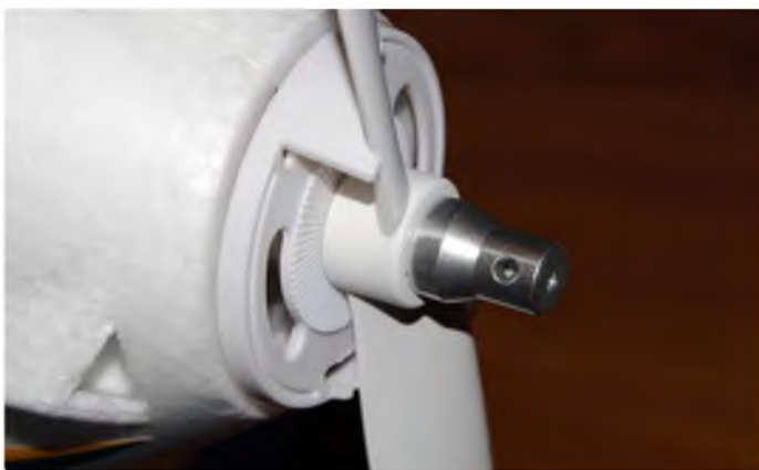
The prop nut is tightened using an Allen key or similar as a tommy bar
