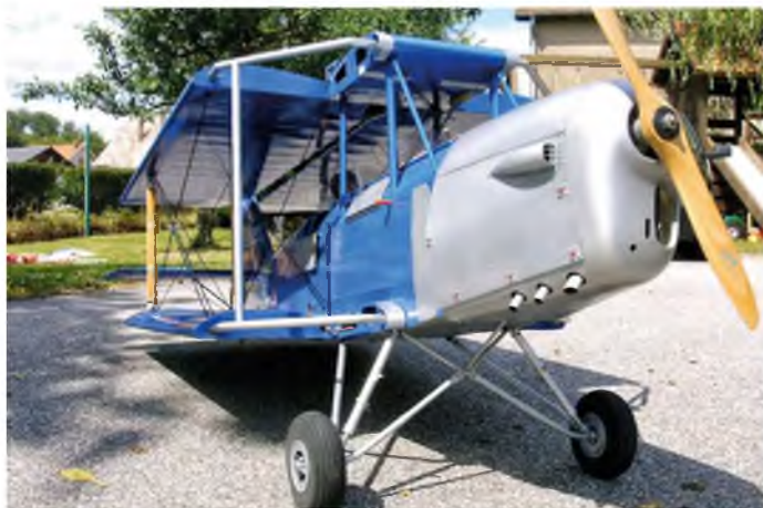
With wings folded, just as the original. I am assured that the tubular ground handling wing securing assembly is also scale and that even the small leading edge wing joining covers work exactly as the original
