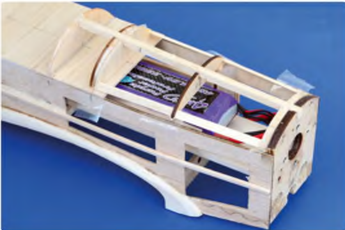
Building the battery hatch into the front decking is simple and it means a perfect fit
