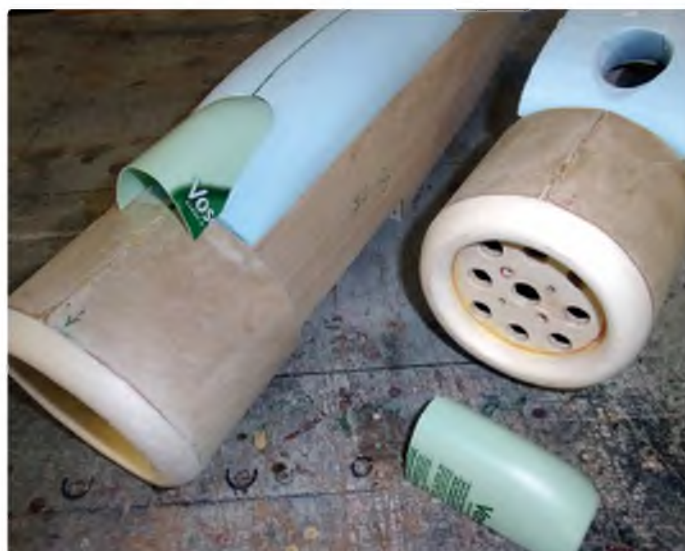
Nacelles with air intakes to ESCs
