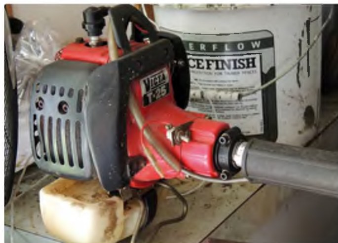
Weed whacker engines are generally a good choice for adaptation as the drive shaft is prominent and easy to adapt for driving a propeller
