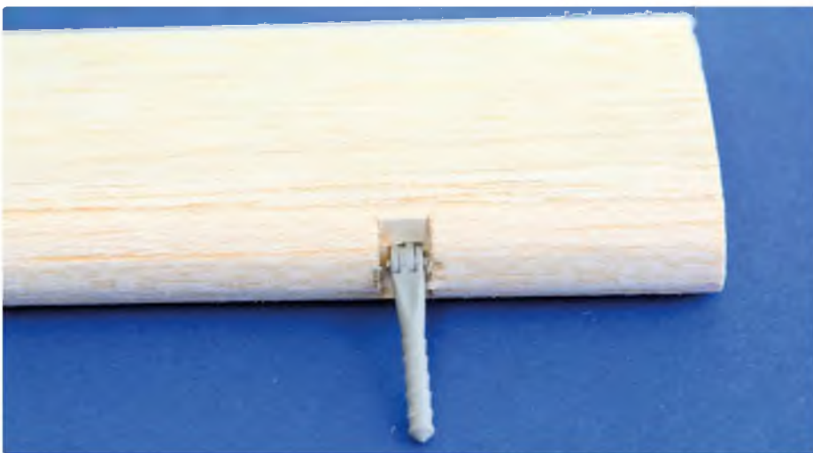
Above & below: The hinge line on Robart hinges is behind the bull-nose of the control surface, which means scale-like cut outs are put into the control surfaces
