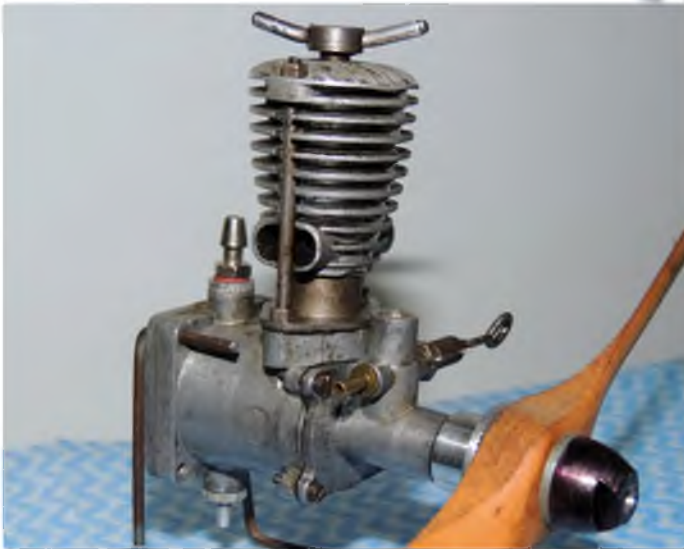
This is a Frog 100 diesel, the engine that started so many modellers on the path to IC powered models
