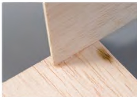
Edge on joints work well on either Depron or balsa
