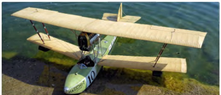
The M-7 features a replica Isotta Fraschini V-6 250 HP motor engine made from wood. In 1922, Giosellino Corgnolino came third with this plane in the Schneider contest at Naples . Power is from an OPS 60 Speed SPPRCA turning a 13 x 5 pusher prop
