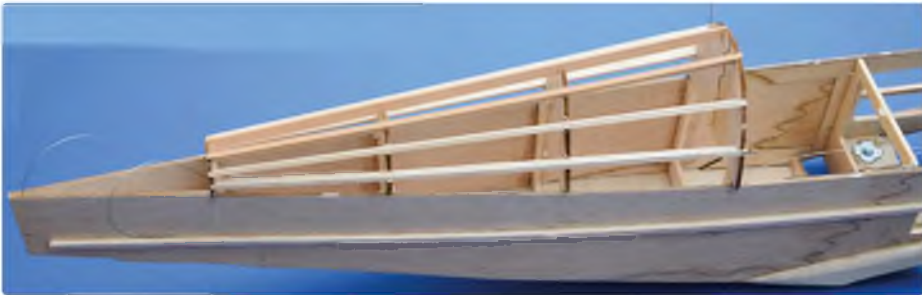
Only the top two stringers need to be spruce for the electric version. Make sure the control systems are installed before gluing the stringers otherwise the air will turn blue!
