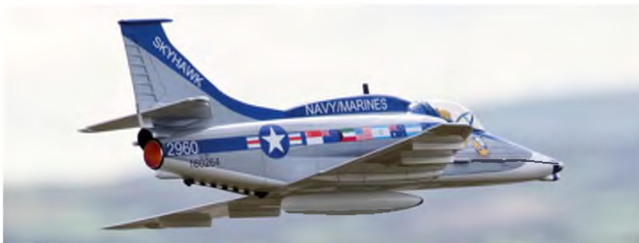
Chris Barlow's A-4M in flight. The commemorative scheme details all the nations' flags who operated the type. Note that the central fuel tank is fitted; the store is dropped safely upon command prior to landing
