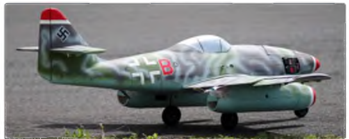
This beautifully built Me 262 was unusual as it used two pusher motors
