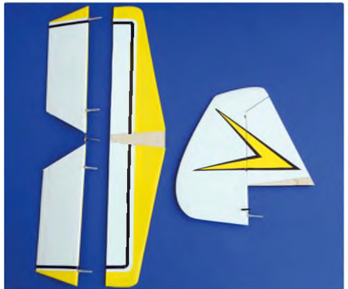
Completing most of the finishing before assembly makes life easy but make sure that areas to be glued are not covered
