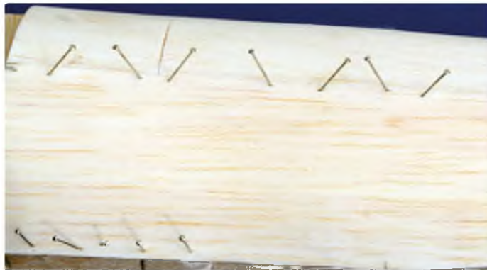
When pins have to hold difficult joints they will only work if angled opposite to each other, which stops the wood riding up on the pins
