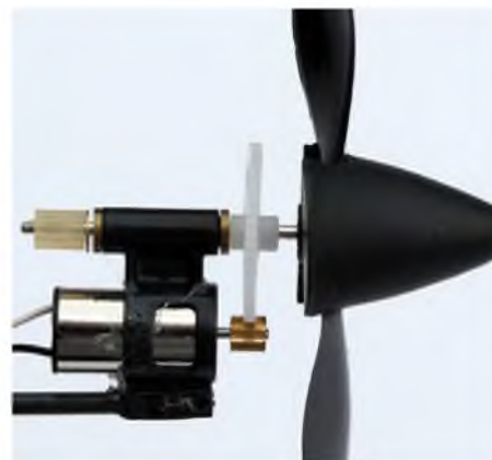
After test flights I replaced the supplied motor unit with a Mini Vapor version, as shown here
