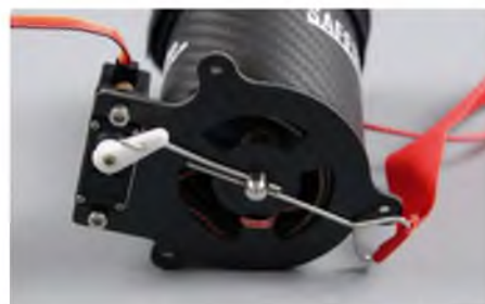
The parachute is ejected by a strong spring when the servo operated pin is withdrawn. A safety pin is also inserted for storage, fitted with a 'Remove Before Flight' flag
