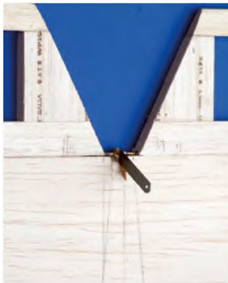
To fit the elevator horn inside the fuselage it needs to be angled to allow sufficient up movement
