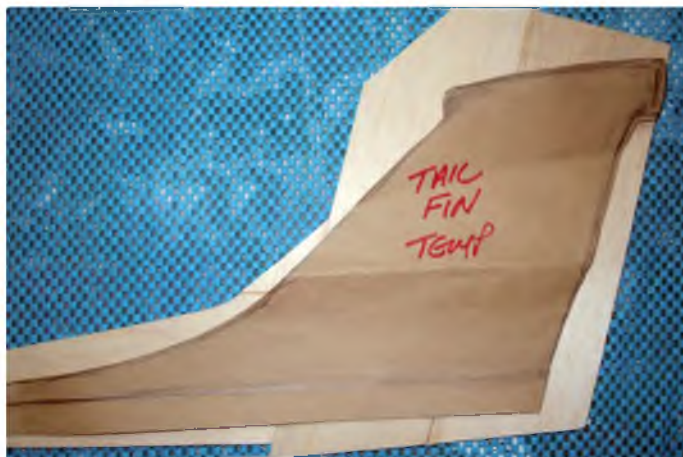
Glue up sheet balsa roughly to shape and mark out the fin using the template
