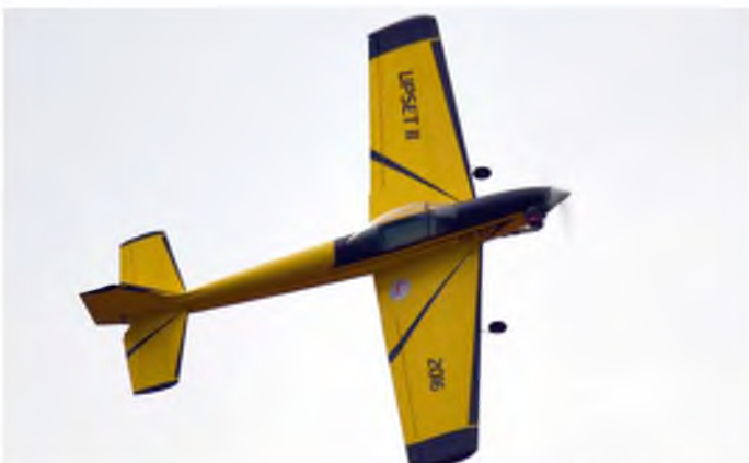
Top left rudder for an effortless knife-edge with the author's 'Upset II'
