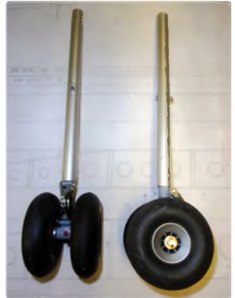
Robart oleo legs with aluminium tube extensions
