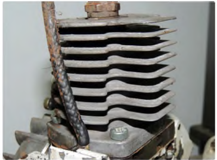
One consideration, if you do decide to adapt a chainsaw engine, is the very deep head finning, which is ideal for tight cowls on models
