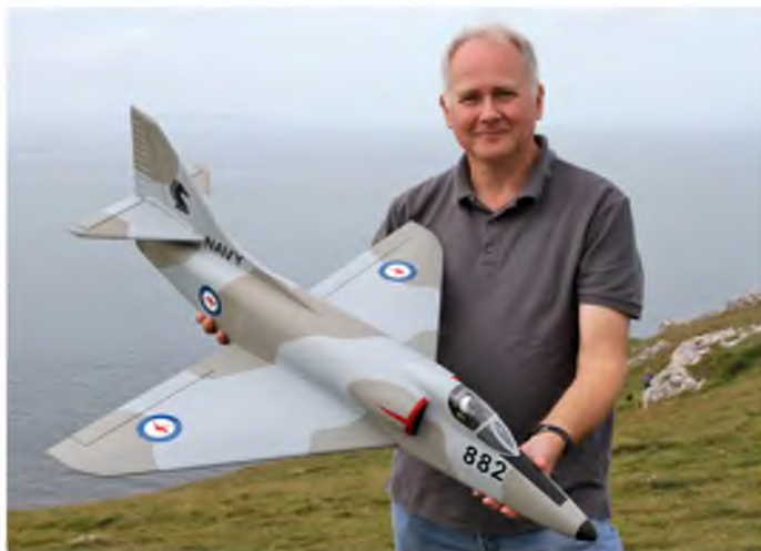
ISA member Steve McLaren with his superbly finished Australian Navy example of the A-4. Covered in a mixture of tissue and film with brushed paint, this A-4 was one of the lightest built at 2 lb 6 oz
