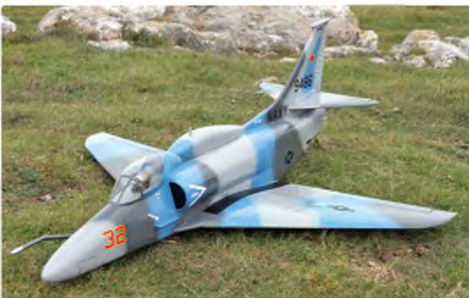
Matt Jones' A-4 was modified with a spine hump and larger canopy to accurately portray the lines of a later A-4M variant, and finished in a stunning three colour Aggressor scheme from the US Navy Fighter Weapons School
