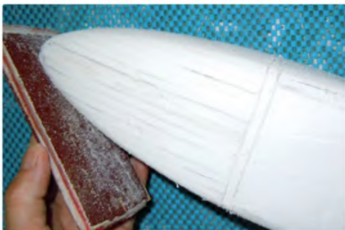
After attaching to fuselage, sand the nose to shape
