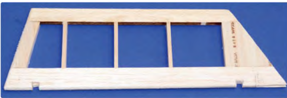
Above & below: The hinge line on Robart hinges is behind the bull-nose of the control surface, which means scale-like cut outs are put into the control surfaces
