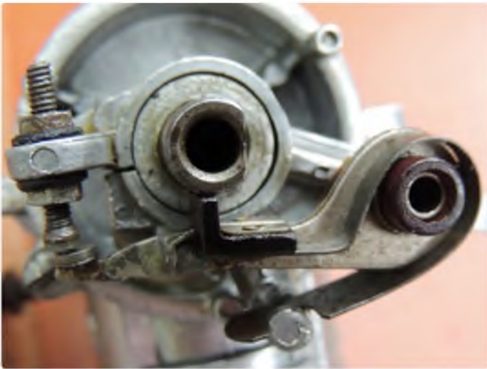
An example of the points used on spark engines. They had to be kept clean of oil and correctly adjusted. Spark erosion of the points was always a problem that needed addressing
