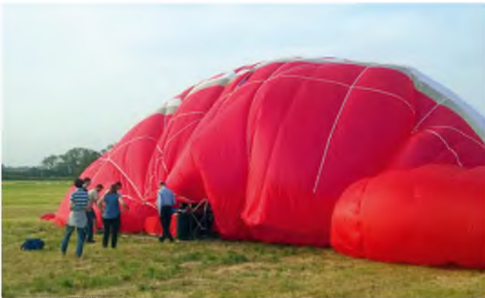
Something's growing at our farm flying site! Steadily filling up a dirigible using a portable cold air fan unit. Hot air goes in next
