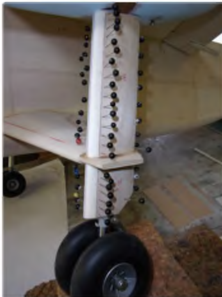
Leg extension fairings are completed with 0.4 mm ply
