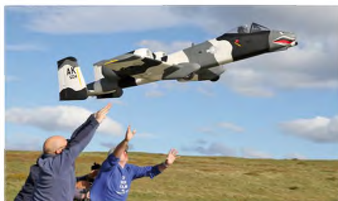
It wasn't all just Skyhawks. All types of PSS models were flown throughout the weekend, including the superb 1/6th scale A-10 Thunderbolt II built by Andy Meade. Here the 110" span 'Hog' gets a launch from a band of helpers
