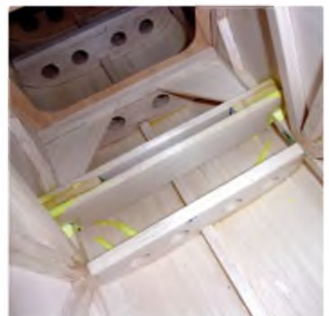
Winglet spar connecting bars inside fuselage
