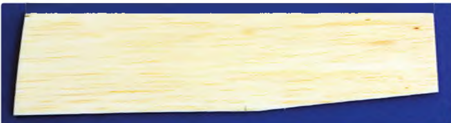
Since the front fuselage is curved in three dimensions the balsa used to form it will not be a straightforward rectangle
