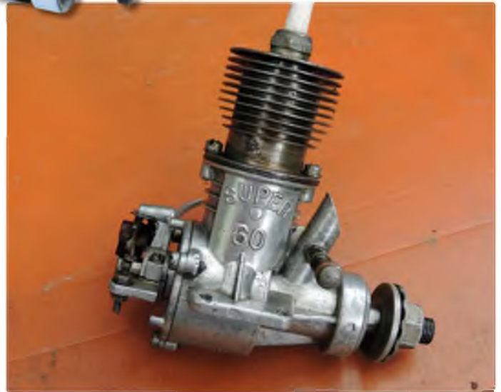
Spark ignition engines were expensive and a bit of a specialist area as they had variable timing that had to be tuned, along with the carburettor, to get a good balance
