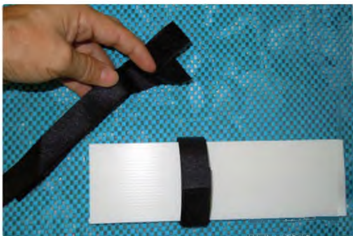
Make the battery floor and fit a hook and loop strap
