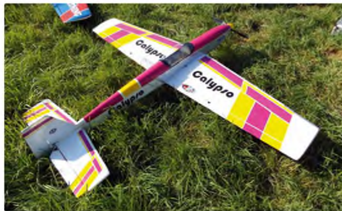
Model Tech 'Calypso' flown by Graham Fox. Originally powered by OS RFP 61, it is now converted to an OS 502 motor and 6S LiPo
