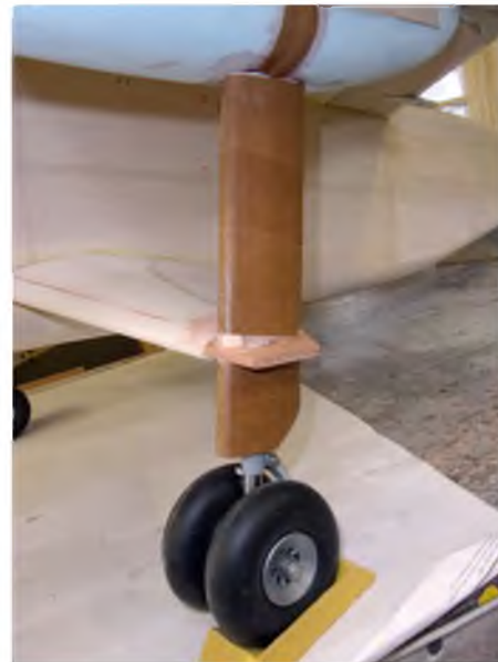
U/C leg finished with brown paper, PVA'd in place
