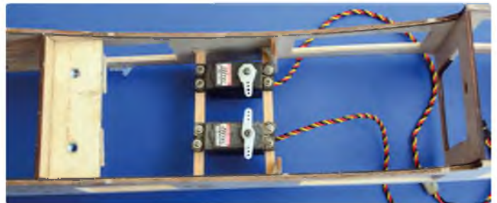
Hardly any building work done and the servos are already in
