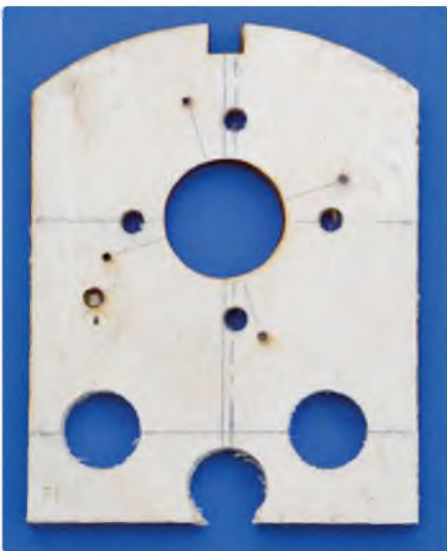
Holes cut in the F1 former to help cooling for the controller. The dotted line is an offset centreline. Do these things before gluing them to the fuselage structure
