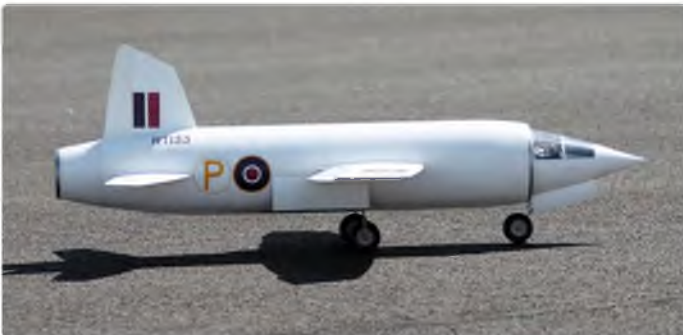
Will Beavor's new, larger M.50 has a complete retract system with functioning doors – some tricky installation issues, I'm sure!
