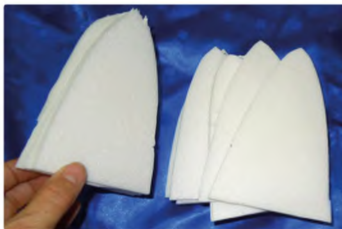
Cut out the nose section and laminate with spray adhesive
