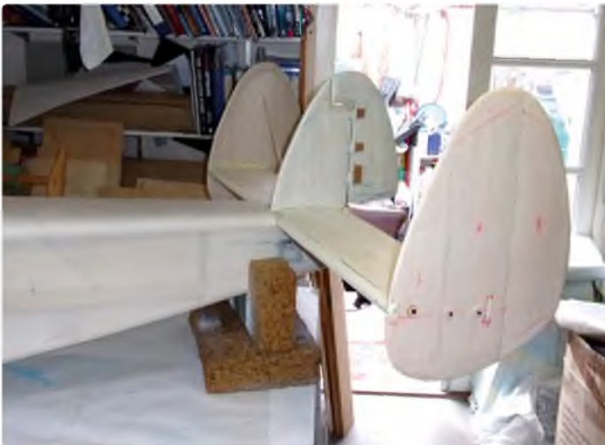
Triple fins in place
