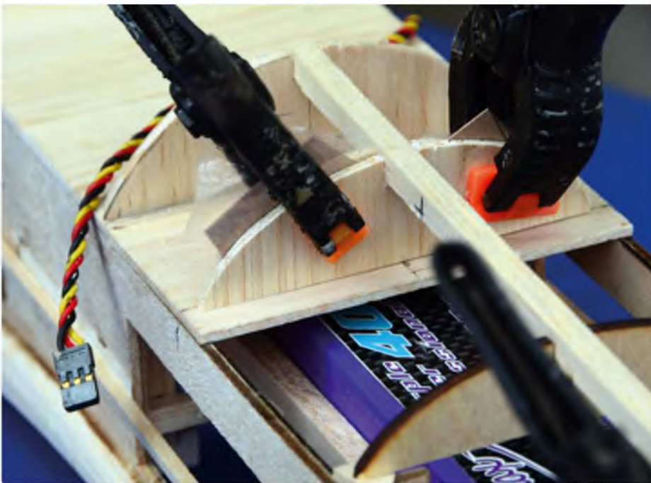
Use 1/32 inch ply shims to create a gap between the rear of the hatch and the fuselage
