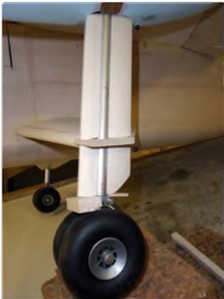
Leg extension fairings epoxied in place
