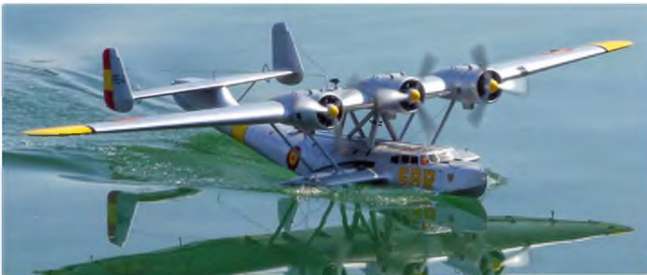
Three electric motors power this perfect scale model of the Do.24 when in Spanish service
