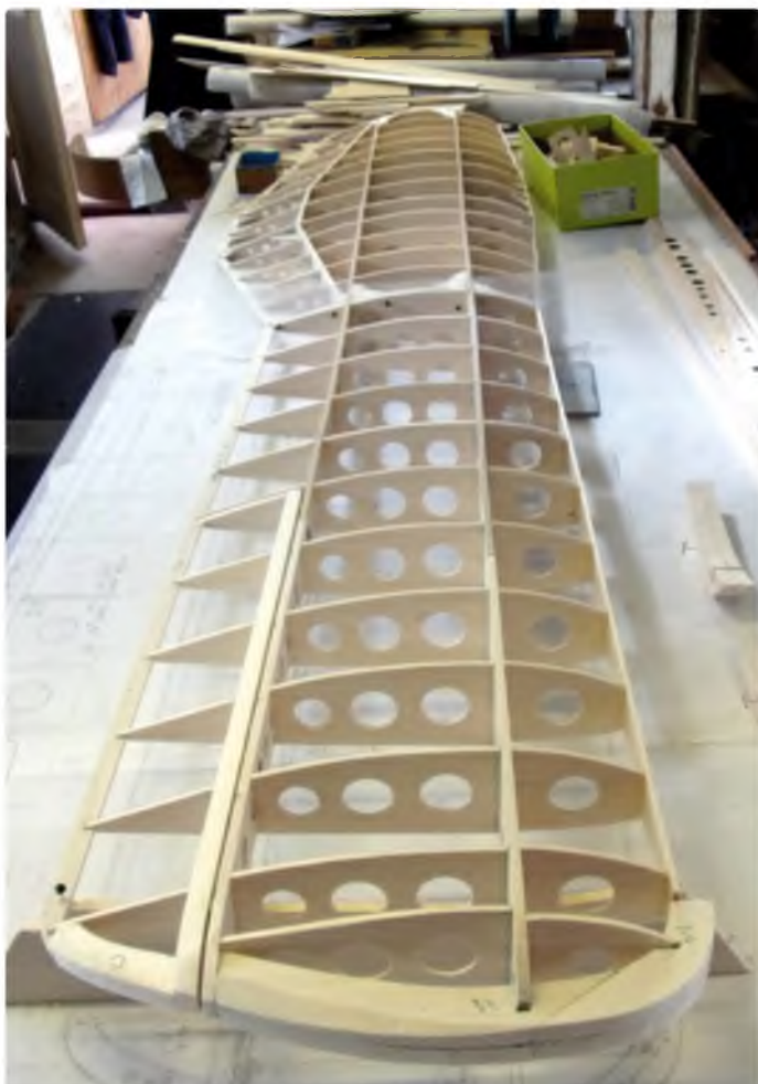
Outboard wing panel in build
