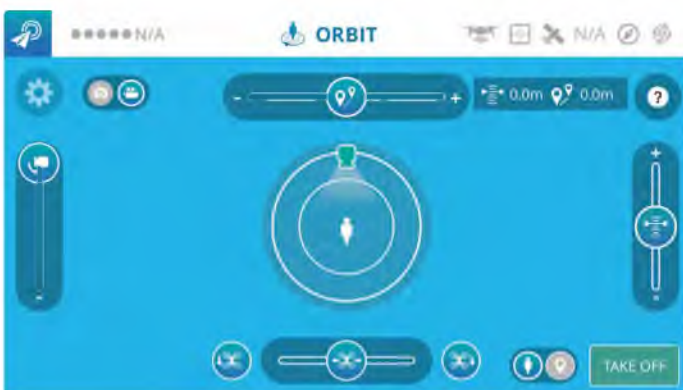
Automated modes, like Orbit shown here, use sliders to give you fine control of the quadcopter
