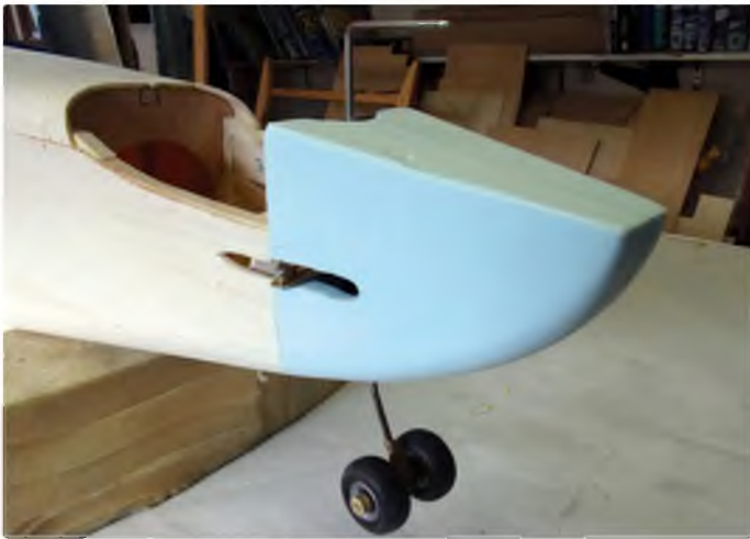
Tail wheel assembly and rear fairing in place
