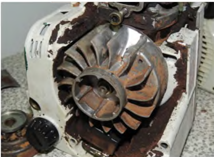
This is an example of a flywheel magneto as used on most hand tool engines and...
