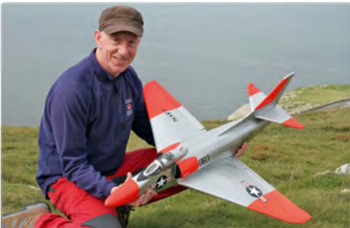
Harry Twist with his superb looking A-4D prototype. The model was covered in 25 g glass cloth and Eze-Kote prior to a spray paint finish, giving an AUV of just over 3 lb
