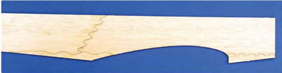
To make value for money kits it makes sense to cut wood from standard size planks. The wavy lines ensure close joints between the parts
