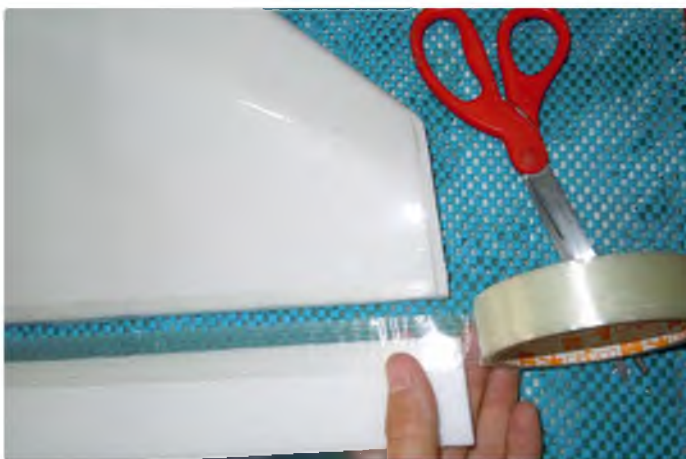
Use glass reinforced tape for attaching the TE and ailerons
