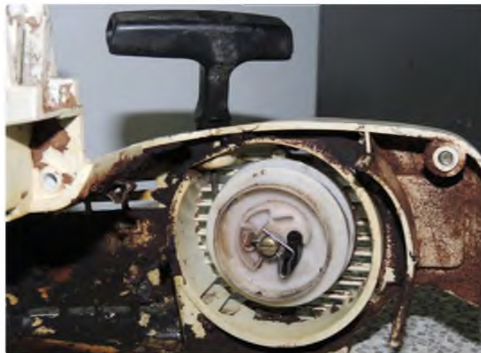
...this is the pull cord method of easy starting – much faster than hand flicking
