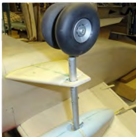
Winglet mounted and U/C leg fitted to nacelle
