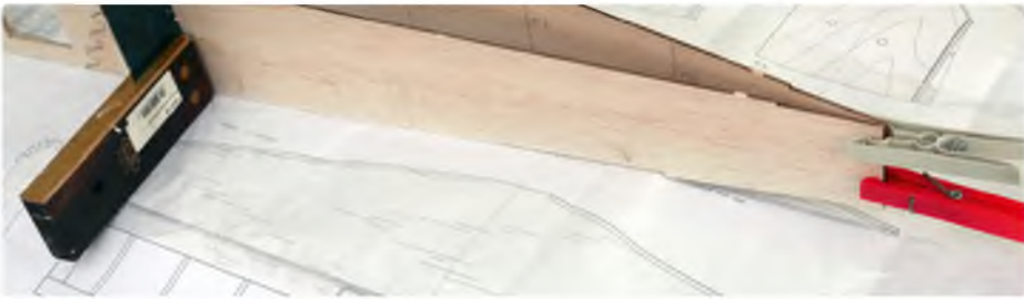
The first fuselage side is pinned to the plan along the fuselage outline. Note the clear poly sheeting laid over the top of the drawing to stop the fuselage sticking to the plan
