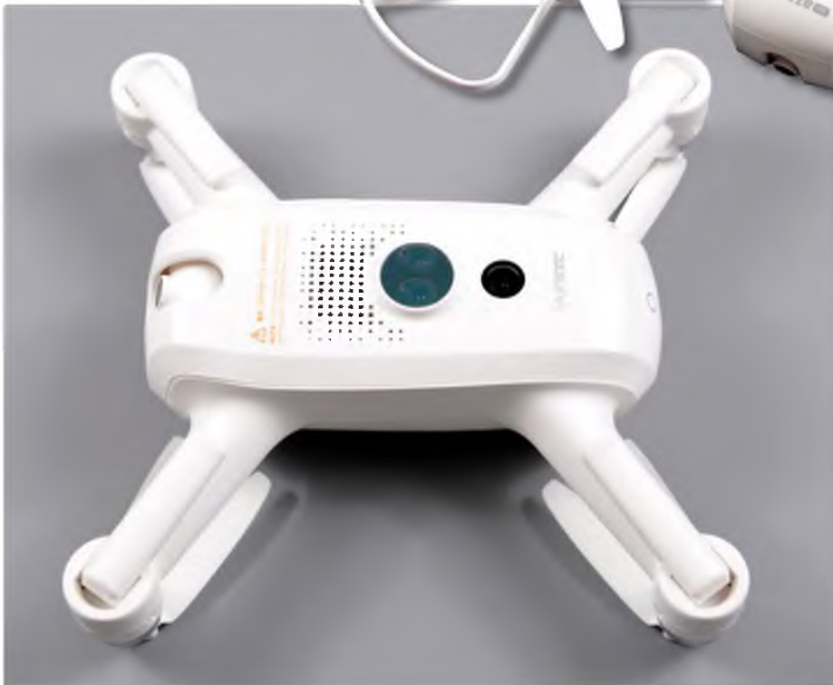
Bottoms up! Here you can see the optical flow and infrared positioning sensors
