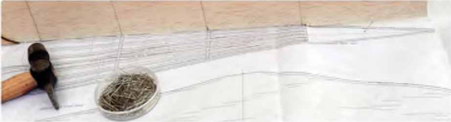
Mark the fuselage sides with the former positions to make it easy keep them vertical whilst gluing
