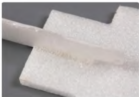
Edge on joints work well on either Depron or balsa
