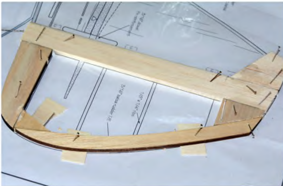
If the trailing edge of the rudder and elevators are not supported by shims you will get warped control surfaces
