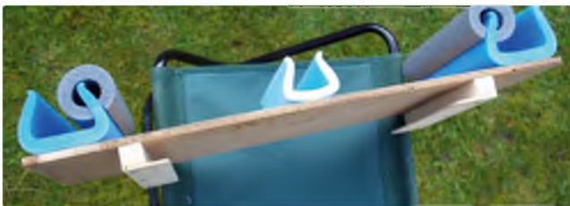
Front elevation of the stool top model stand, described in the text. The 'U' shaped PVC foam is usually used for protecting furniture legs and edges. The round stuff is normal pipe lagging, with the outside diameter chosen to fit snugly inside the 'U' channel, for storage. The 'L' shaped pieces fit round the stool top rail
