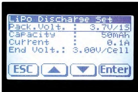
Left: The two circuits can discharge LiPo packs too. The default End Voltage is wisely set to 3 V per cell
