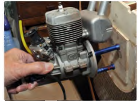
Rear exhaust NGH petrol engine fitted to stand-offs. The box is not glued yet and is free to slide in and out to make sure the cowl distance can be accurately set
