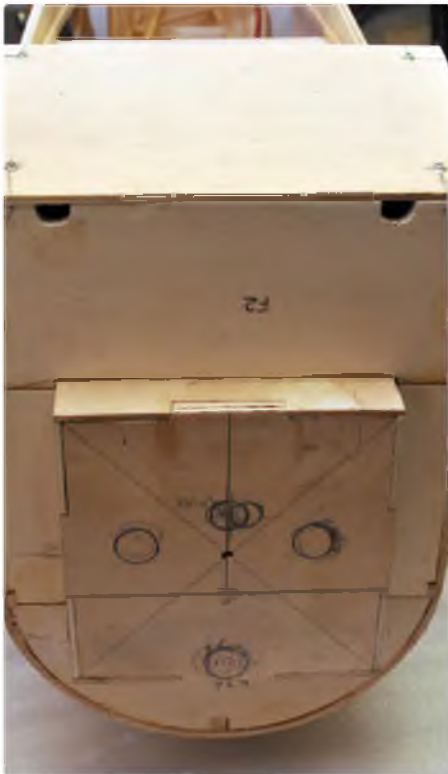
Fuel tank box and engine firewall mount marked up. Care must be taken here to ensure accurate alignment
