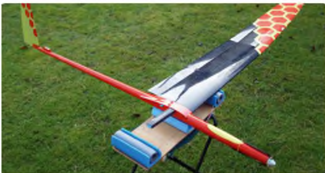
Stand in action, with a Pike Perfection part assembled. The width of the plywood top (575 mm) was chosen to allow a model to balance (just!) in this condition, while I reach for the other wing. The Pike wing is quite low mounted and the round foam is not needed, so is left in 'store'
