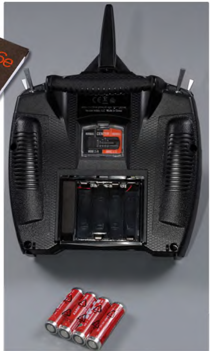
Back of the case showing the spring configuration switch and battery box. Four AA cells are provided so that you can use the DX6e straight out of the box
