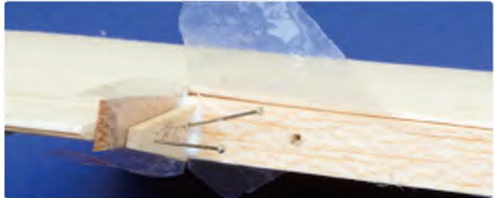
Next stage is to add end ribs with spacers to ensure easy movement
