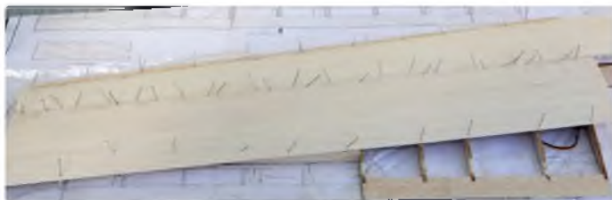
Build the wing to this stage and leave it to dry completely before removing from the building board. The washout is now locked into the build
