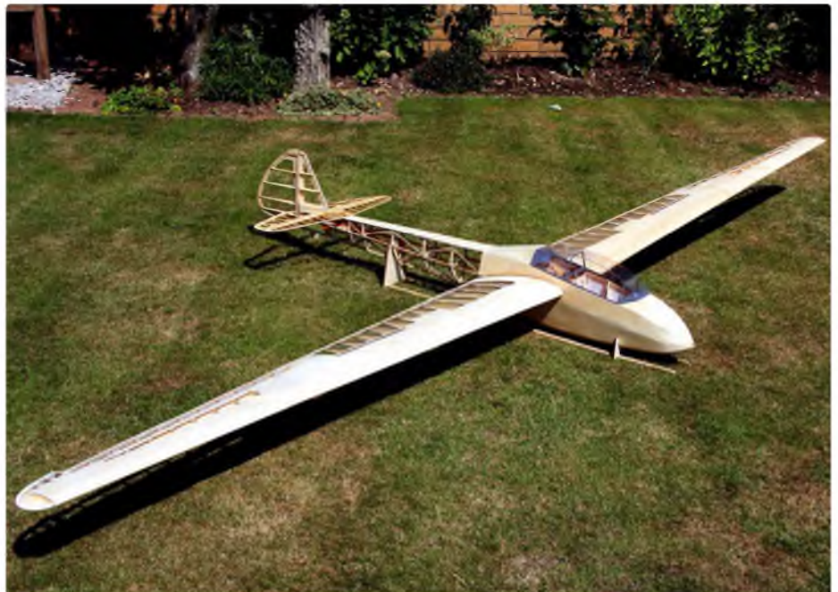
Trail assembly of fuselage and wings before covering. In this state it would make a very nice display model
