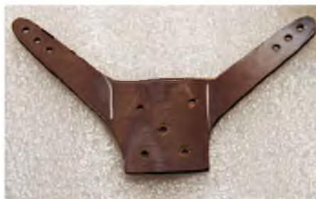
Above & below: Cardboard template was made to ensure the correct size of rudder control horn, and the final Paxolin horn ready for finishing
