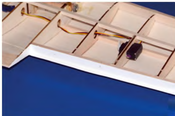
If the aileron housing isn't covered before fitting the aileron it will never be possible to do the job properly
