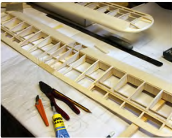
Lower wing panels propped up to the correct dihedral for joining with ply braces
