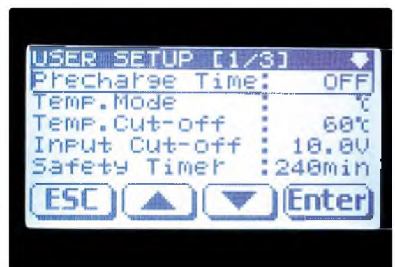
Left & Right: Scrolling round the arrows brings you to the Setup page where you can set up the charger to suit personal preference over three pages of different parameters. Other pages are accessed via the small arrow, top right
