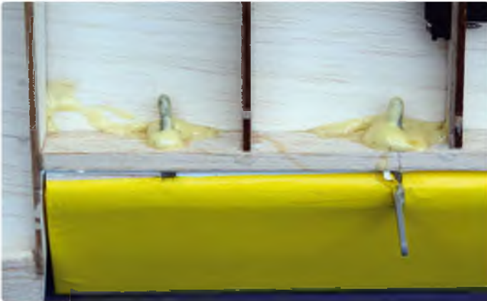
Four hours later Gorilla glue is rock-hard and everything near it is glued solidly in place
