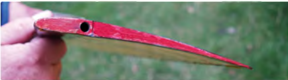
The Low Drag Airfoil on Gary Peck's home built 2m wing. Thin and cambered, it's not what eSoarers are used to! Maybe we will be, in time?
