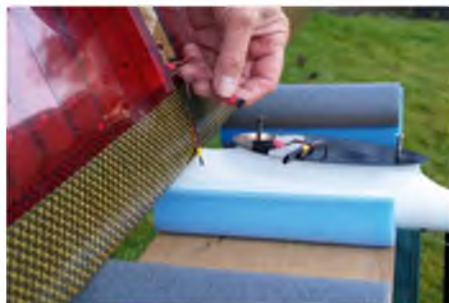
Once set for a high wing model the wing can be conveniently balanced while connections are made, before dropping it in place to secure the fixing screws
