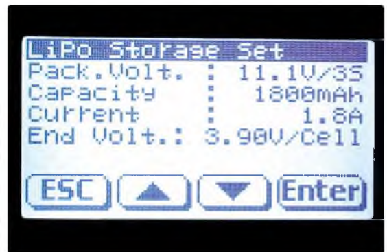
Right: Storage mode will automatically charge used packs or discharge unflown packs to a safe storage condition. Default 'End Voltage' is 3.85 volts per cell, but I've tweaked it a bit higher to suit the recommendation from the manufacturer of the pack I've been flying
