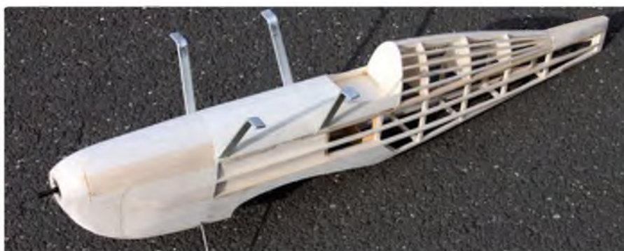
Build up the front decking. Add the rear formers, spine and stringers, along with the block balsa tail mount
