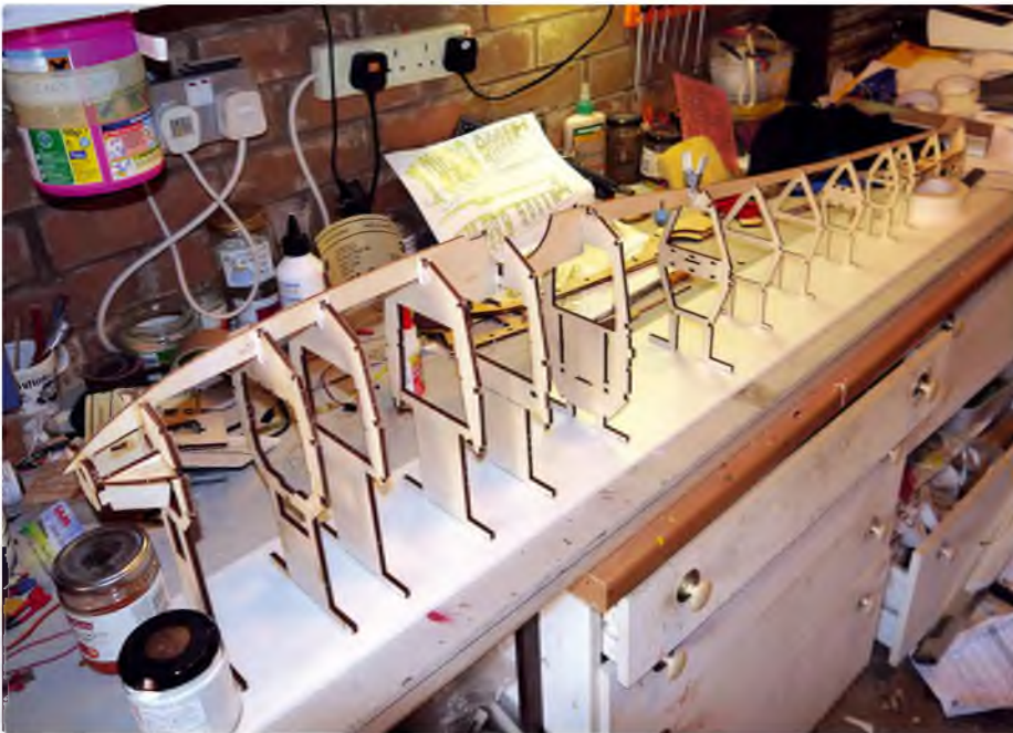
The fuselage is built inverted using the foam templates to position the fuselage formers. Note the building tabs and interlocking keel to ensure everything is aligned correctly. Apologies for the messy building board!
