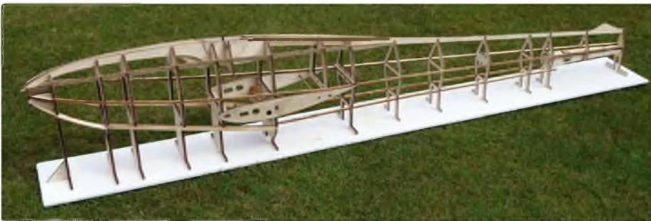
The basic fuselage assembly is complete and ready to be removed from the foam building jig
