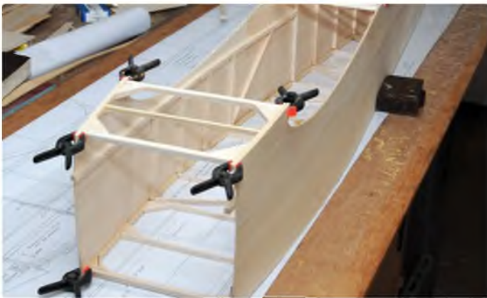
Sides glued and clamped in place to the top and bottom pre-fabricated frames
