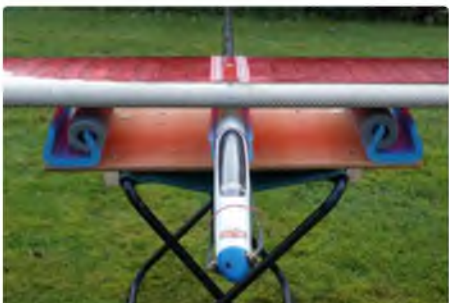
If using a model like this AVA, with a high mounted wing, the extra lagging is used to fill the gap to stop the wing wagging
