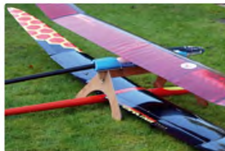
This simple slot-together holder can be used for assembly and, as shown here, for double-decking models in gazebos when space is at a premium. Normally the model with the greater dihedral goes on the bottom
