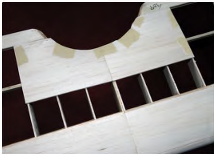
Sheeting the top wing centre section
