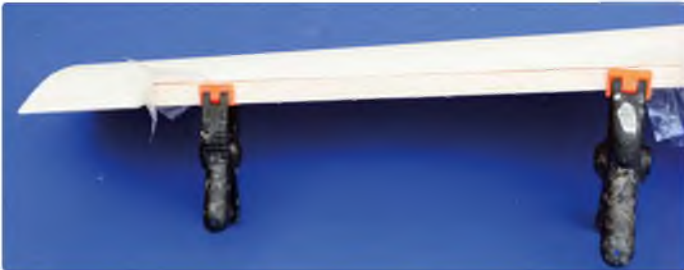
Position the aileron leading edge against the rear spar and butt up against the overhanging sheet
