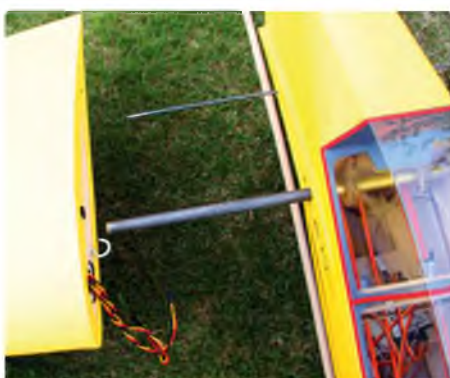
Wings are supported by a strong steel wing joiner, which slides into brass tubing in the wings and fuselage. The thin wire joiner at the rear of the wings provides alignment
