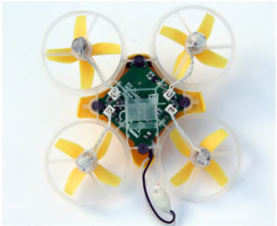
The PCB board is visible under the quad. Plug-in motors make for easy replacement
