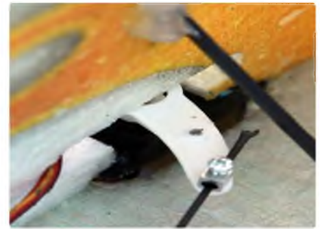
The extended aileron output arm requires a more powerful micro servo
