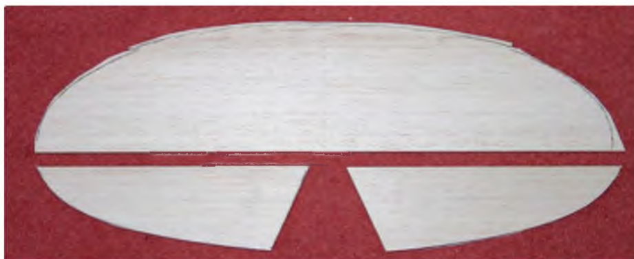
The tailplane is from medium soft 3/16" balsa sheet. Transfer the shape to the balsa and rough cut to shape
