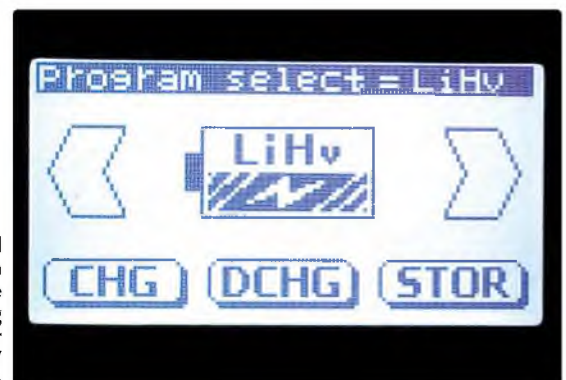
Right: Typical Main Screen page. This one is the starting point for charging LiHV packs
