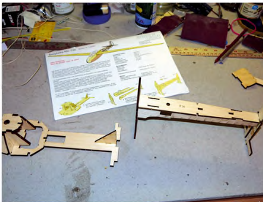
Building starts by assembling the fuselage nose and tail sections with interlocking parts. The printed manual is in German but a very good English version is available for download from aero-naut's website
