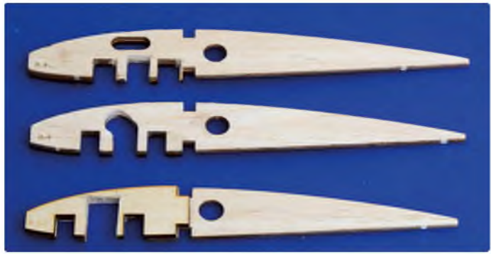
Holes for the electric retract unit, oleo legs and cabling significantly reduce support for the undercarriage mounts
