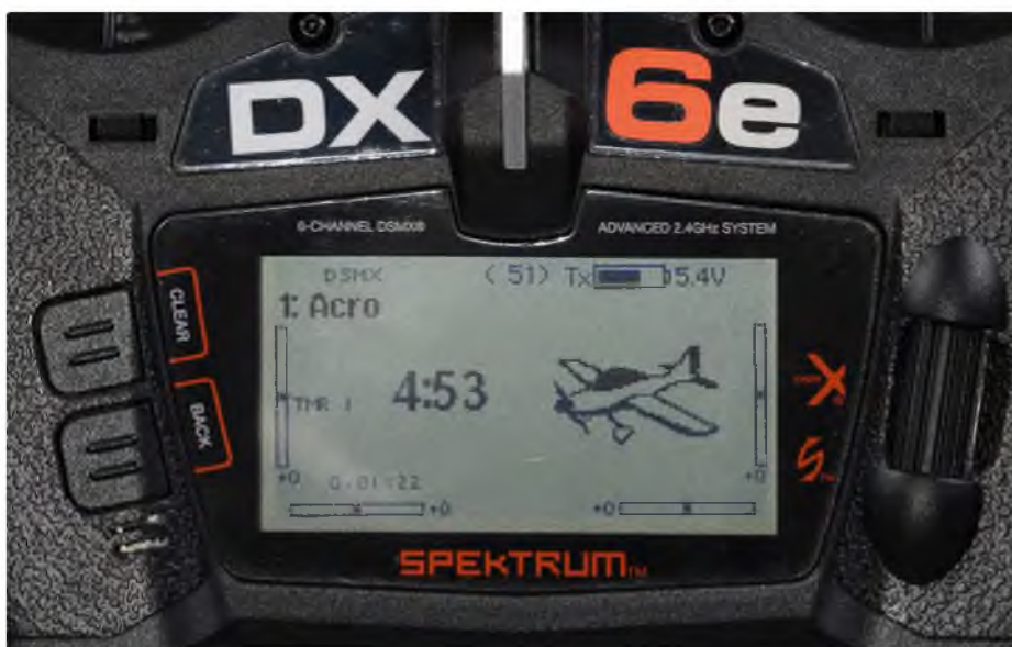
Menus are easily navigated on the clear LCD screen using the scroll bar (right) and push buttons (left)
