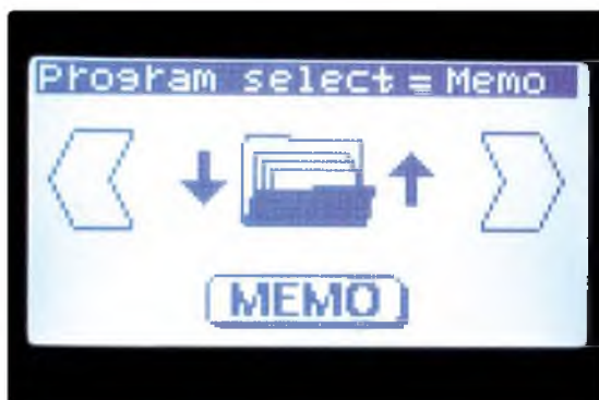
Left & Right: Memory is accessed via the Charge or Discharge icons and can be used to save the parameters of up to 20 battery packs. This provides a quick way to set up the charger for your favourite packs
