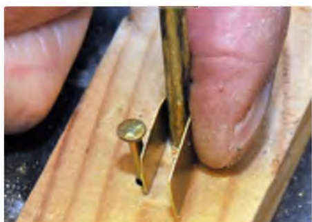
Bending sheet brass on a simple jig to form the windscreen fixing brackets. Much patience is required! They are then crimped to final shape before finessing and drilling for the retaining bolts
