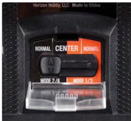
The patent-pending gimbal design lets you change spring configurations simply by moving this slider switch on the back of the Tx
