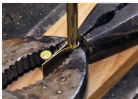
Bending sheet brass on a simple jig to form the windscreen fixing brackets. Much patience is required! They are then crimped to final shape before finessing and drilling for the retaining bolts
