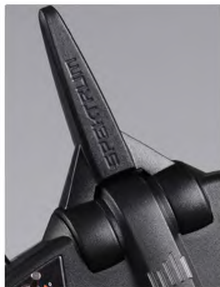
The angular aerial moulding is mounted on an inverted Y shaped pivot
