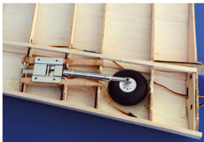
This is how the leg needs to sit in the wing. Note how the forward mounting bearer has had to be cut away to allow the leg to retract
