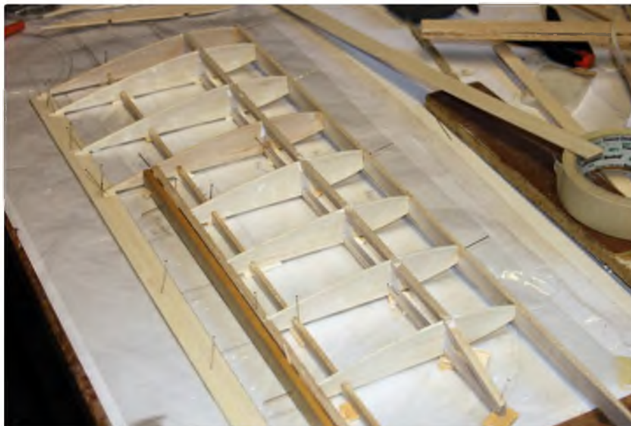
Wing panels are built one at a time directly over the drawing on a flat board. Pin the trailing edge down over the plan and then the two lower spars using 1/16" sheet packing pieces to lift them to the same height as the trailing edge
