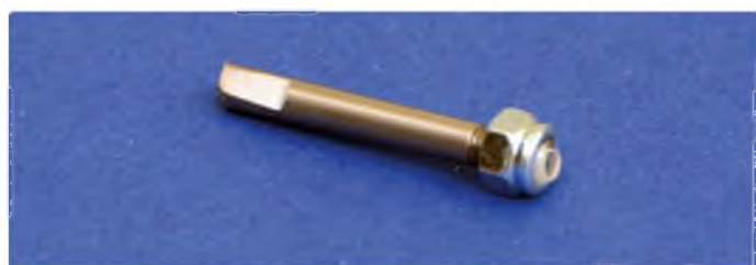
Flat spots on the piano wire give the grub screws that hold it in place something to grip onto and also prevent the wire rotating and falling out of the holders
