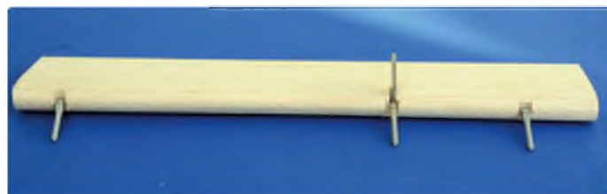
Robart hinges are also available with a moulded in control horn to make life simpler
