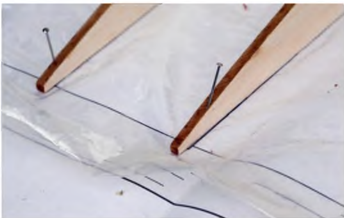
The ribs behind the spar are flat, making accurate building easy
