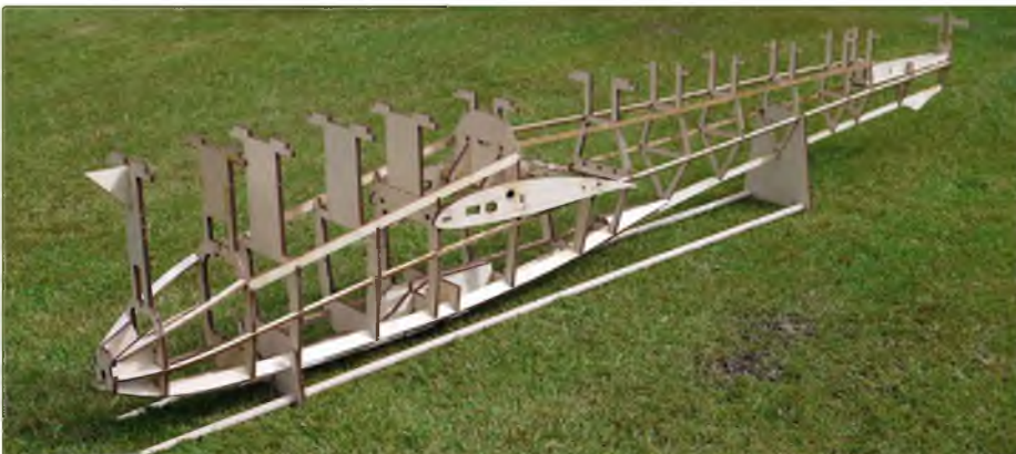
After the fuselage is removed from the foam building jig the building tabs on each former need to be cut off. A stand is thoughtfully provided to hold the fuselage in the upright position
