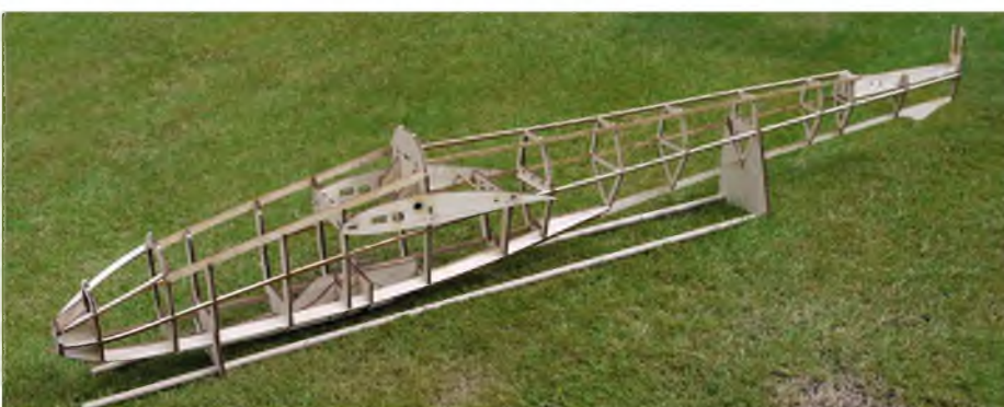
Basic fuselage after the building tabs have been removed
