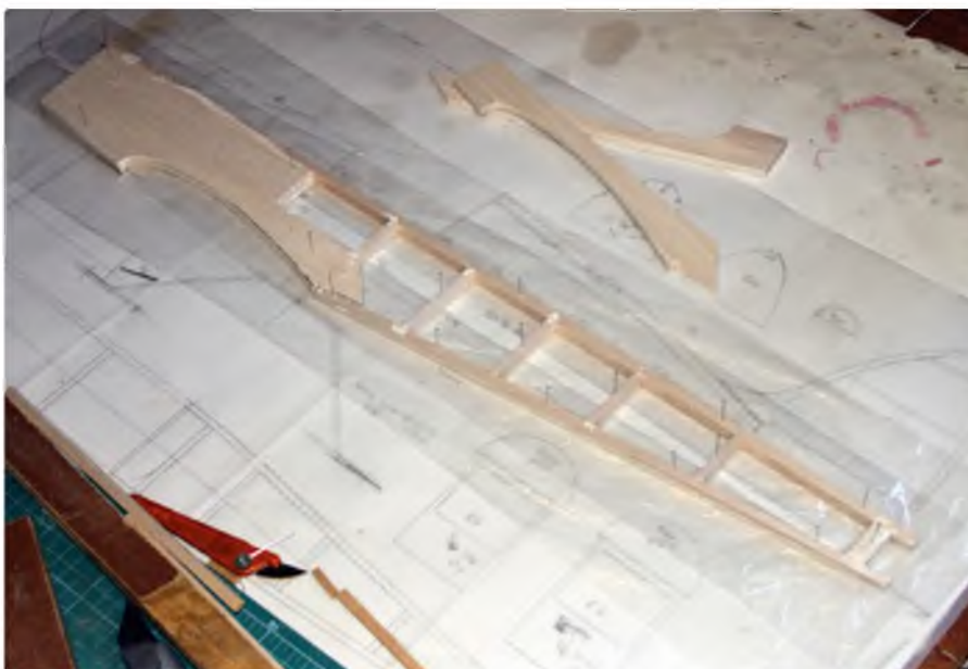
Pin the fuselage longerons down and fit the uprights and sheet balsa parts. When dry build the second side directly over the first
