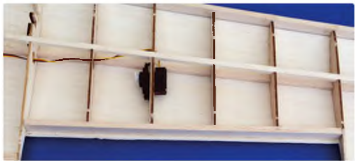
Sheeting needs to extend past the back of the rear wing spar for the shrouded aileron system
