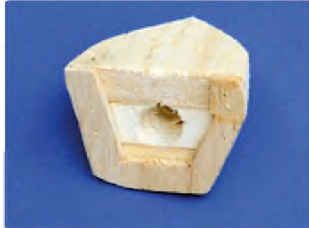
The rear of the cooling tunnel needs to be made from scrap block balsa. The hole mimics the full size aeroplane's construction and allows the tunnel to be used effectively
