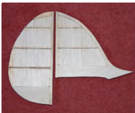
The fin and rudder are built up using 1/16" sheet balsa cores. Spars and ribs are then added to each side
