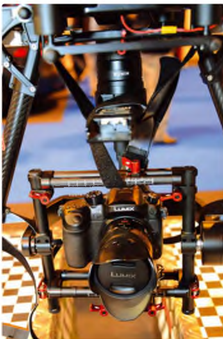
The Panasonic stand featured a DJI Matrice fitted with a Lumix GH4 camera on a Ronin gimbal
