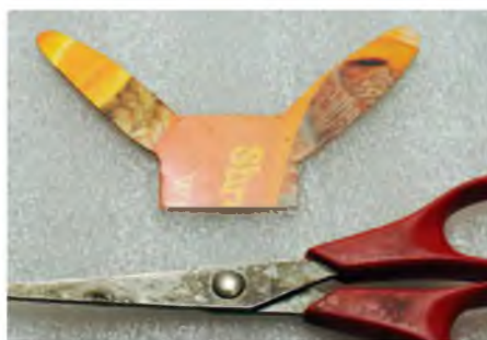
Above & below: Cardboard template was made to ensure the correct size of rudder control horn, and the final Paxolin horn ready for finishing
