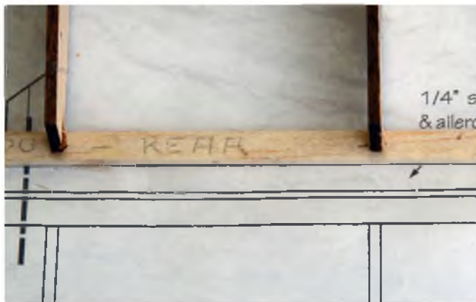
Position the jigs so that the wing spar follows the washout line
