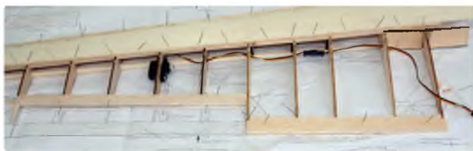
Ribs 1-5 are built flat on the building board; the rest are lifted for washout
