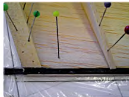
Ding-proofing the rudder. Carbon fibre being laid between the balsa skins at the TE
