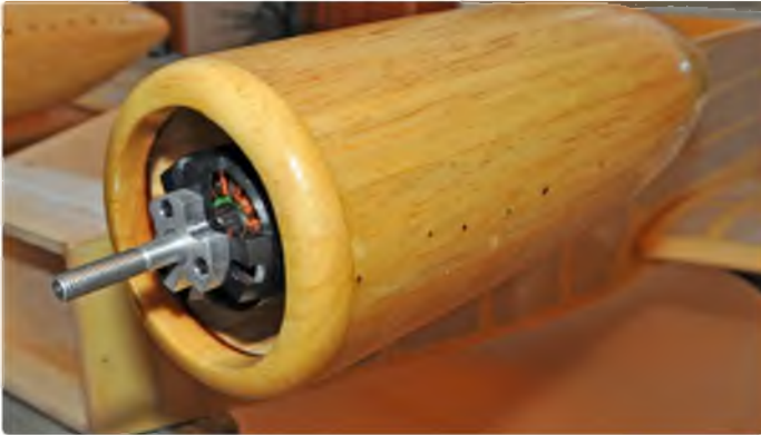
Motor pods are circular in cross-section, built on a horizontal crutch to which half-formers were added. Each assembly was then planked with half inch strips of 1/8" balsa
