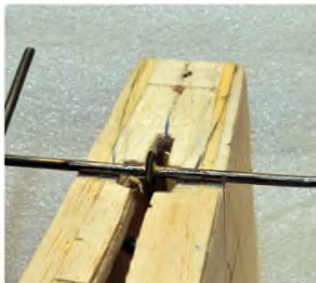
One piece elevator control arm silver soldered to control horn
