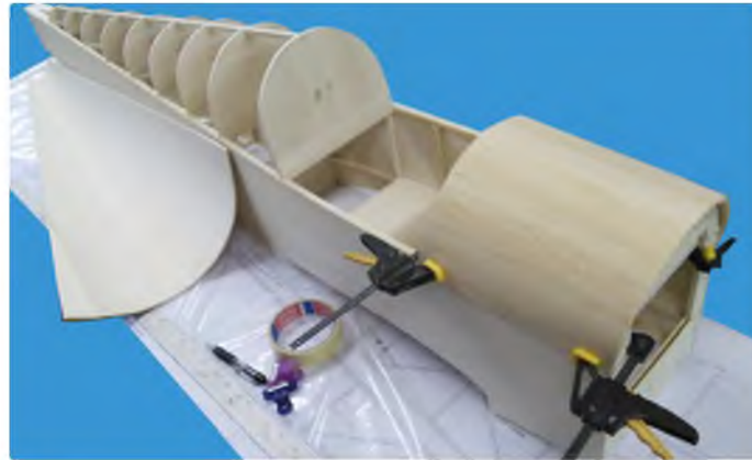
Test fitting the pre-formed front deck balsa skins
