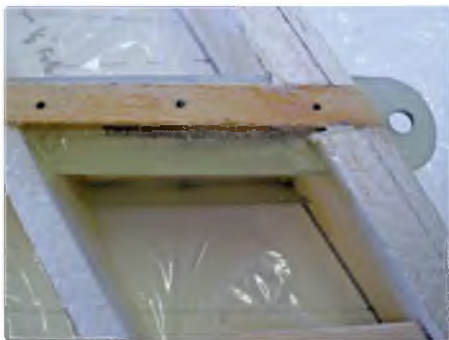
Tailplane pivots bonded to fin spars – note the holes for the alignment pins
