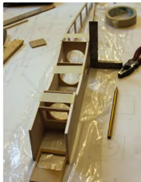
Fit formers, then use a try square to make sure that the sides are at 90 degrees to the building board
