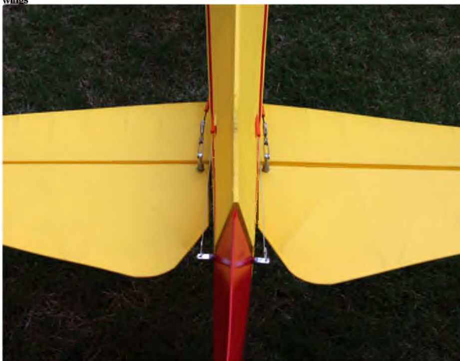
Rudder control is by closed loop and elevators by wire pushrods running in tubes. Metal horns are glued into position after covering
