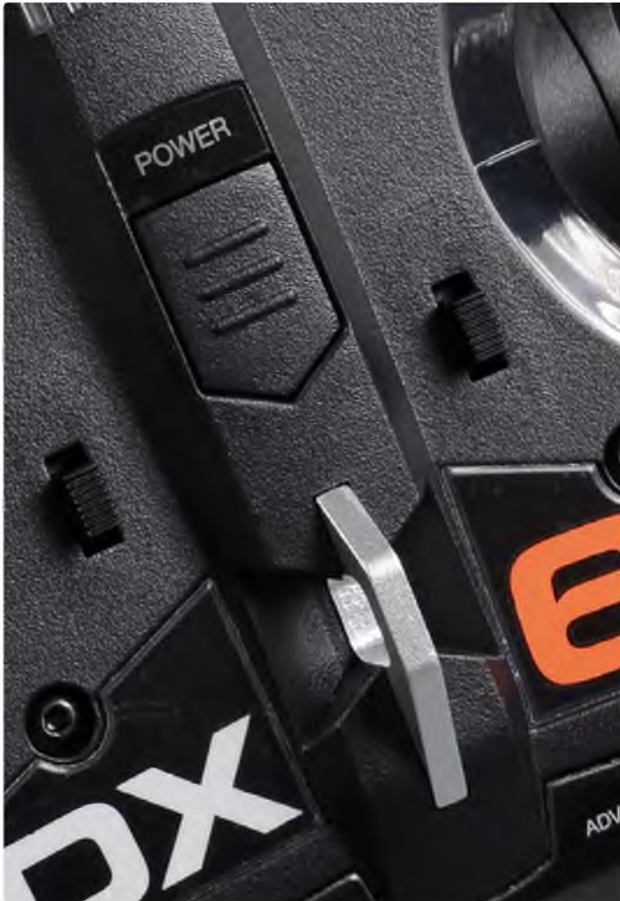
Close up showing the push button power switch and the low mounted neck-strap hook that offers near perfect balance
