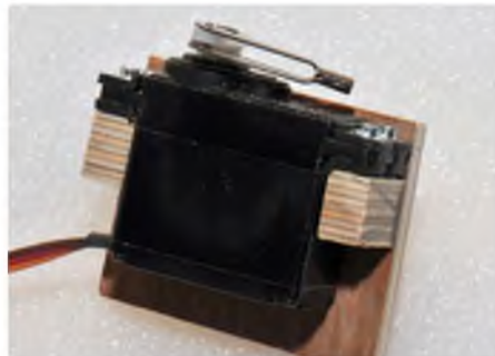
Throttle servo on its custom made mount and ready for fitting
