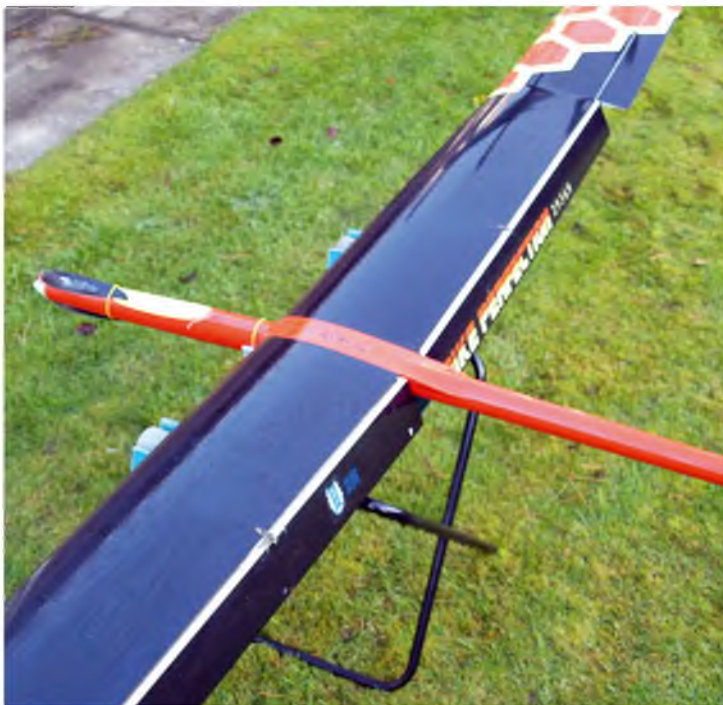
Once assembled the model sits happily on the stand and with the flap hinge line just beyond the foam the full brake flap deflection can be checked. If the weather is breezy the stool frame can be pegged down for stability. This is more essential if using a taller stool
