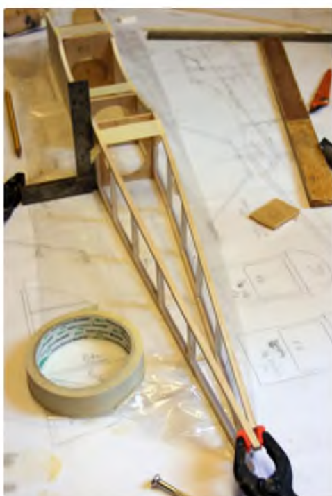
Pull in, glue and clamp the tail posts together, making sure the fuselage is straight before leaving to dry
