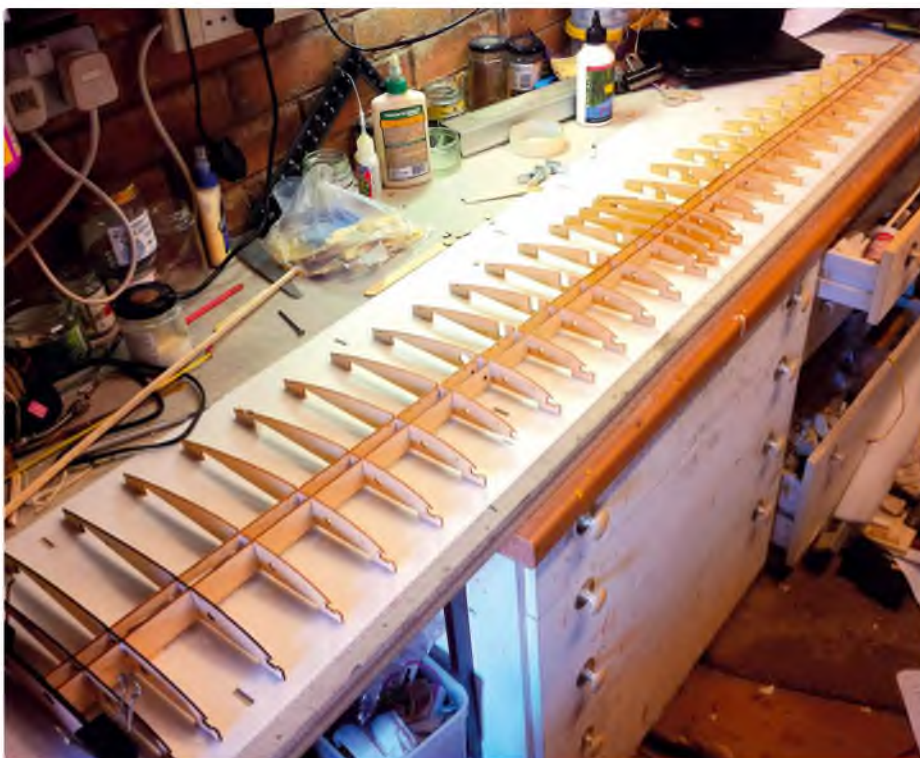
Wing construction starts by fitting the ribs into two ply spars. Placing the tabs into slots in the foam building jig ensures an accurate build
