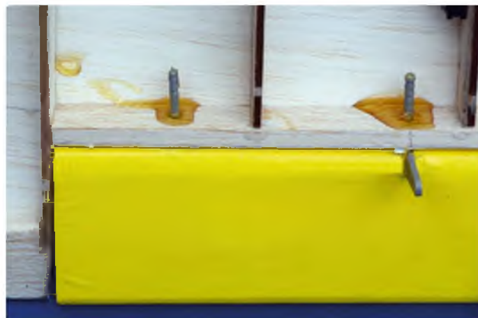
Gorilla glue is very sticky but quite runny when first applied
