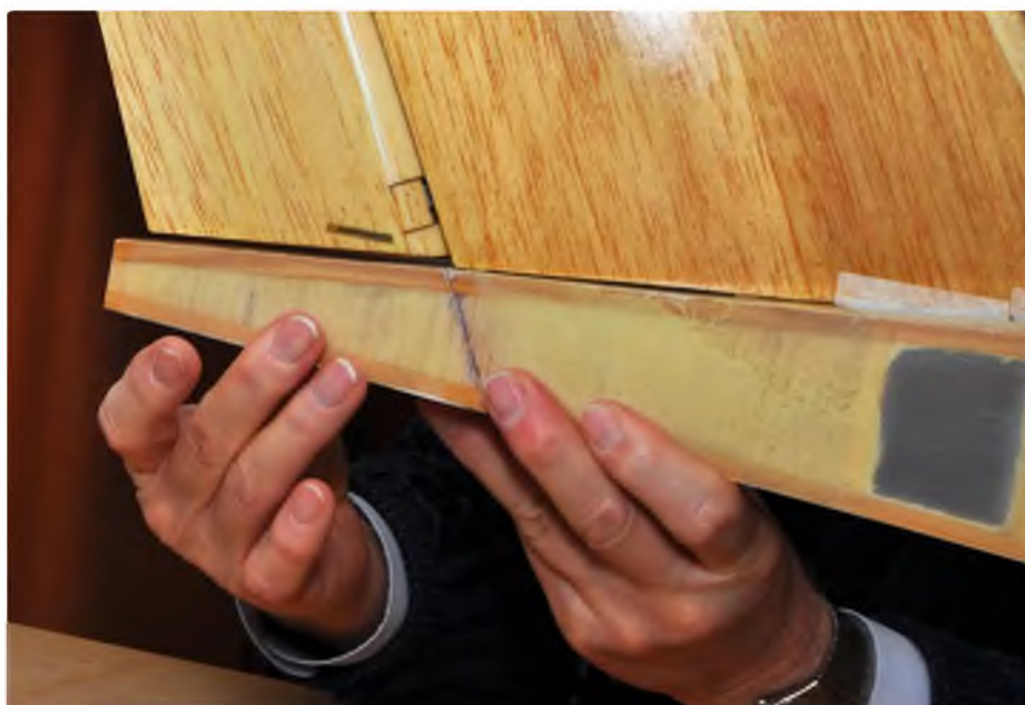
The rear of the fuselage had to be made removable to fit the rudder after finishing
