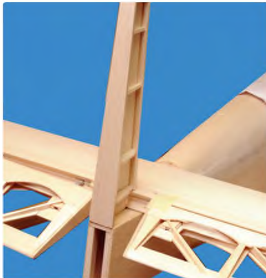
Test fit of fin and tailplane to check the hinge positions
