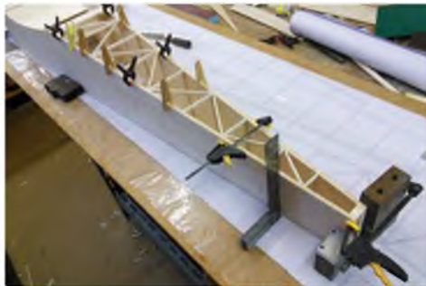
Clamping the tail stock and making sure all is square
