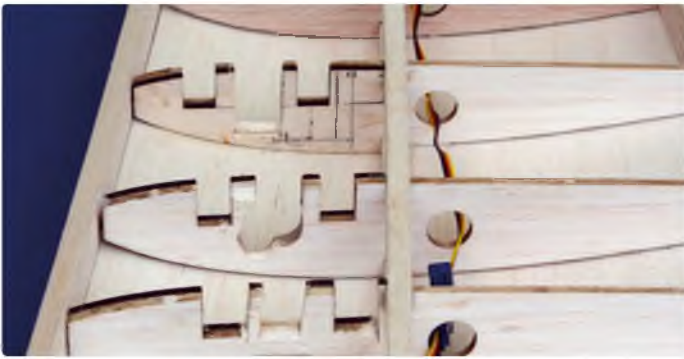
Lots of cut-outs were needed to accommodate the retracts
