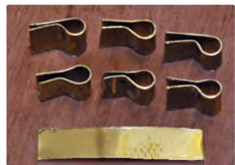
Bending sheet brass on a simple jig to form the windscreen fixing brackets. Much patience is required! They are then crimped to final shape before finessing and drilling for the retaining bolts
