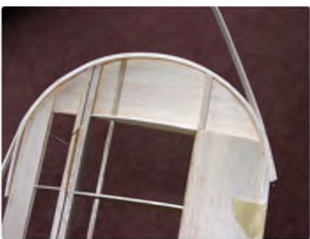
Wingtips are made from balsa sheet capped with 1/16" laminations
