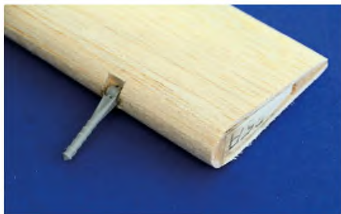
Completed aileron with curved nose section and recessed Robart hinge
