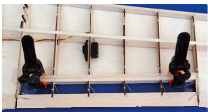
Intermediate ribs stiffen up the aileron before sheeting is applied
