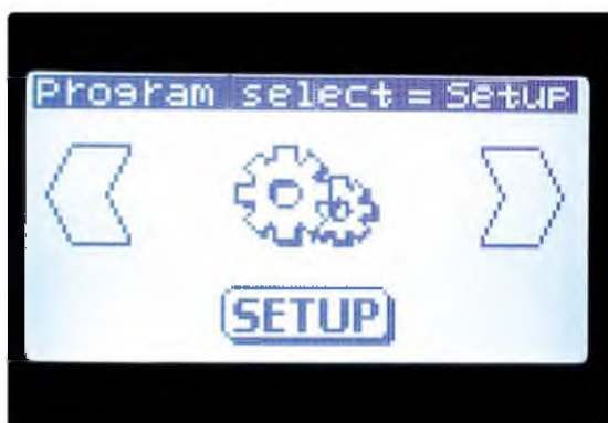
Left & Right: Scrolling round the arrows brings you to the Setup page where you can set up the charger to suit personal preference over three pages of different parameters. Other pages are accessed via the small arrow, top right
