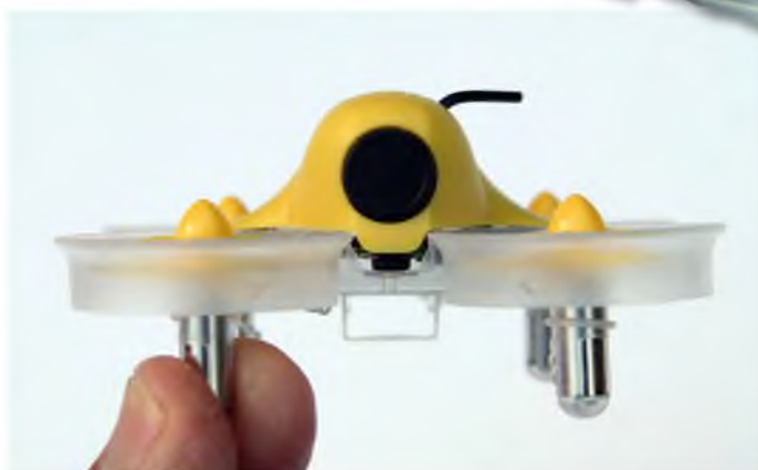
My fingers give scale to this diminutive FPV quad. Motors provide the landing gear for this tiny 'small space FPV flyer'
