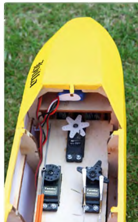
Just visible are the ballast boxes in the nose for adding weight to obtain the required Centre of Gravity. A removable plate above the ballast boxes houses the receiver battery
