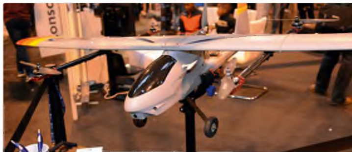
Consortiq also displayed this interesting fusion of fixed wing and quadcopter airframes
