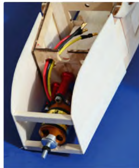
The cowl sides need gluing in place with cross pieces to keep them positioned properly
