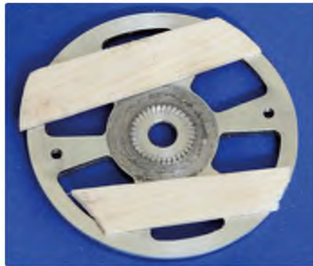
Use scrap balsa temporarily glued to the spinner backplate to create a gap with the cowl front
