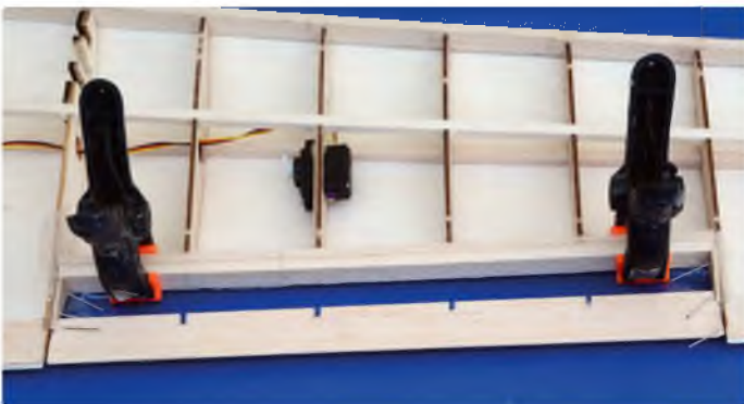
The aileron trailing edge can be aligned to the wing trailing edge and that creates an aileron following the wing washout
