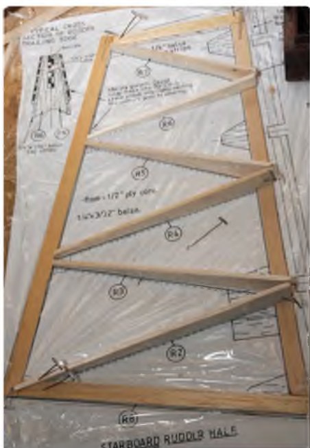
Outer frame of rudder with half formers in place
