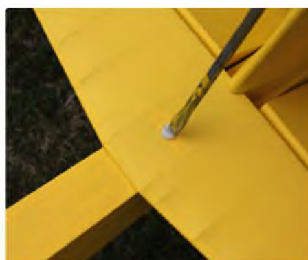
The tailplane is fitted with a single plastic bolt, with a pin between the tailplane and rudder ensuring alignment
