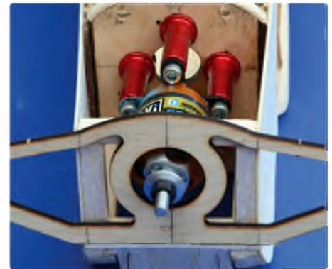
The cowl front can be lined up with the cowl framework once it has been allowed to dry
