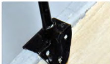
The brass tube windscreen former is held in place with brass brackets
