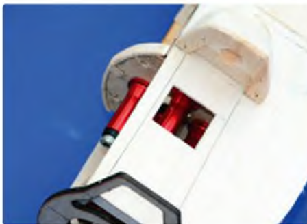
A cut out in the cowl side will create a pressure differential, which will remove hot air from around the motor
