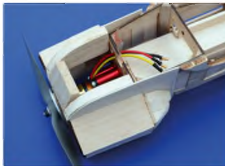
The interior frame of the cowl is made from 9 mm (3/8") balsa to allow for curving of the cowl shape later on
