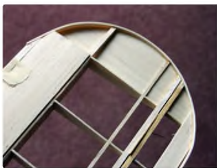
Wingtips are made from balsa sheet capped with 1/16" laminations
