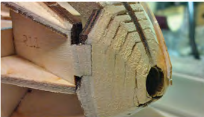
The nose section is made up of laminated parts sanded to shape. The hole allows for fitment of a tow-release for aerotowing
