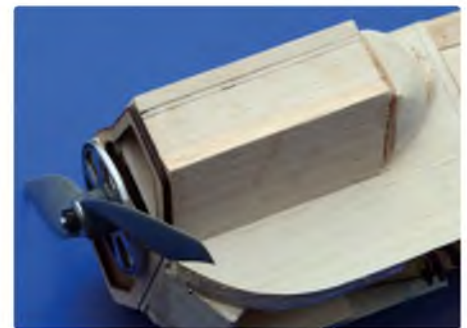
Hollow cowl cheeks can be made with scrap 1/8" or 1/4" balsa. As an added bonus the cooling tunnels can be used to do the job they are designed to do!
