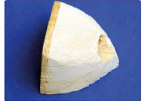
The rear of the cooling tunnel needs to be made from scrap block balsa. The hole mimics the full size aeroplane's construction and allows the tunnel to be used effectively
