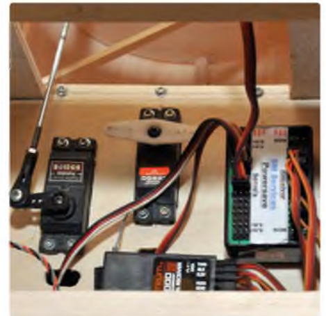
Radio bay showing the receiver, Powersaver, rudder and elevator servos
