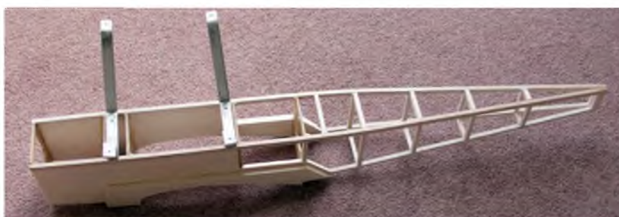
Basic fuselage assembly with cabane struts trial fitted
