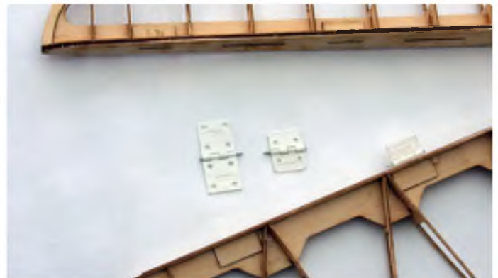
Pin type hinges are provided for the rudder and elevator. These require cutting down to fit, as shown
