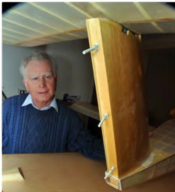
The rudder leading edge fits into a neat shroud at the back of the fin
