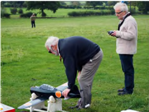
Neville holds the Zero firmly as Jonty advances the throttle on the still new O.S. 46 engine
