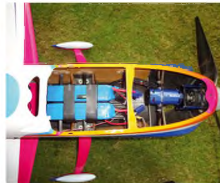
O.S. OMR-4043-172 brushless motor with gearbox fitted into Mikey Blake's Oxai Hybrid biplane
