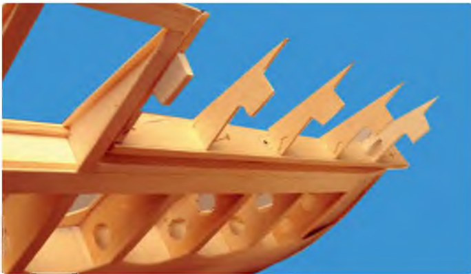
Ribs pinned to leading edge of aileron
