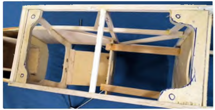
Looking down into the fuselage showing the undercarriage mounting plate and servo rails
