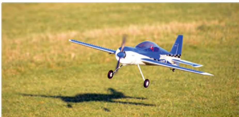
Lined up nicely for landing. It's best not to pull in large amounts of elevator in the flare or the AS3X system may compensate and push the model onto the ground
