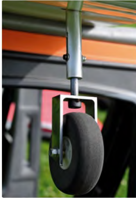
Aerospace quality materials form the nose leg
