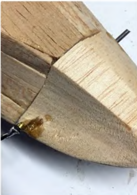
A wheel collar at the top will secure the nose gear leg
