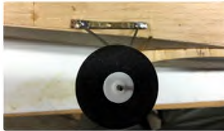
How the undercarriage is secured
