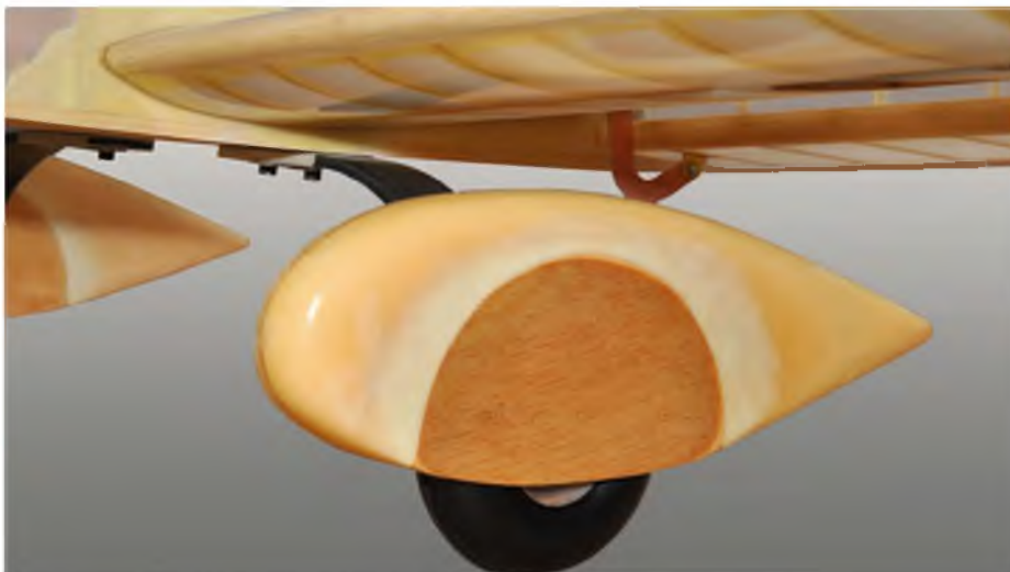
Underside view of the spat and undercarriage
