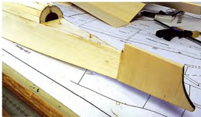
Left & below: The 1/4" tail end piece seemed vulnerable so I strengthened it with a fillet of balsa on both sides, running back to the fuselage sides and faired in
