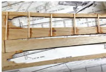
Positioning the uprights on the fuselage sides. See text
