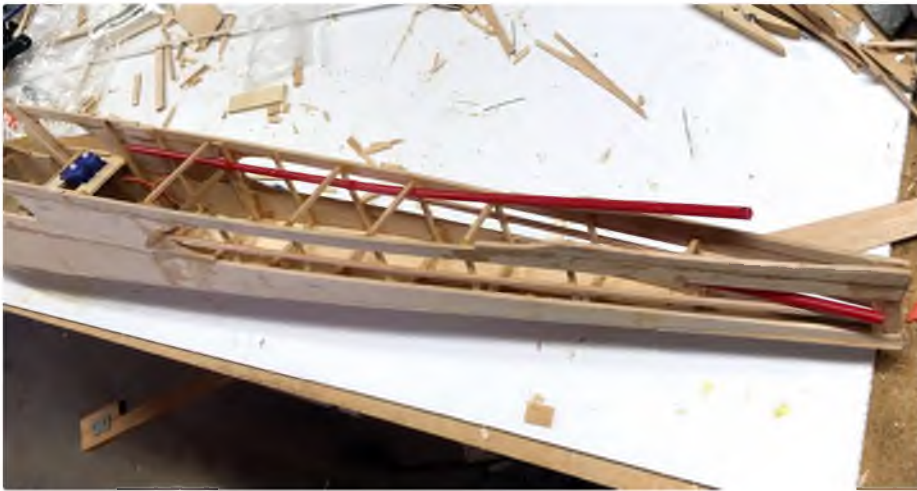
The servo rails and pushrod outer tubes were put in place while still accessible
