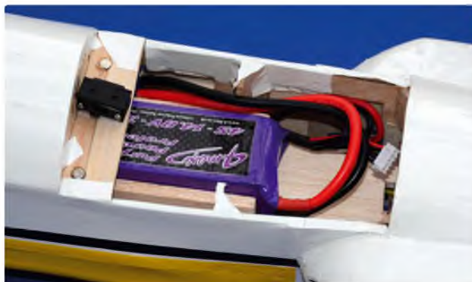
Make the battery box oversized so that the LiPo can be repositioned to get the C of G as you want
