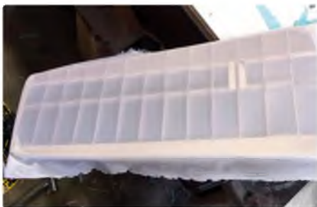
Nylon stuck to wing outer frame, awaiting doping
