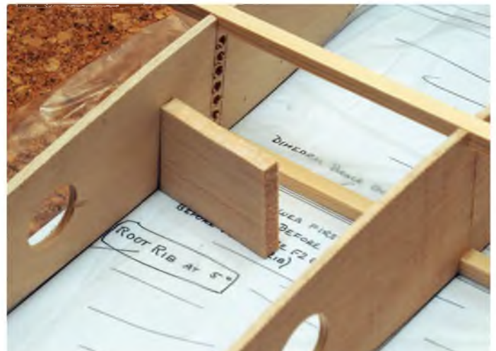
Setting the dihedral angle. Do this on both wings
