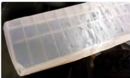
Nylon on the wing undersurface, doped and shrunk. Another coat of dope would have been good
