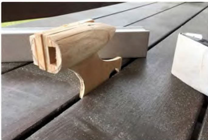
Shaping the nacelle. It's cosmetic but make sure the firewall is at the correct angle
