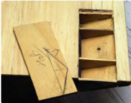
Ply ribs and plates for the wing bolt stress area
