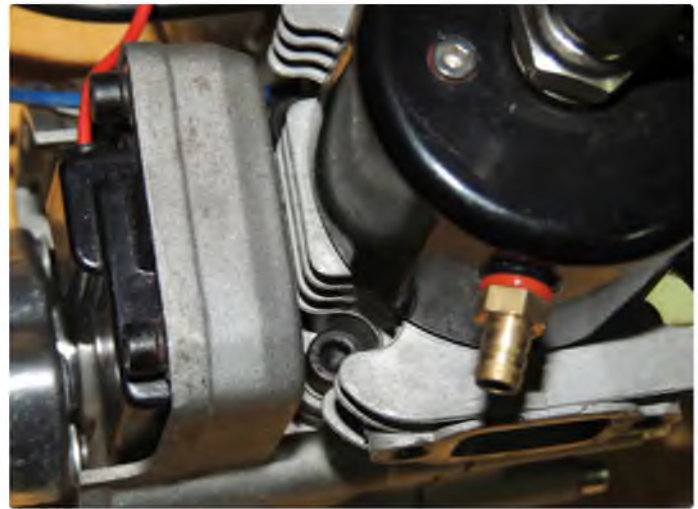
This is the access for that screw – not at all a friendly design
