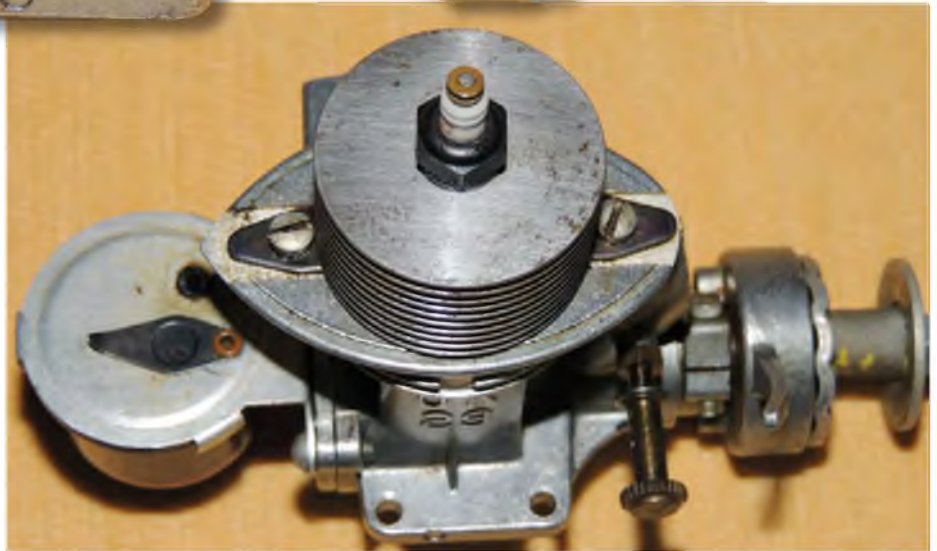
Another view of the OK 29. Those two small tags with the slotted screws retain the entire top end of the engine to the crankcase
