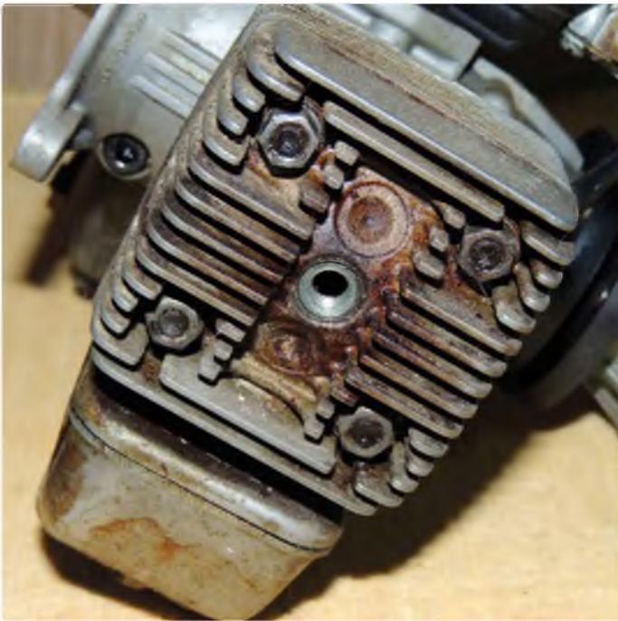
The head nuts on the cylinder studs of this twin engine are not at all easy to access but..
