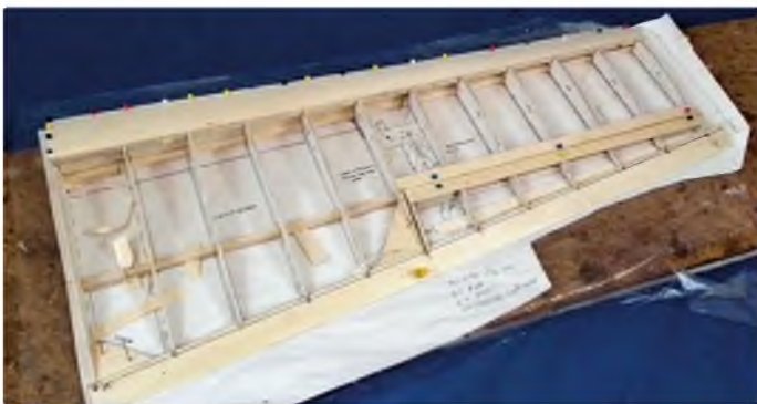
The wing ready to be lifted from the building board. The sequence described guarantees no warps
