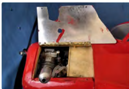
The hinged cowl side panels can be opened without removing anything
