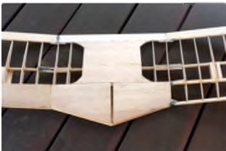
Outer panels attached. The left one needs LE sheeting at this point
