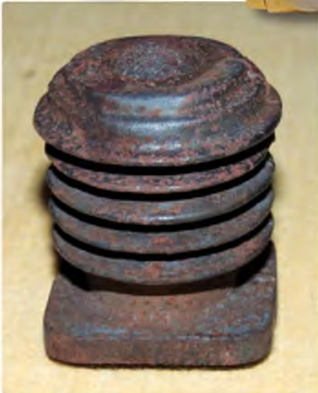
From a quite old DIY kit I have to build a medium capacity petrol four-stroke, this is the casting for the cylinder/liner – all in solid (damned heavy) cast iron
