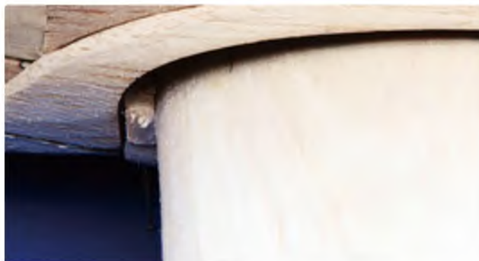
The wing has a very different shape at the exit point from the fuselage, but don't worry as it is easy to fill and is normal for a tapered wing design
