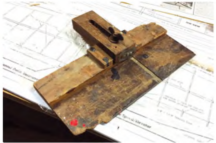
My old balsa stripper was useful for making missing balsa strips. It's older than the kit! A stiffer blade would be even better
