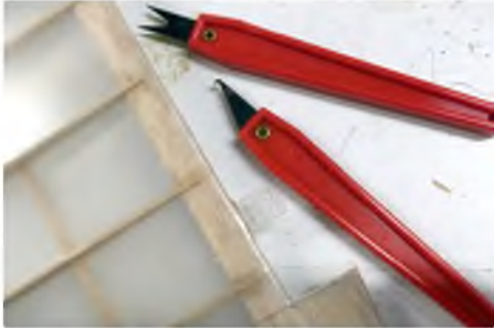
The covering film used on the tailplane would not accept any glue so I couldn't use the cloth strips. Be very careful when cutting hinge slots in 1/8" balsa!
