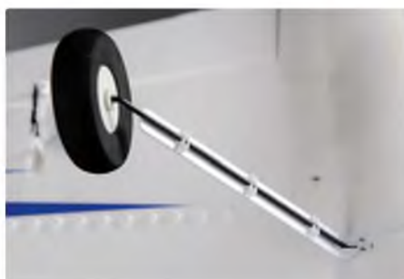
Oops! Don't forget to fit the leg covers, which are secured by the undercarriage fixing screws
