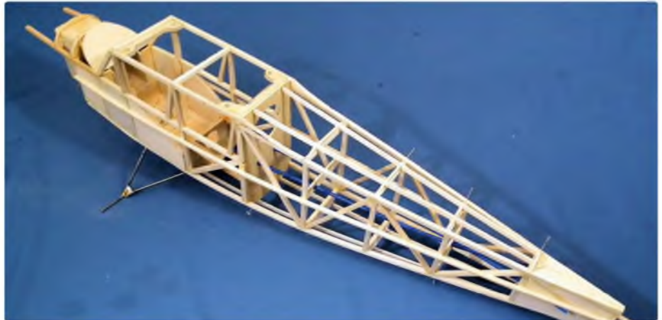
The stringers being added. One more on the sides is still to be fixed
