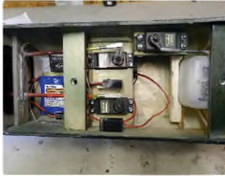
Radio installation. Note the rear mounted battery to help balance the fighter at its forward balance point for the maiden flights
