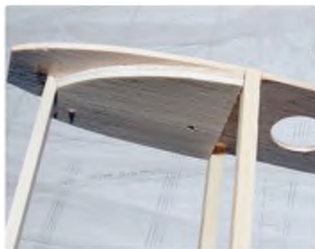
A balsa tip doubler is used to form the curve of the slot inner sheeting
