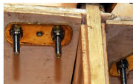
For all undercarriage brackets add a backing plate for the nuts to bite into
