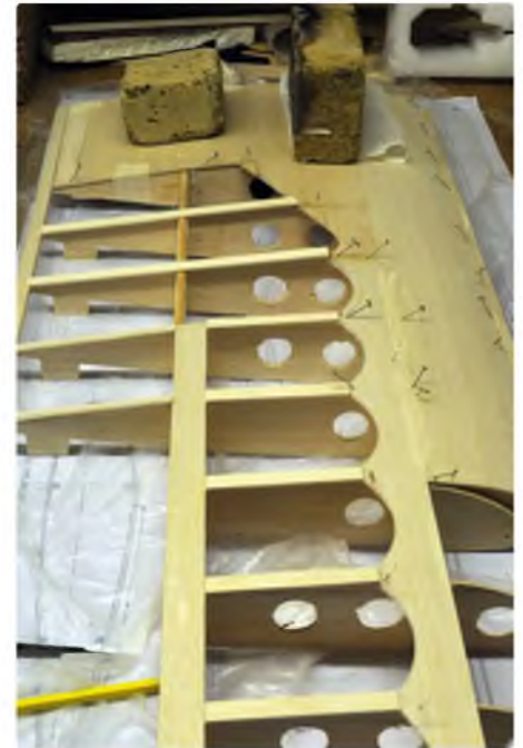
Top sheeting pinned and weighted to keep it in place. Note the separate scalloped piece
