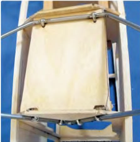
Underside showing U/C mounting in detail
