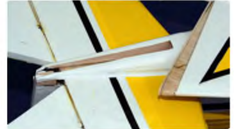
Solid fin mounting with a large area for gluing
