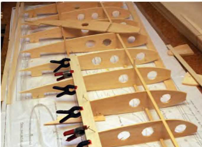
Ribs glued in place with reinforcing sheet on the ribs at the aileron spar
