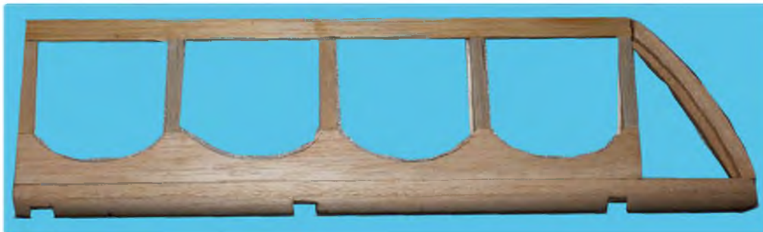
Ribs pinned to leading edge of aileron
