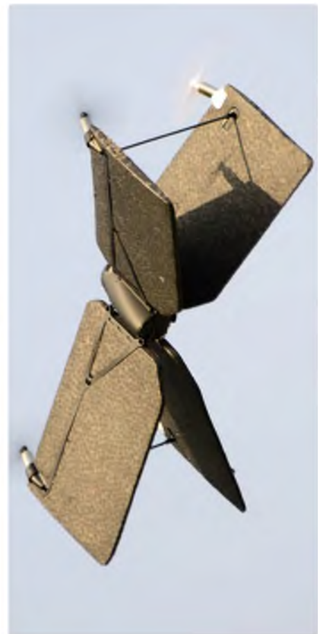
The EPO foam wing panels may seem fragile but have proved to be quite robust. Note the black underside to the body and wing struts
