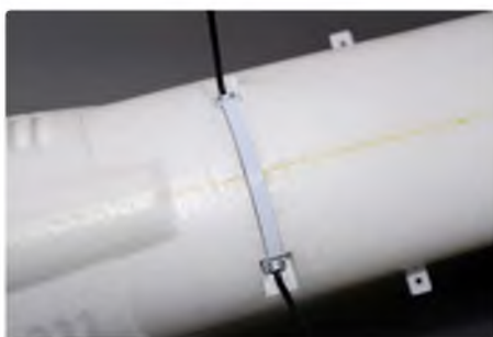
The wire undercarriage is fixed in place with a plastic strap
