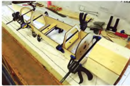
Clamping the front formers in place
