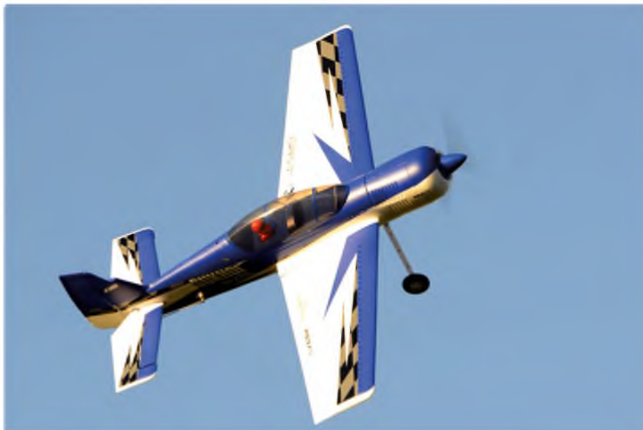
Ample rudder deflection during a knife-edge pass but the 13 g micro servos can deliver a lot more throw than that. Big throws at high rates are great for 3D stunts!
