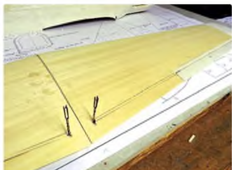
A channel is made either side for the torque rods. The well greased rods are glued in with epoxy and the veneer strips are put back on top. A neat job...
