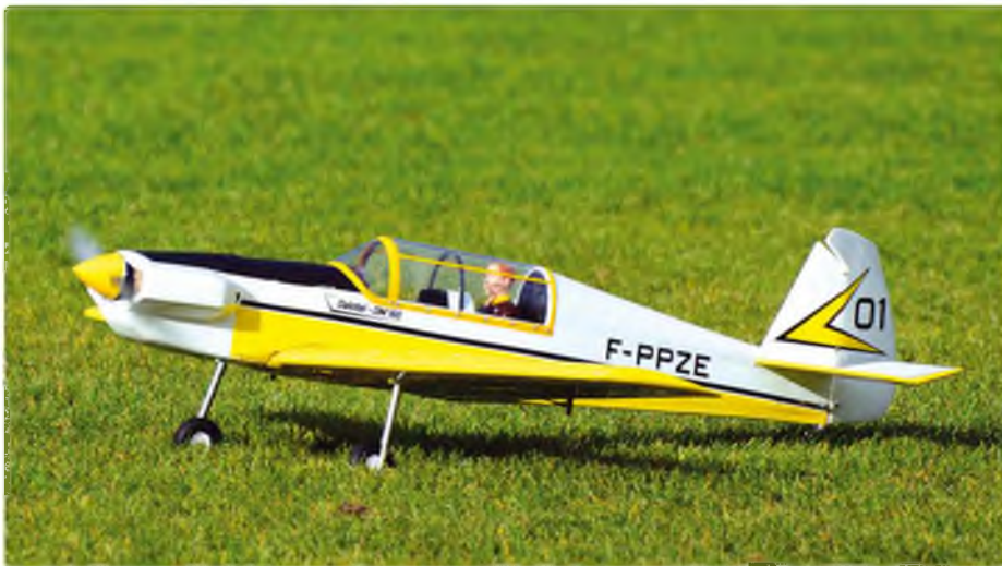
To combat the wet, relatively long autumn grass lots of up elevator was needed to stop the plane from nosing over at the start of the take-off run
