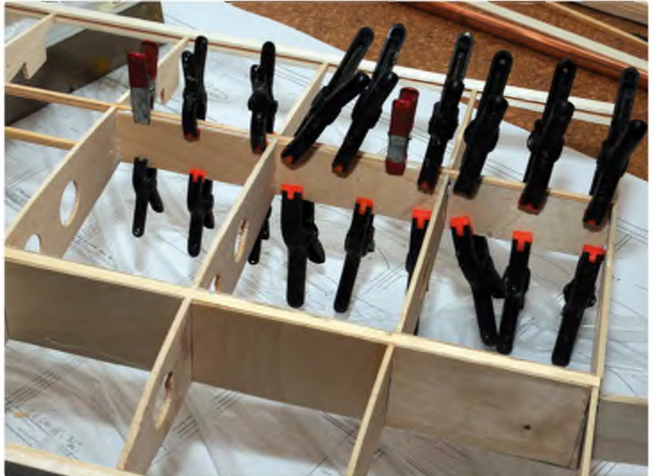
Ply spar webs to support the wing joiner
