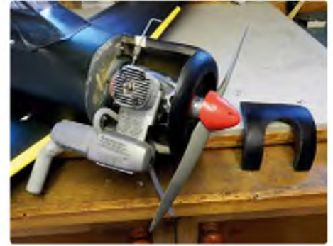
Reviewer's mod! The top of the cowling was made removable to allow easy access to the engine but it needs to be well secured in flight!
