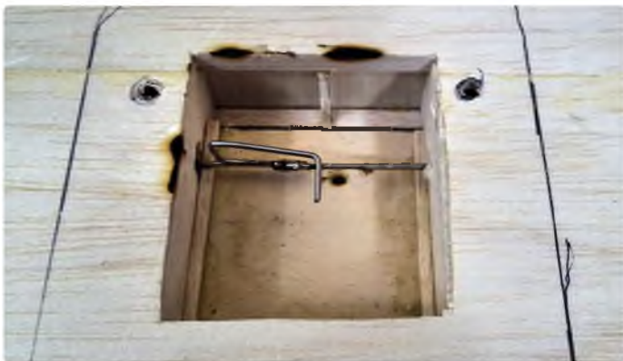
Aileron servo bay. Mount the servo with Radio Active servo mounting brackets
