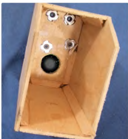
Inside of the tank box showing triangular stock and blind nuts
