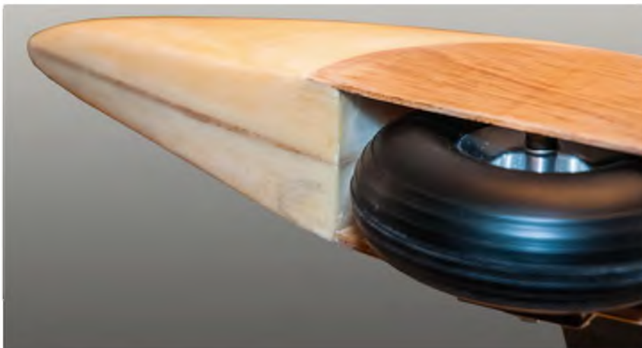
Spat construction method is evident here
