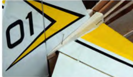
Glue the fin supports in place using the fin to position them accurately. Shape the supports once they are dry and cover them before finally fitting the fin
