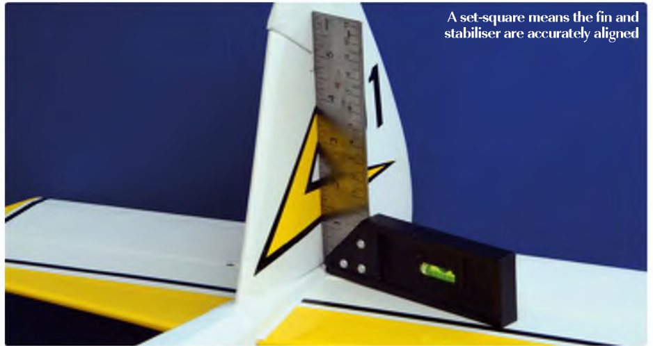
Glue the fin supports in place using the fin to position them accurately. Shape the supports once they are dry and cover them before finally fitting the fin
