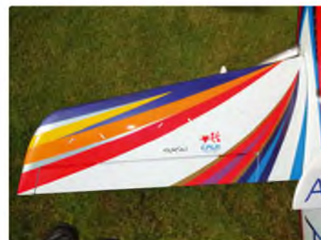
Turbulators on Shane's Wind helped in the windy conditions
