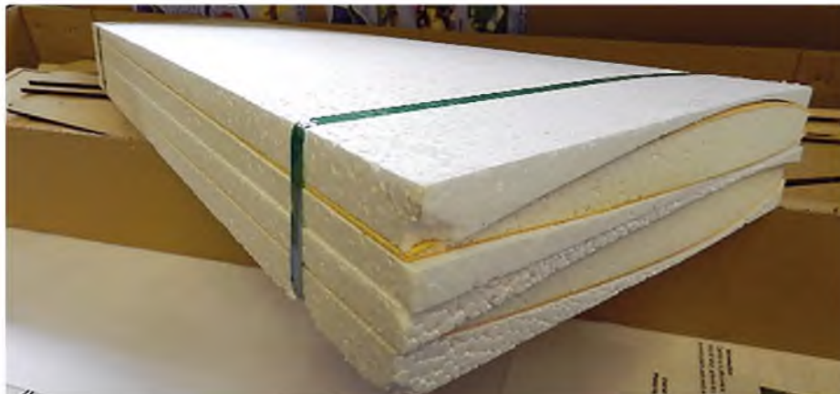
Remember these? It's nice to work on a set of veneered foam wings again
