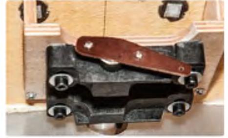
The nose leg mount/pivot uses a modified fibre-filled IC engine mount
