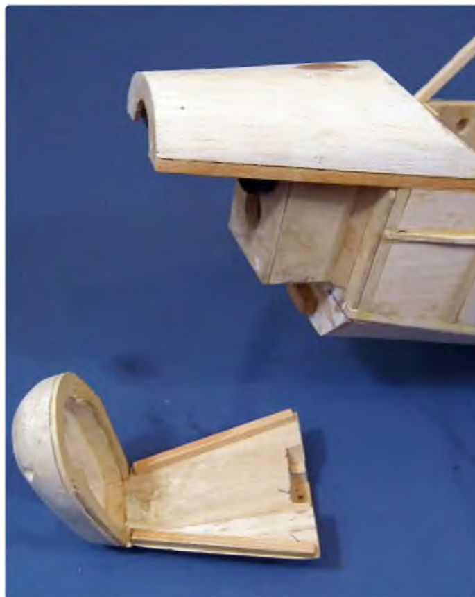
Lower part of the cowl glued together. This is screwed to the upper part
