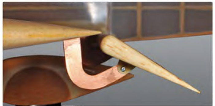
Flaperon hinge from epoxy printed circuit board
