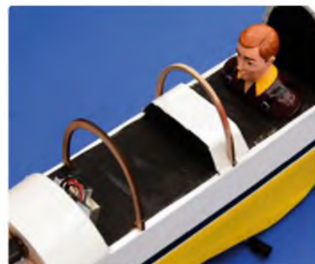
Two cockpit formers are provided in the kit but life will be easier if a third former is made up to support the acetate cockpit
