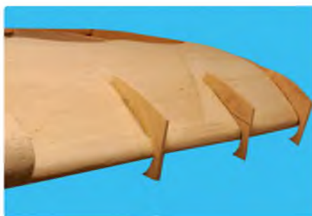
Inner slot skin with spacer ribs fixed in place
