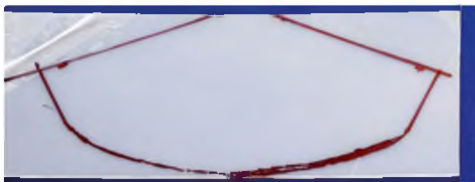
Covered acetate makes painting easy. Draw the front cockpit shape free-hand. Always over-estimate the size and trim back when trial fitting
