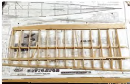
Building the wing outer panels is easy. The spar is lifted off the board by packing to keep it clear of bottom covering
