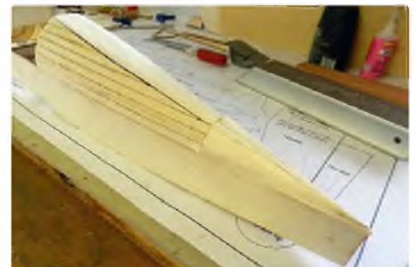
The temporary tail platform allows the tail fillets to be blended in perfectly
