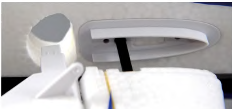
Tailplane halves push into cuffs moulded on each side of the horizontal stabiliser mount
