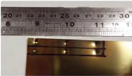
The undercarriage securing strips were marked out and holes marked with a centre punch before drilling and cutting out. Note the use of a marker pen, not a pencil
