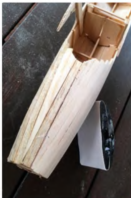
Sanding the planking. I would bevel the edges on assembly if doing it again
