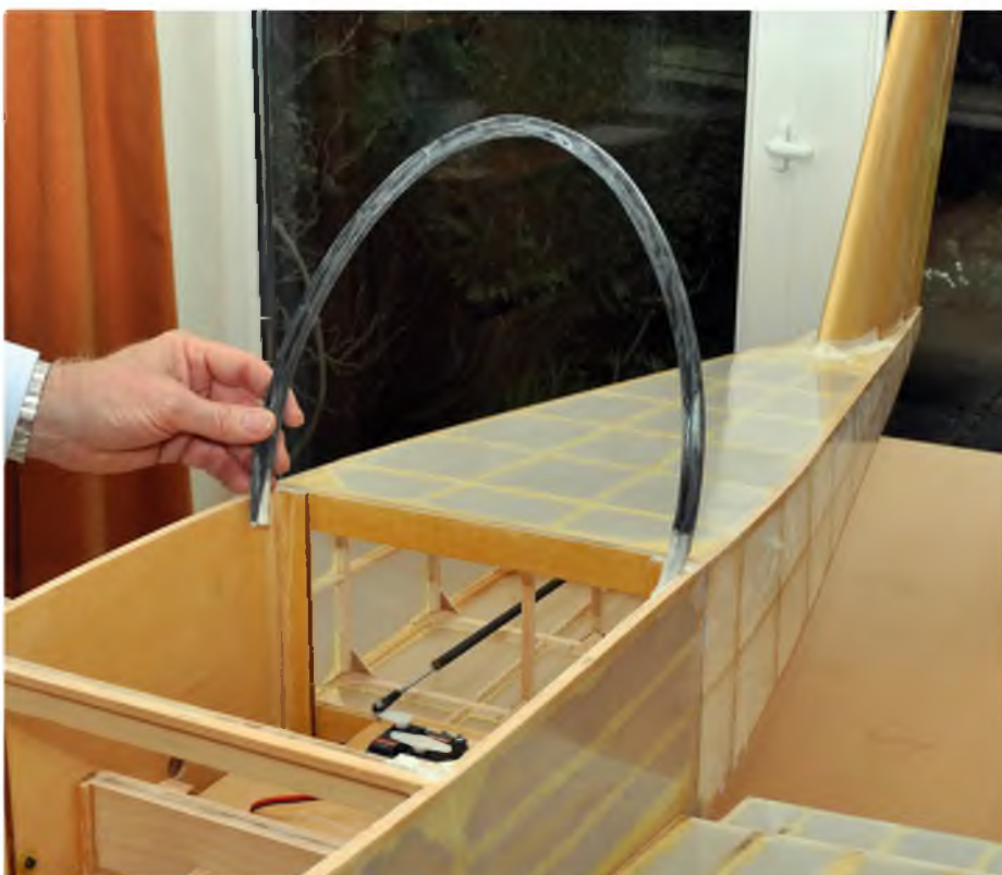
Checking a moulded canopy hoop for fit
