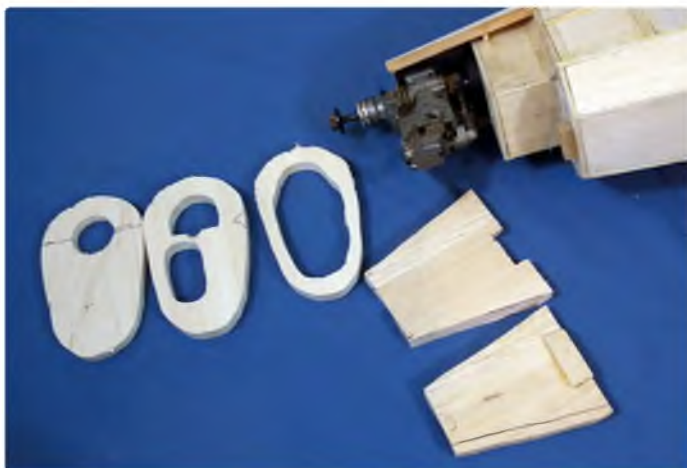
Balsa parts for the cowl roughed out
