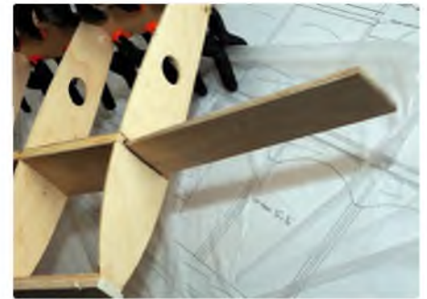
Wing joiner/dihedral brace in situ. Make sure it is well glued!
