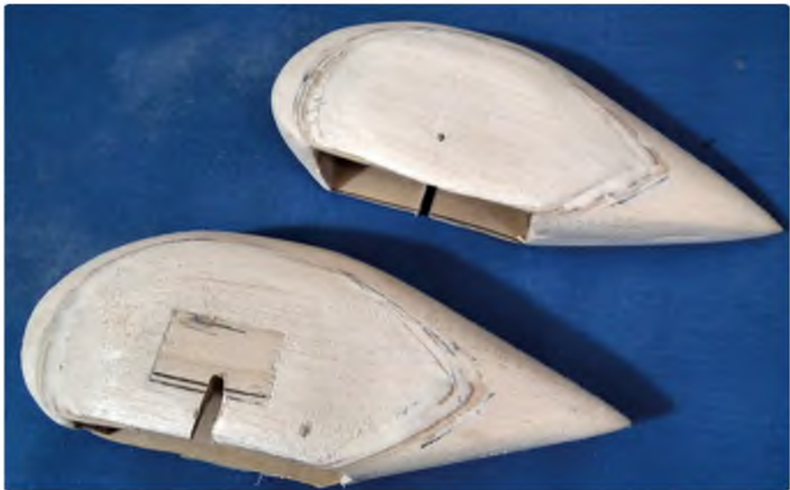
Spats ready to be drilled for the blind nuts. Note the slot on the inside and the hole on the outer face
