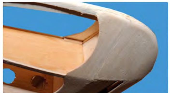
Open structure wingtip after sheeting
