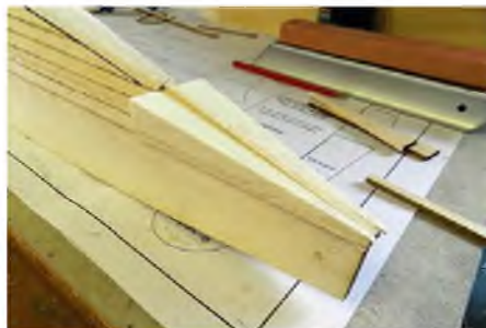
The temporary tail platform allows the tail fillets to be blended in perfectly
