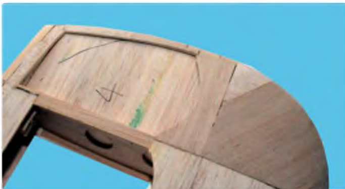
Sid's wingtip build method uses a central balsa core
