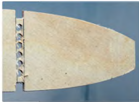
Holes drilled in the root rib to make cutting the slot for the dihedral brace easier later
