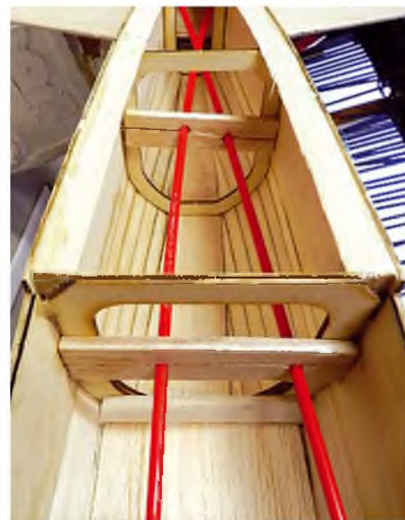
I opted for snake pushrods, supported about halfway along their length to prevent any bowing
