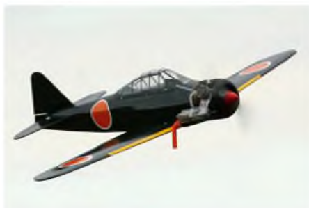
Subsequent test flights were made with the top cowling removed. At least the new engine was well cooled!
