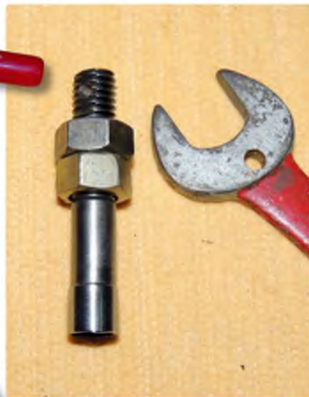
My custom socket tool machined from a high tensile socket head cap screw. Lock the nuts tightly together – use the bottom one for loosening and the top one for tightening
