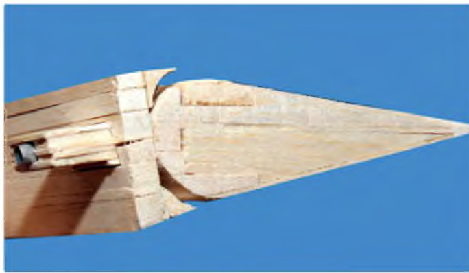
Aileron hinge point and spar with added balsa to form the curve
