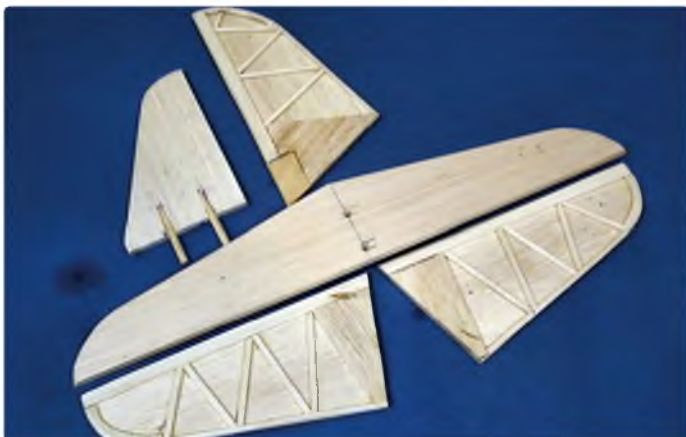
Simple tail components. Or you could just make the elevators and rudder from soft 1/4" sheet
