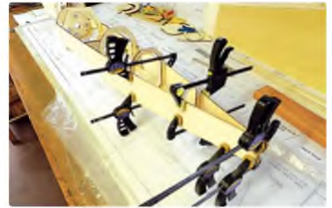
Clamping up the rear fuselage while the glue dries
