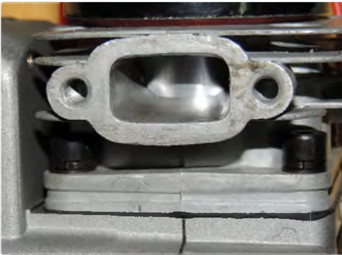
Look at the socket screw lurking in the shadow of the exhaust manifold. Sometimes it can be just damned difficult
