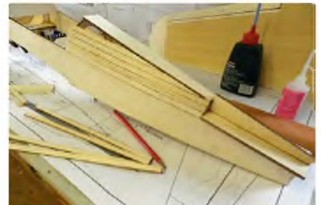
Planking the rear turtle deck. Note the temporary tail platform
