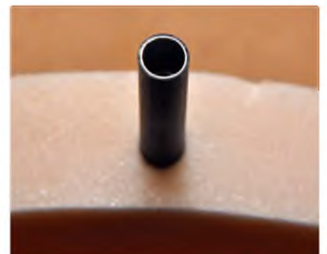
Arrow shaft pushrod material in cross section
