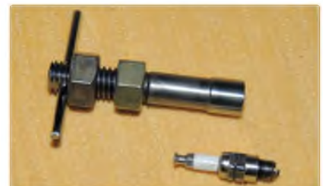
Some of these spark plugs are quite long so I drilled into the shank of the tool to allow a full-in fit
