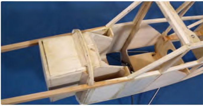
Detail at the front showing the scarf joint for the spruce strip
