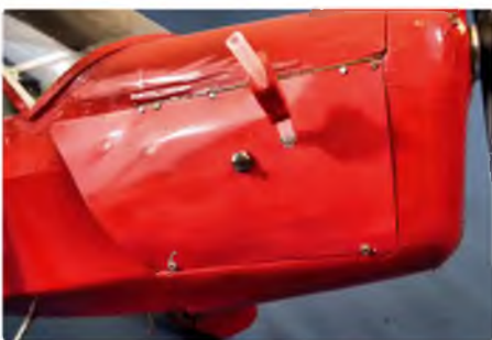
Right side of cowl showing fuel filler and remote glow connector
