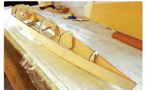
A nice, straight fuselage ready for decking
