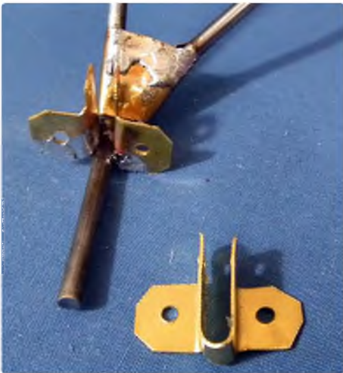
U/C leg joint and showing the bracket that holds the spat on and takes the bottom of the dummy shock strut. This must be soldered on securely
