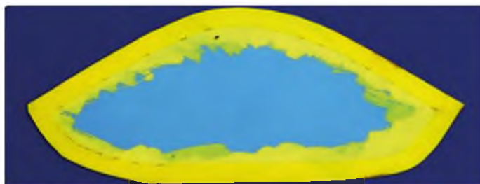
Covered acetate makes painting easy. Draw the front cockpit shape free-hand. Always over-estimate the size and trim back when trial fitting
