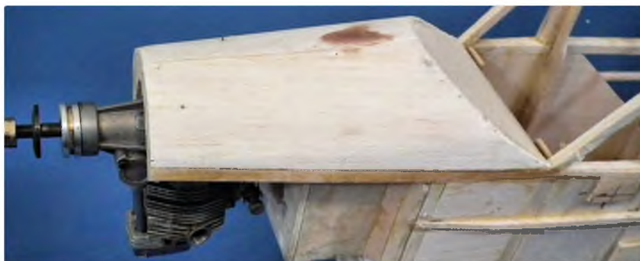
Top sheet fitted and engine temporarily installed
