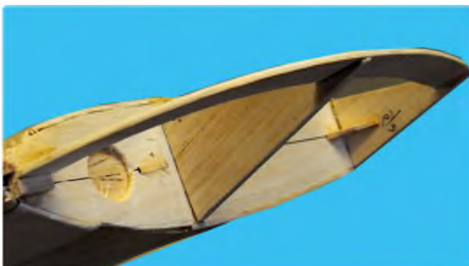
Open structure wingtip with single piece slotted ribs
