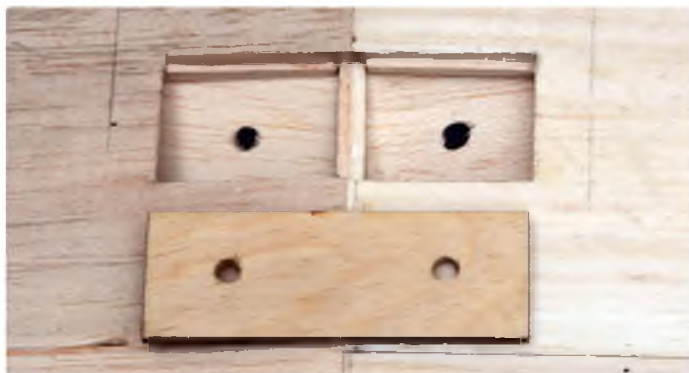
Nice seating arrangement for the wing bolt plate
