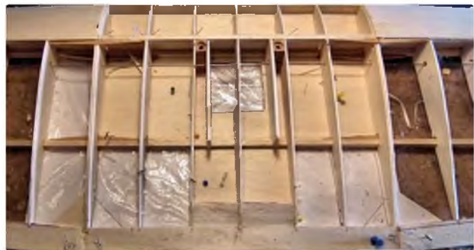
The centre section with the outer panels joined on. This shows the hardwood blocks for the front wing bolts
