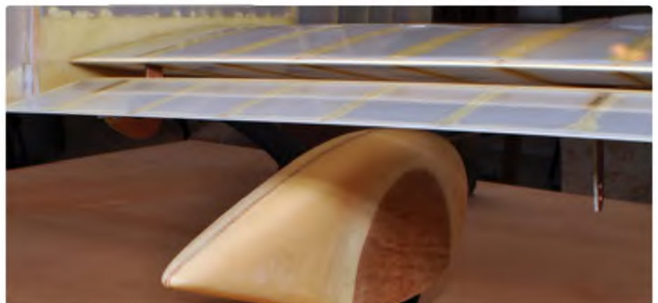
The 'Junkers' style slotted flaperon
