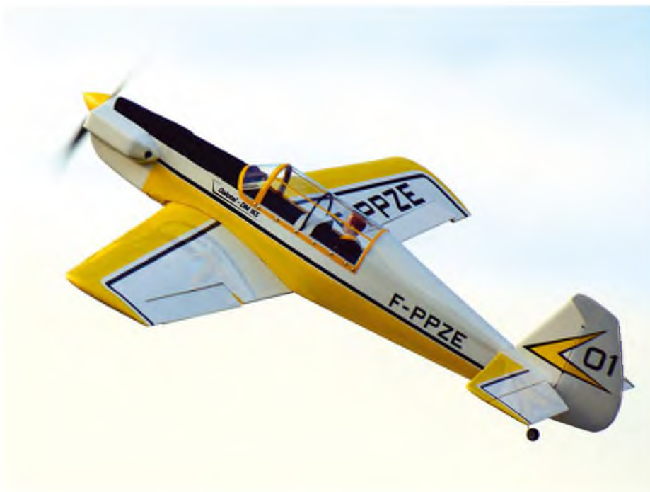
Safely away on the first flight but it needs a bit of trimming and aileron differential
