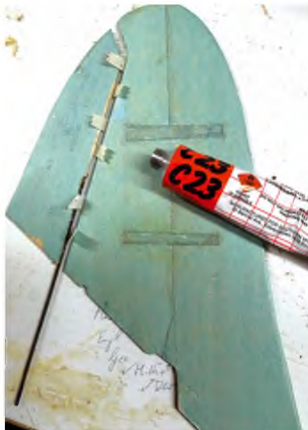
Old fashioned cloth strip hinges on the rudder. Note the balsa strips let into the rudder sheet to counter warping
