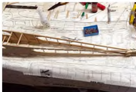
Make sure the fuselage is straight!
