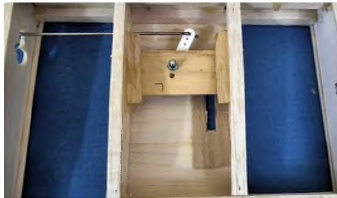
Aileron bellcrank bay. The aileron pushrod can be fitted after covering
