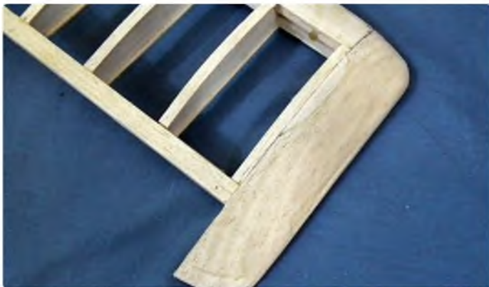
Wingtip carved from block, or two layers of 1/2" sheet plus a little scrap wood
