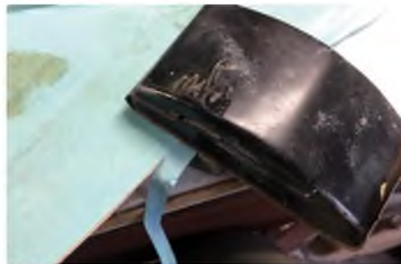
Doped tissue is easily trimmed with a light touch of the sanding block
