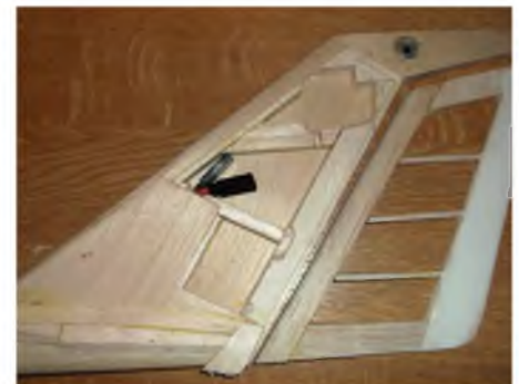
Building the fin and showing the servo locations
