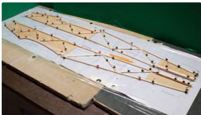
A good way to avoid making two of the same fuselage side is by laying out both sides at the same time, top to top
