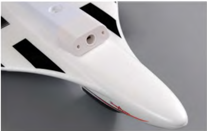
Besides acting as a central landing skid, the bottom cover also houses the optional FPV camera
