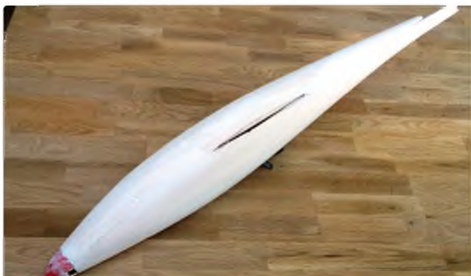
The fuselage is shaped as one piece, ready for cutting out the hatches and the installation of the fin
