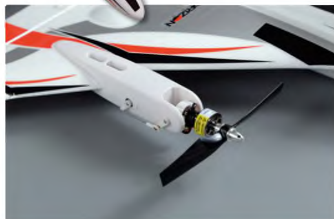
Same motor facing forward for aeroplane flight
