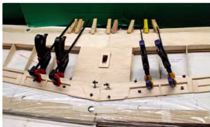
Groove the centre-section TE for the aileron torque rods, then glue it onto the rear spar
