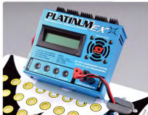
A metal bracket is provided that slots into the vent holes and which can be used to support a small charger
