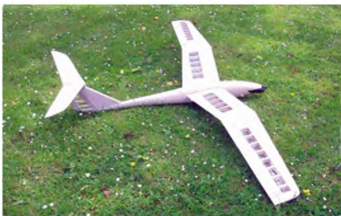
Completed T-Bird airframe, ready for covering
