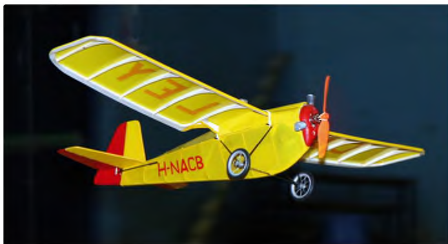
My Carley Racer rubber power conversion was kept really light by not covering the undersides of the wing
