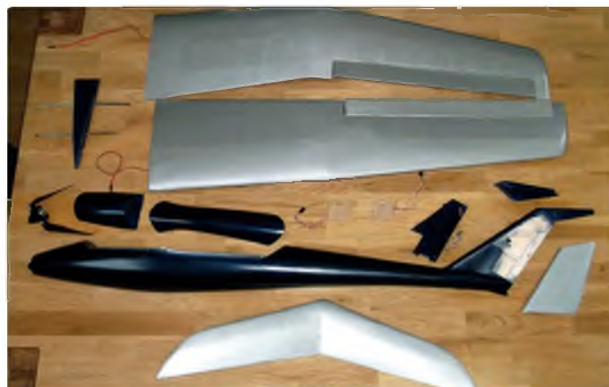
All the components finished and ready for radio installation
