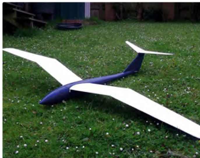
T-Bird's predecessor, a gull wing T-tail design that I named 'Chuff' after the famous Cornish seabird
