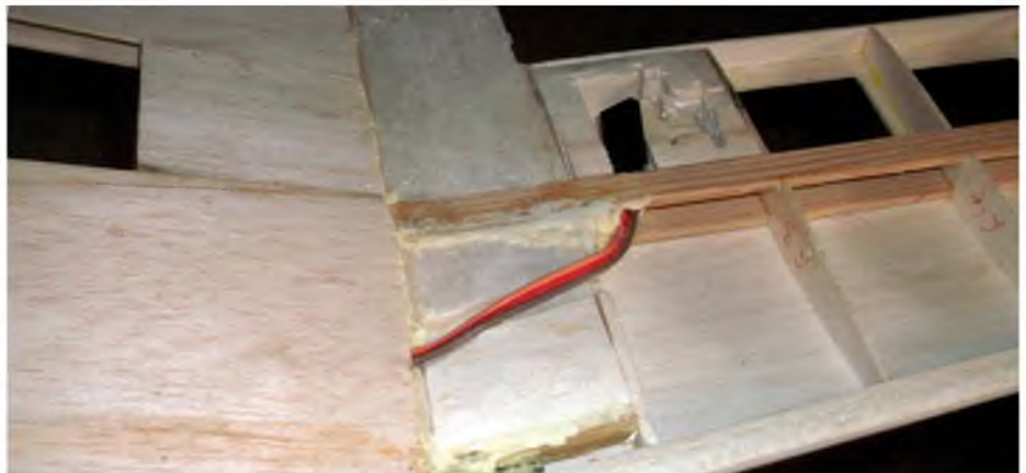
Joining an inner and outer panel
