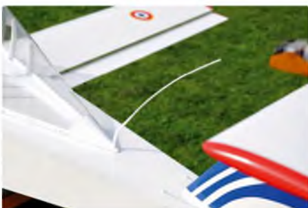
Scale aerial from bits of soldered brass and plastic tube
