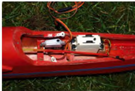
The nose area on old soarers was nothing like as constricted as today. A 'standard servo' of the time takes up the space of at least two modern 'wing servos', which have much more power and metal gears to deliver it!
