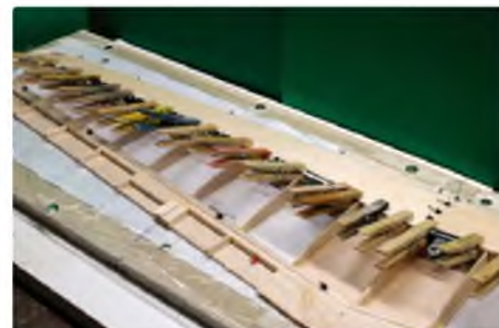
Moisten the sheet's outside, run a bead of slow-drying glue along the top of the ribs and the top spar, then bend the sheet down over it. Do one side, then the other and cut through both along the centre line. Remove the excess wood, then clamp the sheet down to dry thoroughly
