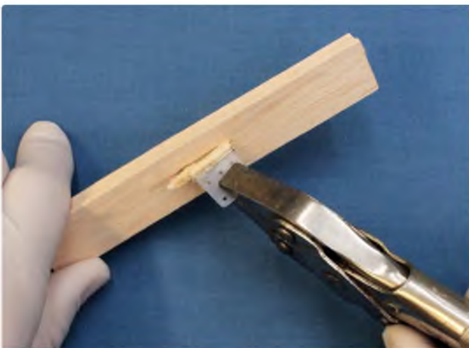
Super 'Phatic! glue has an affinity to foam and plastics, making it ideal for gluing hinges
