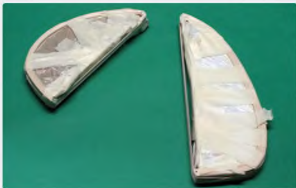
Left: Criss-cross the corrugations to stiffen the lamination forms, then wrap with plastic sandwich wrap. Shown are wingtip and rudder forms
