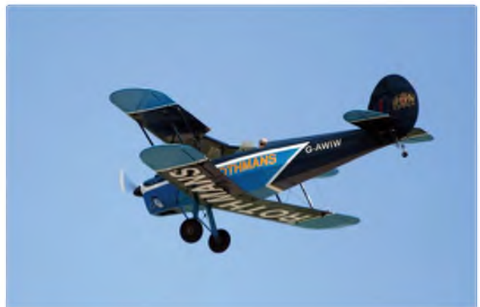
Right: Martin Stirling is a skilled flyer who always turns in a good performance with his models. His Stampe is built from the Precedent kit: 1/4 scale, weight 10.5 pounds, ASP 1.20 FS
