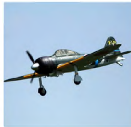
Jeremy Wilkinson's A6M Zero has a span of 55 inches, features split flaps and uses a 38 mm brushless motor, plus a 4S 3.2 Ah LiPo
