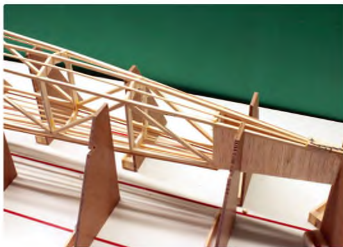
Fuselage underside longerons. The tail wheel strut is sewn to ply plate with Kevlar fishing line and thin CA. Note that the aft side sheet is fitted between the longerons and the grain is vertical
