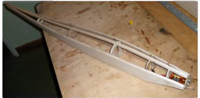
Adding the lower longeron. Note that the motor is fixed in place from this point
