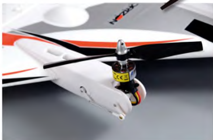
Front motor in its raised multirotor position
