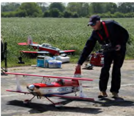
2016 was Gordon Hill's first season in the WSL. His Great Planes Ultimate Bipe is 65" span, weighs 16 pounds and is powered by a DLE 55 with an EME electric autostart
