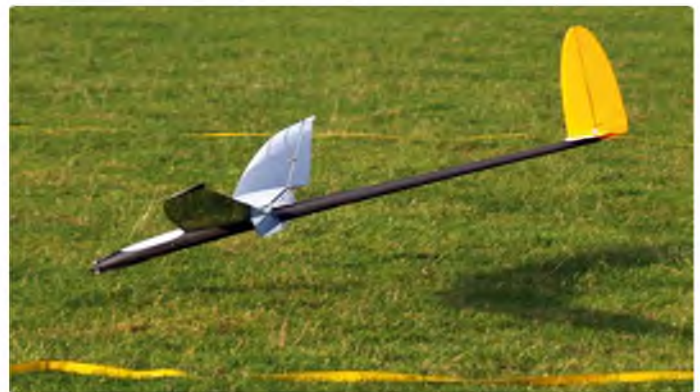
For those who wonder how much flap is used for accurate landings, this shot should answer the question – a lot! You can just about make out that there is quite a bit of down elevator compensation there as well. Despite being well nose down, forward speed is low
