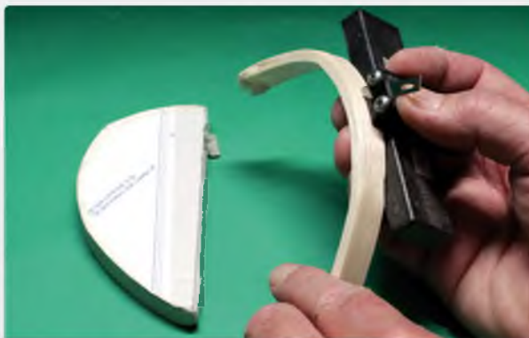
Right: Making both wingtips at once, then separating them with a balsa stripper is an easy way to ensure they match
