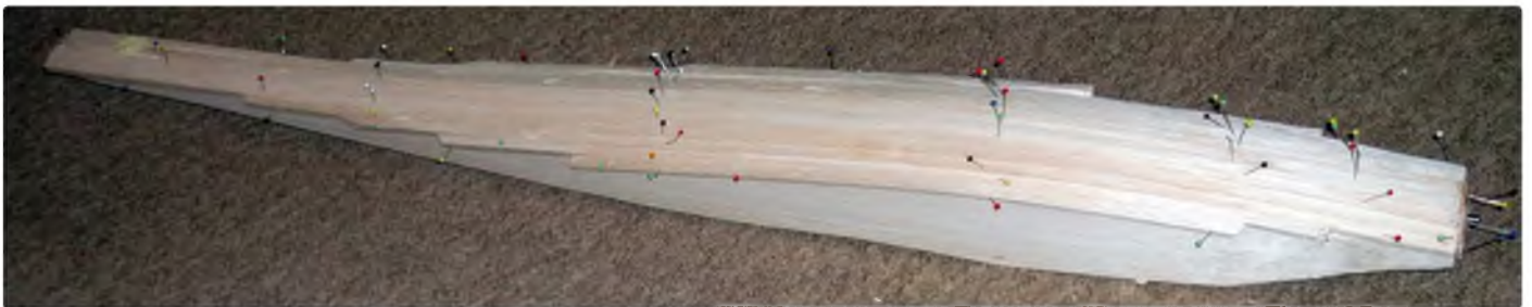
Attaching the underside planking
