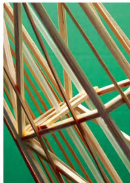
Notched balsa strips hold the plastic pushrod tubes at F7, F8 and F9, ensuring that the pushrods won't bend – even under those panic pull-outs!
