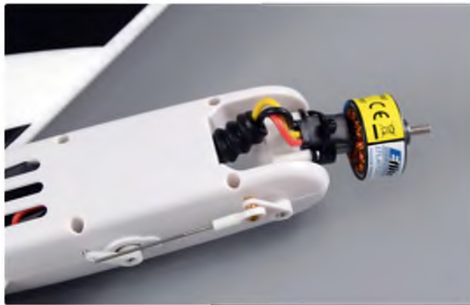
Flexible gaiters support the motor wires when bending backwards and forwards during transitions
