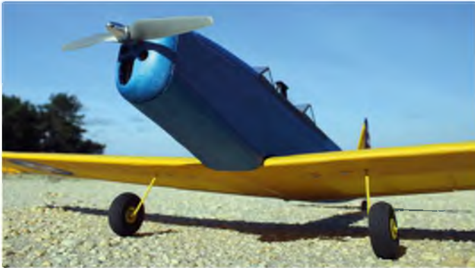
Lightly glue the nose bowl in place after covering but leave a seam so it can be removed for motor servicing or adjusting the down and side thrust
