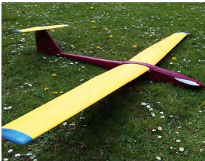
Zephyr 2 with plastic Correx inner fuselage
