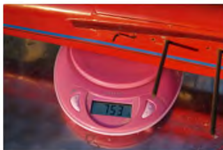
Fuselage and nose weight total 753 g. A modern electric soarer fuselage with all its equipment can achieve a total of 600 g reasonably easily
