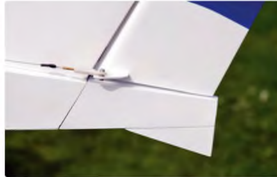
The removable tail end is necessary to fit the rudder
