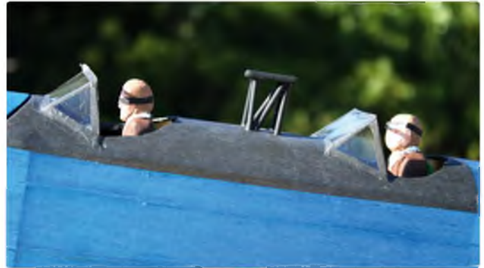
Overturn pylon is made from scrap plastic tubing and bass bits, whilst the pilots are carved and painted blue foam. Weight is virtually nil but somebody's got to be in the cockpits!
