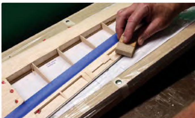
Sand the TE and ailerons to a smooth taper using a strip of masking tape to protect the rear spar and 1/8" music wire to set the TE thickness
