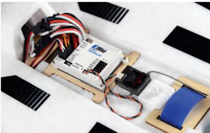
View of the serial receiver and flight controller. A standard 6-channel Rx can be used if you buy the PNP version instead
