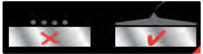
Fig. 4 – For adhesives to work well they have to spread and wet the surface. If the adhesive beads up it has a greater affinity for itself rather than the surface to which it is being bonded
