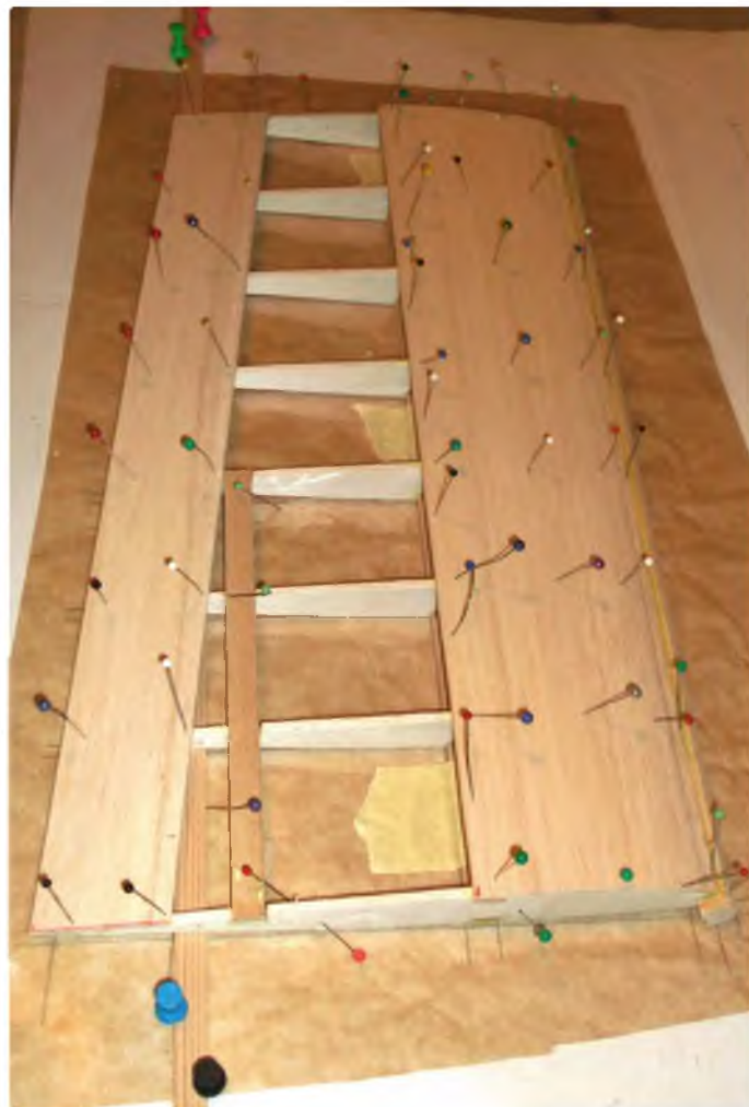
Making an inner wing panel frame
