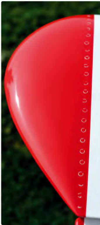
Lightweight balsa wingtips, with more (flush this time) rivets!
