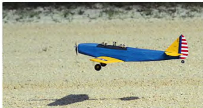
Wide landing gear stance helps with smooth landings, even on our rough, gravelly runway
