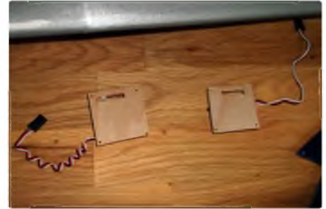
Wing servos are attached to ply plates
