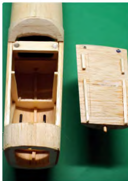
Scrap balsa block hatch has 1/8" square alignment guides on the bottom and a 1/8" dowel retaining pin in front. Magnets at the rear latch onto two flat-headed screws. If the hatch won't 'click' satisfactorily replace one (or both) screws with more magnets
