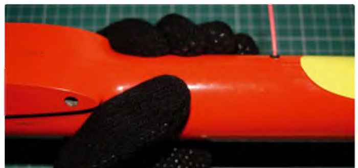
The general tendency is to launch any model from the C of G for good balance, but slim gliders can be very difficult to handle in turbulence. Holding ahead of the wing, where possible, gives more to grip and keeps the nose down
