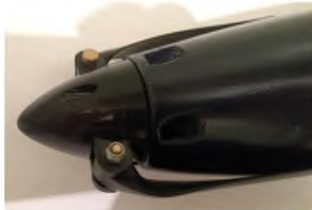
Cooling holes for the motor
