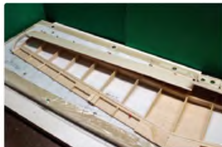
When sheeting the wing LE glue the sheet to the LE first and let it dry
