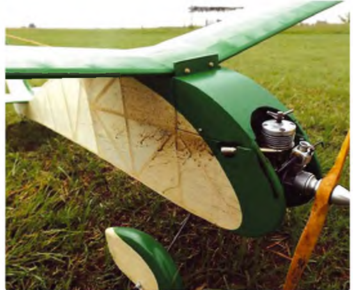
The business end of the Super Murgatroid, showing off its Webra 2.5 cc diesel. Your author fondly remembers being in awe of the power of this engine during his earliest club days!
