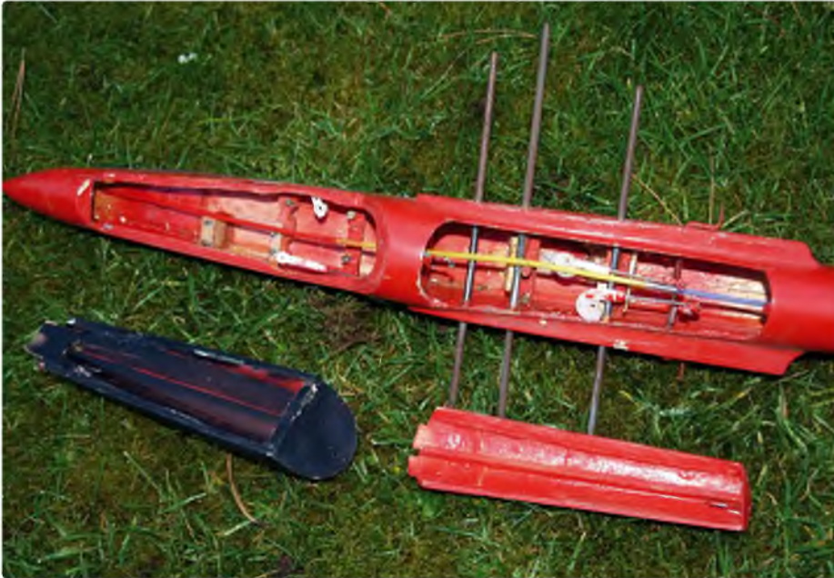
Left: Look back in amazement. Were models this large and did they really contain so many wire bits? Yes! This old tow line glider recently surfaced and shows just how far some things have reduced in size and complexity over time. Note the three round wing dowels used, at a time when two were the norm. Also the large hatches to give access to the big servo/flaperon connections and for adding ballast
