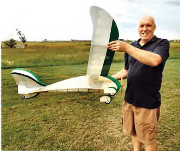
Chris looks very pleased with his Super Murgatroid, which flew 'off the board'. In keeping with its status as a modern vintage style model it features a suitably mixed-media finish, incorporating doped silk, iron-on film and paint trim
