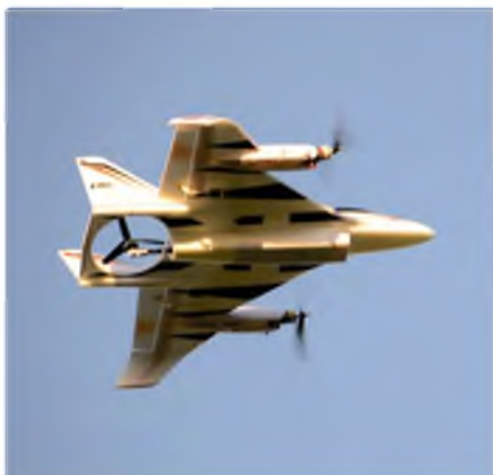
Entering the transition. The tail fan is still static as the main rotors start to lift
