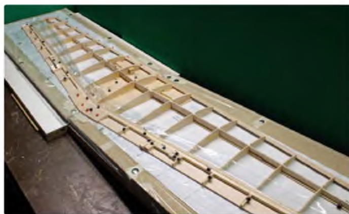
...Or the whole wing can be built in one process, using a hinged building board
