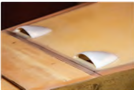
Plastic spoons make excellent air scoops to cool the ESCs
