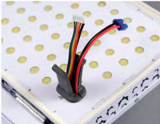
Charge and balance leads sandwiched between the two halves of the wireway bung. Keep your hands clear of the filter when pulling it through – those holes would make a good cheese grater!
