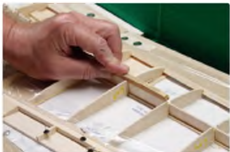
Sandpaper glued to a scrap of old spar material of the same width makes a handy tool to ensure the shear webs are level and the spar slots line up
