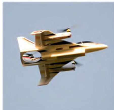
With all three motors now running and supporting the weight of the aircraft, Convergence settles into a high hover. That was easy!
