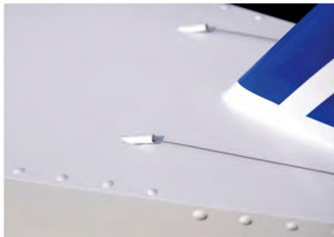
Close loop exit guides – and rivets!
