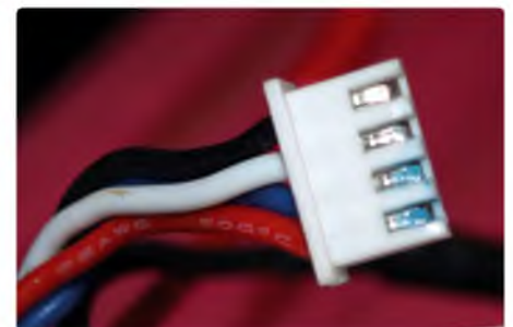
I noticed this corrosion starting on a LiPo balance lead the other day. It had not yet progressed to the inner part of the plug where the actual electrical contact is made and was quickly cleaned off, but clearly this is another area which needs monitoring on our models
