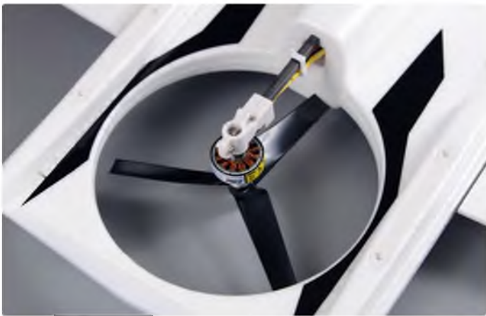
The rear fan is mounted on a fixed carbon boom
