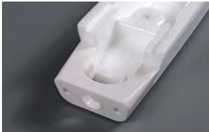
Wingtip detail, shown inverted. Plastic covers protect the tips when the model is sitting on the ground
