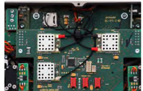
The three separate transmitters are shown here. There are two 2.4 GHz transmitters, each with twin aerials for diversity, and a single 900 MHz transmitter
