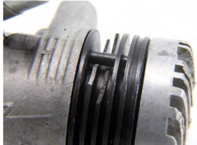
Above: This is a combination of a cast iron liner with integral barrel fins. Can you see a problem here?
