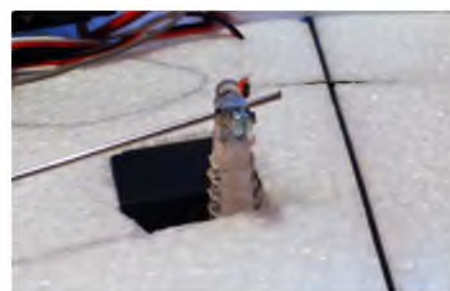
Clear plastic extensions, bound to the servo arms, are used to increase control throw movements
