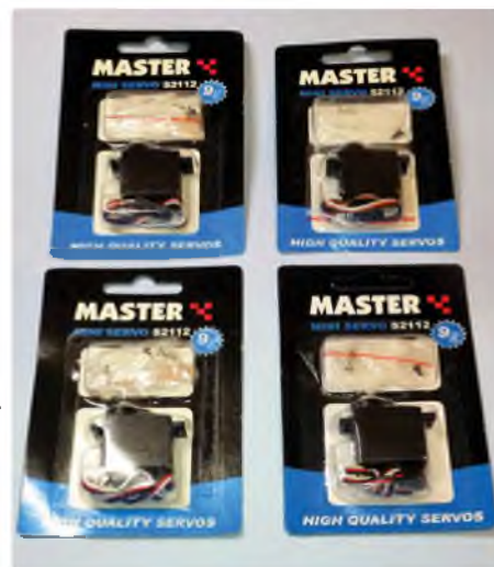
Right: Four off Master S2112 9 g servos were used for the review model and have proven very reliable
