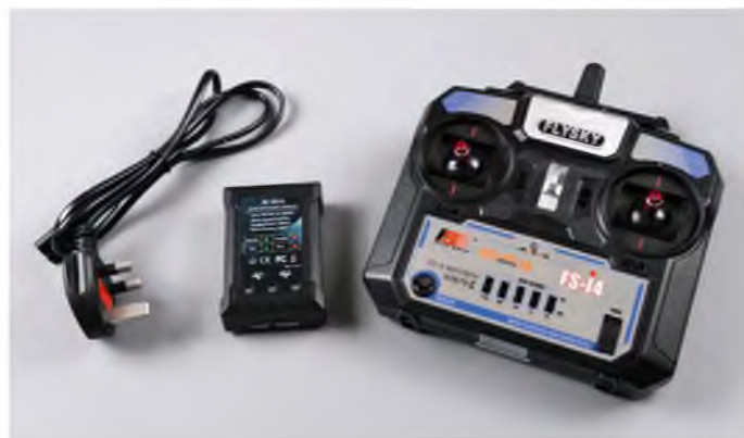
Super EZ comes with a mains powered LiPo charger and a FlySky FS-i4 radio system. The servo reversing and V-tail mix switches are best taped over once you have set up your aeroplane
