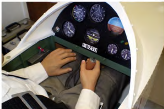
The instruments are properly spaced, with the glazing and instrument pointers made as separate items. The bezels were made from bits of plastic tube
