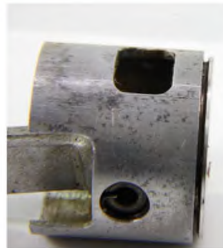
First is the ring groove, right at the top of the piston. Then the thin crown section is considerably smaller in diameter to allow the combustion gas to expand the ring from the inside
