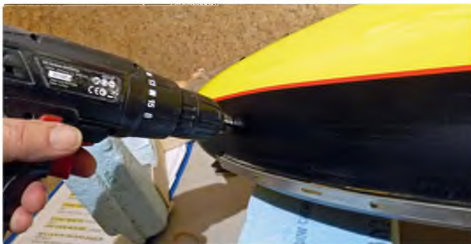
Using a cone cutter to retro-fit the Smallpiece release
