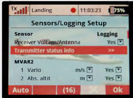
The DC-24 has extensive user configurable data logging capabilities to log both telemetry and transmitter control position data
