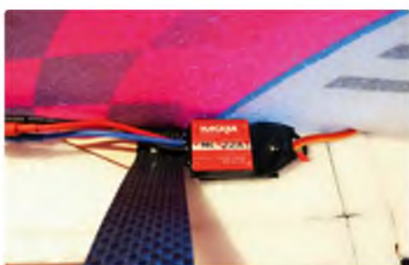
Hacker's MC 22 A ESC is mounted via hoop and loop tape on the underside of the fuselage
