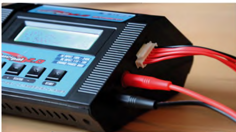
The balance board and charge leads connect to the side of the unit
