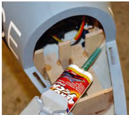
AeroT<ch is ideal for bonding formers into glass composite fuselages
