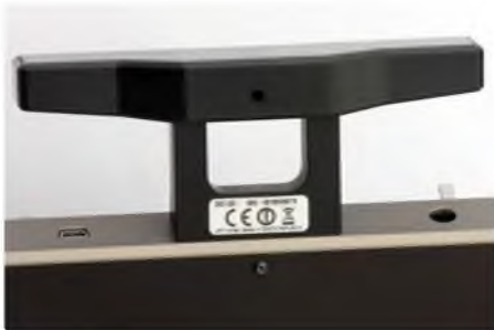
The carry handle houses the 2.4 GHz and 900 MHz aerials. The socket in the handle is for a PPM stream for use with flight simulators and also external devices, e.g. FPV head trackers. The ports on top of the transmitter are for the charger and a USB port for hooking up to your PC
