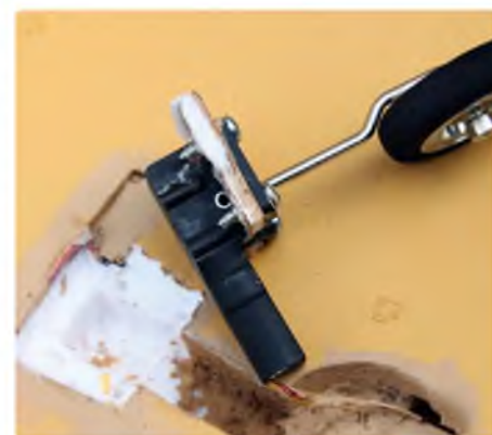
Without strengthening, the mounting block can quite easily pull out but is easily repaired
