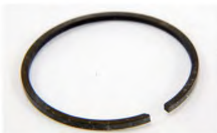
A standard design cast iron ring used on almost all ringed engines. The section is generally rectangular (there is a formula for the sizing) but they are occasionally square in section. The ring is expanded and heat treated to give it the 'spring out' effect
