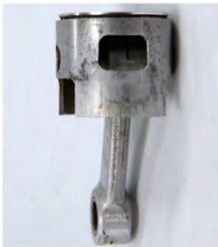
Now we have a piston from an engine that employs a Dykes ring and there are several differences to consider
