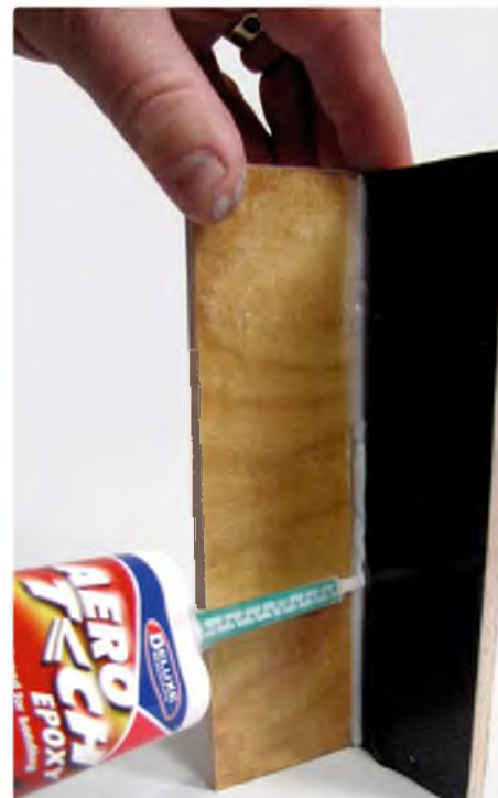
AeroT<ch forms a visible bond so you can see where the glue is
