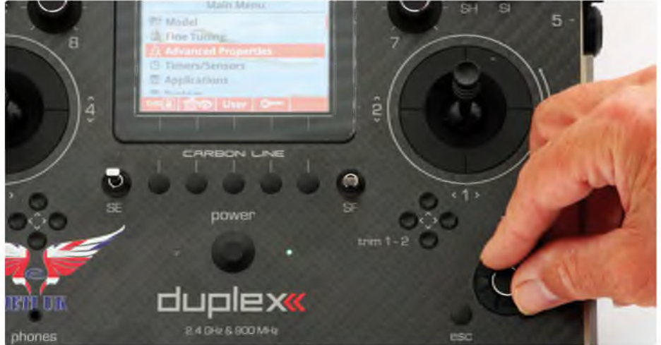
Programming is by the buttons and the 3D wheel on the lower right of the transmitter
