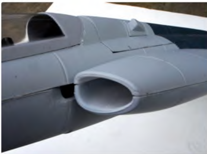
These small intakes were fine for an Avon but not for an EDF unit!
