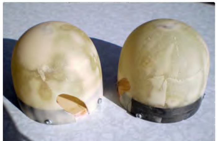
The spinners were easy to make using ply back plates and the 'lost foam' method. The carbon/glass shells weigh next to nothing
