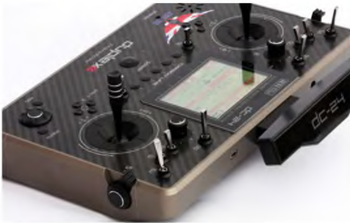
The main case is machined from lightweight alloy. The sticks fall easily to hand for pinch flyers, while shorter sticks are available for thumb flyers
