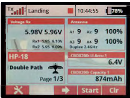
Main model screen is user configured. Here the primary display has been set to show the supply voltage and signal quality at each of the RSat aeriels. Note the screen background colour and model image can also be changed. Model images can be loaded from your PC via the USB interface
