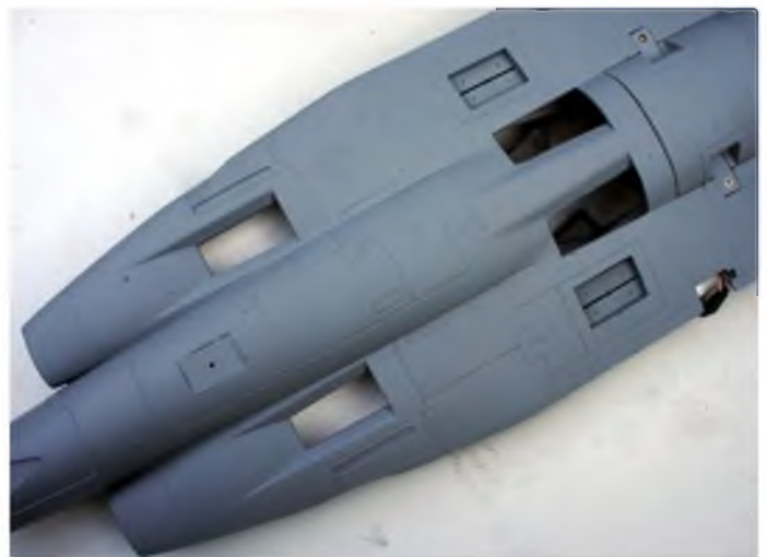
Four auxiliary air intakes form 'cheater holes' in the underside of the fuselage; there are four more holes on top of the fuselage! The rear cheater holes are convenient for fitting retracts
