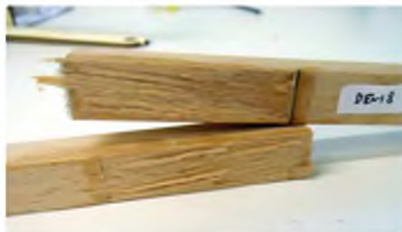
The adhesive's properties are assessed using hardwood test pieces
