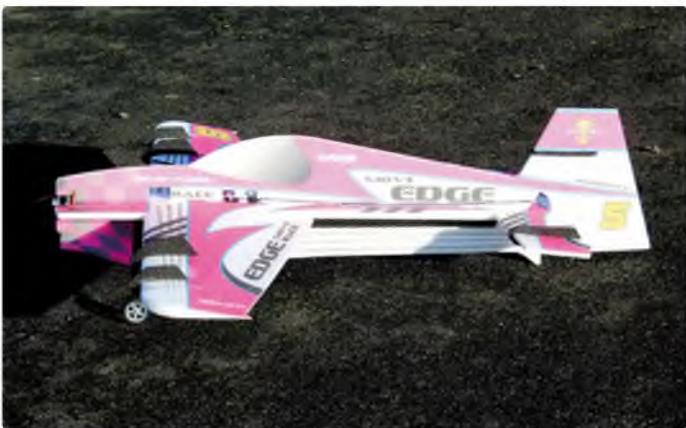
Starboard side, showing how long the control rods are for the rudder (and elevator). However, there is no 'slop', with the model flying very accurately
