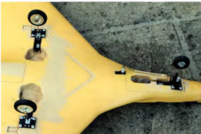
On the JetTiger the main U/C units fitted in very easily, but the nose unit had to be fitted in a potentially weak area
