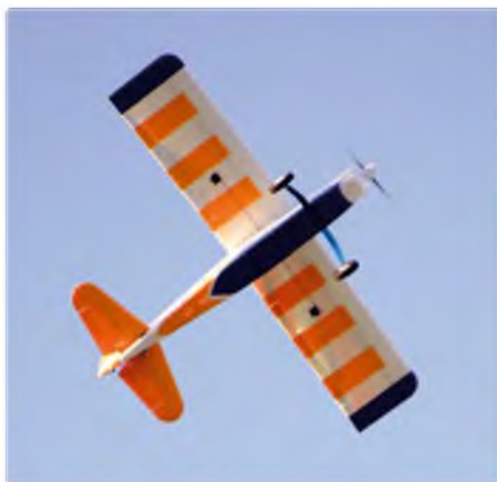
Yellow bands on the undersides of the wing are good aids for orientation
