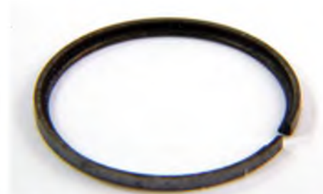
Also cast iron, the Dykes ring has a L shaped section and it a rather loose fit on the piston. It is commonly left 'green', i.e. not heat treated, but that depends on the manufacturer
