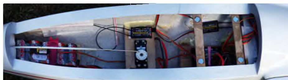
A quarter scale Pat Teakle glider was one of the models used to test fly the DC-24. Here the Central Box 200 was used with two 2.4 GHz Rsats, the RC switch and a vario sensor
