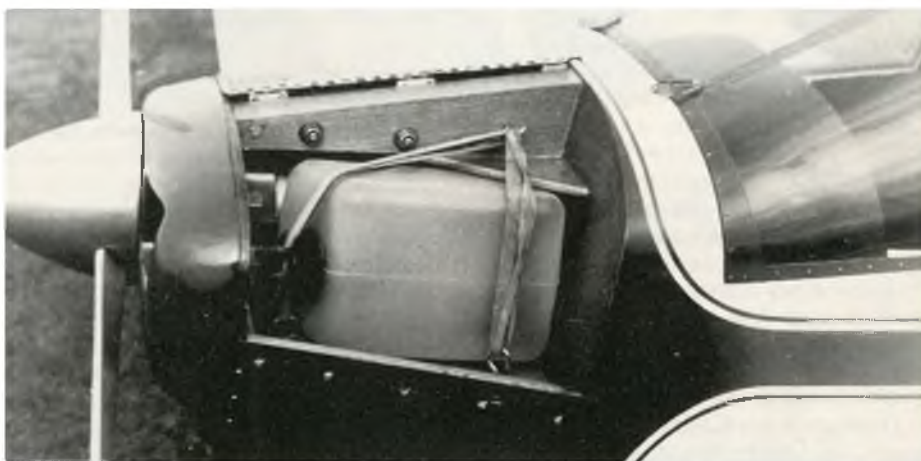
Centre hinged 'bonnet' provides easy access to the fuel tank. Apologies for the high contrast of the black and white pictures, which have been scanned from the original magazine article
