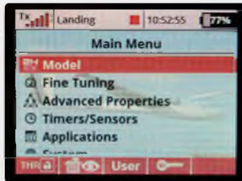
Programming is entered via the menu button, which takes you to the various menu options. Scroll down to the relevant option and the relevant sub-menus can then be accessed
