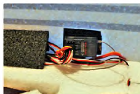
My four channel receiver is secured with hook and loop tape. The black EPP fuselage strengthening former is ideal to hide servo leads behind for a neater fit
