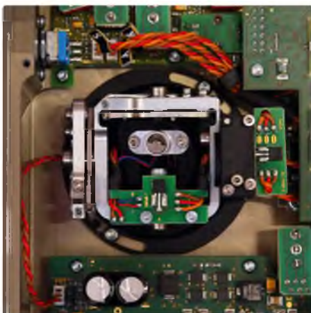
Stick gimbals with hall effect position sensors are CNC machined and adjustable for spring tension and ratchet. They can also be rotated to follow your natural hand movements. Note the haptic vibration units at the base of the stick
