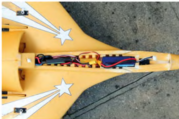
Not a lot of room! A 3S 1500 LiPo could just be squeezed in
