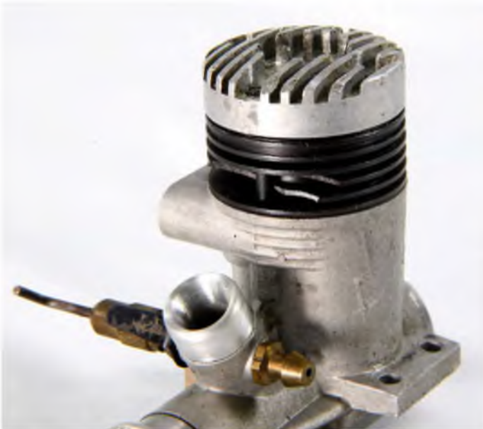
Above: This is a combination of a cast iron liner with integral barrel fins. Can you see a problem here?
