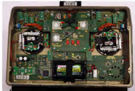
Removing the rear cover reveals a well thought out design. All boards plug into each other and the switches plug directly into the boards also. The only interconnecting cables are from the gimbals
