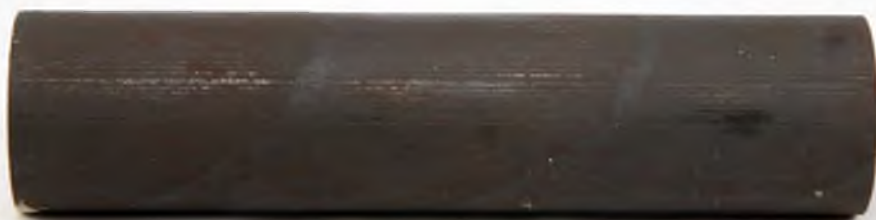
Centrifugally cast iron (Meehanite) is ideal for piston rings, pistons and liners. Note the spiral marks indicating the rotation while being formed
