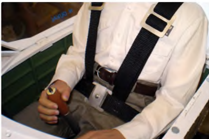
'Hugues' needed a belt to keep his trousers up, a joystick to hold and a seat harness made using haberdashers webbing. The fittings were made from thin alloy sheet
