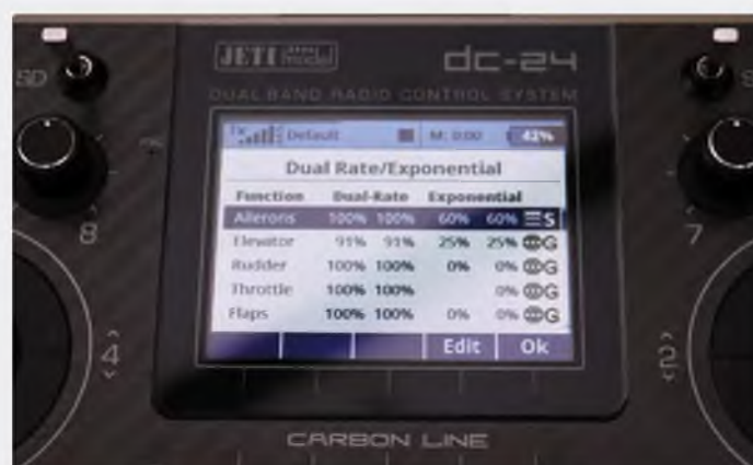
Dual rate and exponential values are listed. The ailerons are flight mode specific and the rest are global. Highlighting and entering a control brings up that control's editing menu
