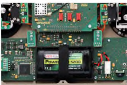
Power is provided by a 2S 5200 mAh Li-ion battery. Battery life is around 12 hours, which is more than adequate for a day's flying. A charged spare could be carried as a back-up for weekends away when without access to charging facilities
