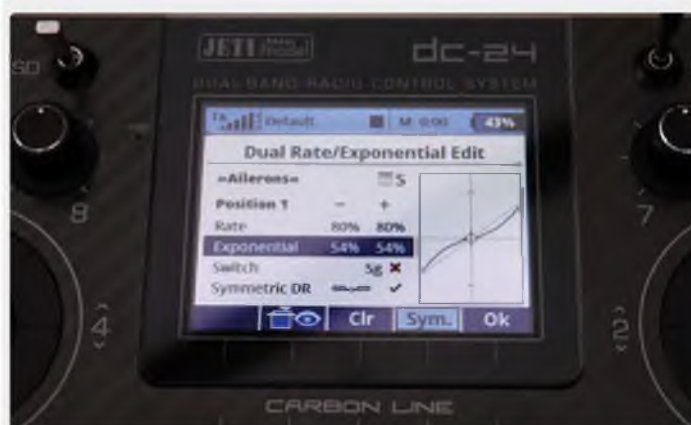
Dual Rate and Exponential can be set for each flight mode and are shown graphically. If you have dual servos you can set separate rates and exponential for each surface
