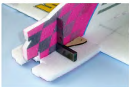
Using a small 'right angle' square to ensure that the fuselage is a perfect 90 degrees to the motor mount and wing
