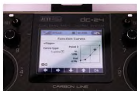
Left: Function curves can be assigned to all controls. These can be a constant value, 3, 5, 7 or 9 point curves or one of six predefined types. They can be made global or flight mode specific
