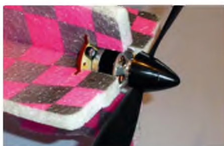
Hacker 'M' Force A2826CA-15 brushless motor is secured to a ply motor mount via screws. No downthrust or sidethrust is used
