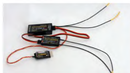
Standard R series receivers can utilise either a second 2.4 GHz or 900 MHz Rsat. Here a R9 receiver is shown with a 2.4 GHz RSat and a 6S LiPo voltage monitor sensor
