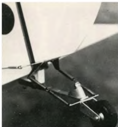
Closed loop system to the rudder and the nicely constructed sprung tail wheel assembly
