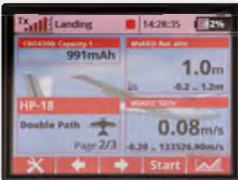
Using the function buttons underneath the screen you can scroll between the different, user configurable telemetry screens. Here the second of three screens shows the output of the vario sensor and also the receiver battery mAh consumed
