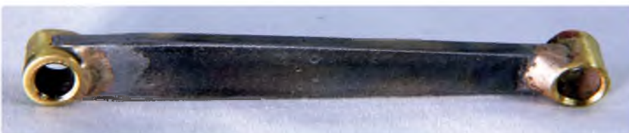
Here it is – the connecting rod to end all 'rod' designs! These were very easily fabricated conrods; the two eyes (big and little ends) were silver brazed onto a steel shank. There is still a lot of merit in this design and we will look into it further down the line
