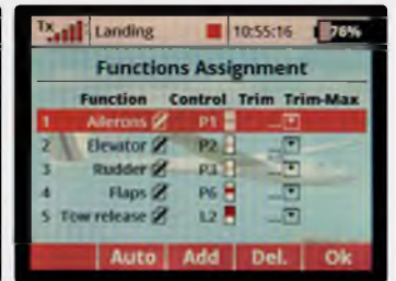
The functions assignment menu allows the controls/switches for various functions to be selected. Apart from the basic functions the other functions are named by the user
