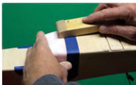
Protect the fuselage with strips of masking tape and pin or tack glue the balsa or foam exhaust blank in place. It's okay to rough shape the foam with a razor saw or very sharp knife but leave fine shaping and finishing to sandpaper. This is the original, stepped aft fuselage – see the next picture for the updated version with belly strake
