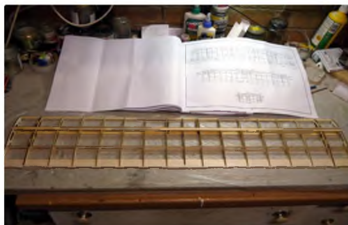
All parts are self-jigging so no plan is needed. The photo assembly instructions in the manual include drawings that identify all parts
