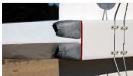
Above left & right: Once the outer surfaces of the dummy exhausts are roughed out, hollow with a hand grinder and sanding bits. Don't use Warp 9 speed, lest the foam disappears! Fine sand the finished foam, then coat it with water based balsa filler and sand with very fine (400 or better) grit sandpaper or sanding sponges. Finish with foam safe paints
