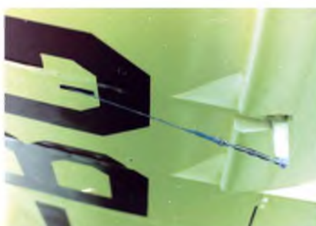
Aileron horn and cable, kept taut using a tumbuckle
