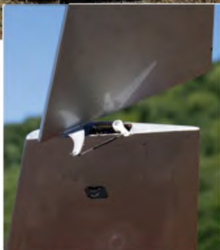
Right: The Archaeopteryx has a 2.5 gram servo driving each wingtip evelon. The object seen a few inches below the servo is a cut out for installing the wingtip evelon pivot
