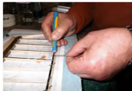
The rib caps go right over the trailing edge to form a very strong joint and are cut to length as each one is fitted. I'm sure I would need rubber gloves for this!
