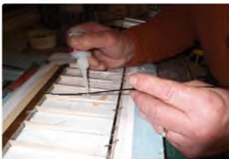
The final straight. Carbon capping is applied to the top of the ribs, joining them to the 'D' box top (this is actually the tailplane) before the wing is removed and reversed for the installation of the bottom caps
