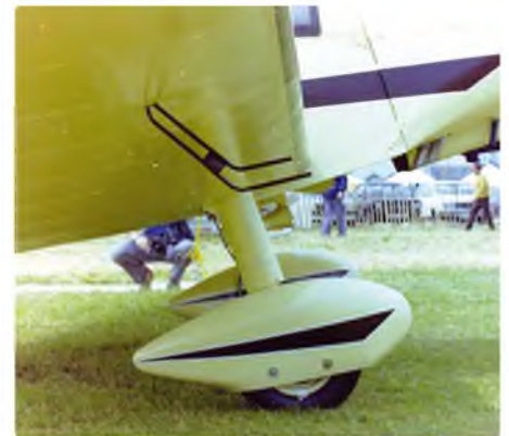
Leg fairings and spats, and pitot tube location
