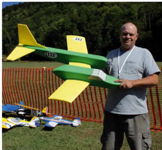
Above & below: John McGrath scaled up Terry Dunn's Parallax (May, 2014 Model Aviation) and extended the tail for smoother flight. John's version, spanning 42.5" and weighing 33.5 oz, boasts a fuselage of pink insulation foam and a Depron wing with carbon fibre spars
