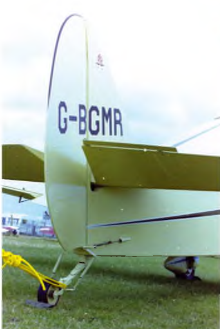
Rudder and tailwheel detail. Note how the elevator is locked fully up when parked
