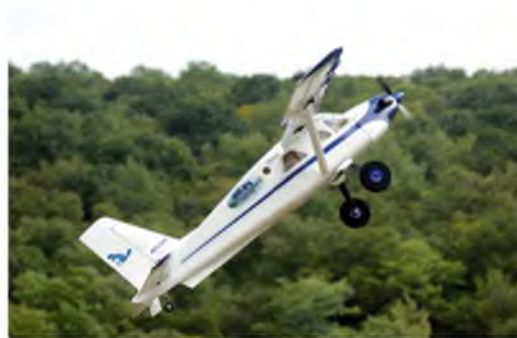
Right: Alan Mostek's Turbo Bushmaster in the alternative colour scheme. Loosely based on the DHC Turbo Beaver, their lightweight structure, large control surfaces, aerodynamic tweaks, and gobs of power give them excellent 3D acrobatic performance
