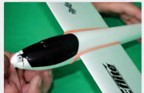
...Brian then wrapped a small elastic band around the aft fuselage, reinstalled the wing, and snapped the band around the forward fuselage (a heavier-than-needed elastic band is shown so it is visible in the photo - a thinner one will work). Increased model survivability during less than perfect arrivals is well worth the slight weight and drag gain
