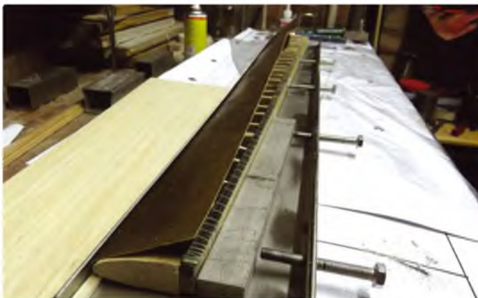
The tricky bit! This cramping tool is used to push the spar/rib assembly into the 'D' box to ensure that it is in contact with the ribs at all points. This prevents the thin Kevlar box from wrinkling when twisted by flight loads
