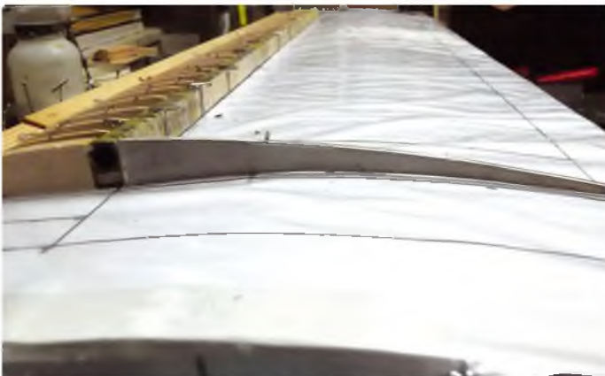
LDA section at the heart of Gary's new, home built, lightweight 3.7 m model. The extreme undercamber, compared with 'normal' eSoarers, requires the interesting construction techniques described in the text, starting with this aerofoil profile building board
