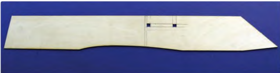
Never rely on a simple butt joint for fixing the servo rails. These cut-outs in the fuselage doublers mean that the rails have proper support
