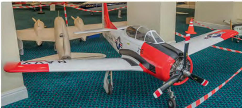
Harold Dowbekin's North American T-28 Trojan has a 12 foot wingspan and an Evolution 260 cc seven cylinder radial. The model should look and sound superb in the air!
