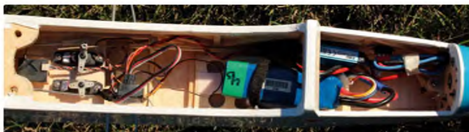
There's plenty of room inside Shrike's spacious fuselage. The green band (plus a large written 4) on the LiPo pack is how I tell 4S packs from my 3S (blue band) packs and 2S (red band) packs
