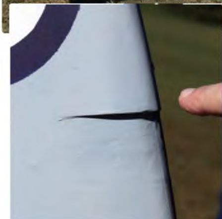
Left: A nifty trick Jim Lloyd put in the Spit is the NASA drooped aerofoils recessed into the tips. Although barely visible they reduce the model's tendency to tip stall
