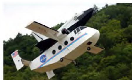
The McQuistans found that they needed to release the Shuttle going into wind otherwise the Shuttle would slide back into the Skyvan's tail! Despite learning that the hard way the original Shuttle and Skyvan survived
