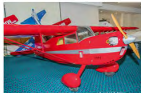
Rearwin Speedster built by Doug Rigby. Wingspan is 17' 6" and it has a ZDZ 180 cc petrol engine under the cowl
