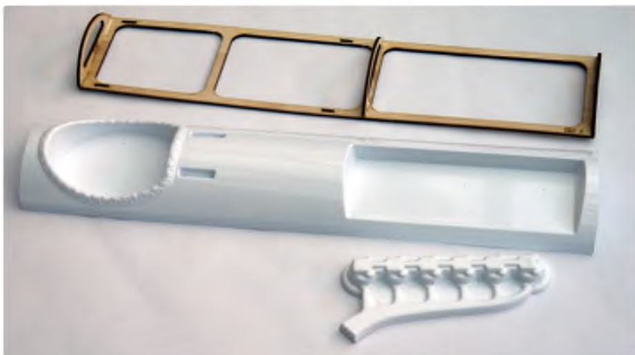
Forward upper fuselage and battery access hatch is made from a ply tray with a moulded plastic cockpit and engine
