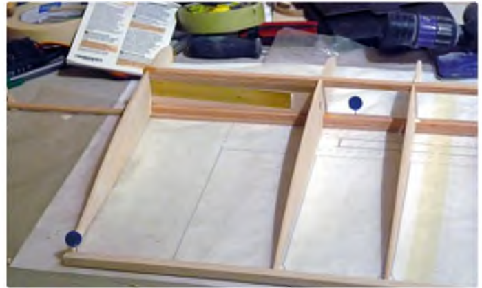
Fitting the wing joiner box between the spars
