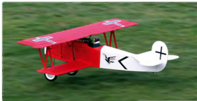
On a 4S LiPo the D.VII is away before hitting half throttle. Note the tail skid used by the reviewer instead of the steerable tail wheel supplied
