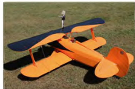
Another McQuistan model. This DIY store pink foam, 4.5 lb Krier Great Lakes Special (with spruce spars) is painted with ordinary Glidden house paint. A Suppo 60 on 4S-2200 LiPos provides more than enough power for slow, scale flight – right side up or upside down!
