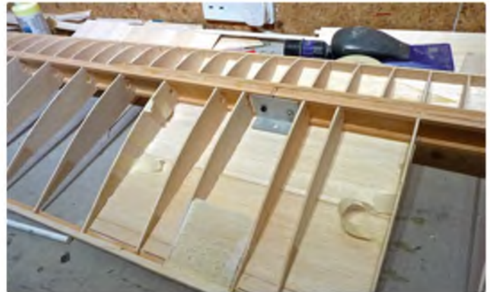
Aluminium bracket bolted to the ply infill between the spars
