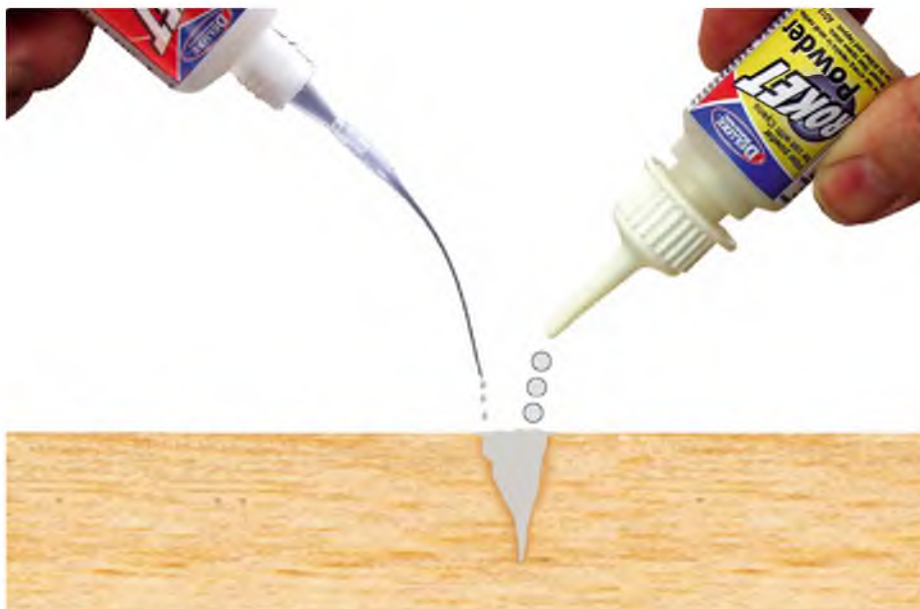
Gap filling using filler powder and a few drops of cyano
