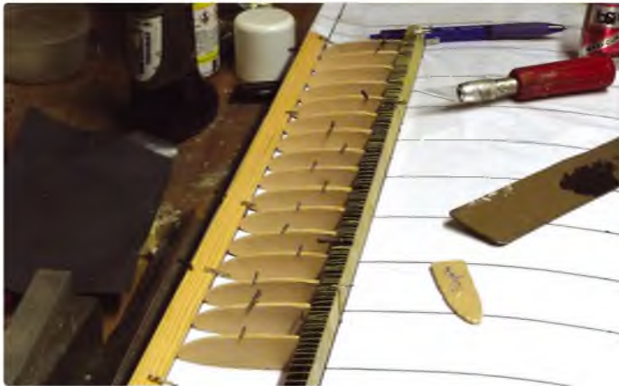
Nose section construction continues with the introduction of riblets between the full rib positions, to give more rigidity to the very thin 'D' box structure when it is wrapped around them
