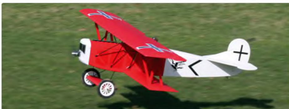
Landings are very straightforward. The forward set undercarriage helps reduce any nosing over tendency
