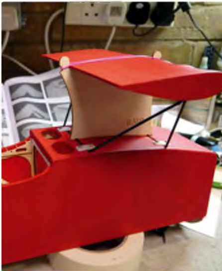
A template is provided to position the undercarriage winglet while it is being glued, using epoxy, to the undercarriage legs
