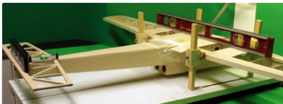
To keep the horizontal tailplane in line while the glue dries both surfaces are levelled with bubble levels and braced as needed. Slow curing epoxy or aliphatic glue is best here. Once the tailplane joint is dry the vertical fin gets added
