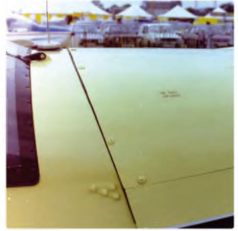
The upper cowling is fixed in place using quick release Dzus fasteners
