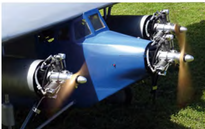
All systems go! Three times three cylinder 30 cc Saitos burbling away beautifully
