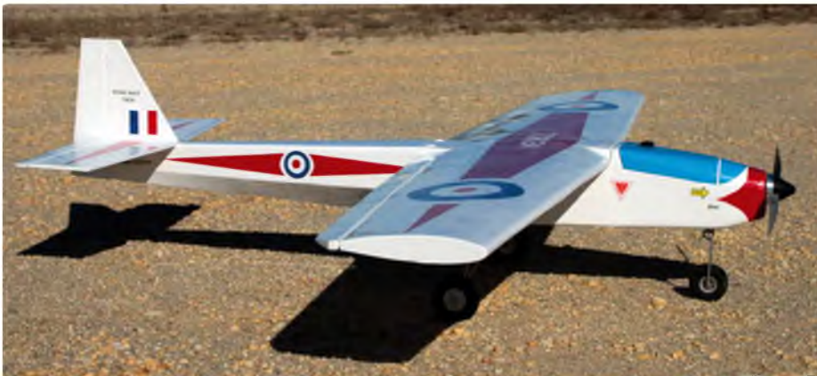
I used the Easy Roundel kit from Traplet to make the wing roundels. All of the red, white, and blue markings were cut from Profilm/Ultracote using a Gyro-Cut, also from Traplet. The black object behind the top of the 'canopy' is the hatch-latch, masquerading as a periscope/antenna!
