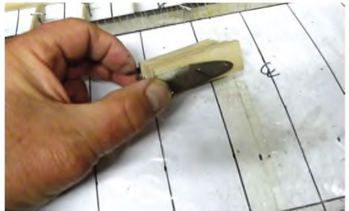
The spar has been constructed and is fixed to the board. Some of the nose ribs are jugged and fixed in place, whilst others have just been produced by the 'sandwich' method, to complete the panel
