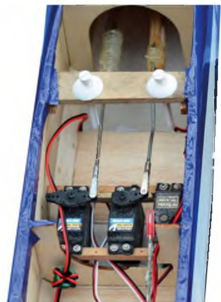
This arrangement allows the flaps to deploy to a more useful 45 degrees
