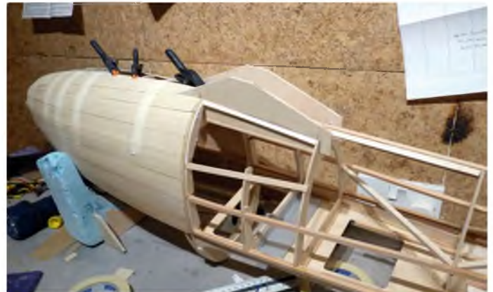
Completing the front ply planking
