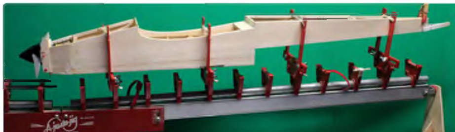
A fuselage jig is the best way to avoid building a banana
