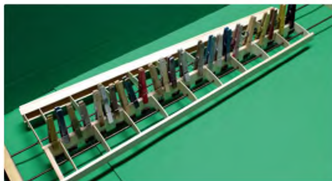
Since my jig has a short base I had to use binder clips to hold the bottom of the shear webs against the bottom spar, whilst spring pegs worked fine for the top edges. Be sure to glue the shear webbing to the FRONT of the spars so that you have an edge to clip onto when sheeting the leading edges. Yes, some of those cloth pegs are rather colourful, having been used to hold model parts whilst painting over nearly 40 years!
