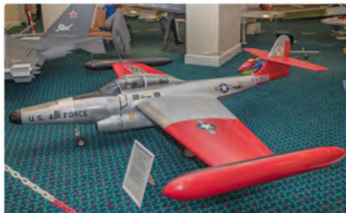
James Ladell's Northrop F-89D Scorpion built from the Air C Race composite model. The model has only one jet engine, a Jet Cat P160, which is offset to counteract asymmetric effects when applying the throttle
