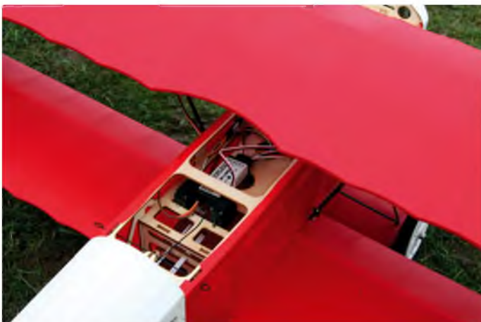
Battery hatch is removed by releasing the latch and pulling it back behind the upper wing. A telemetry receiver was used to monitor current in flight
