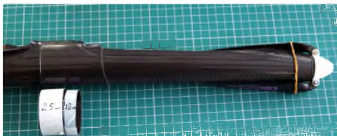
To get my Xplorer to balance correctly, using a 'heavy' 130 g motor, I first removed a 25 mm ring from the nose section to give an approximate C of G. Then, after careful balancing, I cut another 12 mm section. The fuselage spigot needed shortening a little to allow it to fit
