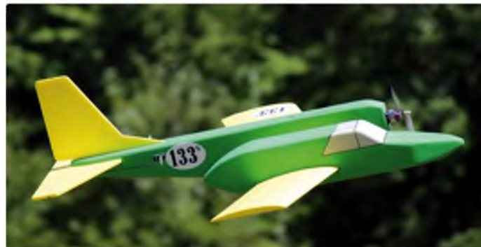
Above & below: John McGrath scaled up Terry Dunn's Parallax (May, 2014 Model Aviation) and extended the tail for smoother flight. John's version, spanning 42.5" and weighing 33.5 oz, boasts a fuselage of pink insulation foam and a Depron wing with carbon fibre spars
