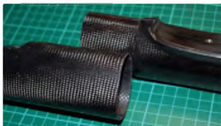
Xplorer F5J has been lightened for 2017 and the fuselage is in two pieces. The joint is in the parallel section just ahead of the wing, making it very easy to shorten should you wish (or need!) to do so
