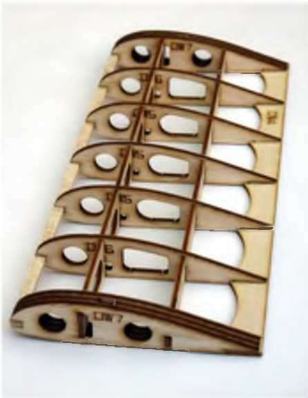
Undercarriage winglet. The middle three ribs have holes for the axle and the outer ribs have slots to allow the axle to flex, providing some suspension. The outside ribs are of laminated construction, with provision for the undercarriage legs
