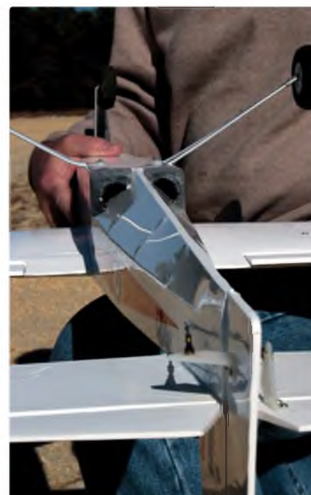
Above left & right: Once the outer surfaces of the dummy exhausts are roughed out, hollow with a hand grinder and sanding bits. Don't use Warp 9 speed, lest the foam disappears! Fine sand the finished foam, then coat it with water based balsa filler and sand with very fine (400 or better) grit sandpaper or sanding sponges. Finish with foam safe paints
