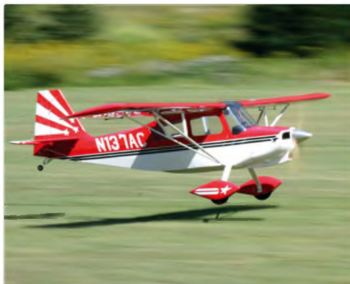
The plan was for Gerald's Hangar 9 Citabria Decathlon to be able to fly ten minutes of acros, three times, on a single charge. Hence it has a 12S-16000 (yes - 16,000!) LiPo powering its Easy Tiger 100 motor
