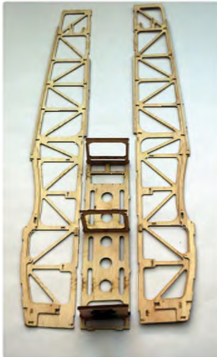
Fuselage sides and battery tray with doublers and formers ready for assembly. Make sure you make left and right sides!
