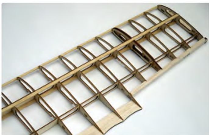
Note the pre-shaped scalloped trailing edge
