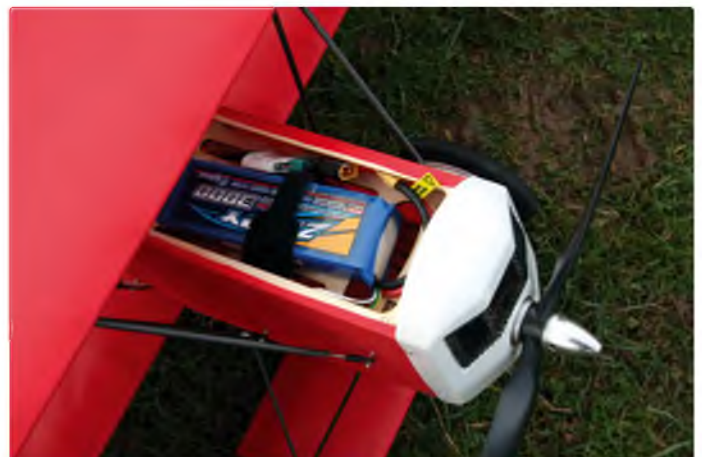
Plenty of room for 3S and 4S batteries. The 3000 mAh 4S battery used for the initial flight test was replaced by a 3000 mAh 3S pack as the 3S set-up was more than adequate
