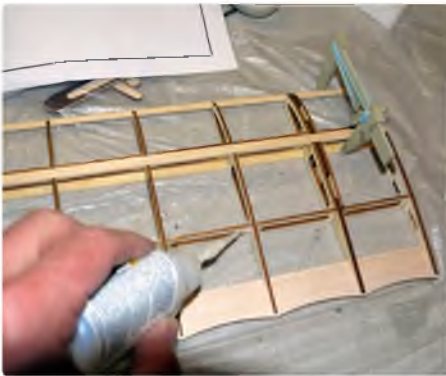
Superphatic glue was run into all joints
