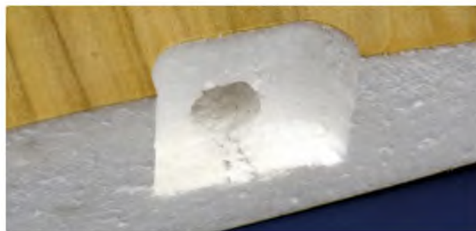
Having pre-cut routes for extension leads makes things really easy when installing the servos
