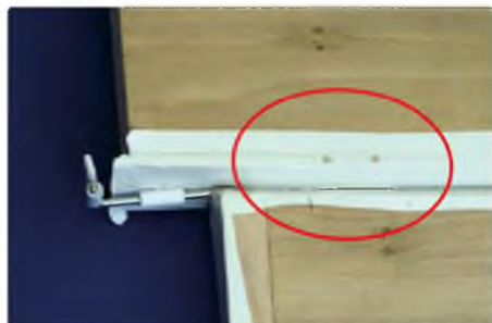
Hinge and pin all control surfaces before final covering
