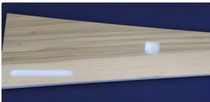
Cut outs in the foam wings ease the building process but be prepared to resize them to suit your servos or to add extra ones for flap servos
