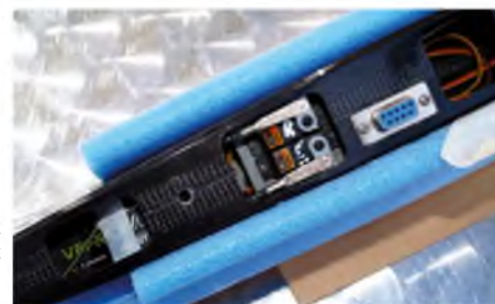
Right: Underwing area on the 2017 Xplorer has more access openings than previous models. You might wonder why the eight channel Rx has '4 channel' written on it? So do I!
