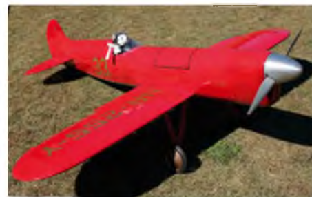
This Brown B-2 (possibly an old Bridi kit) sat in Mark Senior's basement for 20 years. It now has an Astro Brushless 80 Geared, turning a 19 x 12 on a pair of 4S-5000 packs
