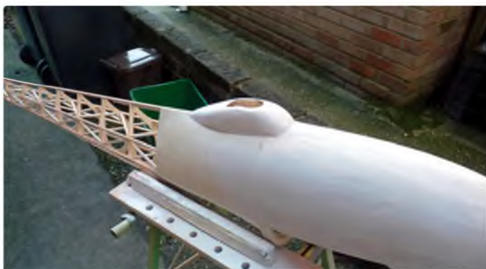
Completed wheel fairing
