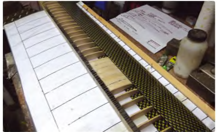
Once the spar and front rib sections are complete they are ready to be glued into the 'D' box. As this is the centre panel there is extra reinforcement added for the wing to fuselage joiners
