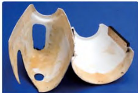
The ABS cowl will need strengthening if you use an IC engine
