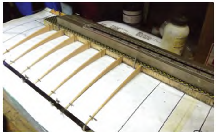
Several steel bars hold the 'D' box in place on the board as it cannot be pinned down, whilst the rear ribs are fitted to the spar and trailing edge carbon strip. Note that only the pin heads retain the ribs in position
