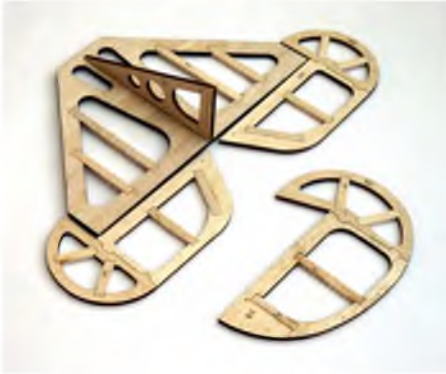
Tail surfaces are made from laser cut sheet pieces with strengthening pieces orientated to prevent warping
