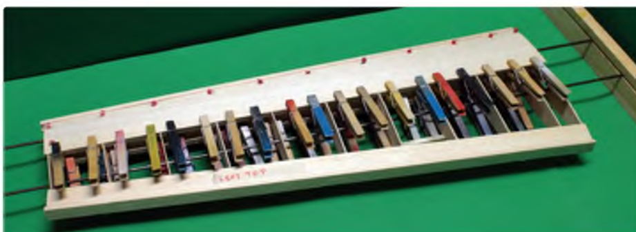
Sheet the bottom LE, then flip the wing in the jig and sheet the top. Note the second layer of clothes pegs under the first – a large collection of pegs is good to have!
