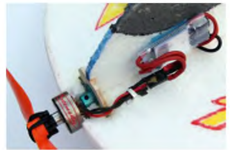
The more powerful motor still only needs a 3S 800 mAh LiPo pack for good performance
