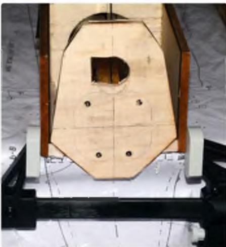
The massive amount of bend needed in the fuselage front is obvious in this picture. The F1 former should be glued to the triangular fillets before anything else is done
