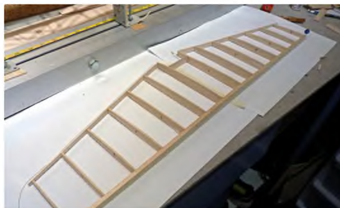
Basic tailplane structure
