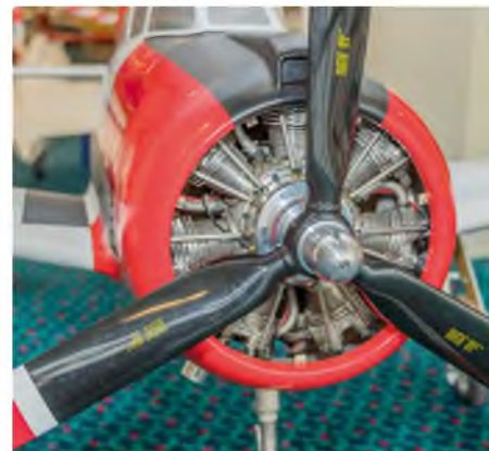
Harold Dowbekin's North American T-28 Trojan has a 12 foot wingspan and an Evolution 260 cc seven cylinder radial. The model should look and sound superb in the air!
