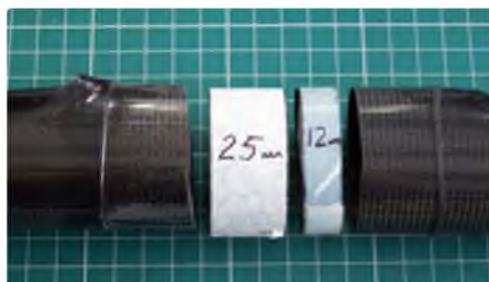
To get my Xplorer to balance correctly, using a 'heavy' 130 g motor, I first removed a 25 mm ring from the nose section to give an approximate C of G. Then, after careful balancing, I cut another 12 mm section. The fuselage spigot needed shortening a little to allow it to fit
