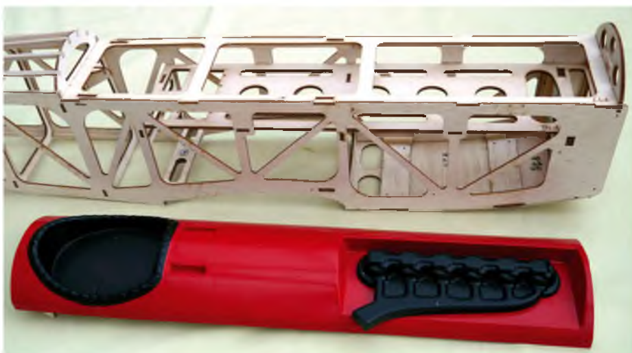
The top hatch was sprayed red and the engine and cockpit area painted black
