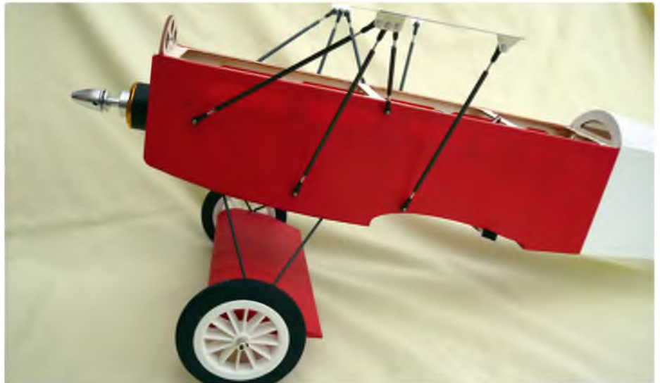
Upper wing mount is fixed to the fuselage with carbon tubes and ball joints. The wing is secured to the metal mount by four screws
