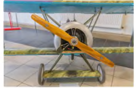
Andy Sherborne's scratch built 1/3rd scale Fokker D.VI, which has a Saito 450 three cylinder radial for power
