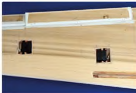
Part of the solution to making working flaps is to run each flap from a separate servo. You will need to make your own wing cut-outs
