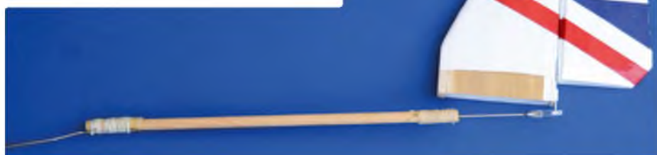
Right: Finish the fin and rudder before fitting them to the fuselage and tailplane
