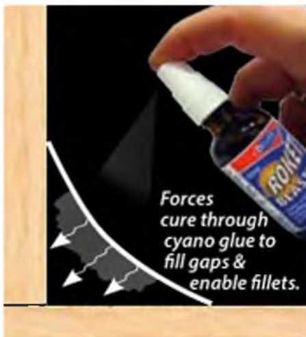
Using kicker to fill gaps and make fillets
