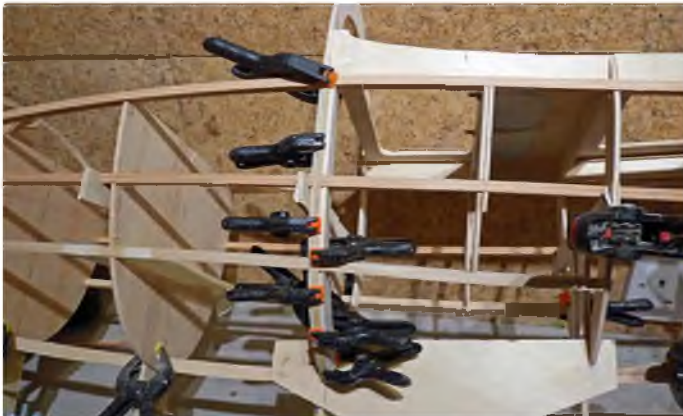
Doubling up F6 with 6 mm balsa to increase gluing area
