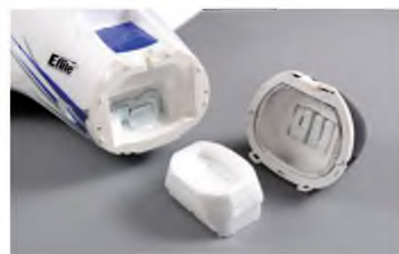
The standard nose (and the model!) is supplied with plenty of glued-in nose-weights
