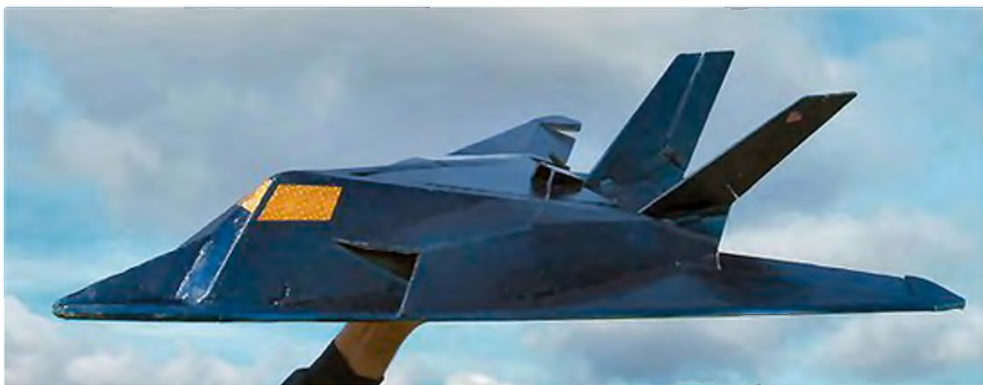
'Midnight Blue' stealth fighter is a piece of classic Mike White Depron electric design. 1500 KV motor drives a prop-in-a-slot. You just know it's going to be quick. Choice of control mix offers 'impressive' to 'outrageous'!
