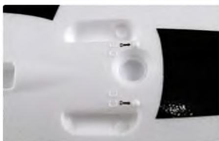
Close-up on the finger pockets for launching and the C of G dimples
