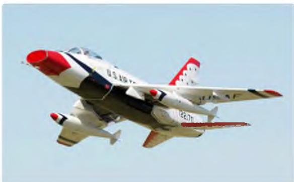
Pastor Greg Hames' 1/5 scale Fei Bao F-100. 85 in wingspan, 55 lb, JetCat turbine
