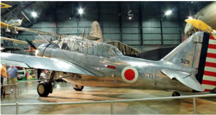
Typical of a failed concept in Army support, the O-47 was too heavy for rough fields and too slow and clumsy to survive against fighters. Expensive, it had to be based at fields with paved runways. Its liaison and forward observation duties were instead performed by converted light aircraft, capable of staying with the troops and providing quick, responsive support
