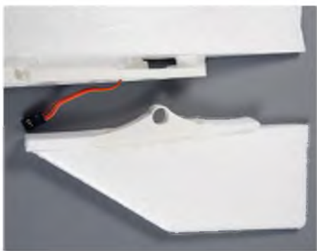
Short vertical fins locate in slots moulded into each wing root
