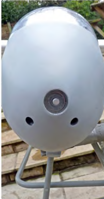
Motor shaft bearing is recessed in the solid nose. Note the cooling vents underneath
