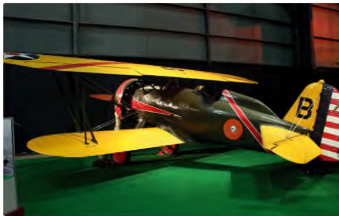
Boeing built the P-12 for the US Army, whilst a very similar model served the US Navy as the F4B-4. Known as a very nimble, fun to fly aircraft, many WW2 US aviation commanders learned their trade on the P-12/F4B series
