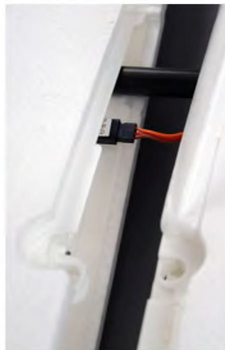
Each servo extension lead plugs into a connector that is firmly fixed within each wing root
