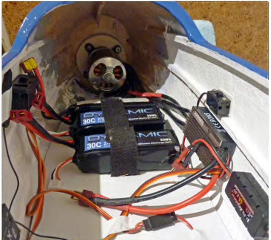
Motor shaft bearing is recessed in the solid nose. Note the cooling vents underneath
