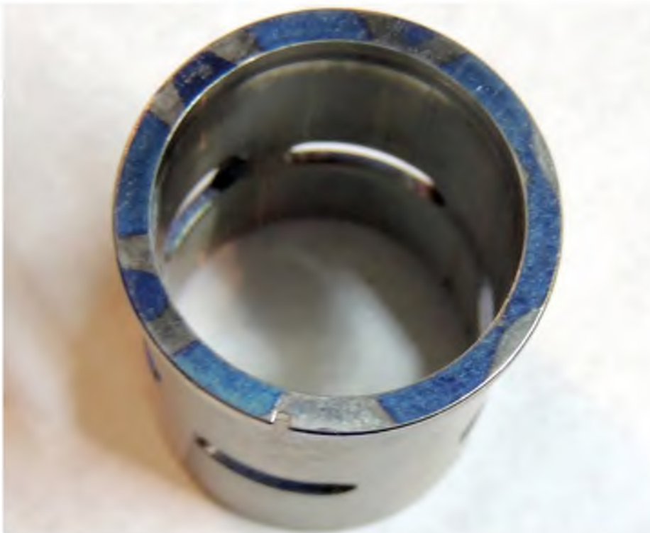
The colours on the rim of this liner indicate use of one of the evaporative coatings, such as evaporated nickel or a bi-metal coating, either of which are super slick and extremely hard
