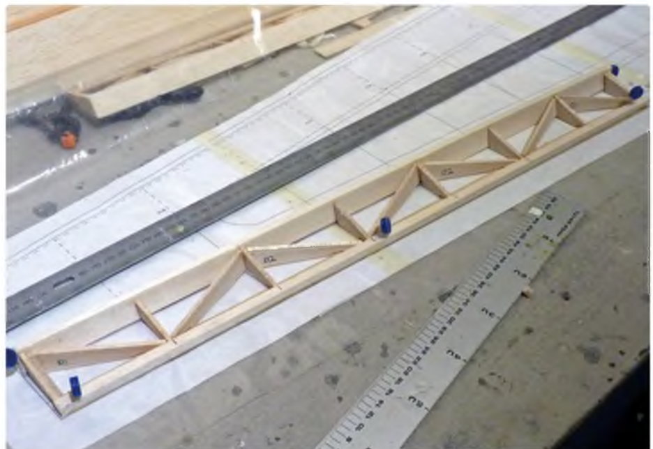
Ailerons are built flat on the board
