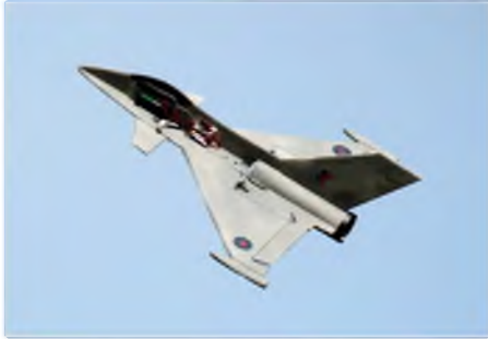
Micro Typhoon number two climbing away. The straight, non-VT tail-pipe can be seen
