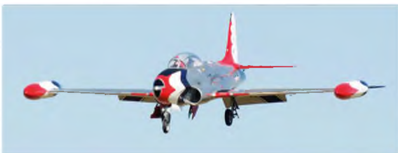
Roberto Zelaya's Fei Bao T-33. 108 inch span, KingTech 210 turbine, DX-20 radio
