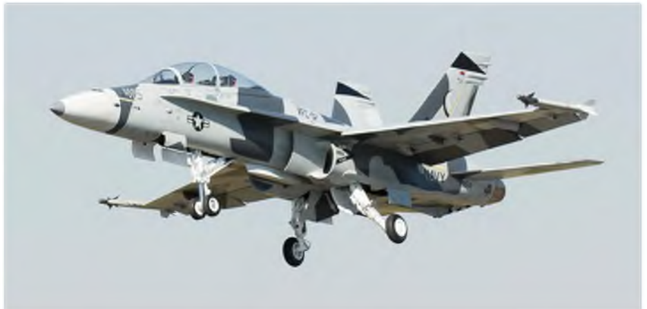
Kristopher Gunter's Skymaster F-18D Hornet. 117 inches long, twin KingTech K-180 turbines
