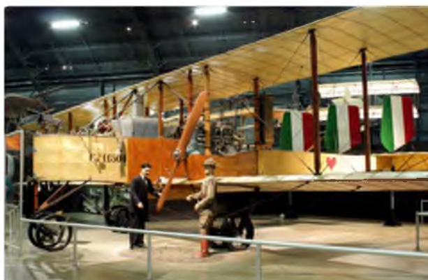
The tri-motor, twin-boomed, triple tailed Caproni C.A. 32 to 36 series of bombers was the backbone of the WW1 Italian bombing force. Note the two fuel tanks immediately behind the pilots - no need to post a 'No Smoking' sign!
