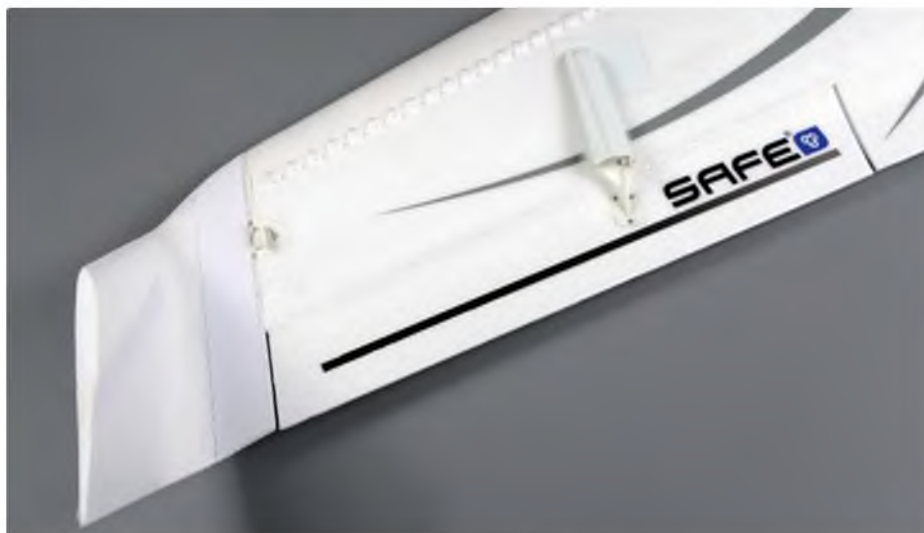
Top view of the port wing showing the winglet and locking pin in place. Note also the top mounted elevon servo shroud and the vortex generators along the leading edge
