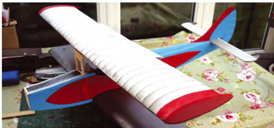
For covering small models I now use heavyweight tissue and PolyC sealer. This is water based and does not smell, so the job can be done indoors
