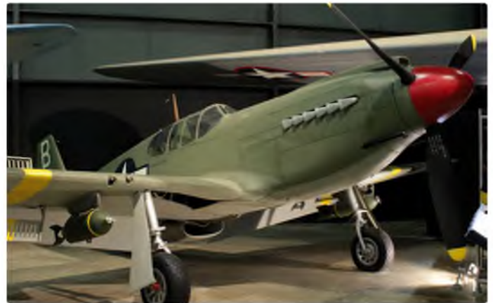
No, it isn't quite a P-51. The A-36, derived from the early Mustang design, maintained the early version's Allison engine and machine guns mounted underneath the nose. Visible above and below the wings are the brakes required for dive-bombing
