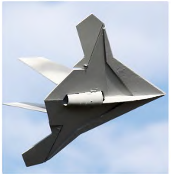
Underside view showing the EDF unit and elevon shape
