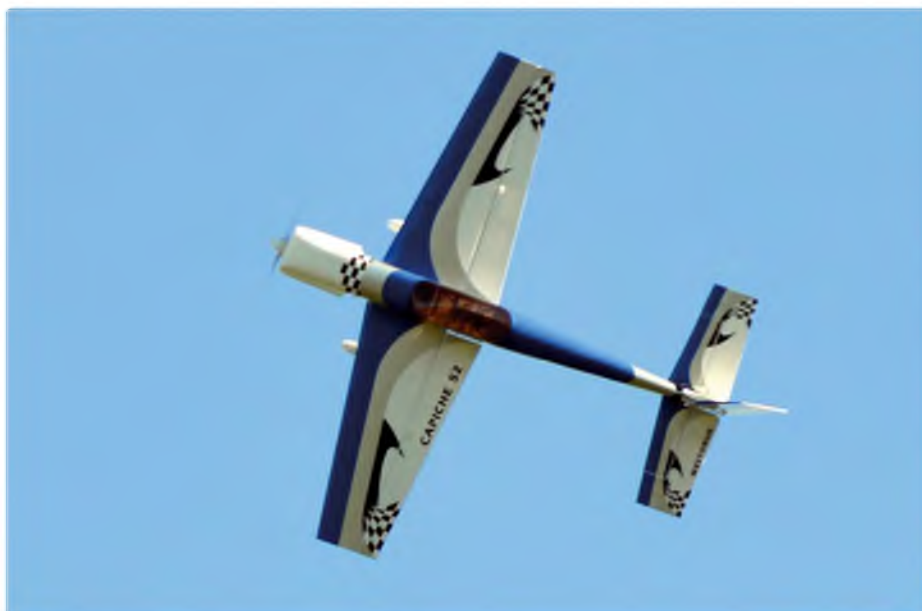
A small tuck to the undercarriage in knife-edge was cured with a two percent mix of up elevator
