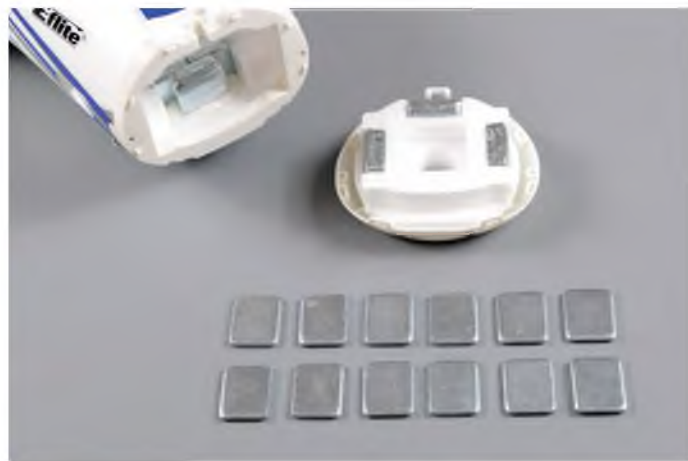
A set of weights are provided for maintaining the C of G when swapping between different cameras
