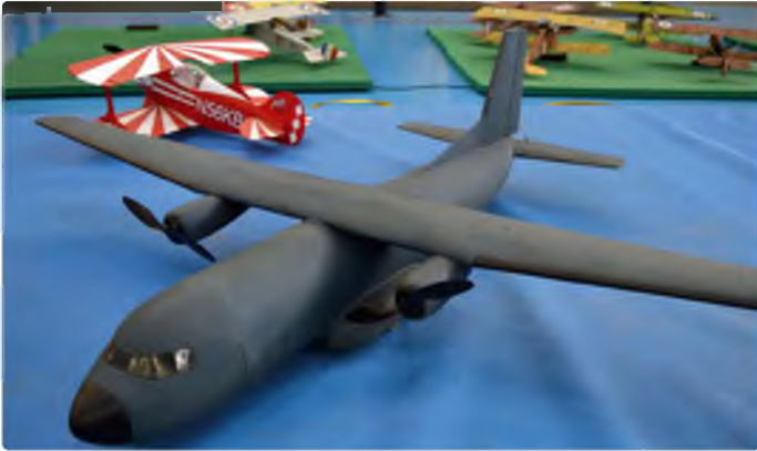
Yann Dobignard's C160 Transall in threatening 'night' paint. A very able model that flies at a remarkably low speed and 'turns on a sou' thanks to the differential motor control
