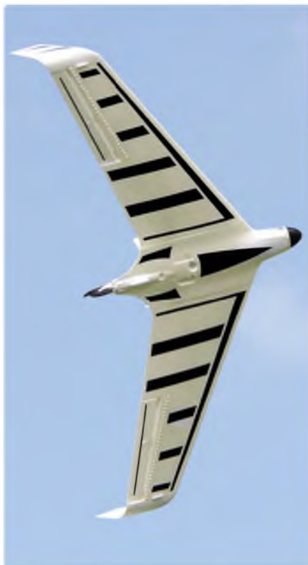
Black underside stripes help orientate the model when flying at higher altitudes
