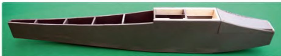
Formers are mostly cut from 6 mm Depron, apart from those around the wing and U/C mounts, which are from 6 mm lite-ply. I line the wing openings with 6 mm balsa and pre-drill the wing dowel holes in both pieces before I glue them to the Depron
