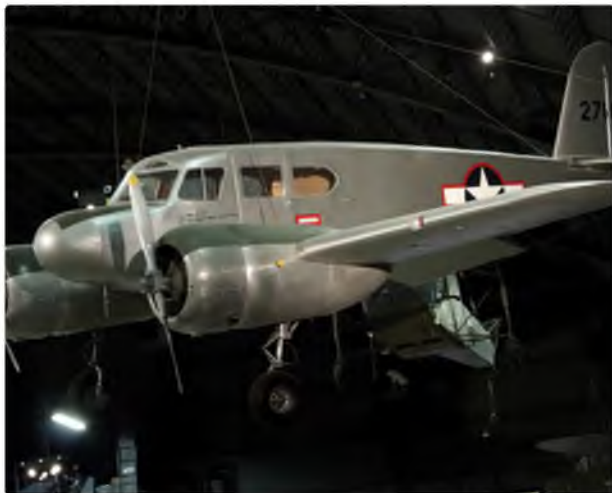
Often called the 'Bamboo Bomber', the Cessna UC-78 Bobcat (civilian T-50) was used by several Allied nations as a light transport, trainer and all-round utility aircraft. Some of us may recall that Sky King's first Songbird was a Cessna Bobcat (from repeats of the TV series, that is - I'm not that old... Stop snickering, Micki!)
