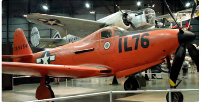
The Bell P-63 was what the P-39 could've been, had Bell been allowed to equip it properly. This P-63E King Cobra is painted as an RP-63A, a variant equipped with lightweight armour, to serve as a target for aerial gunner trainees (with special, frangible ammunition in their guns). When a trainee scored a hit, a strobe in the spinner would flash
