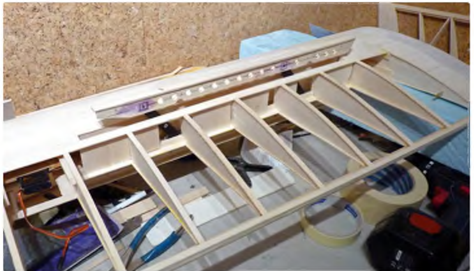
Fitting the airbrake to the wing
