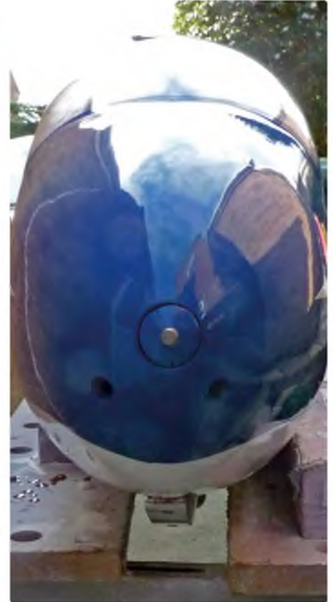
When not in use the motor shaft is covered by a blanking plug
