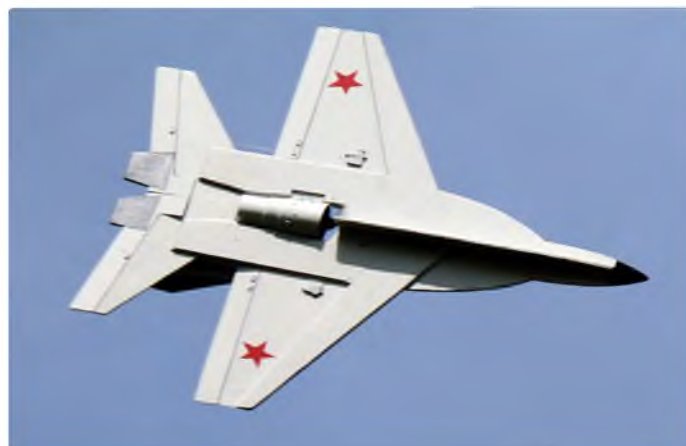
This view shows off the underside and my strengthening with Depron
