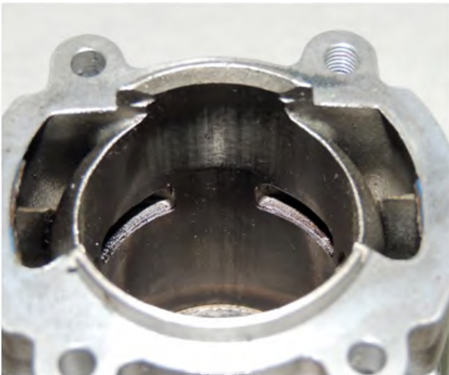
An example of a large capacity petrol engine cylinder with an integral chrome liner. Hard chrome is applied directly onto the inner surface of the cast aluminium alloy cylinder – a very popular surface coating
