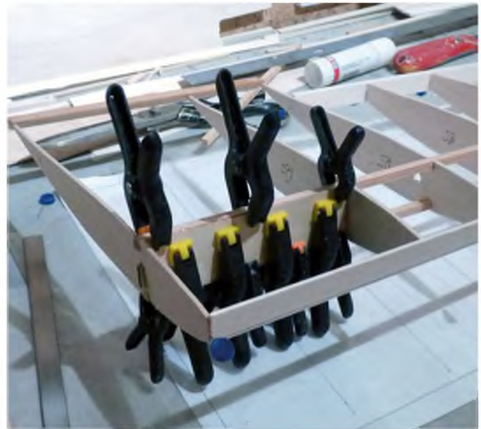
Closing off the wing joiner box with 0.8 mm ply webbing
