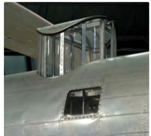
An interesting feature of the B-18 is the retracting dorsal turret. Not much visibility upwards but it could be a nasty surprise to an attacker coming from behind
