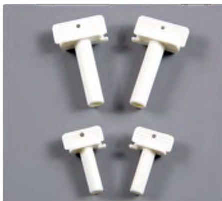
Large locking pins are used to secure the wing panels. Smaller ones are used to fix the winglets
