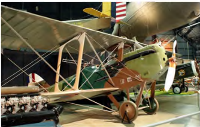
Designed by a French officer working with the American Packard Company, the two-seat Packard-LePere US Army Combat (LUSAC) 11 was a two-seat fighter, of which only a handful were built. Several soldiered on, doing valuable experimental work into the early 1920s
