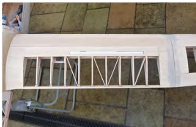
Diagonal supports in the wing to support the TE
