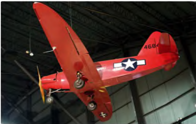
The Culver PQ-14 had a full, enclosed cockpit and could be flown as a nice little single-seater. Or it could be flown by radio control and blown to bits for anti-aircraft practice!
