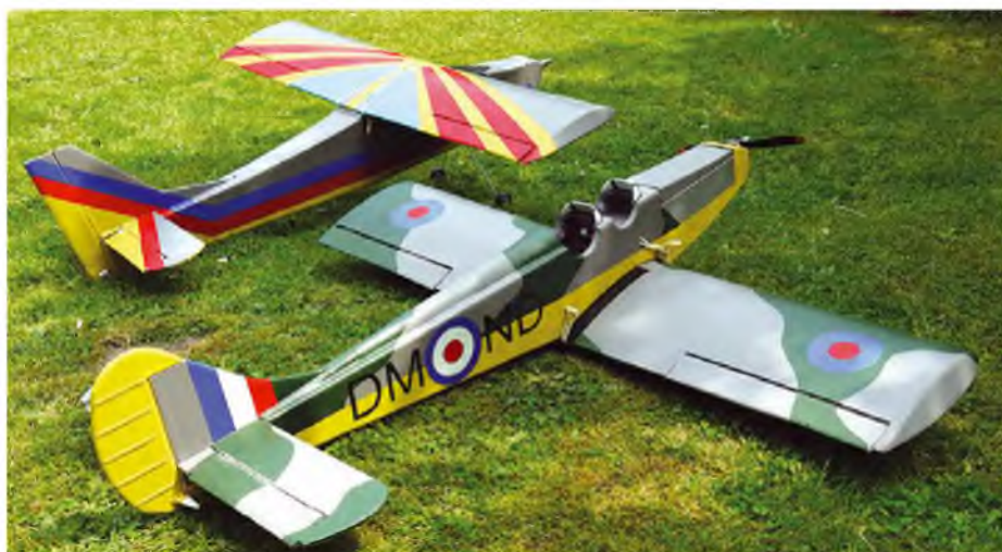
When painting a model I use household emulsions bought from my local DIY store. Tester pots are an economical way of applying different colours
