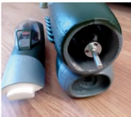
Motor access is a cinch thanks to the Typhoon's large diameter cowling
