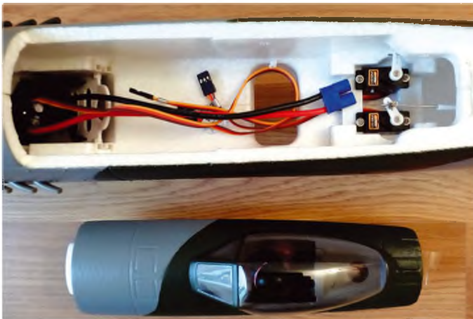
The battery bay has ample room for a 3S-2200 LiPo
