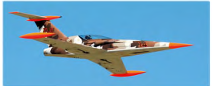
Todd Witkoff's Diamond from Aviation Design. 98 in span, 38 lb, JetsMunt 200 turbine, DX-18 radio
