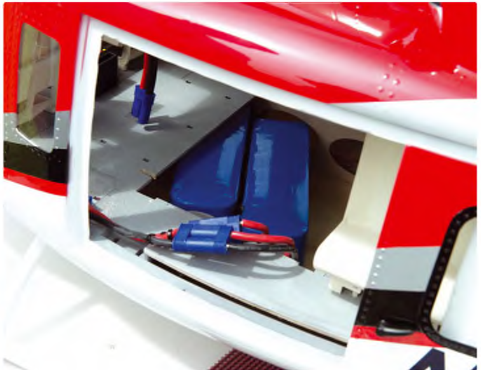
Battery access for my installation is via the left/hand sliding passenger door and the twin OptiPower 6S packs sit in an underfloor cavity in the passenger cabin. Pre-flight, both packs are connected to a Y-lead and then pushed right to the front of the cavity to obtain the correct Centre of Gravity. Then a flexy-foam block (that I concocted) is pushed into the remaining space to keep the batteries in place. To finish, the cabin floor is clipped in place. This securely retains the battery packs and leaves the cabin free of any battery clutter, apart from the ESC to battery connections
