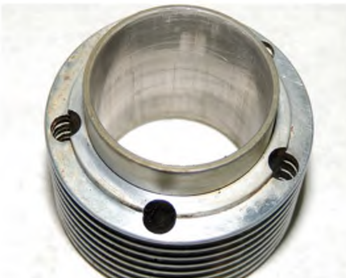
Nickasil surface coating is now used in all Laser engines and they have a reputation similar to the O.S. liners of not showing signs of wear even after, possibly, hundreds of hours of use
