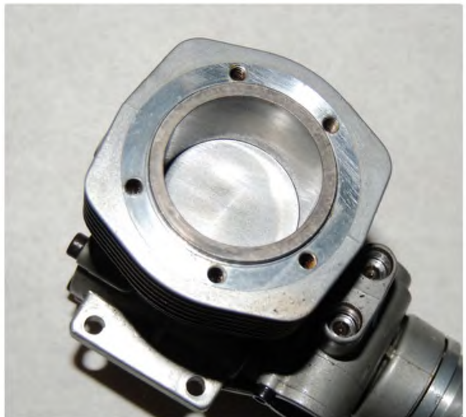
One of the most well known and respected liners is used in many O.S. engines. Hardness treated steel of super accurate roundness, they have a reputation for never wearing out (under conditions of reasonable use)
