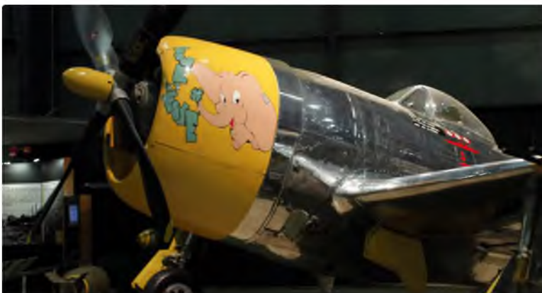
The massive P-47D was the largest and heaviest single-engined fighter of the war. Armed with eight .50 calibre Brownings it wasn't as manoeuvrable as its opponents but it had a hefty punch and was rugged enough to bring home its pilot after a mauling
