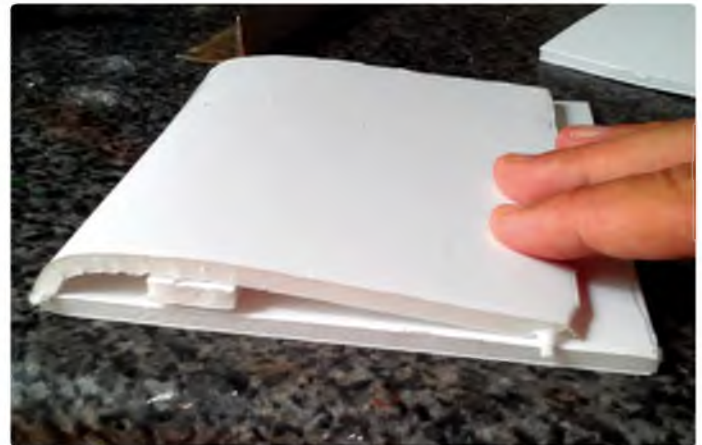
Dave's model is constructed from 6 mm foam board, which can be folded to form the wing
