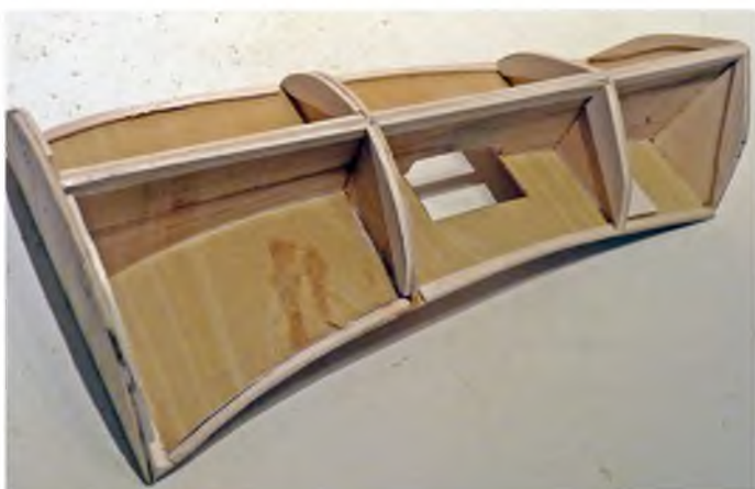
Wing fairing structure
