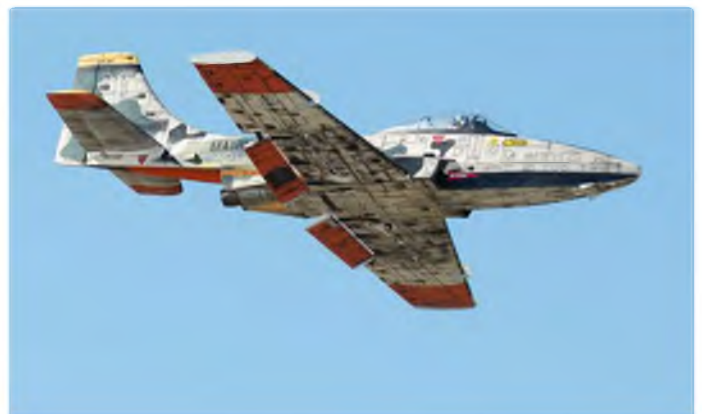
Dana Thrasher's Turbinator of 76 in wingspan, 26 lb, with P140X turbine. Marine Corp colour scheme
