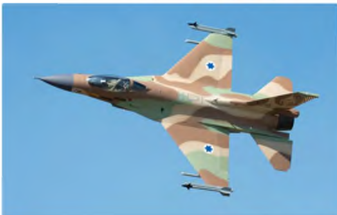
Eduardo and 'Jet Girl' Anna Esteve's new 1/5 scale BVM PnP F-16C. 80 inch wingspan, 46 lb, KingTech 210 turbine, DX-18 radio
