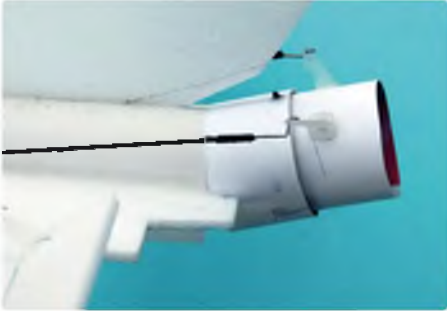
A close up of the VT tail-pipe
