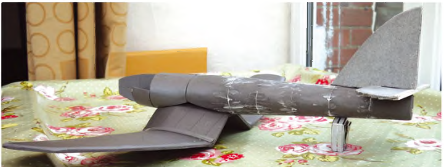
This F/F gull wing Supermarine model is powered by a KP02 motor. Test glides have been promising so a larger R/C version will be started soon
