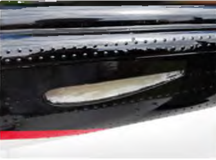
The tail boom recesses, which are used to mount the tailplane halves, after I had ground out the paint to give a good glue joint
