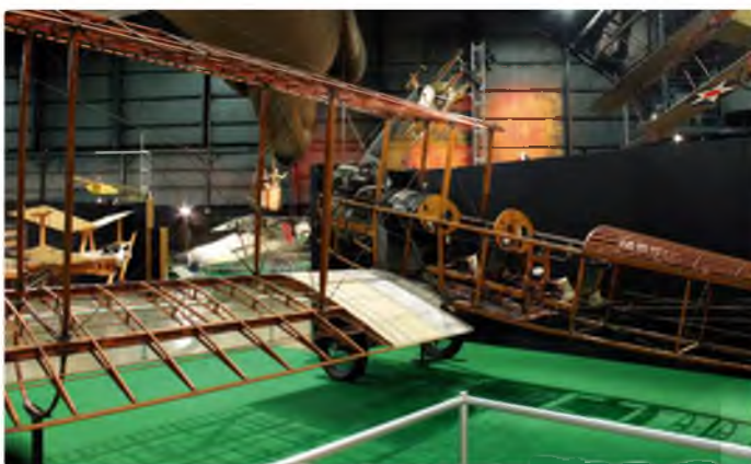
A second Standard is displayed, minus its doped linen covering. I'm always amazed by the intricate wood-working on pre-Golden Age aircraft, especially the carefully routed spars with integral shear webbing
