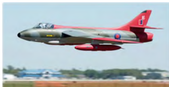
Rei Gonzalez's Fei Bao Hawker Hunter. 120 inches long, 88 in wingspan, Jet Central Cheetah turbine
