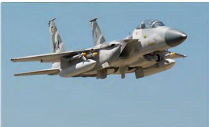
Michael Sarysz's Fei Bao F-15, winner of a Special Recognition Award. 73 inch wingspan model is powered by a Mammoth SE turbine
