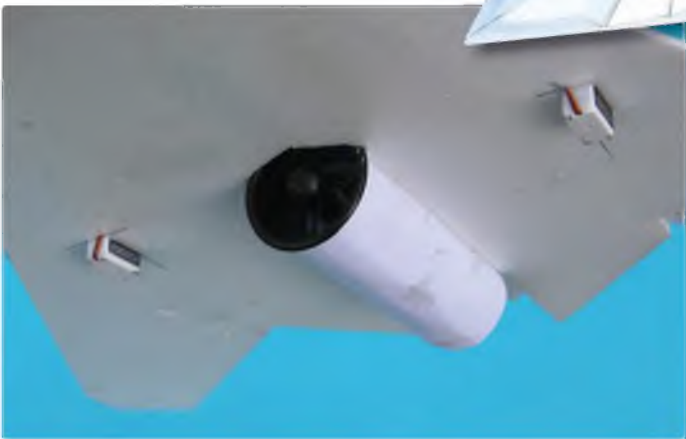
An underside view shows the EDF position. Stay off the concrete when landing!
