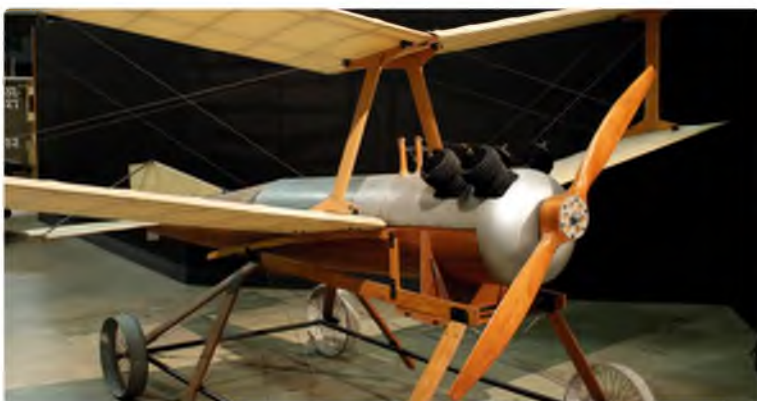
Looking like a large free flight model, the Kettering 'Bug' was the worlds first 'cruise missile'. Armed with a 180 lb warhead, the Bug was to be launched from a short track and dolly. Guided by pre-set pneumatic and electric controls, the Bug would cruise for a pre-determined interval, then the engine would stop and the wings would fall off. The Bug would fall and the bomb would detonate. Not completed in time for WW1, development was cancelled shortly after the Armistice was signed
