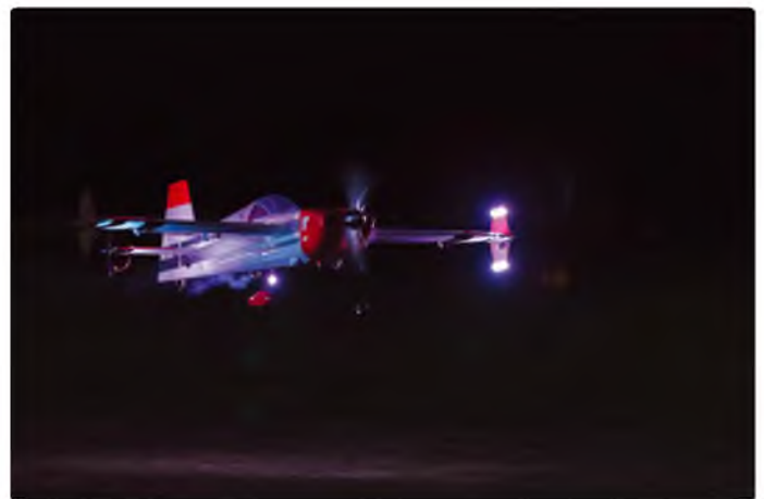
Team Global RC pilot Ross Baseley flying an Edge 540 3DHS of 106-inch wingspan and powered by a DLE 111
