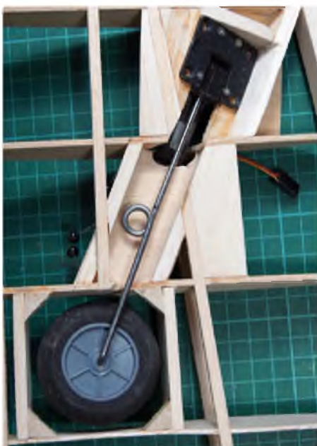
Retract units are mounted at an angle, fore and aft and vertically too!
