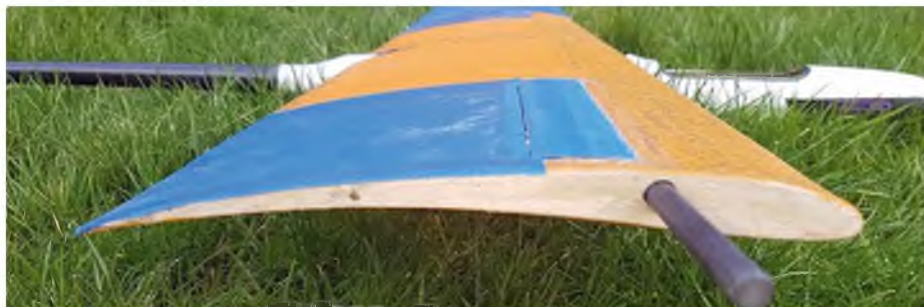
The Low Drag Aerofoil used on Gary's model and a view of the wing joiner. Much more undercamber than a 'normal' electric soaring glider but it works in lightish air
