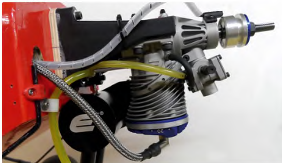
The engine was fitted to a plastic mount, as recommended by Horizon
