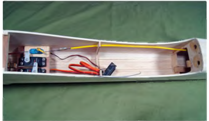
The throttle is controlled by a small servo and snake – just make sure the servo is well secured!
