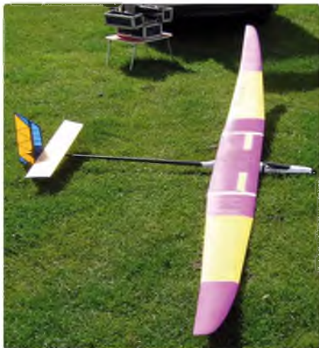
The next generation is already upon us! Gary's latest eSoarer is slightly smaller in span than the one described and uses a different aerofoil, with less camber
