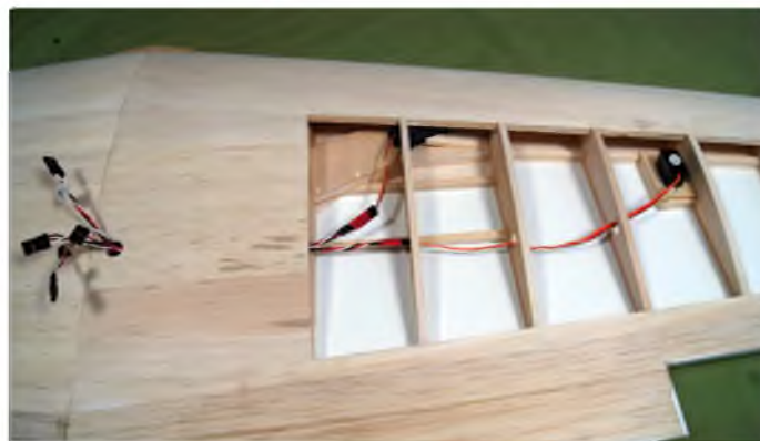
Direct aileron connections make for snappier control responses
