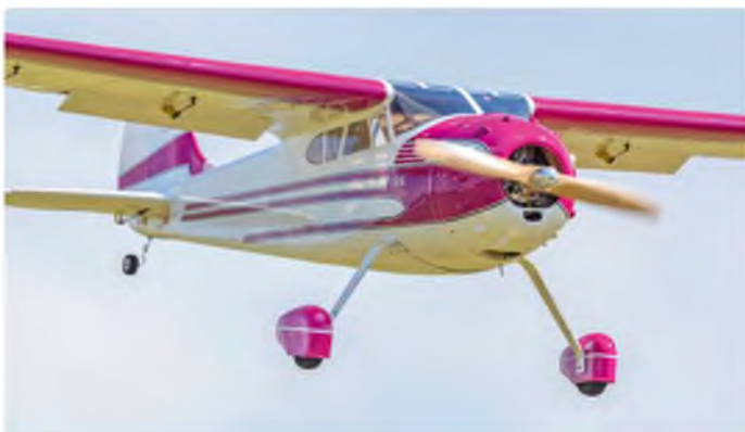
A lovely looking model of the Cessna 195 from the YT International range. The model has a three cylinder Saito 60 cc petrol engine for power
