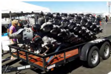
Only in America! Two 36 cylinder R3400 engines were 'Siamesed' to produce a 5,000 hp engine. It will need a very special airframe
