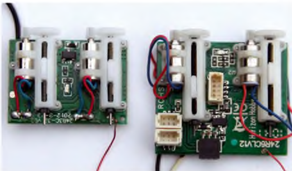
The small size of the Mini Vapor Rx/module is shown here. A lead for the motor connection has to be soldered to the board. Get out the magnifying glass!
