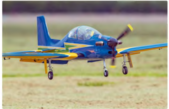
Ken McCormack's Phoenix Models Volcano. The Volcano is powered by a Wren 44 turbo prop engine
