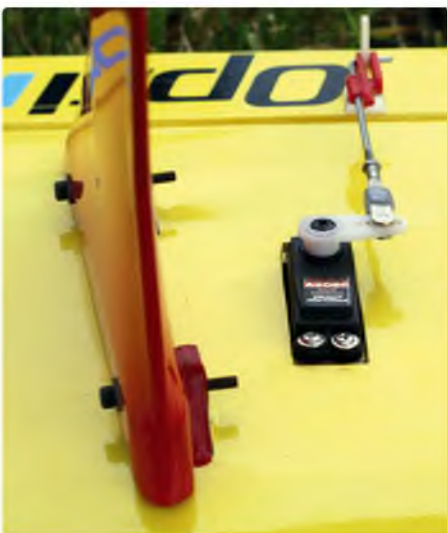
Each of the four ailerons is now driven by a wing mounted servo rather than by just two servos and connecting rods
