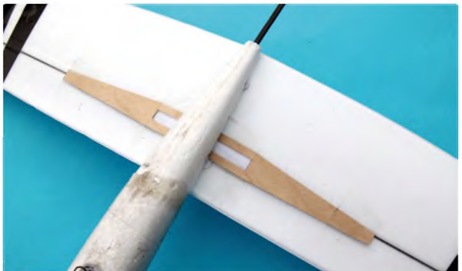
My Whipet wing strengthening uses 1 mm ply and has worked fine
