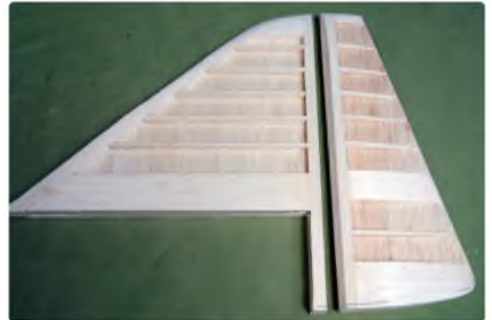
Tail feathers are built using a thin balsa core with a lightweight structure glued on either side
