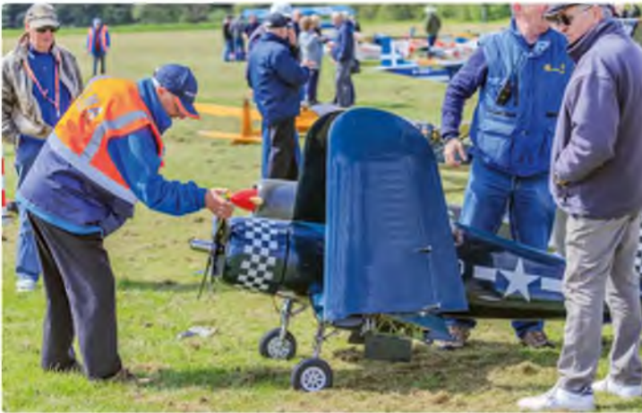
Tony Hooper about to start the large Moki radial engine in his CARF-Models Corsair, which also features the CARF folding wing system
