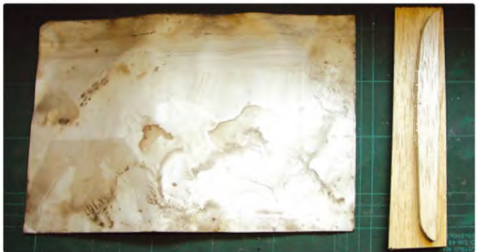
An annealed square of lithoplate next to a forming jig
