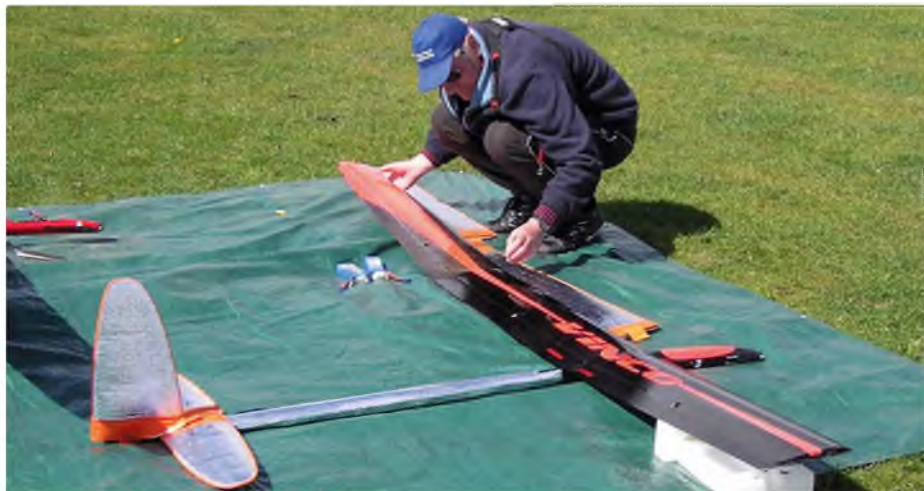
Richard Brown assembling his Vinco 4 m lightweight eSoarer at the 1st Northern eSoaring League event. Model uses DLG type, solid Rohacell-cored flying surfaces, to achieve minimum weights of close to 1,100 g
