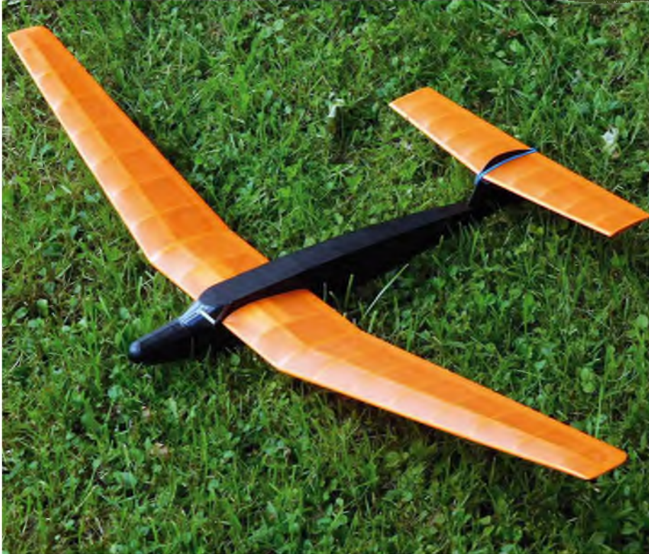
Another of Peter Fisher's distinctive Performance Kits designs brought back to life by Simon Rogers. The 33" span 'Neutron' towline glider has quirky Fisher styling throughout and features a two piece knock-off wing. It proved to be a very capable flyer, seen in flight over Salisbury Plain
