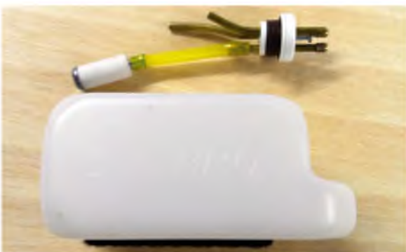
You can save weight in a petrol powered plane by using a much smaller fuel tank
