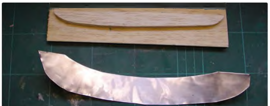
Soap residue cleaned off and cut oversize to make a wing stub
