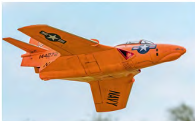
The Skymaster Grumman Cougar of Mark Hinton stands out well in its orange experimental aircraft livery. A JetCat P120 turbine powers this 85" wingspan model
