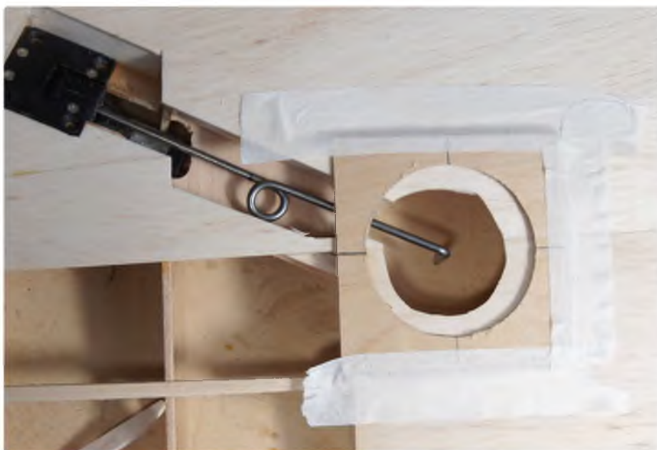
Use a card template to cut neat holes for the wheel wells
