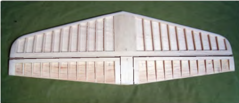
Tail feathers are built using a thin balsa core with a lightweight structure glued on either side
