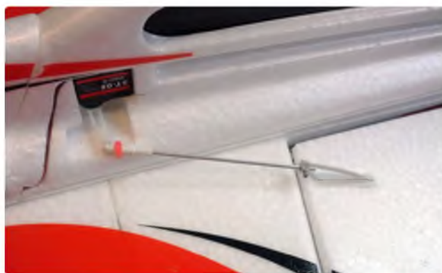
Underside view showing the main plane bracing
