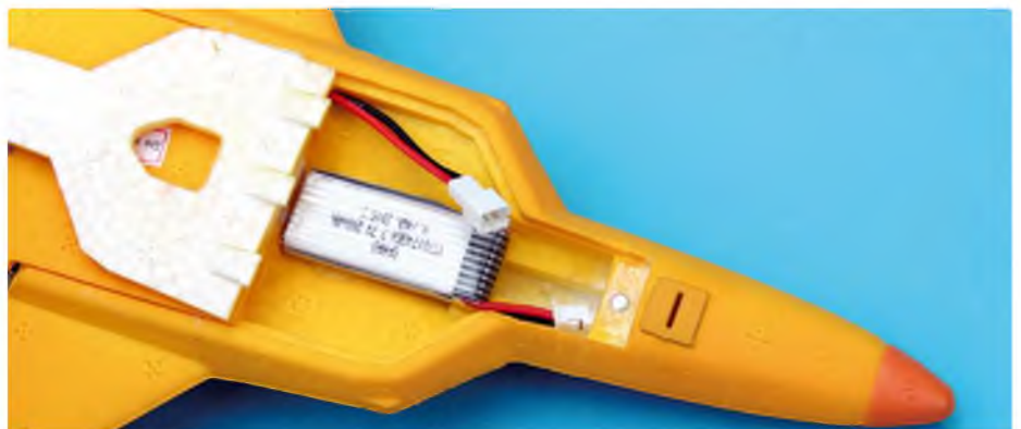
The 1S LiPo is situated under a hatch near the nose. The model can be flown without the U/C
