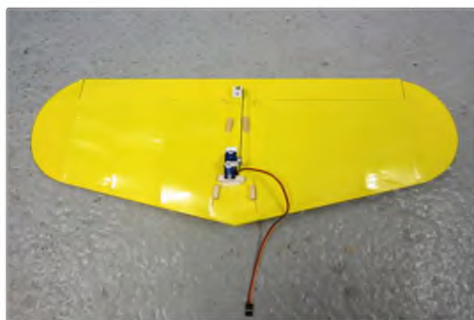
Like the wing, the tailplane is banded on. You can either mount a micro servo on top or use a long pushrod to operate the elevator – your choice!
