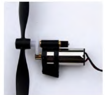
The geared motor/prop units used on these models are very inexpensive and have applications on other models
