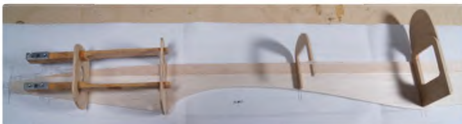
Adding the formers to one fuselage side before adding the second side
