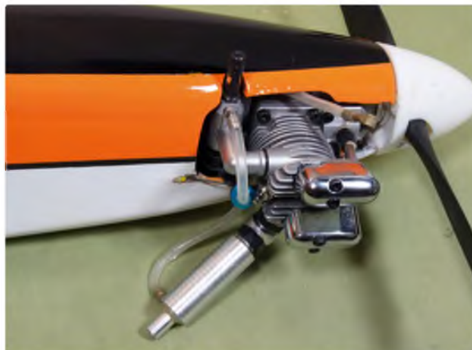
The Saito FA-40 four-stroke is neatly faired in
