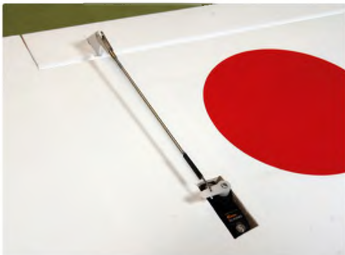
Cover the bottom of the wing first, then fit the U/C and aileron servos with their extension leads while they're still accessible
