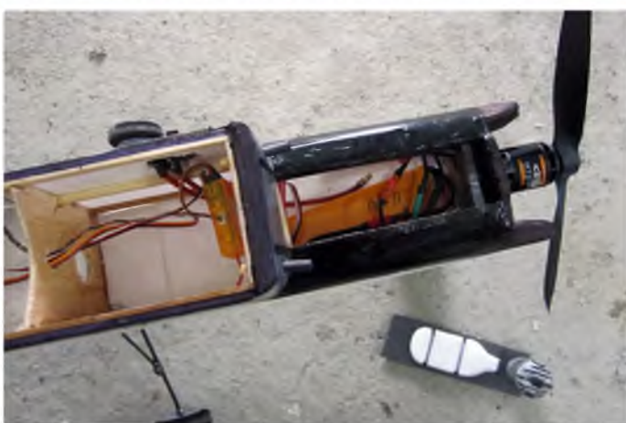
Front end view. Note the dummy diesel engine and fuel tank on top of the battery bay hatch
