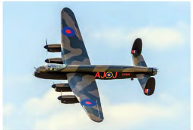
Andy Johnson's 18 ft wingspan Lancaster uses four Zenoah 38 cc petrol engines for power
