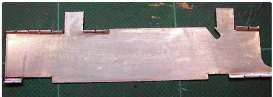
Flat panel with hinges formed over a piano wire pin
