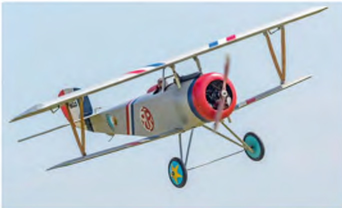
Steve Kasch's Nieuport 17 has an 80" wingspan, with a CRRC 26 cc petrol engine up front
