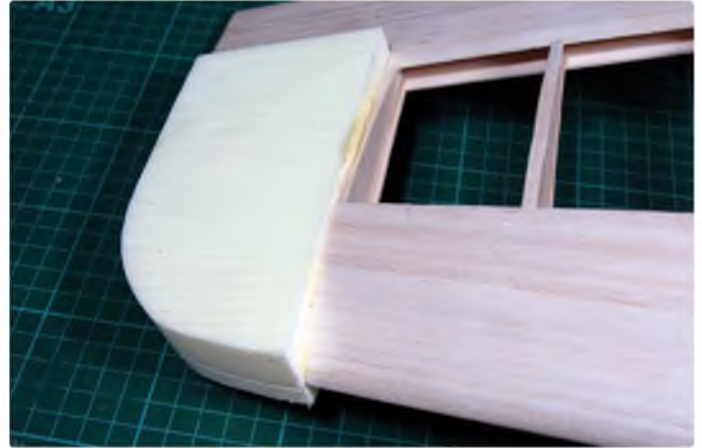
Wingtips can be made from a wooden core and foam sandwich
