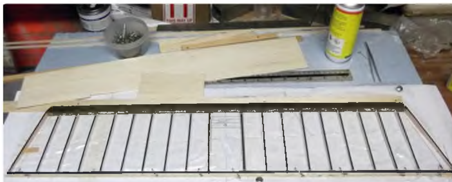
Tailplane construction on Gary Peck's eSoarer is much the same as the wing described last time but the D-box leading edge is much smaller
