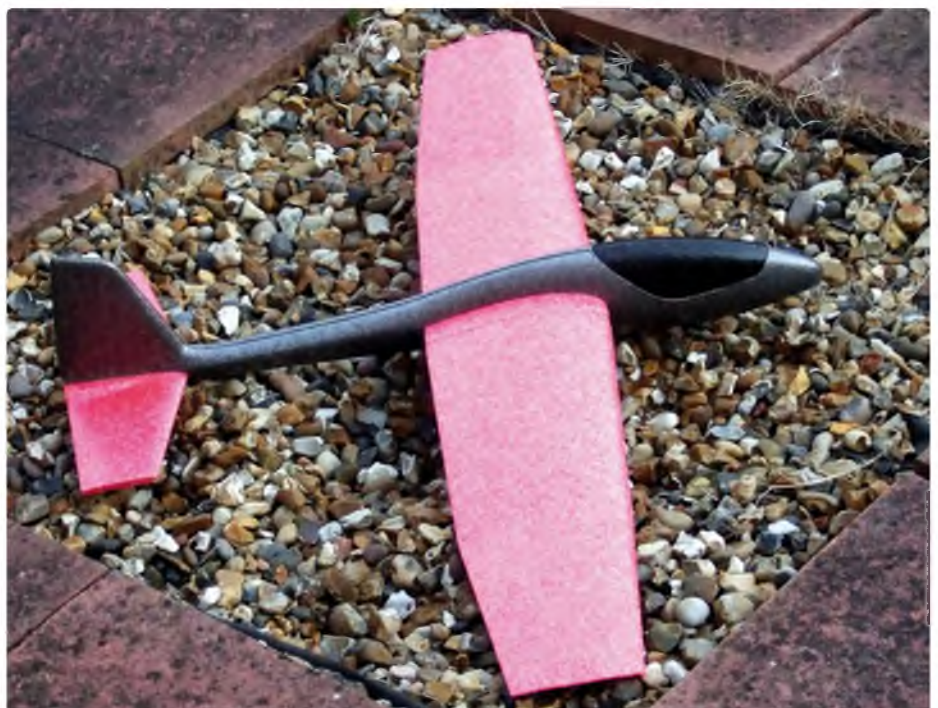
Unexpected item in the bagging area! The Playtive 'XL Glider' is available from some Lidl supermarkets. 34" wingspan, moulded in EPP, the model is sold for F/F but it's already proving popular for R/C conversion (Photo by Nick and Robert Simmonds - now that's what I call a spot-landing!)
