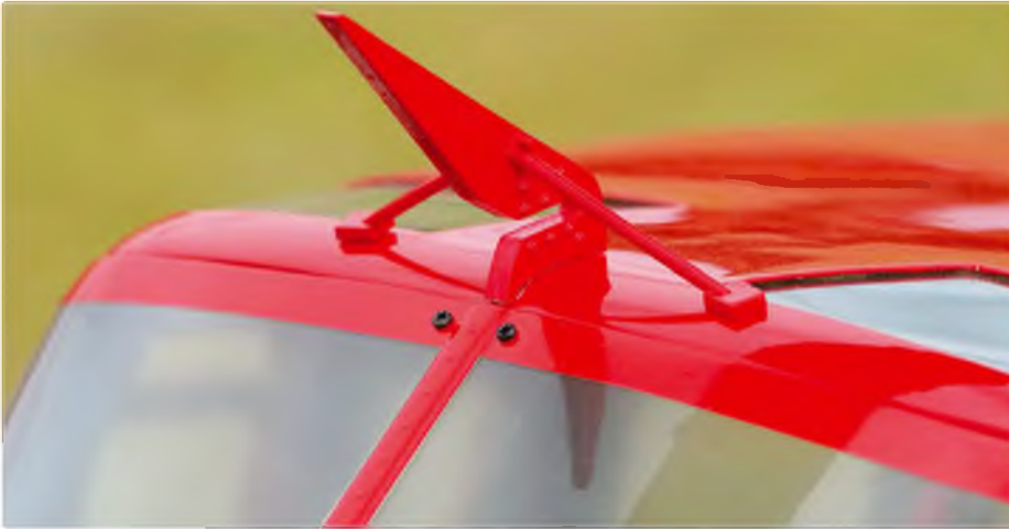
The cabin top 'wire-cutter' is well simulated and far less vulnerable than its lower mounted counterpart, which I've had to glue back on several times due to workshop incidents
