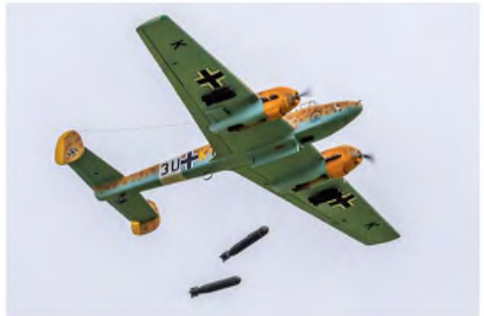
Tony Hooper's Messerschmitt Bf 110 was built from the Chris Gold plan (Traplet Shop, MW3489). The model has two AXI 4130/20 electric motors and features dropping bombs and a Benedini sound system for the realistic sound of the Daimler Benz engines
