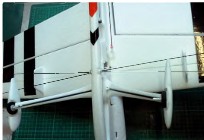
Underside view showing the main plane bracing
