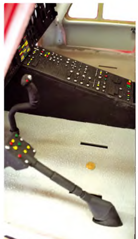
A view of the central instrument console prior to fitting the pilot and co-pilot seats
