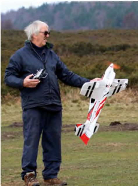
Preparing for a vertical take-off, Josh supports the Sbach until the thrust matches the model's weight...
