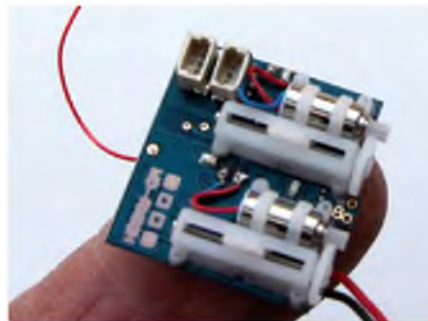
The HK Rx/module is nicely small but also needs a motor lead to be soldered to the board. This unit may not work easily for you unless you have a 'channel assign' function on your Tx
