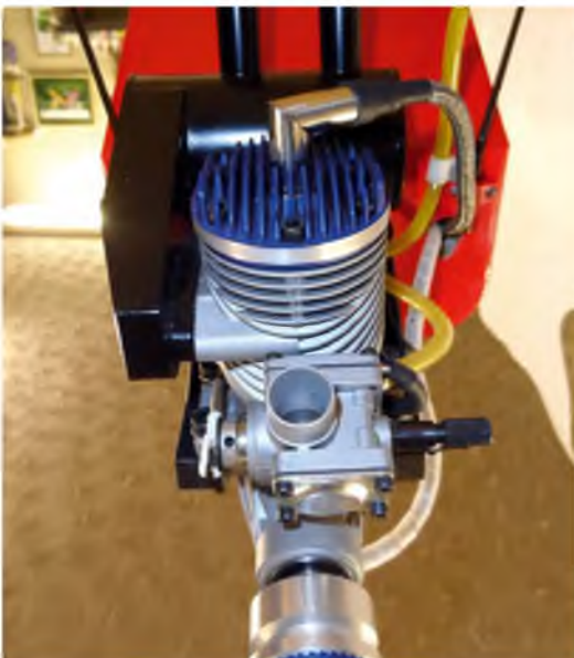
Left above & below: New engine installation based on the Evolution 20GX
