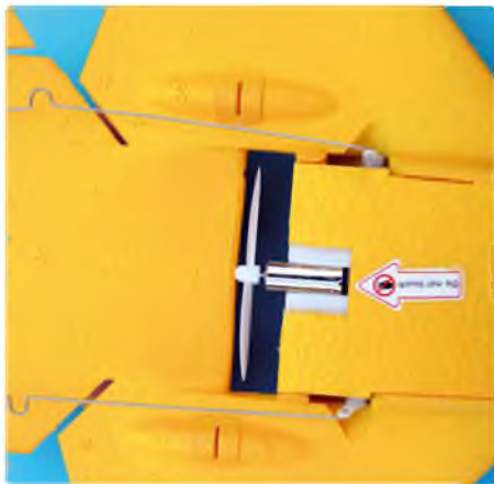
The pusher motor has an important 'do not touch' warning notice!
