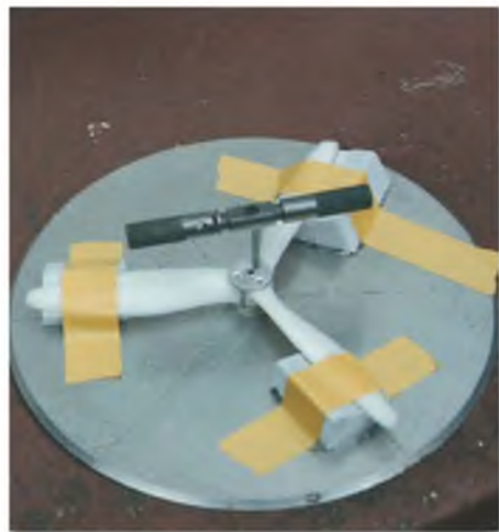
Building the pusher props
