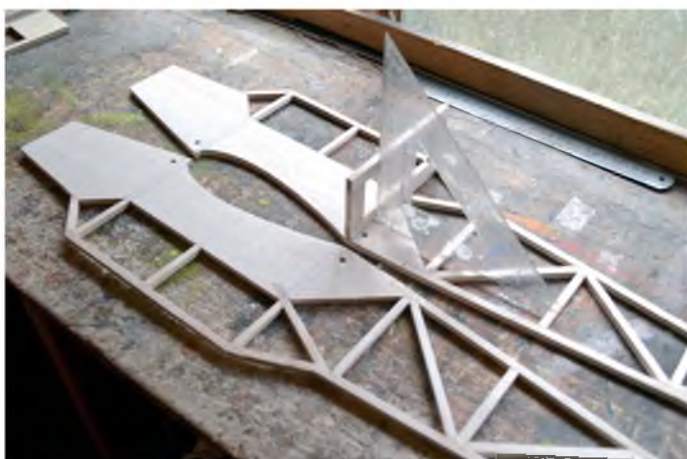
Ensure the formers are glued in square
