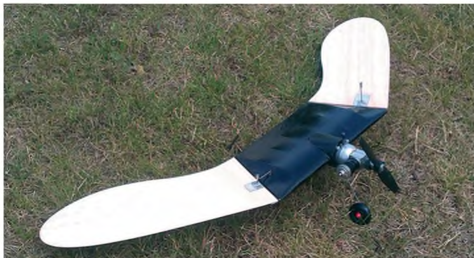
Easily the best hybrid control liner/ornithopter we've ever featured. Well, yes, it's also the only one... Simon Roger's bizarre 'Flapalong' from 1951 uses its articulated wingtips for elevator control. (Eh? - See text)
