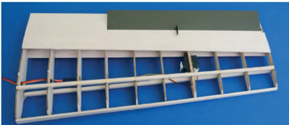
To avoid frustration the ailerons and wing recesses can be covered and finished before the ailerons are permanently attached to the wing
