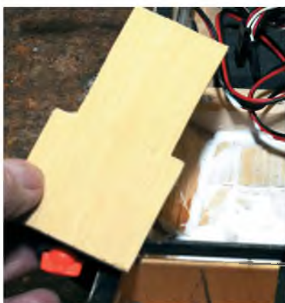
Shaped plywood 'floor doubler' about to be placed onto the damaged fuselage. It was fixed with white glue and clamped firmly in place
