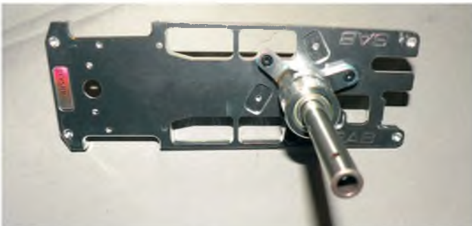
Here we see the main shaft located in place and its support attached to the main mechanics plate. Note the serial number on the plate
