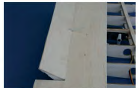
When the aileron is deflected up the area in front of the hinge point dips down into the wing, giving a smooth airflow over the control surface
