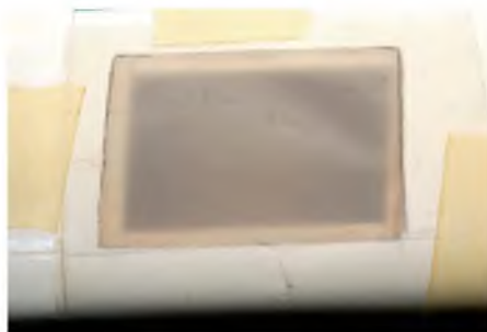
Damaged wood was removed from the wing and tracing paper was placed over the hole to obtain its shape. The replacement balsa panel was made from the tracing
