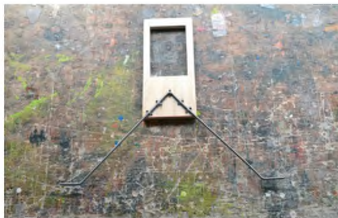
Undercarriage securely sewn and glued to former F2
