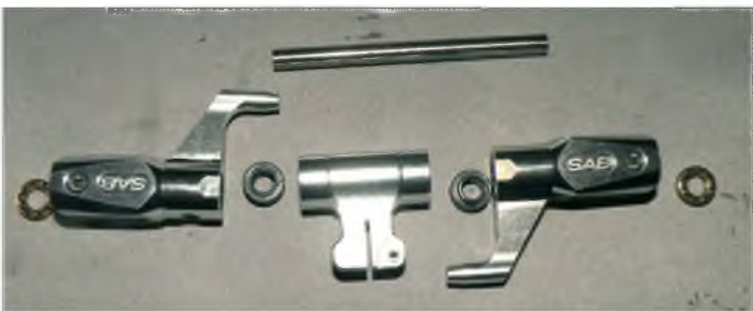
The metal blade grips are fixed to the feathering spindle, which passes through the metal rotor head hub
