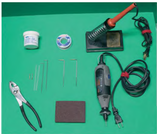
Supplies and tools needed to make a pair of torque rods (from left; top row): solder flux, acid-core solder and a soldering iron. Middle row (from left): brass tubing (about 1"), music wire, plastic tubing, a pair of almost completed torque rods, plus a drill and bit. Bottom row (from left): strong pliers and fine grit sandpaper. Not shown is a music wire cutter
