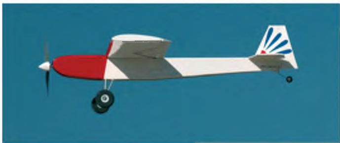
Senior Sassy's bones are all balsa, ply and Lite-Ply, all easily covered in Profilm
