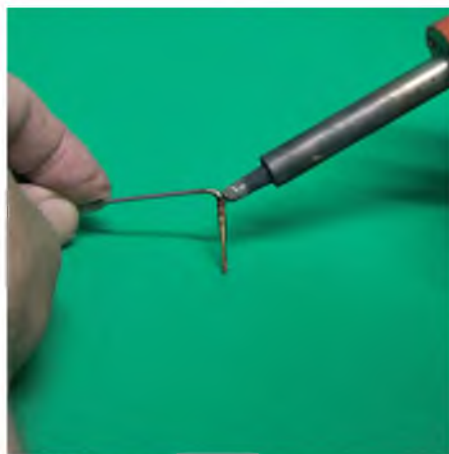
Use sandpaper to clean the short end of the bent music wire, and then add flux and tin with acid-core solder. Slide the tubing over the wire (you'll probably have to heat it) and solder it in place. Make sure the flattened bit of the tubing is perpendicular to the long axis of the music wire! When cooled, rinse with tap water to remove excess acid
