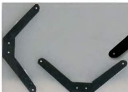
Wing ribs are an interference fit over the spars and can be cyanoed in place when they are vertical
