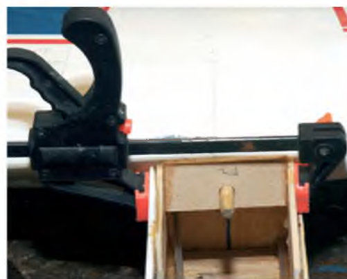
New wing retaining plate, glued and clamped in place, with the wing in situ to ensure correct alignment
