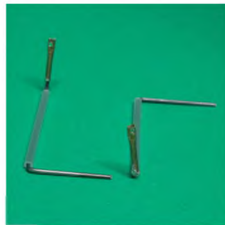
Slide on the plastic tubing, then bend the wire and cut off excess. Double check before you bend the second torque rod, to ensure you make a right and a left side! Unless you plan to add differential movement to your ailerons, make sure all the bends in the 1/16" music wire are as close to 90 degrees as you can make them
