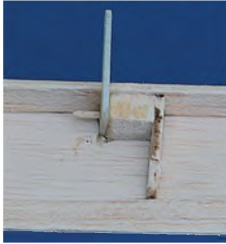
Balsa blocks are used to support the control horns
