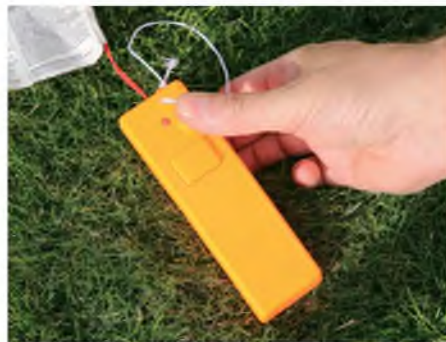
The launch controller has two buttons. This photo shows a thumb pressing down the removable safety button/key. The second button (in the middle) is then pressed to launch the rocket
