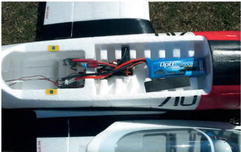
Cavernous battery bay allows for plenty of experimentation with different battery packs
