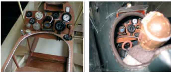
Instrument dials are photos of the real thing, printed on glossy photo paper then sandwiched between discs of thin ply and acetate
