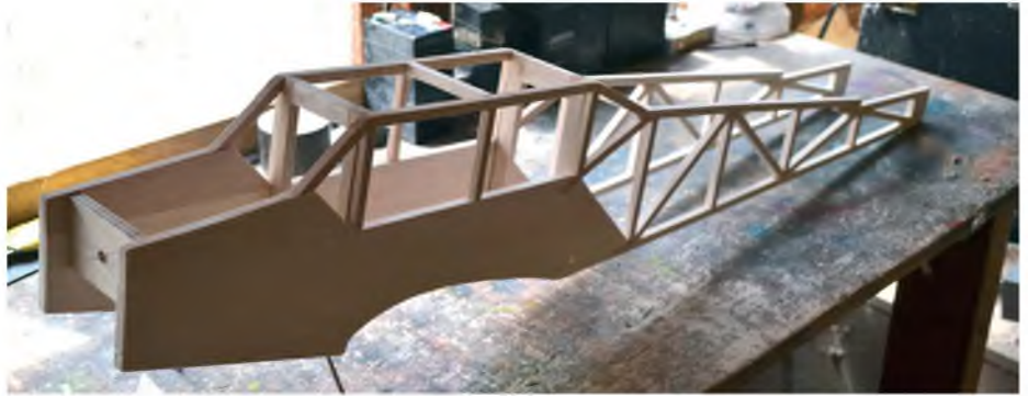
Ensure the fuselage sides are square and the fuselage is straight. Use a jig if you have one
