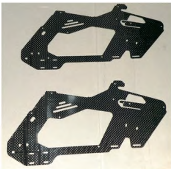
The first stage is removing any sharp edges from the carbon side frames
