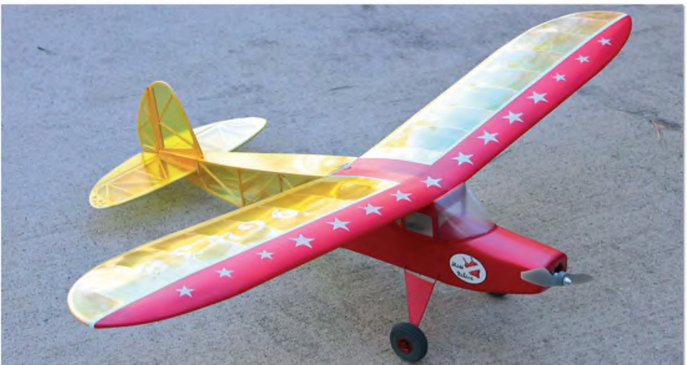
Above & below: Miss Bikini boasts a large amount of dihedral, which makes her more stable during those long gliding flights as she seeks thermals. Since she has no ailerons the dihedral has to work with her rudder for turning
