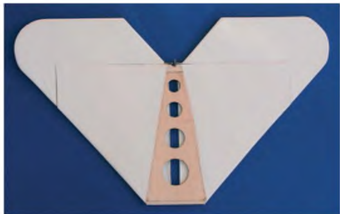
Make sure that none of the bits that will be glued have any covering near them. Here you can see that the tailplane mount is left as bare wood
