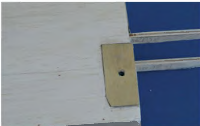
Ply is recessed into the covering over the wing mounts to give durability to the model
