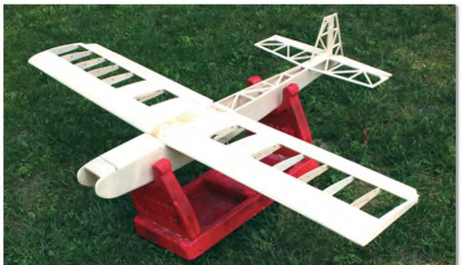
Senior Sassy's bare bones, ready to cover and with the control surfaces masking taped in place. Before you ask... No, Robart stands don't come in red. I repainted mine as bare balsa doesn't show up well against the white foam
