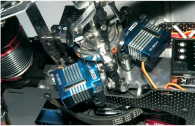
Arranged around the rotor head are the three cyclic servos operating the metal swash-plate
