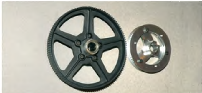
The main and tail front pulleys are fitted to the main shaft and contain the autorotation unit
