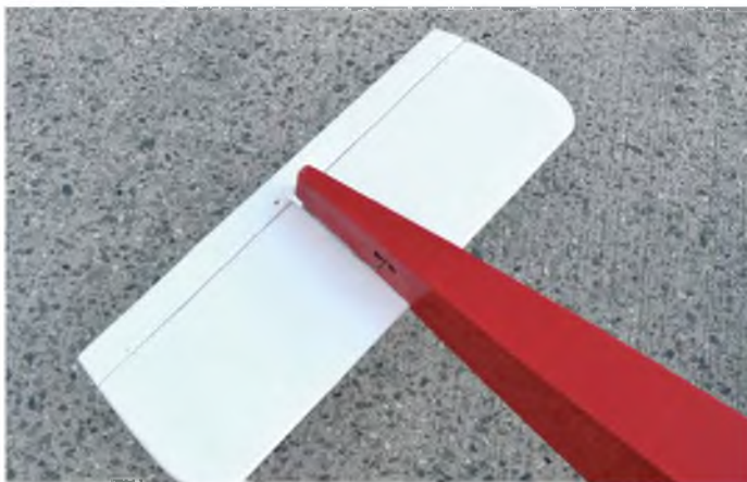
Elevator pushrod exits out the side of the fuselage
