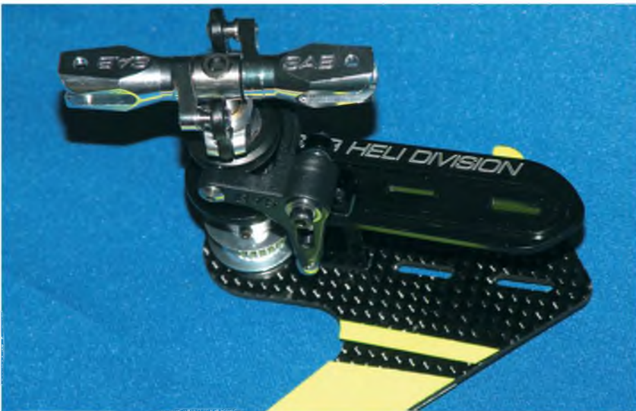
The tail assembly is quite conventional, being belt driven through a carbon fibre boom
