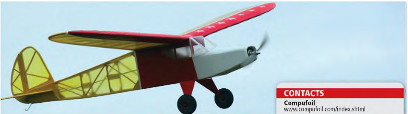
Above & below: Miss Bikini boasts a large amount of dihedral, which makes her more stable during those long gliding flights as she seeks thermals. Since she has no ailerons the dihedral has to work with her rudder for turning
