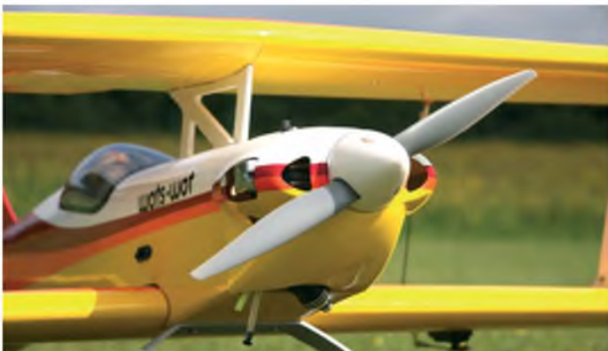
Cowl fitted to engine after cutting to clear the cylinder head, needle valve, exhaust header and silencer. Final installation looks quite neat
