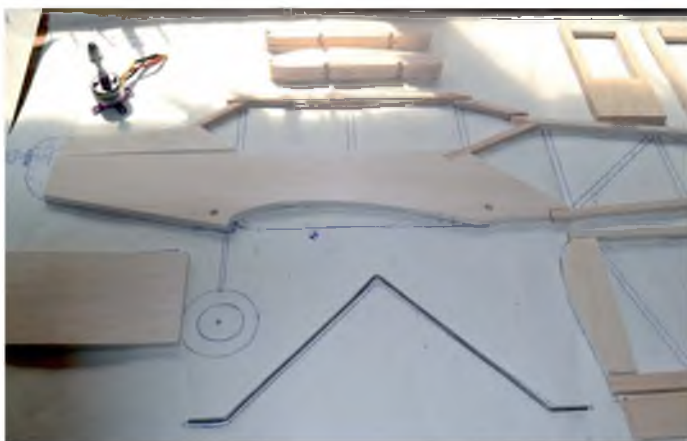
Choose light balsa wood for the aft fuselage and tail feathers
