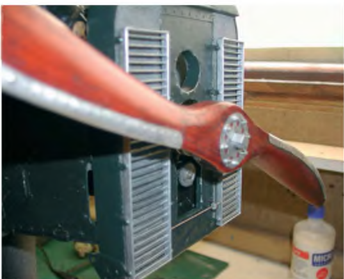
The cog on the synchro pump mechanism just below the propeller hub acts as a disguised radio switch
