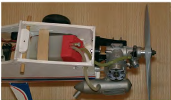
Clean the tank before reinstalling the fuel system
