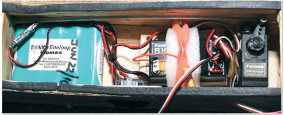
Replacement receiver and battery. The throttle servo was replaced. The rudder and elevator servos are located in the rear of the fuselage and were undamaged
