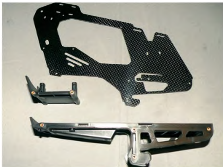
Here we have the battery tray tail servo support and a side frame ready to be assembled
