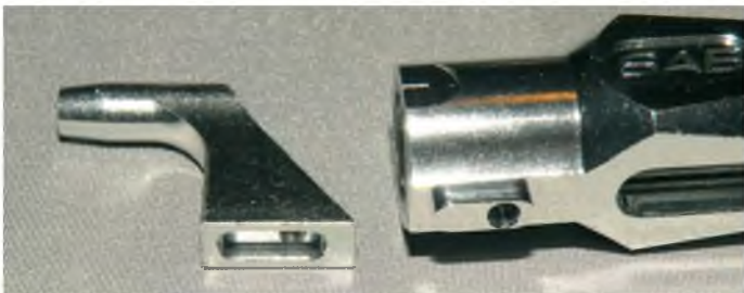
Each blade grip is made up of two parts held together by a single bolt and a tenon joint
