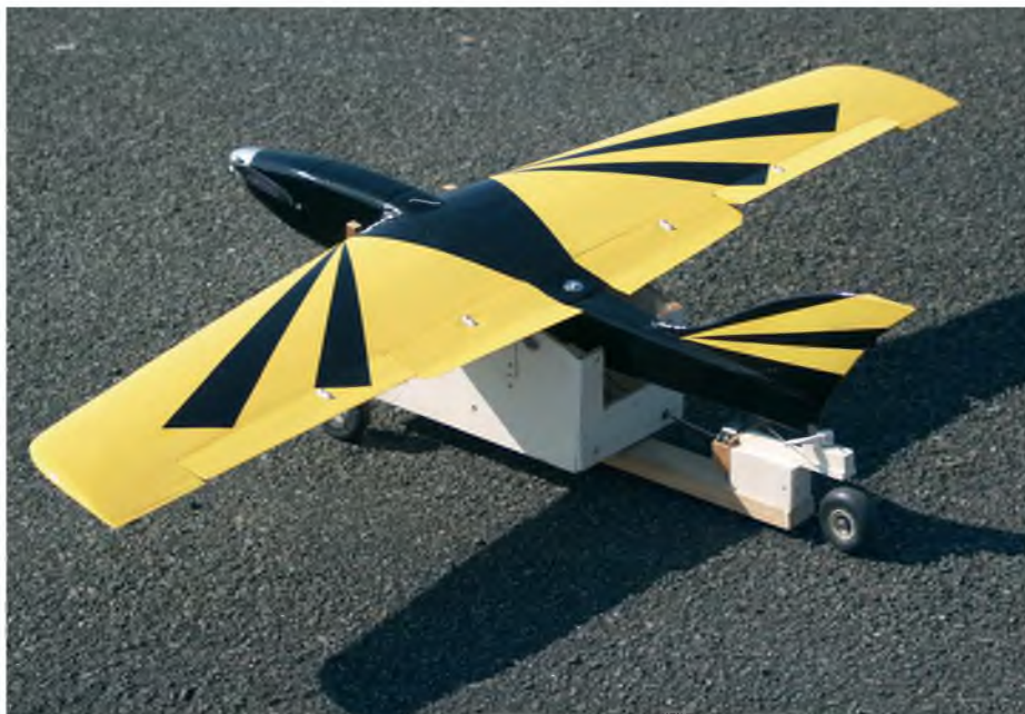
Mike White's 'Pipedream', a fast aerobatic wing and new out of the workshop. Power from a Turnigy 3536/8, 1000 KV, 9" x 6" prop, 4S, drawing 33 amps/410 watts output. Weight 2 lb 12 oz. Flies from this dolly, which has its own Rx and steers off the model's rudder channel
