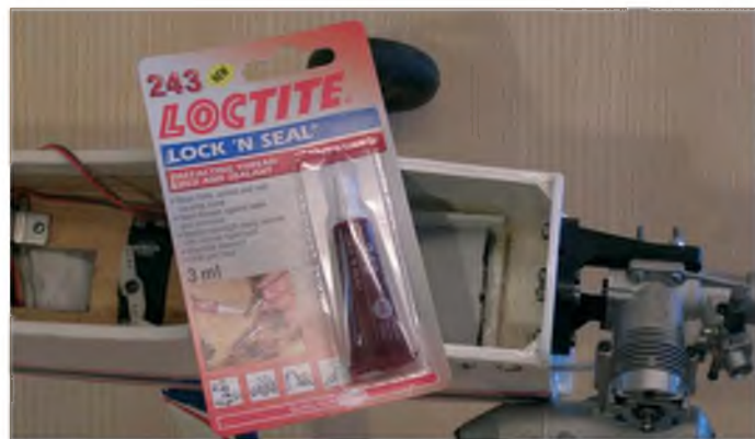
Use thread sealant on mounting bolts or use locking nuts
