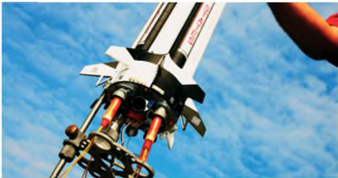
Zika Josipovic (SRB) displays his Saturn 1B, serial number SA-205. Note the cluster of motors employed at the base, which splits during the boost to launch the second stage. This model employs contemporary composite construction
