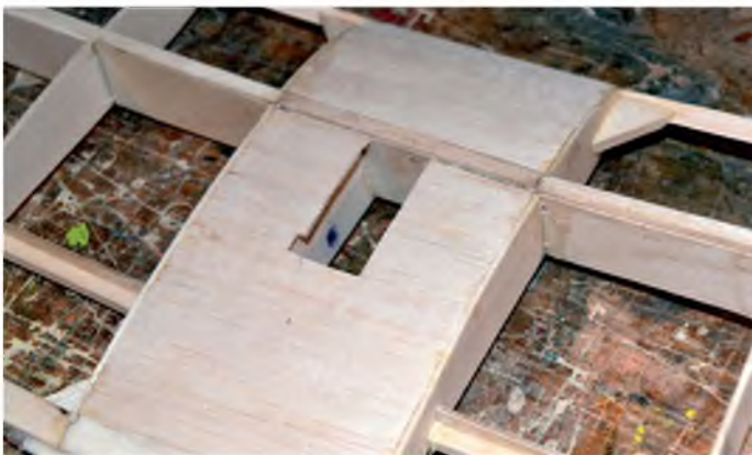
Cut a hole in the wing top sheeting to fit the size of your aileron servo
