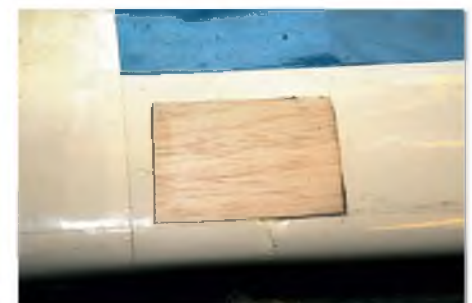
Damaged wood was removed from the wing and tracing paper was placed over the hole to obtain its shape. The replacement balsa panel was made from the tracing
