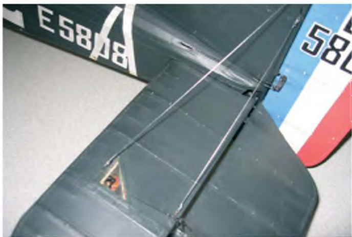
Bracing wires from the adjuster attach to the trailing edge and alter the incidence as the adjusting bolt is screwed in or out
