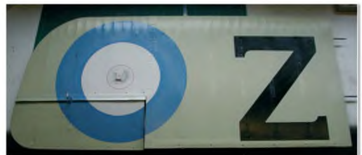
A small piece of Lite-Ply taped to the wing at the centre position protects the covering and makes a positive location for the trammel
