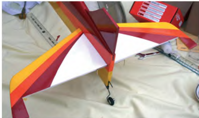
Tailplane and vertical stabiliser glued in place. The elevator joiner and tail wheel have to be fitted before fitting the corresponding control surfaces
