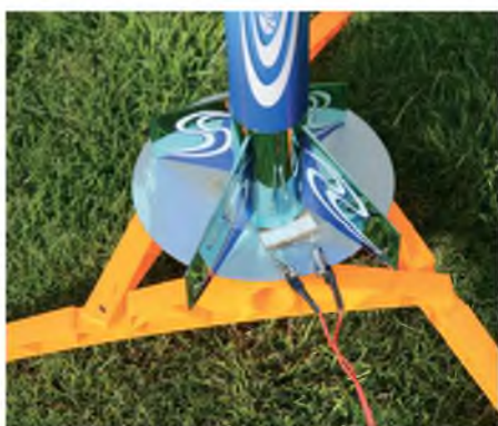
Electrical leads with crocodile clips attach to the igniter wires
