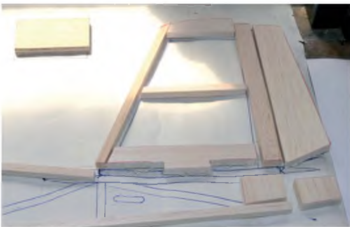
Tailplane and rudder are built in a similar fashion. Use light balsa
