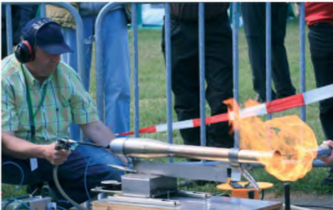
Hubert Leubner starting one of his own new engines in the test area – always an entertaining time for onlookers, with plenty of noise and flames as the settings are optimised and a new valve is broken in. If you cross Hubert's palm with Euros, he'll build you an engine too!
