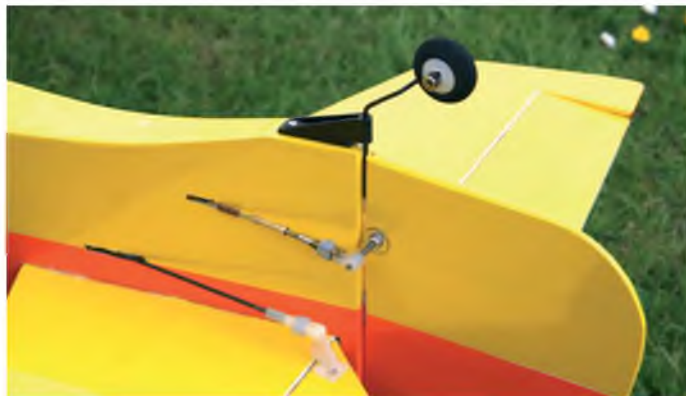
Standard control horns are used for the elevator and ailerons. The rudder uses a closed loop control system
