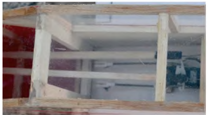
Use suitable fittings to link the aileron servo to the threaded torque rod ends
