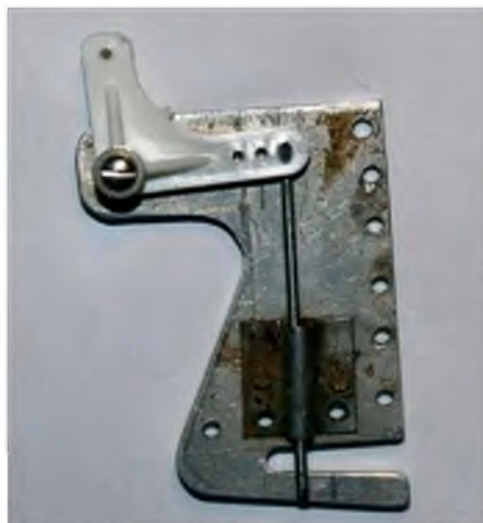
A piece of true aeromodelling/engineering. Mike White's homebrewed releasable towhook, developed from the late 1960s and flown on-board soarers under 'challenging' conditions
