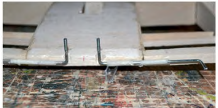
Torque rod tube wrapped in masking tape and glued to trailing edge
