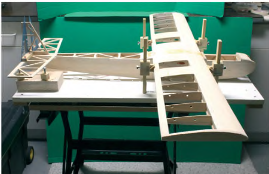
No matter how you do it, keeping the tail feathers straight with the wing solves most trimming issues before the model gets to the field. Here, Senior Sassy sits in the Frankenjig, as the slow cure epoxy and microballoons perform their magic
