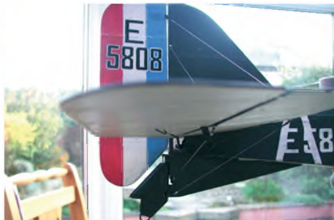
The elevators also use a cable and pulley system
