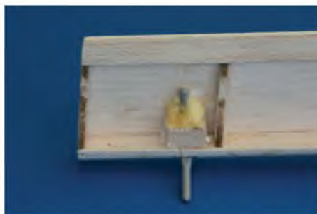
During trial fitting the barbs of the hinge will rip away at the surrounding wood. A blob of Gorilla Glue locks the hinge securely in place when you are happy with its final position
