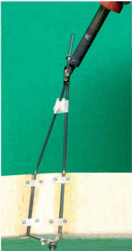
It's easiest to solder the main gear together when it is temporarily installed on the plane. Use a bit of masking tape to tack the struts together and then wrap the joint with a length of thin copper wire before soldering. Please use acid-core solder for this and save the rosin-core for electronic soldering. But make sure you give the joint a good water rinse after soldering to clean off the excess acid!
