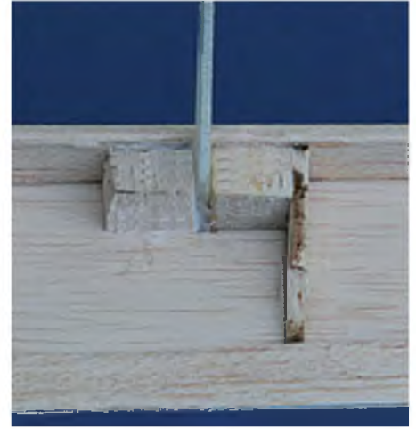
Balsa blocks are used to support the control horns
