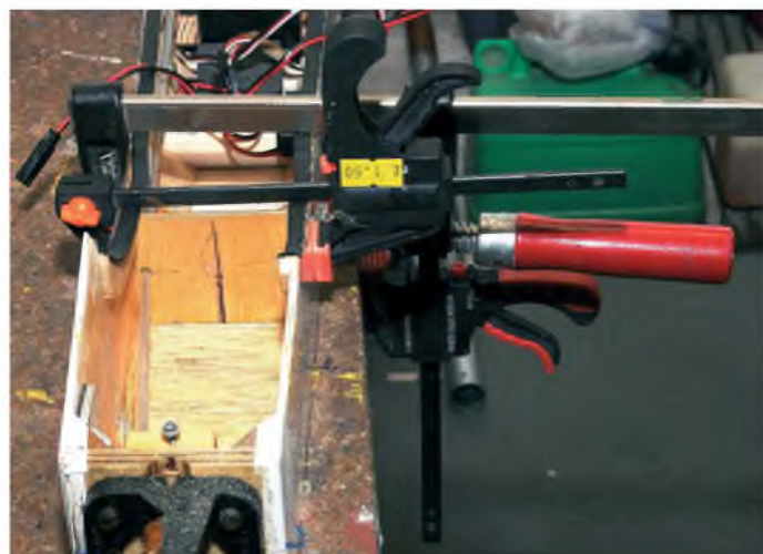
Fuselage sides clamped together to original bulkhead
