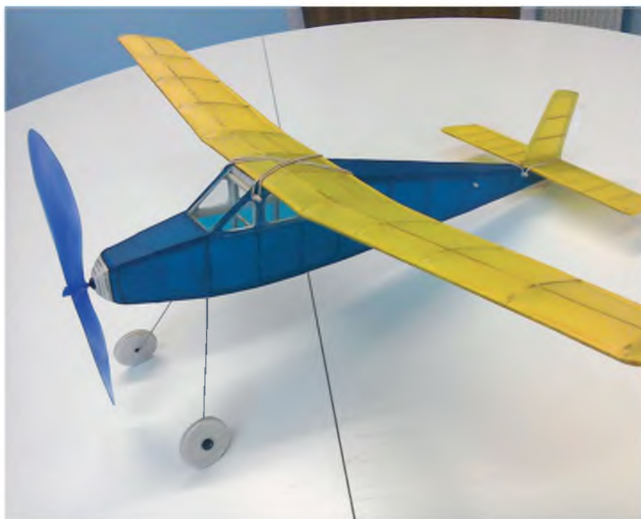
Successful first venture into all things 'stick and tissue' by John Chapman. 20" span 'Sparrowhawk' rubber sport design is by The Vintage Model Company, who do 'real aeromodelling' extremely well. Check them out!
