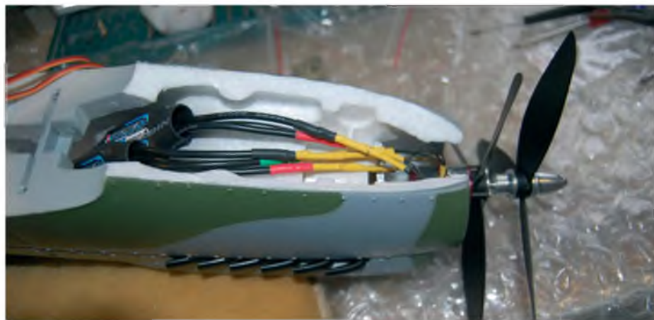
Contra motor installed in the Spitfire. The cooling duct was removed to fit the controllers and then glued back on afterwards
