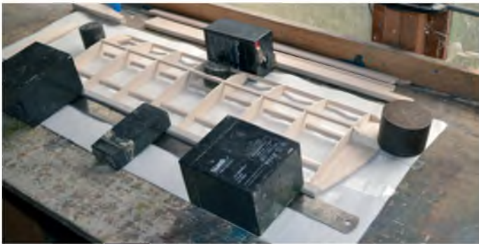
Weights are used to ensure the wing is built flat on the board
