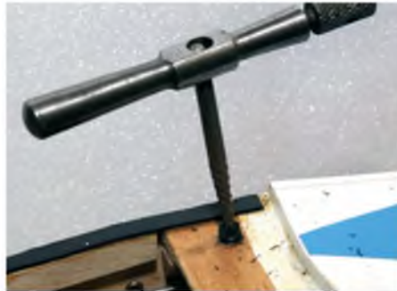
Removing a sheared bolt with the Easy Outs
