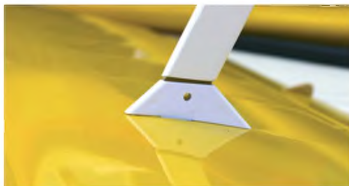
Inter-wing struts are held in place by some neat holders which are epoxied into slots in the wings
