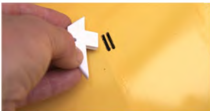
Inter-wing struts are held in place by some neat holders which are epoxied into slots in the wings
