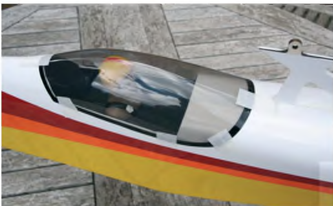
Canopy held with masking tape while the canopy glue dries. The canopy was a very good fit. Make sure the pilot is well secured!
