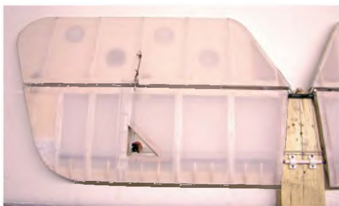
The cables run in a plastic tube in both halves of the tailplane
