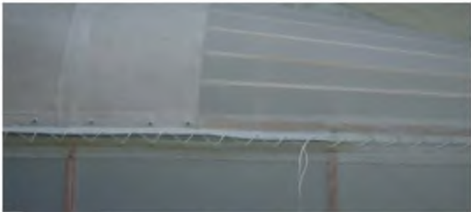
Fuselage lacing is added after the fuselage has been covered
