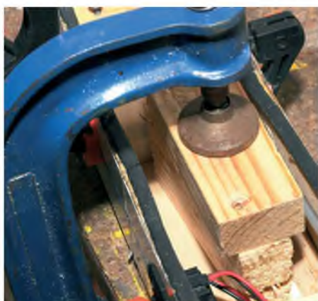
Shaped plywood 'floor doubler' about to be placed onto the damaged fuselage. It was fixed with white glue and clamped firmly in place
