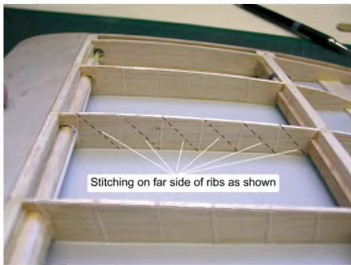
This photo shows the centre section stitching. The bottom covering and rib stitching has to be done first and is why the cotton is recessed into the ribs
