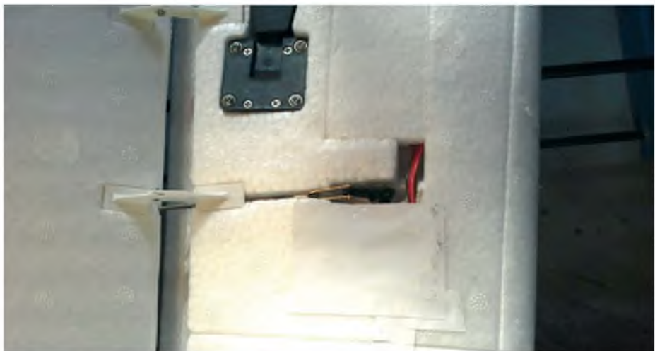
Close up on the optional flap linkage, using white film to cover the user supplied servo
