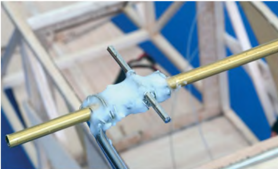
The solder will only run where there is flux so don't stint when applying it. More on silver soldering next time!
