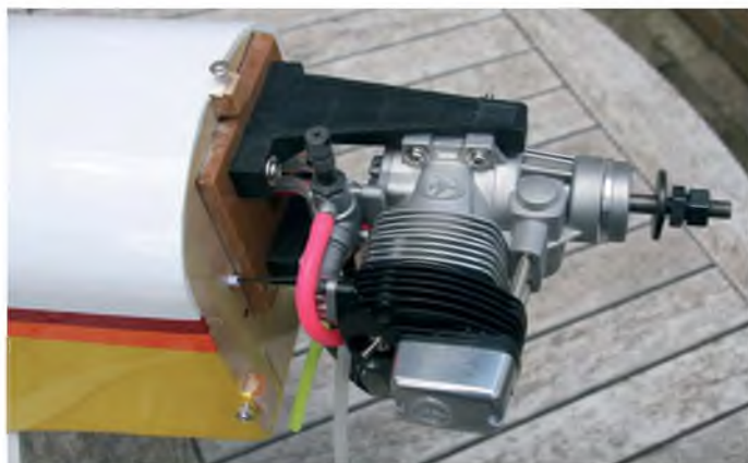
Thunder Tiger 75 four-stroke installed. The throttle control rod was raised to line up with the carb on this engine
