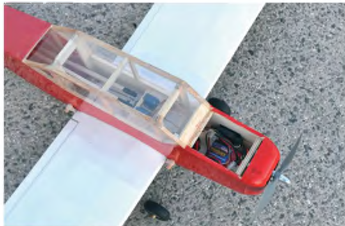
The nose compartment has room for a small LiPo
