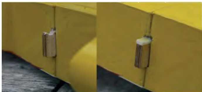
The lower wing retaining tab wore after a few flights (left), so a small fibreboard plate has been added to provide a harder wearing surface (right). If building the I/C version it's probably worth hardening the tab with cyano before the first flight
