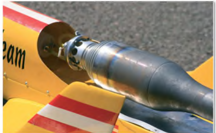
Delphinio is a very old Italian canard design that was expressly drawn around its Zanin Z23 or Z24 engine. Both Zanin and model are very reliable performers, with the former starting faster and with less effort than your average glow engine
