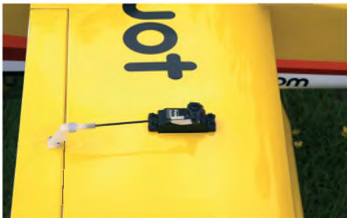
Linkages to the ailerons on the lower wing are short and direct, giving precise control
