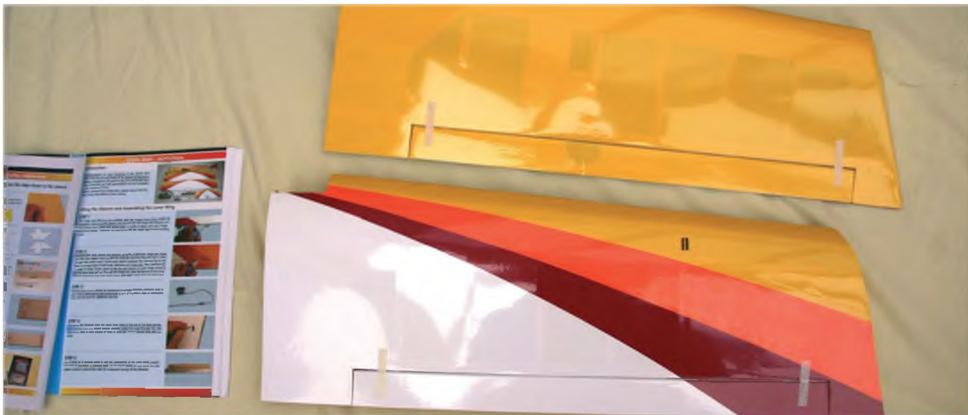
Upper and under sides of lower wings, with well illustrated instruction manual. The ailerons are taped to wing for shipping, but need to be hinged with furry type mylar hinges and cyano
