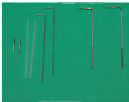
Three parts per rod: 1" brass tubes, 1/16" music wire and plastic tubing to the left, with a pair of almost ready to use rods on the right
