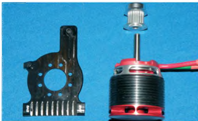
Power to drive the helicopter is provided by the Kontronik Pyro 380-09 once fitted to its mount and the pulley added
