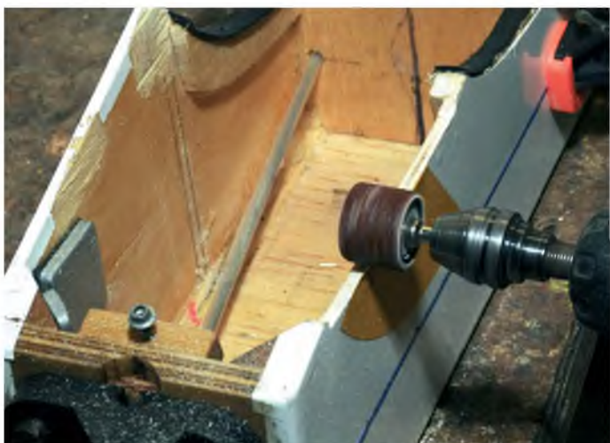
Carefully shaping the new 'doubler' on the fuselage
