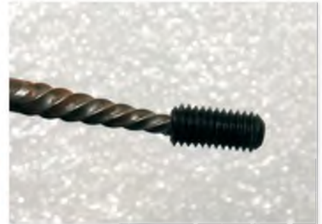
Removing a sheared bolt with the Easy Outs
