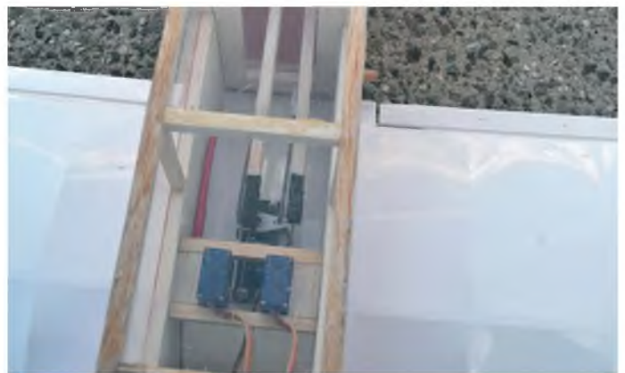
Top view looking down into the fuselage. Note inverted tail servo mounting and balsa pushrods
