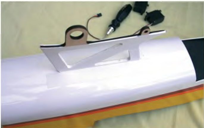
Upper wing cabane support is epoxied into a slot in the fuselage. Note use of masking tape to stop epoxy marking the fuselage
