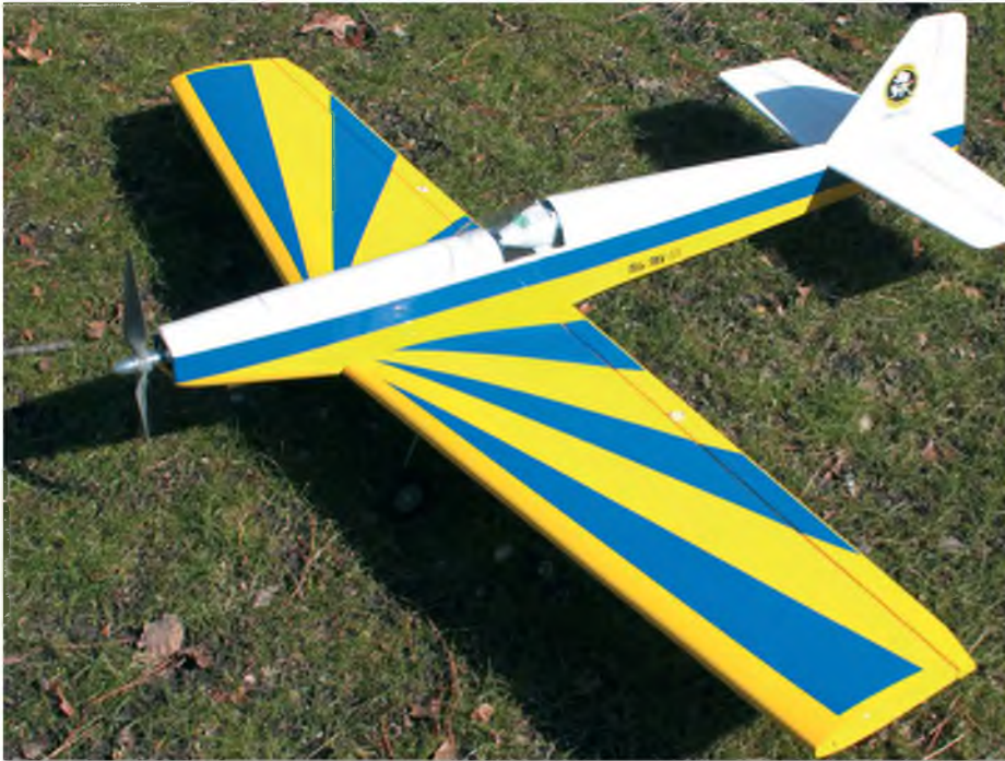
Designed for pattern-type acrobatics, the Ulu series uses a fully-symmetrical aerofoil. It flies the same upright and inverted. Wing LE sweep back takes the place of some dihedral, making the Ulu stable when both upright and inverted
