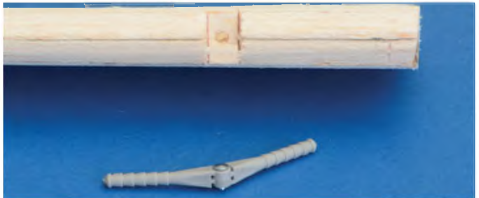
Recess the aileron leading edges to accommodate the fulcrum or bend point of the Robart hinges
