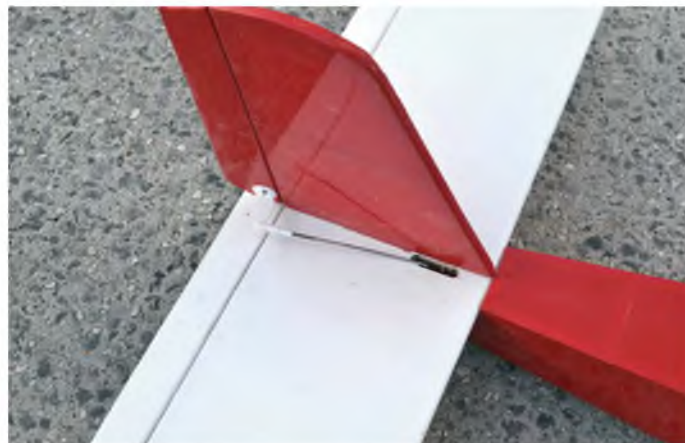
Rudder pushrod exits out the top of the tailplane
