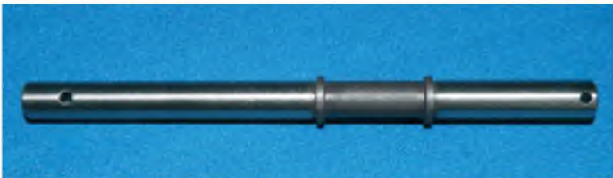
The main shaft is hollow and is located between bearings on the two larger diameters, with any free movement being taken up by shims
