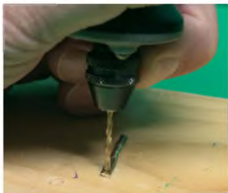
Yes, this is staged, otherwise there'd be a clamp holding down the tubing. Drill the flattened tubing for the clevis. Please, use a METAL, not a plastic clevis, otherwise the brass tubing can cut through the clevis pin! (Alternatively, put the clevis at the servo end and use a Z-bend on this end.) Either way, a scrap block under the work protects the workbench and helps keep the work being drilled from trying to run and hide under my wife's truck!
