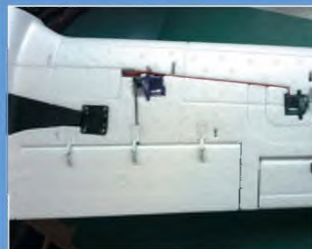
The flaps were easy to get working using the cantilever hinges supplied
