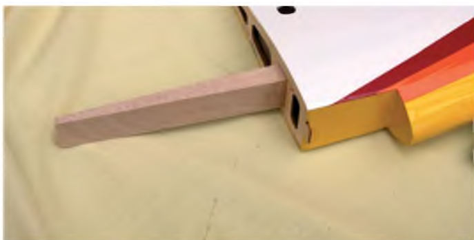
Lower wing halves are held with a substantial hardwood joiner, all epoxied together
