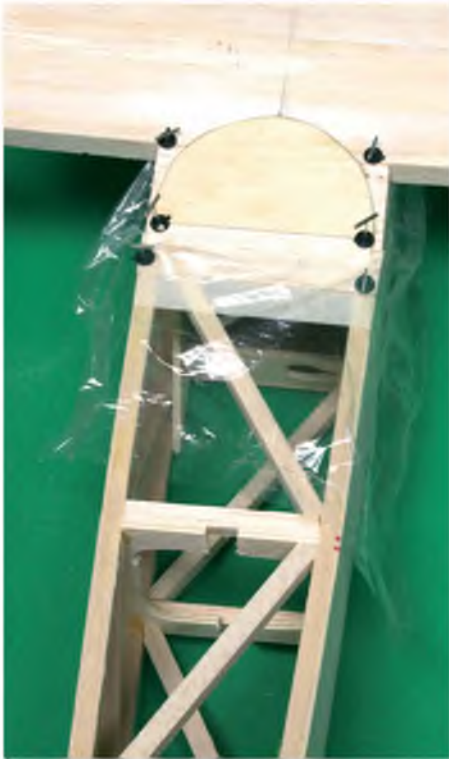
A bit of scrap behind the wing centre section TE helps fair it in, whilst sandwich wrap keeps the wing from being glued to the fuselage. One of the original, too narrow, bulkheads is visible, as are the cut through it and the reinforcement added to make up for the cut
