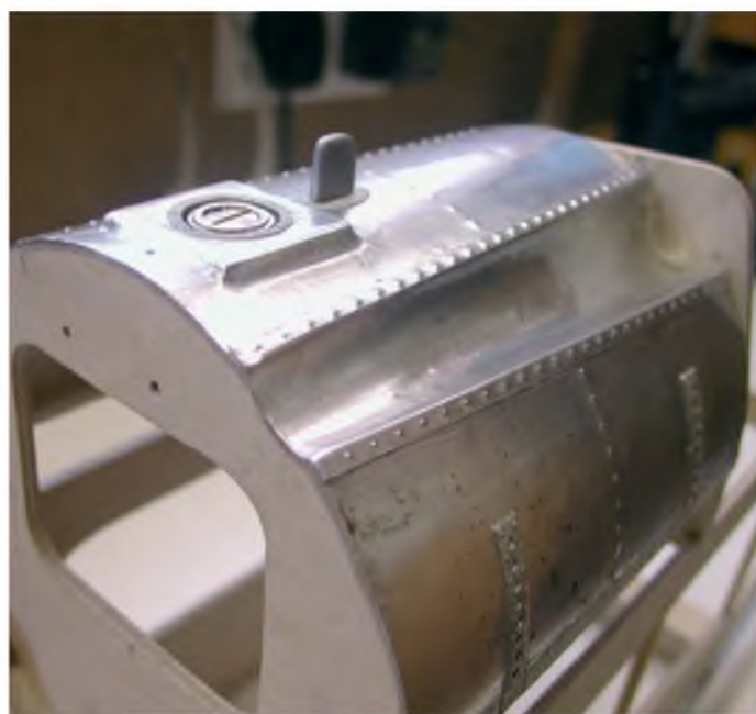
Tank cover during construction, and the finished article in place underneath the top wing
