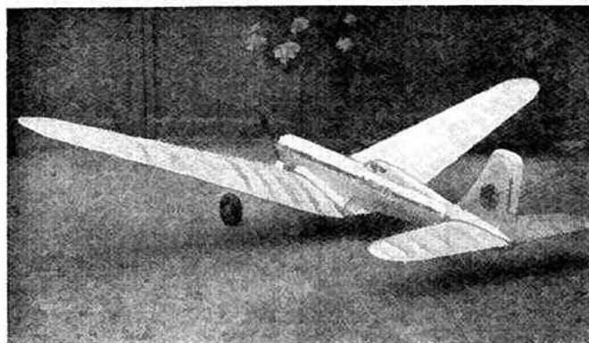
Fig. 1. Col. Bowden's low wing petrol model which, it is suggested, might suffer from wing flexing troubles.
