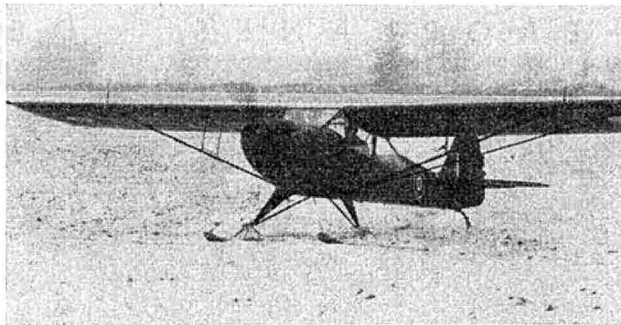
Winter Operation. First tested in France early in the War, this Auster on skis demonstrates still further the amazing versatility of this little aircraft.
