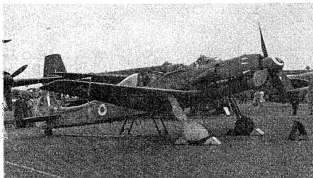
Welkin Rival. High-aspect ratio wings distinguish this Focke Wulf Ta 152 high-altitude fighter from the closely-related Fw 190D. The new designation "Ta" signifies Kurt Tank, the designer of the Fw 190 series. (A.T.P. Photo.)
