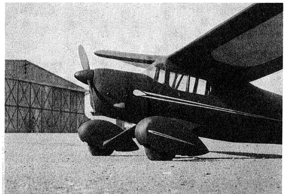
(Above) Model of the month.—A superb constructional effort by B. H. Orchard of Norbury, London, late of Southern Rhodesia, takes first place in this month's Concours d'Elegance. The model is a "Mercury II," 8 ft. span petrol model designed by Mick Smith. Powered with a Forster 99, it has gained several places in Rhodesian competitions. Too seldom do we see petrol models with this "solid" finish.
