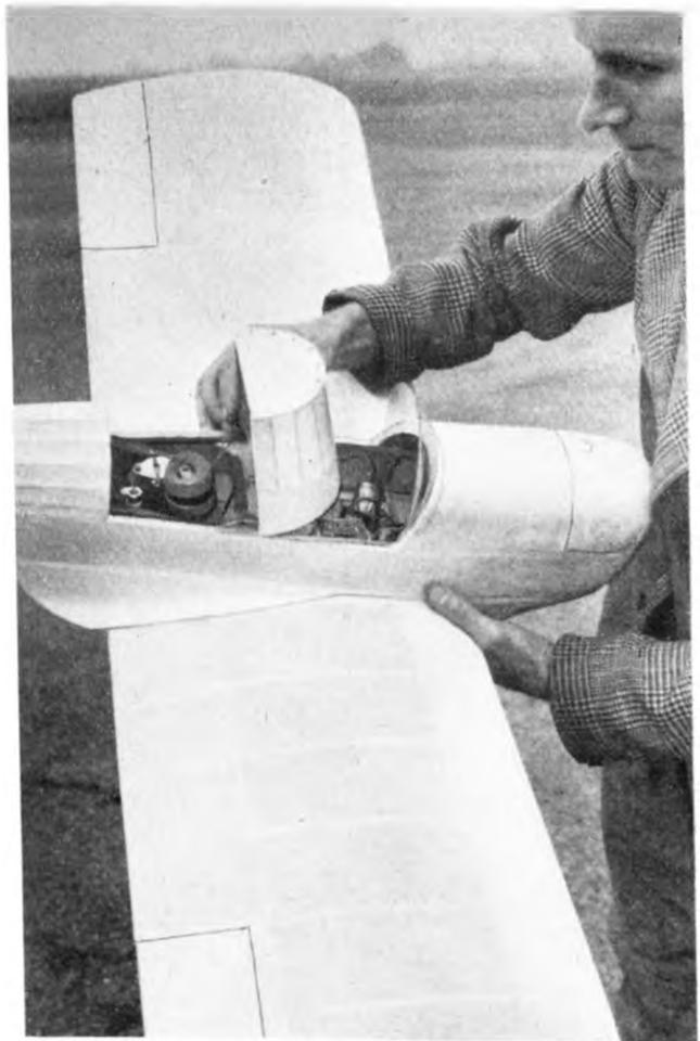
to vibrate and unwind all the turns on the rubber. This vibration is believed to be due to slight flexibility in the engine mounting as it developed after a time on the second model. The trouble has been overcome in the second model but the exact cure is not known as besides tightening up the engine mount a new control system has been installed, which does not rely on a rubber band being wound up. This system may be described in a later article.
