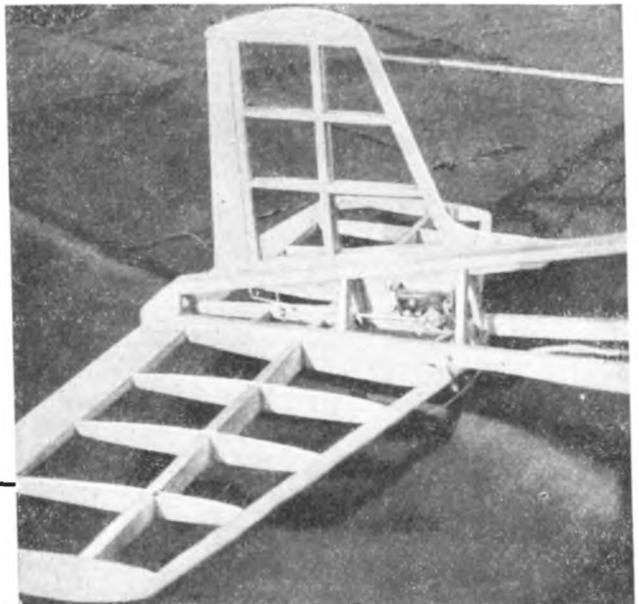
The constructional photographs on this and previous pages, together with the cut-away drawing, give an indication of the simple yet efficient design of this outstanding model. Close-up of tail unit shows installation of the magnetic actuator (Pat. No. 29978) used on the "Aeromodeller" Rudder Bug, brain child of our old friend Howard Boyd.
