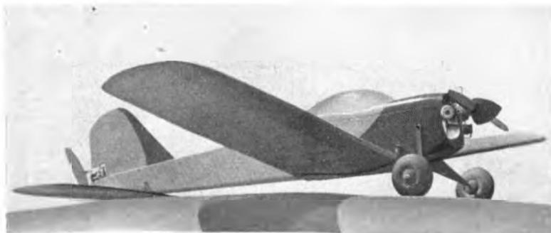
Heading photo:—Control-line Boeing P-12F built in Kansas. Power is a Vivell 35 petrol motor.
