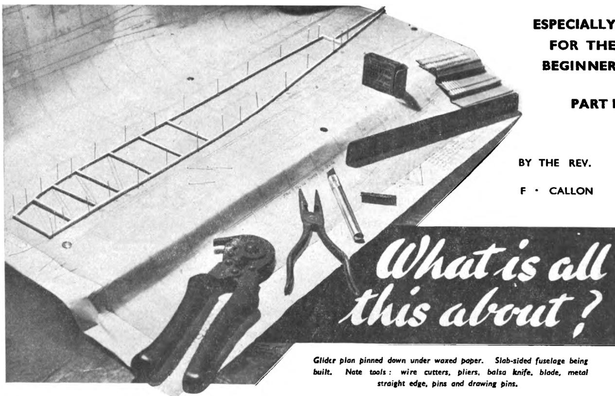
*Glider plan pinned down under waxed paper. Slab-sided fuselage being built. Note tools: wire cutters, pliers, balsa knife, blade, metal straight edge, pins and drawing pins.*
