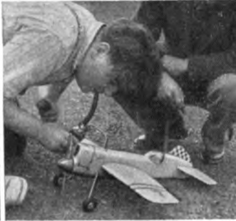
Centre: Fastest refuelling method is the air pressure system here demonstrated by Len Steward (W.E.A.) A large bore tube supplies air pressure to the fuel surface, neoprene feeds fuel to the tank.
