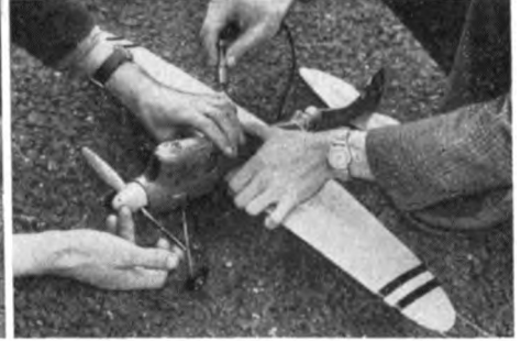
Right: An 85 m.p.h. racer by Ken Marsh known as the 'Saint' and later developed into the 'Gay Deciever', has an ETA 29. This picture shows the starting assistant in the act of connecting the 'Kurckgio' connector, whilst the starter has already refueled and is beginning to flick.
