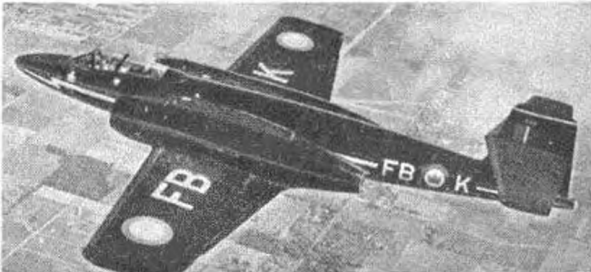
Third CF-100 built was this Mk. 2 (left) which was first to have Orenda engines, and the early shape of nose, root fairings and cockpit may be seen. First two Avon-powered prototypes (right) were glossy black overall, which contrasted with the matt rubber de-icers as seen here on the second machine.
