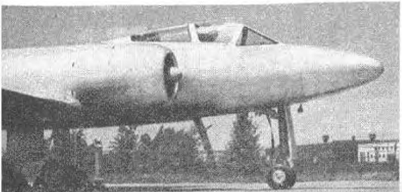
Third CF-100 built was this Mk. 2 (left) which was first to have Orenda engines, and the early shape of nose, root fairings and cockpit may be seen. First two Avon-powered prototypes (right) were glossy black overall, which contrasted with the matt rubber de-icers as seen here on the second machine.
