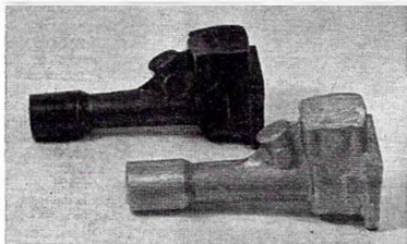
Pattern (rear) and casting (front) are for Dave's next engine, to be described at the conclusion of this series.
