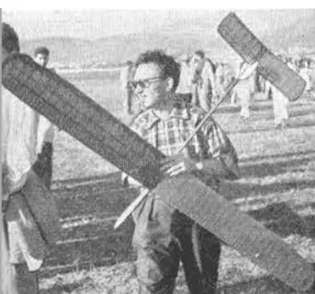
Left, is Borge Hansen of Denmark who placed fourth. Note pod type fuselage, dihedralised tailplane and close rib spacing on wing
