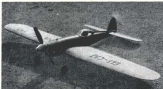
Simple yet racey lines of ElfCat make it an easy-to-build good looker with full stunt performance. Flight pattern with a 1½ c.c. diesel is fast and sippy. Flaps help to tighten the looping radius and sharpen the square turns.
