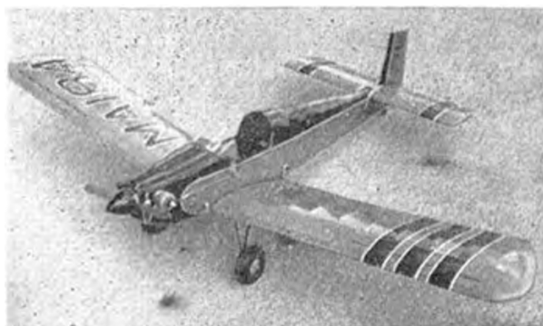
Claude McCullough of Iowa has this 6-lb. 64-in. Turbulent flying with a Min-A Rx for proportional rudder and trimmable motor, scaled from Aeromodeller plans for an Atwood .49
