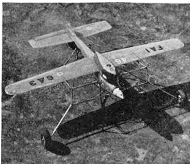
Ready for action, the Devil sits in its wire dolly. Photo opposite shows the ejector bar which trails on the ground and forces dolly from model at take-off
