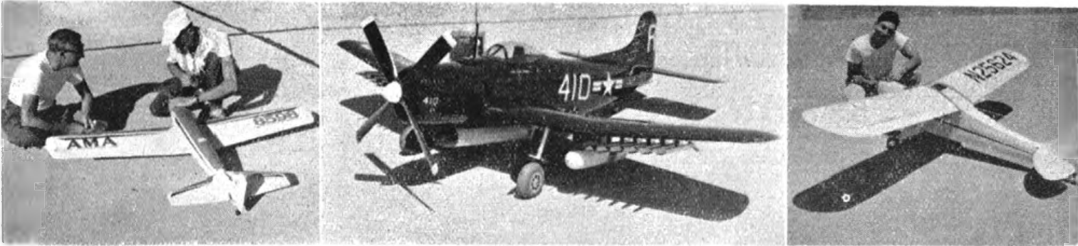
Left. Maxey Hester of Des Moines with his Orion C.G. Superhet equipment and K. & B. 45. Centre. Claude McCullough's Martin Mauler, McCoy 60 powered. Right. 9 feet span Piper Cub by Eddie Morgan. Has Orbit B channel radio, two inlined McCoy 60's, weighs 14½ lbs.
