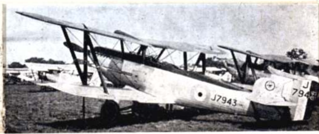
Left: Fairey Fox I which used the original Curtiss D.12 engine. (Courtesy: Real Photographs Co. Ltd.) Right: Fairey Fox of B Flight No. 12 Squadron, fitted with the Kestrel engine or F12 Rolls Royce as from January, 1929. (Air Ministry Photo)
