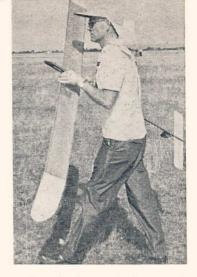
model will rise much faster, and the last trick is to lead the model round carefully into its natural circle, this helps enormously in not stalling the model off the line, with consequent loss of height.
