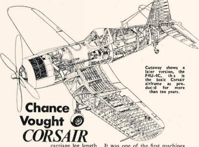
carriage leg length. It was one of the first machines to employ a spot welded skinning, and this gave the very smooth rivet free fuselage finish while fabric covering on the outer mainplanes further reduced drag.
