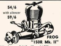
Wt. 3.1 oz. B.H.P. .15 at 14,500 r.p.m, A really "hot" 1.5 c.c. Contest engine especially suitable for ½A Team racing. Very low fuel consumption. Easy restarting for minimum "pit" time.
