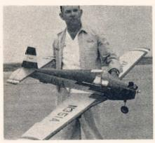
Beautiful MOONEY MITE (left), by Bud A kinson of Blue Springs, Missouri, placed 2nd in 1963 U.S. Nats using Orbit 12 and K & B 45. Weight is 9 lbs., span 74 in., extra channels used for flas, retractable undercarriage and lights!
