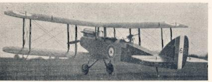
Dennis Thumpston's DE HAVILLAND 9 (above), is to 1/7th scale for Orbit 10 channel, making it 72 in. span with Veco 45. Extraordinary well detailed, complete with rigging the D.H.9 weighs 7 lbs and Dennis hopes to have it entered for the 1964 British Nats.
