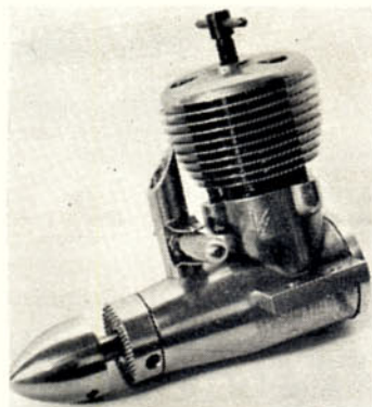
The Allouchery Eclair Cormoran and component parts at left. This attractive looking little 1 c.c. diesel weighs 2.7 oz. Right the Allouchery Eclair Komak 2.47 c.c. diesel. They claim no less than 0.5 bhp for it. Below the highly unorthodox induction system of Allouchery's "Turbold" avec compresseur. Not to be taken too seriously!
