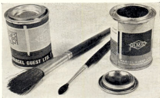
For fuel proofing use soft hair brushes of good quality as this last glossy coat will reflect every brush mark, especially loose bristles! Wash fuel proofer out of the brushes before it dries or it will ruin the brush.
