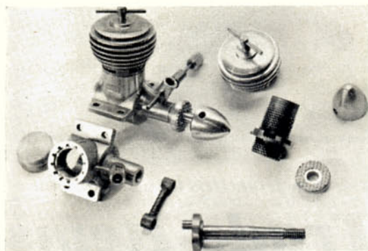
The Allouchery Eclair Cormoran and component parts at left. This attractive looking little 1 c.c. diesel weighs 2.7 oz. Right the Allouchery Eclair Komak 2.47 c.c. diesel. They claim no less than 0.5 bhp for it. Below the highly unorthodox induction system of Allouchery's "Turbold" avec compresseur. Not to be taken too seriously!
