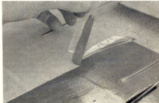
When removing masking tape never pull it straight off as shown, always double it back on itself or the paint will pull off with the tape, with some paints remove tape whilst paint is wet. Tape edge can be sealed with clear dope.
