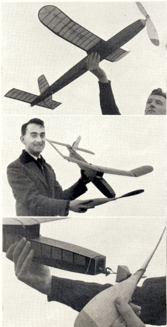
Opposite: Heading photo is of a prototype made by Erik Speakman, note different colour tissue for tip panels. Right: Top is George Swallow with his "Delinquent". Centre: Alan Platten with another, note the twin pylon wing supports and fin to one side of fuselage. Bottom, the nose block assembly of George Swallow's model, showing something of the "S" hook, the locating key on nose and the simple prop shape. Delinquent is far from being a "difficult" subject, but when flying it is definitely "wayward".
