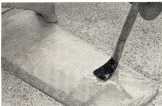
When applying the first coat of clear dope to tissue thin 50 per cent with thinners and try to flow it on rather than brush it in. Cheap brushes are suitable for clear dope application and should be stored in the dope if possible by attaching the handle to the lid.
