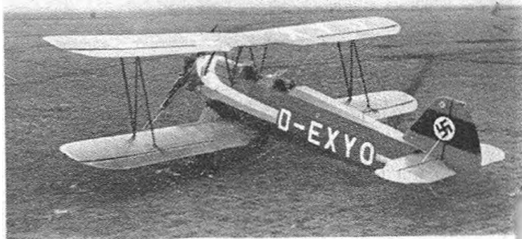
Wide gap between high aspect ratio wings, large ailerons with coarse movement, big rudder and generous elevators make the 'Stieglitz' a perfect scale subject for R/C aerobatics - if you like a biplane!
