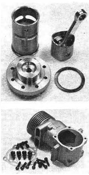
Left: The shaft assembly of the G.60R. Right: Latest Super-Tigre rotary-valve, as seen on the G.60R, features thin, hardened steel valve disc, almost perfectly balanced and running on hardened steel pin. Below: Unique piston and cylinder assembly of G.60R includes aluminium piston without rings and a brass cylinder-liner with chromed bore. Note wide squish-band on head, used in conjunction with flat crown piston. Bottom: Main casting used by G.60R, also employed by several other large Super-Tigre engines, features very big transfer passage and is robustly proportioned.
