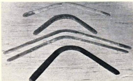
A selection of five quite different boomerangs made by the author, showing the variations in included angles and aspect ratios which have been used for experiment.
