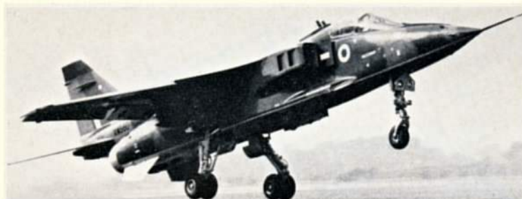
XW560, the B.A.C. built prototype, breaks ground at Walton with partial flap, and depressed leading edge. Compare with close-up photographs on previous pages for undercarriage extension, and the change of airbrake perforations, in this case four rows of six holes, later reduced to 20 holes, currently 10! Twin VHF Homer aerials behind cockpit are also an S-06 distinction. Flat base of fuselage is evident in flight shot below, where leading edge slats are drooped. Bottom left is the first Jaguar, the French E.01 two-seater.
