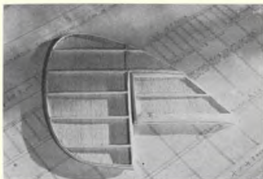
All the tail surfaces consist of a central core of \frac{1}{16} in. balsa sheet, to which are added the half ribs and balsa strip outlines either side – this results in a thin warp-free section.
