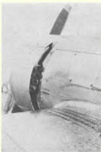
Above: Both canopies slide rearwards to provide access for the cockpits. Fully duplicated controls were fitted although the radio was operated from the front seat only.
