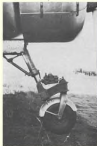
Right: Close up of front wheel reveals hydraulic shimmy damper and oleo-pneumatic shock absorber. Low pressure tyre has closely fitting alloy mudguard.
