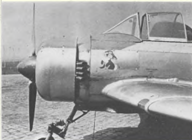
Above, short nose moment and forward cockpit position gave excellent visibility for the trainee pilot who occupied the front cockpit position. Production aircraft used constant speed, metal WR1 propellers.
