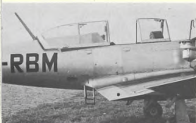
Above: Both canopies slide rearwards to provide access for the cockpits. Fully duplicated controls were fitted although the radio was operated from the front seat only.
