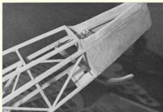
View of fuselage rear end reveals the sprung tailskid (note elastic band from top of skid to piano-wire hook) and \frac{1}{16} in. sheet balsa stiffening below tailplane mount.
