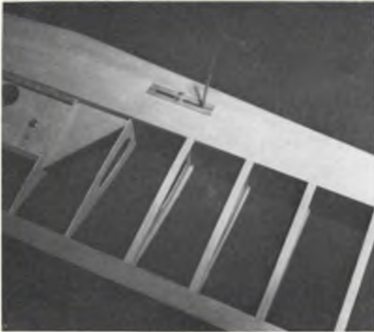
Undercarriage mounting is of the torsion bar principle, and as used on the majority of R/C models. An added advantage is that the leg may be easily replaced if necessary.
