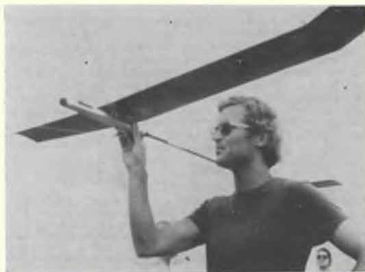
At left, time-keepers record the duration of Loffler's winning Wakefield flight – lack of drift evident! At right, Pym Ruyter holds for team-mate, Van Bragt of Holland. This glider features an aluminium nose cone, glass fibre rod fuselage.
