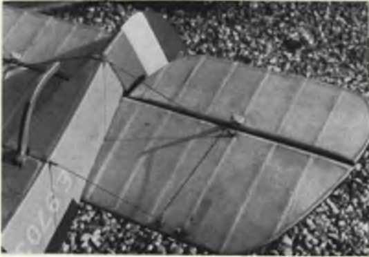
Underside of tailplane - note 22 swg bracing wires soldered to tinplate tags epoxied to framework. Rib tapes are from heavy-weight tissue doped over the silk covering.
