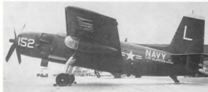
Right, Grumman Guardian AF-3S of which only 40 examples were eventually built. This machine was a modified AF-2S carrying a Magnetic Anomaly Detector boom. Photo: via Richard Hill.
