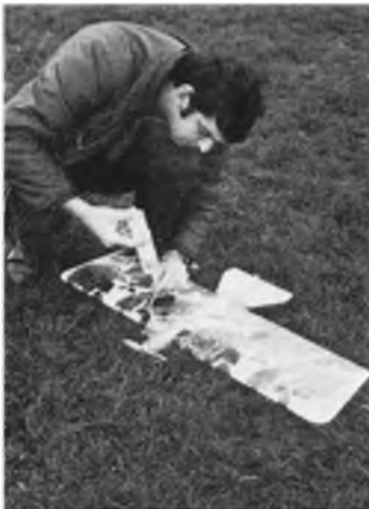
Bill Burkinshaw editor of the SMAE's 'Model Flying' newsletter performs the re-fuelling operation via a large capacity plastic syringe purchased from Michaels Models of Finchley at £1.25. It proved ideal for inflating the pacifier fuel tank.
