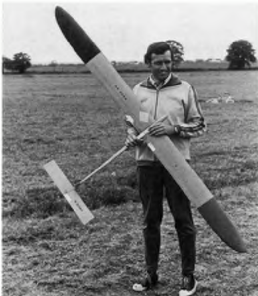
Gottfried Zach of Austria— the new A/2 glider European Champion. He uses this elliptical-tipped design with sheeted, plug-on wings — and interestingly enough, no circle towhook . . .
