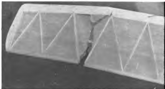
Things like fences don't co-exist too well with models. Here in addition to tissue tears, a piece of the wing leading edge has gone and is in need of the treatment drawn below.
