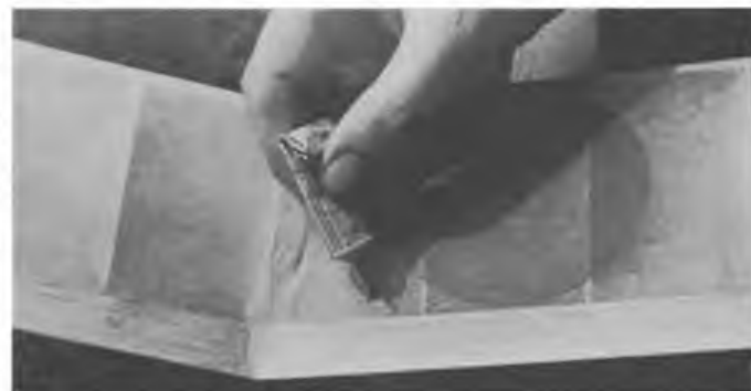
Quick repair to small tissue tears can be achieved on the flying field using balsa cement along the rear line as shown here.
