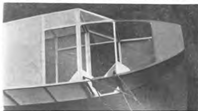
Same fuselage cleaned up, with replacement spacer gusset reinforced and ready to take new tissue covering.
