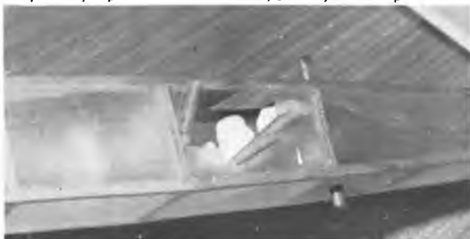
You're winding away merrily and - suddenly twang - the rubber motor has burst, usually with at least this result to tissue just ahead of the rear motor peg.
