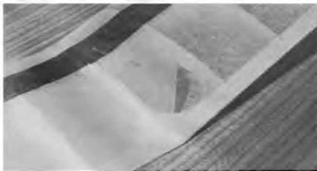
A nasty tissue tear at the wing centre section - often caused by a breaking rubber band. Usual repair is to trim out tissue and replace as demonstrated for fuselage.
