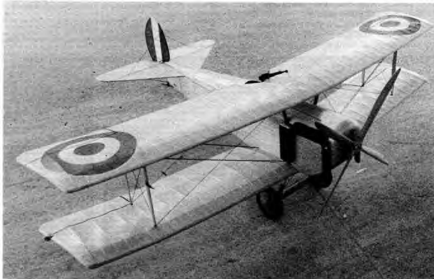
Rick Granger's Large Austin-Ball AFB 1 was Telco powered with the motor mounted on a crash resistant rubber plate. Model flew very well but lacked tank capacity for long flights.
