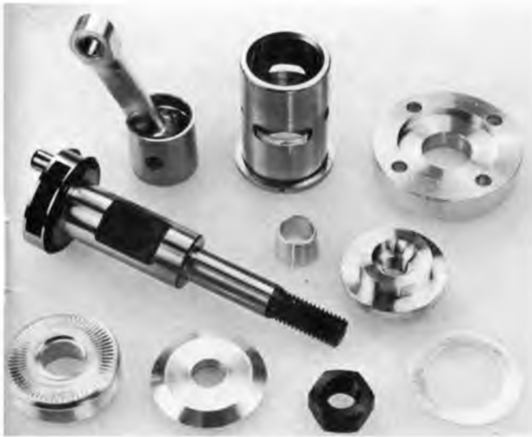
Second left: OPS 2.5-SLA is built around sturdy OPS 3.5-SLA main casting. Backplate has O-ring seal as well as gasket. Left: like all OPS motors, 2.5 features Schnuerle scavenging and ABS piston/liner assembly. Note large diameter crankshaft and two-part cylinder head.
