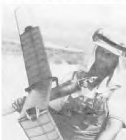
Left: gull wing breaks at dihedral intersection. Elastic band tension over carbon fibre plates opens wing.
