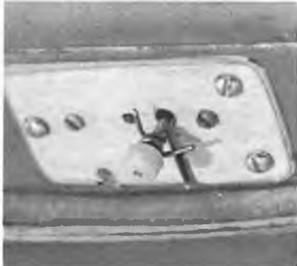
Above left: concealed timer on Lepp's A/2 uses a spiral labyrinth disc since timer rotates several times in three minutes. Notches in periphery release rudder hold arm (lower right), while D/T hold-down line is wound onto the spool at top right, locked by wire arm that moves radially across disc till released. Note audio buzzer to right of timer. Above right: Phil Ball used this Snoopy timer to operate VIT on his Wakefield, placing fourteenth. Left: Germany's Karl-Heinz Sauer used this neat chart recorder showing thermistor and anemometer traces for thermal detection. Two R/C servos drive the pens, and the electric paper drive is geared down via a Seelig timer gear train. Below: Giora Herzberg of Israel used a propeller start trigger to utilise all the first power burst. Dural arm at left holds stationary till model leaves the hand.
