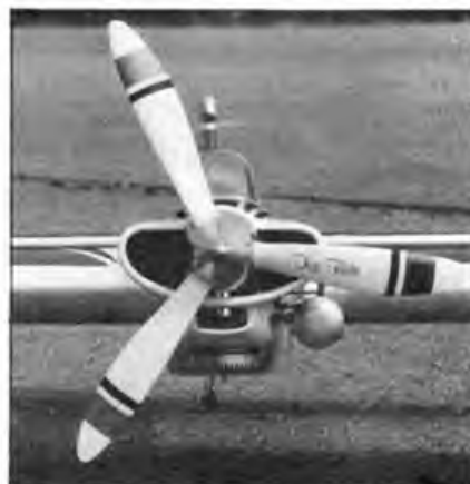
Right: this front view shows the generous air intake. Note how the engine cylinder just protrudes below the cowling.
