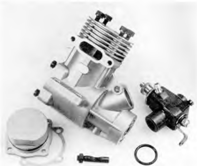
OPS 2.5-SLA in its standard or STD version with 4mm peripheral jet venturi. Note engine's substantial proportions
