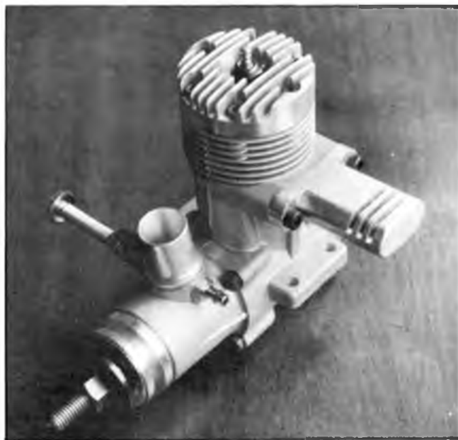
Left: OS FSR Stunt-chrome liner by Nelson Engines, Dykes ring by Vic Garner and J. H. Designs mini-silencer. Note engine has been 'turned around' from normal configuration. Below: Dion Beesley with his Sirius.
