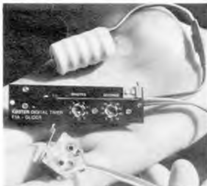
Above left: electronic timer for gliders produced by Thomas Køster, weighs 17.5 grams, rechargeable batteries weigh 17 grams. Start switch at bottom of picture can be installed in front of swinging-type towhook, timer can be set in six second steps, up to a nine minute 54 second maximum. A single charge is sufficient for about 400 timer runs. Above right: new Soviet F1C engine features integral brake and flood-off nipple. Built in Kiev, both Nakonechni and Onufrienko were involved in the design. Right: bunt mechanism of Soviet F1C model is enclosed in transparent dust cover. Below: new F1C model by Tom Køster of Denmark used a laminar flow Eppler airfoil and flaps which moved up for climb, reverting to this profile for glide. Dural foil covered wing is built in female upper and lower surface moulds, the tips consisting only of shells, with no internal structure.
