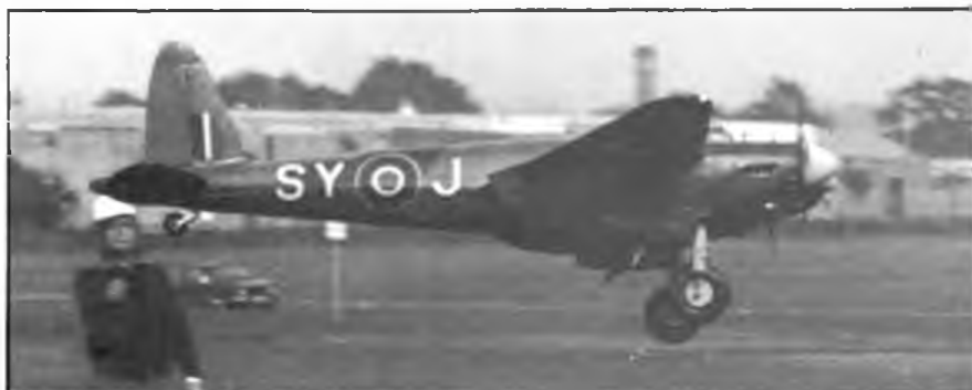
Hugh Swatton on his first flight with his DH Mosquito. Power is two OS Max 40's and the undercarriage is fixed. span 63in.
