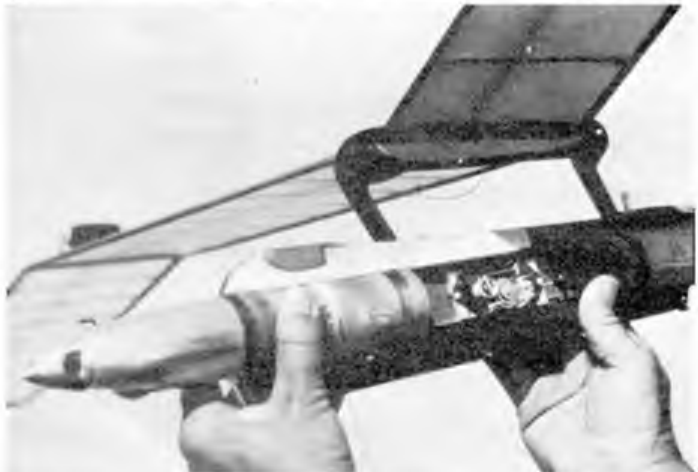
Left: gull wing breaks at dihedral intersection. Elastic band tension over carbon fibre plates opens wing.
