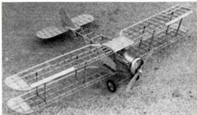
Left: beautiful construction on John Coker's Sopwith Triplane. Note the scale sprung U/C and expertly hand beaten cowl. John's tips on metalwork will appear in a later article. Above: another fine structural shot is Michael Smith's Bristol Fighter. This model is larger than average 55in. and flies very sedately. It uses all the standard techniques for a fabric covered biplane.
