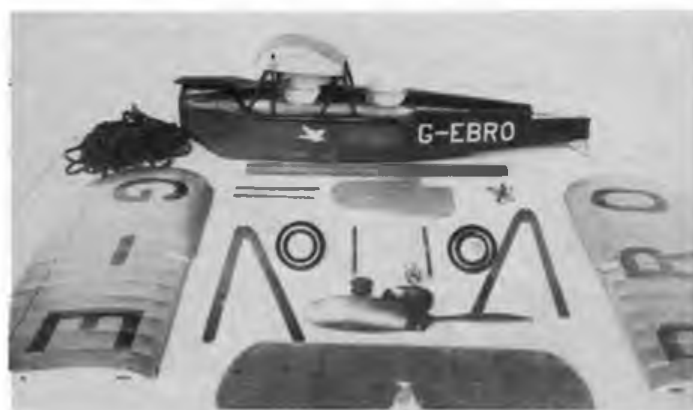
Right: parts spread of the rubber powered original Conversion details for small diesel or glow motors are now included on the plan as shown below.
