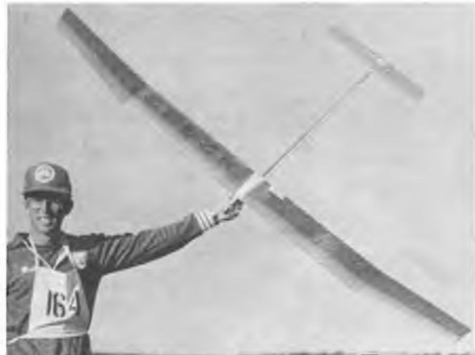
Left: Matt Gewain's winning model, 'Pacer' features much use of carbon fibre structure reinforcing in wings plus Horejsi style timer delayed auto rudder. Right: proving the strong yet smooth wind was really no problem, Holland's ace flyer Peter DeBoer often towed for 20-30 minutes, note Dutch style mini-rod winch.
