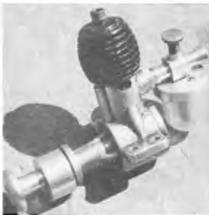
Left: a Mills .75 - actually a Doonside replica - fitted with a shaft extension. This is simply a hollow threaded bolt which fits closely into a spacing collar. Right: this Tiger was built by Charlie Newman, and has ideal proportions for free flight. A shaft extension is used to bring the motor back from the front cowling. Below: this Hawker Nimrod is by Eric Coates by an ED Super Fury. Photo C. De la Nougerede.
