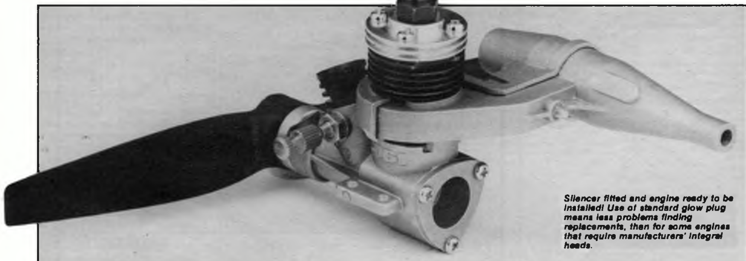
Above, seen here full size the G-Mark .061 shows generous mounting lugs and overall compact size for a 1 c.c. engine.
