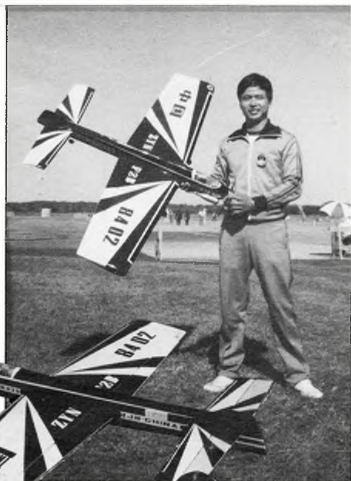
Right and below right - one man and his model. World Champion in F1B Zhu Younan from the Peoples Republic of China. Model is 55in. span uses an OS45 ABC motor with a homemade, laminated three blade propeller.
