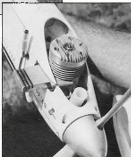
Right, powerplant and (ST 60) of Jim Casales' 'Spectrum' - model is 64 ins. span, 750 sq. ins., 50 ozs., and has foam flying surfaces covered with balsa 'veneer'.
