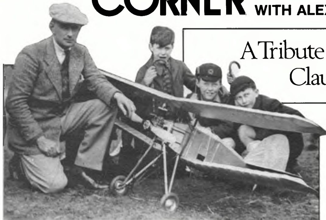
Captain C E Bowden with 'Kanga' on Wimbledon Common in 1932 with some youthful admirers. 'Kanga' in its original state with piano wire tailunit and the 28cc Wall installed upright.
