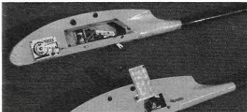
Left, two "Turning Point" front ends, note battery in the Mk IV (top) to power retrieval aid beeper, bottom - latest version with pivoted hatch revealing latest two hook - the skid protects the hook from damage on landing.
