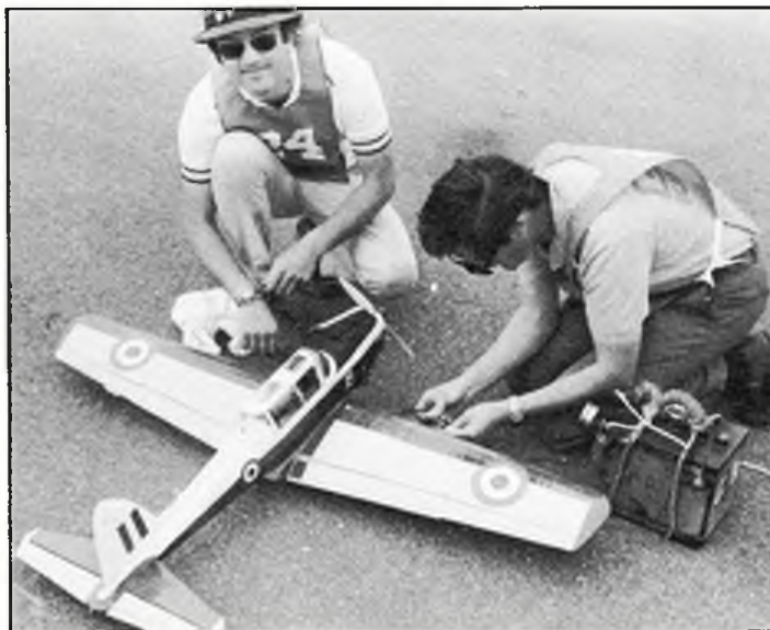
Left, Vic Wilson with D.H. Chipmunk at the Lakehurst World Champs. Model was 53in. span, powered by an OS-40 and used four line control (elevator, throttle and flaps).
