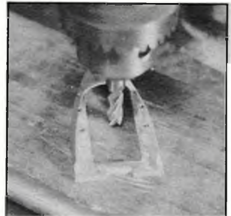
Above, removing surplus metal by moving the pan freehand against a rotating end mill with the table set at a suitable height to leave about 1/8 inch of metal in the base of the L-section.
