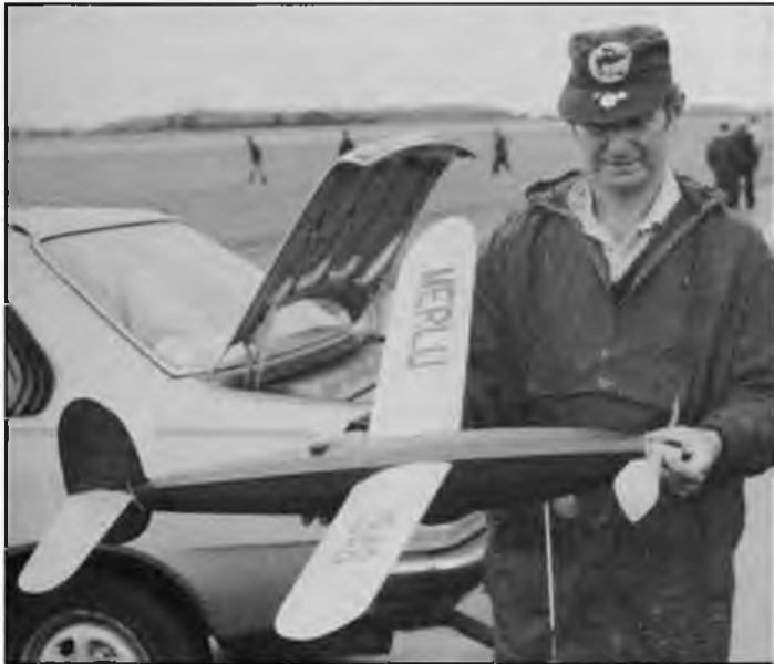
Right Bob Jones also built this 1/4 size 'Quaker Flash' powered by Davis/Cox 020 Co2 conversion using a Modela propeller. The model, which weighs 4 1/2 ounces was flown at last year's Old Warden Vintage Weekend.
