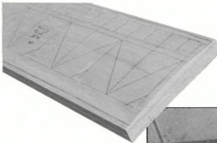
Left, one of Phil's cambered building jigs together with Mylar plan (see text). Below, an early wing jig - note the packing under the tip for washout, below this is the custom-built jig from Joe Maxwell.
