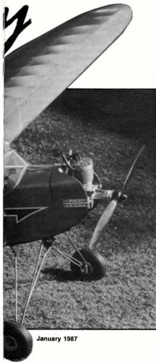
Left: Vital statistics of this beauty queen are: wingspan, seven feet and weight, five-and-a-half pounds. Above: The cowl hinges to allow easy access to motor controls. Note the glass-fibre engine bay reinforcement which also acts as fuel-proofer.
