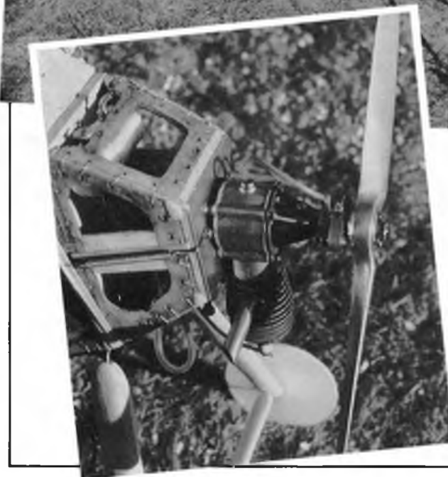
Top photo shows Blue Dragon soon after restoration began in 1985. The complete airframe is seen above, with the engine bay at left; note the 'sewn-in' plywood panels. Heading photographs on previous page show Alwyn with pristine model and (inset) Blue Dragon in original trim.
