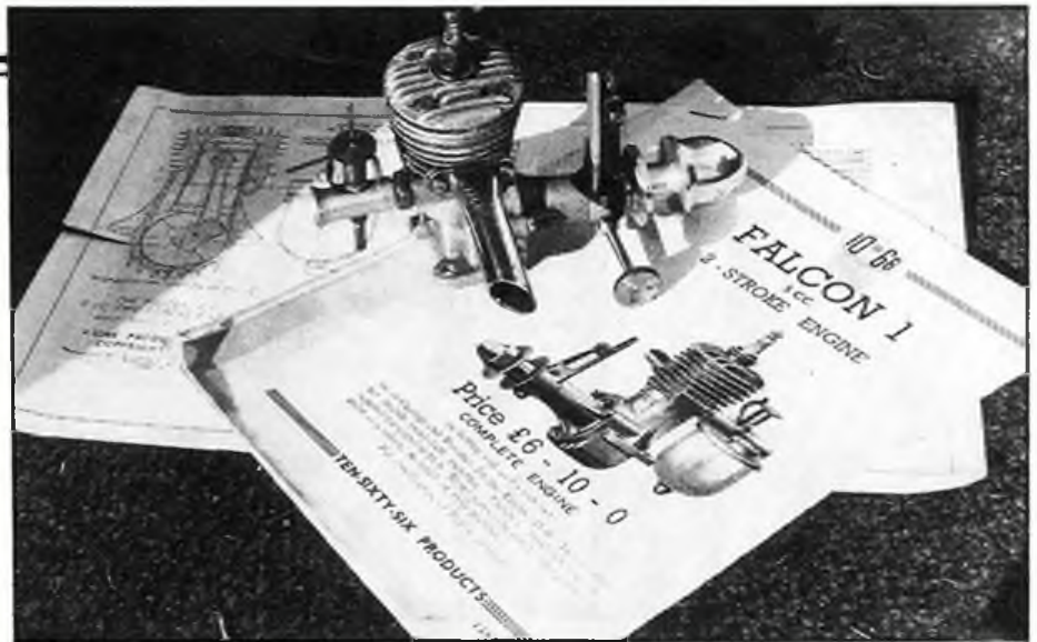
Above: Gordon J. Rae's photo shows the Falcon I 5cc petrol engine resting on some of the literature that accompanied the 1066 set of castings from which the engine was made in 1948. Left: The Stitt M80 spark plug is shown here full-size. Manufactured by Stitt Spark Plug Company, PO Box 327, Conroe, Texas 77305 USA, this 1/4in. by 32 TPI plug is available in the UK. Below: Thoughts of the M.E. Exhibition - last year's SAM 35 stand. Going in '88? See you there!
