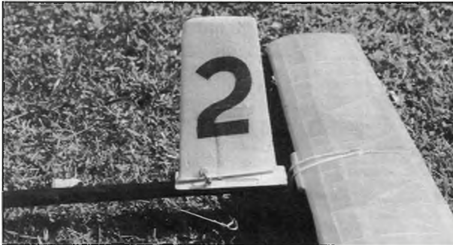
Top left: Timer details, simple towhook and nose-skid shown here. Top right: Fuselage pod with wings detached and timer linkages disconnected. Above: All-moving fin and warp-resistant tailplane are features of the Adonis. Above right: Auto-rudder linkage details. Right: Substantial fin platform allows space for adjustment screw housings. Below: All the bits ready to-go! Adonis has shown the capability to be among the winners - could this be you?
