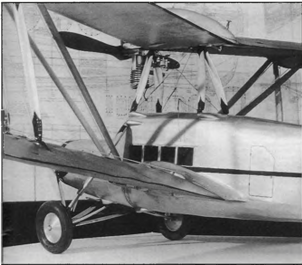
Left: Fuselage is massive. Plan detail shown below. Painted-on door is a nice touch! Note lower wing trailing-edge undulations despite its birch construction.
