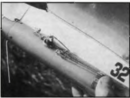
Top: Stafford Screen's F1C bunt mechanism. Below: Russian nine-minute timer used on 'No. 32' model. Note also finger grips on boom.
