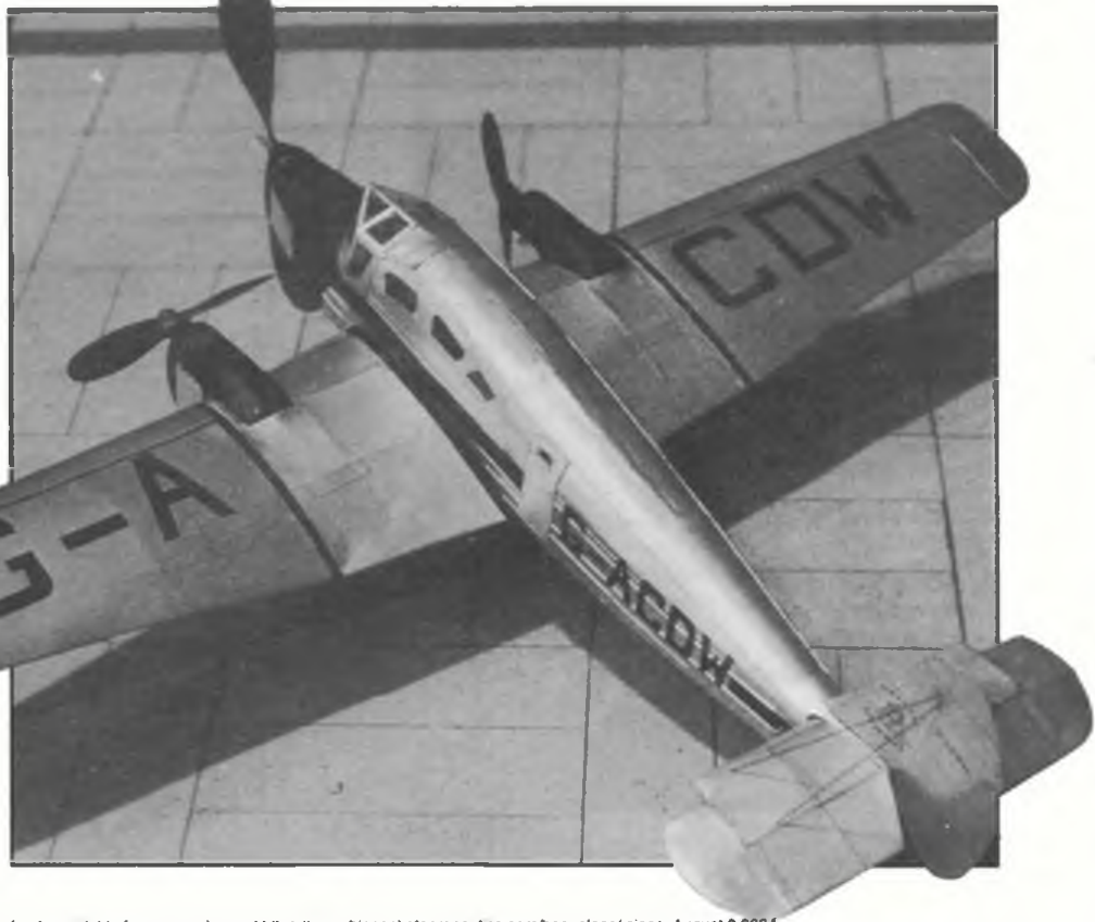
Right: Impressive Spartan Cruiser, also by Neville Coldrick, is of largely paper construction - perhaps a bit heavy?
