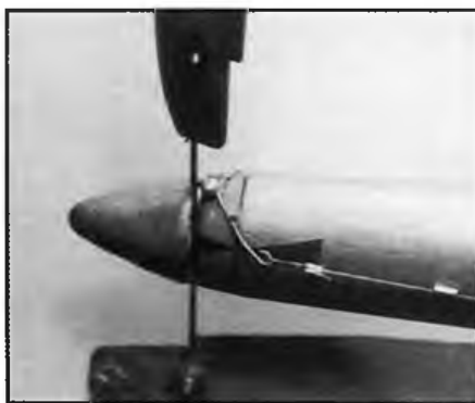
Coupe DPR arm connected up. Arm is sprung onto outrigger. Arrows aid alignment.
