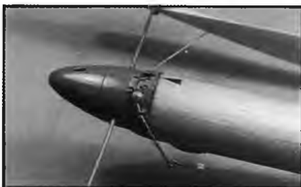
Shirring elastic holds one blade in on fold – gravity holds the other. Spinner hole is for locking pin through hub and noseblock.
