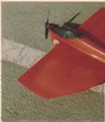
Right: Smith/Brown's winning Team Race model; Cippola power, moulded carbon-fibre fuselage. Far right: Tony Pujalte looks worried as he flushes the tank of Carlos Olive's F2A craft.
