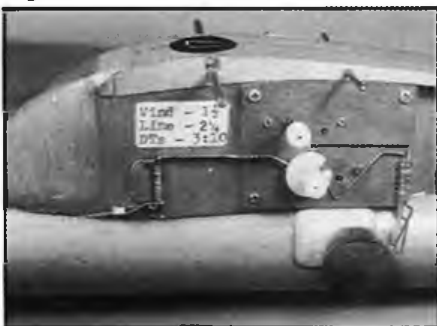
F1B timer with DPR connected. All the tension is taken by the pivot; only a light pull needed to unlatch. Note spacer to prevent hook riding up trigger arm.
