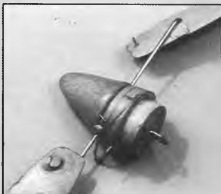
Coupe d'Hiver prop system is similar to F1B arrangement.
