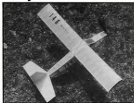
Above: Angular outlines to ease the lot of beginners are apparent in VH-146 Marissa, a simple small field cabin rubber model, one of his last published designs. Below: Rascal gliders showing auxiliary raised slats of different configurations on identical 45 degree delta wing. Models showed good stability. With CG at 40 per cent of the main wing chord, they immediately returned to a level attitude when launched in a bank.
