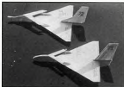
Above: Angular outlines to ease the lot of beginners are apparent in VH-146 Marissa, a simple small field cabin rubber model, one of his last published designs. Below: Rascal gliders showing auxiliary raised slats of different configurations on identical 45 degree delta wing. Models showed good stability. With CG at 40 per cent of the main wing chord, they immediately returned to a level attitude when launched in a bank.
