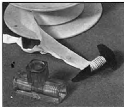
To prevent air leakage at high pressure, wrap a couple of layers of PTFE tape round needle thread.
