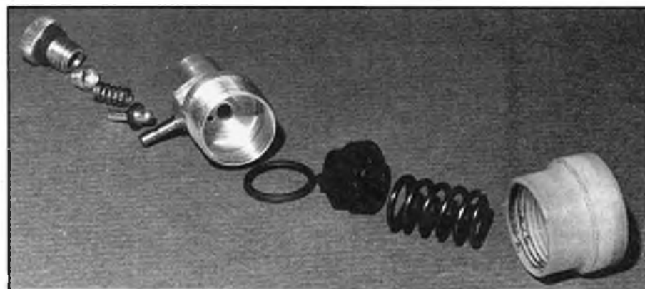
Commercial components make up the main internals of the regulator and a lighter casing reduces the all-up weight – still quite heavy though at 25 grams.
