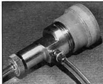
To prevent air leakage at high pressure, wrap a couple of layers of PTFE tape round needle thread.
