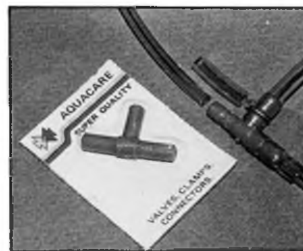
T-piece comes from pet shops, and must be grooved to take twisted soft iron wire securing bands.
