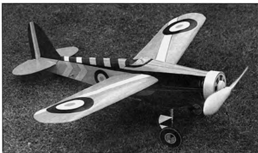
Norman Peacock's second Rigby Condor of 23 inches span flies well: all-card construction. Model weighs 3.3 ounces.
