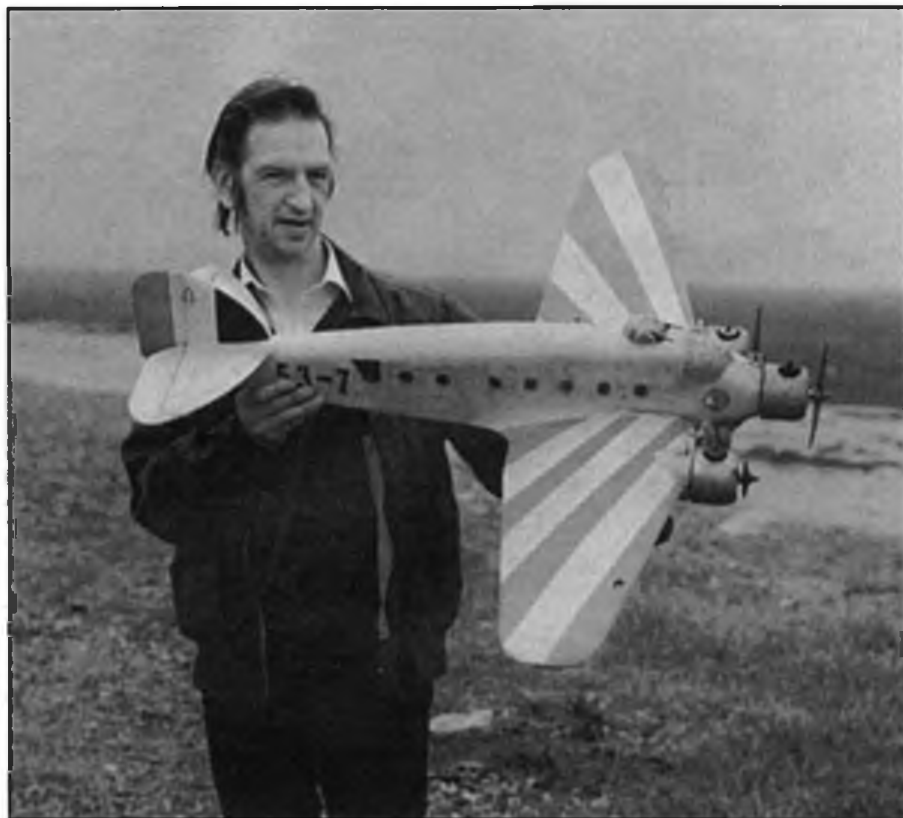
Characterful Savoia-Marchetti SM 79 is converted from the Aeromodeller F/F plan. A Frog 150 and a pair of AM 10s provide the urge.
