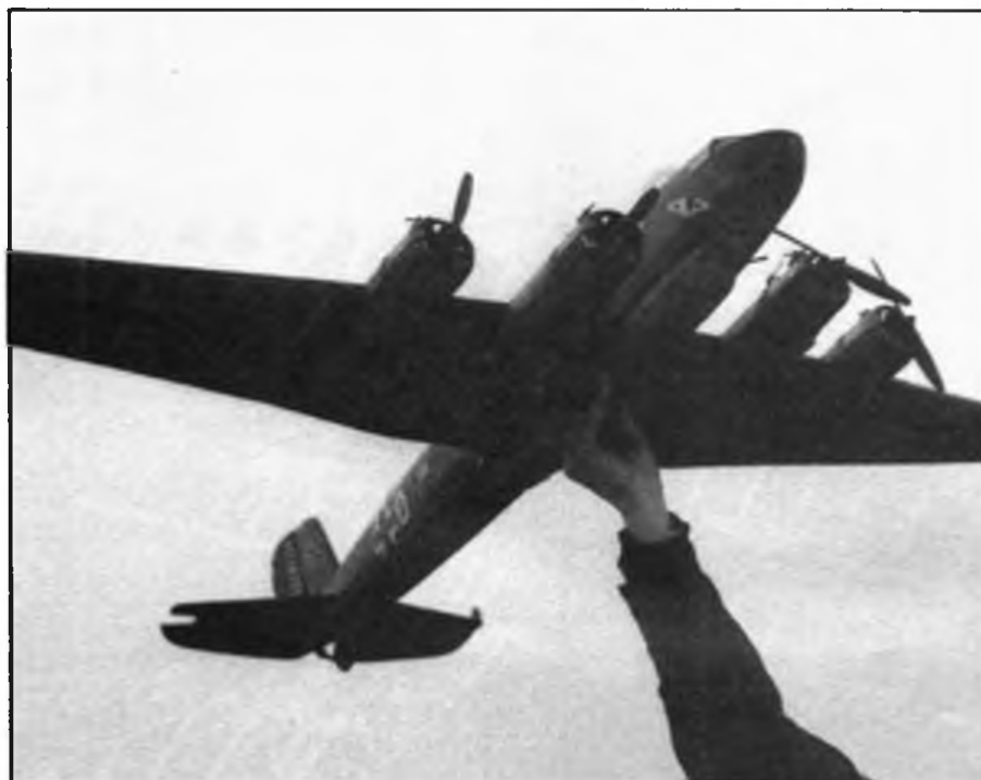
Four Frog 150 diesels power the Focke-Wulf Condor which, like the other multis discussed here, is at least ten years old and has accumulated dozens of hours of flight time.
