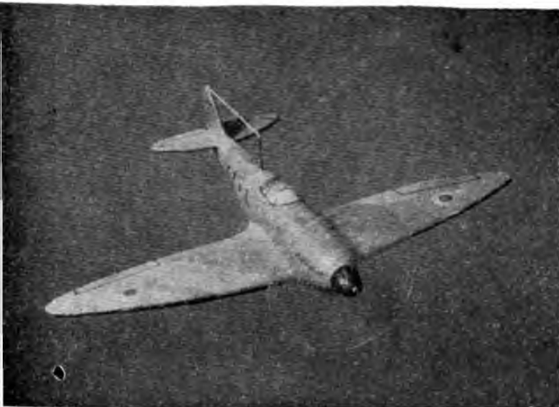
Above: D. J. A. Smith of Weybridge with his interesting and unusual model, incorporating a number of novel features. Note the treble fins, high mounted tailplane, and motor tube. The girder-type mainspar is also noteworthy.
