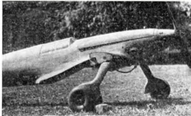
Photo No. 6. Showing undercart shock-travel.
