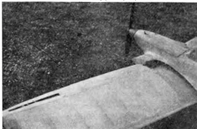
Photo No. 2. Wing partially displaced.
