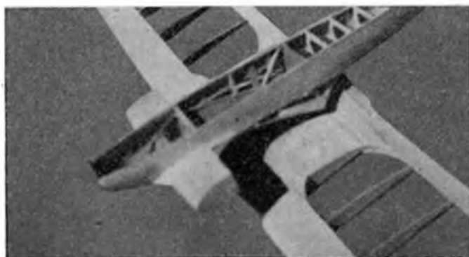
Photo No. 3. Note centre-section bulkhead.
