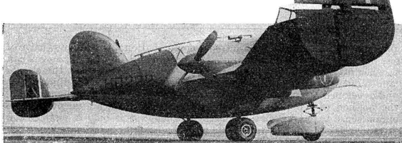
Wings to Come. Aptly named is the Handley Page Manx tailless experimental two-seater. The manufacturers have long been noted for their interest in unorthodox aircraft.
