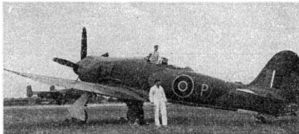
The "Aeroplane" Photo. Naval Newcomer. The prototype Hawker Sea Fury, SR 661, is a normal Fury fighter fitted with a stinger deck hook (visible just below the rudder). The land version of the Fury (a development of the Tempest II) is notably faster than its predecessor, with a top speed of 470 m.p.h. It is reported that the production Fury may revert to the Sabre in-line motor.
